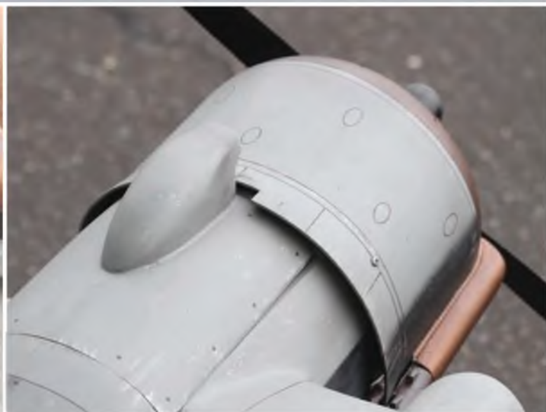
Crisp cowl detailing, with barely noticeable, but eminently practical fasteners for a twin.
