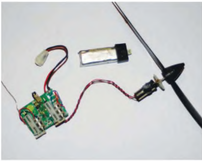
Typical of what you will salvage from a 3 channel RTF model. The receiver has two servos and a speed controller built into it and runs on a single LiPo cell.
