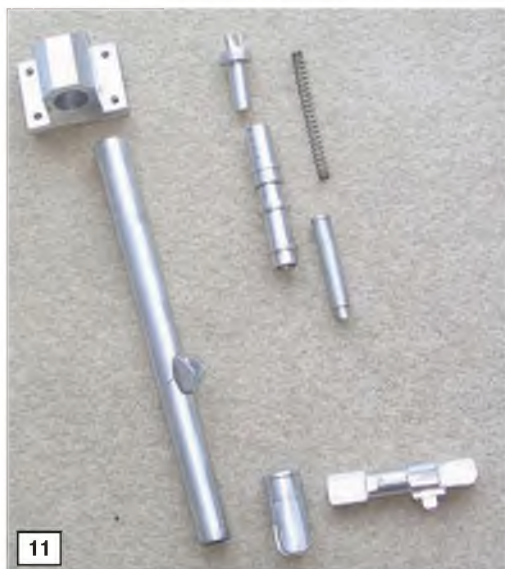
11: Components of the main undercarriage, ready for assembly. Peter Shaw acquires a lathe for this job and learned the techniques required as the work progressed. 12: In freshly turned metal, the assembled main undercarriage leg.
