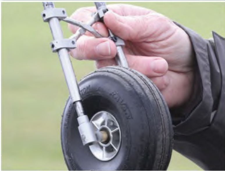
Dennis had to widen the undercarriage struts to take the 5" wheels.
