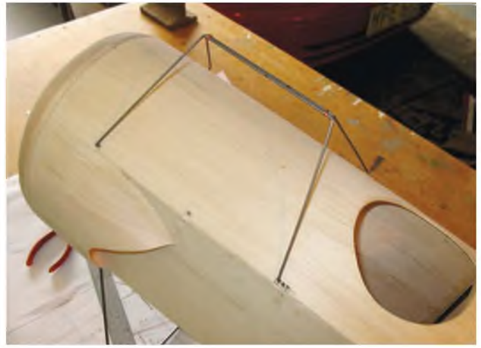
Centre section strut wires plug into tubes and are bound and soldered at the apex.
