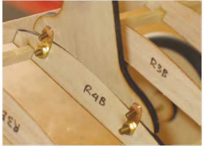
Brass strips, with soldered nuts make for a very secure inter-plane strut fixing.
