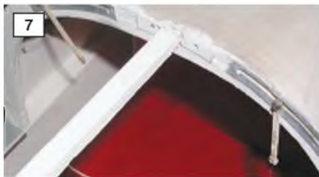
7: Detail showing the cabin door locking stays. 8: View of the fuselage underside, showing the lithoplate fuselage/wing fairings. 9: The blind nuts referred to in text, preferred by Peter Shaw to secure the main undercarriage to the wing mainspar.
