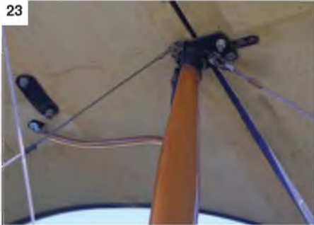
20: General view of the centre-section wing-to-fuselage struts. 21: Upper wing centre section front strut attachment bracket. 22: Lower attachment of front C/S front strut. 23: Rear C/S strut top attachment point. 24: Further view of the C/S strut attachments. 25: Lower wing root, showing the cockpit access tread plates. 26 & 27: Two views of the lower wing interplane strut attachments. 28 & 29: Propeller-driven generator mounted on front right interplane strut. 30: Pitot head on left front interplane strut. 31: General view of wing interplane struts.
