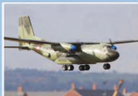
Paul Marsh's CM Pro C-160 Transall on short finals. Twin OS .25 FP glow engines.
