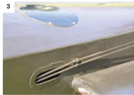
1: Centre fuselage showing fabric access panel stitching and cockpit mounting stirrups. 2 & 3: Rear fuselage showing control cable runs. 4: Engine cowl showing panel lines. 5: Hinged access panel on front fuselage side. 6: Air blower on left side cowl rear. 7: Stitching line and access panel line at rear cowl. 8: Propeller boss showing Hucks Starter socket. 9: Engine cylinder detail. 10: Draw-pin to engine cowl access panel.
