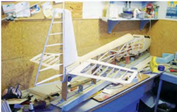
1/3rd scale Topaze under construction on purpose-made aluminium jig .
