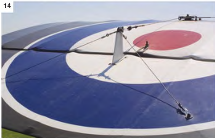
11-13: Aileron close-ups. 14 & 15: Upper wing top surface showing control horn, control cable and cable guide pulley wheel. Aileron control cables are all external to wing surfaces. 16: Inside the rear cockpit. 17: Rear cockpit windscreen. 18 & 19: Two views of the front cockpit.
