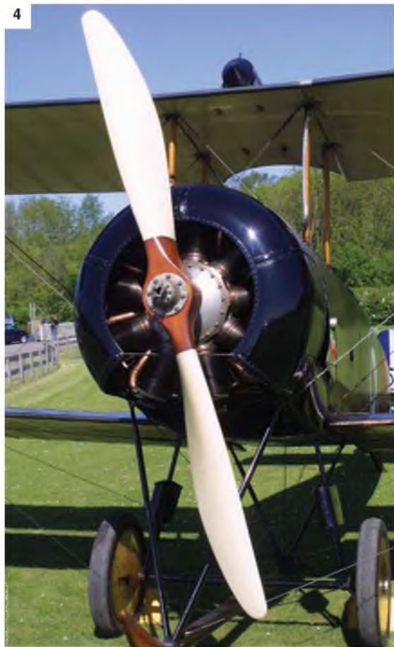
1: Centre fuselage showing fabric access panel stitching and cockpit mounting stirrups. 2 & 3: Rear fuselage showing control cable runs. 4: Engine cowl showing panel lines. 5: Hinged access panel on front fuselage side. 6: Air blower on left side cowl rear. 7: Stitching line and access panel line at rear cowl. 8: Propeller boss showing Hucks Starter socket. 9: Engine cylinder detail. 10: Draw-pin to engine cowl access panel.
