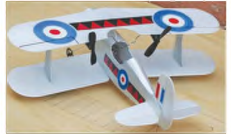
50p for some foam plus a little glue and paint and you have a rather nice home grown model for thrust steering equipment. Certainly cheap enough to experiment with.
