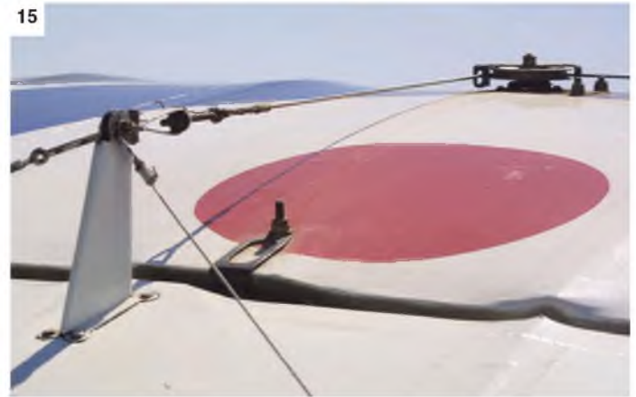
11-13: Aileron close-ups. 14 & 15: Upper wing top surface showing control horn, control cable and cable guide pulley wheel. Aileron control cables are all external to wing surfaces. 16: Inside the rear cockpit. 17: Rear cockpit windscreen. 18 & 19: Two views of the front cockpit.
