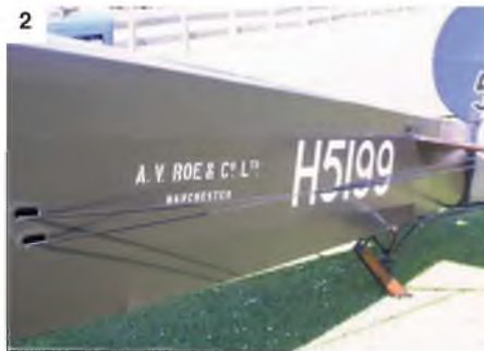
1: Centre fuselage showing fabric access panel stitching and cockpit mounting stirrups. 2 & 3: Rear fuselage showing control cable runs. 4: Engine cowl showing panel lines. 5: Hinged access panel on front fuselage side. 6: Air blower on left side cowl rear. 7: Stitching line and access panel line at rear cowl. 8: Propeller boss showing Hucks Starter socket. 9: Engine cylinder detail. 10: Draw-pin to engine cowl access panel.
