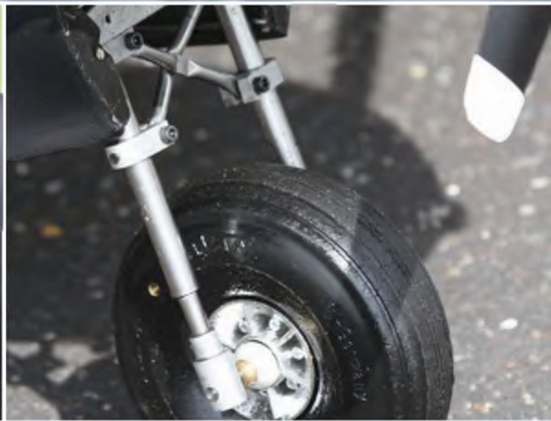
Dennis relocated and altered his Sturmovik undercarriage. Century retracts used.
