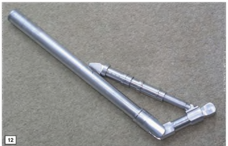
11: Components of the main undercarriage, ready for assembly. Peter Shaw acquires a lathe for this job and learned the techniques required as the work progressed. 12: In freshly turned metal, the assembled main undercarriage leg.
