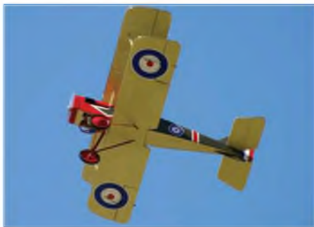
At 65cm/ 26" span Ken's little WWI biplane flies well on 1300x3S LiPos.
