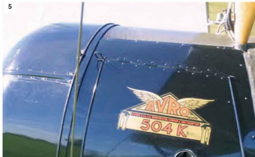
1: Centre fuselage showing fabric access panel stitching and cockpit mounting stirrups. 2 & 3: Rear fuselage showing control cable runs. 4: Engine cowl showing panel lines. 5: Hinged access panel on front fuselage side. 6: Air blower on left side cowl rear. 7: Stitching line and access panel line at rear cowl. 8: Propeller boss showing Hucks Starter socket. 9: Engine cylinder detail. 10: Draw-pin to engine cowl access panel.
