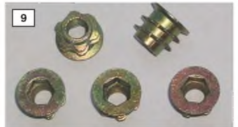
7: Detail showing the cabin door locking stays. 8: View of the fuselage underside, showing the lithoplate fuselage/wing fairings. 9: The blind nuts referred to in text, preferred by Peter Shaw to secure the main undercarriage to the wing mainspar.
