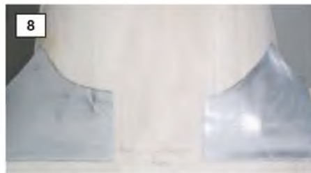
7: Detail showing the cabin door locking stays. 8: View of the fuselage underside, showing the lithoplate fuselage/wing fairings. 9: The blind nuts referred to in text, preferred by Peter Shaw to secure the main undercarriage to the wing mainspar.
