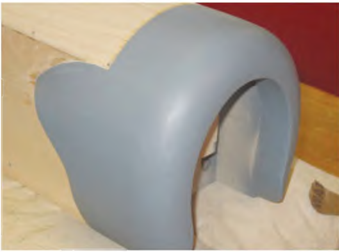
The laminated parts in place, shaped, glassed and sprayed with primer. Pat opted for glassing to add strength and weight where weight is needed.
