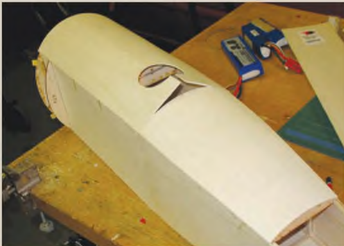
The bulk of the cowl is built as part of the fuselage with the front section added from laminated balsa parts.
