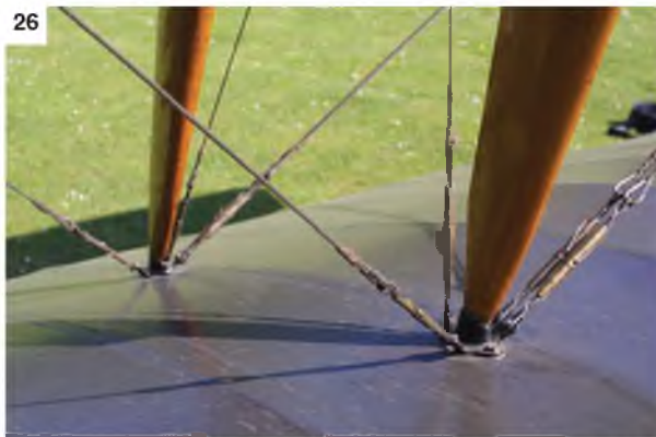
20: General view of the centre-section wing-to-fuselage struts. 21: Upper wing centre section front strut attachment bracket. 22: Lower attachment of front C/S front strut. 23: Rear C/S strut top attachment point. 24: Further view of the C/S strut attachments. 25: Lower wing root, showing the cockpit access tread plates. 26 & 27: Two views of the lower wing interplane strut attachments. 28 & 29: Propeller-driven generator mounted on front right interplane strut. 30: Pitot head on left front interplane strut. 31: General view of wing interplane struts.
