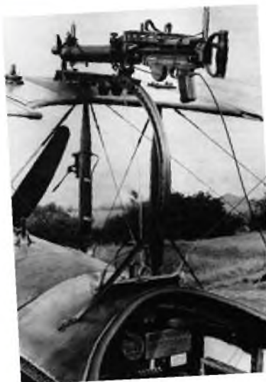
ABOVE: Lewis Gun in Foster mount installed above the upper wing of one of the single-seat Avro 504K aircraft employed by one of the Home Defense Squadrons during 1917 to combat Zeppelin airships, at that time engaged in bombing raids of Britain.
