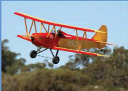
The scratch-built Fly Baby flies a treat on a petrol DLE 55.
