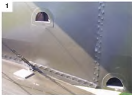
1: Centre fuselage showing fabric access panel stitching and cockpit mounting stirrups. 2 & 3: Rear fuselage showing control cable runs. 4: Engine cowl showing panel lines. 5: Hinged access panel on front fuselage side. 6: Air blower on left side cowl rear. 7: Stitching line and access panel line at rear cowl. 8: Propeller boss showing Hucks Starter socket. 9: Engine cylinder detail. 10: Draw-pin to engine cowl access panel.
