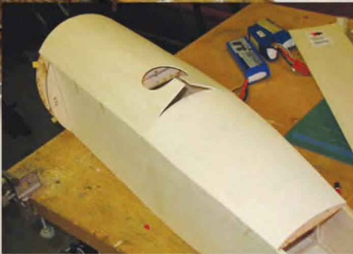
An undersize cockpit cut-out, combined with a slit in the balsa aids getting a good fit in this area.
