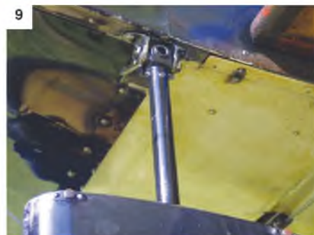
1-6: One of the most prominent features of the Avro 504K is the anti-noseover skid mounted on the main undercarriage. 7: Avro logo on the wheel axle bearing. 8: Main undercarriage shock absorber. 9: Upper main undercarriage strut anchor point. 10 & 11: Rear main undercarriage strut anchor points. 12 & 13: Mainwheel inside face and axle. 14: Mailwheel viewed from the outer face. 15: Mainwheel viewed directly from the rear illustrates the profile.
