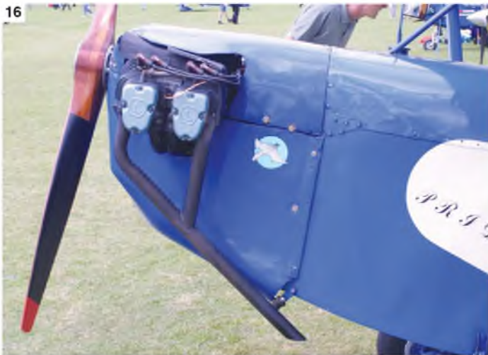
14 & 15: Two views of the Lycoming Flat Four engine. 16: Simple engine cowl and exhaust stack. 17: One side of the engine, viewed from underneath. 18: Upper wing strut anchor point and cables. 19: Faired main undercarriage leg. 20 & 21: Lower and upper aileron control horn and control cable links. 22: Pitot head, right hand wing. 23: Rudder horn and control cable. 24: General view of the tailcone. 25: Fin/rudder hinge line. 26: Simple tailwheel unit. 27: Another view of the main undercarriage anchor point on the lower furlage, also showing the lower wing strut attachment.
