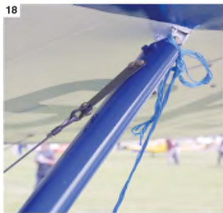
14 & 15: Two views of the Lycoming Flat Four engine. 16: Simple engine cowl and exhaust stack. 17: One side of the engine, viewed from underneath. 18: Upper wing strut anchor point and cables. 19: Faired main undercarriage leg. 20 & 21: Lower and upper aileron control horn and control cable links. 22: Pitot head, right hand wing. 23: Rudder horn and control cable. 24: General view of the tailcone. 25: Fin/rudder hinge line. 26: Simple tailwheel unit. 27: Another view of the main undercarriage anchor point on the lower furlage, also showing the lower wing strut attachment.
