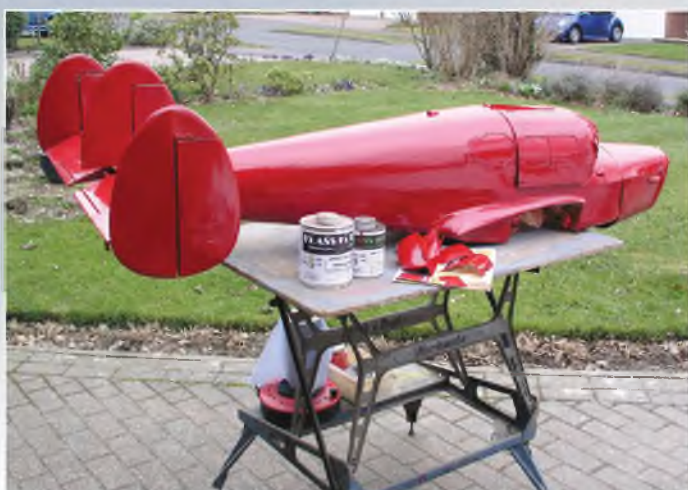
The fuselage masked up and the first coat applied - a slow cure means a lot of rubbing down will be necessary, before the final coat.
