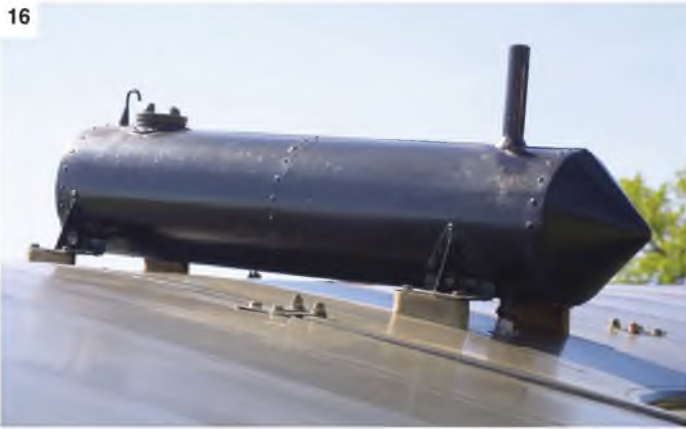
16 & 17: Two views of the fuel tank above the upper wing. 18: & 19: The heavily braced tailskid. 20 & 21: Two views of the elevator control runs, showing the guides on the tailplane leading edge. 22: Elevator control horn and duplicated control cables. 23: Tailplane underside, showing the strut braces. 24: Another detail of the elevator control cable, showing the threaded adjusters. 25: Wing tip protector hoop mounted on the lower underside wing tip.
