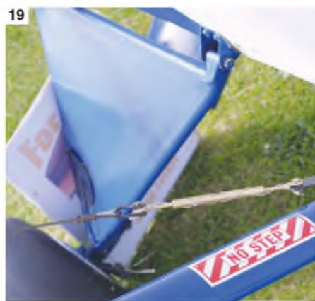
14 & 15: Two views of the Lycoming Flat Four engine. 16: Simple engine cowl and exhaust stack. 17: One side of the engine, viewed from underneath. 18: Upper wing strut anchor point and cables. 19: Faired main undercarriage leg. 20 & 21: Lower and upper aileron control horn and control cable links. 22: Pitot head, right hand wing. 23: Rudder horn and control cable. 24: General view of the tailcone. 25: Fin/rudder hinge line. 26: Simple tailwheel unit. 27: Another view of the main undercarriage anchor point on the lower furlage, also showing the lower wing strut attachment.
