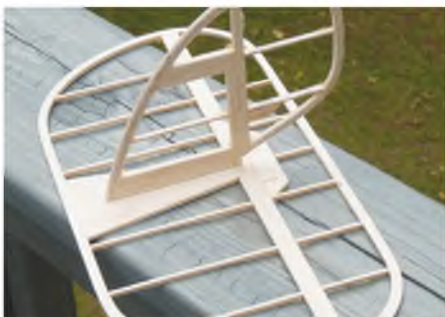
Laminated outlines impart great strength but without adding the weight of more heavily built, cut sheet outlines.
