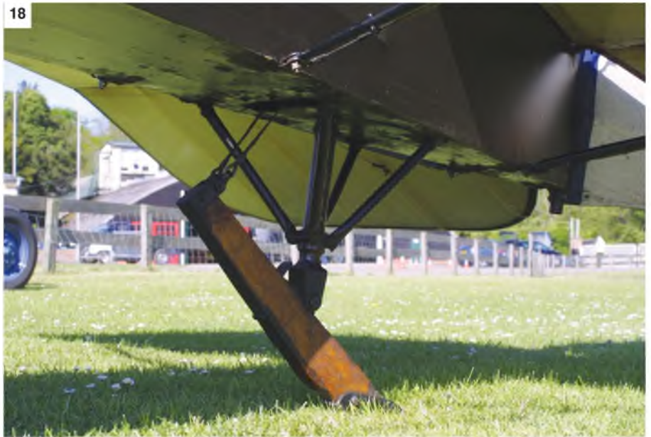
16 & 17: Two views of the fuel tank above the upper wing. 18: & 19: The heavily braced tailskid. 20 & 21: Two views of the elevator control runs, showing the guides on the tailplane leading edge. 22: Elevator control horn and duplicated control cables. 23: Tailplane underside, showing the strut braces. 24: Another detail of the elevator control cable, showing the threaded adjusters. 25: Wing tip protector hoop mounted on the lower underside wing tip.
