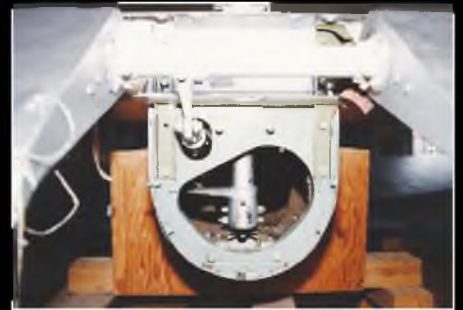
View of the full-size rudder and elevator linkages.
