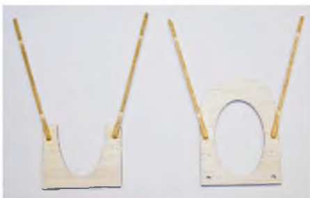
Bass struts glued into formers is a good way of eliminating the need for wire and are adequately strong on the tiddlers we are talking about.
