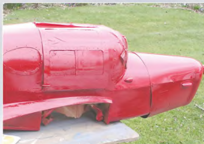
All the glazing in place and carefully masked up - time spent applying adequate masking is crucial to the final finish.
