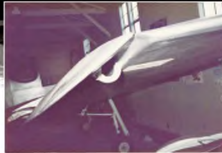
Shot of one of the aileron hinges.
