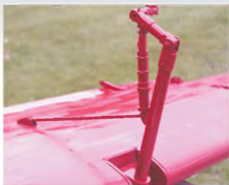
Detail of the U/C leg that Peter turned on his lathe as detailed last month - compare to the full-size shot shown on following pages.
