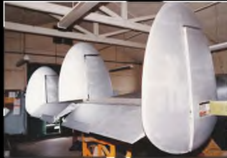
Full-size tail fins showing access panels and elevator trim tab detail.
