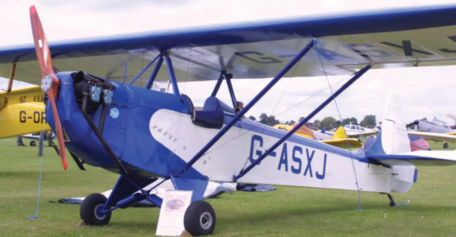
G-ASXJ seen here and at right, is a classic example of the variations that comebuilders have applied to the basic Luton Minor design. Photographed at the PFA Rally, Cranfield, in September 2003, this example is powered by a 55 hp Lycoming O-145-A2 flat-four engine.
