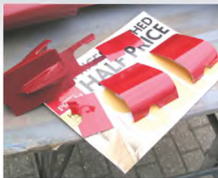
Panels and tail fairing are painted separate to the main model airframe assemblies.
