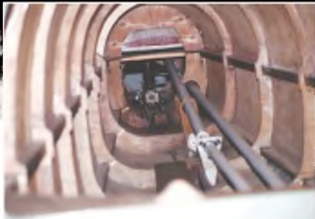
View inside the full-size fuselage showing the ply formers and skin panels.
