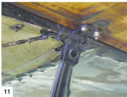
1-6: One of the most prominent features of the Avro 504K is the anti-noseover skid mounted on the main undercarriage. 7: Avro logo on the wheel axle bearing. 8: Main undercarriage shock absorber. 9: Upper main undercarriage strut anchor point. 10 & 11: Rear main undercarriage strut anchor points. 12 & 13: Mainwheel inside face and axle. 14: Mailwheel viewed from the outer face. 15: Mainwheel viewed directly from the rear illustrates the profile.
