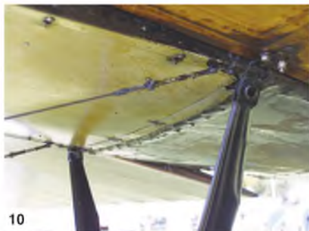
1-6: One of the most prominent features of the Avro 504K is the anti-noseover skid mounted on the main undercarriage. 7: Avro logo on the wheel axle bearing. 8: Main undercarriage shock absorber. 9: Upper main undercarriage strut anchor point. 10 & 11: Rear main undercarriage strut anchor points. 12 & 13: Mainwheel inside face and axle. 14: Mailwheel viewed from the outer face. 15: Mainwheel viewed directly from the rear illustrates the profile.
