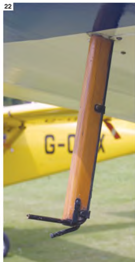
14 & 15: Two views of the Lycoming Flat Four engine. 16: Simple engine cowl and exhaust stack. 17: One side of the engine, viewed from underneath. 18: Upper wing strut anchor point and cables. 19: Faired main undercarriage leg. 20 & 21: Lower and upper aileron control horn and control cable links. 22: Pitot head, right hand wing. 23: Rudder horn and control cable. 24: General view of the tailcone. 25: Fin/rudder hinge line. 26: Simple tailwheel unit. 27: Another view of the main undercarriage anchor point on the lower furlage, also showing the lower wing strut attachment.
