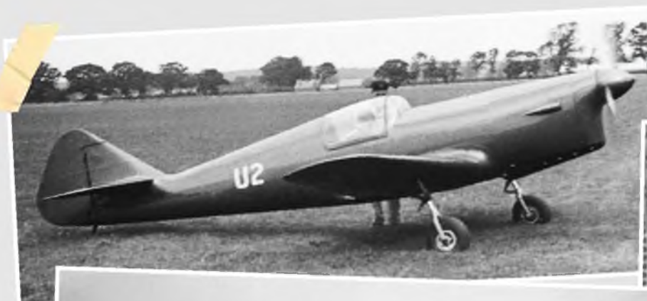
LEFT: Engine running up ready for air test, without the main undercarriage covers.
