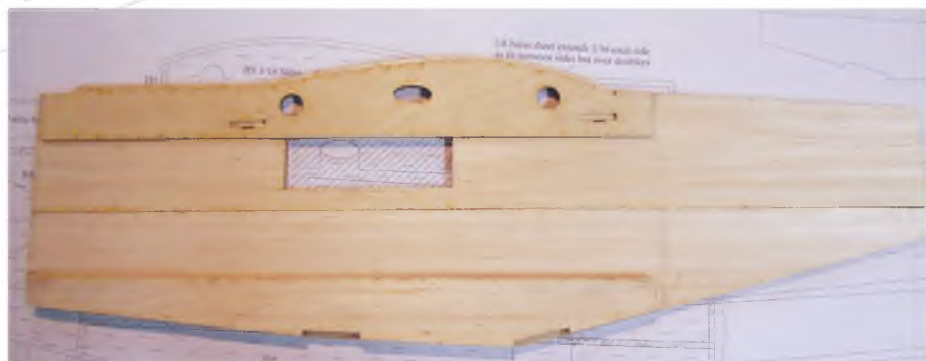
Front fuselage sides joined, doublers fitted and the position of the score line marked before the real building starts.
