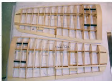
At 13" chord, these are not small wings. Lots of area to carry the model though, despite the taper.
