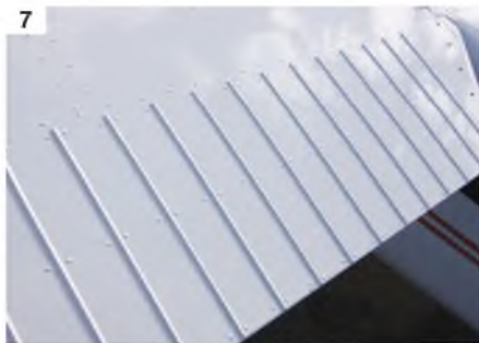
7: The corrugations on the control surface have been faithfully reproduced. 8: This over wing shot gives some idea of the sheer accuracy of the model. 9: The Luscombe has scale control horns and cable runs. 10: Keith and Doug have put an amazing effort into surface finish. 11: Elegant fin and rudder treatment, with retrained, but effective, flashes of colour. 12: Trademark Silvaire spats faithfully reproduced, complete with Silvaire logo. 13: Working lights, upgraded in power since this photo.
