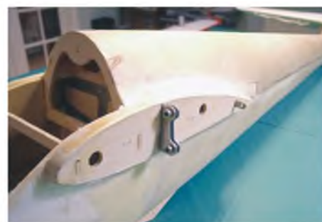
Rigid mounting on Geoff Crew's CNC Modellbau Minimoa.
