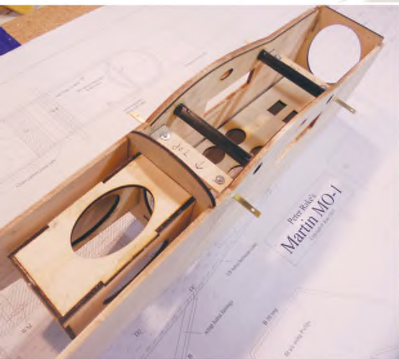
The basic front fuselage section showing the substantial motor mount, radio/battery tray, joiner tubes and brass wing retaining straps.
