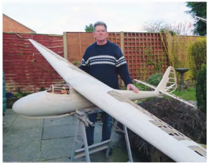
Author with completed Rhonadler airframe, ready for covering.
