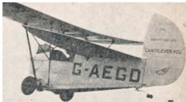
Another example, 'The Cantilever Pou' in which the struts were replaced with bracing wires and unbraced rear wing.
