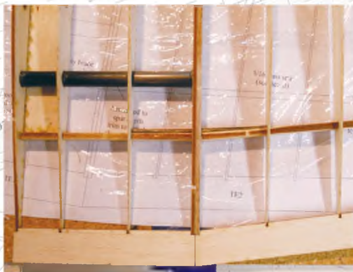
Lower the spar over the plan to build the main section of the wing, using the wedges and ply brace to join the rear spar.
