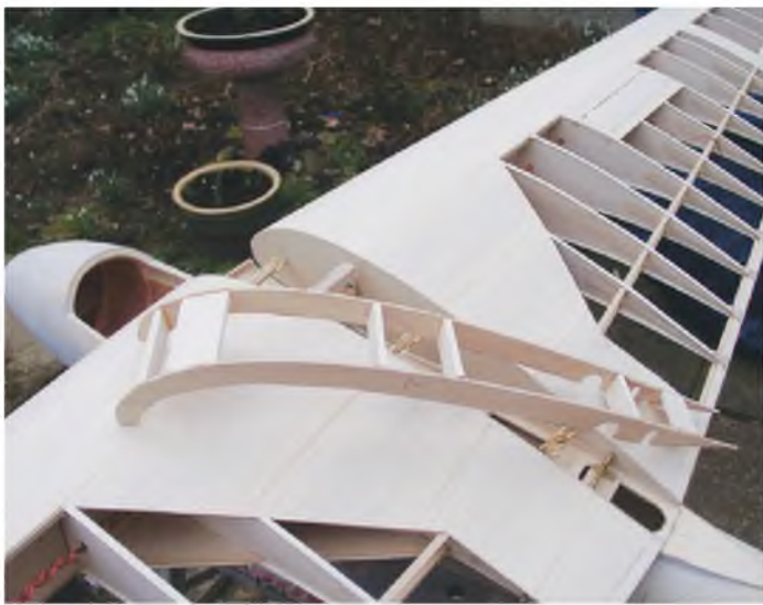
Making up the wing centre-section fairing.
