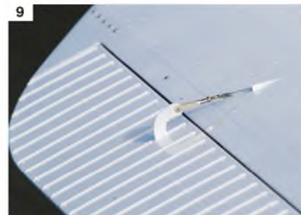
7: The corrugations on the control surface have been faithfully reproduced. 8: This over wing shot gives some idea of the sheer accuracy of the model. 9: The Luscombe has scale control horns and cable runs. 10: Keith and Doug have put an amazing effort into surface finish. 11: Elegant fin and rudder treatment, with retrained, but effective, flashes of colour. 12: Trademark Silvaire spats faithfully reproduced, complete with Silvaire logo. 13: Working lights, upgraded in power since this photo.
