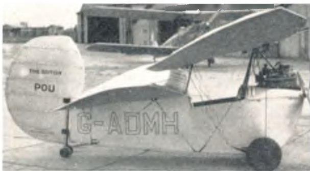
The 'Appleby Pou' with Carden Ford 28 h.p. engine, announced 'Ready to Fly Away' for £198, from Heston airfield, west London in October 1935.
