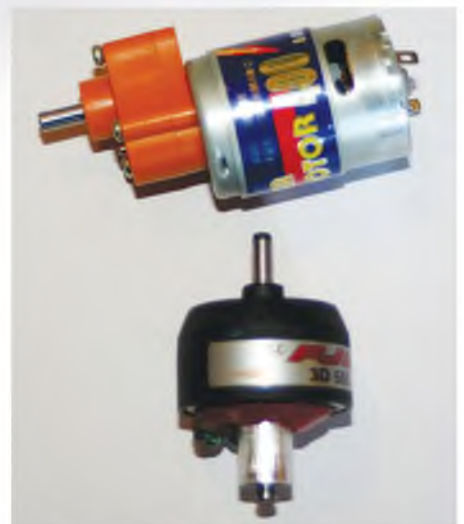
A geared 400 like this would suit something like the Moska nicely. Not much different in size, the brushless motor is much more powerful.
