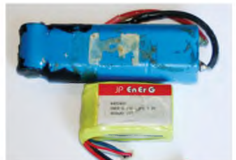
A Ni-Cad pack (7 cells, 8.4 volts and 600 mAh) next to a 2S (7.4 volts and 800 mAh) which would power the same model at much less weight penalty.
