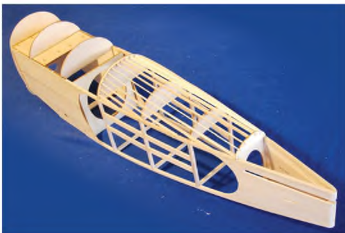
Even more complex fuselages use the same basic structure beneath all the more curvaceous parts.
