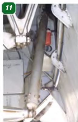
6: Exhaust outlet, lower side of engine cowl. 7: Exhaust stub positioned between the cowl rear and the main undercarriage door. 8: Adjustable exhaust outlet just in front of the main undercarriage bay. 9: Engine cowl front ring. Note air scoops top and bottom. 10, 11 & 12: Inside the main undercarriage bay, showing the door hinges. 13: Exhaust gills, viewed from front. 14: Propeller spinner and prop. blade cuffs. 15 & 16: Rear fairing of the engine nacelles. 17: Air scoop in front ring of engine cowl.
