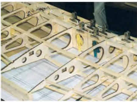
Joining the wing panels.
