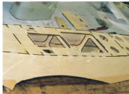
Basic assembled fuselage, note the laser cut edges.
