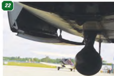
18: Front firewall of the left engine nacelle and main undercarriage door. Note the fixed stay that links the lower hinged undercarriage door to the firewall. 19: Close-up of stay attachment. 20, 21 & 22: Lower hinge line of the two-part main undercarriage door. 23: Upper hinge line of the main undercarriage door. 24: Rudder hinge line. 25 & 26: Detail of the rear gun turret. 27: Fin and rudder hinge line.
