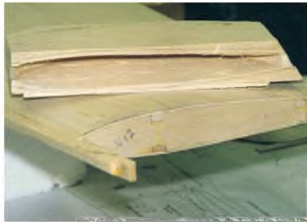
The block wing tip hollowed out and ready for fitting.
