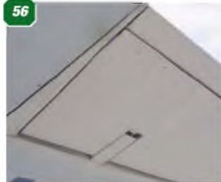
52-55: Main undercarriage leg and wheel. 56: Hinge line of the aileron. 57: Close-up of an aileron hinge. 58: Navigation light and hatch. 59: Landing light in right wing leading edge. 60: Wing-to-engine nacelle fairing fillet.
