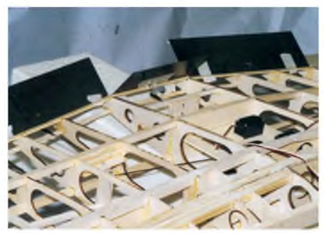
Fitting the flap mechanism. Inset - the bellcrank and bracket.
