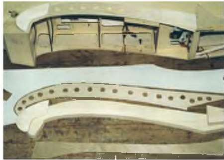
Building the wing fillet (note the styrene sheet fuselage protector).
