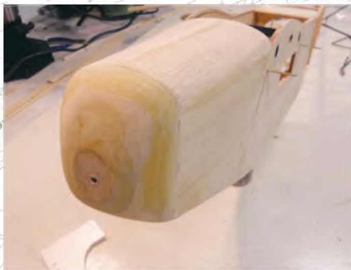
Decking in place and templates used to assist with shaping the nose block. It's definitely starting to look like a Martin MO-1.
