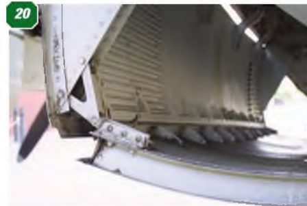
18: Front firewall of the left engine nacelle and main undercarriage door. Note the fixed stay that links the lower hinged undercarriage door to the firewall. 19: Close-up of stay attachment. 20, 21 & 22: Lower hinge line of the two-part main undercarriage door. 23: Upper hinge line of the main undercarriage door. 24: Rudder hinge line. 25 & 26: Detail of the rear gun turret. 27: Fin and rudder hinge line.
