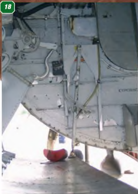
18: Front firewall of the left engine nacelle and main undercarriage door. Note the fixed stay that links the lower hinged undercarriage door to the firewall. 19: Close-up of stay attachment. 20, 21 & 22: Lower hinge line of the two-part main undercarriage door. 23: Upper hinge line of the main undercarriage door. 24: Rudder hinge line. 25 & 26: Detail of the rear gun turret. 27: Fin and rudder hinge line.
