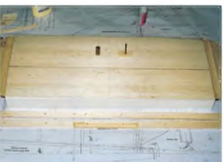
Foam covered tailplane and elevator, the two spars are pre-drilled for the hinges.
