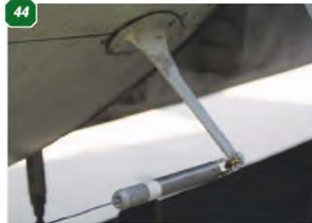
40: Blister fairing, bottom of fuselage behind nose undercarriage position. 41: Window, lower rear fuselage left side. 42: Tail bumper on fuselage underside below fin/rudder position. 43: Window in fuselage rear lower right side. 44 & 45: Two masts supporting radio aerial, lower rear fuselage. 46: Ventral hatch in fuselage rear underside. 47: Top of undercarriage noseleg. 48: Inside the nosewheel bay, showing the hinged undercarriage door. 49-51: Three views of the undercarriage noseleg and wheel.
