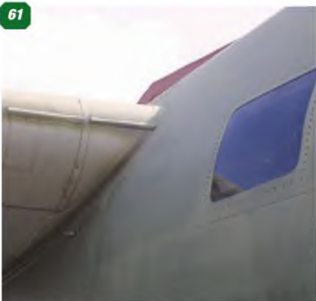
61: Window, right fuselage side, just ahead of the wing leading edge. Note the two spoiler strips on wing leading edge. 62: Landing light, left wing leading edge. 63: Pitot head, left wing tip leading edge. 64: Navigation light wing underside. 65: Wing-to-fuselage fairing fillet. 66: Pitot head on right wing tip leading edge.
