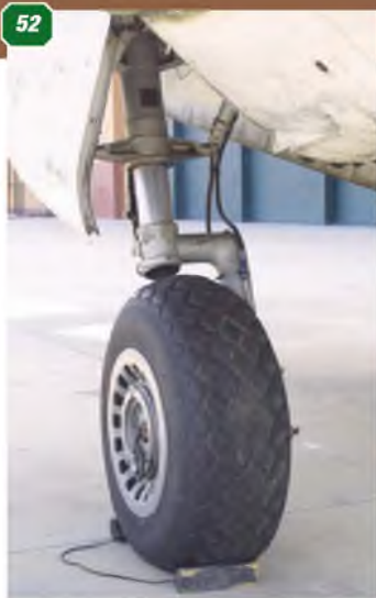
52-55: Main undercarriage leg and wheel. 56: Hinge line of the aileron. 57: Close-up of an aileron hinge. 58: Navigation light and hatch. 59: Landing light in right wing leading edge. 60: Wing-to-engine nacelle fairing fillet.
