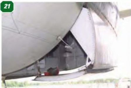
18: Front firewall of the left engine nacelle and main undercarriage door. Note the fixed stay that links the lower hinged undercarriage door to the firewall. 19: Close-up of stay attachment. 20, 21 & 22: Lower hinge line of the two-part main undercarriage door. 23: Upper hinge line of the main undercarriage door. 24: Rudder hinge line. 25 & 26: Detail of the rear gun turret. 27: Fin and rudder hinge line.
