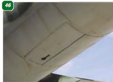
40: Blister fairing, bottom of fuselage behind nose undercarriage position. 41: Window, lower rear fuselage left side. 42: Tail bumper on fuselage underside below fin/rudder position. 43: Window in fuselage rear lower right side. 44 & 45: Two masts supporting radio aerial, lower rear fuselage. 46: Ventral hatch in fuselage rear underside. 47: Top of undercarriage noseleg. 48: Inside the nosewheel bay, showing the hinged undercarriage door. 49-51: Three views of the undercarriage noseleg and wheel.
