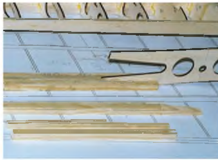
Showing how wing joiner fits into undercarriage spar.
