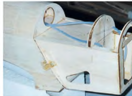
Fuselage cowling framework in position.
