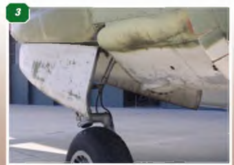
1 & 2: Engines Nacelles viewed from lower rear. 3: Another view of the engine nacelle viewed from front, showing main undercarriage door. 4: The complete right hand engine nacelle. The engine is tightly cowled. 5: The same nacelle viewed from the rear.
