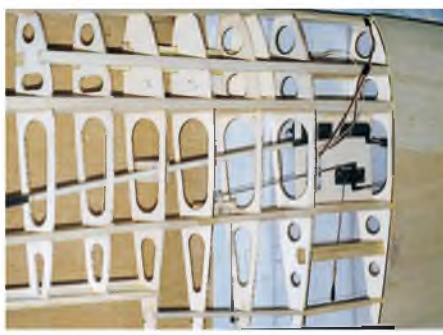
Fitting servos, rods and horns prior to skimming wing.
