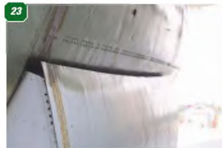
18: Front firewall of the left engine nacelle and main undercarriage door. Note the fixed stay that links the lower hinged undercarriage door to the firewall. 19: Close-up of stay attachment. 20, 21 & 22: Lower hinge line of the two-part main undercarriage door. 23: Upper hinge line of the main undercarriage door. 24: Rudder hinge line. 25 & 26: Detail of the rear gun turret. 27: Fin and rudder hinge line.
