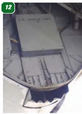
6: Exhaust outlet, lower side of engine cowl. 7: Exhaust stub positioned between the cowl rear and the main undercarriage door. 8: Adjustable exhaust outlet just in front of the main undercarriage bay. 9: Engine cowl front ring. Note air scoops top and bottom. 10, 11 & 12: Inside the main undercarriage bay, showing the door hinges. 13: Exhaust gills, viewed from front. 14: Propeller spinner and prop. blade cuffs. 15 & 16: Rear fairing of the engine nacelles. 17: Air scoop in front ring of engine cowl.
