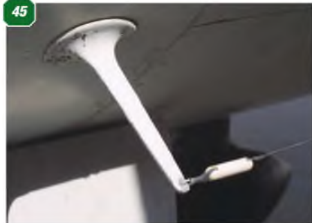
40: Blister fairing, bottom of fuselage behind nose undercarriage position. 41: Window, lower rear fuselage left side. 42: Tail bumper on fuselage underside below fin/rudder position. 43: Window in fuselage rear lower right side. 44 & 45: Two masts supporting radio aerial, lower rear fuselage. 46: Ventral hatch in fuselage rear underside. 47: Top of undercarriage noseleg. 48: Inside the nosewheel bay, showing the hinged undercarriage door. 49-51: Three views of the undercarriage noseleg and wheel.
