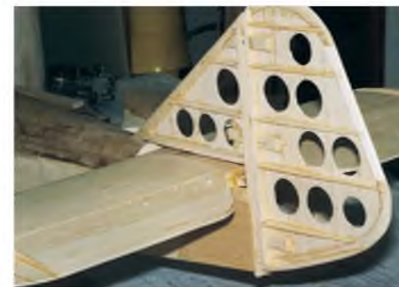
Trial fitting of the tail surfaces to facilitate the control linkages and fittings.
