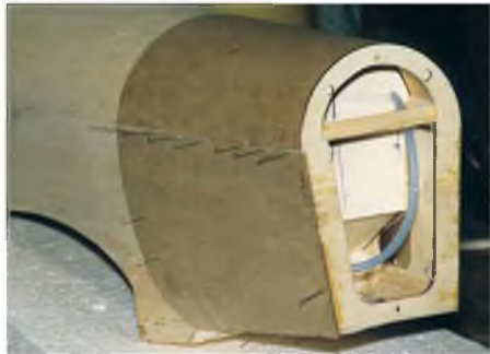
Plywood sheeted cowling, 0.4mm to sides, 0.4mm on top.
