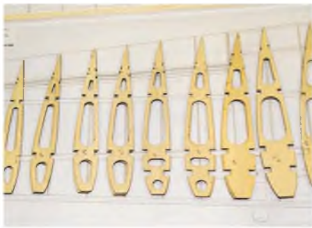
Laser cut wing ribs are more accurate and make construction easier.
