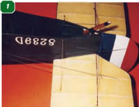
FIG.1: Dacalage (zero tail)
