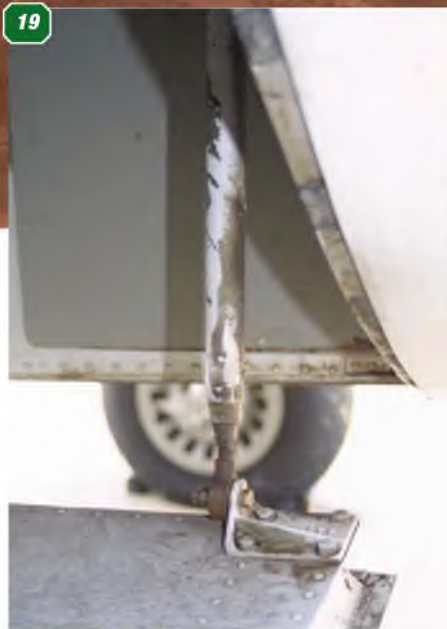
18: Front firewall of the left engine nacelle and main undercarriage door. Note the fixed stay that links the lower hinged undercarriage door to the firewall. 19: Close-up of stay attachment. 20, 21 & 22: Lower hinge line of the two-part main undercarriage door. 23: Upper hinge line of the main undercarriage door. 24: Rudder hinge line. 25 & 26: Detail of the rear gun turret. 27: Fin and rudder hinge line.
