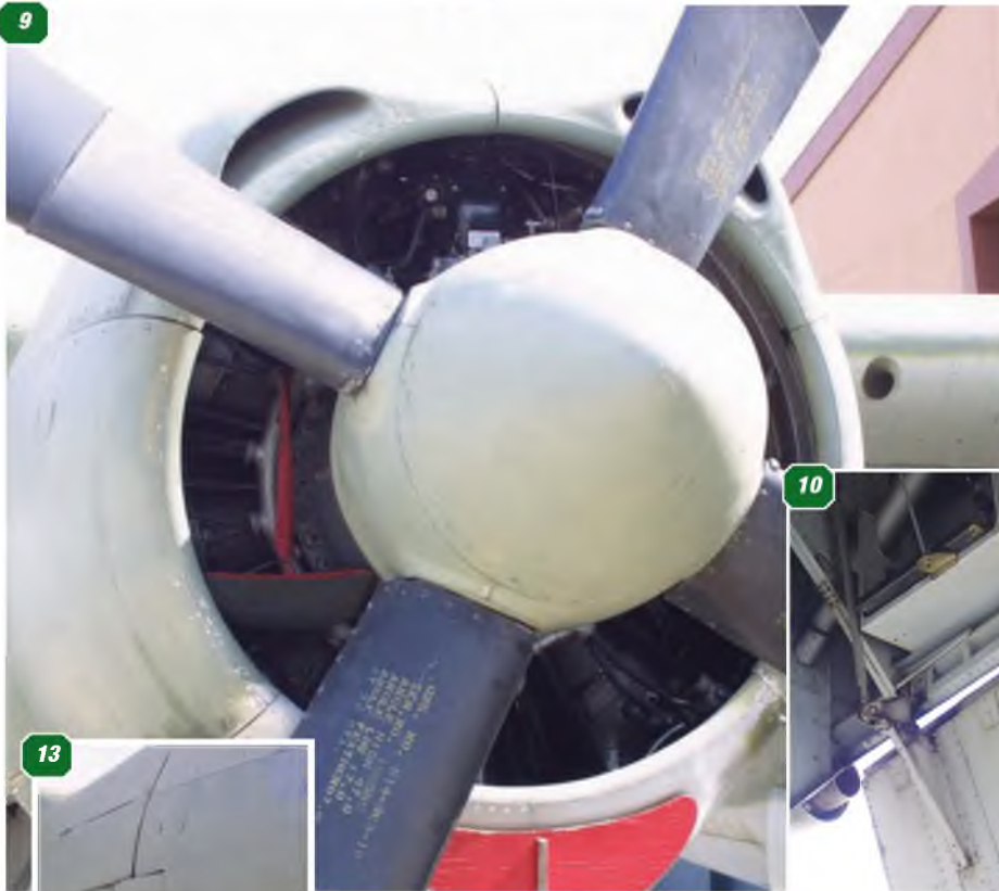
6: Exhaust outlet, lower side of engine cowl. 7: Exhaust stub positioned between the cowl rear and the main undercarriage door. 8: Adjustable exhaust outlet just in front of the main undercarriage bay. 9: Engine cowl front ring. Note air scoops top and bottom. 10, 11 & 12: Inside the main undercarriage bay, showing the door hinges. 13: Exhaust gills, viewed from front. 14: Propeller spinner and prop. blade cuffs. 15 & 16: Rear fairing of the engine nacelles. 17: Air scoop in front ring of engine cowl.
