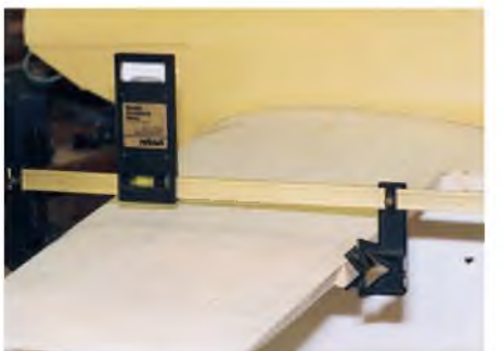
Setting the wing incidence - note the packing piece to 'square' the aileron spar.
