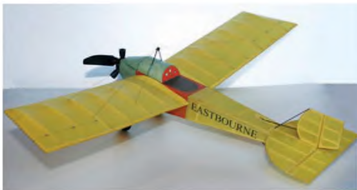
ABOVE: An exercise in printed tissue technique, lightweight building and imaginary detail, the author's 18" span Eastbourne Monoplane. RIGHT: As you see, the weather did improve and I was able to test fly the mini Eastbourne and it performed pretty much as anticipated. Some models fly well no matter what size they are.
