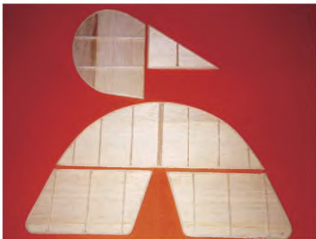
Tail surfaces using a sheet core. Outlines can be balsa, all tube, or cane.
