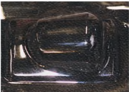
Windscreen moulding - rear curve is only for moulding purposes
