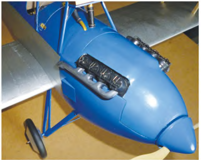
Lots of interesting details here. The dummy engine, hatch separation line and the way the radiator hoses neatly disguise the servo lead. Also clearly seen is the glassed foam spinner.
