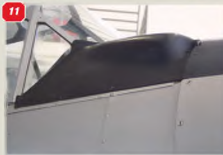
7 - 10: Major feature of the AT-6 is its long multiple-pane sliding cockpit canopy which demands much attention in a scale model replica. 11 & 12: Offset fuselage blister on the right of the fuselage ahead of the front winscreen. 13: Complete tailcone. 14, 15 & 16: Fin and rudder, showing aerodynamic balance. 16: Rudder control horn and cable. 17: Navigation tail light.
