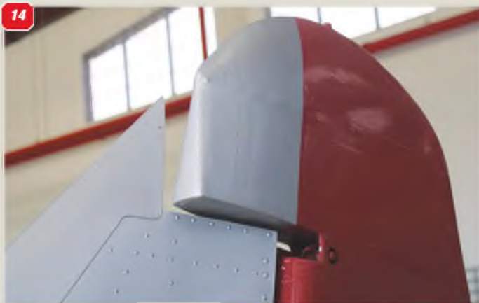
7 - 10: Major feature of the AT-6 is its long multiple-pane sliding cockpit canopy which demands much attention in a scale model replica. 11 & 12: Offset fuselage blister on the right of the fuselage ahead of the front winscreen. 13: Complete tailcone. 14, 15 & 16: Fin and rudder, showing aerodynamic balance. 16: Rudder control horn and cable. 17: Navigation tail light.
