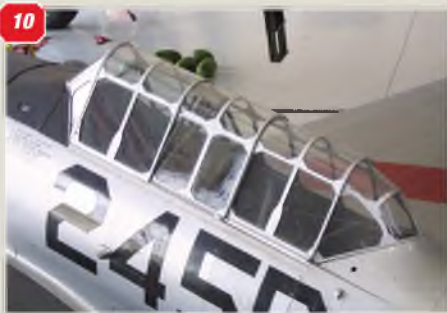
7 - 10: Major feature of the AT-6 is its long multiple-pane sliding cockpit canopy which demands much attention in a scale model replica. 11 & 12: Offset fuselage blister on the right of the fuselage ahead of the front winscreen. 13: Complete tailcone. 14, 15 & 16: Fin and rudder, showing aerodynamic balance. 16: Rudder control horn and cable. 17: Navigation tail light.
