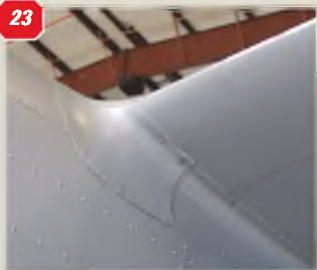
22: Elevator/taillplane hinge line. 23: Tailplane-to-fuselage cuff. 24: Elevator trim tab. 25: Fuselage panel detail at rear end of cockpit canopy. 26: Panel-line detail at the wing training edge, showing wing-to-fuselage fairing shape. 27: Upper rear fuselage surface panel detail just ahead of the fin leading edge. 28: Panel and annotation detail on upper fuselage, just ahead of the cockpit windscreen
