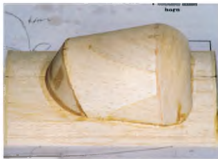
Checking the fitting of the windscreen mould on the fuselage mould
