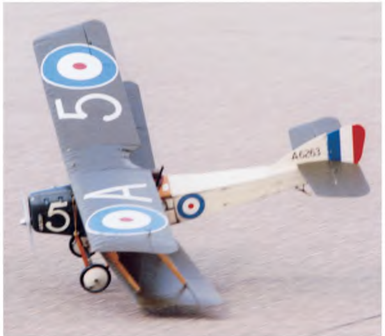
Take off is always a crucial time for these delicate models - if the model turns crosswind, the gusts can lift a wing, causing a cartwheel and subsequent damage. Here, Mike Smith's Martinsyde Elephant catches a crab!
