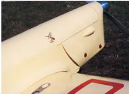
Fuselage/wing joint needs silicone filling
