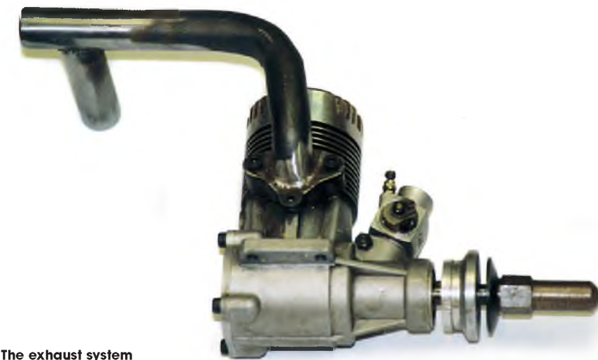
The exhaust system proved to be a little restrictive
