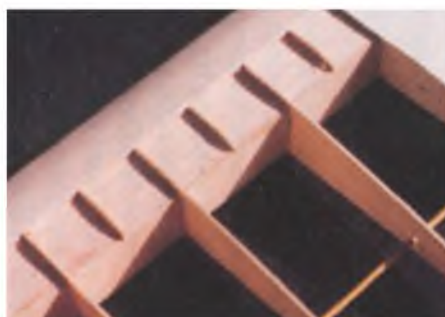
The wing sheeting in place, together with the leading edge riblets, over the mainspar. Note the dowel aileron-operating rod the passes through holes in the ribs.
