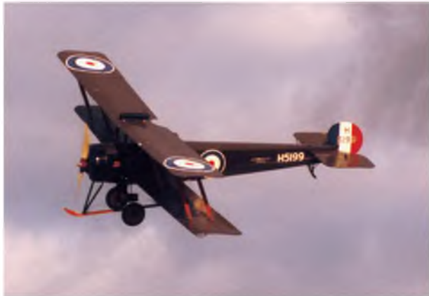
Undercarriages are always vulnerable on F/F scale models - Some of the early training aircraft had a skid to prevent nosing over - in model form, it can take some of the load off of the main legs - and the prop!
