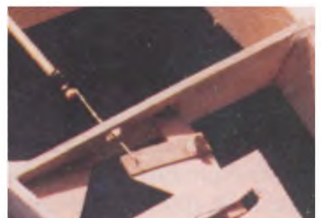
The other end of the aileron push rod, linked to the aileron bellcrank, mounted on a strip of plywood between the ribs, just outboard of the wing dihedral break.
