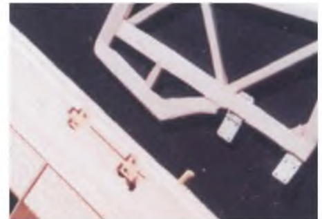
Here the main undercarriage has been removed, prior to covering. Note the sheeting is cut away to allow the wire legs to be clamped directly against the pine mounting plate. The fin is made up from strip, cut from balsa sheet.
