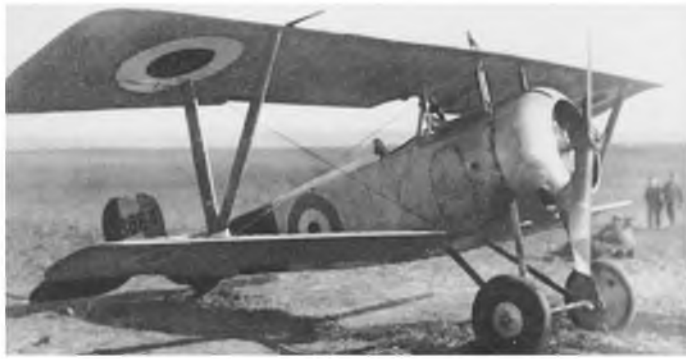
This British RFC N.17 fell into German hands during the Battle of Arras during April-May 1917. It has a top-wing leading edge pitot head.
