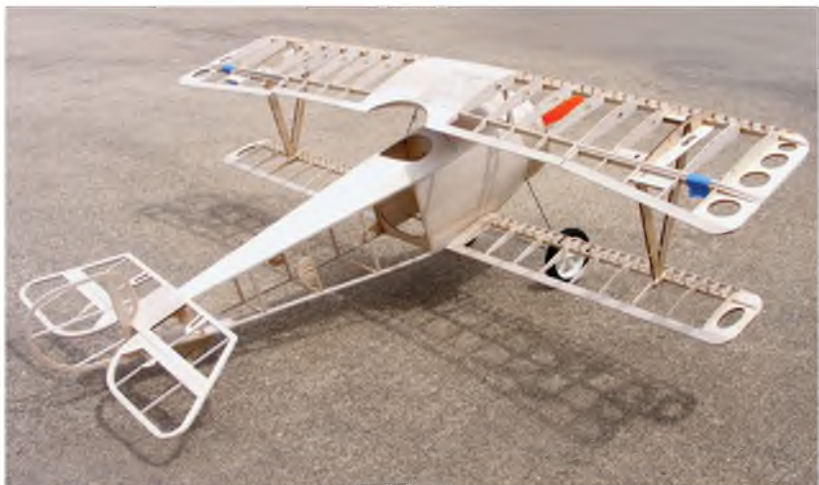
The obligatory naked model shot reveals the uncomplicated nature of the construction - just lots of sub-ribs.
