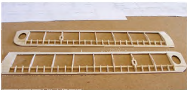
By comparison with the top wing, the lower wing panels are simple affairs to build.
