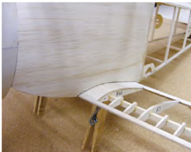
Use the locating dowels to align the lower wings and cut away the fuselage sheet to clear them.
