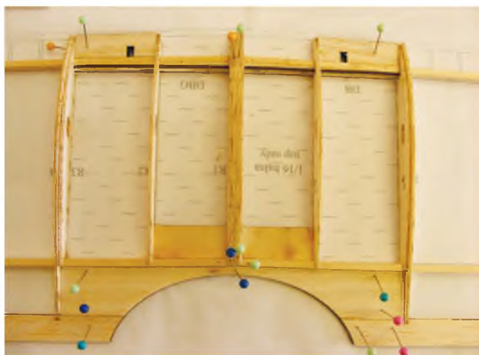
Demonstrating that Jim did in fact build his top wing as a single unit. Note the wedge for the brace and the strut plates all securely glued in place.
