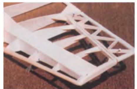
The ailerons feature 'Warren' style construction to guard against warping. The tapering depth spar box holds the built-in washout (just like the full size) of the wing tip.
