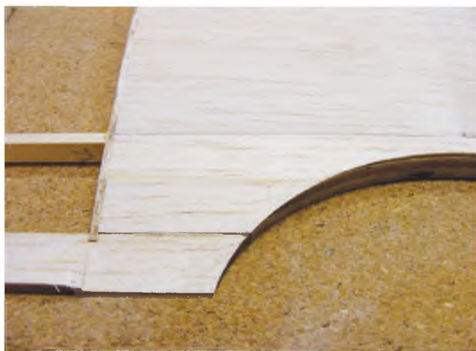
Here you see the c/s sheeted and the laminated CS parts sanded to shape.
