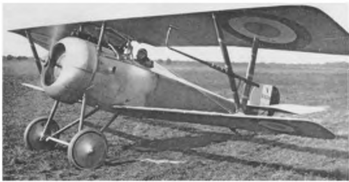
A French N.17 with fuselage-mounted Vickers Gun and experimental pitot 'yawmeter' attached to the V-interplane strut.
