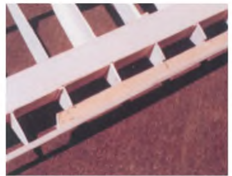
The basis of the wing is a full depth box spar (strong and light), the vertical components being web pieces between the ribs. Note the pine undercarriage mounting strip at the leading edge.
