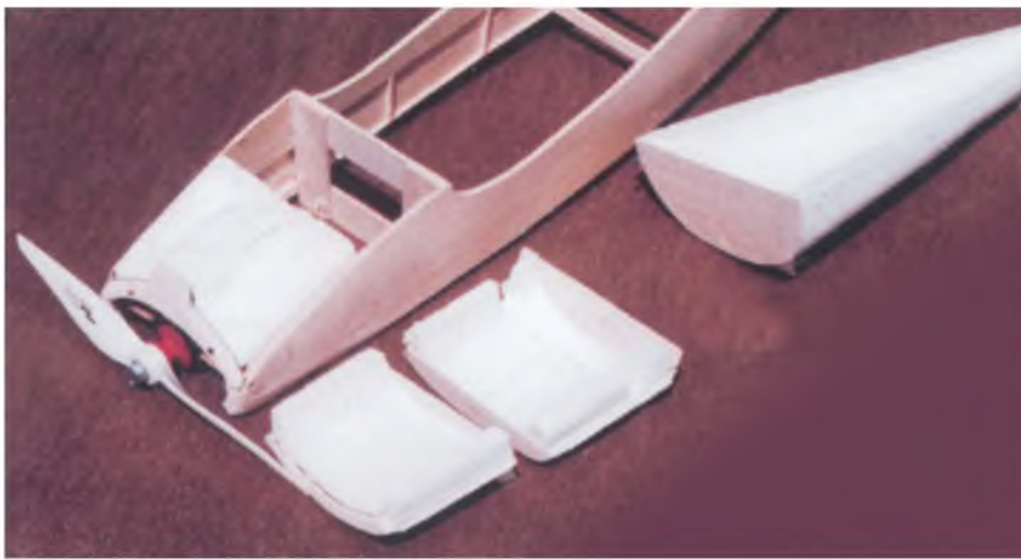
The simple, lightweight build philosophy is evident throughout the entire model. Here is the basic fuselage 'box', with the carved white foam cowl, top hatch and rear top decking.
