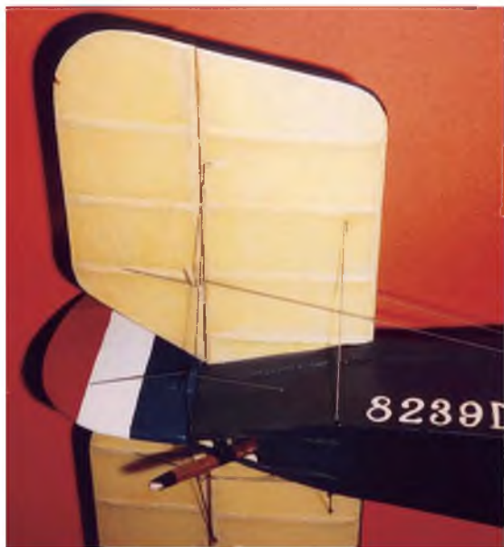
Even at this scale size, rib tapes and stitching and lacing should be reproduced.
