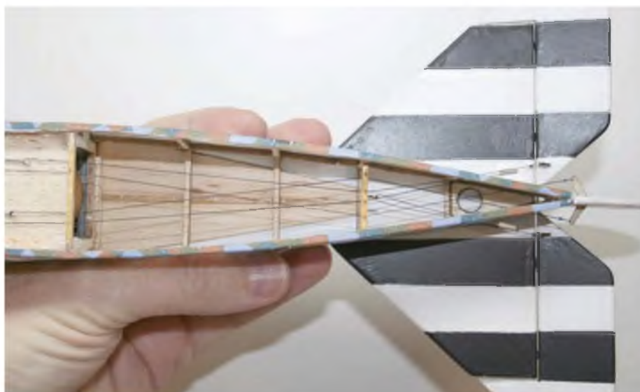
Fishing hook eyes provide pivot points so the cables can exit in the correct positions. Jon's hand lends scale to the Fokker DVIII model.
