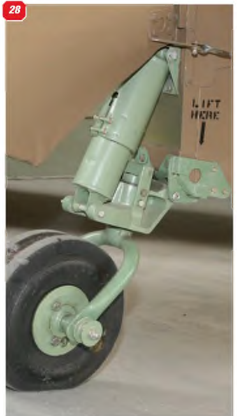
24: View of the elevator centre, where it runs through the fin. 25: Panel detail on the side of the rear fuselage. 26: Close-loop control cable and rudder horn. Also showing lower tailwheel unit mounting bracket. 27: Panel and stencilling detail ahead of the rudder post. 28: Detail of the complete tailwheel unit.
