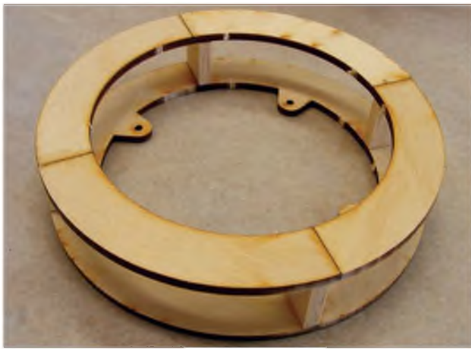
Spacers used to hold the assembled cowl rings while they are wrapped with ply.
