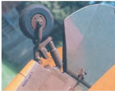
Three views of the fuselage rear, detailing the tailwheel unit and the tailplane. Note the closed loop rudder linkage, the elevator hinges and the dummy elevator trim tab.
