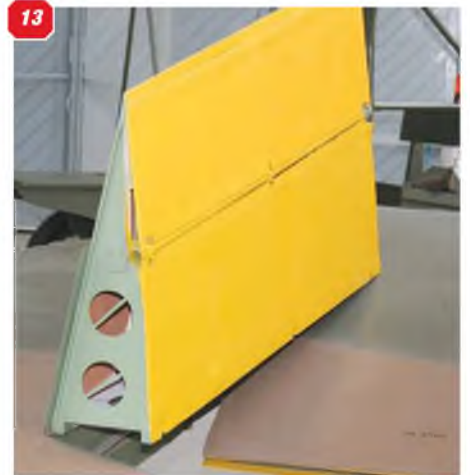
11: Another view of the folded wing, also showing the wing-to-fuselage fairing. 12: Close-up of the tail light mounted on the rudder. 13: close-up detail of the wing component that folds into the vertical position to facilitate the wing fold. 14: View forward over the cockpit/cabin. 15: Navigation light at the wing tip leading edge. 16: Further view of the tailcone. 17: Landing light in the wing leading edge. 18: Tailplane root and the cuff panel that fairs over the tailplane mounting.
