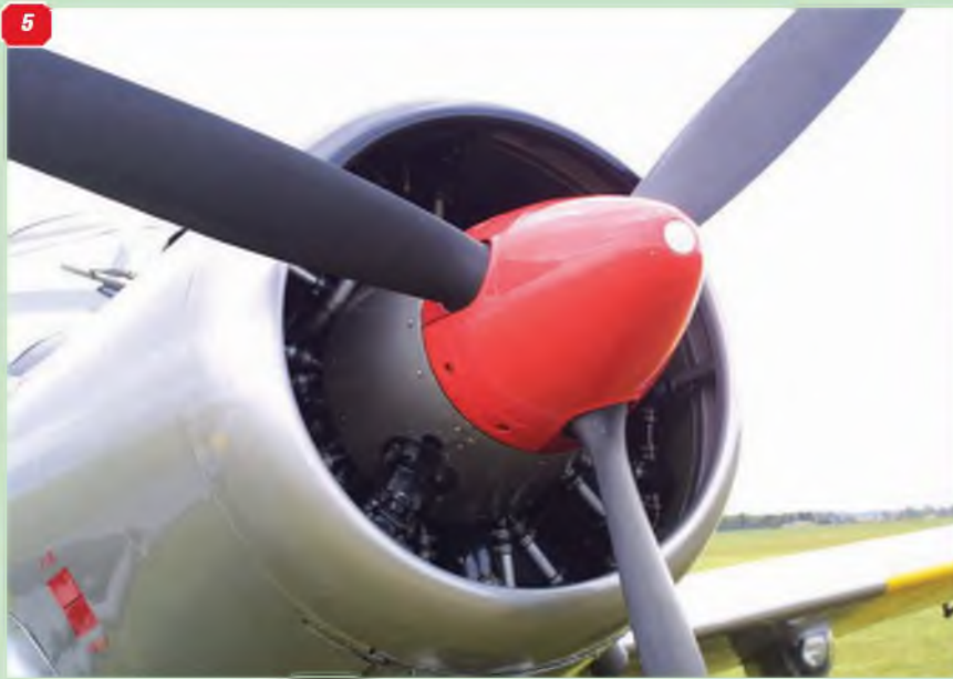
5: Engine cowl housing the Alvis Leonides engine. 6: Large centrally positioned air scoop in the cowling underside. 7: Exhaust, left side, ahead of wing leading edge roof.
