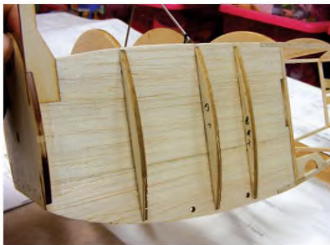
Side formers added to form the side sheeting around. Left and right sides are different, so take care with this.
