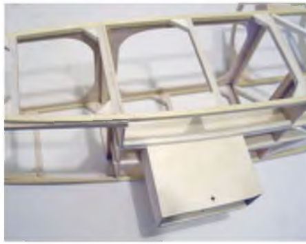
The deep fairing for the fixed monowheel.
