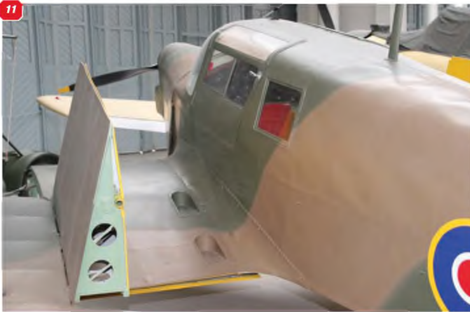
11: Another view of the folded wing, also showing the wing-to-fuselage fairing. 12: Close-up of the tail light mounted on the rudder. 13: close-up detail of the wing component that folds into the vertical position to facilitate the wing fold. 14: View forward over the cockpit/cabin. 15: Navigation light at the wing tip leading edge. 16: Further view of the tailcone. 17: Landing light in the wing leading edge. 18: Tailplane root and the cuff panel that fairs over the tailplane mounting.
