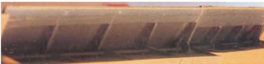
Wing underside trailing edge showing the split-type flap and reproduction of the flap internal structure.
