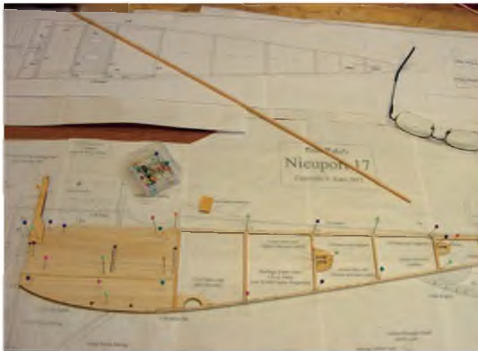
Although Jim used the forward fuselage side as a guide while building the rear frame they remain two separate items - not glued together.
