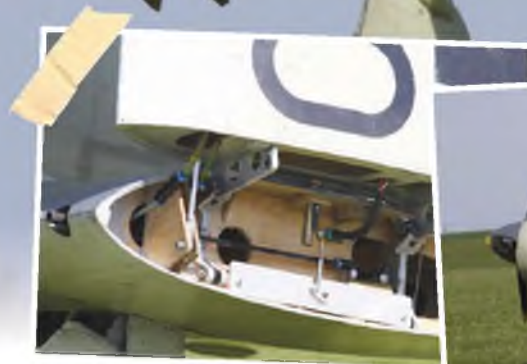
As promised, for all you anoraks out there: the folding wing / hinge mechanism on Mick Burrell's superb Sea Fury.
