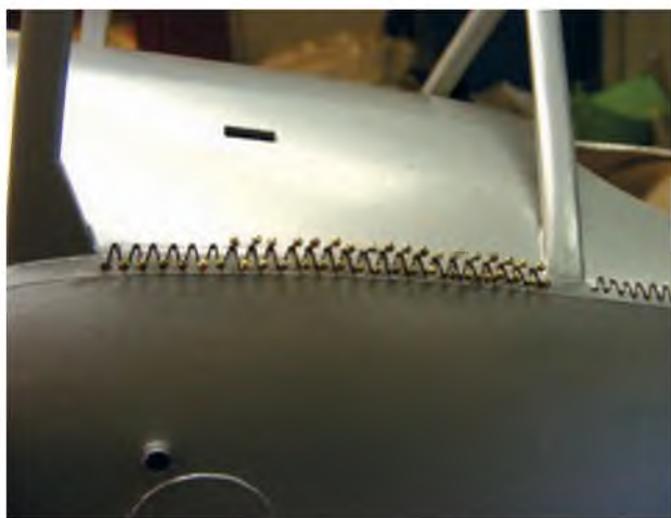
A neat way to create the prominent lacing so obvious on Nieuport types.
