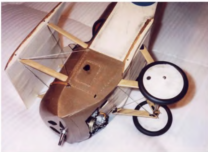
Access panels, side panel staining and under fuselage gunge all faithfully reproduced on Andy's Tabloid. Note the simple 'sprung axle' undercarriage and wire joiner plug-in wings.
