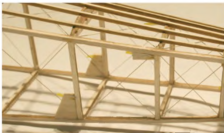
Control cable exits at scale locations will be completely hidden once the covering is applied.
