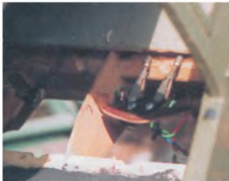
The servo tray in the rear of the wing seat. Closed loop control runs were used on the prototype model.
