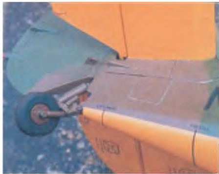
Three views of the fuselage rear, detailing the tailwheel unit and the tailplane. Note the closed loop rudder linkage, the elevator hinges and the dummy elevator trim tab.
