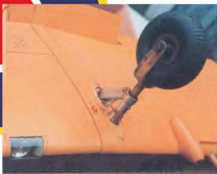
Wheel trouser removed here to reveal the main undercarriage leg.
