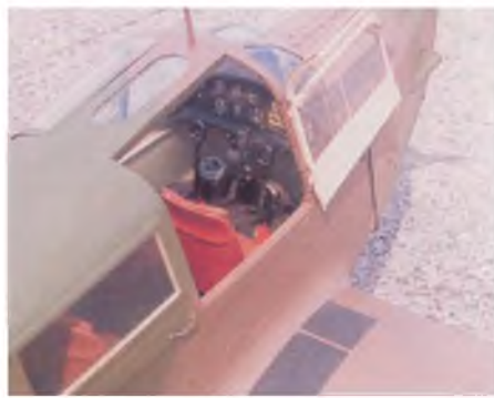
A further view of the cockpit, showing the cockpit access door and the wing tread panel.
