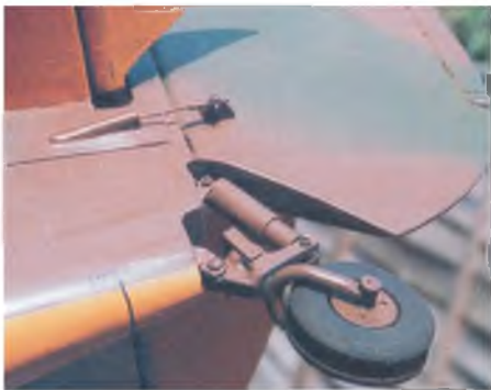
Three views of the fuselage rear, detailing the tailwheel unit and the tailplane. Note the closed loop rudder linkage, the elevator hinges and the dummy elevator trim tab.
