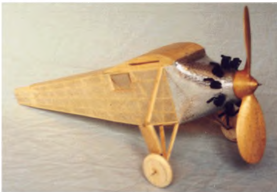
Even small models can be enhanced with the application of a scale finish. Here is a rubber-powered Ryan NYP, showing the 'turned aluminium' cowling panels - so distinctive of this type.
