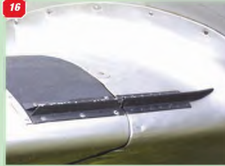
13: Wing root showing the pressed metal fairing and the cockpit access tread patch. 14: Aileron hinge. 15: Wing underside, showing the main drive and trim tab linkages. 16: Leading edge spoiler, right hand wing. 17: Tailwheel.
