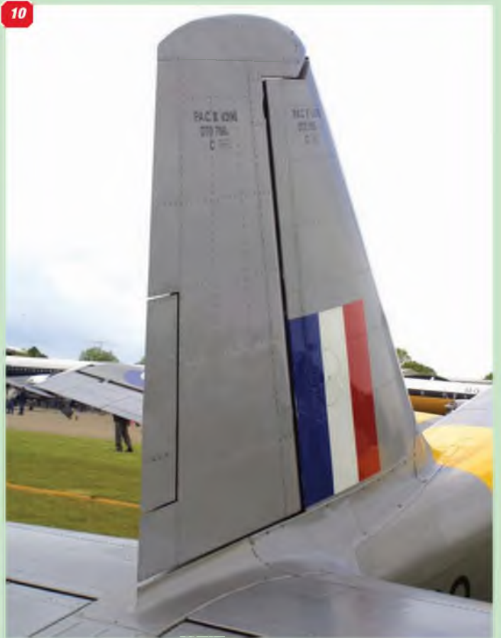
8: Grip handle on fuselage side at cockpit position. 9: View of the engine cowling from the rear, showing the air outlet and the wing root fairing. 10: The tall fin and rudder. Note the cuffed rudder-to-fin hinge line and trim tab. 11: Detail of the elevator, showing the external trim tab linkage. 12: Tailplane flap, showing the line of the aerodynamic balance.
