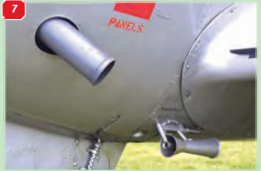
5: Engine cowl housing the Alvis Leonides engine. 6: Large centrally positioned air scoop in the cowling underside. 7: Exhaust, left side, ahead of wing leading edge roof.
