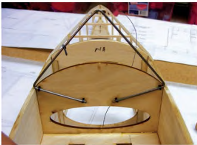
The rear c/s strut firmly bound to the former. Note the fishing hook eye used to attach it to the wing.
