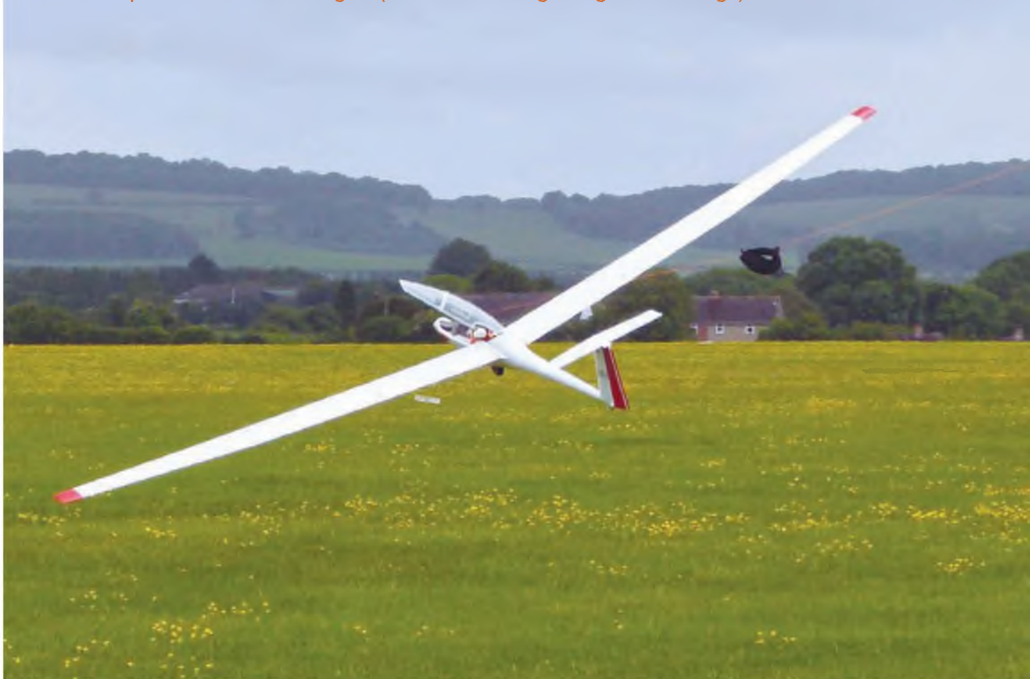
Brian Sharp's Kestrel in dire straights (note towline at right-angles to fuselage).
