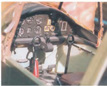
Never throw away anything - it may come in handy sometime! Long after the model was wrecked, designer Roy was able to resurrect the airframe for these cockpit photos showing the instrument panel and cockpit furniture.
