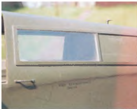
Detail of the cockpit rear windows. Note the handgrip and re-inforcement strakes.
