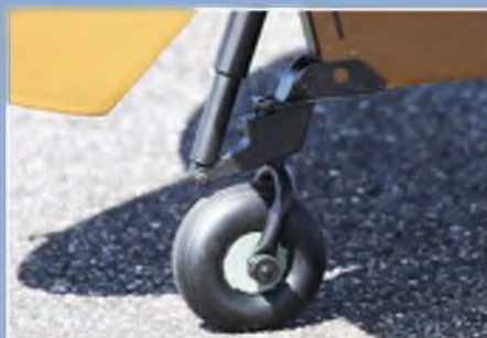
As you might expect, the tailwheel is proper engineering.
