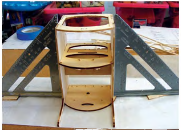
Squares and the way the formers fit the sides assure a square forward fuselage assembly.
