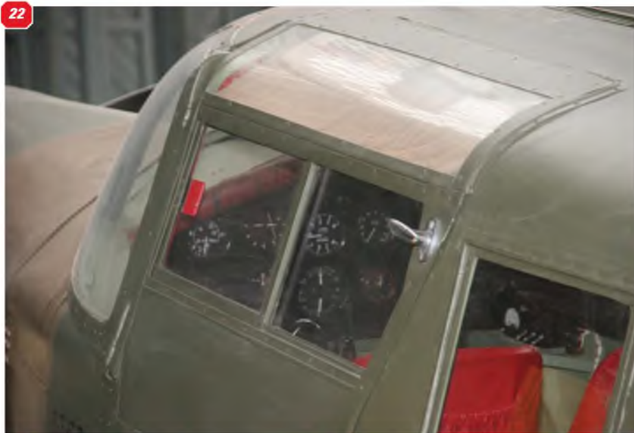
19: Detail of the fuel tank filler cap on the wing upper surface. 20: Tailplane hinge-line detail showing the slotted hinge position. 21: Further view of the fin/airplane fairing. 22: Cockpit window frame detail. Note the access door latch handle. 23: Right side of the cabin/cockpit showing the line of the access door.
