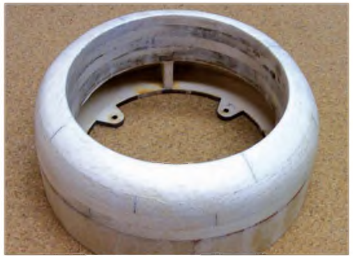
Ply and front rings added and the cowl all nicely sanded to shape.
