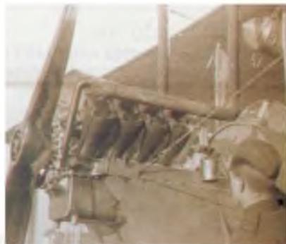
The eight-cylinder RAF 1a engine installation that applied to most DH 6s.
