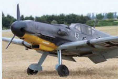
Stunning Me 109G by Staffen Zaun. Spans 3.3 metres, weighs 37 Kgs, and powered by a King B2 195 petrol engine.
