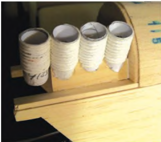
They may only be thread wound paper tubes but the dummy cylinders will add a lot of realism to the finished model.
