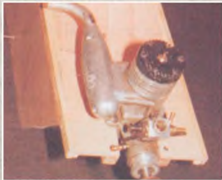
An elderly Merco 61 (yes, there are still some around!) provided more than necessary power for the prototype model. A .46 or .51 engine would be quite suitable.
