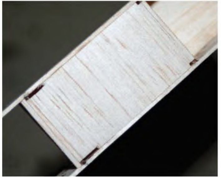
The sheeting between F2 and F3 will need to be slotted for the U/C legs to fit into.
