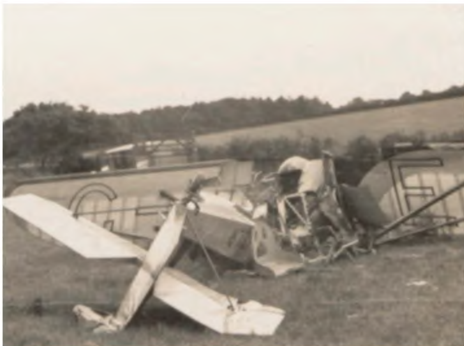
In September 1937 the Pup was sold to Anthony E. Green. In August, he stalled the aircraft while taking off from Bishop's Tachbrook aerodrome, Leamington and it was written off. By this time the Pup's Ava engine had been replaced by the more powerful Bristol Cherub. (via Richard Riding)
