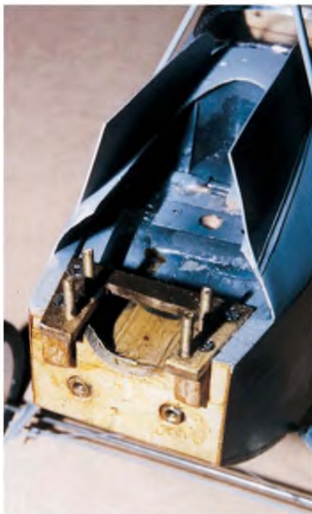
LEFT: Mills 75 diesel engine and dummy replica are here removed to reveal the engine bearers. BELOW: Mills diesel and dummy re-installed. RIGHT: Detail of the dummy scale Austro-Daimler engine and wheel. BOTTOM RIGHT: Cabane struts, dummy tank and radiator.
