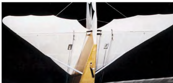
Tailplane underside showing scale support struts and dummy control cables to elevator and rudder.
