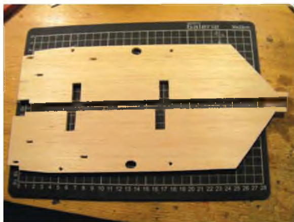
The main components of the forward fuselage box; the 3/16 balsa sides. Note the cut outs for the struts and control cable exits.
