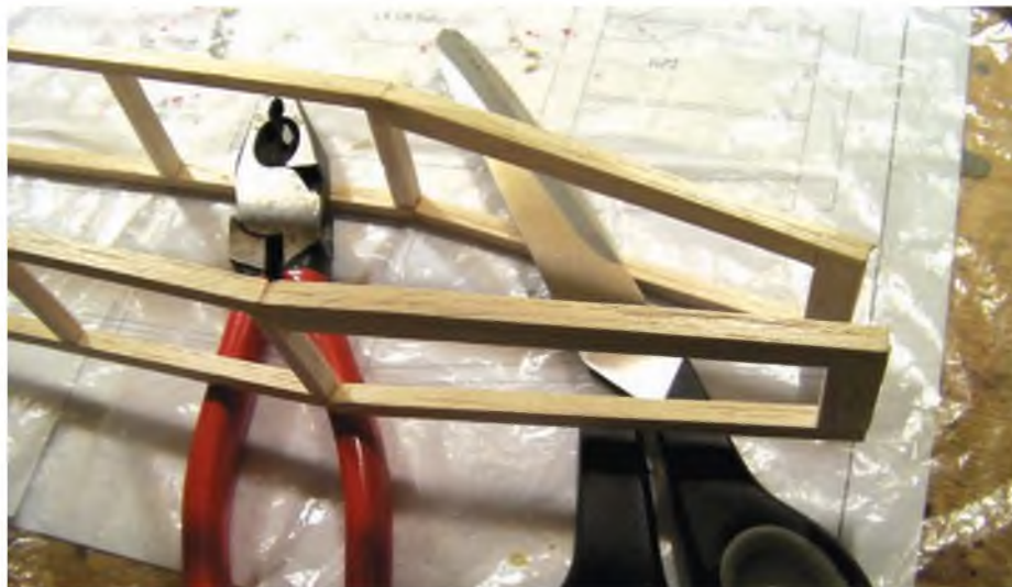
Working over the plan to get the break angles at the tail correct before actually joining the tail-posts.
