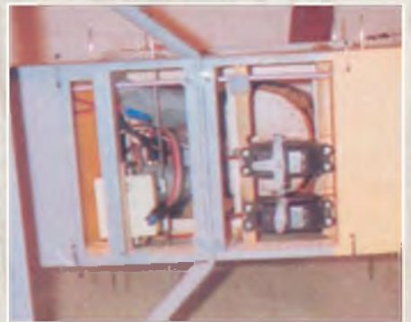
The airborne radio system is accessed via the hatch in the fuselage underside and provides plenty of installation space.
