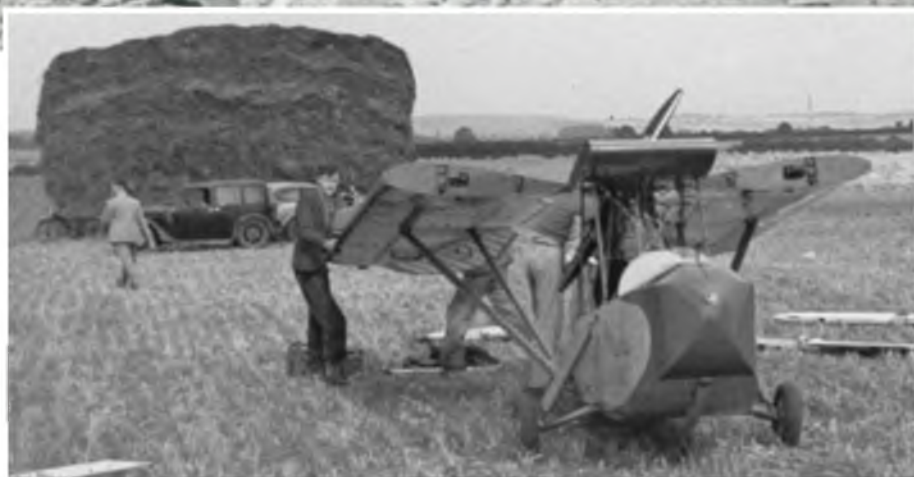
The Dart Pup's width, with wings folded was 9 ft 8 in and here it is seen after being towed from Dunstable to nearby Loosey Farm. (via Richard Riding).
