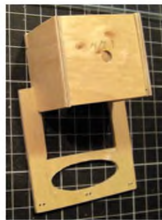
The firewall, with the motor mount attached. Make sure you get the right parts in the correct place.
