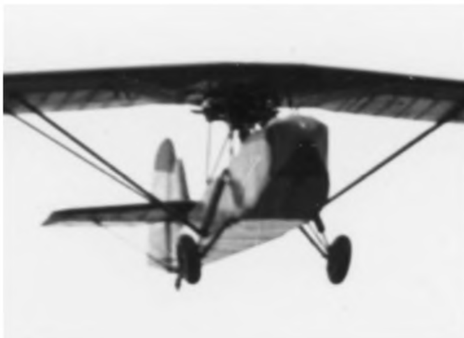
This airborne view of the Pup shows the pronounced sweepback on the semi-cantilever wings. With no dihedral, the wings had an area of 114 sq ft, a loading of 6.18 lb per sq ft and a NACA 23012 aerofoil section. (A.H. Curtis via Richard Riding).
