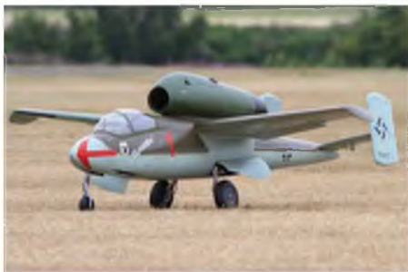
Superb Heinkel Salamander by Armin Morgenweck. Weighs 19.6 kgs, 2.3 metres, powered by an Alfred Frank Raptor gas turbine.
