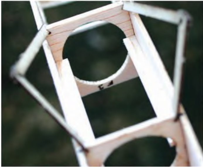
How the u/c assemblies will eventually fit into formers F2 and F3.
