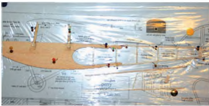
Totally conventional, the fuselage sides are built over the plan in the usual way.
