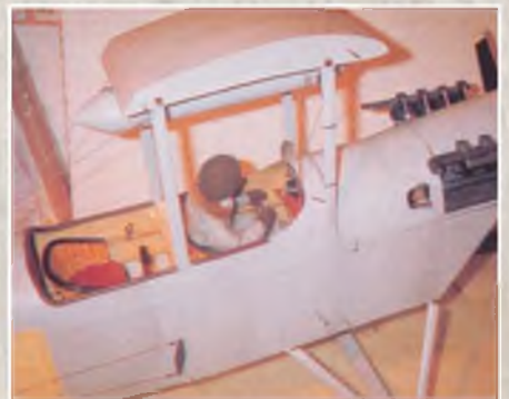
Instrumentation in the cockpit is rudimentary. Note the wicker instructor's seat, similar to that occupied by the student pilot.
