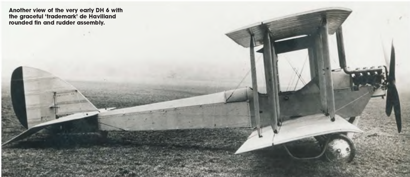
The nose profile of this DH 6 features a blunt 'flat-face' radiator typical of other aircraft of the period and may well had a Curtiss OX-5 engine installed.
