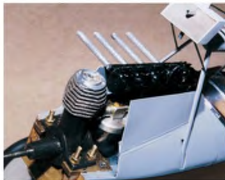
LEFT: Mills 75 diesel engine and dummy replica are here removed to reveal the engine bearers. BELOW: Mills diesel and dummy re-installed. RIGHT: Detail of the dummy scale Austro-Daimler engine and wheel. BOTTOM RIGHT: Cabane struts, dummy tank and radiator.
