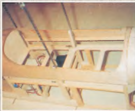
Top fuselage decking is shaped to size, but not glued in place until the cabanes have been bound and glued.
