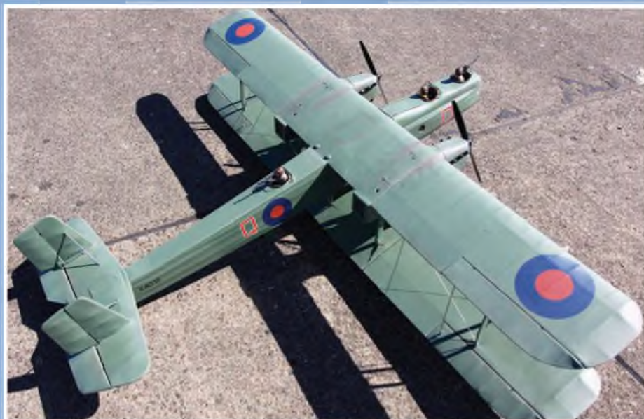
This angle displays the quite high aspect ratio of the wing.
