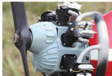
Nifty dummy Pobjoy radial on John Carpenter's 1/4 scale Comper Swift effectively hides the Laser 180 FS underneath!
