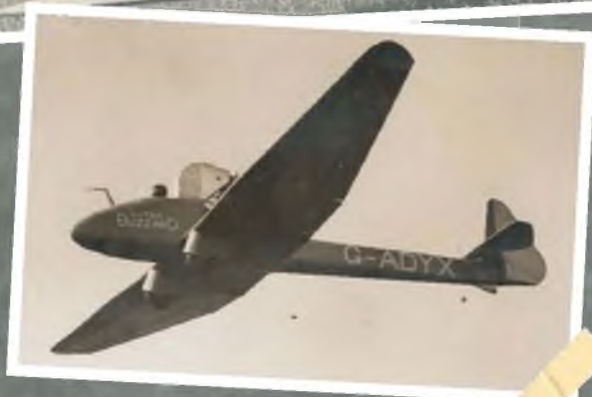
This early airborne view of Luton L.A.1 Buzzard Mk I G-ADYX shows the rather ugly initial installation of the 35 hp Anzani engine.
