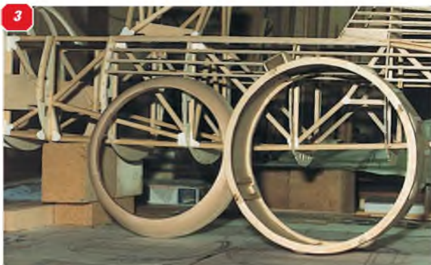
1: Model features scale stringer spacing throughout fuselage. Wing Structure uses 1/4" sq. spruce or hard basswood. Two wing tubes glued and taped to structure. 2: Sheeted area ahead of cockpit forward to firewall. Undercarriage anchors at bottom. Battery and first-aid hatch is thin plywood. 3: Engine cowl and cowl ring, make from in wood - no glass fibre moulding! Formers are wrapped with 1/32" plywood in four layers.
