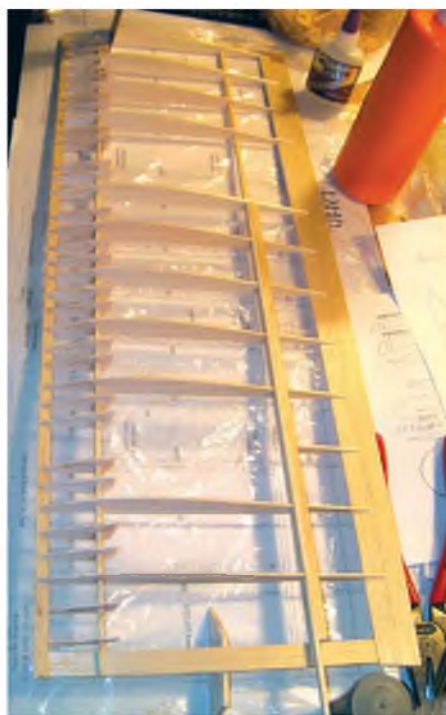
The wing tip packed up while the root rib is glued in place at the correct angle for dihedral. (all four panels)
