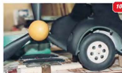
9: Main undercarriage 'trousers', built from layers of sheet balsa. 10: The fully finished main undercarriage. Side covers, as per full size, removed to reveal the wheel.
