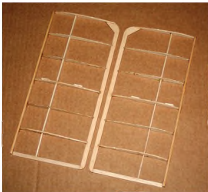
The wings all trimmed and sanded ready for joining to the c/s. Those 1/32 ribs and soft balsa trailing edges played havoc with the shrinking.
