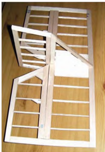
Tail surfaces really don't get any easier than this. Nothing but straight bits of wood as far as the eye can see.
