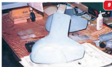
9: Main undercarriage 'trousers', built from layers of sheet balsa. 10: The fully finished main undercarriage. Side covers, as per full size, removed to reveal the wheel.
