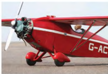
John Carpenter's new Comper Swift one-third scale, Laser 180 powered, covered in Solartex.
