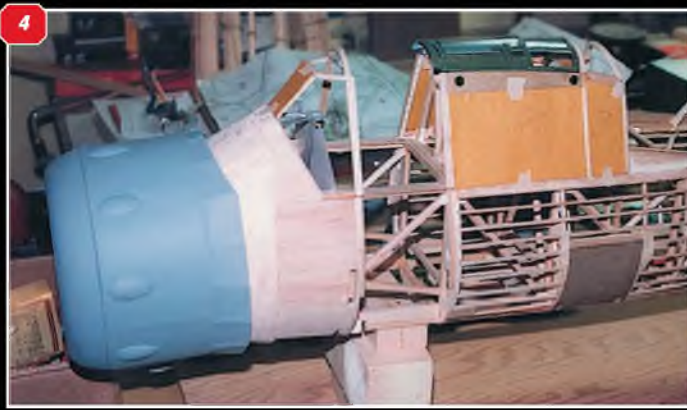
4: Engine cowl complete and fitted. Note cardboard over cockpit area for marking off 'green-house' frames, to be made in clear plastic. 5: The sliding section of the forward cockpit frame is removed to facilitate wing attachment. Aileron tubes are inserted. 6: Finished dummy Bristol Mercury radial engine hides .56 two-stroke engine, mounted side-winder. 7: The fully finished with dummy exhaust stack, cowl dummy engine and pilot's bucket seat. 8: Nose, showing the dummy Bristol Mercury engine in place and dummy scale propeller fitted.
