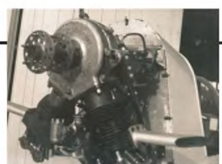
A photograph showing the installation of the inverted Vee air-cooled 35 hp 'Luton' Anzani engine in the Luton Buzzard modified for pusher layout by having an additional thrust race.
