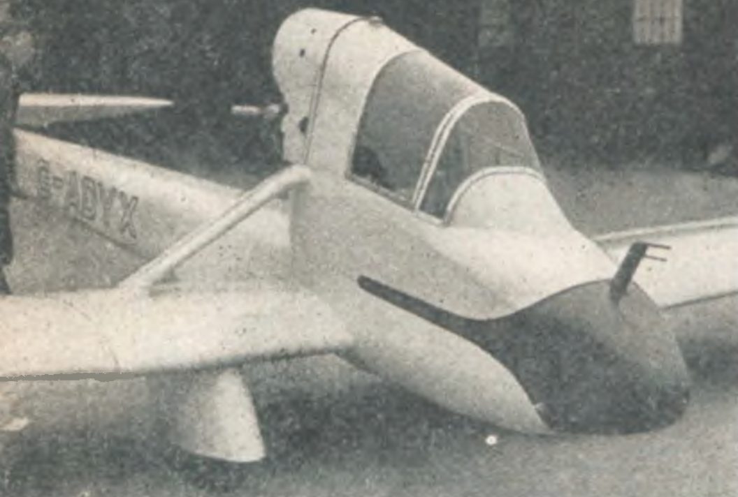
The Buzzard Mk.II's enclosed cockpit was a feature seldom applied to light aircraft of the 1930s.
