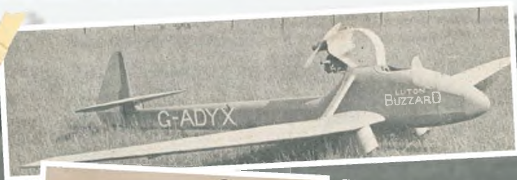
This early airborne view of Luton L.A.1 Buzzard Mk I G-ADYX shows the rather ugly initial installation of the 35 hp Anzani engine.
