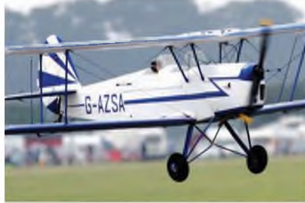
Andrew Bowman's 1/4 scale Stampe SV4b from the Svenson kit, bought in 1982. SC 180 power driving a 18"x8" prop.
