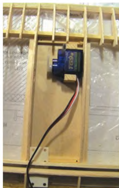
A good shot showing how the strut sockets are created and how the servo tray fits into the bottom wings. No servo arm exit slot yet though.
