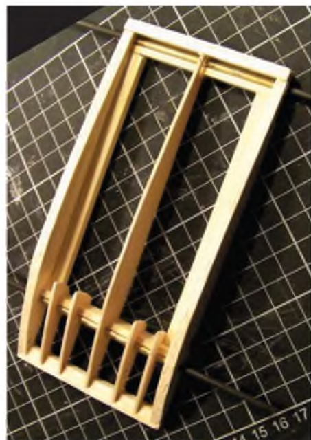
The top wing centre section, complete with joiner tubes and carbon rod wing dowels.
