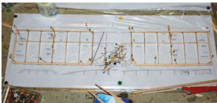
Wing construction follows the usual practice of building over the plan.
