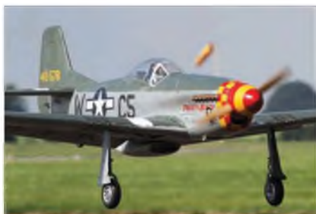
P-51 Mustang by Richard Scarborough from the Nick Zirolli plan. 3W 60 petrol power, and glasscloth covered.
