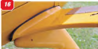
12: View of the elevator upper surface, again showing the trim tab which is hinged on the top surface. 13: View under the tailplane showing the mounting lugs that attach it to the fuselage. 14: Tail light on the rudder trailing edge. 15: The tail wheel unit. 16: The wing strut, where it fairs with the fuselage. 17: The wing strut-cum-undercarriage mount, viewed from the rear, is a complicated arrangement. 18: Foot step for access to the cabin. 19: Front view of the wing strut, showing the bare metal face plate around the leading edge.
