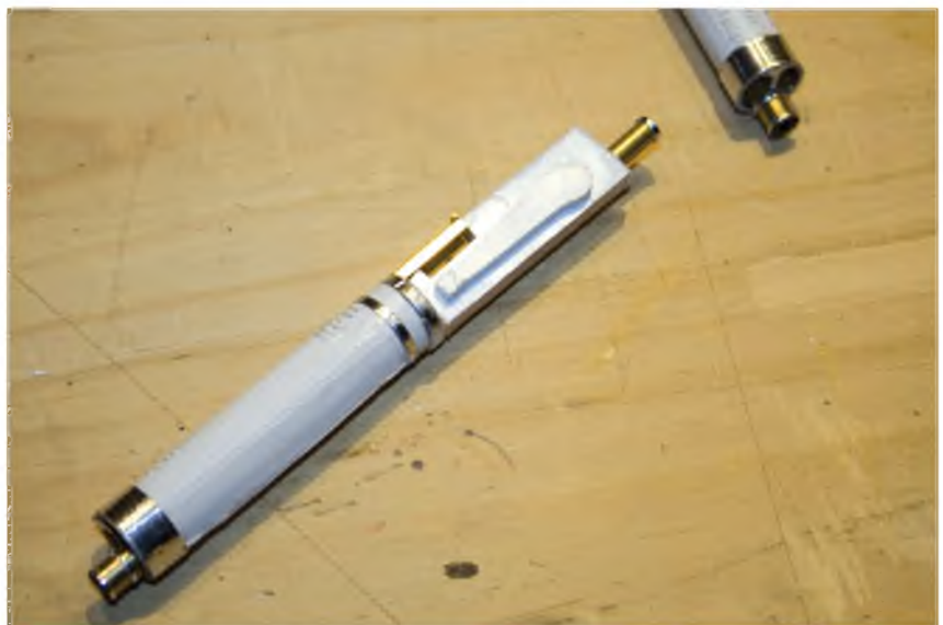
More details added from wood, plastic card and metal tubing complete the basic gun.
