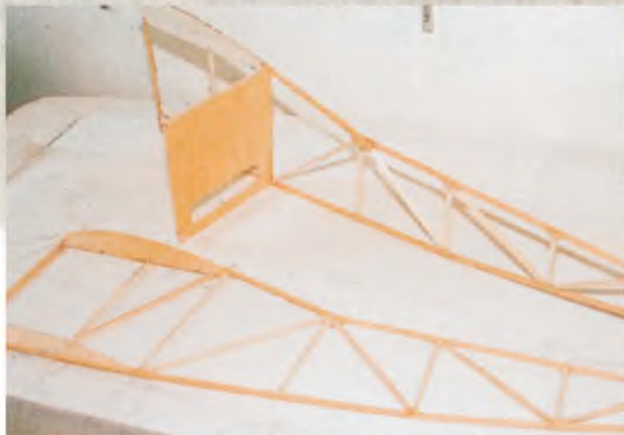
Start of the fuselage box assembly, commenced by joining the sides with former.
