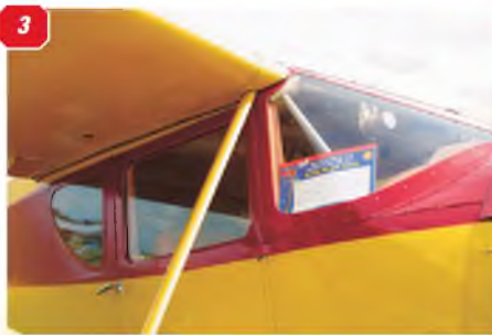
1: Nose section showing panel lines and air intakes. 2: Cabin door hinge and the fairing where the wing/undercarriage strut meets the fuselage. 3 & 4: Two views of the cabin area showing the line of the cabin access door and the window panelling.
