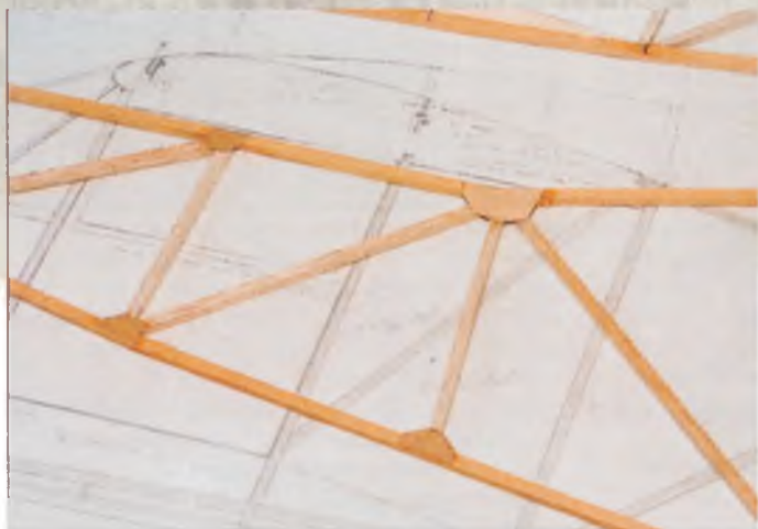
Basic fuselage sides made up from balsa strip, showing 0.4mm ply reinforcement gussets.
