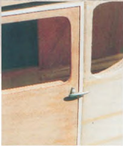
The prototype model has opening doors for access to wing bolts.
