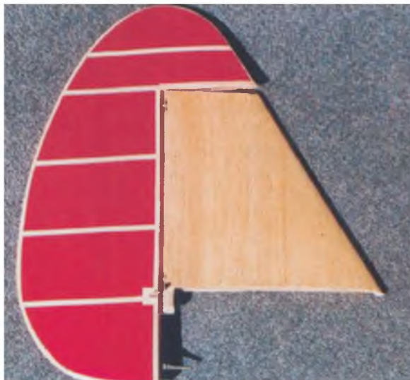
The covered fin and rudder. Note the rib tape on the rudder.
