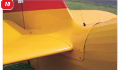
5: View under the engine cowl showing the exhaust stack, offset to the right. 6: Engine cowl, showing panel lines and air vent. 7: Further view of the engine cowl underside, showing panel lines and vents. 8: Nose close-up, showing air intakes. 9: Two blade wooden propeller. Tips are metal clad. 10: Metal cuff panel that fairs the tailplane and rudder joint. 11: Right hand elevator, viewed from the rear, showing the trip tab.
