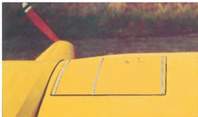
The dummy access panels for the wing tanks on the wing upper surface.
