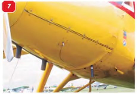
5: View under the engine cowl showing the exhaust stack, offset to the right. 6: Engine cowl, showing panel lines and air vent. 7: Further view of the engine cowl underside, showing panel lines and vents. 8: Nose close-up, showing air intakes. 9: Two blade wooden propeller. Tips are metal clad. 10: Metal cuff panel that fairs the tailplane and rudder joint. 11: Right hand elevator, viewed from the rear, showing the trip tab.
