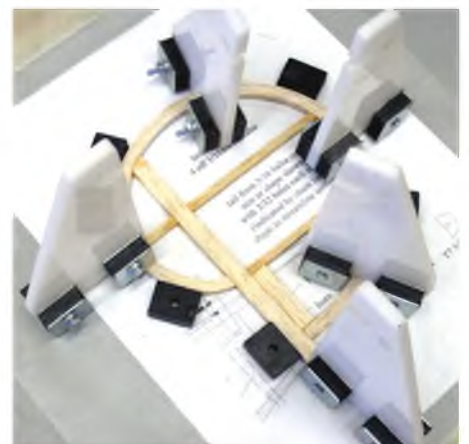
The basic rudder core being built over the plan. Darrin uses a magnetic building board, so no pins.
