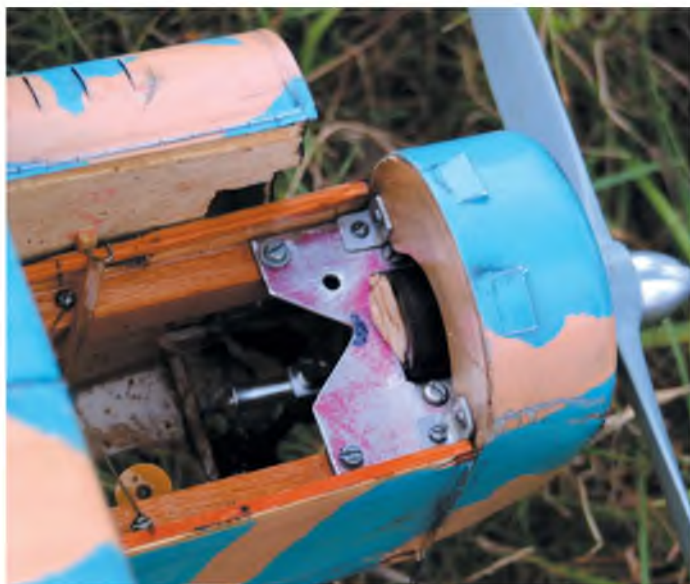
Practising what you preach! Metal mounting plate for thrustline adjustment, with cut-out for access to needle valve and choking. Note the rubber band-tensioned cowling hinge - dead easy for an inline engine on Andy Hewitt's Airco DH4.
