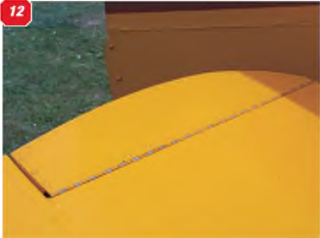
12: View of the elevator upper surface, again showing the trim tab which is hinged on the top surface. 13: View under the tailplane showing the mounting lugs that attach it to the fuselage. 14: Tail light on the rudder trailing edge. 15: The tail wheel unit. 16: The wing strut, where it fairs with the fuselage. 17: The wing strut-cum-undercarriage mount, viewed from the rear, is a complicated arrangement. 18: Foot step for access to the cabin. 19: Front view of the wing strut, showing the bare metal face plate around the leading edge.
