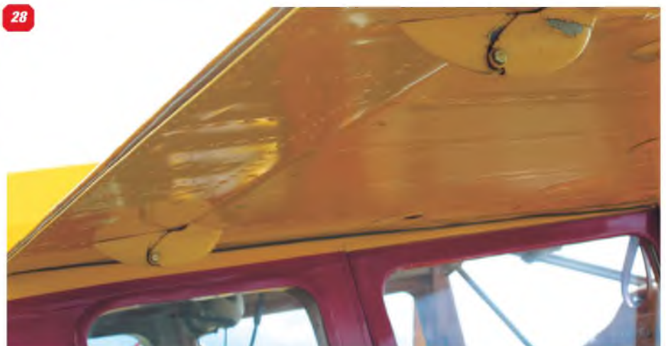
25: Front and rear wing struts converge to a single fuselage attachment point and are heavily faired with folded metal sheet. 26: Same position as 25 viewed from a different angle again reveals folded sheet metal components. Note also the bare metal leading edge face plate. 27: Detail of wing root. 28: Faired hinges to the wing flap on the wing underside.
