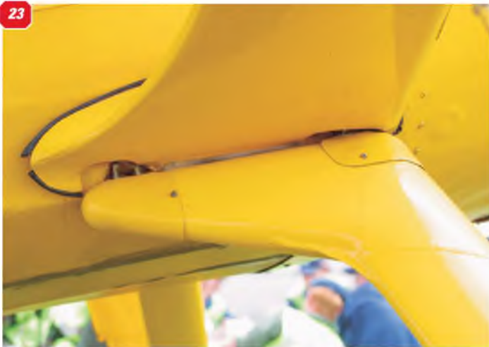
20 & 21: Two views showing the main undercarriage wheel and strut arrangement. 22: One of the main wheels seen from the opposite side. 23: View of the bottom of the fuselage, showing the mating and fairing of the wing strut and main undercarriage, where these attach to the fuselage. 24: Fairings over the wing strut attachment points.
