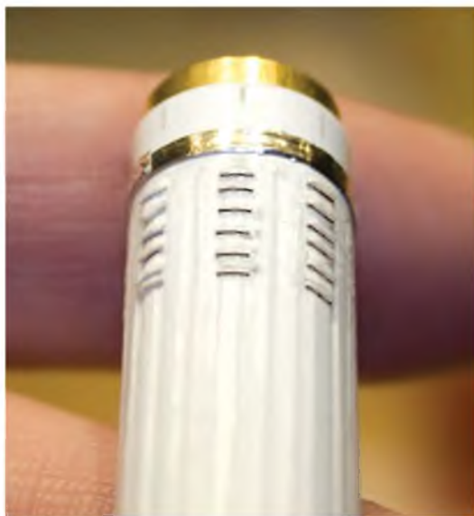
Cooling louvers chiselled in and a few bits of tube help add 'life'.
