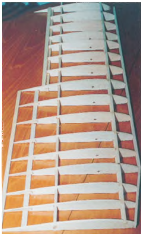
The basic wing structure complete, before addition of tip components.
