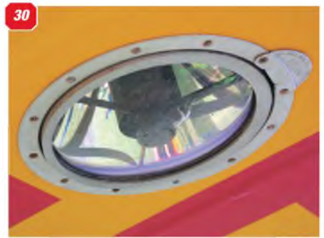
29: Wing root at the leading edge. 30: Landing light on the left wing underside, seen in the retracted position, flush with the wing surface. Unit is hinged to face forward when deployed. 31: Wing underside showing the flap hinge line and one of the faired hinges. 32: Aileron hinge line viewed under the wing. Note that the centre hinge is different from the other two and is seen, close up in 33 . 34: One of the other two aileron hinges. 35: Metal panels on the wing upper surface, viewed from behind the wing trailing edge. 36: Further view of the aileron hinge line viewed from under the wing. 37: Wing tip navigation light.
