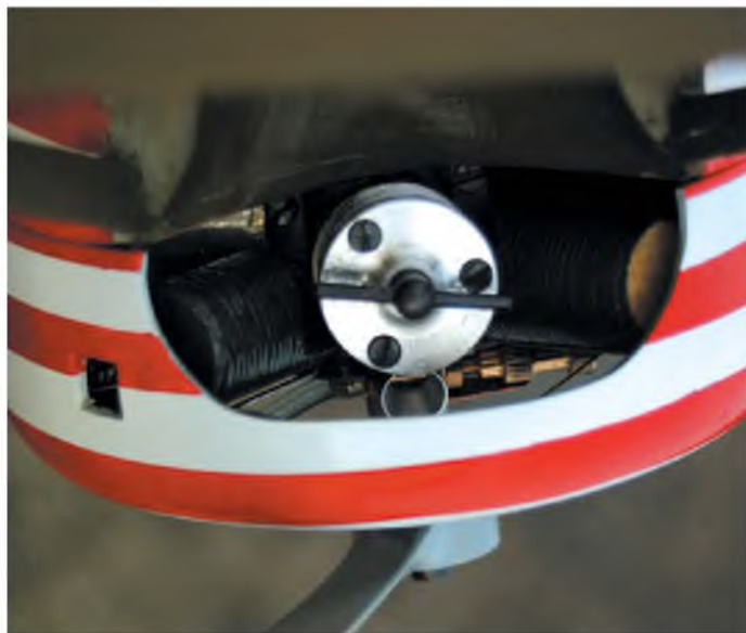
The front induction PAW 100 in John Rimmer's Sopwith Camel - not easy to get at, when running - but easier than if a rear induction motor was fitted!
