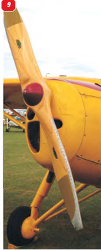
5: View under the engine cowl showing the exhaust stack, offset to the right. 6: Engine cowl, showing panel lines and air vent. 7: Further view of the engine cowl underside, showing panel lines and vents. 8: Nose close-up, showing air intakes. 9: Two blade wooden propeller. Tips are metal clad. 10: Metal cuff panel that fairs the tailplane and rudder joint. 11: Right hand elevator, viewed from the rear, showing the trip tab.
