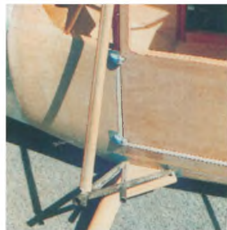
The strut and main undercarriage assembly. This is a prominent feature of the aircraft, so it's important to get it right.
