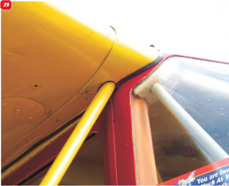
29: Wing root at the leading edge. 30: Landing light on the left wing underside, seen in the retracted position, flush with the wing surface. Unit is hinged to face forward when deployed. 31: Wing underside showing the flap hinge line and one of the faired hinges. 32: Aileron hinge line viewed under the wing. Note that the centre hinge is different from the other two and is seen, close up in 33 . 34: One of the other two aileron hinges. 35: Metal panels on the wing upper surface, viewed from behind the wing trailing edge. 36: Further view of the aileron hinge line viewed from under the wing. 37: Wing tip navigation light.
