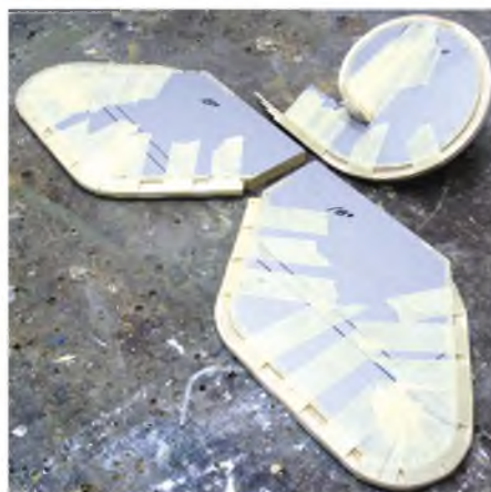
Here we see the tail surface outline laminations securely strapped to a substantial former.
