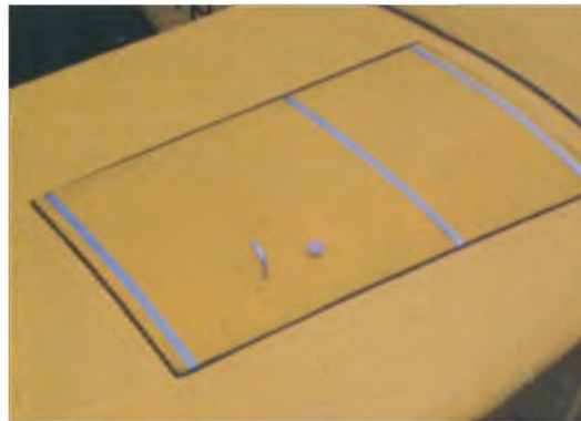
Further view of the dummy fuel tank access panels on the wing upper surface. Note the filler cap and vent.
