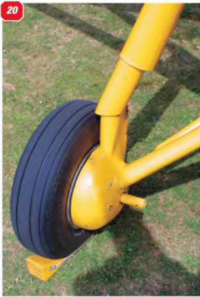
20 & 21: Two views showing the main undercarriage wheel and strut arrangement. 22: One of the main wheels seen from the opposite side. 23: View of the bottom of the fuselage, showing the mating and fairing of the wing strut and main undercarriage, where these attach to the fuselage. 24: Fairings over the wing strut attachment points.
