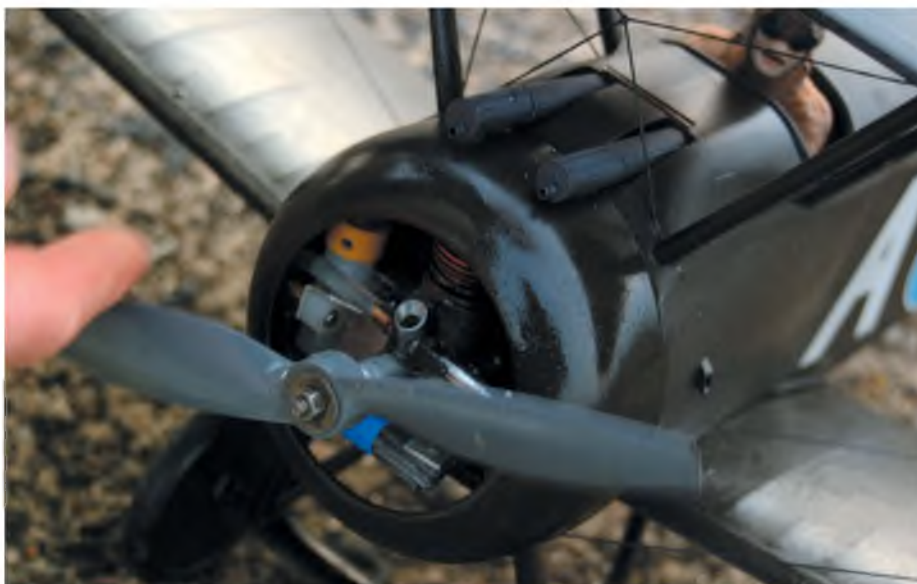
It's a short nose, so it's all crammed in the cowl! Charlie Newman's little Sopwith Camel cowl sports a 0.5cc DC Dart, fuel tank - and lead weight - and it fits!
