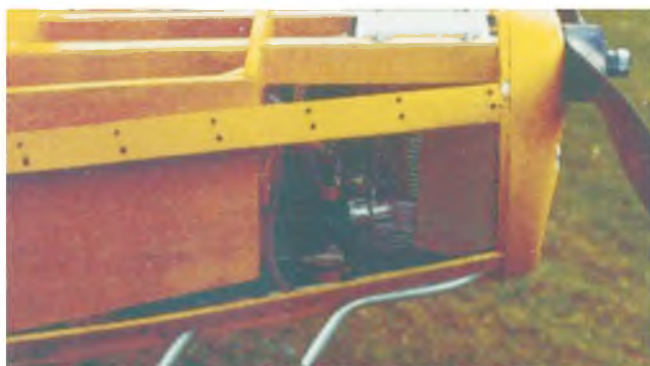
View of the inverted Laser 150 with the cowl panels removed.
