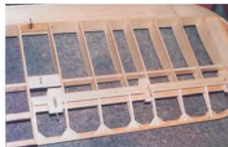
The wing before covering, showing the Robart hinges fitted in extension tubes.
