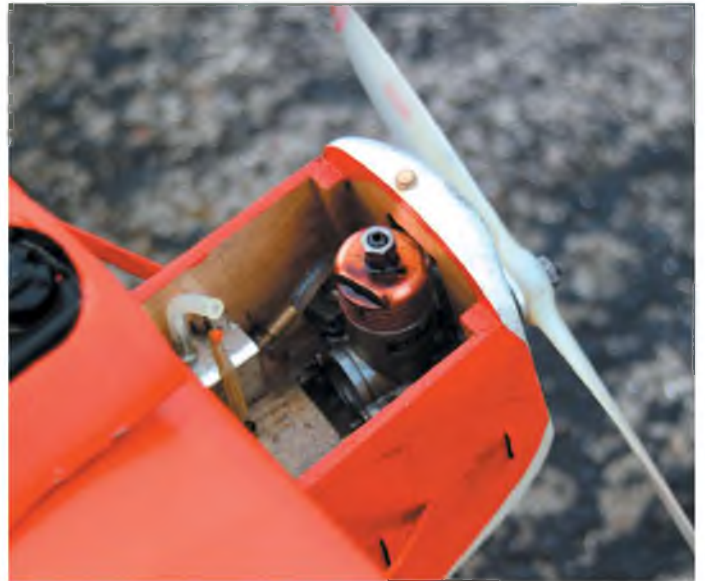
The Fokker D.VII offers a more straightforward approach. The upright DC Sabre has a modified Allen key comp screw - note short length of fuel tube!
