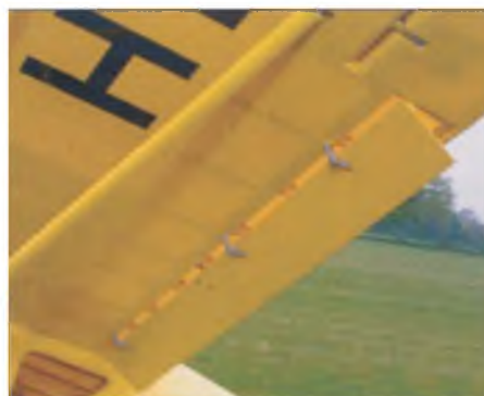
The wing flaps in the deployed position. Note Robert 'Hinge Point' hinges arranged to achieve the required action.
