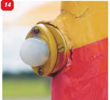
12: View of the elevator upper surface, again showing the trim tab which is hinged on the top surface. 13: View under the tailplane showing the mounting lugs that attach it to the fuselage. 14: Tail light on the rudder trailing edge. 15: The tail wheel unit. 16: The wing strut, where it fairs with the fuselage. 17: The wing strut-cum-undercarriage mount, viewed from the rear, is a complicated arrangement. 18: Foot step for access to the cabin. 19: Front view of the wing strut, showing the bare metal face plate around the leading edge.
