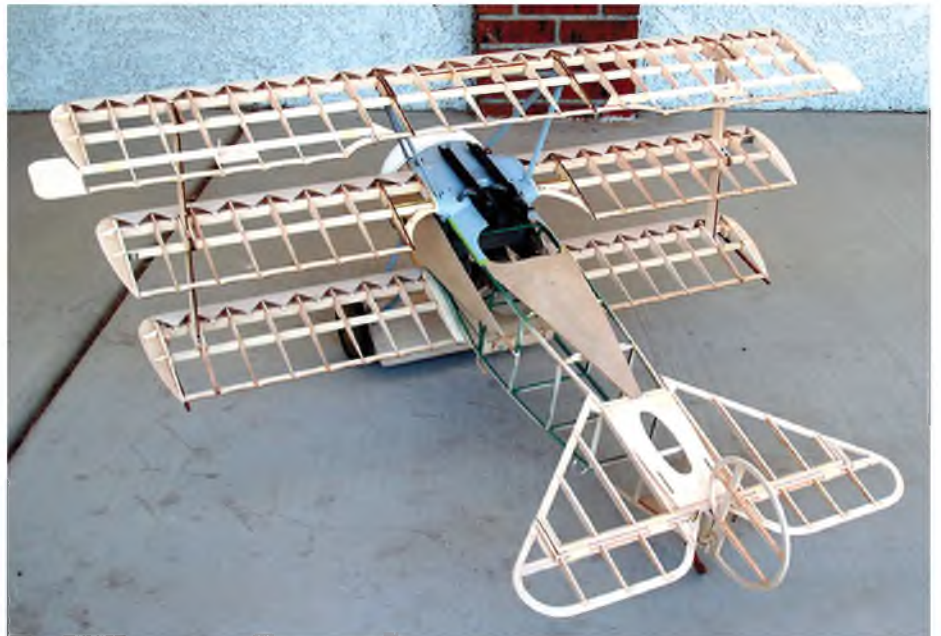
The intricate, but not overly complicated structure is evident here. Note Darrin's use of litho plate to form the cockpit decking and centre wing fairings.
