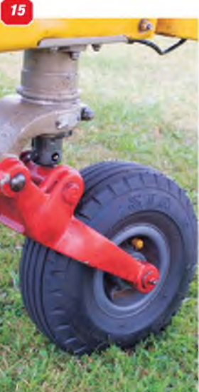
12: View of the elevator upper surface, again showing the trim tab which is hinged on the top surface. 13: View under the tailplane showing the mounting lugs that attach it to the fuselage. 14: Tail light on the rudder trailing edge. 15: The tail wheel unit. 16: The wing strut, where it fairs with the fuselage. 17: The wing strut-cum-undercarriage mount, viewed from the rear, is a complicated arrangement. 18: Foot step for access to the cabin. 19: Front view of the wing strut, showing the bare metal face plate around the leading edge.
