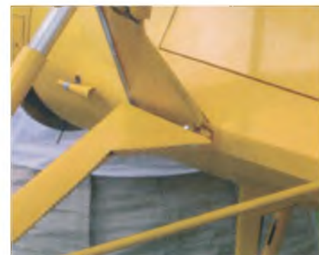
Close-up of the wing strut and main undercarriage anchor point on the fuselage.
