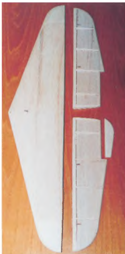
The tailplane and elevator prior to covering. Both are made up over a 1/16" balsa centre-line plate.
