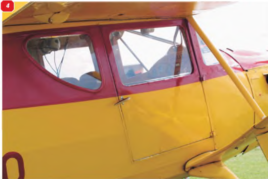
1: Nose section showing panel lines and air intakes. 2: Cabin door hinge and the fairing where the wing/undercarriage strut meets the fuselage. 3 & 4: Two views of the cabin area showing the line of the cabin access door and the window panelling.
