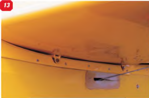
12: View of the elevator upper surface, again showing the trim tab which is hinged on the top surface. 13: View under the tailplane showing the mounting lugs that attach it to the fuselage. 14: Tail light on the rudder trailing edge. 15: The tail wheel unit. 16: The wing strut, where it fairs with the fuselage. 17: The wing strut-cum-undercarriage mount, viewed from the rear, is a complicated arrangement. 18: Foot step for access to the cabin. 19: Front view of the wing strut, showing the bare metal face plate around the leading edge.
