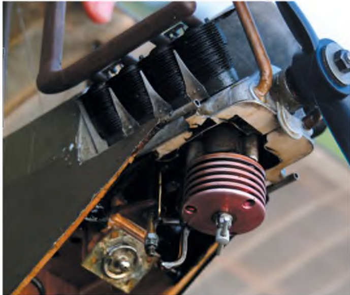
Another solution - an inverted mounting (Russian rear induction engine?), despite the large top 'scoop' cowl on Mike Kelsey's BE2. Note the press stud lower cowl mounting point.
