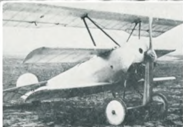
First of the line, the Fokker V.3 that served as the initial prototype. Lack of aerodynamic balance to the ailerons and elevators make the controls very heavy - not exactly what was wanted for the ultimate dog-fighter. Modifications quickly followed.
