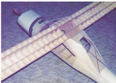
Fuselage nose section, showing the ply side plates, formers and engine bearers for sidewinder mounted engine.
