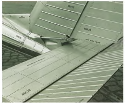
ABOVE: Wilga C tailcone showing the rivet lining and the fluted skin on the elevator.
