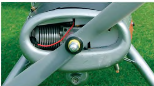
Engine cowl close-up, showing neat Laser 90 four-stroke installation.
