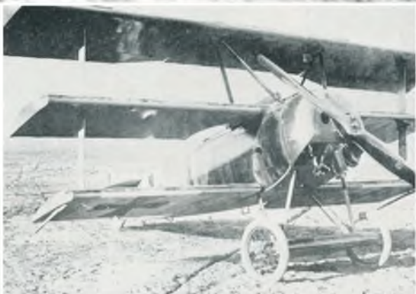
And here is the result - Fokker Dr.1 serial 141/17, the subject of official performance trials. The horn balance on the aileron can be clearly seen. Note also the protective wing tip skids
