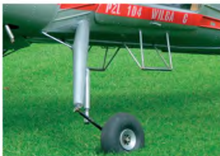
The 'knee-bend' undercarriage of the prototype model uses J.Perkins oleo units.
