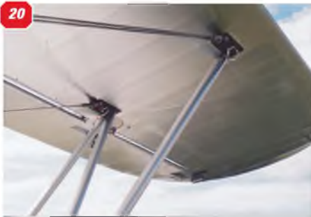
15: Another view of the cabane strut arrangement. Note the cuffs on the front strut. 16 & 17: Front and rear interplane struts on the right hand wing showing anchor points on upper wing underside and pitot head. 18 & 19: Two views of the interplane strut anchor points on the upper surface of the lower wing. 20: Further view of the interplane strut anchor points. 21: the complete cabane strut arrangement. 22 - 24: The sturdy main undercarriage, designed to absorb the rigors of carrier deck operations. 25: Inner face of the main undercarriage wheel and axle.
