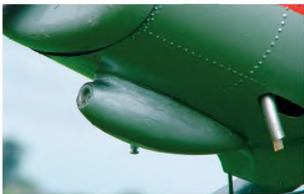
Engine cowl underside showing dummy air intake fairing
