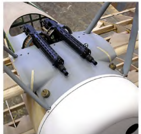
How the litho plate Darrin used fairs in the centre wing panels and rear c/s struts.
