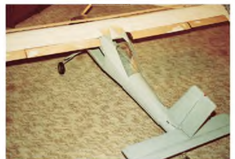
Trailing edge flaps and leading edge slats are very much a part of the character of this aircraft.
