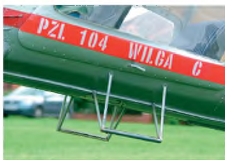
The mounting stirrups, for left and right side cockpit access are a prominent detail that should be replicated.
