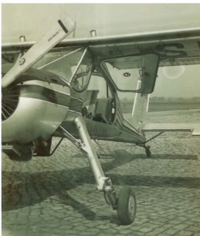
Two views showing the undercarriage of the Wilga 35. This arrangement permits operation from rough field sites.
