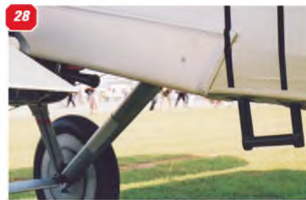
26: Unlike the right-hand side cabane struts, the left hand side struts have no cuff fairings. 27: Wing leading edge light close to the wing tip on top wing. 28: Cockpit mounting stirrup, left fuselage side behind wing trailing edge. 29 & 30: Details of lower wing root. 31: Tailplane/elevator, showing hinge line, hinge and control horn.
