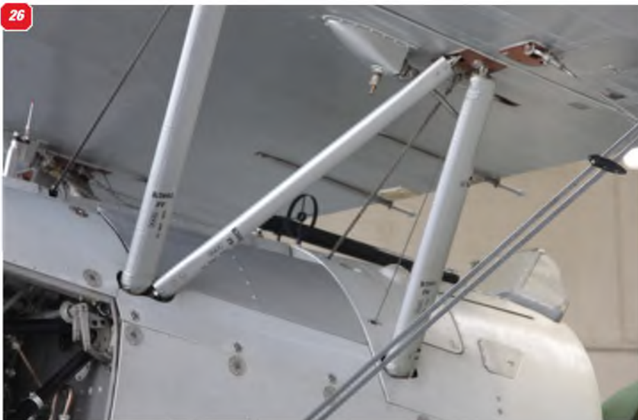
26: Unlike the right-hand side cabane struts, the left hand side struts have no cuff fairings. 27: Wing leading edge light close to the wing tip on top wing. 28: Cockpit mounting stirrup, left fuselage side behind wing trailing edge. 29 & 30: Details of lower wing root. 31: Tailplane/elevator, showing hinge line, hinge and control horn.
