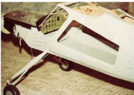
Here the fuselage is fully skinned and the instrument panel is in place. Important to add such detail in such a fully visible cockpit.
