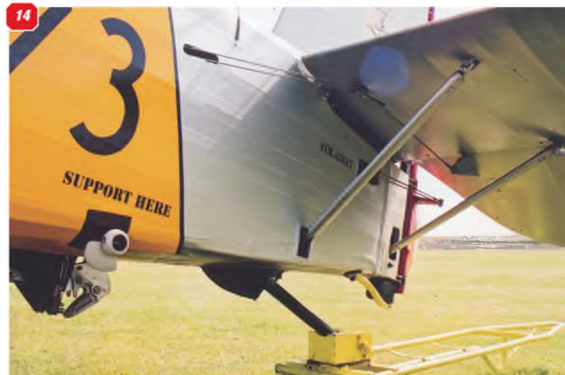
10: Detail of the oil cooler mounted on the engine cowl underside. 11: Exhaust stack along the fuselage side, and cabane struts. 12: Another view along the upper fuselage from rear to front, showing surface panel detail around the cockpit. 13: The arrestor hook. 14: Rear fuselage, showing the tailskid and tailplane bracing struts.
