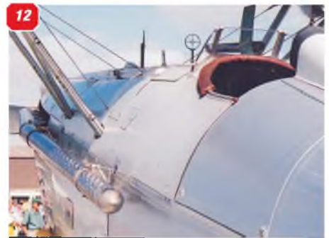
10: Detail of the oil cooler mounted on the engine cowl underside. 11: Exhaust stack along the fuselage side, and cabane struts. 12: Another view along the upper fuselage from rear to front, showing surface panel detail around the cockpit. 13: The arrestor hook. 14: Rear fuselage, showing the tailskid and tailplane bracing struts.
