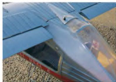
View of the cockpit rear screen. Note the X-shape braces.
