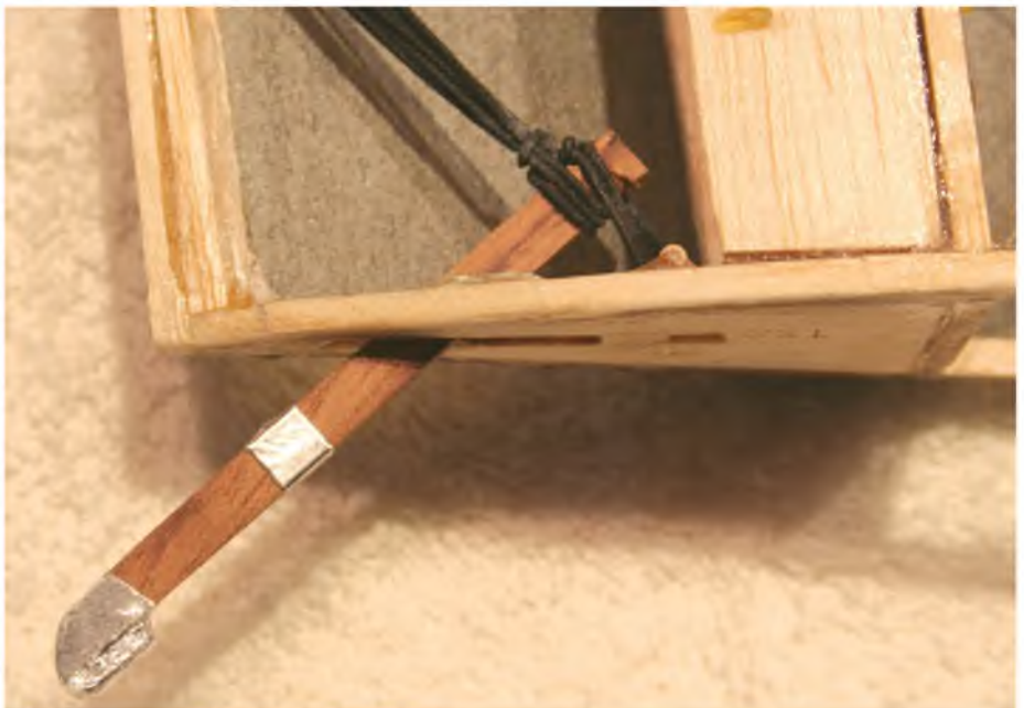
A nice hardwood skid and plenty of elastic cord suspension take the strain.
