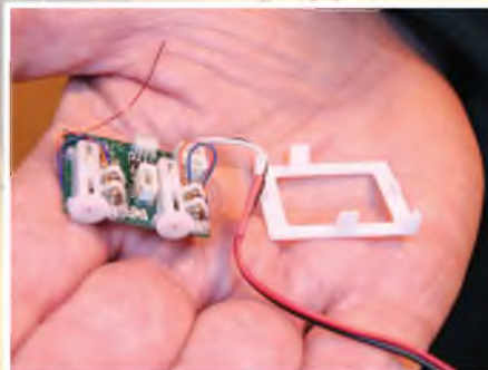
3D-printed radio clip. Secure your commercial radio gubbins to your scratch built model with one of these from Eric Stefford.
