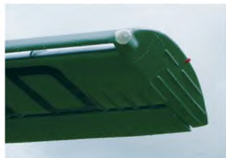
Wing tip, showing dummy light and strengthener flutes.
