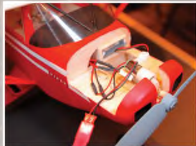
Geared electric motor in Richard Crossley's Piper Tripecer.
