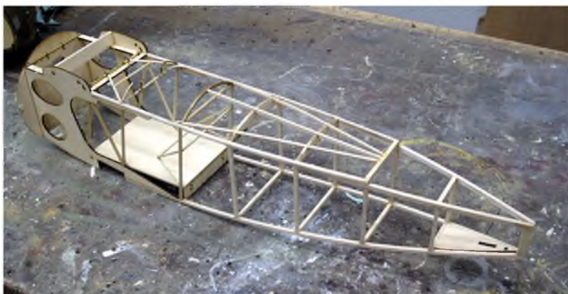
The basic fuselage with the outside of the longerons rounded to better represent tube.
