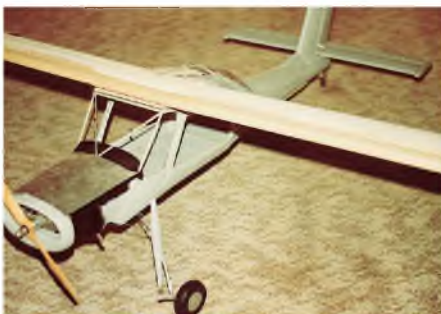
The basic airframe complete, with undercarriage in place.
