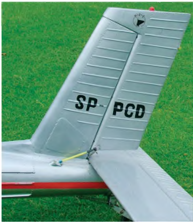
Detail showing the replication of the stiffener flutes pressed into the skin of the rudder, fin, tailplane and elevator. The 'snake' push rod to the rudder is actually quite accurate to full size, but really needs a lick of paint to replicate the metal of the full size machine.
