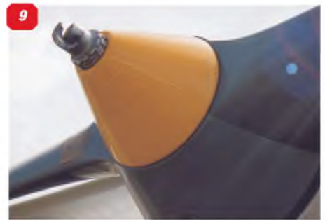
5: Engine cowl side panel removed to reveal Rolls Royce Kestrel engine. 6: The proverbial 'full-frontal', showing the nose profile, radiator, oil cooler. 7: Further view of the underside radiator and the undercarriage leg oleo. 8: Another view of the spinner and small air scoop. 9: Propeller spinner close-up showing the link for an external starter.
