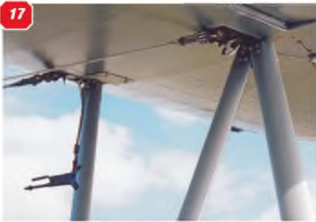
15: Another view of the cabane strut arrangement. Note the cuffs on the front strut. 16 & 17: Front and rear interplane struts on the right hand wing showing anchor points on upper wing underside and pitot head. 18 & 19: Two views of the interplane strut anchor points on the upper surface of the lower wing. 20: Further view of the interplane strut anchor points. 21: the complete cabane strut arrangement. 22 - 24: The sturdy main undercarriage, designed to absorb the rigors of carrier deck operations. 25: Inner face of the main undercarriage wheel and axle.
