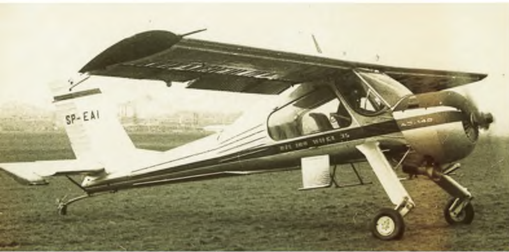
Two views of a Wilga 35, showing the pressed metal strengtheners on the rear fuselage. Note also the kicking plate on the right hand side boarding step. The tailwheel extends far further rearward than on the Wilga C.
