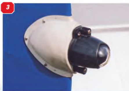
1: The cockpit area, showing cockpit coaming, windscreen, gun sight and headrest fairing. 2: Rudder mass balance and aerial mast. 3: Tail light on rudder trailing edge. 4: Fin/rudder hinge line showing fin-to-tailplane brace link and rudder hinge.
