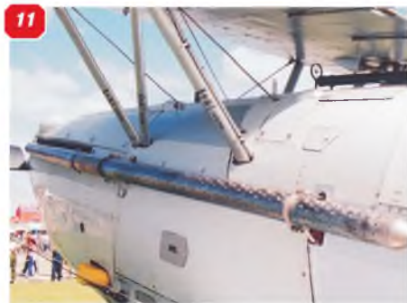
10: Detail of the oil cooler mounted on the engine cowl underside. 11: Exhaust stack along the fuselage side, and cabane struts. 12: Another view along the upper fuselage from rear to front, showing surface panel detail around the cockpit. 13: The arrestor hook. 14: Rear fuselage, showing the tailskid and tailplane bracing struts.
