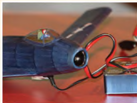
Derek Knight's new prototype 18mm Electric Ducted Fan unit.
