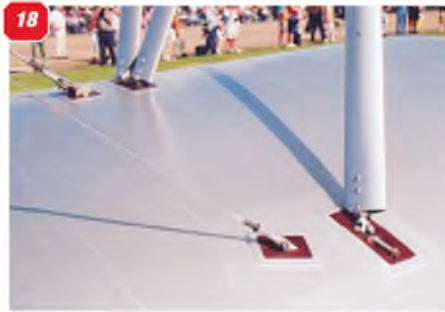
15: Another view of the cabane strut arrangement. Note the cuffs on the front strut. 16 & 17: Front and rear interplane struts on the right hand wing showing anchor points on upper wing underside and pitot head. 18 & 19: Two views of the interplane strut anchor points on the upper surface of the lower wing. 20: Further view of the interplane strut anchor points. 21: the complete cabane strut arrangement. 22 - 24: The sturdy main undercarriage, designed to absorb the rigors of carrier deck operations. 25: Inner face of the main undercarriage wheel and axle.
