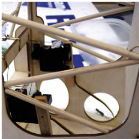
Aileron servo mounting and mock-up cables to aid positioning exit guides.
