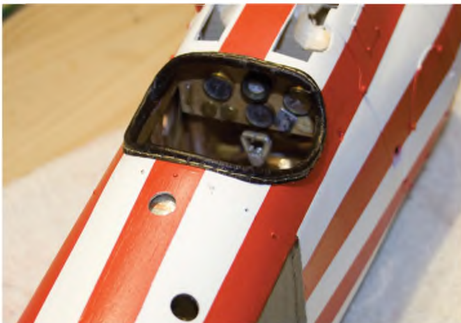
A piece of wire, some vinyl and a bit of thread results in a very realistic representation of the leather coaming used on the original.
