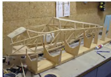
The fuselage removed to reveal the jig.
