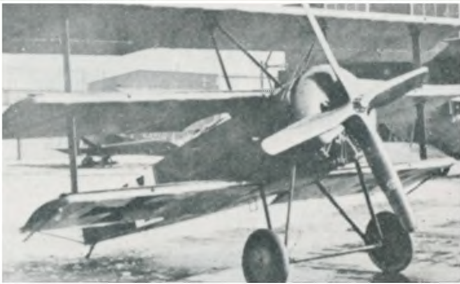
One of the attempts to improve performance of the Dr.I was the V.7 with Siemens-Halske Sh.III rotary engine and four-blade propeller.
