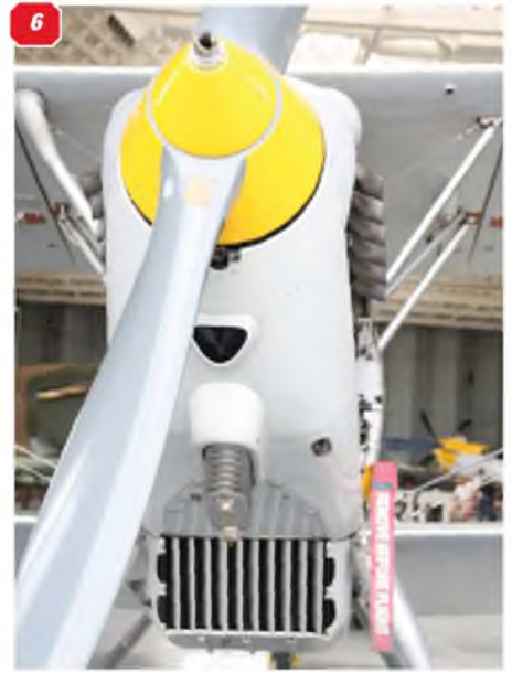
5: Engine cowl side panel removed to reveal Rolls Royce Kestrel engine. 6: The proverbial 'full-frontal', showing the nose profile, radiator, oil cooler. 7: Further view of the underside radiator and the undercarriage leg oleo. 8: Another view of the spinner and small air scoop. 9: Propeller spinner close-up showing the link for an external starter.
