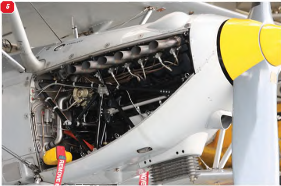
5: Engine cowl side panel removed to reveal Rolls Royce Kestrel engine. 6: The proverbial 'full-frontal', showing the nose profile, radiator, oil cooler. 7: Further view of the underside radiator and the undercarriage leg oleo. 8: Another view of the spinner and small air scoop. 9: Propeller spinner close-up showing the link for an external starter.
