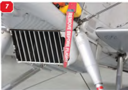
5: Engine cowl side panel removed to reveal Rolls Royce Kestrel engine. 6: The proverbial 'full-frontal', showing the nose profile, radiator, oil cooler. 7: Further view of the underside radiator and the undercarriage leg oleo. 8: Another view of the spinner and small air scoop. 9: Propeller spinner close-up showing the link for an external starter.
