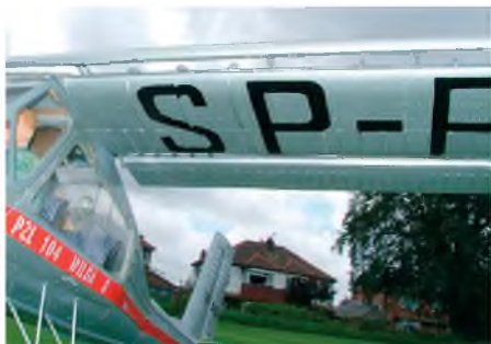
Distinctive Wilga rivet detail seen here on wing underside. PVA glue and talc delivered via hypodermic needle was the technique used.
