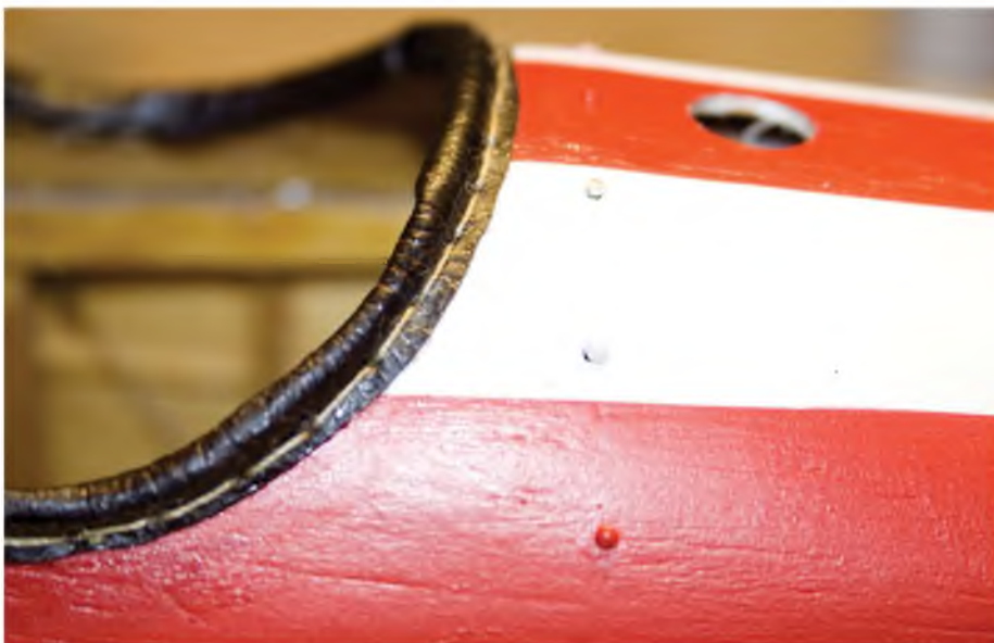
A closer look at the stitching. The wood grain on the rear decking is actually supposed to be there; it was ply on the full-size Camel.
