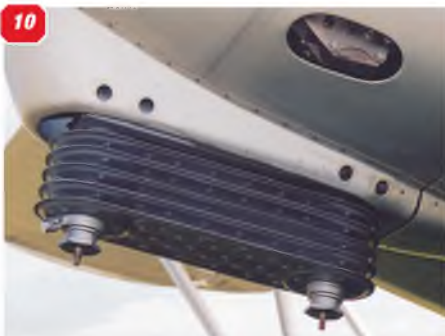
10: Detail of the oil cooler mounted on the engine cowl underside. 11: Exhaust stack along the fuselage side, and cabane struts. 12: Another view along the upper fuselage from rear to front, showing surface panel detail around the cockpit. 13: The arrestor hook. 14: Rear fuselage, showing the tailskid and tailplane bracing struts.
