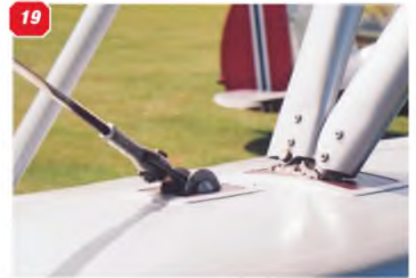
15: Another view of the cabane strut arrangement. Note the cuffs on the front strut. 16 & 17: Front and rear interplane struts on the right hand wing showing anchor points on upper wing underside and pitot head. 18 & 19: Two views of the interplane strut anchor points on the upper surface of the lower wing. 20: Further view of the interplane strut anchor points. 21: the complete cabane strut arrangement. 22 - 24: The sturdy main undercarriage, designed to absorb the rigors of carrier deck operations. 25: Inner face of the main undercarriage wheel and axle.
