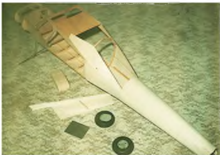
The basic fuselage structure, with the rear fuselage skinned.
