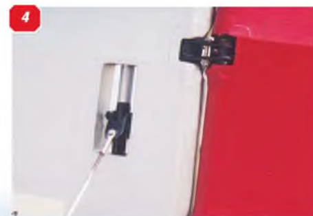
1: The cockpit area, showing cockpit coaming, windscreen, gun sight and headrest fairing. 2: Rudder mass balance and aerial mast. 3: Tail light on rudder trailing edge. 4: Fin/rudder hinge line showing fin-to-tailplane brace link and rudder hinge.
