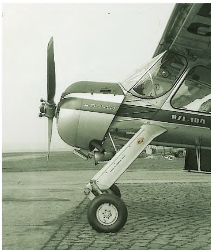
Two views showing the undercarriage of the Wilga 35. This arrangement permits operation from rough field sites.
