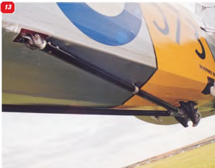
10: Detail of the oil cooler mounted on the engine cowl underside. 11: Exhaust stack along the fuselage side, and cabane struts. 12: Another view along the upper fuselage from rear to front, showing surface panel detail around the cockpit. 13: The arrestor hook. 14: Rear fuselage, showing the tailskid and tailplane bracing struts.
