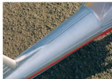
Detail of the rear fuselage, showing the dummy surface strengthener strakes that must be applied to capture the character of the aircraft.
