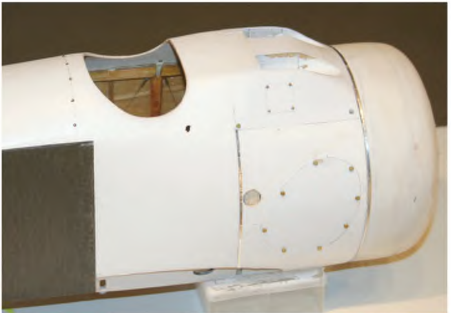
With the forward fuselage primed and detailed, the basic cockpit opening is ready to receive some padding.
