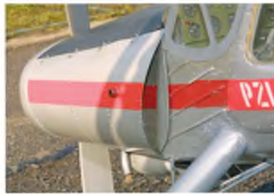
Rear of the engine cowl showing air exit.
