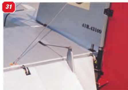
26: Unlike the right-hand side cabane struts, the left hand side struts have no cuff fairings. 27: Wing leading edge light close to the wing tip on top wing. 28: Cockpit mounting stirrup, left fuselage side behind wing trailing edge. 29 & 30: Details of lower wing root. 31: Tailplane/elevator, showing hinge line, hinge and control horn.
