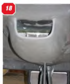
14: General view of the fuselage nose section, showing engine cowl panel lines. 15: Nose section close-up, showing the flash-damper exhaust stack as applied to night fighter aircraft. 16: Spinner and propeller. 17 & 18: Two views of the air scoop on the cowl underside, just ahead of the wing. 19 & 20: Two further views of the night fighter style damper exhaust stacks. 21: Wing, showing the metal strip covering the inner/outer panel joint. 22: The aileron, showing the hinge positions. 23: Wing root underside, showing the inner undercarriage doors. 24: Wing tip light, starboard side. 25: Wing-to-fuselage fairing. 26: Pilot head, Port wing. 27: Landing light, applied to both wings. 28: Forward section of the wing-to-fuselage fairing.
