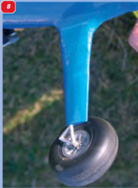
7 & 8: The undercarriage fairing are balsa. To allow the wire to flex without breaking the fairings, a 1cm layer of EPP foam was introduced between the upper fairings and the trouser part, the latter being fixed to the wire with silicone to provide some 'give'. Masking tape over this provided a smooth base for the Profilm covering later. 9: The mainwheel. The Dummy drag link is simply a piece of aluminium tube, appropriately shaped.
