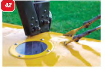
36 & 37: Wing strut and bracing wire anchor points, on upper wing lower surface. 38: Full view of the interplane strut, starboard side. 39: Pitot head on port interplane strut. 40: Wooden bracing wire spacer between upper and lower wings. 41: Anchor point for rear inter plane strut at lower wing trailingedge. 42: Leading edge lower wing strut anchor point. 43: Detail of bracing wire anchor on tailplane underside. 44 & 45: Linkage to the elevator trim tab, top and bottom. It is hinged on the surface. 46 & 47: Close up of elevator hinges. 48: Elevator detail.
