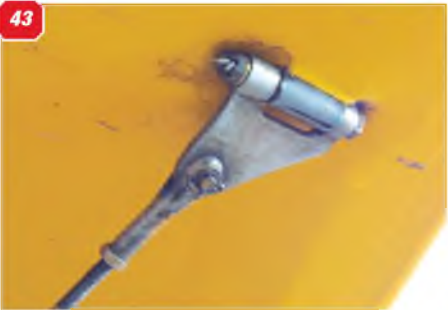
36 & 37: Wing strut and bracing wire anchor points, on upper wing lower surface. 38: Full view of the interplane strut, starboard side. 39: Pitot head on port interplane strut. 40: Wooden bracing wire spacer between upper and lower wings. 41: Anchor point for rear inter plane strut at lower wing trailingedge. 42: Leading edge lower wing strut anchor point. 43: Detail of bracing wire anchor on tailplane underside. 44 & 45: Linkage to the elevator trim tab, top and bottom. It is hinged on the surface. 46 & 47: Close up of elevator hinges. 48: Elevator detail.
