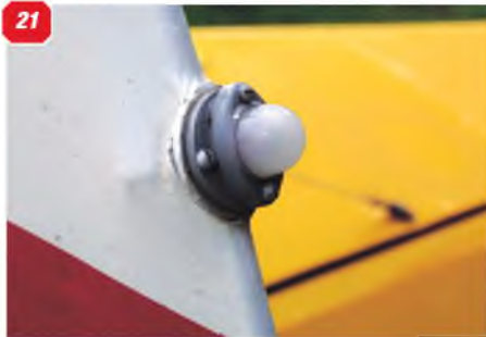
18: Rudder aerodynamic balance and the anchor points for wire braces. 19: Annotation at foot of rudder. 20: Detail of bracing wire anchor point at tailpost. 21: Tail light on rudder. 22: Bracing wire anchor point at fin leading edge. 23: View from rear showing the rudder control horn, angled down 45 degrees. 24: Access hatch on lowering wing. 25: Rear strut anchor, lower wing. 26 & 27: Lower wing undersides showing aileron in up and down positions. 28: Front strut anchor point, lower wing. 29: Hand grip upper wing centre section. 30: Wing tip hand grip, lower wing.
