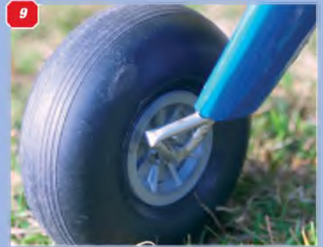
7 & 8: The undercarriage fairing are balsa. To allow the wire to flex without breaking the fairings, a 1cm layer of EPP foam was introduced between the upper fairings and the trouser part, the latter being fixed to the wire with silicone to provide some 'give'. Masking tape over this provided a smooth base for the Profilm covering later. 9: The mainwheel. The Dummy drag link is simply a piece of aluminium tube, appropriately shaped.
