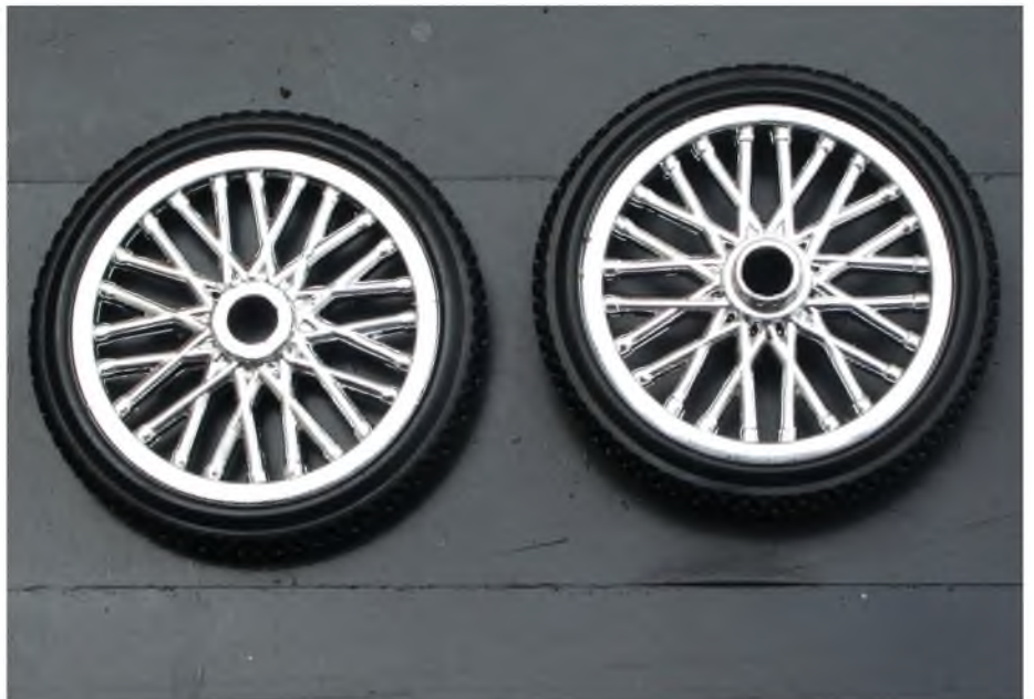
The 'spoked' wheels, stolen from a toy cycle, are reasonably light and much stronger than more expensive model wheels.
