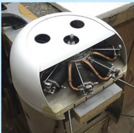
Here you can see how the vac-formed cowl Darrin used fits around the very realistic looking dummy engine. An all-wood cowl is a perfectly feasible alternative.
