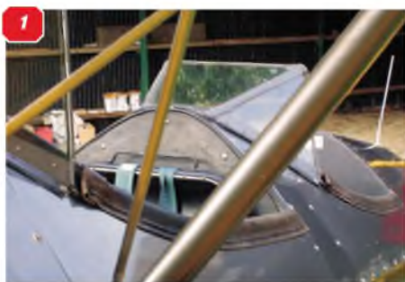
1 & 2: Cockpits showing windscreens and leather coaming. 3: Mirror under wing centre section.
