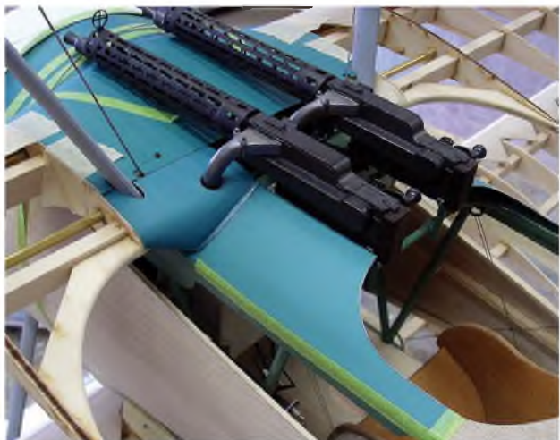
Test fitting the litho plate parts on the temporarily assembled structure. Note how the alleron cables exit.
