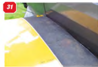
31: Wing-walk panel for cockpit access. Lower portside wing root. Starboard is similar. 32: The anchor points for wing bracing wires at lower wing root. 33 & 34: Two views off the uncowled, nine cylinder engine. 35: Close-up of the propeller hub.
