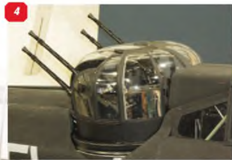
1 - 5: The major feature of the Boulton Paul Defiant centres in the cockpit and the rotating gun turret behind it. 6-8: Enlarged views of the cockpit and gun turret. The upper part of the fairing between the cockpit and the turret retracts to allow a forward field of fire for the gunner. 9: View of the rear upper fuselage behind the turret showing retracting panel behind the turret, seen here in the retracted position. 10: General view of the tailcone. 11: Tailplane tip, showing the aerodynamic balance. 12: The fin and rudder, showing the aerodynamic balance. 13: Tailplane-to-fuselage root, showing the metal cuff fairing. Note also the control link to the rudder control horn.
