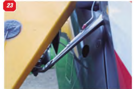
18: Rudder aerodynamic balance and the anchor points for wire braces. 19: Annotation at foot of rudder. 20: Detail of bracing wire anchor point at tailpost. 21: Tail light on rudder. 22: Bracing wire anchor point at fin leading edge. 23: View from rear showing the rudder control horn, angled down 45 degrees. 24: Access hatch on lowering wing. 25: Rear strut anchor, lower wing. 26 & 27: Lower wing undersides showing aileron in up and down positions. 28: Front strut anchor point, lower wing. 29: Hand grip upper wing centre section. 30: Wing tip hand grip, lower wing.
