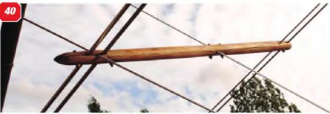
36 & 37: Wing strut and bracing wire anchor points, on upper wing lower surface. 38: Full view of the interplane strut, starboard side. 39: Pitot head on port interplane strut. 40: Wooden bracing wire spacer between upper and lower wings. 41: Anchor point for rear inter plane strut at lower wing trailingedge. 42: Leading edge lower wing strut anchor point. 43: Detail of bracing wire anchor on tailplane underside. 44 & 45: Linkage to the elevator trim tab, top and bottom. It is hinged on the surface. 46 & 47: Close up of elevator hinges. 48: Elevator detail.
