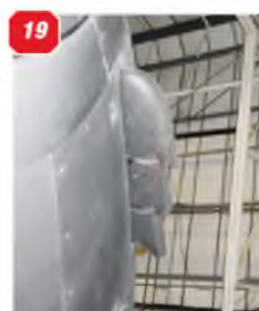
14: General view of the fuselage nose section, showing engine cowl panel lines. 15: Nose section close-up, showing the flash-damper exhaust stack as applied to night fighter aircraft. 16: Spinner and propeller. 17 & 18: Two views of the air scoop on the cowl underside, just ahead of the wing. 19 & 20: Two further views of the night fighter style damper exhaust stacks. 21: Wing, showing the metal strip covering the inner/outer panel joint. 22: The aileron, showing the hinge positions. 23: Wing root underside, showing the inner undercarriage doors. 24: Wing tip light, starboard side. 25: Wing-to-fuselage fairing. 26: Pilot head, Port wing. 27: Landing light, applied to both wings. 28: Forward section of the wing-to-fuselage fairing.
