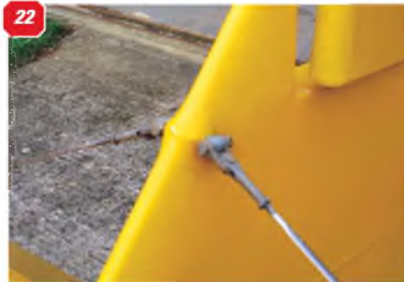
18: Rudder aerodynamic balance and the anchor points for wire braces. 19: Annotation at foot of rudder. 20: Detail of bracing wire anchor point at tailpost. 21: Tail light on rudder. 22: Bracing wire anchor point at fin leading edge. 23: View from rear showing the rudder control horn, angled down 45 degrees. 24: Access hatch on lowering wing. 25: Rear strut anchor, lower wing. 26 & 27: Lower wing undersides showing aileron in up and down positions. 28: Front strut anchor point, lower wing. 29: Hand grip upper wing centre section. 30: Wing tip hand grip, lower wing.
