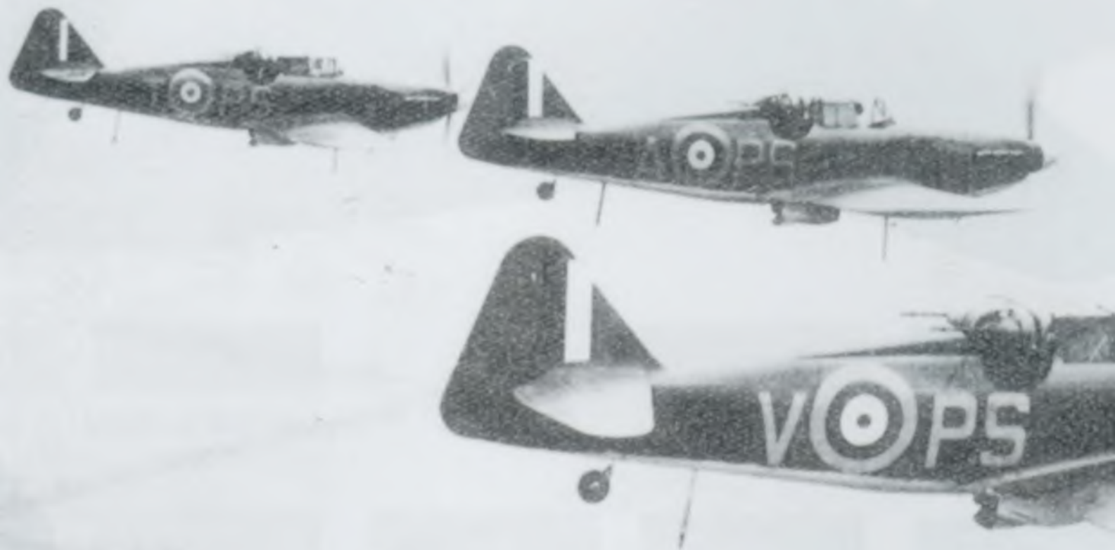
A formation of three Defiant Mk.1s of No.264 Squadron, 1940. The object dangling below the rear fuselage ahead of the tailwheel on each aircraft is an aerial.
