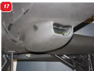
14: General view of the fuselage nose section, showing engine cowl panel lines. 15: Nose section close-up, showing the flash-damper exhaust stack as applied to night fighter aircraft. 16: Spinner and propeller. 17 & 18: Two views of the air scoop on the cowl underside, just ahead of the wing. 19 & 20: Two further views of the night fighter style damper exhaust stacks. 21: Wing, showing the metal strip covering the inner/outer panel joint. 22: The aileron, showing the hinge positions. 23: Wing root underside, showing the inner undercarriage doors. 24: Wing tip light, starboard side. 25: Wing-to-fuselage fairing. 26: Pilot head, Port wing. 27: Landing light, applied to both wings. 28: Forward section of the wing-to-fuselage fairing.
