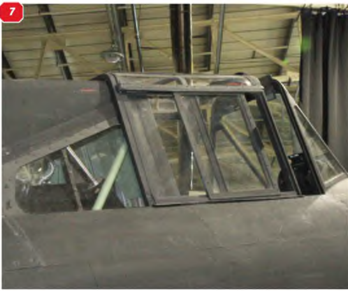
1 - 5: The major feature of the Boulton Paul Defiant centres in the cockpit and the rotating gun turret behind it. 6-8: Enlarged views of the cockpit and gun turret. The upper part of the fairing between the cockpit and the turret retracts to allow a forward field of fire for the gunner. 9: View of the rear upper fuselage behind the turret showing retracting panel behind the turret, seen here in the retracted position. 10: General view of the tailcone. 11: Tailplane tip, showing the aerodynamic balance. 12: The fin and rudder, showing the aerodynamic balance. 13: Tailplane-to-fuselage root, showing the metal cuff fairing. Note also the control link to the rudder control horn.
