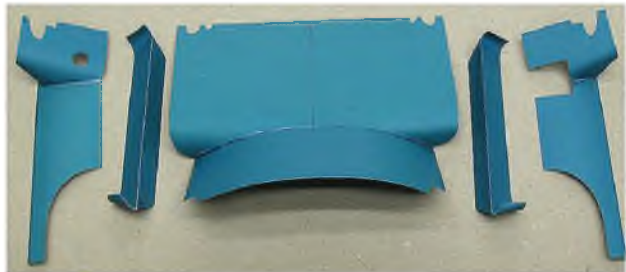
The litho plate panels Darrin made up to fair around the middle wings after the basic assembly was completed.
