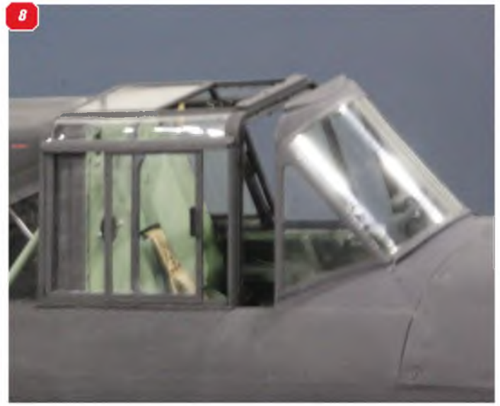
1 - 5: The major feature of the Boulton Paul Defiant centres in the cockpit and the rotating gun turret behind it. 6-8: Enlarged views of the cockpit and gun turret. The upper part of the fairing between the cockpit and the turret retracts to allow a forward field of fire for the gunner. 9: View of the rear upper fuselage behind the turret showing retracting panel behind the turret, seen here in the retracted position. 10: General view of the tailcone. 11: Tailplane tip, showing the aerodynamic balance. 12: The fin and rudder, showing the aerodynamic balance. 13: Tailplane-to-fuselage root, showing the metal cuff fairing. Note also the control link to the rudder control horn.
