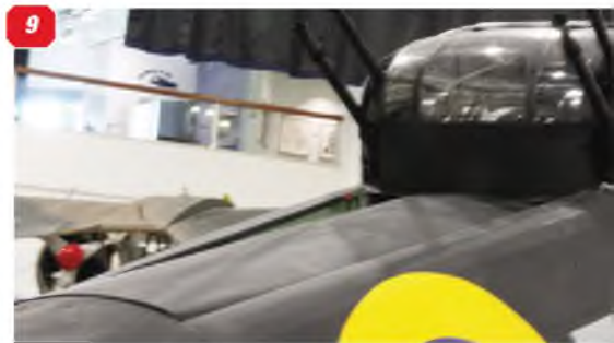
1 - 5: The major feature of the Boulton Paul Defiant centres in the cockpit and the rotating gun turret behind it. 6-8: Enlarged views of the cockpit and gun turret. The upper part of the fairing between the cockpit and the turret retracts to allow a forward field of fire for the gunner. 9: View of the rear upper fuselage behind the turret showing retracting panel behind the turret, seen here in the retracted position. 10: General view of the tailcone. 11: Tailplane tip, showing the aerodynamic balance. 12: The fin and rudder, showing the aerodynamic balance. 13: Tailplane-to-fuselage root, showing the metal cuff fairing. Note also the control link to the rudder control horn.
