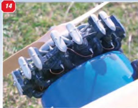
12: Radio and battery pack installation in the fuselage. The wing seat has a generous width. 13 & 14: Two views of the finished dummy engine. The PT-13 used a Lycoming radial, but the Wright radial replica represented by the Williams Bros kit can be translated into the shape of the Lycoming. 15: View of the twin cockpits showing the simplified dummy instrument panels. 16: Close-up of the pilot figure in the front cockpit. 17 & 18: Two further views of the cockpit area. The windshields were cut and folded from clear acetate Report covers.
