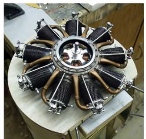
The centre of the Williams Bros. engine was removed to allow clearance, and cooling, for the motor.
