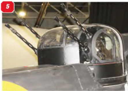
1 - 5: The major feature of the Boulton Paul Defiant centres in the cockpit and the rotating gun turret behind it. 6-8: Enlarged views of the cockpit and gun turret. The upper part of the fairing between the cockpit and the turret retracts to allow a forward field of fire for the gunner. 9: View of the rear upper fuselage behind the turret showing retracting panel behind the turret, seen here in the retracted position. 10: General view of the tailcone. 11: Tailplane tip, showing the aerodynamic balance. 12: The fin and rudder, showing the aerodynamic balance. 13: Tailplane-to-fuselage root, showing the metal cuff fairing. Note also the control link to the rudder control horn.
