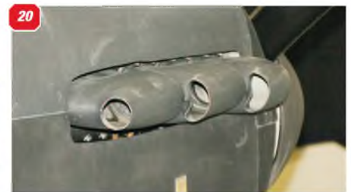
14: General view of the fuselage nose section, showing engine cowl panel lines. 15: Nose section close-up, showing the flash-damper exhaust stack as applied to night fighter aircraft. 16: Spinner and propeller. 17 & 18: Two views of the air scoop on the cowl underside, just ahead of the wing. 19 & 20: Two further views of the night fighter style damper exhaust stacks. 21: Wing, showing the metal strip covering the inner/outer panel joint. 22: The aileron, showing the hinge positions. 23: Wing root underside, showing the inner undercarriage doors. 24: Wing tip light, starboard side. 25: Wing-to-fuselage fairing. 26: Pilot head, Port wing. 27: Landing light, applied to both wings. 28: Forward section of the wing-to-fuselage fairing.
