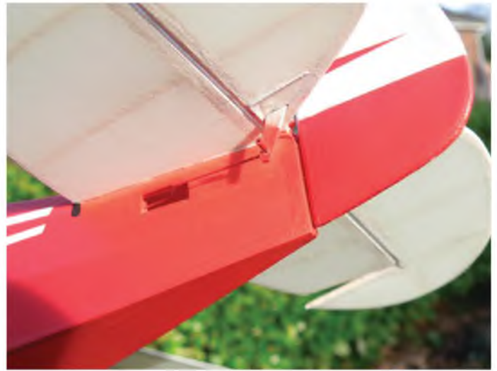
The control horns are made from 1/64" ply sheet. The end of the wire pushrod is simply held in place with sleeving cut from fine electrical wire, fixed with a tiny dot of cyano
