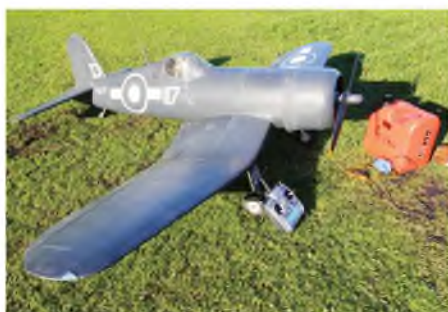
Ozyray Peters' 101" span Meister Corsair in Fleet Air Arm colours. Tony Clark custom can exhaust on the Zenoch 80 petrol engine.
