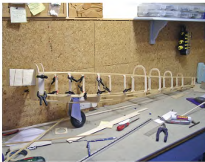
Basic fuselage structure before being braced up in a jig.
