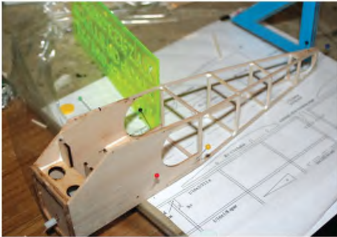
With the second side added the longerons are cracked, the tail pulled in and cross braces fitted.
