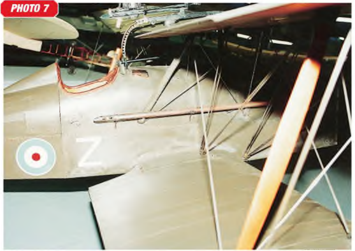
PHOTO 6: Fittings on the Bleriot XIV, photographed at the Musee de l'Air in Paris during writer's visit BACK in 1996, are massive by any standards, and seem to be of British design, if not manufacture. The bracing is of RAF wire outboard, and inboard of this inner strut pair the bracing is wire rod about 6 mm diameter. PHOTO 7: Typical British 'Factory' practice is this SE5a, with RAF wire wing bracing throughout. Note that the 'vibration preventers' are missing.
