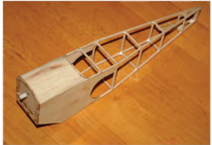
Once the decking is added it's time for some sanding - followed by a final reinforcing of glue joints.
