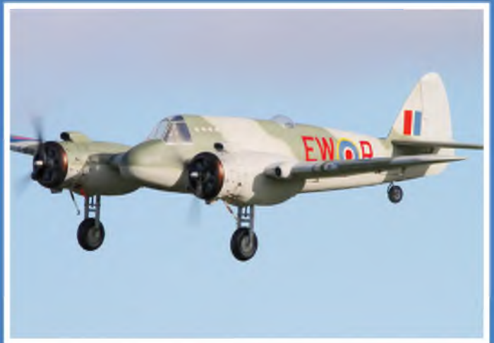
Barry Sherborne's Beaufighter Mk VI F. Twin ASP 61 FS power driving two 12"x 6" (3-blade) Master Airscrews.
