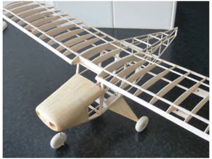
Wings employ a scale rib spacing and slightly increased dihedral. The strut anchor plates are from light 1/16" sheet balsa. This picture was taken before I cut out the cowl hatch.
