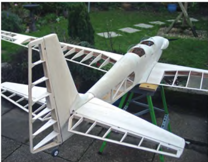
Basic structure, ready for covering.
