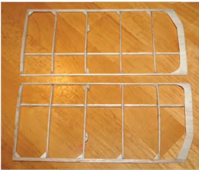
The wings are easy to build but if your ribs are soft you'll need to reinforce them with gussets at the thinnest point.
