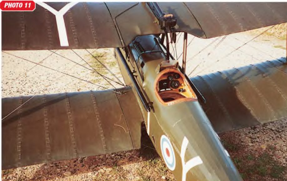
PHOTO 11: The author's SE5a is rigged throughout with .032" piano wire, but with single landing wires and duplicated flying wires. Note the wire vibration dampers, made from small pieces of tin-plate soldered to the flying wires. Note also the rear flying wires passing through a slot in the bottom stub wing. Wire tensioners are installed inside the fuselage. This 1/5th scale model is available as an MAP plan.
