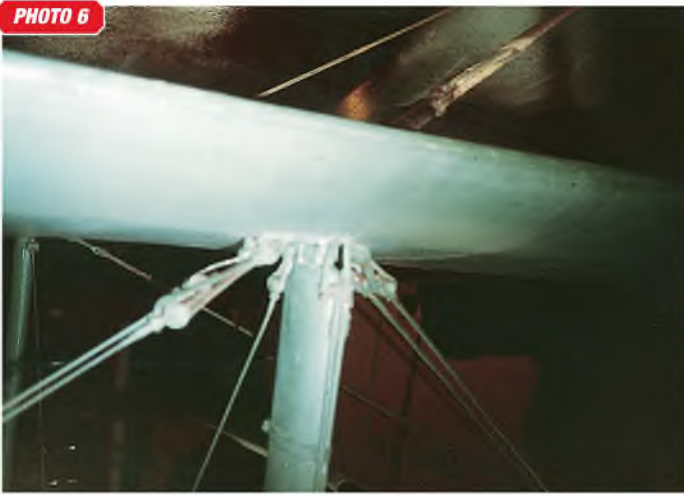
PHOTO 6: Fittings on the Bleriot XIV, photographed at the Musee de l'Air in Paris during writer's visit BACK in 1996, are massive by any standards, and seem to be of British design, if not manufacture. The bracing is of RAF wire outboard, and inboard of this inner strut pair the bracing is wire rod about 6 mm diameter. PHOTO 7: Typical British 'Factory' practice is this SE5a, with RAF wire wing bracing throughout. Note that the 'vibration preventers' are missing.
