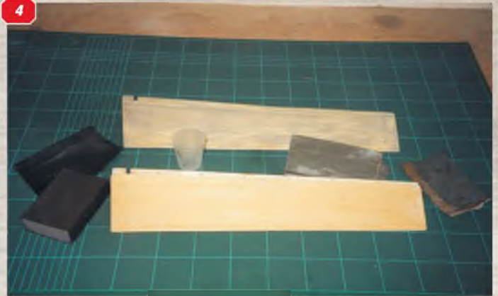
1: The basic materials. Andy used a combination of g/f supplies from Fibretech and Chemie-Technique. 2: Wing covering starts by cutting a piece of lightweight glass cloth to size, allowing a rough overlap which is sanded clear when the first resin coat has been applied. 3: Far left: Use an old credit card to scrape the resin through the cloth and into the balsa, working from the centreline of the panel towards leading- and trailing-edges. 4: Sanding. The initial material removal was by sponge sanding blocks, then Andy used a progression of grades of wet-and-dry paper for final finishing.
