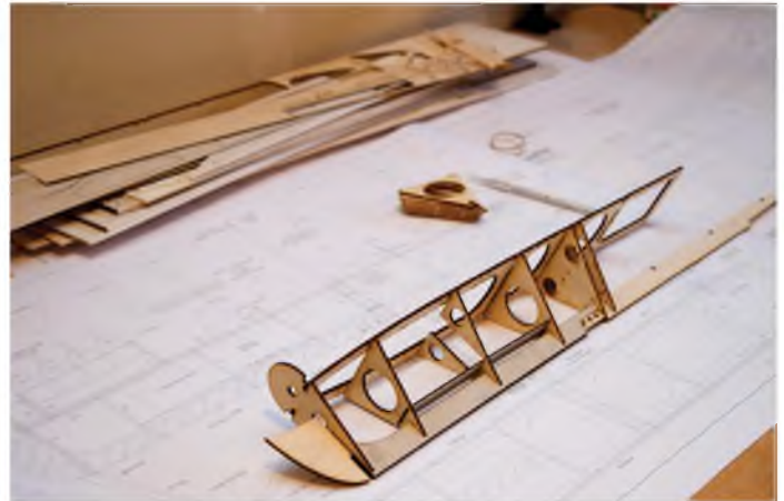
The front end keys together nicely to form a very sturdy assembly.
