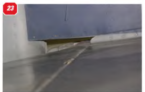
18 & 19: Two views of the rudder control horn and control rod. 20: The unusually shaped rudder trim tab. 21: Rudder trim tab control horn and fairing. 22: Tail light at base of rudder. 23: Free-to-air void at the fin/tailplane base (at the elevator hinge line). 24: Tailplane, showing the aerodynamic balance at the tip. 25: Twin elevator trim tabs, right elevator. 26: Trim tab close-up, right elevator. 27: Counterweighted inner tab, right hand elevator. 28: Single trim tab, left elevator. 29: Camera gun port at right wing root. 30: Twin 20mm cannon, wing leading edge. 31: Pitot head, left wing underside. 32: Wing tip light. 33: Fuselage centre section, showing shape of the big wing-to-fuselage fairing.
