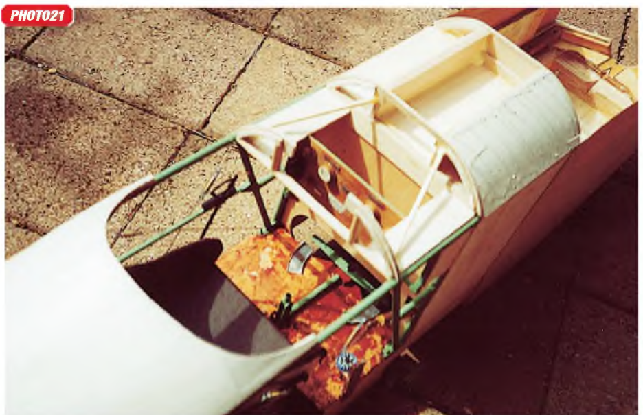
PHOTO 21: Functioning control column on author's Fokker D.7 drives elevator cables only. The 'torque tube' forward of this is a dummy from scrap dowel. Rudder bar is functional but not scale, as the original was a steel tube weldment. Note working compass at right. The 'throttle' on the left side switches on the Rx.
