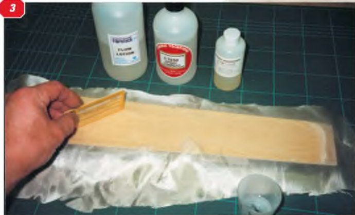
1: The basic materials. Andy used a combination of g/f supplies from Fibretech and Chemie-Technique. 2: Wing covering starts by cutting a piece of lightweight glass cloth to size, allowing a rough overlap which is sanded clear when the first resin coat has been applied. 3: Far left: Use an old credit card to scrape the resin through the cloth and into the balsa, working from the centreline of the panel towards leading- and trailing-edges. 4: Sanding. The initial material removal was by sponge sanding blocks, then Andy used a progression of grades of wet-and-dry paper for final finishing.
