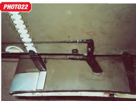
PHOTO 22: The external elevator cables on the Bristol F2B Fighter are 90lb. nylon-covered fishing trace, attaching to the external horn with 2.56 quick-links. Even at 1/4 scale these are a little too large for scale attachments. PHOTO 23: Leading edge protective rubbing strip on the 1/4 scale Brisfit showing wear from contact with an elevator cable. With the model tailplane set at zero incidence the 'up' cable changes direction by one or two degrees. The full-sized aircraft had an adjustable tailplane which could be set several degrees either way, so the contact may have been more severe with the tailplane adjusted up. PHOTO 24: Rudder horn on the Brisfit is typical of all, with an end fitting to move the cable attachment point forward to line up with the rudder hinge. On the model the rudder horn is 0.040" dural, with a 'U'-shaped end fitting from 0.020" steel sheet. An 8BA bolt attaches the rudder cable. Rear bracing is 0.032" wire passing through an aluminium tube epoxied into the rudder and then attached to the other side of the horn.
