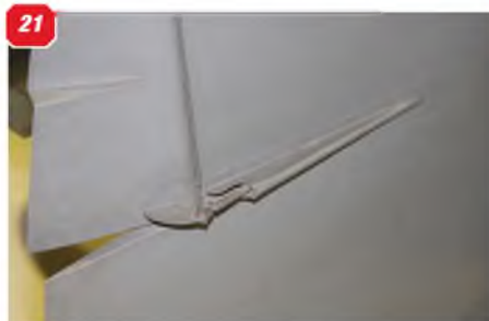
18 & 19: Two views of the rudder control horn and control rod. 20: The unusually shaped rudder trim tab. 21: Rudder trim tab control horn and fairing. 22: Tail light at base of rudder. 23: Free-to-air void at the fin/tailplane base (at the elevator hinge line). 24: Tailplane, showing the aerodynamic balance at the tip. 25: Twin elevator trim tabs, right elevator. 26: Trim tab close-up, right elevator. 27: Counterweighted inner tab, right hand elevator. 28: Single trim tab, left elevator. 29: Camera gun port at right wing root. 30: Twin 20mm cannon, wing leading edge. 31: Pitot head, left wing underside. 32: Wing tip light. 33: Fuselage centre section, showing shape of the big wing-to-fuselage fairing.
