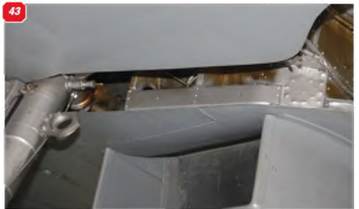
34-39: The Spitfire Mk.24 wing upper surfaces are festooned with with blister fairing over various internals that don't quite fit into the thin wing profile! 40: Rear of underwing radiator. 41: Radiator viewed from front. 42 & 43: the undercarriage well, wing underside. 44 & 45: Fixed spent ammo deflector, on wing underside. 46: Wing underside showing the inward folding wheel well cover. 47: Same, view from rear 48: Dished inner surface of wheel well cover. 49 & 50: Two views of the main undercarriage leg cover.
