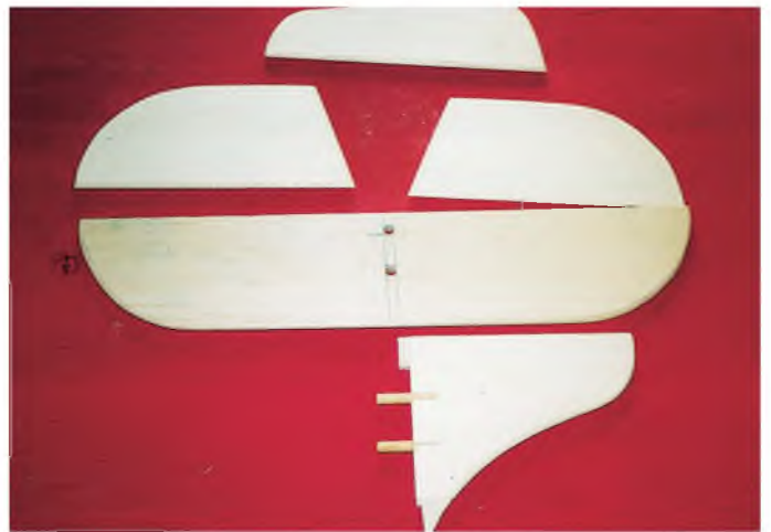
Tailplane parts showing the dowel. DO NOT leave these out.
