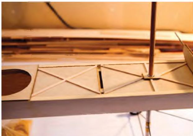
Here you see the false structure on the ply top fuselage plates, and the way the pylon is let into the main u/c tube.
