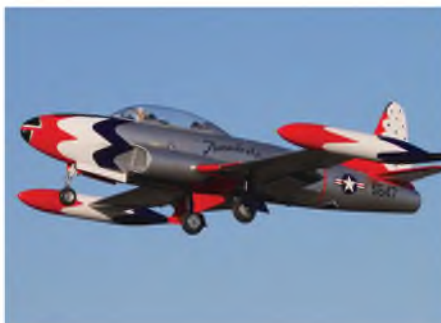
Mick Burrell's Lockheed T-33 Shooting Star in Thunderbirds livery. 105" span, weighs 39 lbs, Merlin 160 power.
