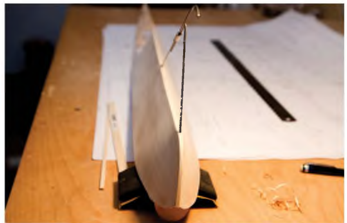
Barry did a really tidy job of skinning the forward sides and capping around the keel parts. Note how early you need to fit some of the u/c wires.
