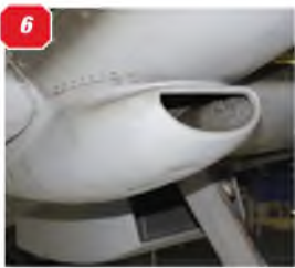
5: Massive bearers for the Rolls Royce Griffon engine. Note the six exhaust stacks 6 & 7: Two views of the carburettor air intake on the fuselage underside ahead of the wing root. 8: Further detail of the engine exhaust, left hand side. 9: Front cockpit side panels and windscreen. 10 & 11: Rear bubble canopy. 12 - 14: The retracting tailwheel and fairing doors.
