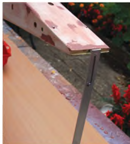
Here's something worth considering. This simple jig with attachment points either end of the fuselage allows the fus. to be rotated during the operation, leaving both hands free for the work in hand.
