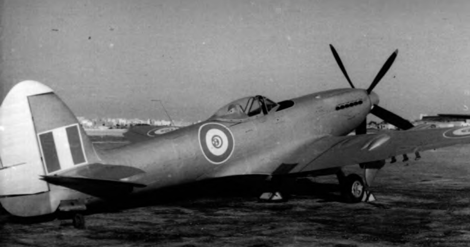
One of the Royal Egyptian Air Force F Mk 22s that staged through Luqa, Malta, showing some wing marking details, such as the non-slip walkway and the position of the national markings (Malta Aviation Museum Foundation)
