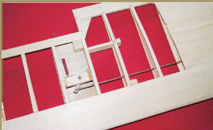
Aileron bellcrank bay, the 1/64 ply on the bottom is the neatest way of making the outlet slot for the pushrod.
