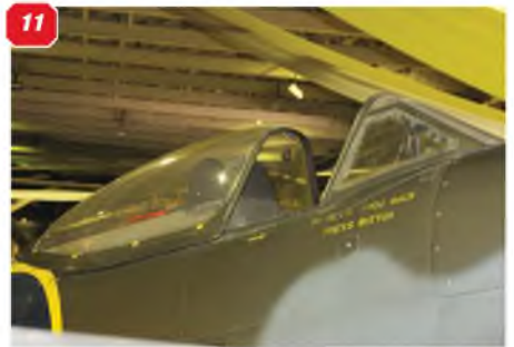
5: Massive bearers for the Rolls Royce Griffon engine. Note the six exhaust stacks 6 & 7: Two views of the carburettor air intake on the fuselage underside ahead of the wing root. 8: Further detail of the engine exhaust, left hand side. 9: Front cockpit side panels and windscreen. 10 & 11: Rear bubble canopy. 12 - 14: The retracting tailwheel and fairing doors.
