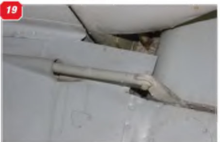
18 & 19: Two views of the rudder control horn and control rod. 20: The unusually shaped rudder trim tab. 21: Rudder trim tab control horn and fairing. 22: Tail light at base of rudder. 23: Free-to-air void at the fin/tailplane base (at the elevator hinge line). 24: Tailplane, showing the aerodynamic balance at the tip. 25: Twin elevator trim tabs, right elevator. 26: Trim tab close-up, right elevator. 27: Counterweighted inner tab, right hand elevator. 28: Single trim tab, left elevator. 29: Camera gun port at right wing root. 30: Twin 20mm cannon, wing leading edge. 31: Pitot head, left wing underside. 32: Wing tip light. 33: Fuselage centre section, showing shape of the big wing-to-fuselage fairing.
