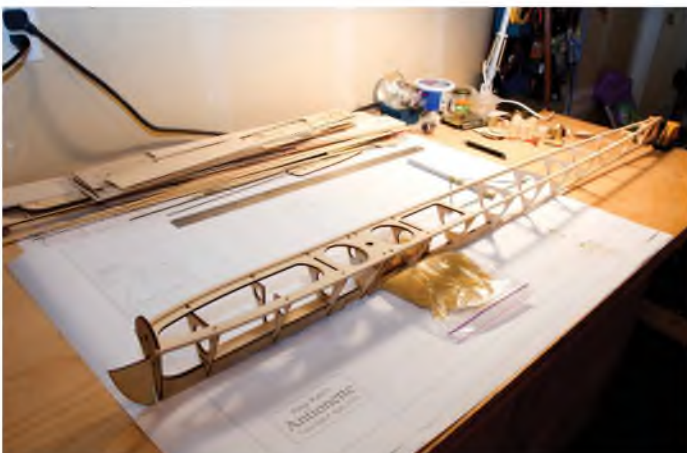
With the longerons and rear formers fitted you can see what a long, narrow fuselage this will be.
