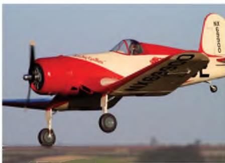
Paul Williams imaginatively schemed Meister Corsair in post-WWII Thompson Tro phyracer scheme. 100" span, DL50 power, weighs 16 kgs.
