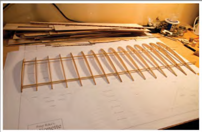
The wing ribs are slid onto the spars, adjusted to match the spacing on the plan and then you build a wing around them. Ailerons are strictly optional on this model.
