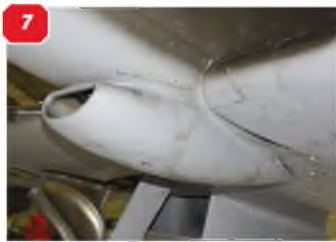
5: Massive bearers for the Rolls Royce Griffon engine. Note the six exhaust stacks 6 & 7: Two views of the carburettor air intake on the fuselage underside ahead of the wing root. 8: Further detail of the engine exhaust, left hand side. 9: Front cockpit side panels and windscreen. 10 & 11: Rear bubble canopy. 12 - 14: The retracting tailwheel and fairing doors.
