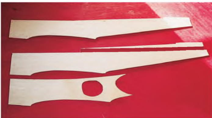
Fuselage side components, note two piece side and hole in doubler.
