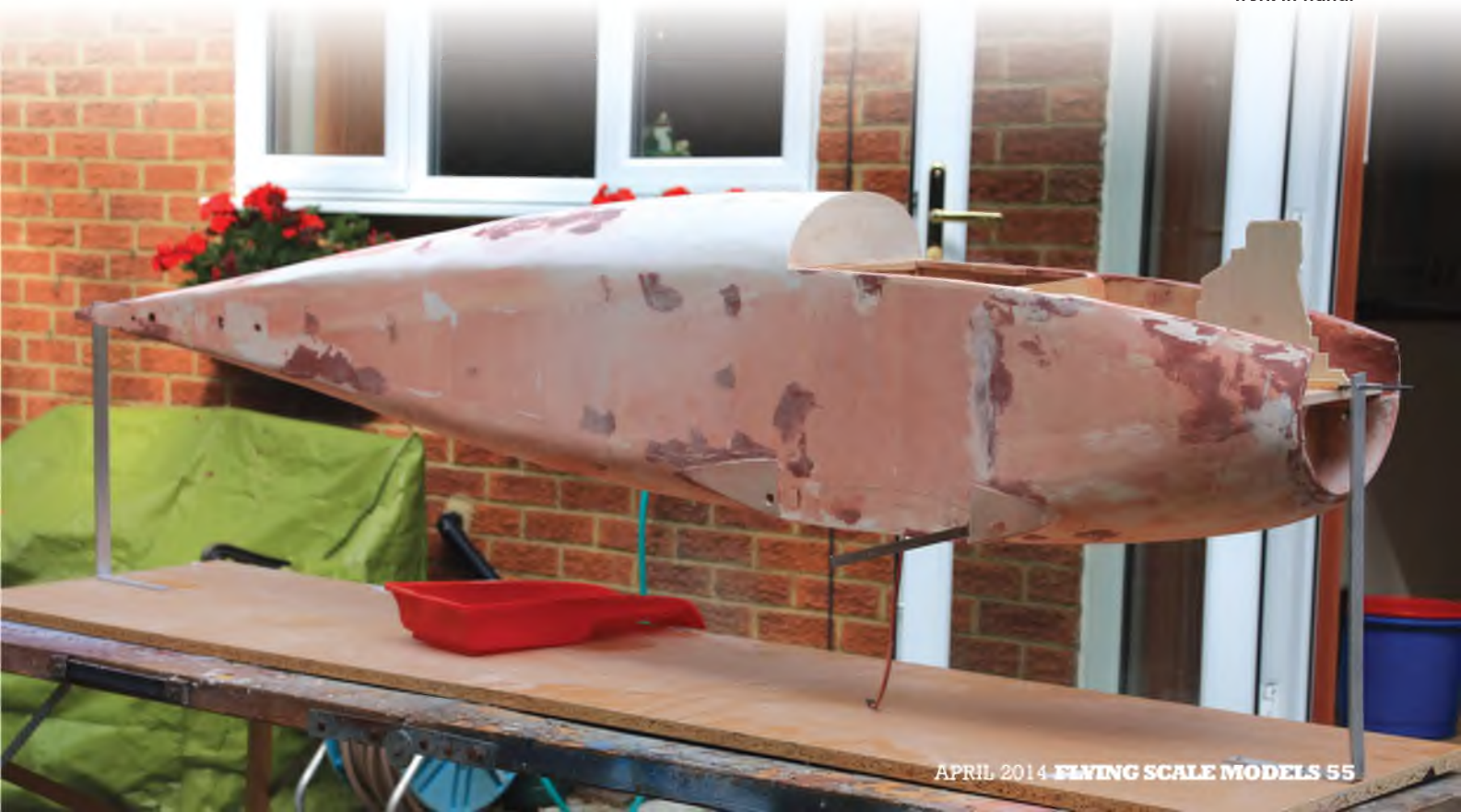
Here's something worth considering. This simple jig with attachment points either end of the fuselage allows the fus. to be rotated during the operation, leaving both hands free for the work in hand.
