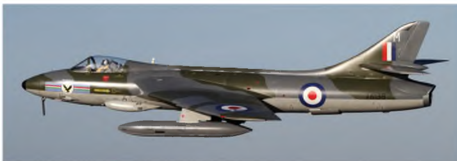
Immaculately prepared Hawker Hunter by Geoff White flashing by on full throttle. 82" span, weighs 45 lbs. Jetcat P-180 power.
