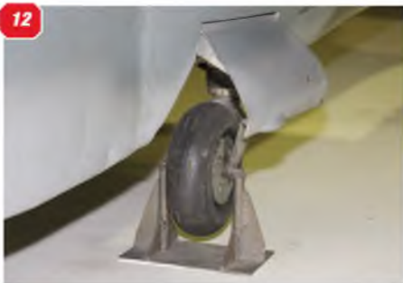
5: Massive bearers for the Rolls Royce Griffon engine. Note the six exhaust stacks 6 & 7: Two views of the carburettor air intake on the fuselage underside ahead of the wing root. 8: Further detail of the engine exhaust, left hand side. 9: Front cockpit side panels and windscreen. 10 & 11: Rear bubble canopy. 12 - 14: The retracting tailwheel and fairing doors.
