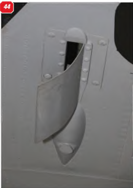
34-39: The Spitfire Mk.24 wing upper surfaces are festooned with with blister fairing over various internals that don't quite fit into the thin wing profile! 40: Rear of underwing radiator. 41: Radiator viewed from front. 42 & 43: the undercarriage well, wing underside. 44 & 45: Fixed spent ammo deflector, on wing underside. 46: Wing underside showing the inward folding wheel well cover. 47: Same, view from rear 48: Dished inner surface of wheel well cover. 49 & 50: Two views of the main undercarriage leg cover.
