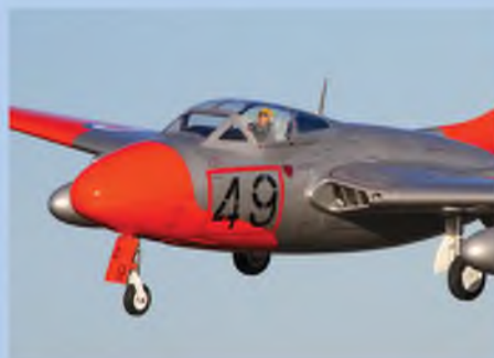
Ali Machinchy's DH Vampire T.11, two seater variant. Spans 110" and is powered by a Kingtech 180 turbine.
