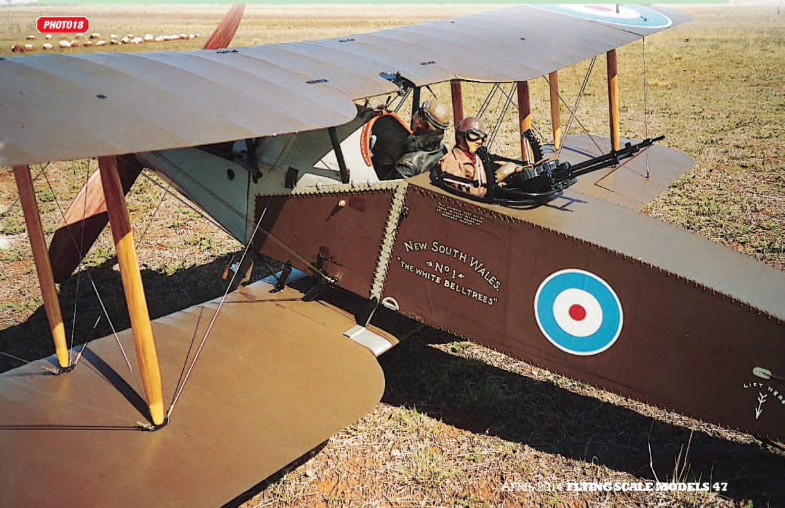
PHOTO 18: Rigging wires are very much obvious on this 1/4 scale Bristol F2B Fighter (FSM Plan 21) and the only reasonable alternative is Mick Reeves flat stainless steel strip and rigging fittings. There's a double ration of everything on the Brisfit, including the massive wing struts which are from Tasmanian Oak with a piano wire core and fittings as per Figures 4, 5 and 6. Note that the wires act some distance out from the struts, and, in theory, meet at the centroid of the spars. The parts are not difficult to make - there are just a lot of them!
