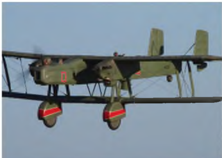
Dennis Richardson's 69" span HP Heyford powered by two OS .30 Four stroke glow engines. Weighs 6 1/2 lbs.
