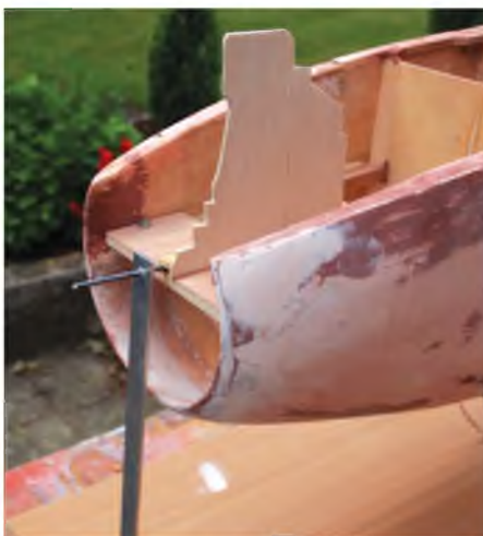
Here's something worth considering. This simple jig with attachment points either end of the fuselage allows the fus. to be rotated during the operation, leaving both hands free for the work in hand.
