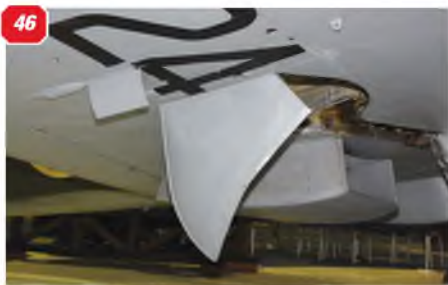
34-39: The Spitfire Mk.24 wing upper surfaces are festooned with with blister fairing over various internals that don't quite fit into the thin wing profile! 40: Rear of underwing radiator. 41: Radiator viewed from front. 42 & 43: the undercarriage well, wing underside. 44 & 45: Fixed spent ammo deflector, on wing underside. 46: Wing underside showing the inward folding wheel well cover. 47: Same, view from rear 48: Dished inner surface of wheel well cover. 49 & 50: Two views of the main undercarriage leg cover.
