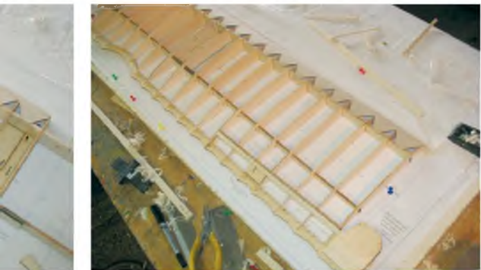
As with the bottom wings, build the top wing panels so that the top surface is flat and the lower surface tapered to provide 'dihedral'.
