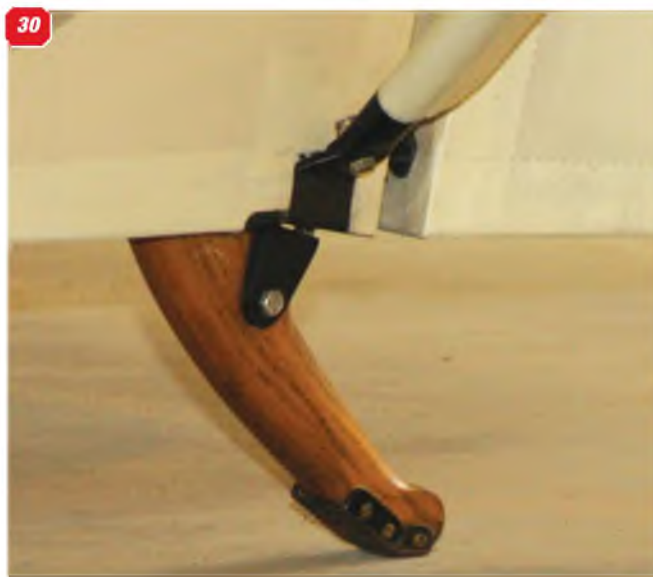
28: Bracing wire anchor point on the upper wing lower surface. 29: Detail of the elevator control horns and control cables. 30: The wooden tailskid and tailplane underside bracing strut attachment to the fuselage at the rudder post.
