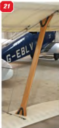
16,17 & 18: Three views of the JAP engine installed in the Shuttleworth Collection's replica aircraft at Old Warden. 19: Cockpit detail, right fuselage side. 20: Panel detail just forward of the cockpit, left side. 21: Interplane strut, left side. 22: Close-up of the upper wing interplane strut anchor point. and aileron control wire. 23 & 24: The interplane strut lower anchor point on the lower wing. 25 & 26: Wing centre section bracing wire. 27: Wooden 'acorn' steadiers at the wing barcing wire crossovers.
