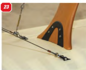
16,17 & 18: Three views of the JAP engine installed in the Shuttleworth Collection's replica aircraft at Old Warden. 19: Cockpit detail, right fuselage side. 20: Panel detail just forward of the cockpit, left side. 21: Interplane strut, left side. 22: Close-up of the upper wing interplane strut anchor point. and aileron control wire. 23 & 24: The interplane strut lower anchor point on the lower wing. 25 & 26: Wing centre section bracing wire. 27: Wooden 'acorn' steadiers at the wing barcing wire crossovers.
