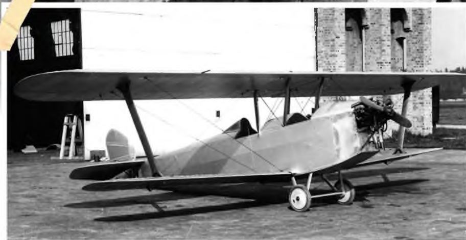
TOP: Along with many other small aircraft of its era, the Hawker Cygnet was design to suit the requirement of private and 'Club' flying, for which fold-away wings were important for hangar storage. ABOVE: No markings identify which of the two examples of the Cygnet, but this one features a headrest fairing behind the rear cockpit. It may well have just been wheeled out after final assembly.
