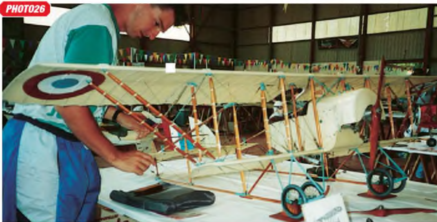
PHOTO 26: All struts, wires and warping! Even the elevators on Vlad Handlick's Caudron G3 (and also on the Taube) warped up and down! PHOTO 27: The author's 1/5th scale LVG C.VI was fitted with scale closed-circuit aileron control driven from a single fuselage mounted servo. PHOTO 28: Tailplane bracing wires exhibiting near-spherical silver-soldered joints between the stainless steel strip and the screw fittings. Similar joints in the wing bracings did not fail.
