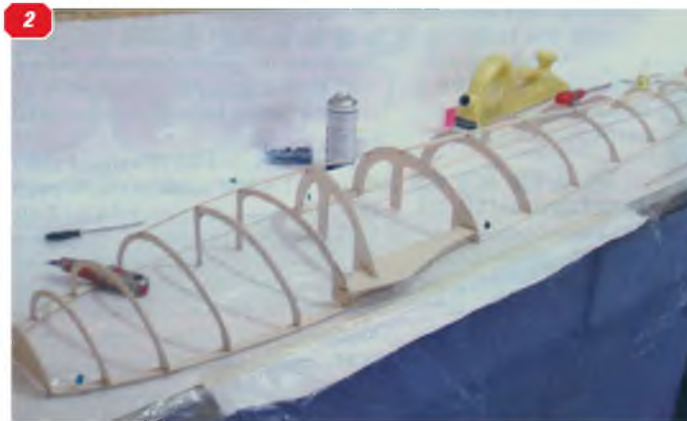
1 & 2: The fuselage formers of this large scale sailplane are typical of the multiple-station frames that need to be plotted.
