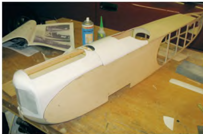
The plastic parts save a lot of filling, sanding and priming around the front end of the model.
