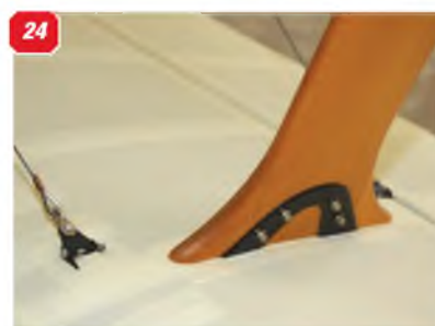
16,17 & 18: Three views of the JAP engine installed in the Shuttleworth Collection's replica aircraft at Old Warden. 19: Cockpit detail, right fuselage side. 20: Panel detail just forward of the cockpit, left side. 21: Interplane strut, left side. 22: Close-up of the upper wing interplane strut anchor point. and aileron control wire. 23 & 24: The interplane strut lower anchor point on the lower wing. 25 & 26: Wing centre section bracing wire. 27: Wooden 'acorn' steadiers at the wing barcing wire crossovers.
