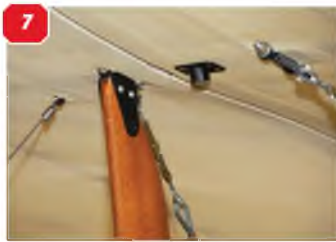
4 & 5: The arrangement of the wing cabane struts and bracing wires. 6: Upper anchor points for the cabane struts. 7: Close-up of one of the struts, showing the shape of the metal reinforcement bracket. 8: Detail of the lower anchor points for the cabane wire cross braces. 9 & 10: Upper and lower wings both have full-span ailerons. Control links to the control horns are bungee cords. 11: All that we could see of the pitot head on the upper right wing. 12: The link tube from the pitot head to the airspeed indicator in the cockpit. Note the clear neoprene tube connectors that can be detached from the metal tubes when the wings are folded.
