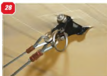
28: Bracing wire anchor point on the upper wing lower surface. 29: Detail of the elevator control horns and control cables. 30: The wooden tailskid and tailplane underside bracing strut attachment to the fuselage at the rudder post.
