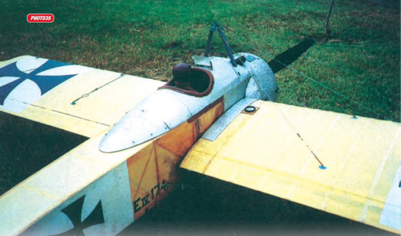
PHOTO 35: The author's model of the Fokker E.IV illustrates the incorrectly painted cable attachments. The Rectangular base was actually covered by fabric and only the hemispherical boss should have been painted grey (or black?). This model was built to 1/6th scale and was powered by an O.S.60 two-stroke. Note the strip ailerons! Most of the Kanones (German for 'big guns' or Aces) flew the E.IV in 1916 and scored most of their victories on this two-gun fighter.
