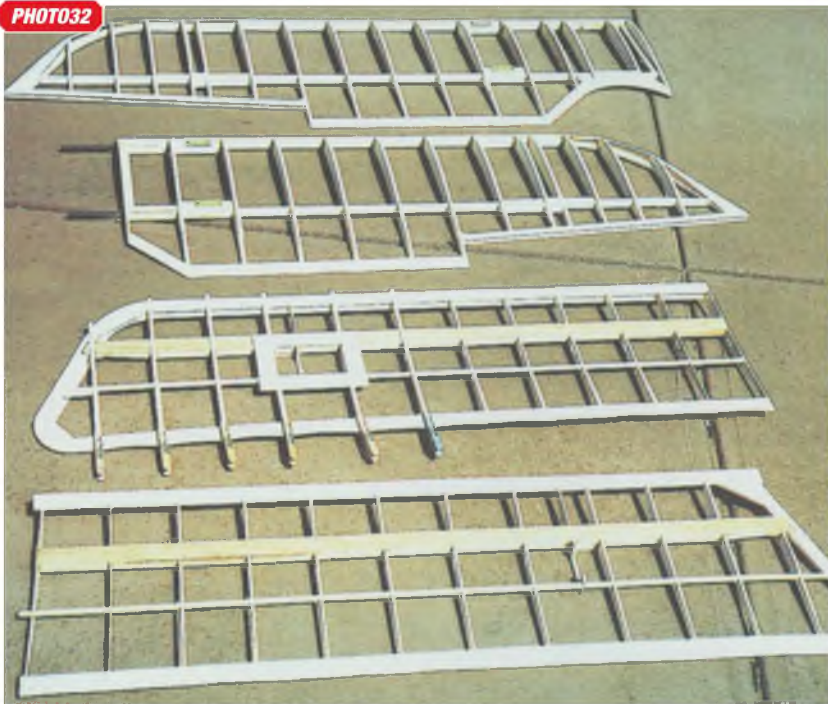
PHOTO 32: The wing panels of the austor's Albatros D.III under construction, show the shallow box spar in the lower wings. PHOTO 33: With the broken wing pinned down onto the building board, the covering is stripped away and timber doublers are glued and clamped either side of the break. PHOTO 34: As an extra precaution, the ribs have been cut away and an additional layer or 1.5mm birch plywood has been added to re-inforce the spar. The auxiliary spar has been repaired. Note the rib caps which are retained, to simply glue back in place, ready for the covering to be restored.
