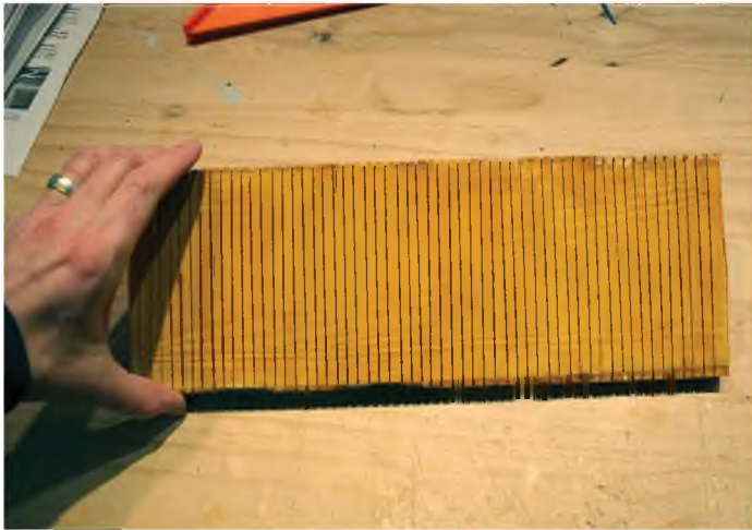
The board Jon mentioned for making rib tapes. Covering in place, thread wound and glued to covering.
