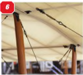
4 & 5: The arrangement of the wing cabane struts and bracing wires. 6: Upper anchor points for the cabane struts. 7: Close-up of one of the struts, showing the shape of the metal reinforcement bracket. 8: Detail of the lower anchor points for the cabane wire cross braces. 9 & 10: Upper and lower wings both have full-span ailerons. Control links to the control horns are bungee cords. 11: All that we could see of the pitot head on the upper right wing. 12: The link tube from the pitot head to the airspeed indicator in the cockpit. Note the clear neoprene tube connectors that can be detached from the metal tubes when the wings are folded.
