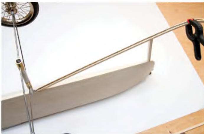
Here you see the wood cladding being fitted around the undercarriage wires -the bane of a skidded undercarriage.
