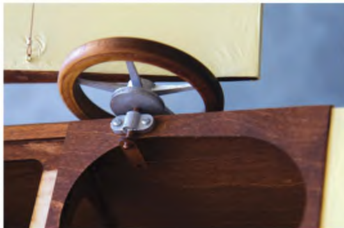
This is the elevator control wheel in place. A pushrod links the horn to the servo and cables around the pulley operate the elevators.
