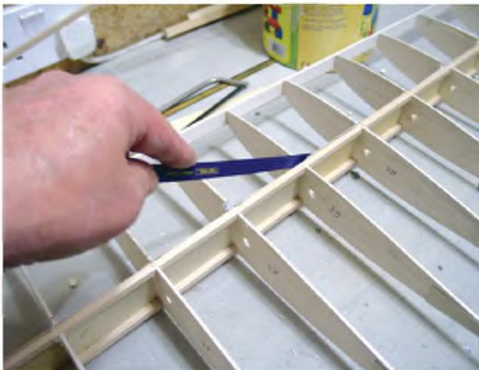
Cutting the slots for the 6mm sq sub-spar is a simple job.
