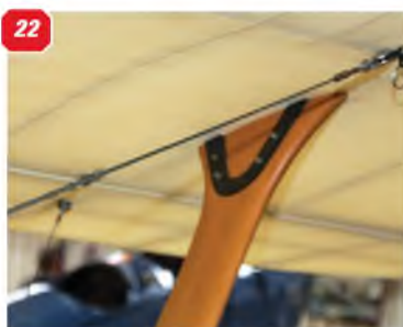
16,17 & 18: Three views of the JAP engine installed in the Shuttleworth Collection's replica aircraft at Old Warden. 19: Cockpit detail, right fuselage side. 20: Panel detail just forward of the cockpit, left side. 21: Interplane strut, left side. 22: Close-up of the upper wing interplane strut anchor point. and aileron control wire. 23 & 24: The interplane strut lower anchor point on the lower wing. 25 & 26: Wing centre section bracing wire. 27: Wooden 'acorn' steadiers at the wing barcing wire crossovers.
