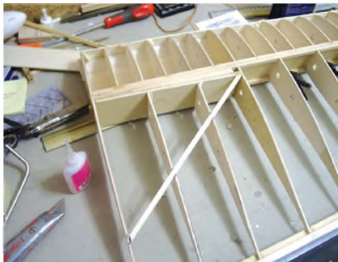
The 'I' beam arrangement on the K.11 wing.
