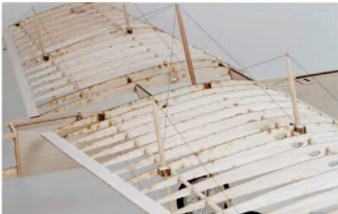
Here you see how the laminated balsa blocks that form the mount positions for the rigging kingposts.
