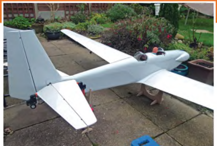
Author's 1/4 scale RF-5b on the CG frame, ready to measure the decalage.
