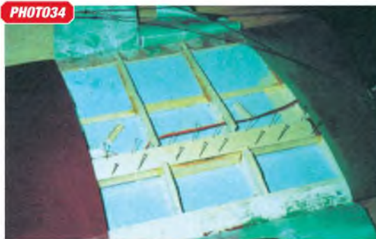
PHOTO 32: The wing panels of the austor's Albatros D.III under construction, show the shallow box spar in the lower wings. PHOTO 33: With the broken wing pinned down onto the building board, the covering is stripped away and timber doublers are glued and clamped either side of the break. PHOTO 34: As an extra precaution, the ribs have been cut away and an additional layer or 1.5mm birch plywood has been added to re-inforce the spar. The auxiliary spar has been repaired. Note the rib caps which are retained, to simply glue back in place, ready for the covering to be restored.
