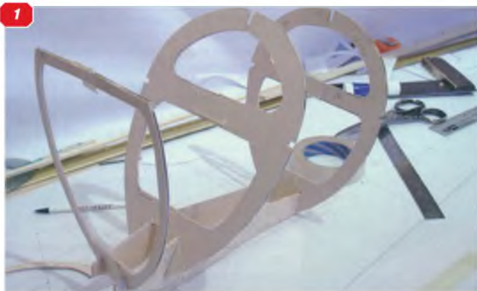
1 & 2: The fuselage formers of this large scale sailplane are typical of the multiple-station frames that need to be plotted.
