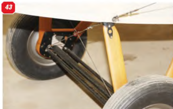
43: The main undercarriage axle and associated front and rear tie-bars seen very much WW1-era technology, but then, since the aircraft was designed only six years later in 1924.
