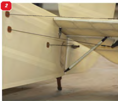
1 The complete rear fuselage, showing the elevator and rudder control cables and the control horns. Note also the circular inspection panel below the tailplane. 2 View under the tailplane, showing the tailplane bracing struts. The control cable exit guides are leather.
