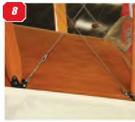
4 & 5: The arrangement of the wing cabane struts and bracing wires. 6: Upper anchor points for the cabane struts. 7: Close-up of one of the struts, showing the shape of the metal reinforcement bracket. 8: Detail of the lower anchor points for the cabane wire cross braces. 9 & 10: Upper and lower wings both have full-span ailerons. Control links to the control horns are bungee cords. 11: All that we could see of the pitot head on the upper right wing. 12: The link tube from the pitot head to the airspeed indicator in the cockpit. Note the clear neoprene tube connectors that can be detached from the metal tubes when the wings are folded.
