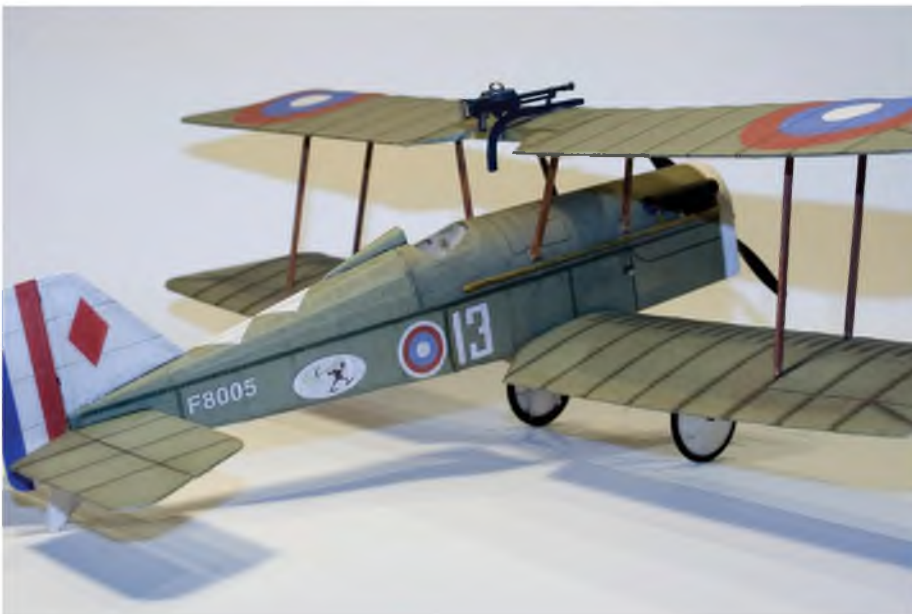
Even small models benefit from careful finishing. This 18" span SE5A uses printed tissue as its' covering.
