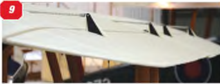
4 & 5: The arrangement of the wing cabane struts and bracing wires. 6: Upper anchor points for the cabane struts. 7: Close-up of one of the struts, showing the shape of the metal reinforcement bracket. 8: Detail of the lower anchor points for the cabane wire cross braces. 9 & 10: Upper and lower wings both have full-span ailerons. Control links to the control horns are bungee cords. 11: All that we could see of the pitot head on the upper right wing. 12: The link tube from the pitot head to the airspeed indicator in the cockpit. Note the clear neoprene tube connectors that can be detached from the metal tubes when the wings are folded.
