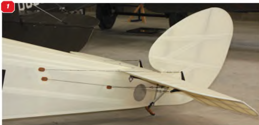
1 The complete rear fuselage, showing the elevator and rudder control cables and the control horns. Note also the circular inspection panel below the tailplane. 2 View under the tailplane, showing the tailplane bracing struts. The control cable exit guides are leather.
