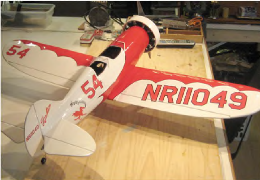
The Gee Bee marking that Jon cut using a vinyl cutter. Could be done by hand too, of course.
