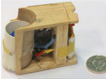
The prototype of Derek Knight's very powerful and controllable 18mm fan EDF unit. That's a 5p piece for comparison.
