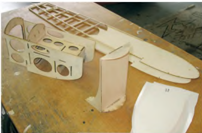
Basic fuselage sub-assemblies seen here with one of Pat's low-tech formed plastic panels.
