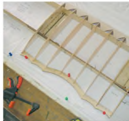
Begin the top wing by building the centre section onto the ready joined spars.
