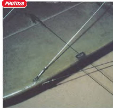
PHOTO 26: All struts, wires and warping! Even the elevators on Vlad Handlick's Caudron G3 (and also on the Taube) warped up and down! PHOTO 27: The author's 1/5th scale LVG C.VI was fitted with scale closed-circuit aileron control driven from a single fuselage mounted servo. PHOTO 28: Tailplane bracing wires exhibiting near-spherical silver-soldered joints between the stainless steel strip and the screw fittings. Similar joints in the wing bracings did not fail.
