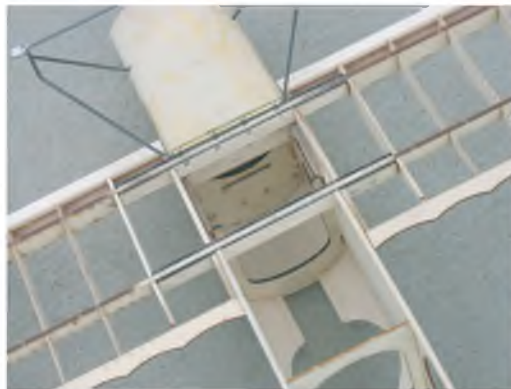
Once complete, the lower wing is a snug fit into the fuselage cut-out.
