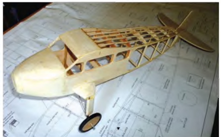
The main undercarriage wires fitted and balsa fairings added.
