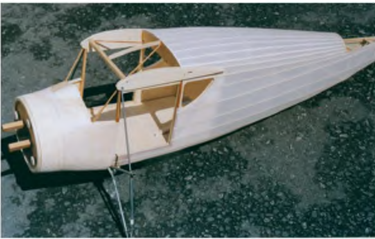
The basic fuselage of the F.24W Argus, with the aft section covered and the wire main undercarriage members fitted.
