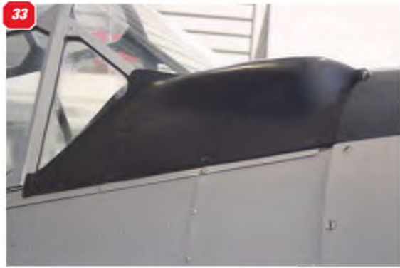
32: Cockpit canopy guide rail at the rear of the cockpit. 33: Another view of the bulged fairing on the right hand side of the fuselage top deck ahead of the cockpit windscreen. This kind of detail varied from version-to-version of the AT-6/SJN/Harvard. 34: Cockpit front windscreen. 35: General view of the full cockpit canopy.
