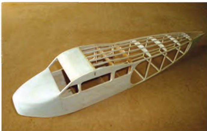
Once the nose is shaped the stringers can be added to form the rounded rear deck.
