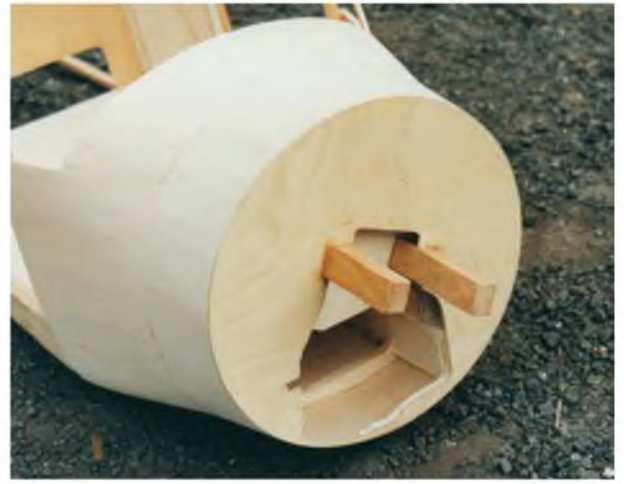
Front Fuselage at the firewall with engine bearers in place.
