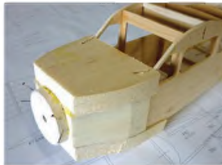
Block balsa and part N glued in place and ready for shaping. Half of N and the bottom block form the access hatch.
