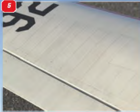
1: Distinctive fin and "tail-cone". 2: Sports scale elevator detailing is crisp. 3: Typical American brush script for the Lucky Gallon Racer. Adds that touch of sparkle. 4: Pinked rib tapes, neatly done. 5: Fine detailing on the wing - rib tapes, flush rivets, and panelling. 6: Canny Paul has grouped his essential switches under a scale panel.
