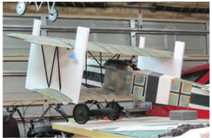
Pat made simple pink foam guides to assist with getting the top wing incidence and alignment correct.
