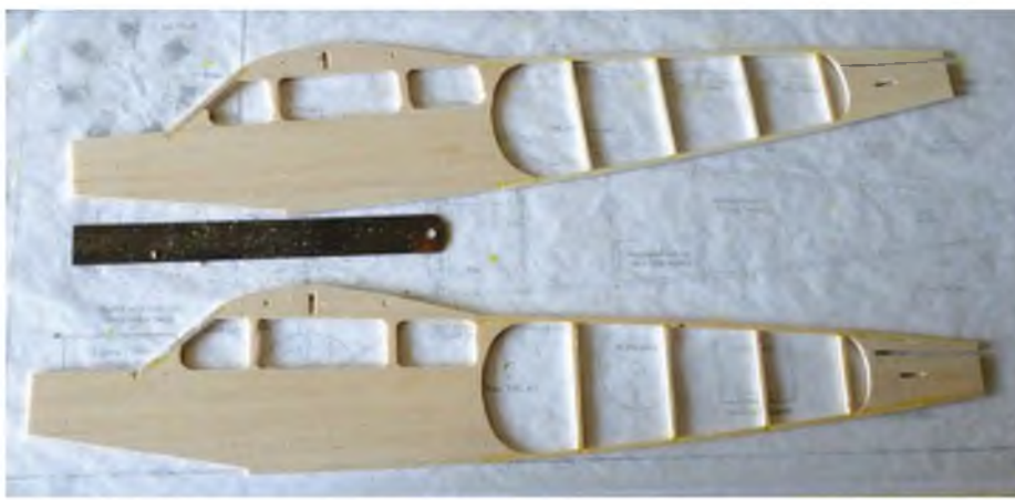
Nothing unusual about producing the basic fuselage sides. Sheet balsa forward sections and built up strip rear end.
