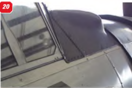
16: Fuselage panel line detail at the rear cockpit position. Note the fixed foot step for access into the cockpit. 17: Panel detail at the wing training edge, showing the small fairing with the fuselage. 18: Panel lines in the fuselage top side, just ahead of the cockpit. 19: Rear fuselage top side fuselage panel detail. 20: The bulged panel on the fuselage, top right side of the cockpit windscreen. 21: Another view of the exhaust stack. 22: Tailplane/elevator hinge line, showing the aerodynamic balance. 23 & 24: Two views of the elevator trim tab.
