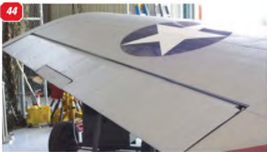
36: Bulged fairing, wing underside, also showing the cover over the wing panel join line. 37: Landing light in the wing leading edge. 38: Pitot head right wing leading edge. 39: Wing tip navigation light. 40: Aileron trim tab. 41 & 42: Aileron hinges. 43: Rubber cockpit access tread-plate, also showing the fairing strip over the inner/outer wing panel joint fairing. 44: The complete aileron, showing the hinge line. 45: Top-side view of the wheel fairing in the wing leadline edge. 46: Further view of the cover strip over the inner/outer wing panel join line. 47: Wing panel line detail aft of the wing leading edge along the termination of the wrap-around leading edge surface skin.
