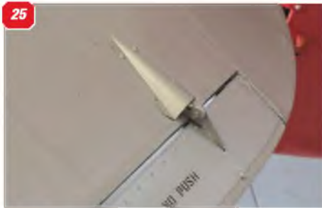
25: Pressed metal fairing cuff at the tailplane leading edge. 26: Main undercarriage wheel well. 27 - 31: The long cockpit canopy is a dominating feature of the AT-6 as these views reveal.
