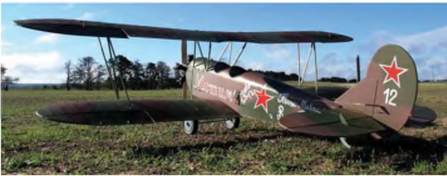
The level of completion at which Pat just couldn't resist a test flight, or two. External rudder and elevator linkages simplify setting up.
