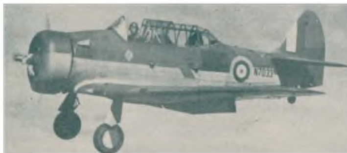
This RAF Harvard Mk.1 features the rounded rudder shape. Note the ample flaps, here fully deployed.
