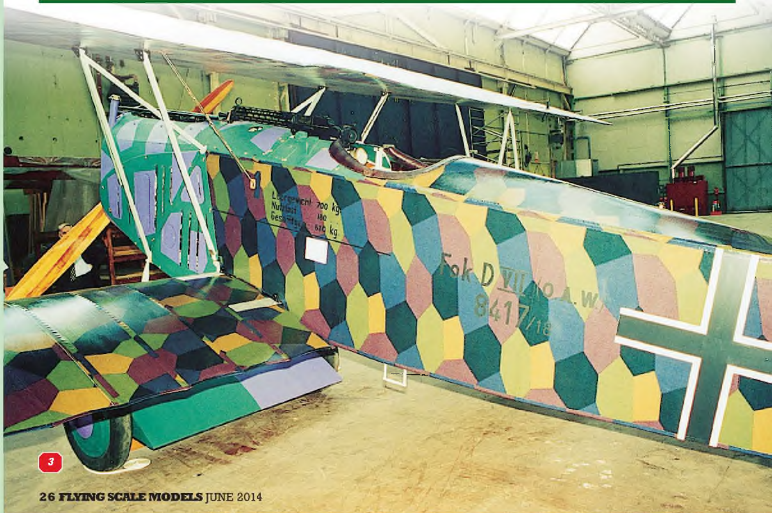
1-2: Some general views of the RAF Museum's machine which features five-colour pattern lozenge camouflage scheme. As mentioned by Gary Sunderland in the instructions for his model, the 'axle wing' is not lozenge pattern covered.
