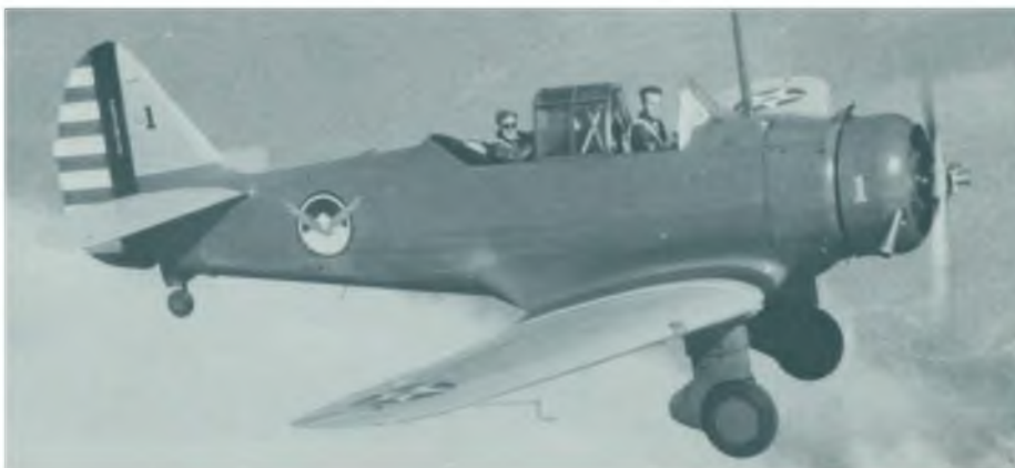
As revised to US Army requirement, the NA-16 became NA-18, with enclosed cockpit, plus main undercarriage fairing and assumed the military designation BC-9 (Army) and NJ-1 (Navy).
