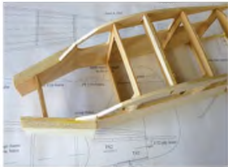
How the forward sides are scored, cracked inwards and joined with the ply firewall.
