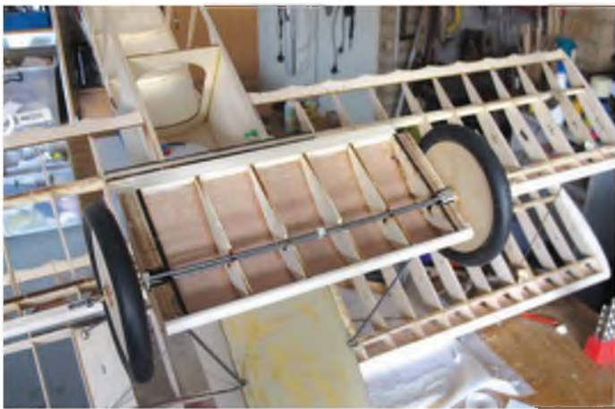
How the axle fairing fits onto the undercarriage, before the end ribs are fitted and the lower surface sheeted.
