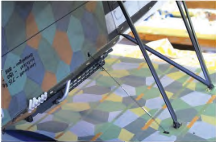
Here you see how the struts bolt to the wing and the aileron cables run from fuselage to wing.
