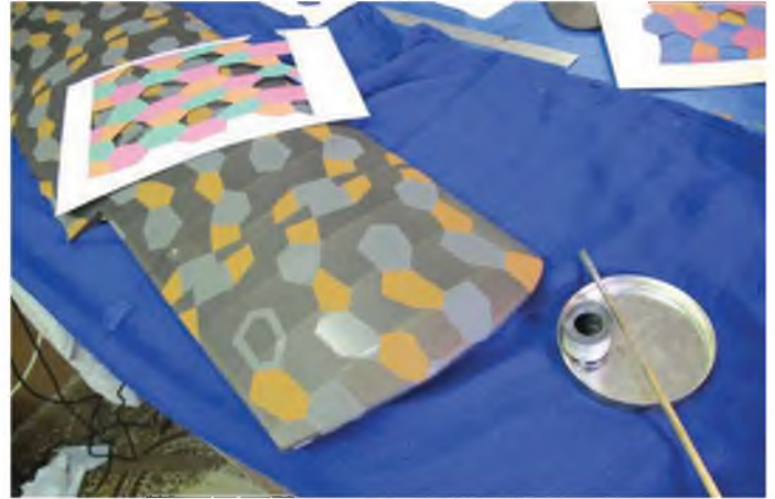
Pat used a series of stencils to mark out the lozenge finish before brush painting it onto the Litespan covering.
