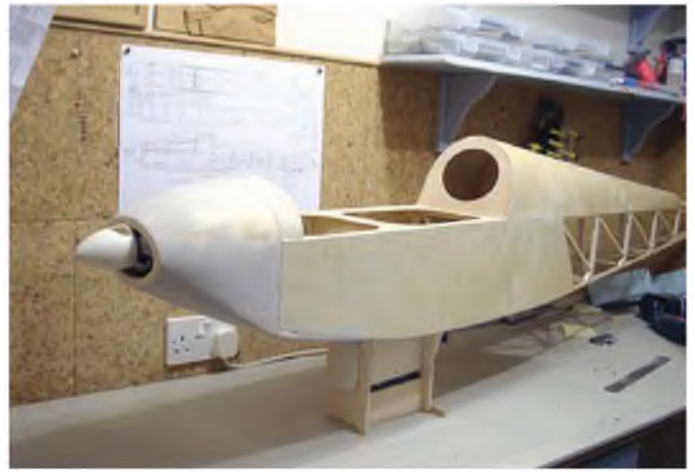
The K11 cowl finished, ready for sealing and painting.
