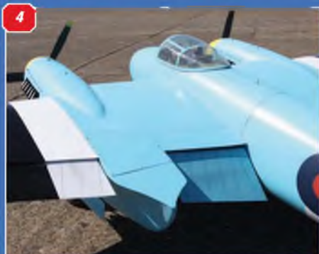
1: Amazingly slim tail and slender fin and tailplane. Note rib detail. 2: Ted's model may have lost a couple of exhaust stacks in action, but the panel detailing is neatly done. 3: Nacelle and door details all present. 4: Distinctive engine nacelles, which had been extended on the DH prototype to counter tail buffeting. 5: Side view of retracts and oleo. 6: Retracts with oleo detailing. Note tyres showing weight of two Merlins!
