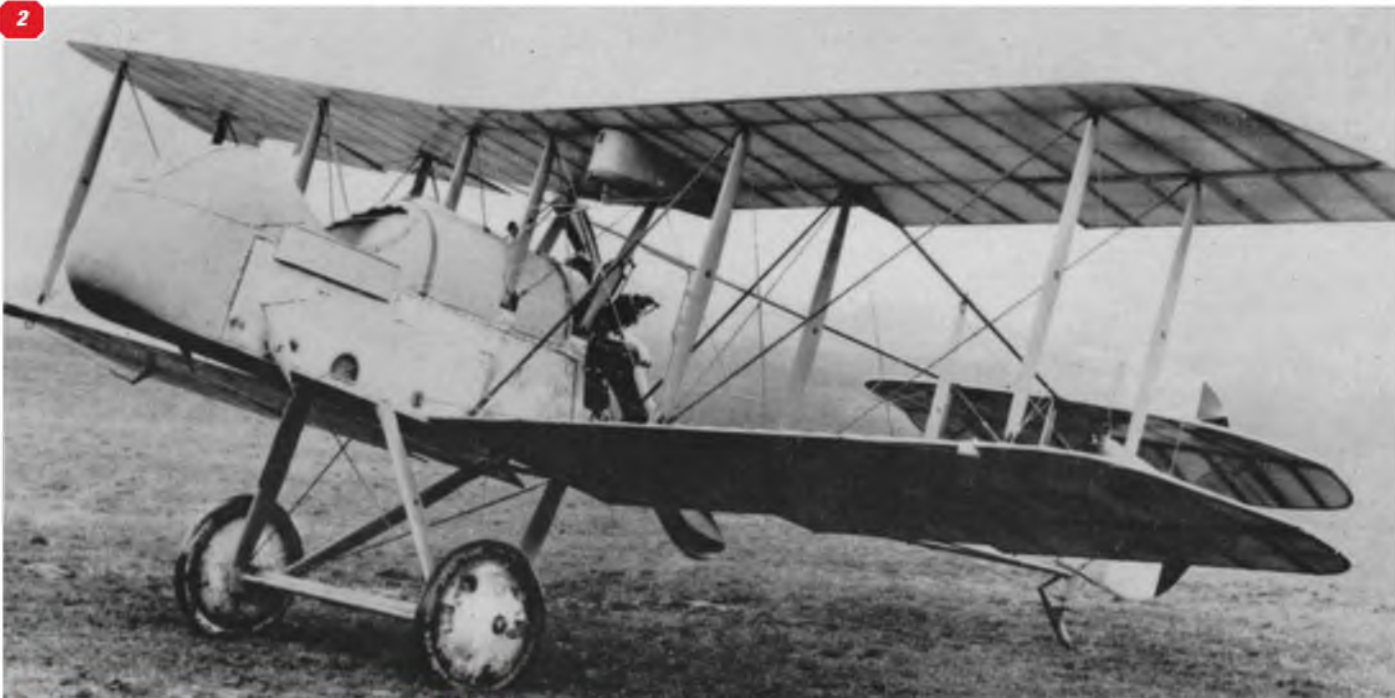
1 "One of our aircraft is missing". German pilots examine the the first Airco DH2 sent to France for tests in 1915 and lost after couple of weeks of operations. German ace Oswald Bloelke is the man in the cockpit. 2 A production DH2 from the first batch with gravity fuel tank mouned under the left upper wing. 3 First prorotype DH2. The nose and windscreen differ from the production example above. 4 This view illustrated the wide spread of the fuselage booms and the tight width of the cockpit. Fuel tank here is mounted above the upper left wing.
