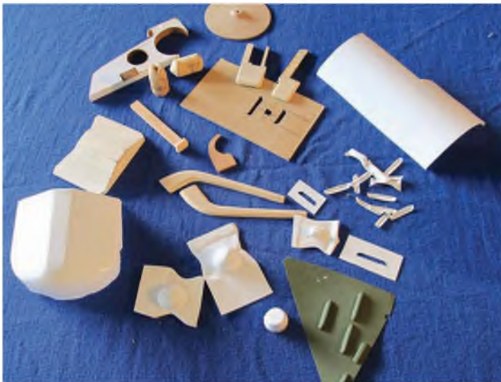
A typical selection of the simple homemade tools used for forming parts, and some of the parts thus produced.
