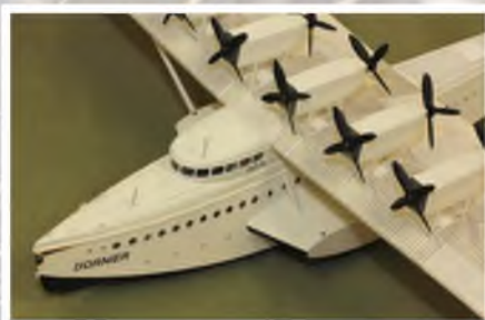
Paul Brigg's ambitious F/F electric powered Domier DoX. Six KP 01 motors driving twelve props on extended double-ended drive shafts.
