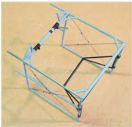
Plastic and aluminium tube, some beading wire and no small amount of ingenuity make short work of creating a basic fuselage structure to adorn the cockpit area.
