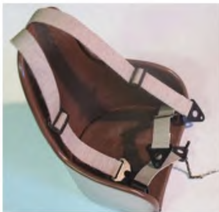
It's amazing what can be created from items likely to be found around the home. Leather effect card, strips of roller blind and assorted bits of plastic make a convincing seat.
