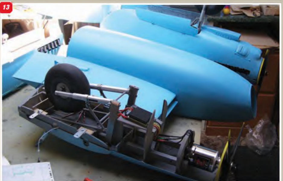
7: The basic glass fibre fuselage/centre section moulding. 8: Basic outer wing panel, mated to moulded engine pod. 9 & 10: Deep inside the fuselage, the radio and power panel trays. 11: Moulded glass fibre components and outer wing panels now assembled. 12: Man at Work! Ted delves into the forward fuselage via the cockpit well. 13: One of the engine nacelle installation trays, that houses the rearward retracting main undercarriage leg and the electric motor.
