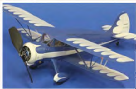
Peter Boys' rubber powered Waco YKS7, scratch-built to 1/25th scale, weighs 26 grams.
