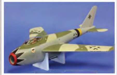
Peter Illiffe's own design Me P1101jet. 17" span, R/C with three servos, built to 1/20th scale.
