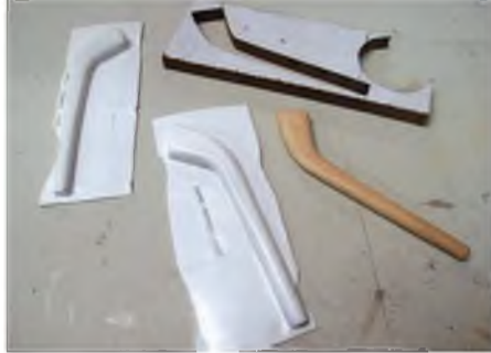
The very simple tools used to create the basis of the exhaust, and samples of the moulded result.
