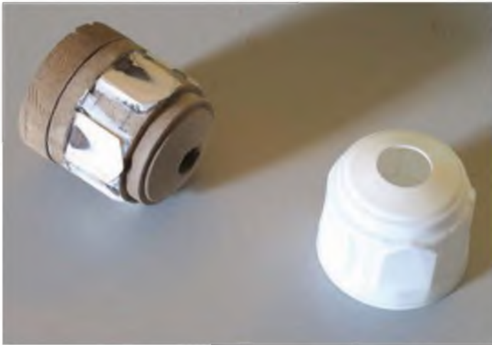
Pat's homemade plug and one of the crankcase mouldings he made from it. Good enough, but still just a bit basic for Pat.
