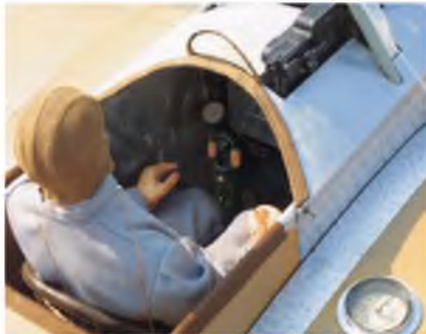
Sometimes, instruments go beyond the cockpit - as with this Fokker Eindekker wish compass set in the wing roof.
