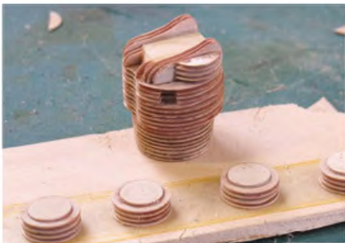
Adding the top fins and filling in pushrod clearance and spark plug positions all add realism to the basic cylinders.
