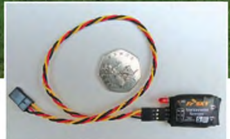
The FrSky Variometer as tested by the author - hardly makes any great demand on fuselage installation space!
