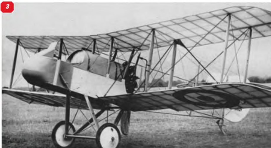
1 "One of our aircraft is missing". German pilots examine the the first Airco DH2 sent to France for tests in 1915 and lost after couple of weeks of operations. German ace Oswald Bloelke is the man in the cockpit. 2 A production DH2 from the first batch with gravity fuel tank mouned under the left upper wing. 3 First prorotype DH2. The nose and windscreen differ from the production example above. 4 This view illustrated the wide spread of the fuselage booms and the tight width of the cockpit. Fuel tank here is mounted above the upper left wing.
