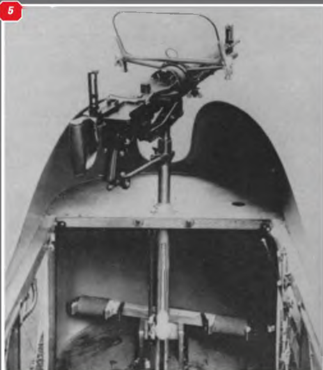
5: The machine gun mount in the cockpit. Note also the rudder control bar. 6: Another early example of the Airco DH2. It has a four-blade propeller here, but most really early examples had only two blades. 7: After being outclassed on the Western Front in France in late 1916/early 1917, Airco DH2 aircraft were sent further afield to the Middle East where the type continued to do useful service.
