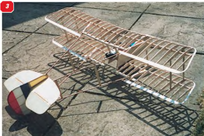
1: Upper and lower wing panels mated to the open form tailboom. 2: One stage further on, with the basic components of the fuselage pod in place. 3: The complete uncovered basic airframe. 4: Tyres for the main undercarriage wheels were mad from closed cell sponge rubber for the prorotype model. 5: Fuselage pod underside showing the main undercarriage struts and the access to the receiver. 6 & 7: Two views of the tail-cone showing the mounting to the fuselage rear boom. 8 & 9: Wing interplane struts. This is a one-piece model, so struts are glued permanently in place. 10: Detail of the tail boom showing the anchor points on the wing amd inter-boom vertical spacers. 11: 'Pilot Pete' in his drafty perch.
