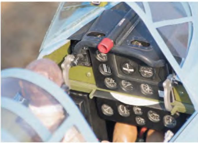
A little bit of fine dust around the instrument panel produces a convincing effect.
