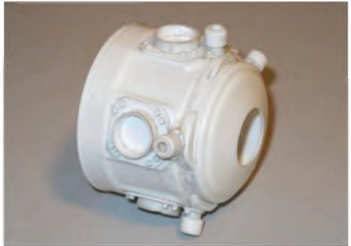
Once a few bits of sheet plastic, plastic tube and slices of hex rod have been added, the crankcase starts to come to life.
