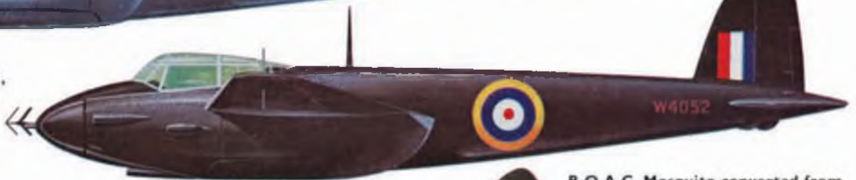
B.O.A.C. Mosquito converted from B. Mk. IV DZ411. Flew the Leuchars-Stockholm route with diplomatic mail and passengers, returning with ball-bearings in the bomb-bay.
