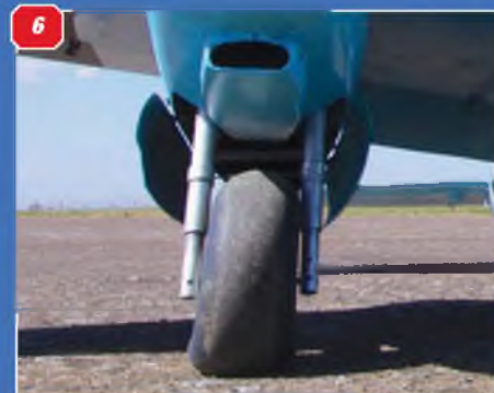
1: Amazingly slim tail and slender fin and tailplane. Note rib detail. 2: Ted's model may have lost a couple of exhaust stacks in action, but the panel detailing is neatly done. 3: Nacelle and door details all present. 4: Distinctive engine nacelles, which had been extended on the DH prototype to counter tail buffeting. 5: Side view of retracts and oleo. 6: Retracts with oleo detailing. Note tyres showing weight of two Merlins!
