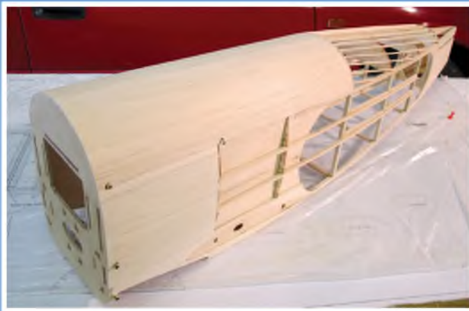
Once the sheeting and side stringers are on the basic fuselage is almost complete. Not the strut and u/c tubes yet to be trimmed flush.
