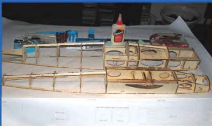
Here you see the 'shell' style fuselage in its' early stages. Upper and lower halves can be almost completed before they are joined.
