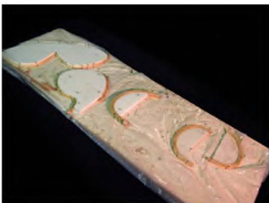
The dreaded laminated outlines drying around their Depron forms. A bit of a pain it but results in strong, light outlines.
