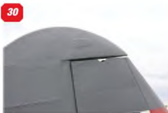
27: Complete fin and rudder, showing trim tab linkage and tail light. 28: Rudder linkage and control horn, left side of rudder. 29: The shape of the aerodynamic balance at the tailplane tip identify this aircraft as a late example of the Mk.IX. See scale drawing elsewhere in this issue for comparison. 30: Aerodynamic balance at the top of the rudder. 31: Trim tab linkage and fairing on the upper face of the elevator. 32: This view shows the gap in the fuselage skin through which passes the elevator joiner.
