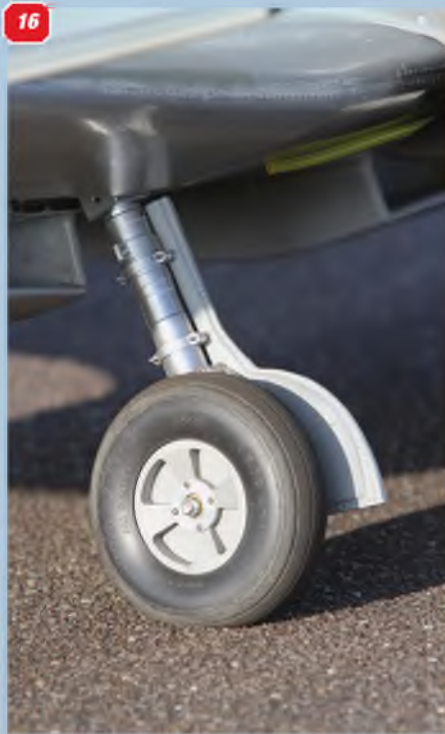
15: Distinctive and elegant Spitfire air intake is finely mounded. 16: Undercarriage and doors are crisply modelled. Robart wheels are used. 17: The correct spinner is very important for any scale model but for a Spitfire, absolute accuracy is essential. 18: Stencils, lettering, and rivets all build the illusion. 19: The brush script and the kills are beautifully done, but the underlying panelling and rivet lining seals the authenticity.
