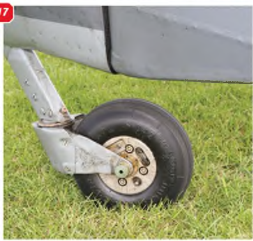
13 & 14: The outward retracting main undercarriage leg and wheel well fairing, also showing the outer face of the main undercarriage wheel.
