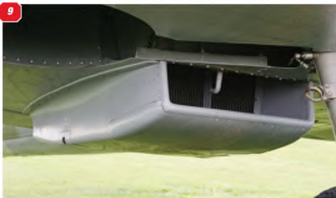
5: Centre-line air scoop under the engine cowl. 6 & 7: The concave curvature of the wing-to-fuselage fairing underside is an important feature to replicate in a model. 8: The wide sweep of the wing-to-fuselage fairing. 9: The Spitfire Mk.IX was the first of the series to use a symmetrical arrangement of air intakes under the left and right wing panels. 10 & 11: Surface bulges and fairings on the wings. The inner one accommodates the retracted mainwheel, the outer one fairs over the 20mm Hispano cannon. 12: Bulge on the wing root fairing at about 20% wing chord.
