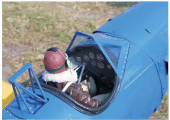
Another example of an open cockpit type, this 1/4 scale Fairchild PT-19 features a realistic cockpit coaming and tubular steel airframe members in the cockpit sides are replicated to good effect.
