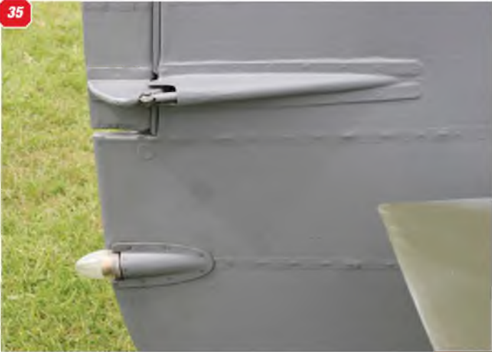
33 & 34: Two views of the pressed metal tailplane fairing cuff. 35: Close-up of the rudder trim tab and the tail light. 36: An even closer look at the rear tail light. 37: "Watch you Six"! The Rear-view mirror, also showing the cockpit winscreen framing.
