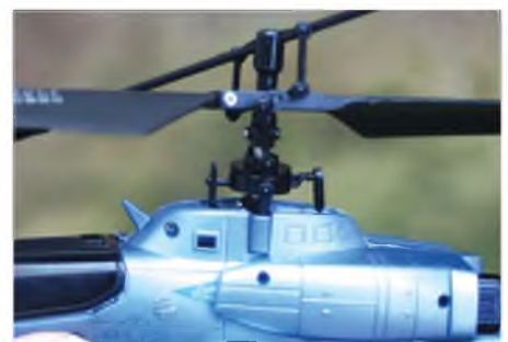
Yes, I know that looks like a conventional swashplate, but the bank part of it is locked rather than connected to a servo. Model still flies well.
