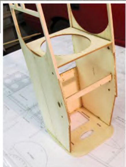
How those parts go together, with the tabs on the inner sides locating in firewall slots and the wing strap part trapped in the inner sides.
