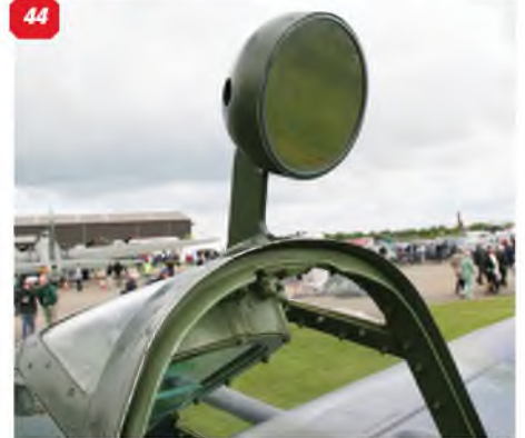
38-41: Cockpit frame, also showing the recessed runner for the rearward opening canopy.
