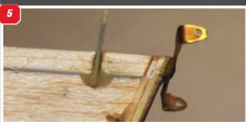
1: First step of the fin construction, adding rib strips over the balsa centreline core. Component then turned over to add ribs on the other side. 2: The first step of rudder construction is the same. 3: Laminated balsa strip outline now glued and pinned in place. 4: The finished, uncovered fin and rudder unit. 5: Rudder horn, epoxy glued in place on the rudder leading edge, together with the steerable tailwheel control bracket, made from brass. 6: Basic strip balsa fuselage sides, drawn together with the front fuselage formers and clipped together at the rudder post. 7: Further view of the basic fuselage, one stage further on, with the rear top-deck formers in place, together with the cabin/wing rib facings. 8: Hardwood undercarriage mounting blocks in the bottom of the fuselage at the cabin area. 9: Completed fuselage detail at the cabin area showing the boxed in roof and facing ribs. Note the scale bracing struts just behind the windscreen position. 10: Front and rear main undercarriage wire struts are faired-in with balsa in-fill, as are the cabin sides between the diagonal fuselage side spacers. 11: Scale cabin access door on the right (starboard) fuselage side. 12: Another view of the uncovered fuselage at the cabin area, showing the wing rib shaped end plates that butt to the wing panels when the latter are mounted to the fuselage.
