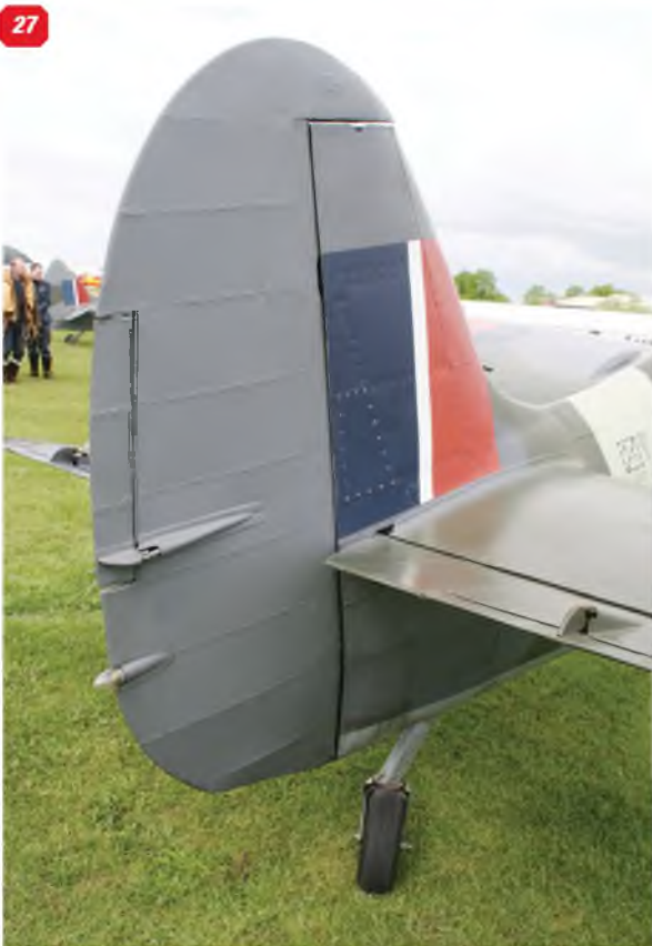
27: Complete fin and rudder, showing trim tab linkage and tail light. 28: Rudder linkage and control horn, left side of rudder. 29: The shape of the aerodynamic balance at the tailplane tip identify this aircraft as a late example of the Mk.IX. See scale drawing elsewhere in this issue for comparison. 30: Aerodynamic balance at the top of the rudder. 31: Trim tab linkage and fairing on the upper face of the elevator. 32: This view shows the gap in the fuselage skin through which passes the elevator joiner.
