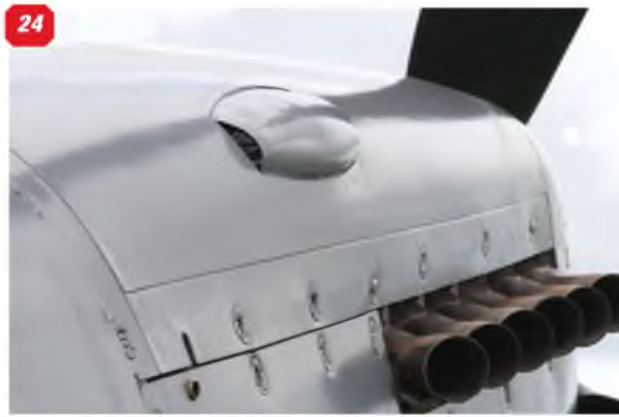
23 & 24: Two views showing panel line details on the nose section ahead of the cockpit. Note that panels overlap each other.
