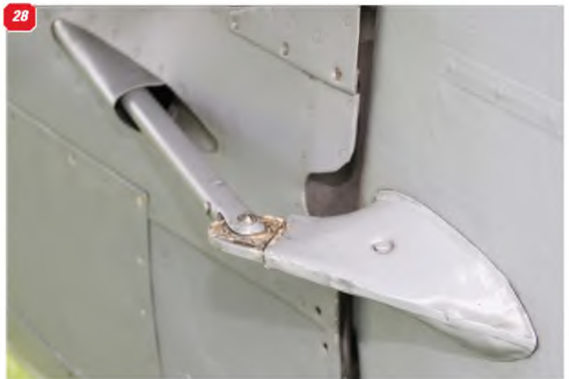
27: Complete fin and rudder, showing trim tab linkage and tail light. 28: Rudder linkage and control horn, left side of rudder. 29: The shape of the aerodynamic balance at the tailplane tip identify this aircraft as a late example of the Mk.IX. See scale drawing elsewhere in this issue for comparison. 30: Aerodynamic balance at the top of the rudder. 31: Trim tab linkage and fairing on the upper face of the elevator. 32: This view shows the gap in the fuselage skin through which passes the elevator joiner.
