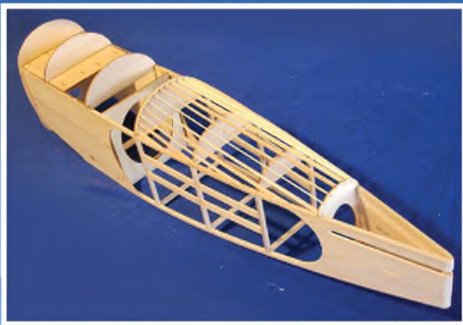
With the tail joined, remaining formers added and that 'interesting' stringer arrangement it starts to look like a fuselage.
