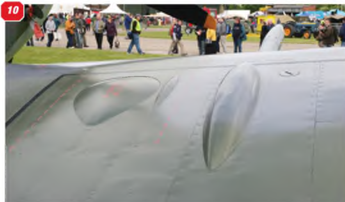
5: Centre-line air scoop under the engine cowl. 6 & 7: The concave curvature of the wing-to-fuselage fairing underside is an important feature to replicate in a model. 8: The wide sweep of the wing-to-fuselage fairing. 9: The Spitfire Mk.IX was the first of the series to use a symmetrical arrangement of air intakes under the left and right wing panels. 10 & 11: Surface bulges and fairings on the wings. The inner one accommodates the retracted mainwheel, the outer one fairs over the 20mm Hispano cannon. 12: Bulge on the wing root fairing at about 20% wing chord.
