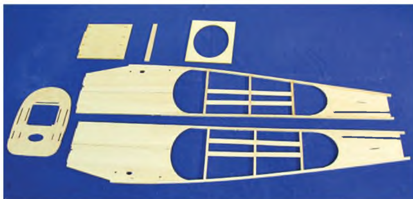
The basic fuselage side frames, along with firewall, strut plate, wing strap mount and a simple former. Just visible are the tabs on the inner side pieces.
