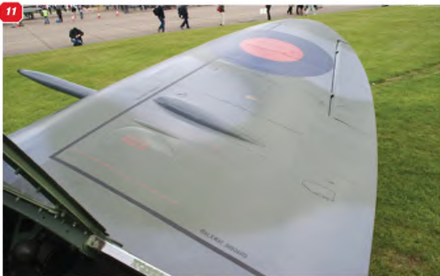
5: Centre-line air scoop under the engine cowl. 6 & 7: The concave curvature of the wing-to-fuselage fairing underside is an important feature to replicate in a model. 8: The wide sweep of the wing-to-fuselage fairing. 9: The Spitfire Mk.IX was the first of the series to use a symmetrical arrangement of air intakes under the left and right wing panels. 10 & 11: Surface bulges and fairings on the wings. The inner one accommodates the retracted mainwheel, the outer one fairs over the 20mm Hispano cannon. 12: Bulge on the wing root fairing at about 20% wing chord.
