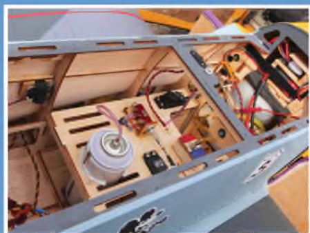
Radio compartment on Dempster Hamilton's Me 109E. Note aerosol-style tank for air retracts reservoir.
