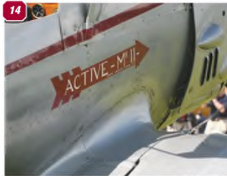
12: Fuselage centre section showing the wing bracing wires and centre section wing strut anchor points. 13: Lower wing fillet and detail of wing bracing wire anchor point. 14: Further view of the lower wing fillet and louvres in the engine cowl. 15: Upper wing centre section detail. 16: Interplane wing struts and detail of the streamlined bracing wires.
