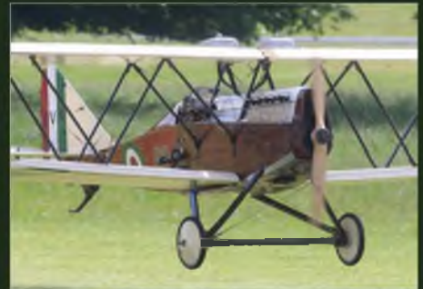
Ansaldo SVA by Carlos Guerra. One third scale, spans 3 metres, and powered by a DLE 170cc twin. Weighs 37 kgs.
