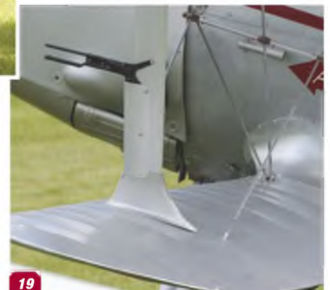
17: Further view of the wing interplane strut. 18: Detail of the spacer bar that steadies the backing wires at their cross-over points. 19: Detail of the 'boot' fairing on the lower end of the interplane strut. Upper attachment point similar. Note also the pitot head. 20: The sprung metal tailskid. Note also the stitching line of the fabric covering.
