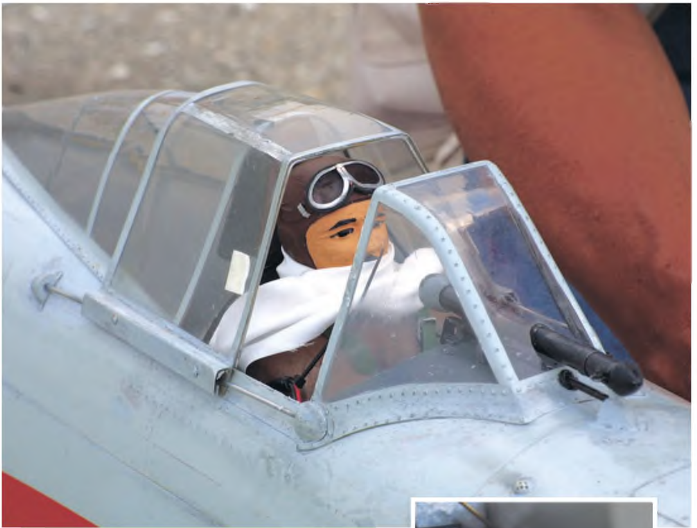
Note the multiple rivet lines on the canopy frames on Takashi Saruwatari's Nakajima Army Type 97. Sliding canopy guide on this one is an external rail.
