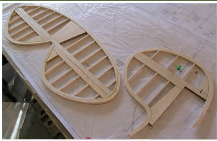
Nothing complicated about the tail surfaces. Just fill in those outlines with a few laser cut parts and some sticks.
