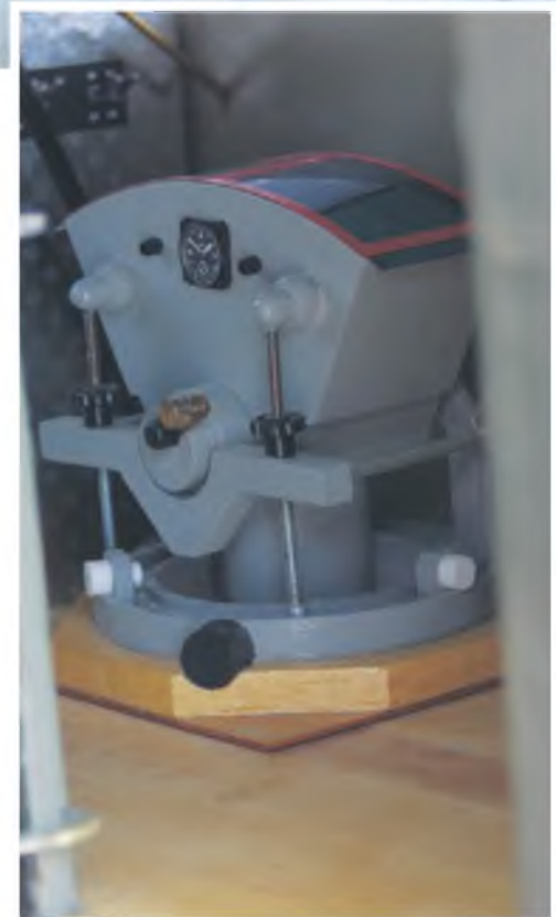
An extreme and unique piece of cockpit furniture in Berk Hazeborg's Koolhoven FK 49 is this aerial survey camera.
