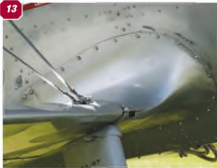
12: Fuselage centre section showing the wing bracing wires and centre section wing strut anchor points. 13: Lower wing fillet and detail of wing bracing wire anchor point. 14: Further view of the lower wing fillet and louvres in the engine cowl. 15: Upper wing centre section detail. 16: Interplane wing struts and detail of the streamlined bracing wires.
