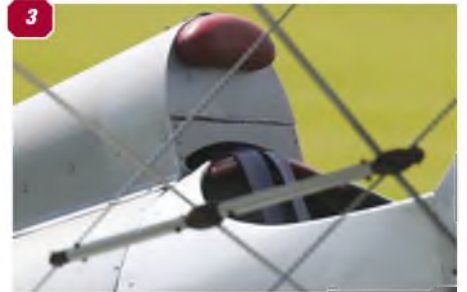
1: A view down into the cockpit well, showing instrument panel, control column and compass. Note also the hinged cockpit access down on the left. 2: Profile of the cockpit rim. 3: Pilot's headrest on the top of the dorsal fuselage fairing. 4: View into the rear of the cockpit well, showing seat and pilot's safety straps. 5: View into the cockpit showing the top of the instrument panel, windscreen and padded head protector. 6: Another view into the cockpit well, showing the pilot's seat. 7-10: Details of the engine cowl, showing louves, air scoops and bulges. Note four-pipe exhaust stack in the bottom of the cowl and the oil coolers, rear of the cowl bottom panel. Centre-section struts, wing fillet and undercarriage attachment also revealed.
