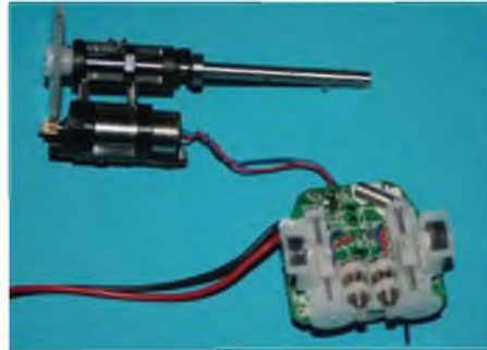
The modified mainframe from the fixed pitch model demonstrates that it may even be possible to make use of the motor and gearbox.
