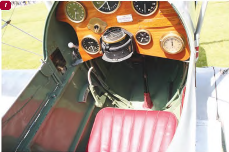
1: A view down into the cockpit well, showing instrument panel, control column and compass. Note also the hinged cockpit access down on the left. 2: Profile of the cockpit rim. 3: Pilot's headrest on the top of the dorsal fuselage fairing. 4: View into the rear of the cockpit well, showing seat and pilot's safety straps. 5: View into the cockpit showing the top of the instrument panel, windscreen and padded head protector. 6: Another view into the cockpit well, showing the pilot's seat. 7-10: Details of the engine cowl, showing louves, air scoops and bulges. Note four-pipe exhaust stack in the bottom of the cowl and the oil coolers, rear of the cowl bottom panel. Centre-section struts, wing fillet and undercarriage attachment also revealed.
