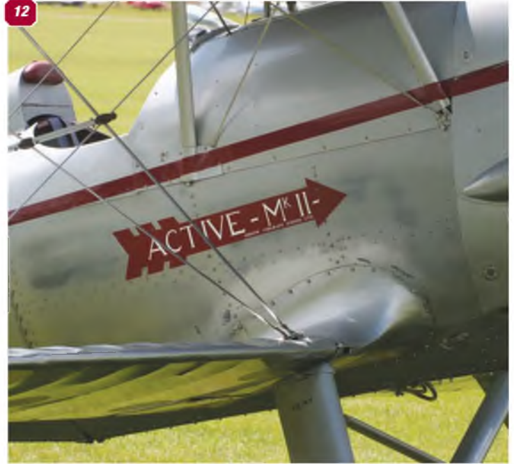
12: Fuselage centre section showing the wing bracing wires and centre section wing strut anchor points. 13: Lower wing fillet and detail of wing bracing wire anchor point. 14: Further view of the lower wing fillet and louvres in the engine cowl. 15: Upper wing centre section detail. 16: Interplane wing struts and detail of the streamlined bracing wires.
