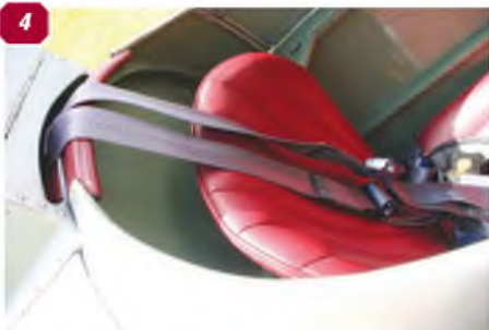
1: A view down into the cockpit well, showing instrument panel, control column and compass. Note also the hinged cockpit access down on the left. 2: Profile of the cockpit rim. 3: Pilot's headrest on the top of the dorsal fuselage fairing. 4: View into the rear of the cockpit well, showing seat and pilot's safety straps. 5: View into the cockpit showing the top of the instrument panel, windscreen and padded head protector. 6: Another view into the cockpit well, showing the pilot's seat. 7-10: Details of the engine cowl, showing louves, air scoops and bulges. Note four-pipe exhaust stack in the bottom of the cowl and the oil coolers, rear of the cowl bottom panel. Centre-section struts, wing fillet and undercarriage attachment also revealed.
