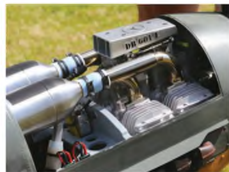
Andreas from Legendary Fighters showed me the impressive twin exhausts and his very clever close-fitting air-cooling ducting on his Me 109.
