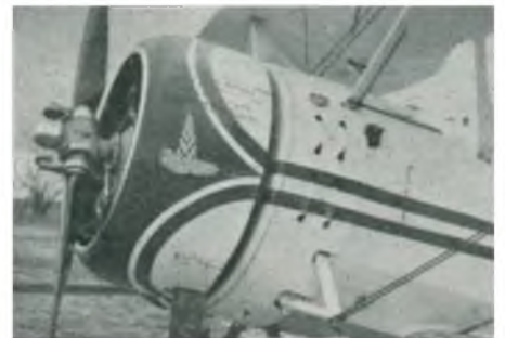
Cowl for the Warner radial engine came from a Fairchild F.24 'Argus'.
