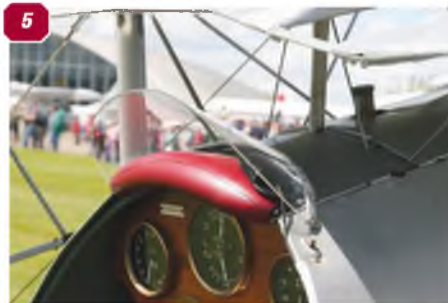
1: A view down into the cockpit well, showing instrument panel, control column and compass. Note also the hinged cockpit access down on the left. 2: Profile of the cockpit rim. 3: Pilot's headrest on the top of the dorsal fuselage fairing. 4: View into the rear of the cockpit well, showing seat and pilot's safety straps. 5: View into the cockpit showing the top of the instrument panel, windscreen and padded head protector. 6: Another view into the cockpit well, showing the pilot's seat. 7-10: Details of the engine cowl, showing louves, air scoops and bulges. Note four-pipe exhaust stack in the bottom of the cowl and the oil coolers, rear of the cowl bottom panel. Centre-section struts, wing fillet and undercarriage attachment also revealed.
