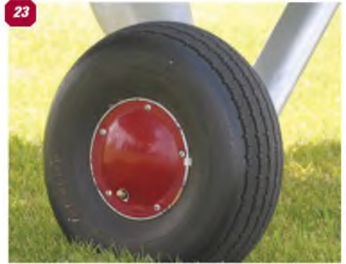
21: Full frontal view of the main undercarriage showing the oleo shock struts and main axle members. 22: Side view shows the shape of the struts. 23: Wheels hub and doughnut type tyres. 24: The main undercarriage, viewed from the rear. 25: Further view of the tailcone. 26: Tailplane and elevator - note the aerodynamic balance. 27: View along the upper wing showing the aileron and its control rod. 28: A full close-up of the wing fairing. 29: Upper wing centre section - top side. 30: Close-up of the aileron control horn and drive rod. 31: Lower wing bracing wing anchor point. 32: Wing strut anchor point showing the streamlined fairing.
