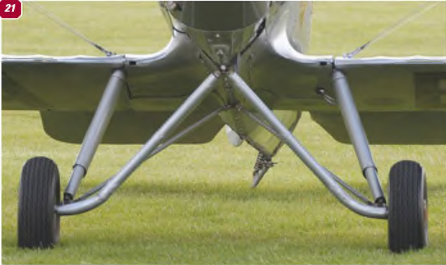
21: Full frontal view of the main undercarriage showing the oleo shock struts and main axle members. 22: Side view shows the shape of the struts. 23: Wheels hub and doughnut type tyres. 24: The main undercarriage, viewed from the rear. 25: Further view of the tailcone. 26: Tailplane and elevator - note the aerodynamic balance. 27: View along the upper wing showing the aileron and its control rod. 28: A full close-up of the wing fairing. 29: Upper wing centre section - top side. 30: Close-up of the aileron control horn and drive rod. 31: Lower wing bracing wing anchor point. 32: Wing strut anchor point showing the streamlined fairing.
