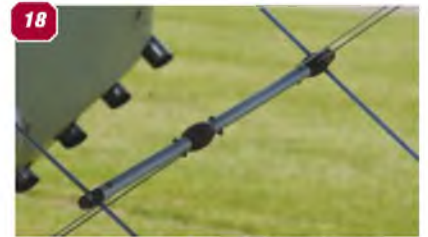
17: Further view of the wing interplane strut. 18: Detail of the spacer bar that steadies the backing wires at their cross-over points. 19: Detail of the 'boot' fairing on the lower end of the interplane strut. Upper attachment point similar. Note also the pitot head. 20: The sprung metal tailskid. Note also the stitching line of the fabric covering.
