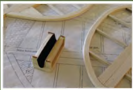
Tail surfaces sanded, and the rather neat little tool Pat made for rounding off the edges.
