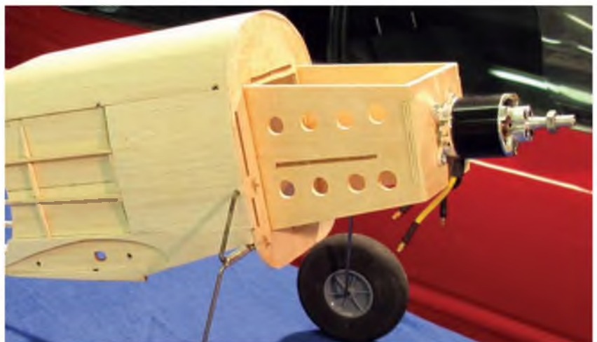
The combined motor mount and battery tray is fitted to the firewall AFTER you finish messing about with cowl parts tacked in place for shaping.
