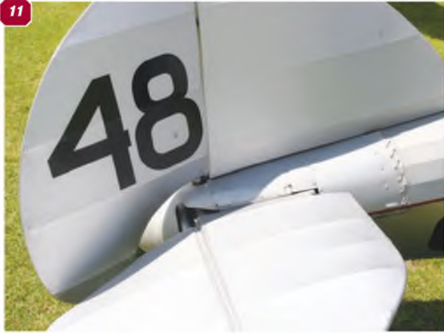
11: Tailplane, fin and rudder. Note the stitching below the fin.
