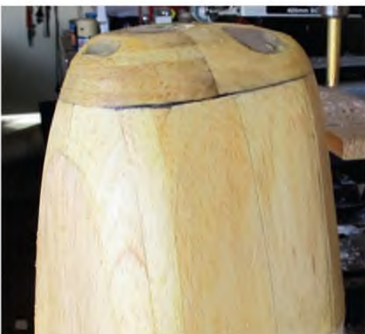
Once it was all shaped Pat treated the cowl to some reinforcing GRP which aids getting a smooth finish at the same time.
