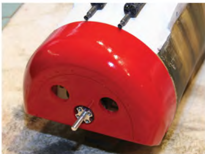
Once painted the CA sealed, and much sanded, cowl paints up looking just like metal.
