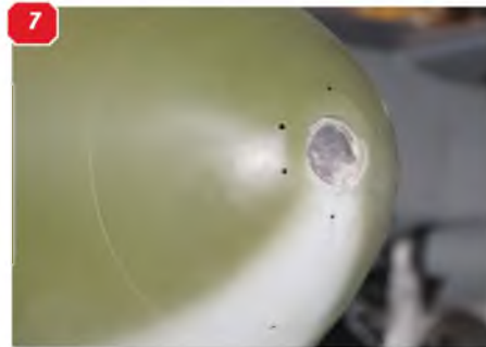
1: Head-on, the fuselage presents an almost benign cheery face, even with for 30mm cannon visible! 2-4: The cockpit canopy provided the pilot with good all-round visibility. 5: Spent 30mm cartridge ejectors - two either side of the lower fuselage nose. 6: Wing-to-fuselage fairing at the wing leading edge. 7: nose-mounted landing light. 8 & 9: Two views of the aerodynamically clean engine nacelle. 10: Nacelle panel detail showing the latched main inspection panel. 11: Front of the engine nacelle, showing the domed internal fairing.
