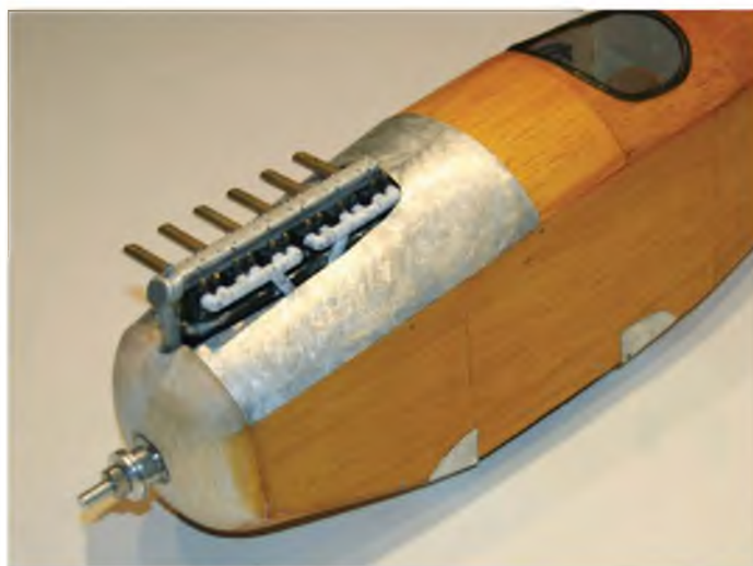
However, nothing represents metal quite like the real thing. Especially if you need a brushed effect finish. The wood area is shellac over balsa.
