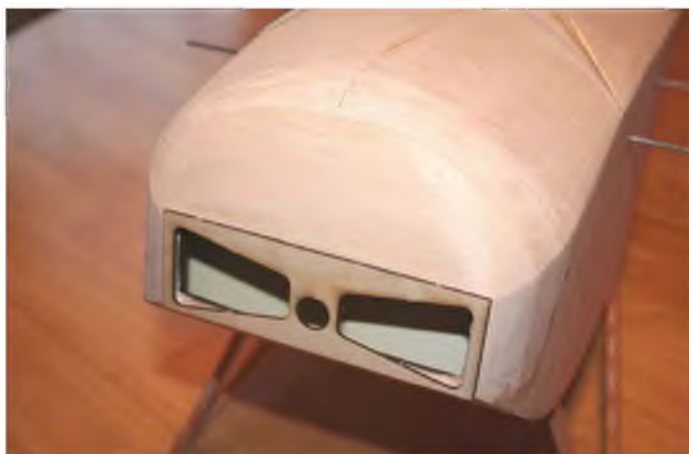
The nicely sanded nose of the author's Ponnier all ready for priming.
