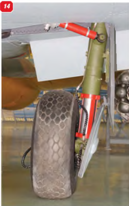
12: Shape of the wing-to-nacelle fairing at the wing trailing edge. 13: Head-on view of the wing-to-nacelle fairing. 14 & 15: Two views of the main undercarriage leg, which is very short. 16: Main undercarriage inner doors. 17: Tailplane, showing the trim tab. 18: Further view of the tailcone, showing rudder trim tab and elevators. 19: Rudder trim tab drive arm detail. 20: Tail light positioned at the base of the rudder. 21 & 22: Two further views of the fin and rudder showing the rudder hinge line and trim tab.
