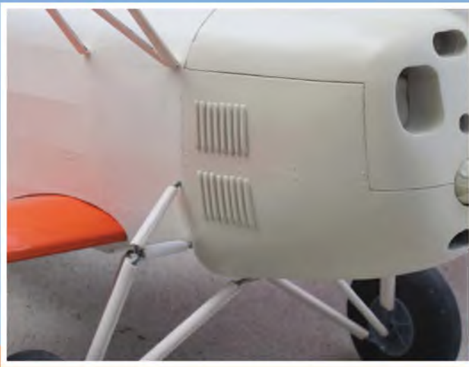
With the u/c and c/s struts plugged into their tubes the cowling separation line is clearly visible in this shot.
