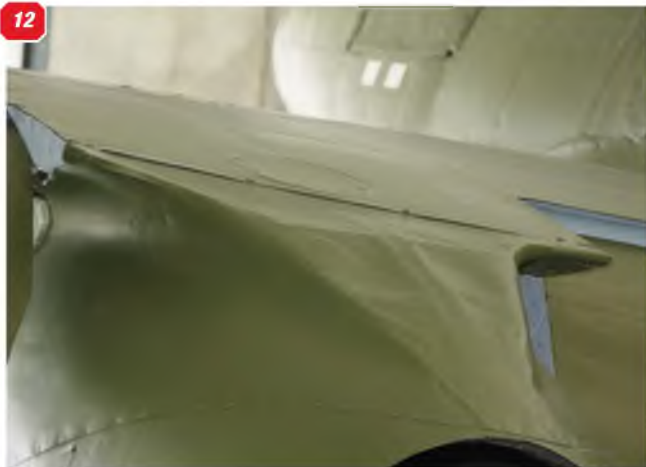
12: Shape of the wing-to-nacelle fairing at the wing trailing edge. 13: Head-on view of the wing-to-nacelle fairing. 14 & 15: Two views of the main undercarriage leg, which is very short. 16: Main undercarriage inner doors. 17: Tailplane, showing the trim tab. 18: Further view of the tailcone, showing rudder trim tab and elevators. 19: Rudder trim tab drive arm detail. 20: Tail light positioned at the base of the rudder. 21 & 22: Two further views of the fin and rudder showing the rudder hinge line and trim tab.
