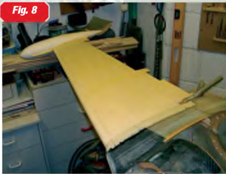
Two views of the fully surface panelled wings, prepared for rivet-live detailing.
