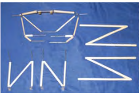
The wire parts and interplane struts all faired and sanded. Note that the front legs don't get joined until after fitting to the fuselage.
