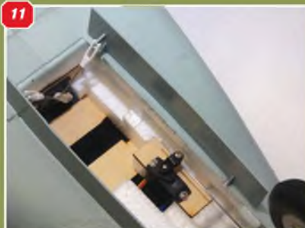
10 Servo at the rear of the nose undercarriage well is sequenced with the undercarriage leg to close after the leg has tucked away and opens the doors before the leg extends. 11 View of the noseleg steering servo in the front wheel well. 12 The forward wheel well cover closes and opens with the leg, to which it is attached.
