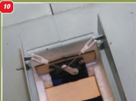
10 Servo at the rear of the nose undercarriage well is sequenced with the undercarriage leg to close after the leg has tucked away and opens the doors before the leg extends. 11 View of the noseleg steering servo in the front wheel well. 12 The forward wheel well cover closes and opens with the leg, to which it is attached.
