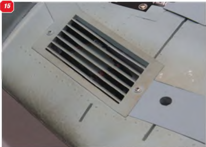
13: Realistic pilot figure in the cockpit. 14: The business end of the Me 252, well replicated by this plastic moulding of the gun ports for the 30mm cannon. 15: Detail of the cooling grille for the ESC in the wing underside, mounted between the fuselage and engine nacelle. 16: Tailcone, showing the rudder and elevator linkages - and the elevator servo mounted in the fin, under plastic cover.
