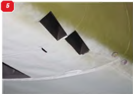
1: Head-on, the fuselage presents an almost benign cheery face, even with for 30mm cannon visible! 2-4: The cockpit canopy provided the pilot with good all-round visibility. 5: Spent 30mm cartridge ejectors - two either side of the lower fuselage nose. 6: Wing-to-fuselage fairing at the wing leading edge. 7: nose-mounted landing light. 8 & 9: Two views of the aerodynamically clean engine nacelle. 10: Nacelle panel detail showing the latched main inspection panel. 11: Front of the engine nacelle, showing the domed internal fairing.
