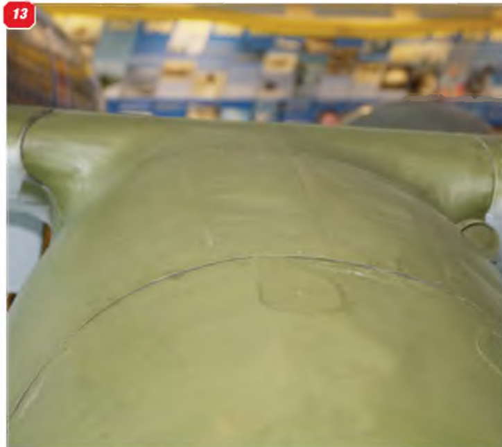
12: Shape of the wing-to-nacelle fairing at the wing trailing edge. 13: Head-on view of the wing-to-nacelle fairing. 14 & 15: Two views of the main undercarriage leg, which is very short. 16: Main undercarriage inner doors. 17: Tailplane, showing the trim tab. 18: Further view of the tailcone, showing rudder trim tab and elevators. 19: Rudder trim tab drive arm detail. 20: Tail light positioned at the base of the rudder. 21 & 22: Two further views of the fin and rudder showing the rudder hinge line and trim tab.
