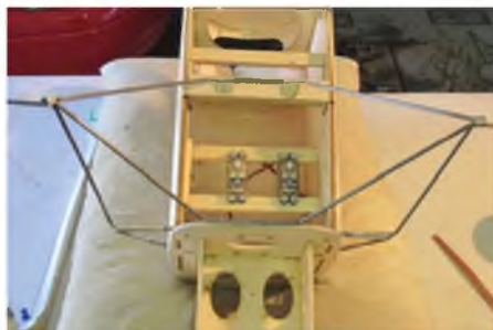
How the u/c fits onto the fuselage. You can see that only one side is soldered up at this stage.
