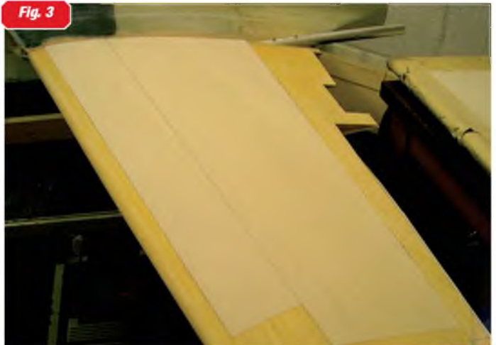
The second paper panel applied. The paper for this panel did not run the full length of the panel shape with the paper in the require stretch direction and an overlap of 2mm was necessary.
