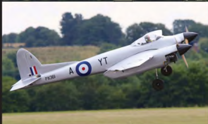
DH Hornet by Karl Mander. 1: 4.5 scale, powered by Zenoh 62 driving 23X10 props. 114 inch in span and weighs 19kg.
