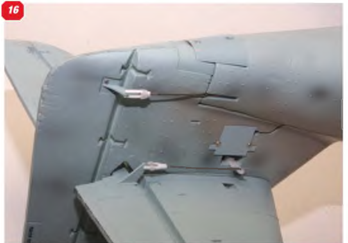
13: Realistic pilot figure in the cockpit. 14: The business end of the Me 252, well replicated by this plastic moulding of the gun ports for the 30mm cannon. 15: Detail of the cooling grille for the ESC in the wing underside, mounted between the fuselage and engine nacelle. 16: Tailcone, showing the rudder and elevator linkages - and the elevator servo mounted in the fin, under plastic cover.
