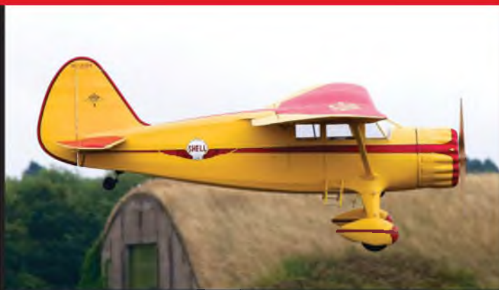
Pat Cuss's lovely Stinson SR16, built to one third scale, 166" in span, and powered by DA 150 twin.
