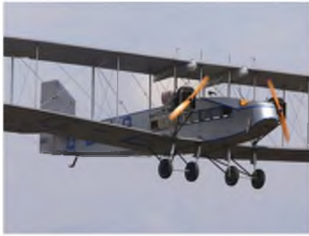
Don Billingham's huge HP W10 flown by Steve Holland. 197" (5m) span, powered by two Laser 100s twin 4-stroke, driving 28"x8" props.
