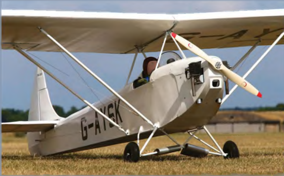
Impressive Luton Minor by Tony Hill, powered by a DLA 112 with a 28"10" prop, 12' 6" span.
