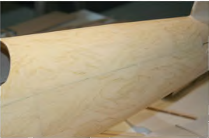
Here a more realistic grain pattern is printed onto the veneer applied to the rounded DVA fuselage very well.
