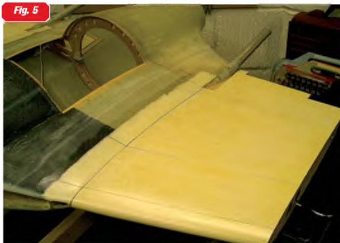
Fig. 5 A further view of the finished paper panelling - ready to move on to the next stage.
