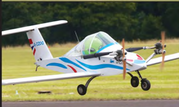
Colomaban Cri-Cri built to 75% scale, powered by two Zenoh 26s, and flown by Dave Hayfield.
