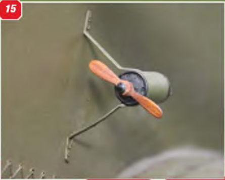
10: Fuselage centre section and interplane struts. 11: External mounted bomb on the fuselage underside. 12: Upper wing struts. The two circular finned details at the base of the struts replicate the wind driven fuel pumps of the full size. 13 & 14: Two views of the biplane tail assembly - plenty of rigging and strutting in there too. 15: Dummy wind-driven generator mounted on the forward fuselage left side. 16 & 17: Main undercarriage use Flair 4" bia. Vintage wheels.
