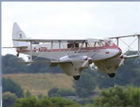
Ted Allinson's DH Rapide G-AGSH Jemma Meeson, powered by two DLE55s. 197" (5m) span, third scale, weighs 43 kgs.
