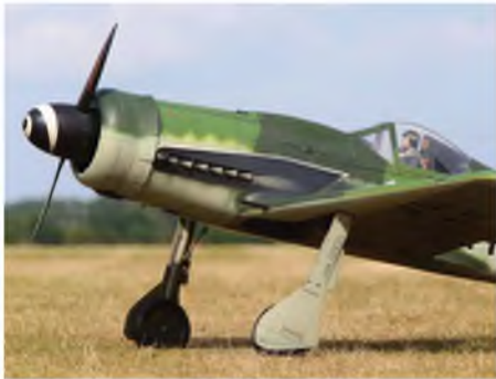
Focke Wulf Fw 190D by Phil Clark of Fighter Aces. Powered by a Zenoah 62, built to one-fifth scale, 83 inches in span, and weighs 33 lbs
