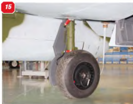
12: Shape of the wing-to-nacelle fairing at the wing trailing edge. 13: Head-on view of the wing-to-nacelle fairing. 14 & 15: Two views of the main undercarriage leg, which is very short. 16: Main undercarriage inner doors. 17: Tailplane, showing the trim tab. 18: Further view of the tailcone, showing rudder trim tab and elevators. 19: Rudder trim tab drive arm detail. 20: Tail light positioned at the base of the rudder. 21 & 22: Two further views of the fin and rudder showing the rudder hinge line and trim tab.
