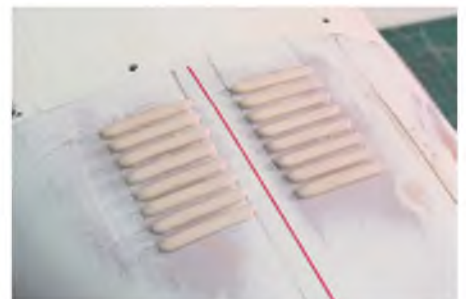
As you see, those effective looking louvers are nothing more than sanded strips of wood.
