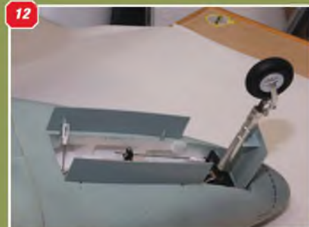
10 Servo at the rear of the nose undercarriage well is sequenced with the undercarriage leg to close after the leg has tucked away and opens the doors before the leg extends. 11 View of the noseleg steering servo in the front wheel well. 12 The forward wheel well cover closes and opens with the leg, to which it is attached.
