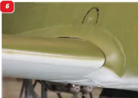
1: Head-on, the fuselage presents an almost benign cheery face, even with for 30mm cannon visible! 2-4: The cockpit canopy provided the pilot with good all-round visibility. 5: Spent 30mm cartridge ejectors - two either side of the lower fuselage nose. 6: Wing-to-fuselage fairing at the wing leading edge. 7: nose-mounted landing light. 8 & 9: Two views of the aerodynamically clean engine nacelle. 10: Nacelle panel detail showing the latched main inspection panel. 11: Front of the engine nacelle, showing the domed internal fairing.
