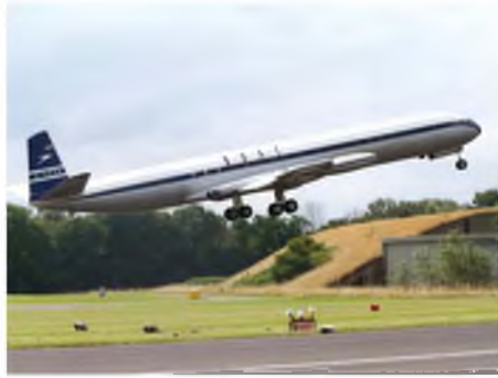
Majestic Comet 4, flown by Steve Rickett. Carries 8 litres of fuel, weighs 120lbs, powered by two Jetcat 120 gas turbines. Utterly convincing.
