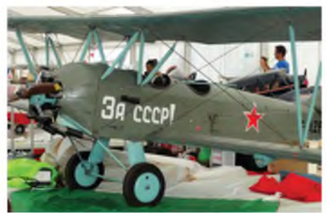
This Polikarpov Po2 from Japan had an interesting approach to modelling the engine. An SC 4 stroke radial was fitted, the crankcase painted to match the prototype and dummy exhausts to complete the picture.
