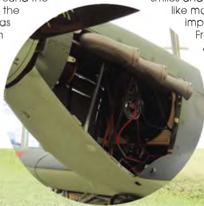
This Hawker Sea Hurricane had a large sound system installed behind the electric motor. The main speaker is just visible attached to the front bulkhead. There is a secondary speaker in the radiator.
