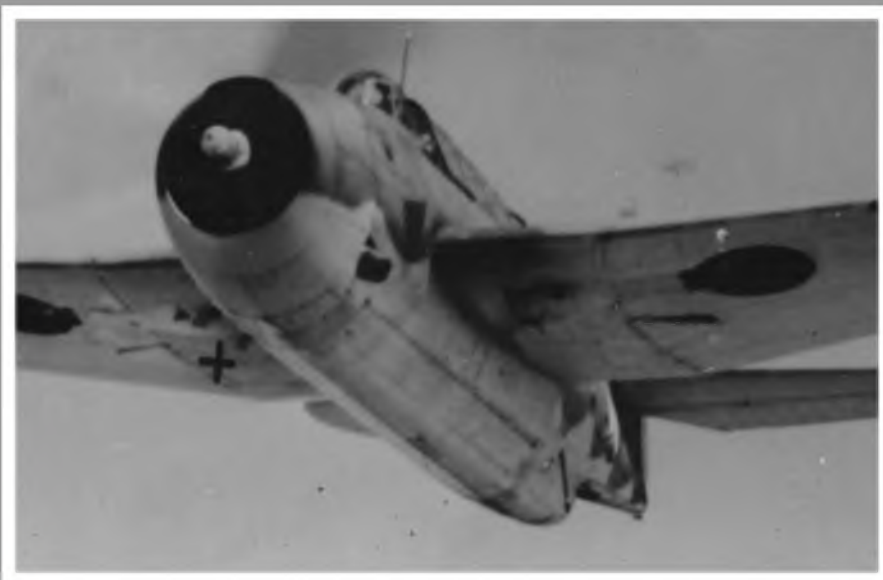
Another very early TBF-1 Avenger, showing the long 'birdcage' cockpit canopy. Although roomy by most standards, the two forward occupants were completely isolated from each other.
