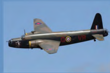
Geoff Graves' Tony Nijhuis Designs Wellington. 11 feet in span, powered by two Zenoah Z 26 petrol engines.
