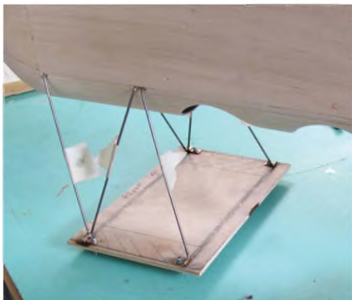
The simple jig used to assist with setting up the centre section struts while soldering. (see text)
