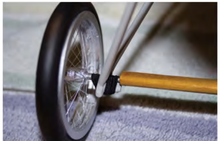
A slightly different technique, but the same basic principal sees the Albatros DIII u/c sprung.
