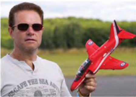
Tony Murphy's tiny Bae Hawk, electric ducted fan, 18" span, all foam construction, sourced from the internet.
