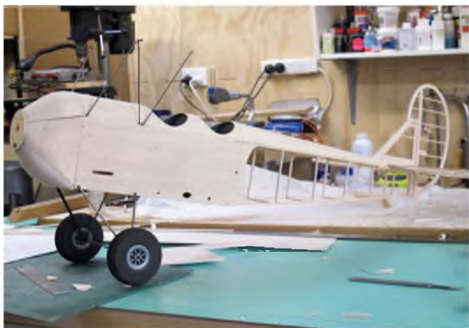
Here you see the shaped nose blocks and the ply motor mount fitted. The dummy engine will hide the motor nicely.
