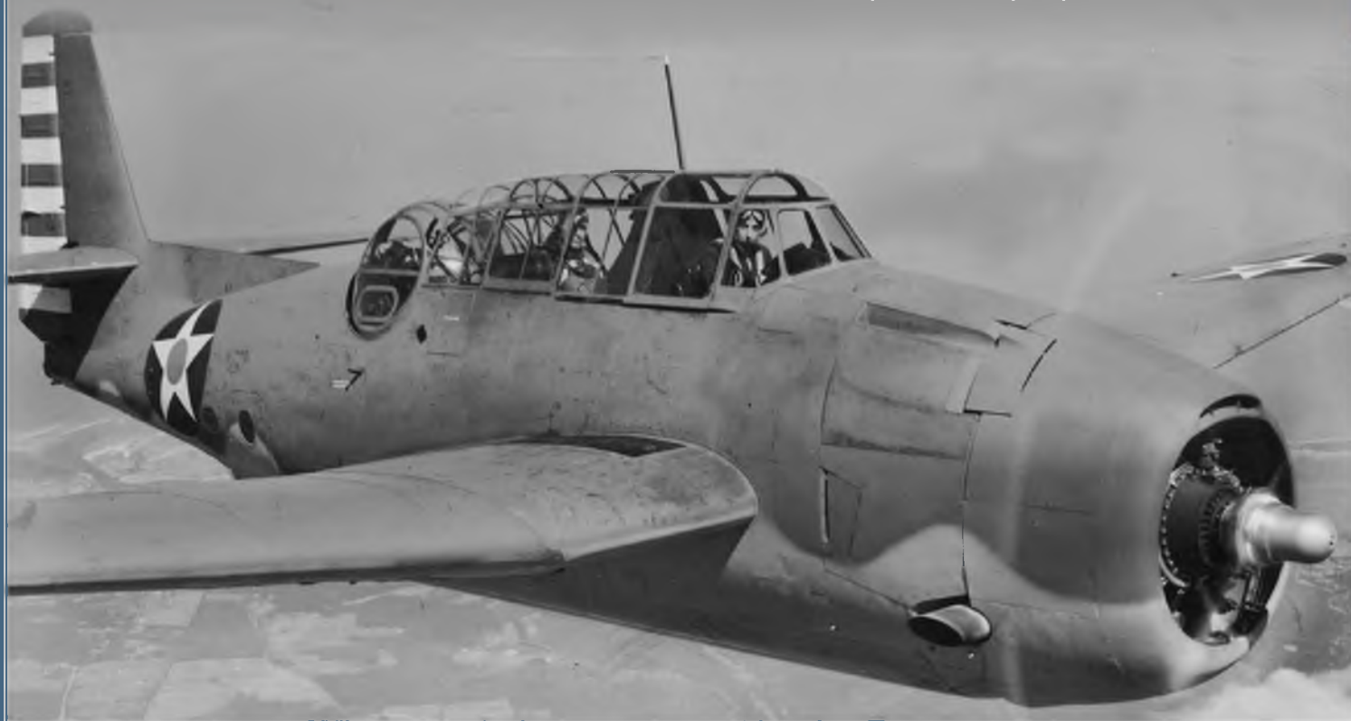
Another very early TBF-1 Avenger, showing the long 'birdcage' cockpit canopy. Although roomy by most standards, the two forward occupants were completely isolated from each other.
