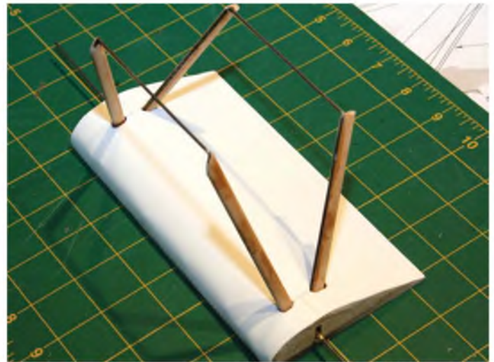
What you get to see after the axle wing is skinned and the u/c fairings added.
