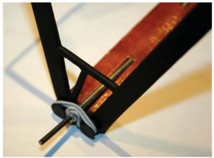
The centre of the laminated ply parts holds the axle centre while the elastic cord allows the ends to absorb landing shocks.
