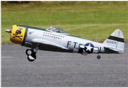
Mark Roberts' YT International P-47 powered by a PTE 36 petrol engine driving a 19"x8" prop. Spans 76" and weighs 8.5 lbs.
