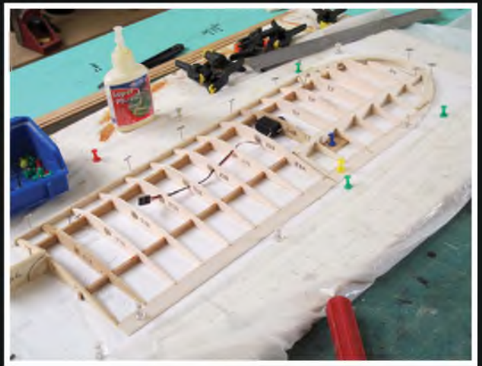
A lower wing panel under construction. The aileron servo lead needs to be extended but do fit the servos before the ribs are all glued in place.
