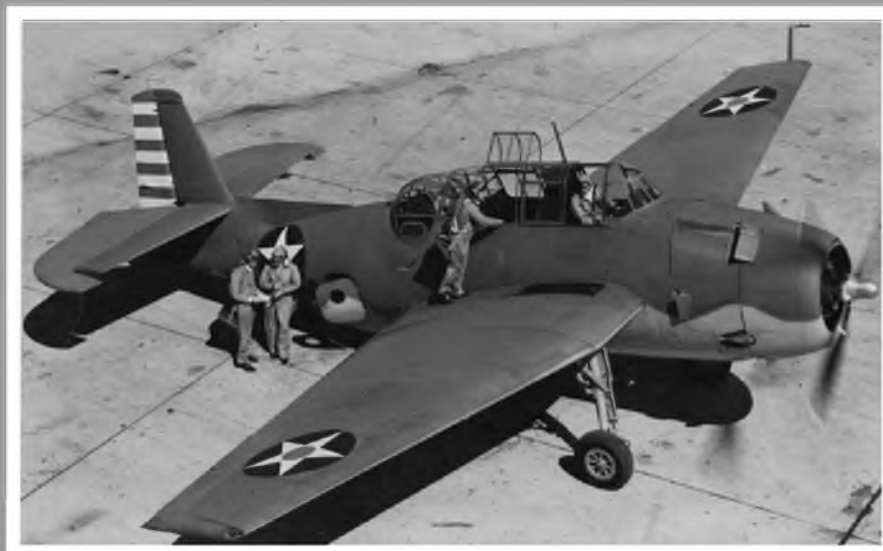
ABOVE: The red national insignia centres and the striped rudder identify this Grumman TBF-1 as one of the earliest produced. BELOW: Underside view reveals the big belly weapons bay and outward retracting main undercarriage.
