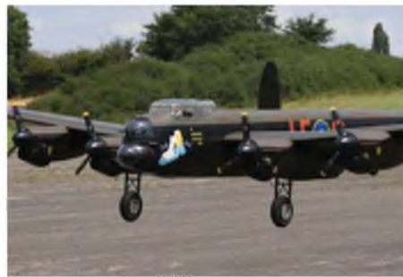
Geoff Graves' Tony Nijhuis Designs Lancaster. 17 feet in span, powered by four Zenoah 38 petrol engines.
