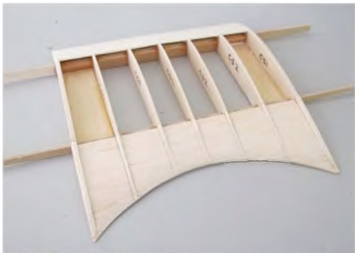
The top wing centre section, showing how Pat added false ribs at the trailing edge area.
