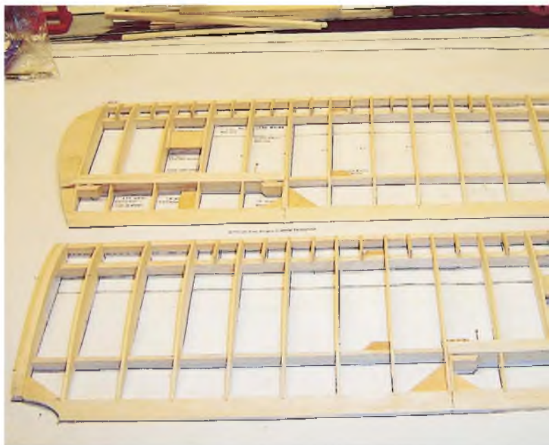
Basic wing structure is light and simple.
