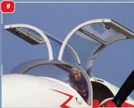
7: The Gemini has interesting glazing, all neatly executed. 8 & 9: You get some idea of the work in the gull-wing doors from these shots. Note scale catches and door handles. 10: Pilot in the office with full seating.
