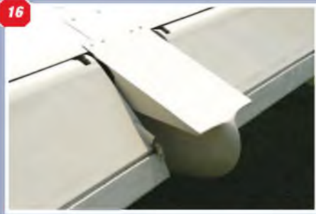
16 & 17: Central rear fuselage fairing between the elevators. 18: Elevator trim tab. 19 - 22: Fuselage cabin window detail and windscreen. 23: View over the wing showing the fuselage-to-wing fairing.
