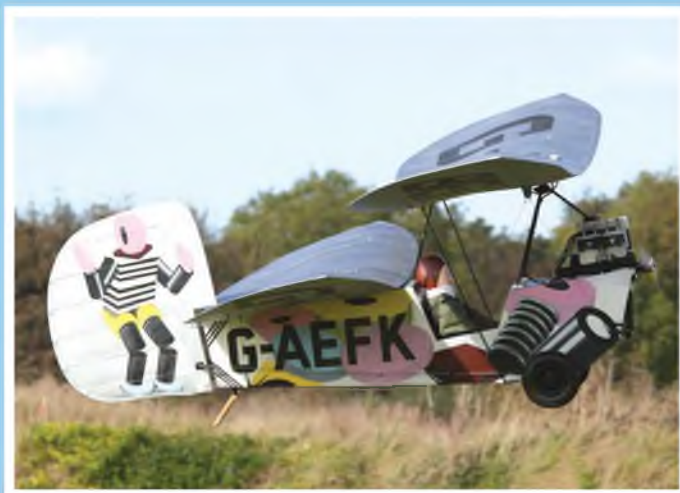
Ian Redshaw's HM 14 Flying Flea. Half scale model weighs 19 kgs and is powered by a Zenoah 62 petrol engine.
