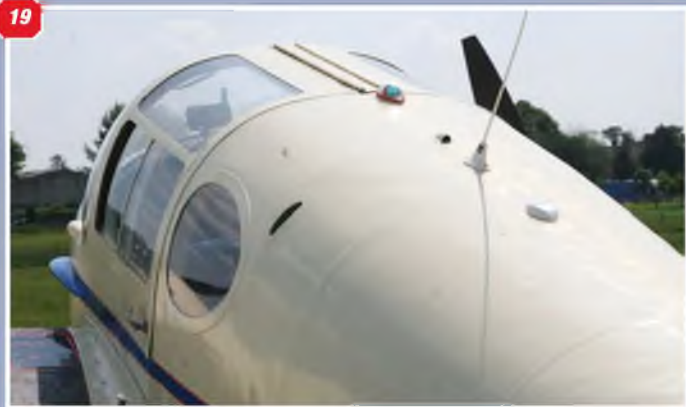
16 & 17: Central rear fuselage fairing between the elevators. 18: Elevator trim tab. 19 - 22: Fuselage cabin window detail and windscreen. 23: View over the wing showing the fuselage-to-wing fairing.
