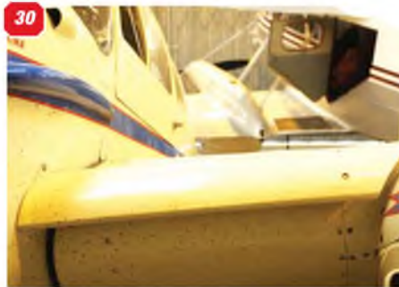
24: Aileron on fully skinned wing. 25: Wing tip aileron hinge, viewed from below. 26 & 27: Wing root, showing the cabin access tread plates left and right, plus the wing fairing. 28: Pitot head on left wing undersurface. 29 & 30: Two more views of the wing leading edge slats between the fuselage and engine nacelle. 31: Wing flap, in the 'up' position. 32: Left wing flap viewed from wing underside, showing the outer hinge and a further view of the pitot head. 33: Right wing flap, showing both hinges and the flap drive arm.
