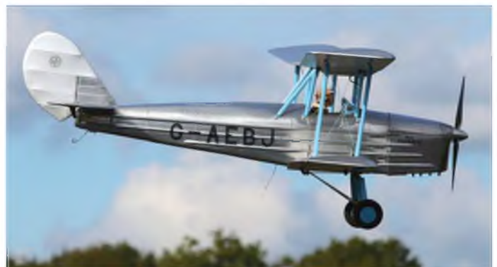
Tim Hooper's own-design Blackburn B2. 66" in span, Turnigy 42-50 motor, 14"x6" prop, and a 60 A ESC with a 5S 4000mAh battery pack.
