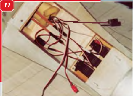
8: View of the wing fairing and wing underside air scoop on the finished model. 9: Underside of the finished wing, showing the wells for the undercarriage. 10: Installation, on the wing centre section upper surface, of the servo and air valve for switching the retracting undercarriage. 11: Side-by-side installation of the rudder, elevator and throttle servos in the fuselage. 12: Although the nose is slim, it hides MOST of the O.S. four stroke motor, but the muffler inevitably protrudes. 13: Detail of the nose, showing the dummy exhaust stacks. Details like this give realism.
