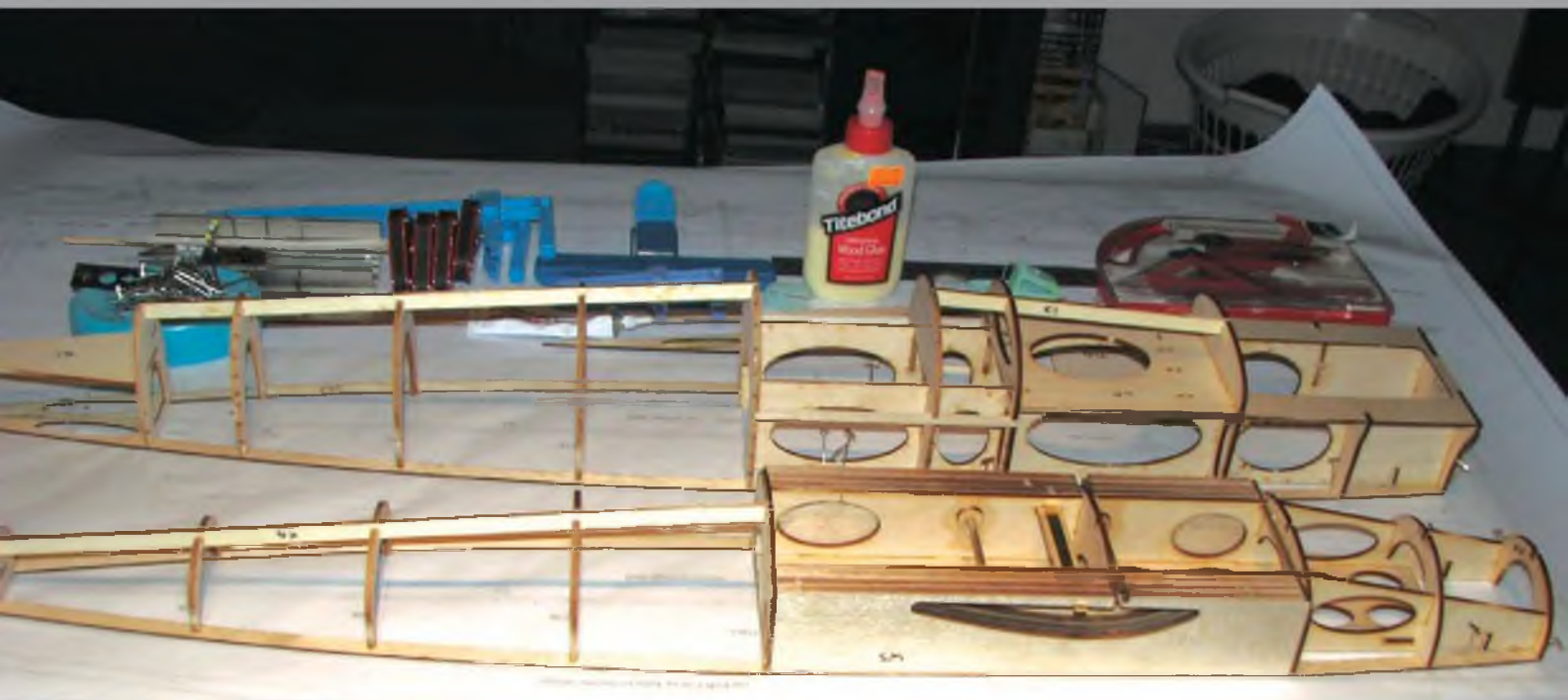
The two basic shell halves. This style of construction means you can do most of the work on the separate shells before joining them.
