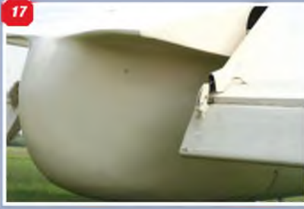
16 & 17: Central rear fuselage fairing between the elevators. 18: Elevator trim tab. 19 - 22: Fuselage cabin window detail and windscreen. 23: View over the wing showing the fuselage-to-wing fairing.
