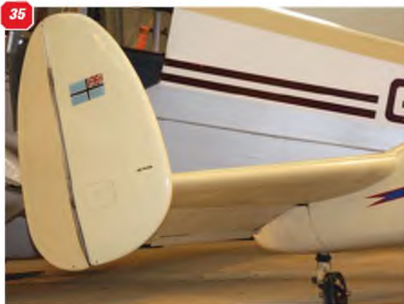
34: Fin and rudder. Note that the hinge line is not 'cuffed'. 35: General view of the tailplane and fin/rudder. 36: The non-retracting tailwheel unit.
