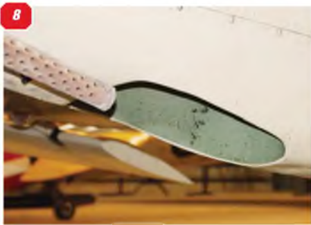
4: Engine exhaust pipe, exits below the engine nacelle. 5: Close-up of the fairing shroud at the exhaust pipe exit. 6 & 7: Two views of the front of the engine nacelle. Note that the engine exhaust pipe is offset from the centreline to clear the main undercarriage. 8: The open well in the bottom rear of the engine nacelle fits the main undercarriage wheel in the retracted position. 9: further view of the engine nacelle rear section. 10 & 11: Two views of the lower front of the engine nacelle showing the fixed air-exit gills.
