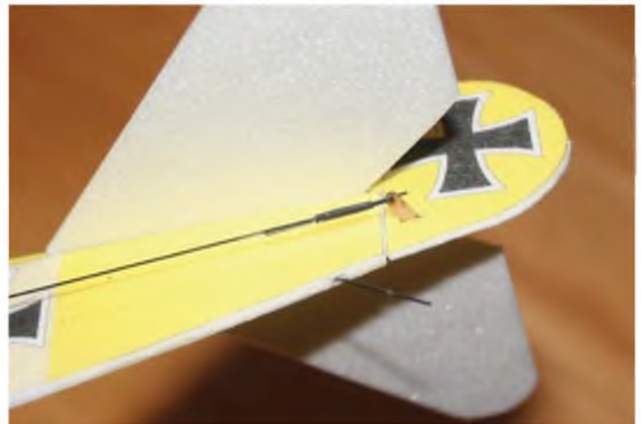
The 1/64 ply control horn is more than adequate for a model of this type. Here you are allowed to use a steel wire pushrod end.
