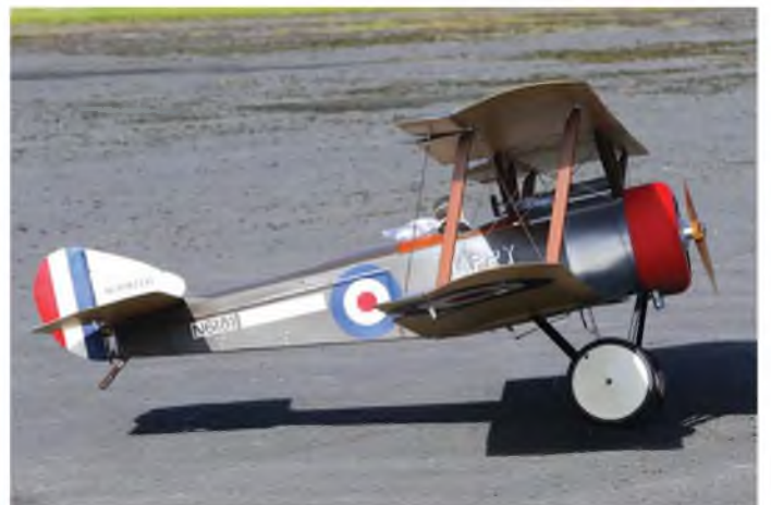
Ken Dallow's fine 1/3rd scale Sopwith Pup. 111" span, with a DLE 111 petrol engine.
