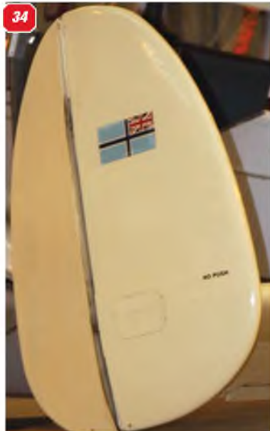
34: Fin and rudder. Note that the hinge line is not 'cuffed'. 35: General view of the tailplane and fin/rudder. 36: The non-retracting tailwheel unit.
