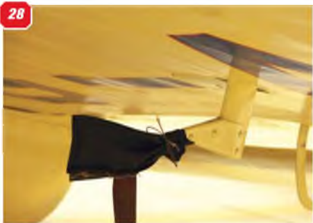
24: Aileron on fully skinned wing. 25: Wing tip aileron hinge, viewed from below. 26 & 27: Wing root, showing the cabin access tread plates left and right, plus the wing fairing. 28: Pitot head on left wing undersurface. 29 & 30: Two more views of the wing leading edge slats between the fuselage and engine nacelle. 31: Wing flap, in the 'up' position. 32: Left wing flap viewed from wing underside, showing the outer hinge and a further view of the pitot head. 33: Right wing flap, showing both hinges and the flap drive arm.
