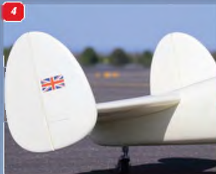
1: Original Super Tigre ST 2500 glow installation with in-cowl dustbin silencer. 2: The engine nacelles are quite slim, so the sidewinder mounted engine cylinder head protrudes. 3: Tail treatment is distinctively Miles. 4: The later Aries variants had bigger fin and rudder volumes than this Gemini. The model's tailwheel had to be tweaked to overcome ground-looping. 5: Trailing edge flaps produce a slight nose down attitude on deployment. 6: It is instructive to compare the relative areas of the aileron and flaps.
