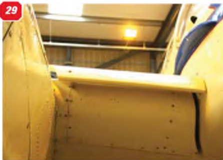
24: Aileron on fully skinned wing. 25: Wing tip aileron hinge, viewed from below. 26 & 27: Wing root, showing the cabin access tread plates left and right, plus the wing fairing. 28: Pitot head on left wing undersurface. 29 & 30: Two more views of the wing leading edge slats between the fuselage and engine nacelle. 31: Wing flap, in the 'up' position. 32: Left wing flap viewed from wing underside, showing the outer hinge and a further view of the pitot head. 33: Right wing flap, showing both hinges and the flap drive arm.
