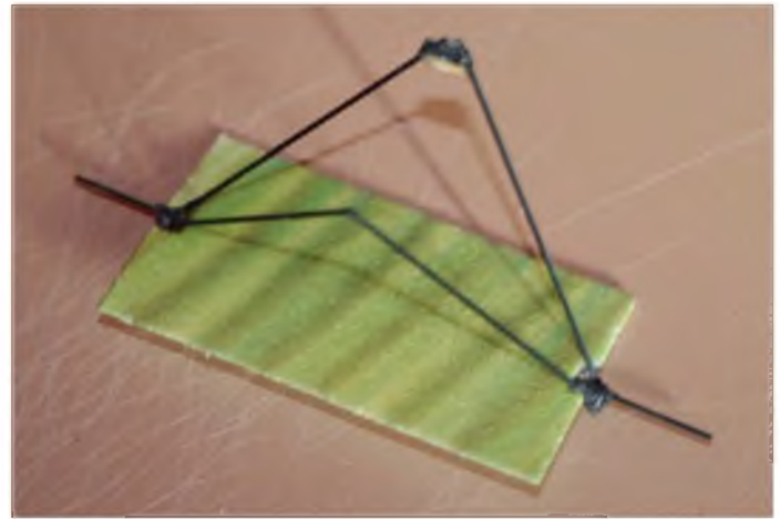
The u/c is assembled from 0.7 mm carbon rod, bound and glued using thread and CA. Uhu Por secures the axle wing.
