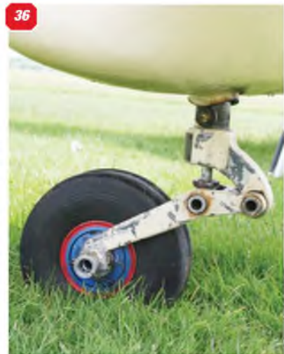
34: Fin and rudder. Note that the hinge line is not 'cuffed'. 35: General view of the tailplane and fin/rudder. 36: The non-retracting tailwheel unit.
