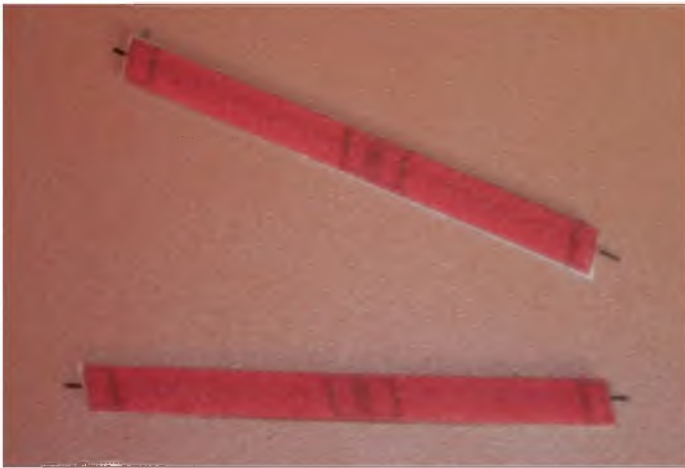
How the carbon rod is trapped between the i/p strut laminations to provide locating stubs at top and bottom.
