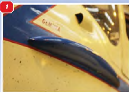
1: Detail of curved side-strake, on the fuselage, below and ahead of the windscreen. 2: Head-on view of the nose section and windscreen. 3: Fuselage forward section, also showing the wing leading edge slat, between the fuselage side and the engine nacelle.
