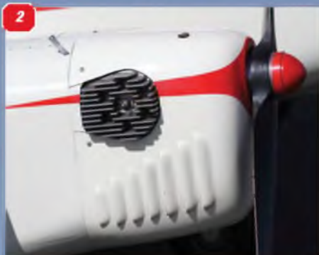
1: Original Super Tigre ST 2500 glow installation with in-cowl dustbin silencer. 2: The engine nacelles are quite slim, so the sidewinder mounted engine cylinder head protrudes. 3: Tail treatment is distinctively Miles. 4: The later Aries variants had bigger fin and rudder volumes than this Gemini. The model's tailwheel had to be tweaked to overcome ground-looping. 5: Trailing edge flaps produce a slight nose down attitude on deployment. 6: It is instructive to compare the relative areas of the aileron and flaps.
