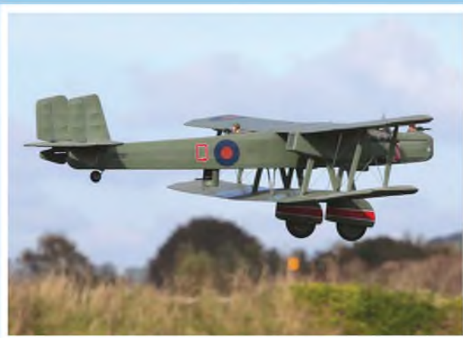
Dennis Richardson's Handley Page Heyford built to 1/13th scale. 69" span, weighs 6 1/2 lbs, twin OS .30 power.
