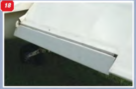
16 & 17: Central rear fuselage fairing between the elevators. 18: Elevator trim tab. 19 - 22: Fuselage cabin window detail and windscreen. 23: View over the wing showing the fuselage-to-wing fairing.
