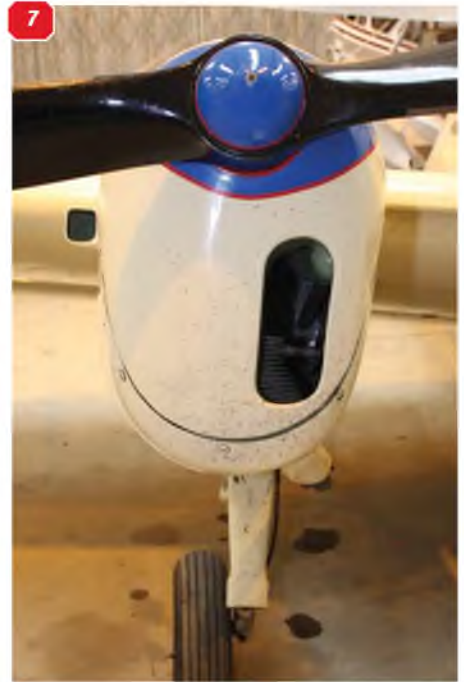
4: Engine exhaust pipe, exits below the engine nacelle. 5: Close-up of the fairing shroud at the exhaust pipe exit. 6 & 7: Two views of the front of the engine nacelle. Note that the engine exhaust pipe is offset from the centreline to clear the main undercarriage. 8: The open well in the bottom rear of the engine nacelle fits the main undercarriage wheel in the retracted position. 9: further view of the engine nacelle rear section. 10 & 11: Two views of the lower front of the engine nacelle showing the fixed air-exit gills.
