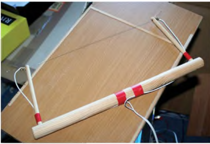
Hardly high tech but this simple foam slicing set-up works well.
