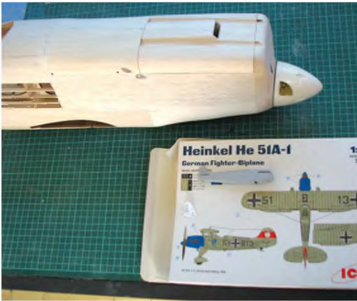
The plastic model Craig used as a guide and the resulting nicely shaped nose section.
