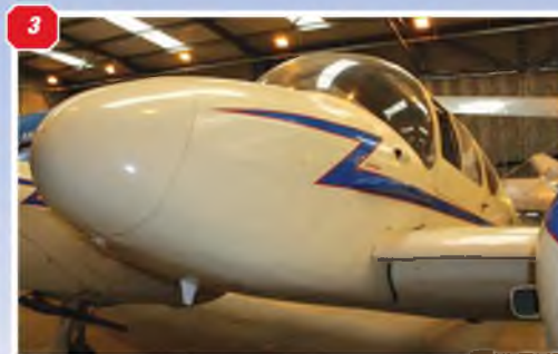
1: Detail of curved side-strake, on the fuselage, below and ahead of the windscreen. 2: Head-on view of the nose section and windscreen. 3: Fuselage forward section, also showing the wing leading edge slat, between the fuselage side and the engine nacelle.
