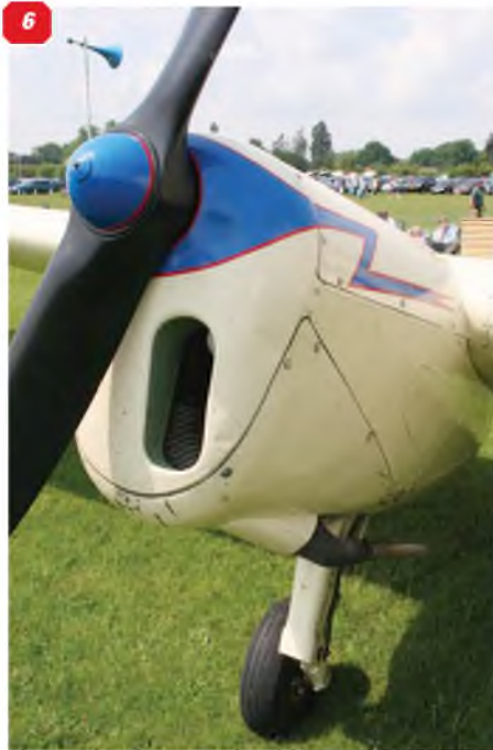
4: Engine exhaust pipe, exits below the engine nacelle. 5: Close-up of the fairing shroud at the exhaust pipe exit. 6 & 7: Two views of the front of the engine nacelle. Note that the engine exhaust pipe is offset from the centreline to clear the main undercarriage. 8: The open well in the bottom rear of the engine nacelle fits the main undercarriage wheel in the retracted position. 9: further view of the engine nacelle rear section. 10 & 11: Two views of the lower front of the engine nacelle showing the fixed air-exit gills.
