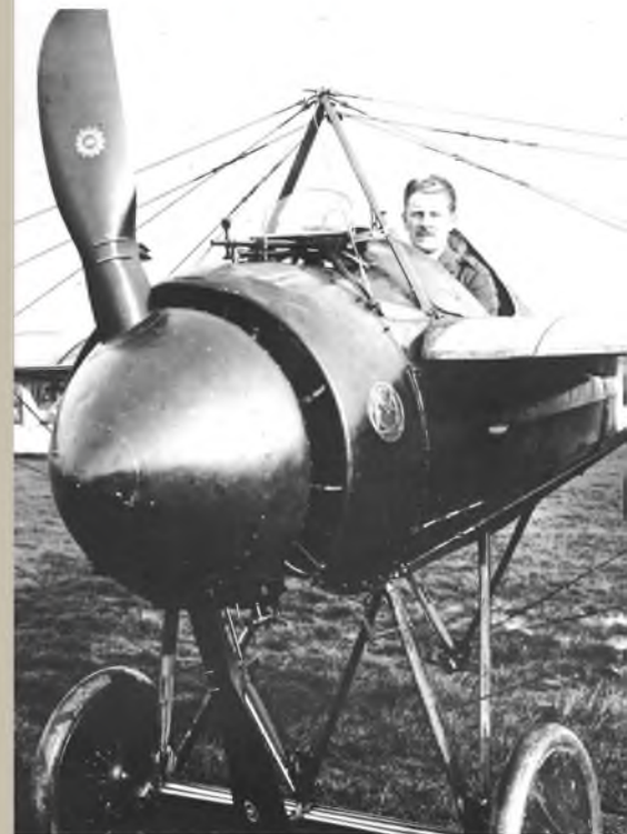
Lt. Bayetto again, installed in his Type N. Note the Hotchkiss gun, with barrel pointing at the deflector plate on the propeller.
