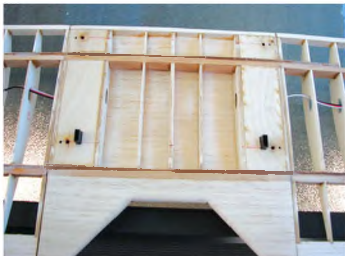
The top wing centre section showing the strut mount positions and how Craig has let in the servo lead extensions.
