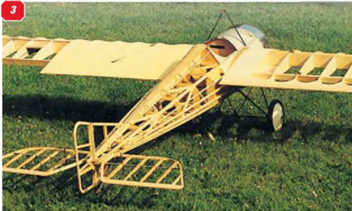
1: The uncovered airframe, showing the open frame, stringered rear fuselage. 2: Detail of the uncovered airframe, showing the shape of the wing structure in the tip area. 3 & 4: These two views of the uncovered airframe reveal a quite simple basic structure. One of the obvious deviations from true-scale is the thickness of the wing section but this change, in the interest of practicality, is not noticeable when the model is airborne. 5: Rear end, showing the open-frame structure and the tail skid. 6: Further detail of the tail cone, showing the tailskid with its bracing and the pivot tube on the all-flying tailplane. 7: The tailplane showing the tubular spar that acts as a pivot for the all-flying control movement.
