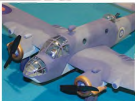
Chris Fouweather's stunning and innovative Bristol Beaufort R/C. Weighs 79 grams. Heat moulded Depron structure.
