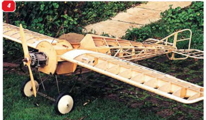
1: The uncovered airframe, showing the open frame, stringered rear fuselage. 2: Detail of the uncovered airframe, showing the shape of the wing structure in the tip area. 3 & 4: These two views of the uncovered airframe reveal a quite simple basic structure. One of the obvious deviations from true-scale is the thickness of the wing section but this change, in the interest of practicality, is not noticeable when the model is airborne. 5: Rear end, showing the open-frame structure and the tail skid. 6: Further detail of the tail cone, showing the tailskid with its bracing and the pivot tube on the all-flying tailplane. 7: The tailplane showing the tubular spar that acts as a pivot for the all-flying control movement.
