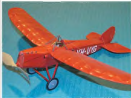
Dave Crompton's Bristol M1C Gypsy Racer from the Derek Buckmaster plan. 19" in span, weighs 30 grams. Esaki tissue and airbrushed Humbrol enamels.
