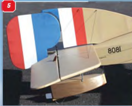
1: The radiator was placed above and behind the engine. Note filler cap. 2: Torpedo and restraints are nicely modelled. The dolly drops off on take-off. 3: The bay and rigging detail is impressive. 4: Dinghy-like tail float has a water-rudder, too. Note scale wire skid. 5: Graceful and rather interesting fin and rudder. Note slender scale size of bracing wire. 6: Tail end of the torpedo - note propeller!
