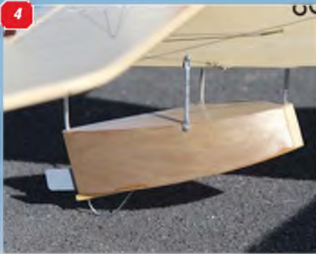
1: The radiator was placed above and behind the engine. Note filler cap. 2: Torpedo and restraints are nicely modelled. The dolly drops off on take-off. 3: The bay and rigging detail is impressive. 4: Dinghy-like tail float has a water-rudder, too. Note scale wire skid. 5: Graceful and rather interesting fin and rudder. Note slender scale size of bracing wire. 6: Tail end of the torpedo - note propeller!
