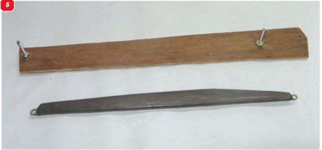
2: Example of cabane struts that splay outwards, showing the metal mounting shoes at the tops of the struts. 3: Cabane struts that converge at the upper wing mounting position, showing the wing joiners. 4: Forming the wire loop attachments that fit at each end of the wing struts. 5: Finished struts and jig that spaces the loops at the strut ends exactly. 6: All the parts that go to make up the struts, including the metal mounting brackets. 7: Bracing wire/ strut brackets in place on wing. Note the aluminium cable swages to secure the rigging wires.
