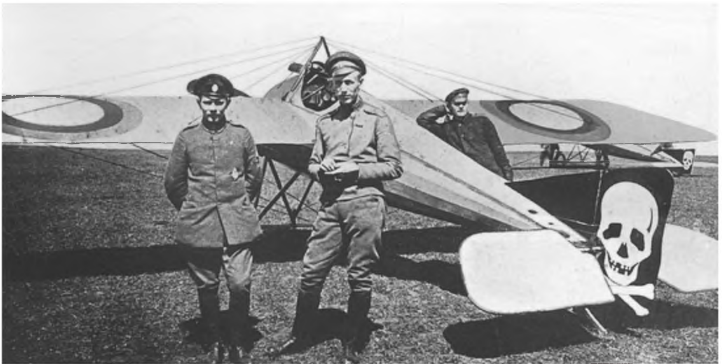
Physically, there was very little difference between the M.S. Type N and the Type I, of which this is an example supplied to the Imperial Russian Air Service. The figure on the left is a captured German airman. Roundels are red outer, blue middle and white centre. Fin and rudder in black.
