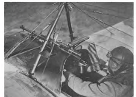
ABOVE: Detail of cockpit and Hotchkiss gun installation. LEFT: A Morane Saulnier Type I in French service. 'Kepi' head gear is the give-away as to the pilot's nationality!
