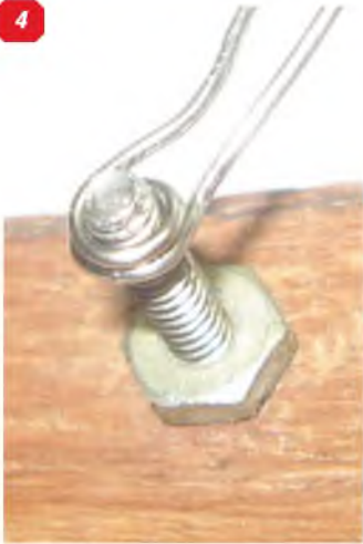
2: Example of cabane struts that splay outwards, showing the metal mounting shoes at the tops of the struts. 3: Cabane struts that converge at the upper wing mounting position, showing the wing joiners. 4: Forming the wire loop attachments that fit at each end of the wing struts. 5: Finished struts and jig that spaces the loops at the strut ends exactly. 6: All the parts that go to make up the struts, including the metal mounting brackets. 7: Bracing wire/ strut brackets in place on wing. Note the aluminium cable swages to secure the rigging wires.
