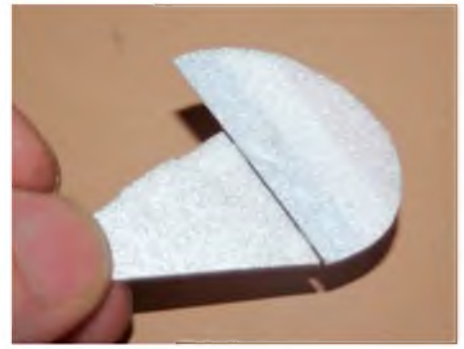
Although they're hard to see, there are two narrow strips of Blendederm tape used to hinge the rudder before joining the laminated halves.
