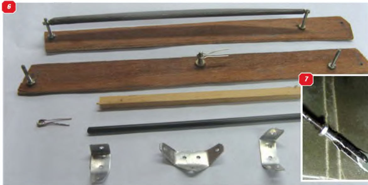
2: Example of cabane struts that splay outwards, showing the metal mounting shoes at the tops of the struts. 3: Cabane struts that converge at the upper wing mounting position, showing the wing joiners. 4: Forming the wire loop attachments that fit at each end of the wing struts. 5: Finished struts and jig that spaces the loops at the strut ends exactly. 6: All the parts that go to make up the struts, including the metal mounting brackets. 7: Bracing wire/ strut brackets in place on wing. Note the aluminium cable swages to secure the rigging wires.
