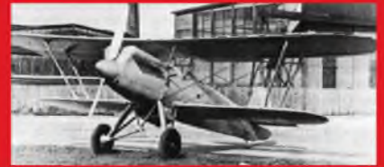
Forerunner of the Heinkel He 52, the He 49 featured a different undercarriage arrangement.
