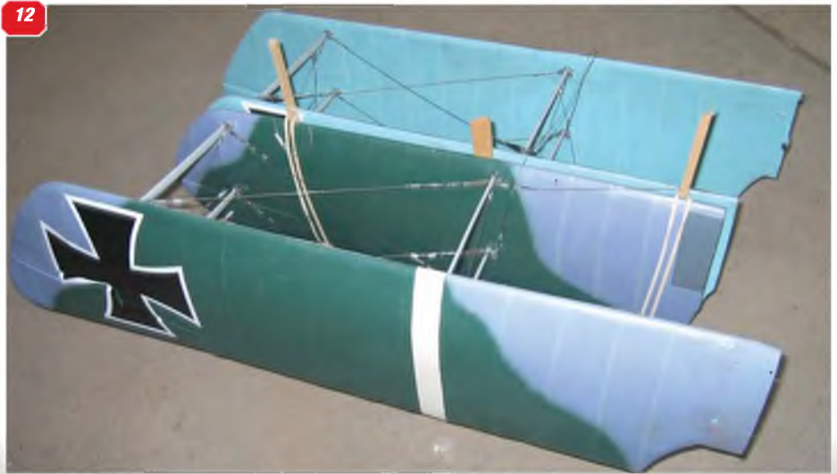
11: All wires fitted and rigged. Mike recommends working from a bench where there is all-round access to the airframe. 12 & 13: Mike uses this system for storing, and transporting the wings and assembling wing panels to the fuselage.
