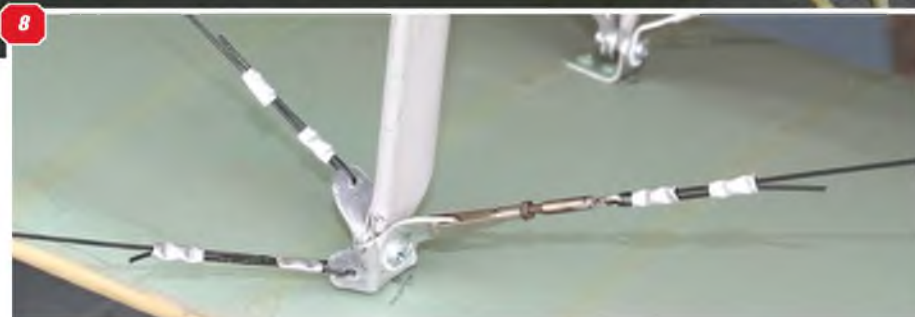
8: Wing-strut attachment brackets, also showing cable swages. 9: Rigging wire adjustable attachment clevis. Note the wire loop at the non-clevis end for attaching the rigging wire. 10: Adjustable clevis and rigging wire showing the cable swages and the attachment bracket made from metal angle strip cut and filed to shape.
