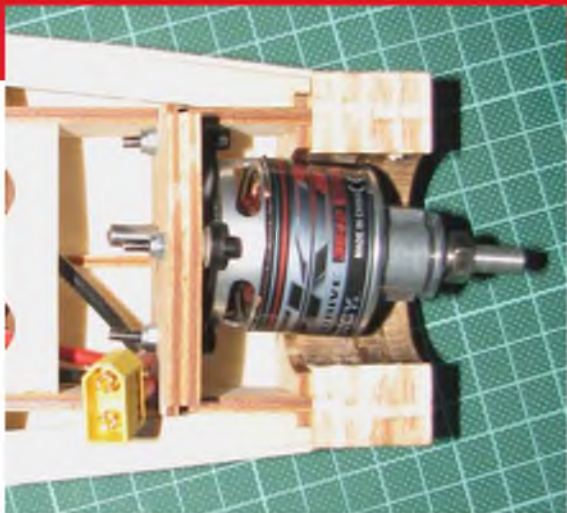
Note how the motor is off-set to allow for down and right thrust and still leave a spinner that is central in the nose.
