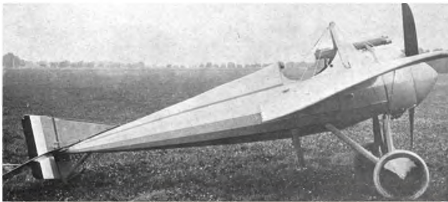
Another example of the M.S. Type I, with 110 h.p. Le Rhone rotary engine and synchronised Vickers machine gun.
