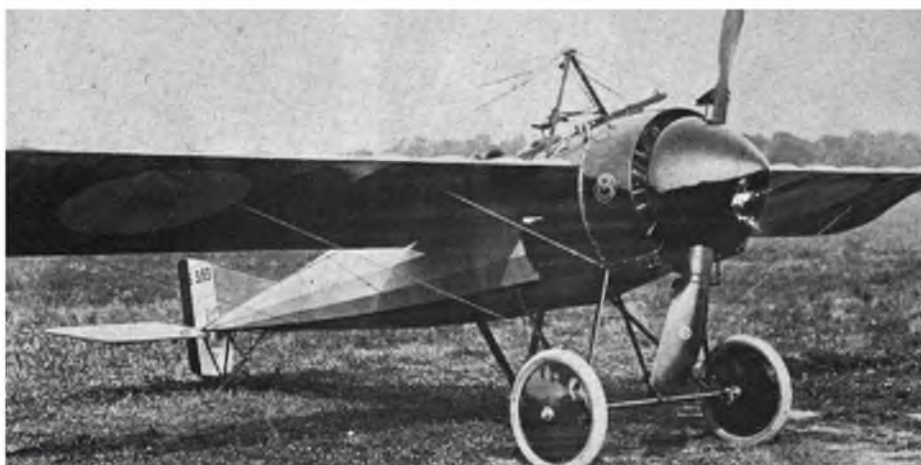
A Morane Saulnier Type N in French service with Hotchkiss machine gun and deflector plate type propeller.
