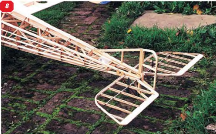
8: Another view of the uncovered fuselage rear. 9: View of the uncovered fuselage showing the wing root with tube for the tubular wing joiner.
