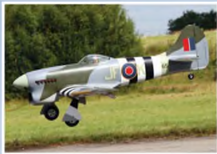
Andy and Colin Wynn's Hawker Tempest V about to land. 1/5th scale, 98" span, DA 85cc power. Weighs 43 lbs.
