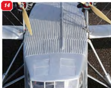
10: The engines nacelles are set very high. Martin home-moulded all 36 cylinders. 11: Lots of absorbing scale detailing wherever you look. 12: The prototype had 4 crew. Look at that crew entrance door. 13: Forward fuselage hatches have that soft metal look. 14 & 15: Fuselage corrugations achieved by Martins innovative balsa strip and Balsalock iron-on process!
