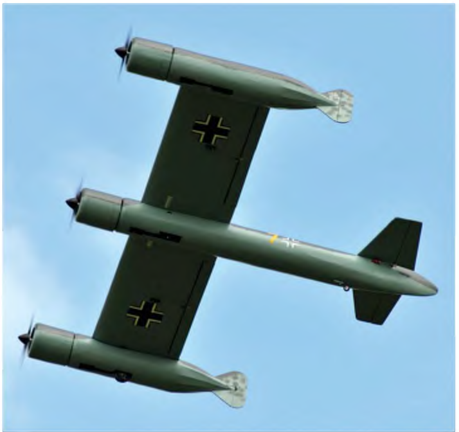
Certainly a competitor for the author's 'most unusual' scale design, the all-electric Blohm und Voss (again) P170 fast interceptor model. Still work in progress taming the beast - it flies, but not comfortably, still experimenting with the motor differential control on the tip motors - a stronger undercarriage needed, too!
