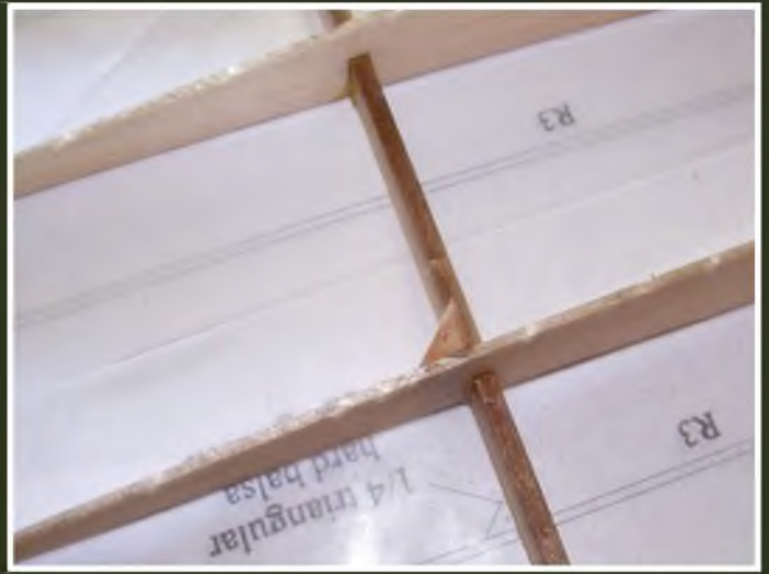
How the rigging blocks glue to spar and wing rib. The rigging cables pass through the blocks, only being glued once all is aligned and adjusted for tension.
