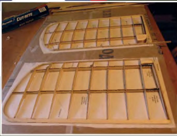
Absolutely nothing complicated about building the wings. Note the joiner tubes bound to the spars and the block area for the rigging pylon tubes.
