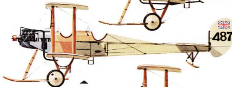
B.E.2b, No. 487; France, 1914. Note bomb rack between undercarriage V- struts. Aircraft subsequently captured intact by German forces.
