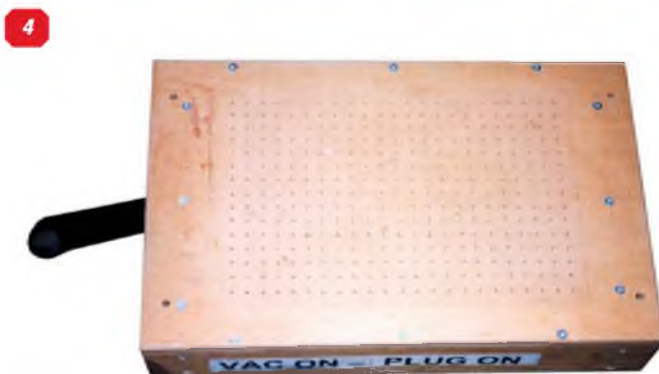
1: The canopy and plug that Denis made for his Spiffire. 2: The cowl is a three piece unit - two sides and the bottom. 3: Denis's system as described here - an old Hoover provides the suck! Note the reminders on the sides! 4: The base unit, showing the holes drilled at 1/2" spacing.
