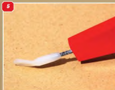
3, 4 & 5: The adjustable nylon end-tags for the wing struts can be distorted with a pair of pliers to lay flush with the wing surface.
