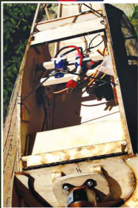
Clancy has his servos well back in the fuselage, possibly accounting for why he needed so much nose weight.
