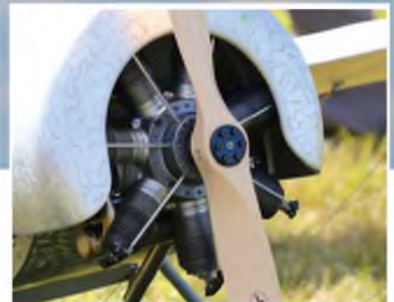
Gerhard Reinsch's very large and very impressive Fokker Eindekker EI from the incredibly detailed Paolo Severin kit. 4 metres in span, weighs around 19 kgs. Featured very convincing dummy Oberursel 7-cylinder radial on Herr Reinsch's imposing Fokker EI. There is a Valachi 120cc petrol engine hidden in there, too.
