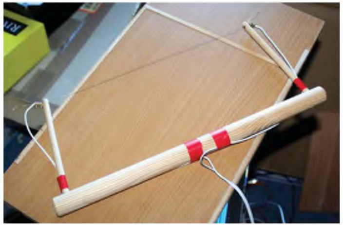
Add in an inexpensive cutting bow, making sure the board is actually flat and a power source and you're all set to slice thin foam.
