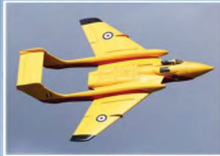
George Firth's own-design, scratch-built DH Vixen. Wren 100 gas turbine powered and weighs 30 lbs.
