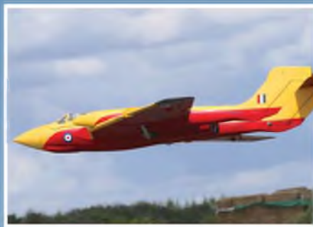
George Firth's nostalgic, seven foot span Sea Vixen. Note the trade mark asymmetric pilot's cockpit. Traditionally built, too.
