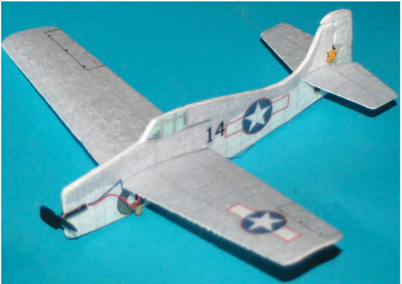
This 8" span model made from sliced RTF packaging weighs less than 3 grams as you see it here. Note the more open appearance of the foam.
