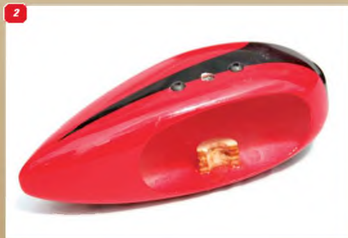
1 & 2: Plywood axle supports, stacked together to provide a locator for the wheel collet, inside with glass fibre moulded wheel spat.
