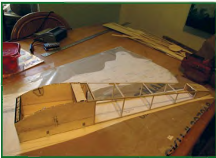
Having a virtually continuous straight edge, and no curve to the sides, makes accurate fuselage box assembly a relatively painless affair.
