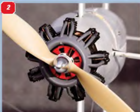
1: Martin chose electric power. Four Emax motors drawing about 300 Watts each on 10"x8" electric props. 2: Electric power obviated the need for bulky, hard to hide, hard to make, engine silencers. 3 & 4: Wonderfully involved tail treatment with outboard trim tab. 5: Pure 1930 kitsch. 6: The prototype luxury airliner could carry 39 passengers, their downward view unobstructed by wings.
