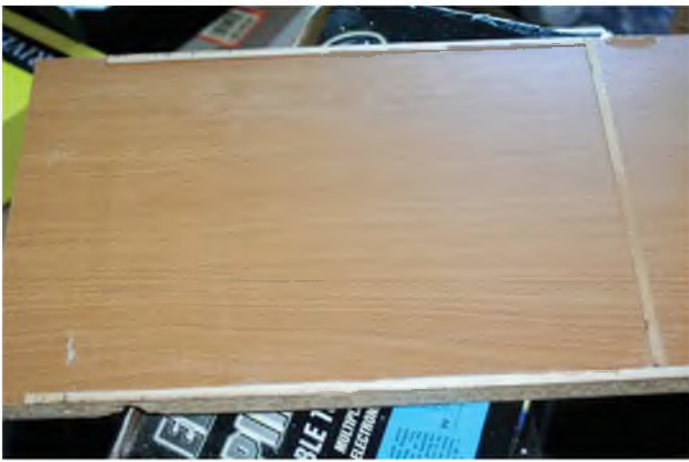
There's nothing complicated about the author's foam slicing board. The ply strips act as guides for the cutting wire.
