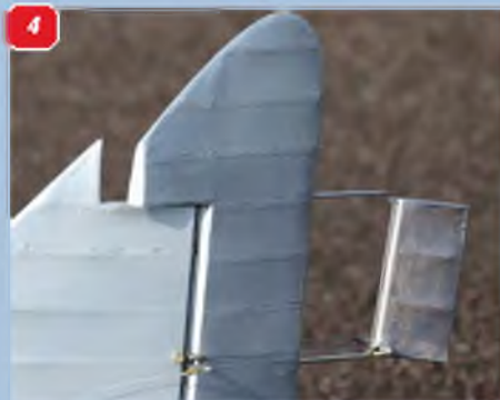
1: Martin chose electric power. Four Emax motors drawing about 300 Watts each on 10"x8" electric props. 2: Electric power obviated the need for bulky, hard to hide, hard to make, engine silencers. 3 & 4: Wonderfully involved tail treatment with outboard trim tab. 5: Pure 1930 kitsch. 6: The prototype luxury airliner could carry 39 passengers, their downward view unobstructed by wings.
