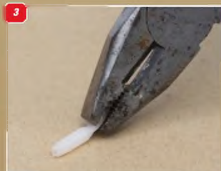
3, 4 & 5: The adjustable nylon end-tags for the wing struts can be distorted with a pair of pliers to lay flush with the wing surface.
