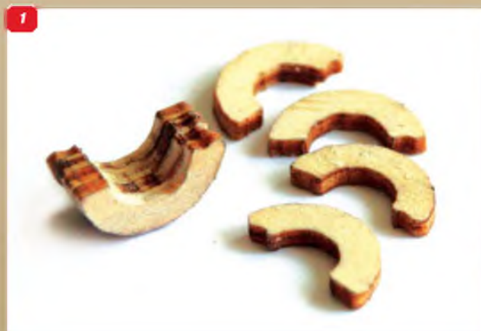
1 & 2: Plywood axle supports, stacked together to provide a locator for the wheel collet, inside with glass fibre moulded wheel spat.
