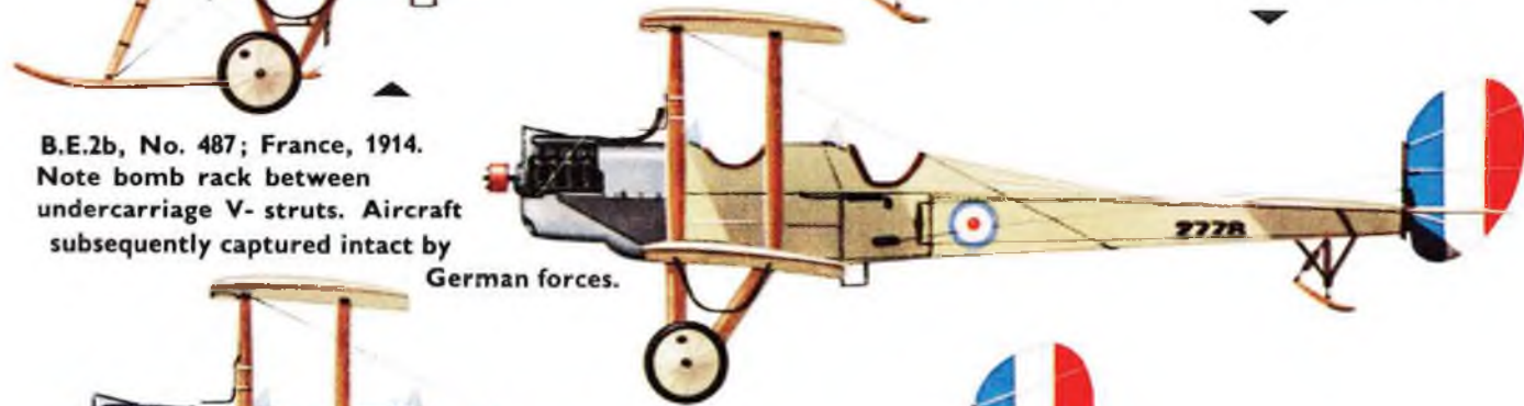
B.E.2b, No. 2778, served with unidentified training unit in United Kingdom, 1915. Note V-strut undercarriage, and cowled engine sump; engine cowling probably salvaged from a B.E.2c.
