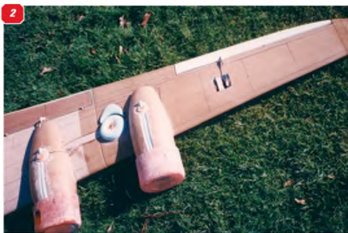
1: The Do335 three-view showing the long nose, tall undercarriage, small tail and underslung fin - each a challenge in its own right! 2: Ways of getting round things! The author's B-24 Liberator had enlarged ailerons, flap servos under the inner nacelle rear fairing and outer wing panels retained by a screw through the dummy undercarriage wheel centre (fixed to the outer panel), into the ply u/c 'leg', fixed to the centre section. 3: The B-24 was a big cheat! The outer engines were dummies and the outer props were taken off for flying - you couldn't tell the difference! It doesn't have to be complicated to look good! 4: Retracting undercarriage geometry can be used to get over scale position problems - angling the mounting blocks allows you to retain scale position, but incorporates forward rake - and ensures wheels fully retract inside the wing (legs on inside of wheels). Wing is the author's Spartan Executive .60 design.
