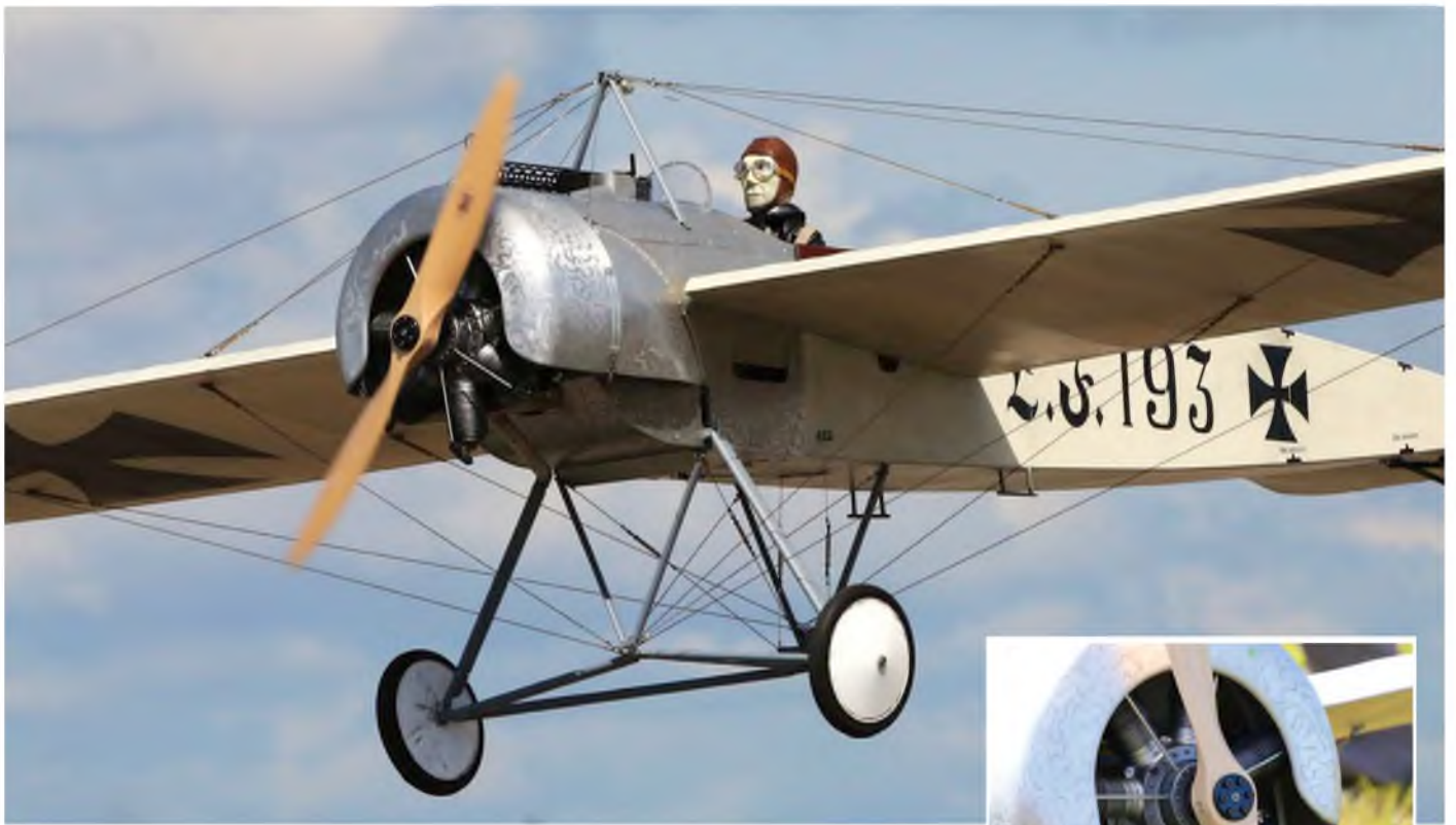
Gerhard Reinsch's very large and very impressive Fokker Eindekker EI from the incredibly detailed Paolo Severin kit. 4 metres in span, weighs around 19 kgs. Featured very convincing dummy Oberursel 7-cylinder radial on Herr Reinsch's imposing Fokker EI. There is a Valachi 120cc petrol engine hidden in there, too.
