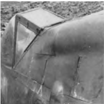
Cockpit wind-screen and cowl bulge ahead of the front screen.
