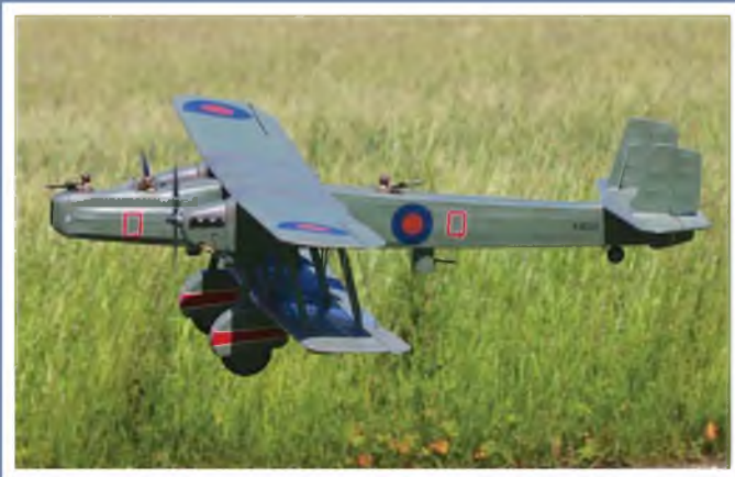
Dennis Richardson's scratch-built 1/13th scale / 69" span HP Heyford. Two OS .30 FS power.
