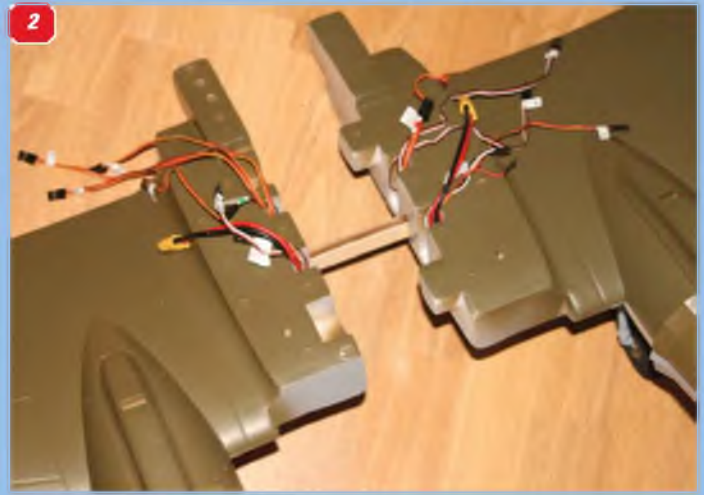
1: The C-47 access door in the fuselage side actually opens! 2: The substantial ply wing joiner in place. Note the channel-labeled servo leads.
