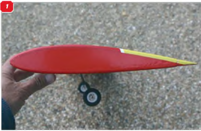
1: A semi-symmetrical section like this (15%) gives a good speed range and allows decent sports model aerobatics - and is well suited to WW2 fighter models. 2: This modified Götting 797 section (19%) is best for slow-flying models (Miles Magister).
