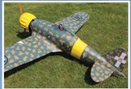
Geoff Dales' markedly changed the appearance of the panels on his Macchi ARTF by rubbing them with auto panel wipes and then satin fuel-proofed the model.
