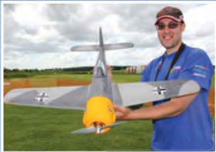
Simon Illsley joined the lunch time foamie flying with his GWS Fw 190A. 40" span / Wasp C3452-1250kV motor/ 10.5" prop / 2200 mAh pack. 50A E-Pro electronic speed control.
