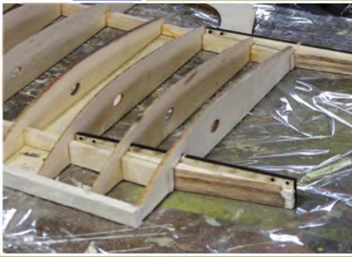
The laminated triangular wedges that take up the sweep in the wing, and the ply dihedral braces that double as pylon mounts.
