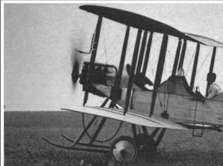
Not blessed with the best forward vision! An early B.E.1 with engine cooling radiator positioned smack in front of the pilot's forward view.
