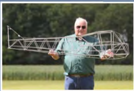
John Elkington told me that the Severin Storch fuselage arrives like this in the kit box. Finished model will be 14 feet in span.
