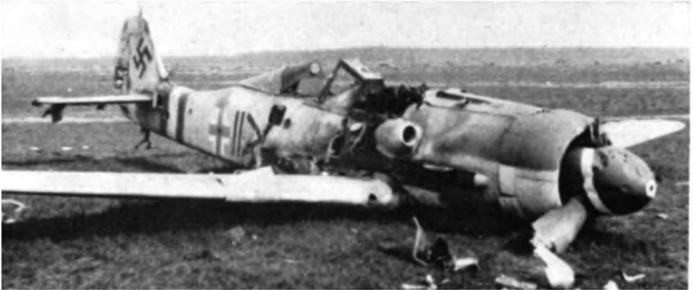
For you, the war is over! Totally wrecked Fw 190D-9 of JG 26at Rhein-Main airfield. The lack of a tailwheel in the wheel-yoke suggests the wreck may have been robbed of parts to keep others flying.
