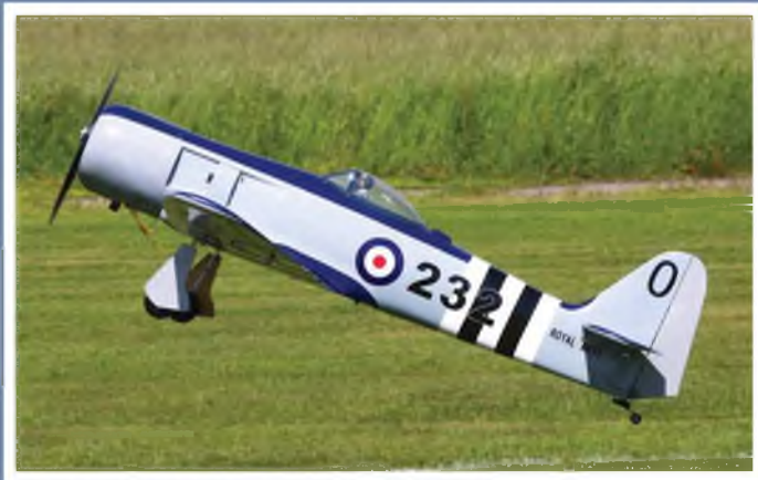
Bob Goodliffe's 80" span Sea Fury hauling off rather steeply in the blow. She is fitted with a 26cc petrol engine, and weighs around 17 lbs.
