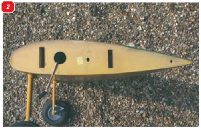
1: A semi-symmetrical section like this (15%) gives a good speed range and allows decent sports model aerobatics - and is well suited to WW2 fighter models. 2: This modified Götting 797 section (19%) is best for slow-flying models (Miles Magister).
