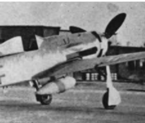
LEFT: Fw 190D-9 with centreline under-fuselage mounted 300 litre drop tank. Lack of any combat unit markings suggest this a factory-fresh aircraft on post-production test. ABOVE: The extreme wing-stretch of the TA 152 is well illustrated in the view of TA 152H Werk nr. 110020 captured intact in the Soring of 1945 and subsequently shipped to USA for evaluation.
