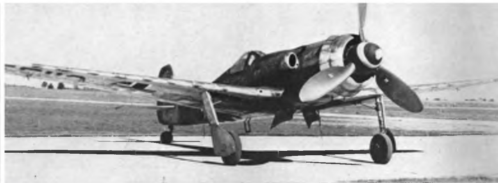
LEFT: Fw 190D-9 with centreline under-fuselage mounted 300 litre drop tank. Lack of any combat unit markings suggest this a factory-fresh aircraft on post-production test. ABOVE: The extreme wing-stretch of the TA 152 is well illustrated in the view of TA 152H Werk nr. 110020 captured intact in the Soring of 1945 and subsequently shipped to USA for evaluation.
