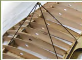
With the pylon wires in position. Notice how the rear c/s laminations aren't completed until AFTER the pylon is bound and glued in place.
