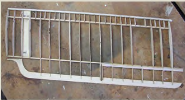
The basic wing panel awaiting tip, servo rib and dihedral braces. See text for details of these.
