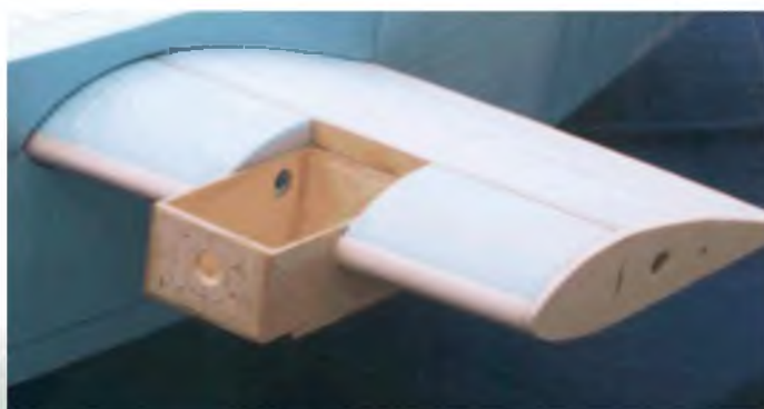
Nothing wrong with foam - it saves drawing all those ribs! The author's Liberator was 90% blue foam. Note the fatter section of the centre section - more like NACA 2418 (18%).
