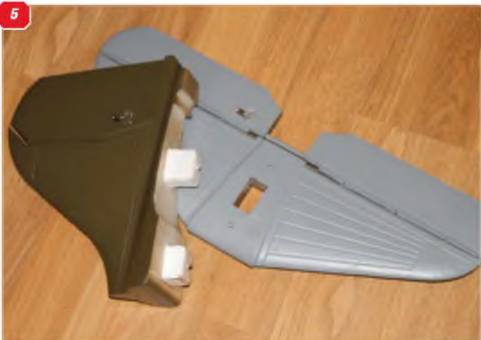
3: Lower swing surface showing aileron and flap servos. Note the undercarriage is 'down'. 4: The various decal sheets supplied - four different variants available. 5: The tail units - the lugs on the bottom of the fin needed a bit of 'thinning down' to fit the tailplane apertures. 6: Detail of one of the cowl, air cooler scoop and scale props. Note balloon ribbed tyres on mainwheel.
