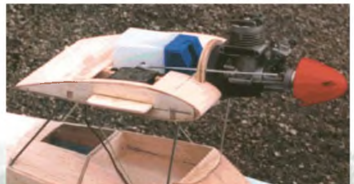
Sheeted centre section of the author's Shavrov flying boat. Uses the NACA 2415 section. Note the outer panel location tab is placed parallel to the rib chord line.
