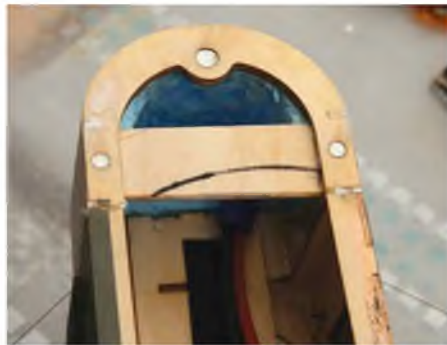
The blue foam replacement nose is hollowed out to allow the lipo to be placed as far forward as possible - the wide ply crosspiece is the support for the additional noseweight needed.
