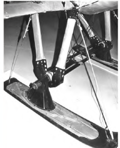
Ski type main undercarriage for winter operations on restored Finland museum F.4 Buzzard aircraft.
