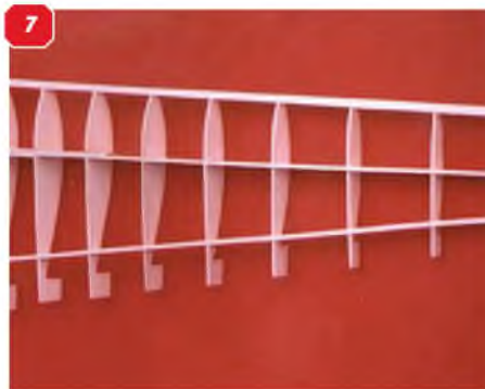
6: For a .40 size fighter, flaps aren't really helpful and add complication and weight - on a bigger model, operating flaps add an extra dimension to the 'realism' factor. 7: A typical .40 size fighter wing structure, before building in the servos, linkages and retract mountings, etc. Note the tabs on the ribs to hold them at the right angle. (Actually an EP Savoia Marchetti SM79 Trimotor wing). 8: Bottom sheeting added and linkages in place, prior to top skins being fitted (SM79).
