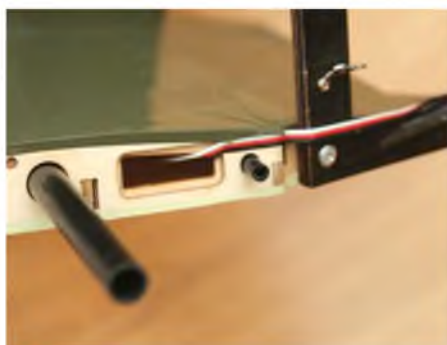
Routing the tail servo leads along the booms and into the wing - a neat solution.
