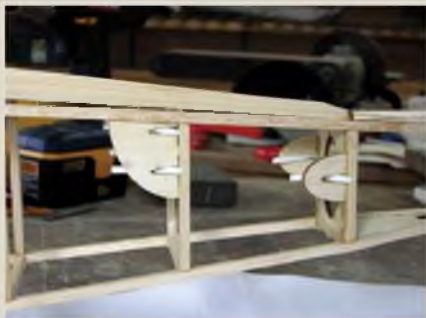
I'd actually intended those exit plates to be flush with the outside and the tubes trimmed off flush. This way, only the tube will come into contact with the covering.
