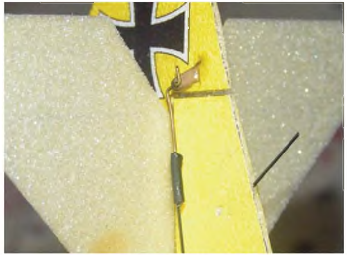
How the wire pushrod end is attached to the carbon rod using heat-shrink tube and CA adhesive.
