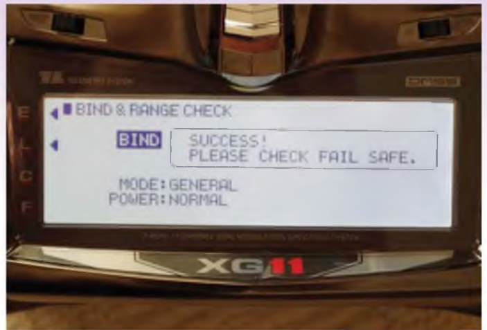
The final screen shot shows the bind screen after the receiver has been bound. Note you have to programme the failsafe on the radio after you set the bind.
