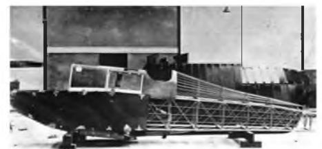
Bare fuselage of Finland Air Museum's F.4 during restoration.
