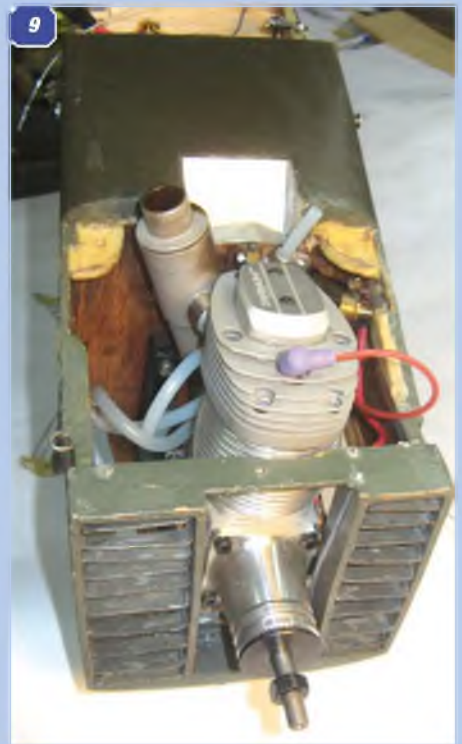
5: The fuselage rear underside, showing the tailskid and the tailplane bracing struts. 6: control system installation, showing rudder, elevator and throttle servos at the compartment rear, receiver soft mounted to the fuselage side. Note the metal bracket that holds the fuel tank in place. 7-9: Engine bay showing the engine and tank installations.
