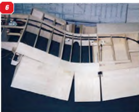
6: For a .40 size fighter, flaps aren't really helpful and add complication and weight - on a bigger model, operating flaps add an extra dimension to the 'realism' factor. 7: A typical .40 size fighter wing structure, before building in the servos, linkages and retract mountings, etc. Note the tabs on the ribs to hold them at the right angle. (Actually an EP Savoia Marchetti SM79 Trimotor wing). 8: Bottom sheeting added and linkages in place, prior to top skins being fitted (SM79).
