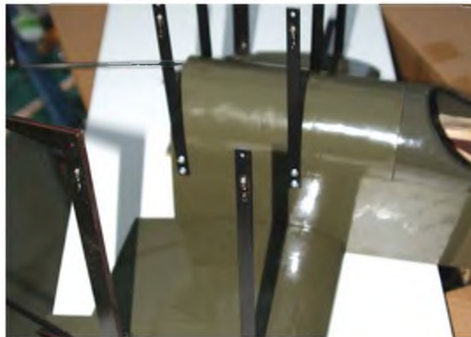
Fitting the inner struts to the fuselage and inner wing panels, before fitting the top wing centre section.
