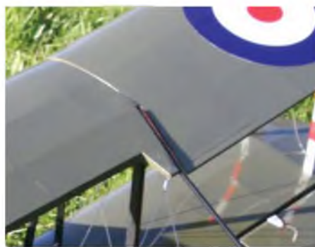
View of the top wing outer panel incidence mismatch from the rear, showing difference in root TE heights.
