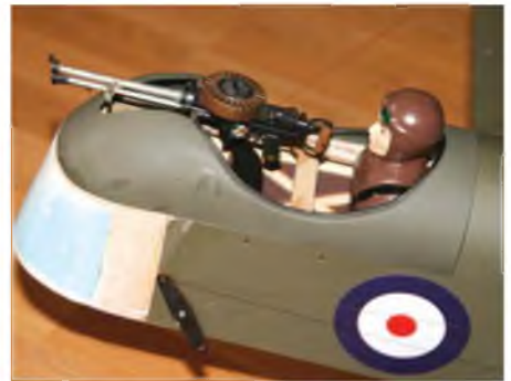
The finished replacement nose, ready for painting to match the overall olive drab finish.
