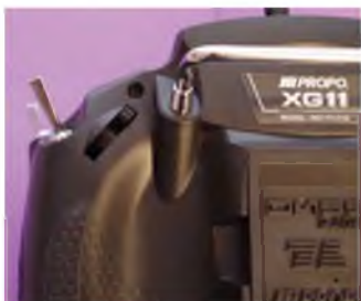
ABOVE LEFT: There are two sliders on the rear of the radio. ABOVE RIGHT: The battery case houses a two cell LiFe battery of 1400 mah capacity. It also encloses the SD card. The SD card allows virtually unlimited model storage plus facilitates updating the software of the radio as JR release new features.
