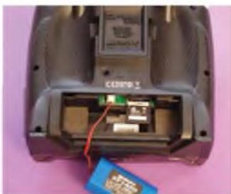
ABOVE LEFT: There are two sliders on the rear of the radio. ABOVE RIGHT: The battery case houses a two cell LiFe battery of 1400 mah capacity. It also encloses the SD card. The SD card allows virtually unlimited model storage plus facilitates updating the software of the radio as JR release new features.
