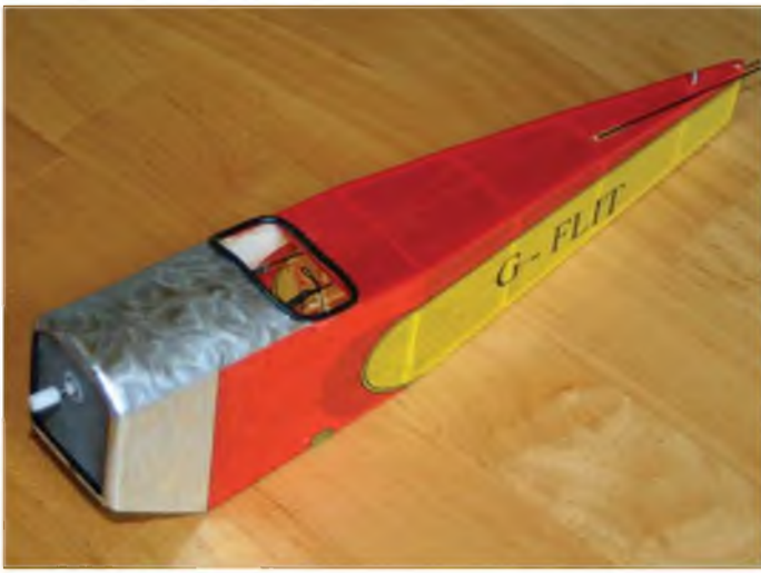
Note the way the pushrods are very much over-length at the rear of the author's White Monoplane.
