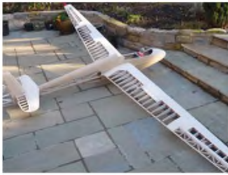
Completed airframe, ready for covering.
