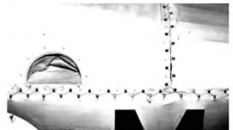
Fuselage detail, showing stitching line to fabric covering. Note also mounting stirrup.
