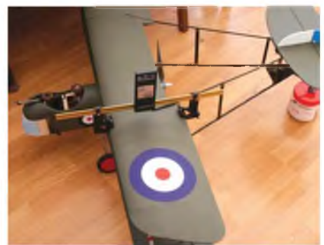
Checking the incidence of each wing panel and centre section - at least the mismatch was even on port and starboard sides, top wing only.
