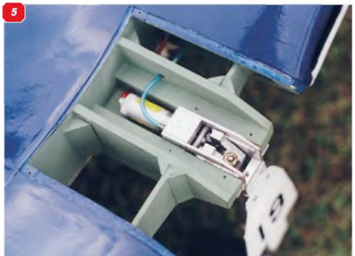
4: They don't have to operate in a scale way! This retract should be twist and lift (Corsair), but who can tell that they're not when they're up? Keep it simple! 5: Scale retracts are available - they're expensive, but are really the business! (this is a Unitract unit designed specifically for a larger F4U Corsair).
