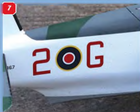
7: Rear of the hull is faithfully modelled. Lower hull is skinned in fibreglass and resin for strength and water resistance. 8: David has kept the detailing simple and "sports-scale". Interesting but practical, based directly on the famous Airfix kit. 9: Home designed vinyl roundels. Simple, effective, and durable in the water environment.
