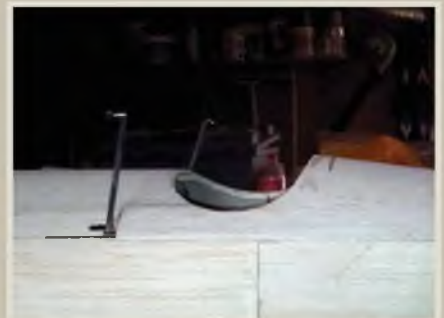
Starting with an undersize cockpit opening, and the sheet behind it slit helps set it up around the change of angle involved.
