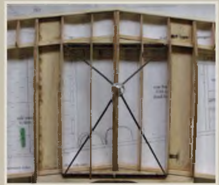
The pylon bound in place onto the ply dihedral braces.
