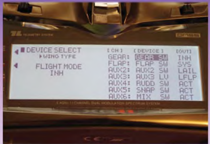
Device select allows you to select which switch or button operates some functions.
