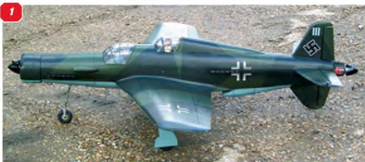
1: The Dornier Do335 referred to in this article has a 4-stroke engine up front, electric outrunner motor in the rear. A very practical set-up.
