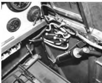
Right side of cockpit showing the hand pump that maintains fuel feed pressure.
