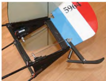
The rudder and elevator servos in place on the top and bottom rear plates. Note the sprung tailskid bolted to the rudder.
