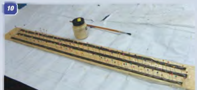
10: SIMULATED STITCHING LINES: These are 3/8" strips of Solartex, sticky side up and pinned to balsa with a clear plastic sheet underneath (Solartex backing). The pins are in a zig zag pattern and a doubled thread is then wound round, onto the next one, round and so on. They are then given a brushed coat of Clearcoat, CoverGrip or similar heat sensitive fabric glue. When removed from the backing, laid on the fuselage and ironed on you get the effect of stitching covered by a strip of covering.
