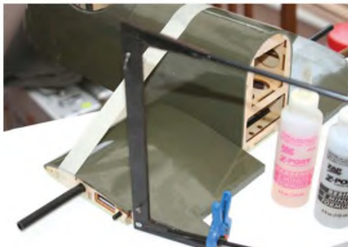
Gluing and screwing the rear frames to the lower wing inner panels.
