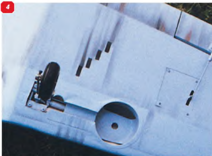
4: They don't have to operate in a scale way! This retract should be twist and lift (Corsair), but who can tell that they're not when they're up? Keep it simple! 5: Scale retracts are available - they're expensive, but are really the business! (this is a Unitract unit designed specifically for a larger F4U Corsair).
