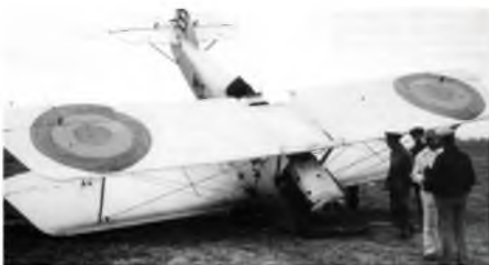
Spanish Air Force F.4 Buzzard in a sorry state after main undercarriage collapse.
