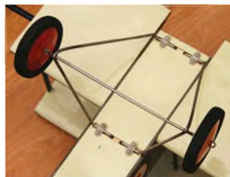
The sturdy uc assembly bolts onto the bottom of the fuselage.
