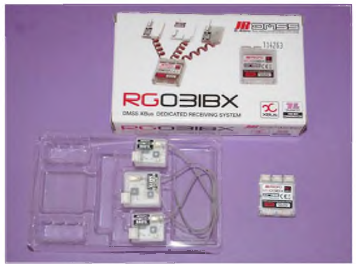
JR RG03IBX is a minute receiver but can cope with at least 28 channels and 112 servos. However there are no servo ports!
