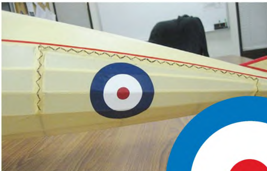
Here you see that fuselage lacing done using perforated covering strips and actual lacing.
