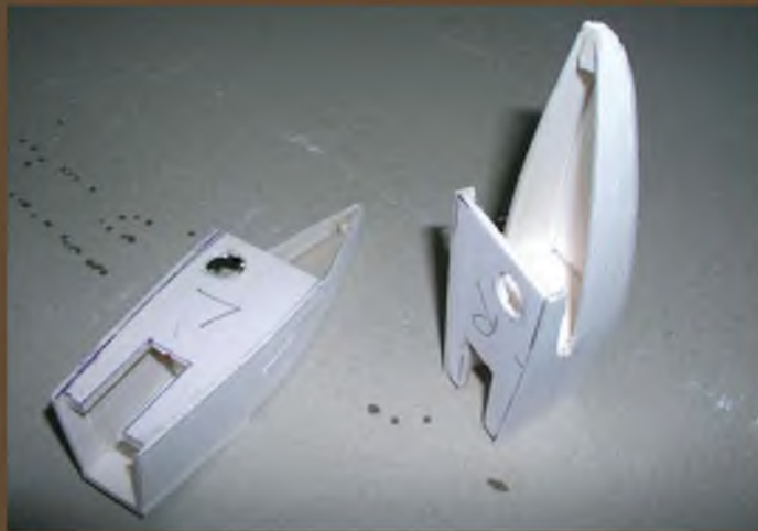
Engine nacelles showing initial box construction.
