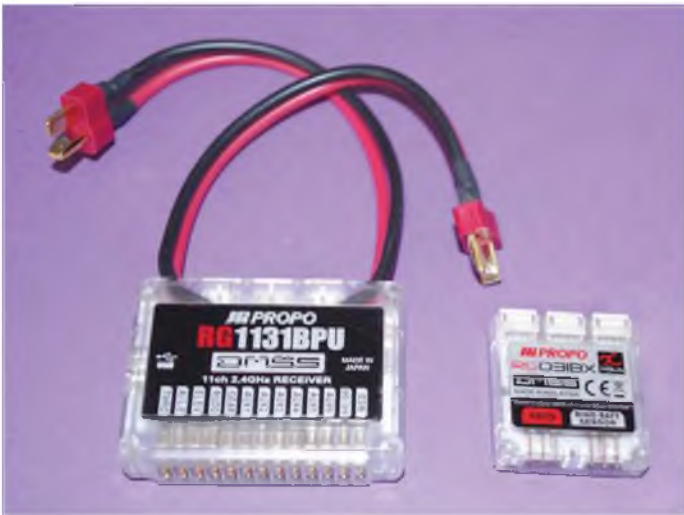
Here we can see quite clearly the absence of servo ports on the smaller receiver (satellites not shown for clarity). This receiver can cope with more channels than its larger brother!
