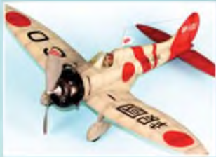
Dave Banks' wonderful Mitsubishi Claude, with its rolled balsa fuselage. 18" in span, rubber powered, and weighs but one ounce!
