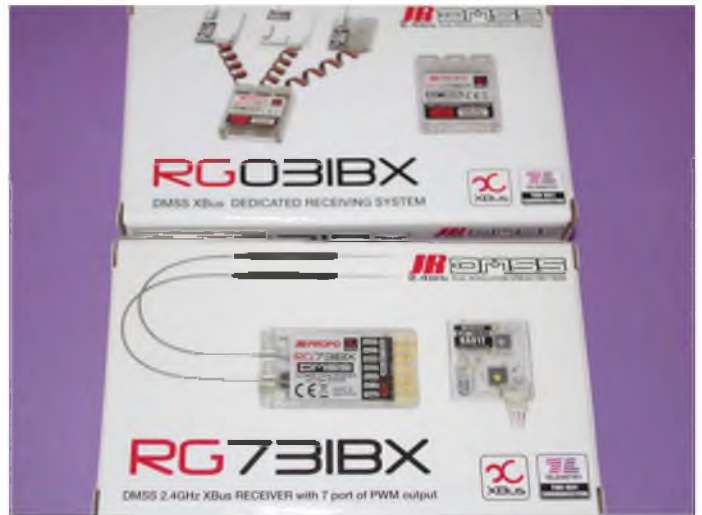
The RG73IBX looks like a traditional 7 channel receiver apart from the extra port marked XBus. This port allows the receiver to receive more channels, up to the maximum your radio is capable of transmitting. In addition each of these channels can be split into 4 sub channels with control of servo travel and rotation etc.
