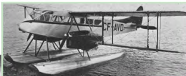
Operation from water suited Canada's vast territorial expanse, with its many lakes and rivers. This, the first Dragon Mk.2 exported to Canada, registered CF-AVD features the revised fin/rudder shape as applied to the Iraqi militarised DH84M.
