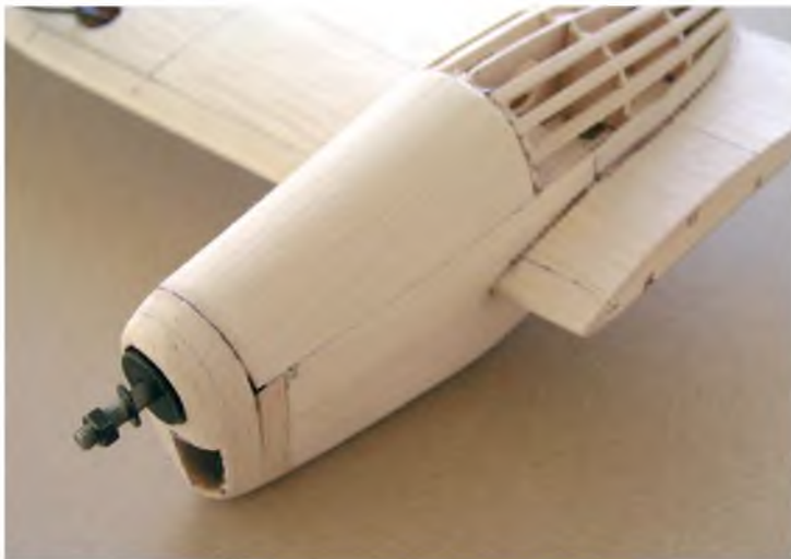
A completed nacelle with shaped sheet noseblock and thin sheet balsa cowl top.
