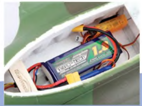
The 3S x 1800mAh lipos used in the review model, in its CG balance position.
