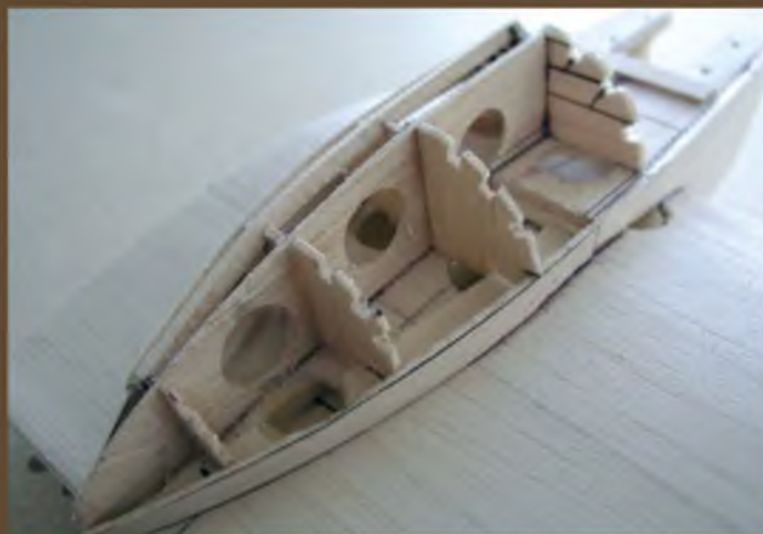
Top rear of a nacelle, showing formers ready for stringers.
