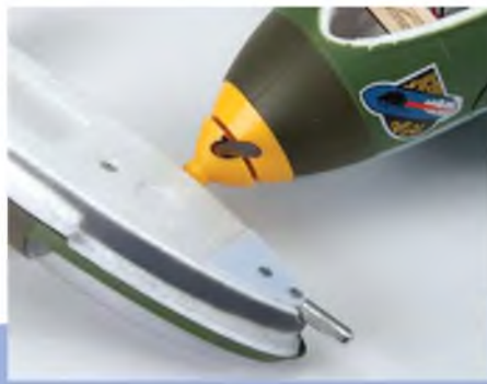
The access hatch removed adjacent to the scale-like moulded spinner.
