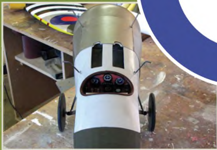
The cockpit area showing the styrene panels, cut outs for the guns, coaming and dummy instrument panel.
