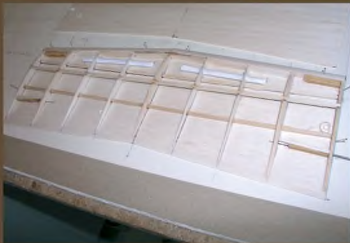
Lower wing centre section ready for top skin. Note hardwood blocks at each end rib to support wire stub joint to outer bottom wing panels. Paper tubes are for motor wiring.
