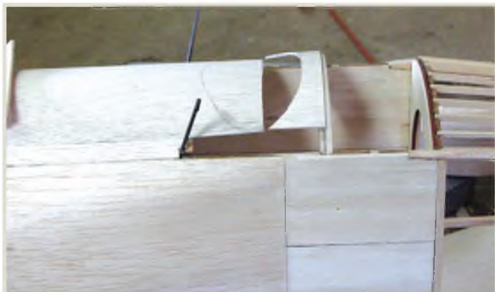
How Charles used different pieces of sheet to make up the decking around the cockpit area.
