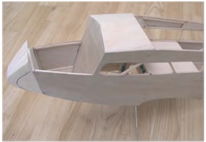
Initial fuselage assembly complete. F5 (horizontal, above lower wing seat) is removed later.
