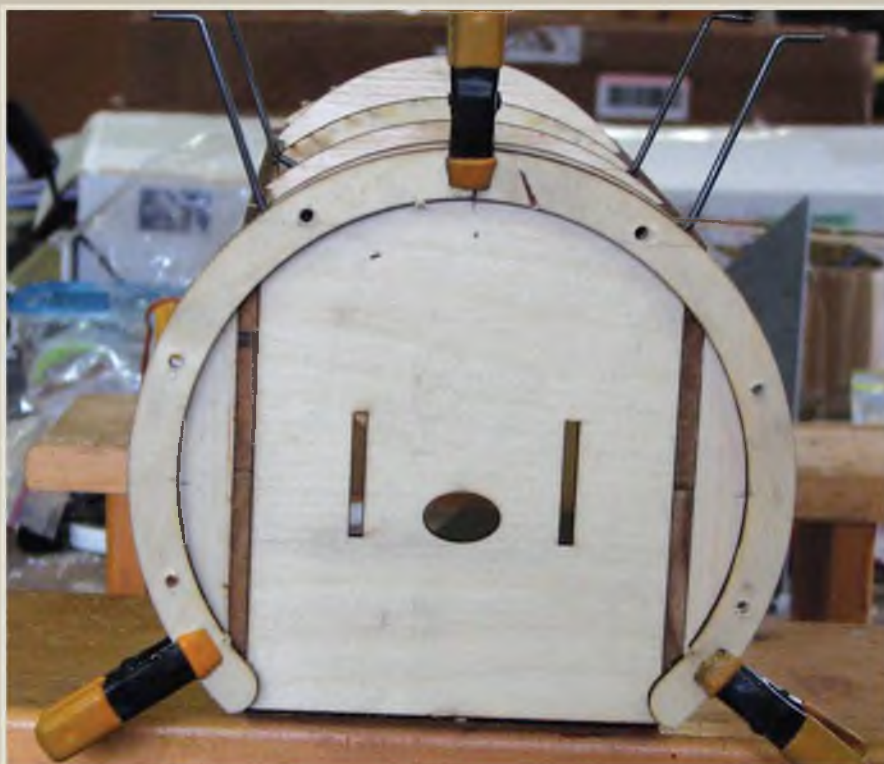
Here you see the rear cowl former held in place while it, and the firewall are prepared for locating dowels and magnetic retainers.
