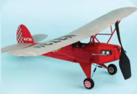
Brian Waterland's first foray into The BMFA Indoor Scale F/F Nats. This is his 17.5" span / 25.5 gram Kit Scale Corben Baby Ace.
