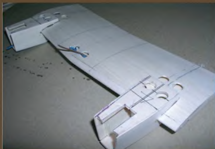
Nacelles glued to wing centre section, with wiring in place.
