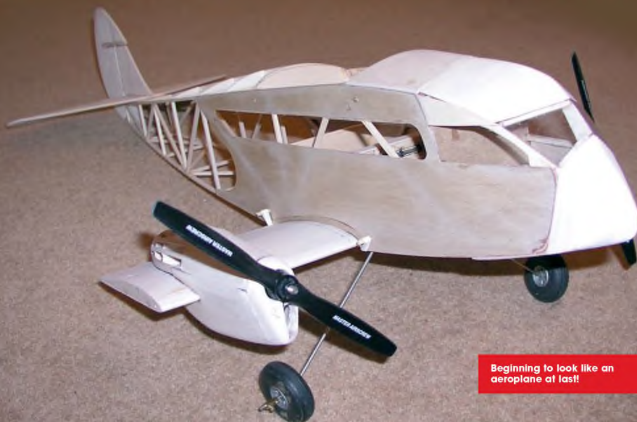
Nacelles glued to wing centre section, with wiring in place.
