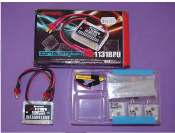
An 11 channel DMSS receiver which isn't XBus enabled and hence you can only use 11 channels with no possibility of expansion.
