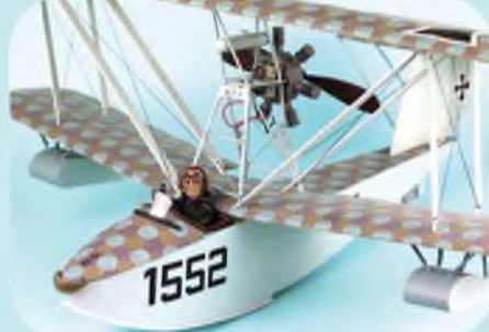
Paul Brigg's Brandenburg W-20 WWI pusher seaplane, from the Mike Midkiff plan. Electric powered, traditionally built, and spans 20".
