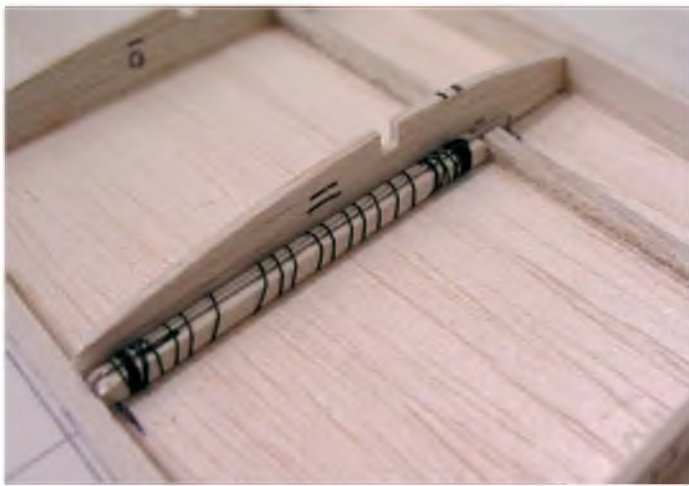
Strut hook wires are bound to balsa strips and glued against rib and skin.
