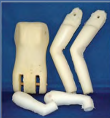
Torso and limbs showing the different foams used.
