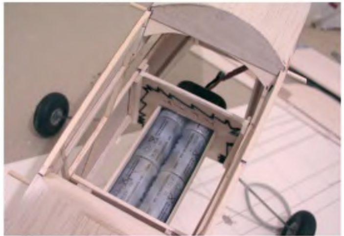
The battery is loaded through the bottom ...and located in a snug-fitting tray.
