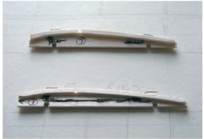
Strut hooks for bottom wing are bent up before being bound and glued.
