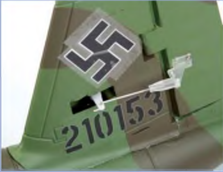
The rudder link and fin-mounted servo - needed for straight take off runs!
