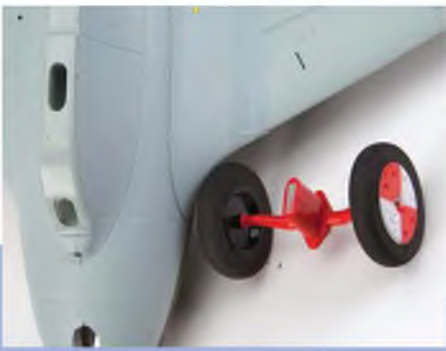
The clever, switch operated magnetic jettisonable take off dolly slots into the landing skid moulding.
