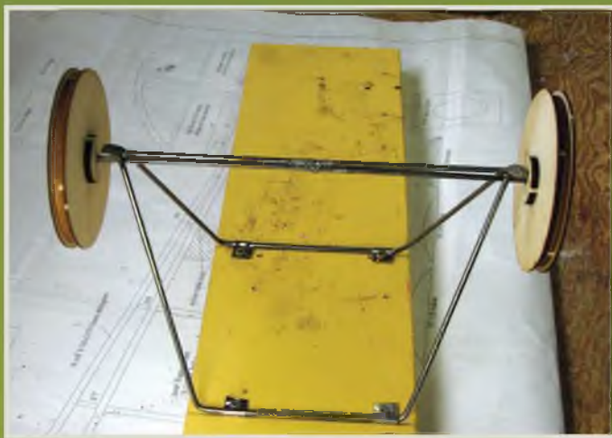
The simple jig used to assemble the u/c wires, and how those laser cut wheel parts go together.
