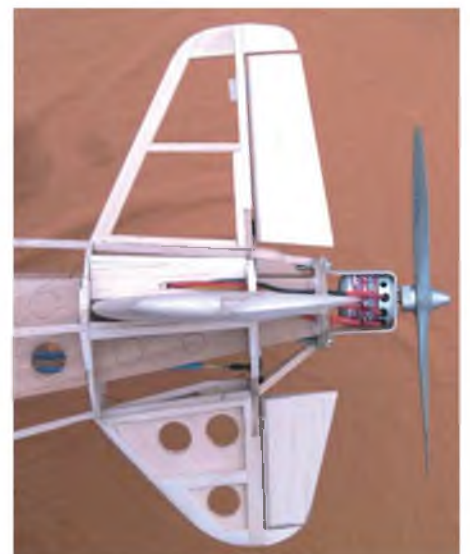
The fin and rudders are conventional build - the lower fin has a sheet core for extra strength (minimal ground clearance!). The outrunner is wired up and the harness run through the rear fuselage.
