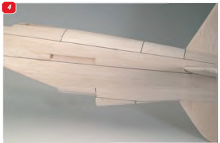
3: The nose skinned - the hole in the side is for cooling air to the esc/battery (scale position of an air intake). The exhaust stub box is flush-mounted, ready for the moulding. 4: The planked rear fuselage with the sheet panel lines highlighted. Well-soaked in water, the soft sheet easily took the double curvatures.
