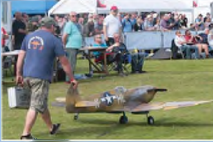
Stewart "Fighter Factory" Clifford wheels out his unusually schemed Spitfire. 1/4 scale, built from the Mick Reeves plan. Fibreglass fuselage.
