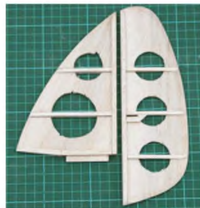
The replacement fin and rudder prior to covering.
