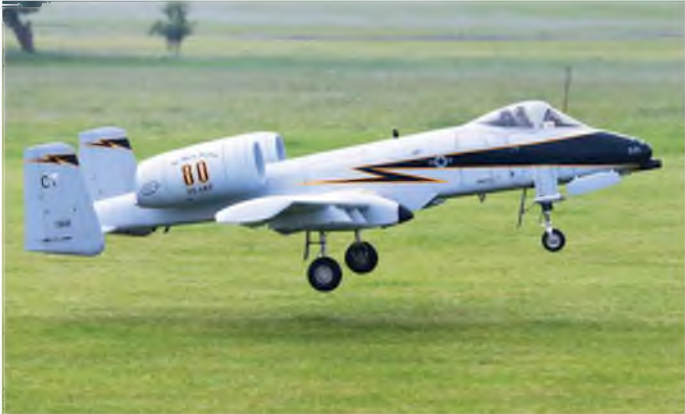
Florian Kellwitz 's Fairchild A-10 Warthog. Twin JetCentral Rabbit turbines, weighs 24.3 kgs.
