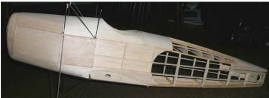
Once all the trimming and sanding is complete this is pretty much what your fuselage should look like.
