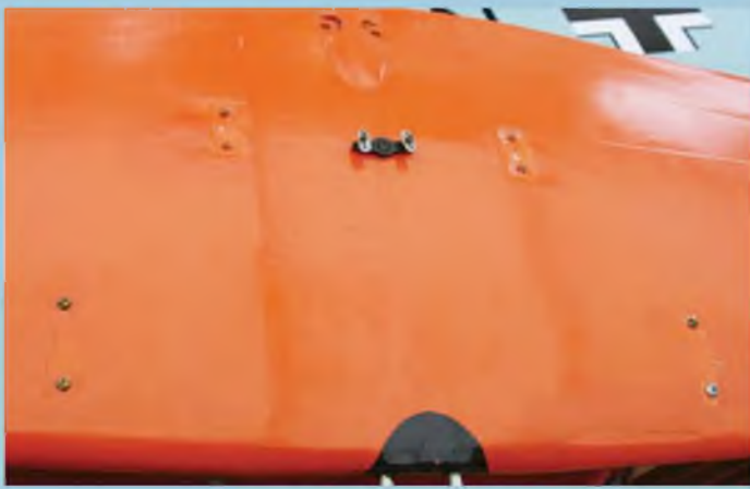
Detail of the float mounting bolt holes in the lower wing surface. Note also the rudder servo arm that operates the water rudders.
