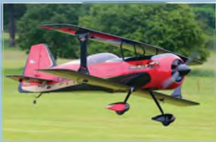
Hangar 9 / Horizon Hobbies version of The Beast full-size aerobatic biplane. 89" span, around 26-28lbs in weight, for DA 100 or EVO 80 tuned pipe.
