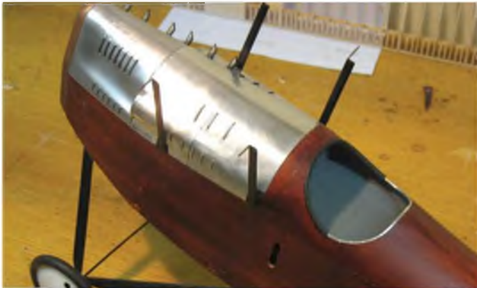
These relatively simple lithoplate panels on the Pat Lynch Ansaldo demonstrate how well it can be persuaded to simulate aluminium panelling.
