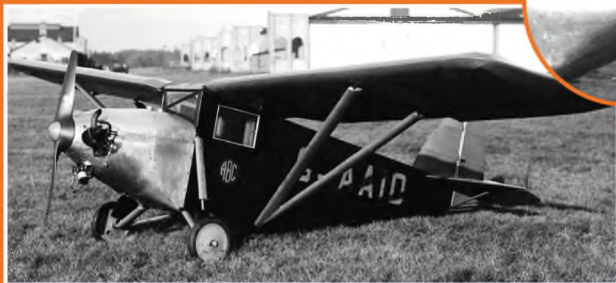
The Robin was modified at Brooklands in late 1929, and is seen here showing the revised windscreen, moved back so that the fuel and filler caps were located in front rather than behind it. In order to improve the handling characteristics the fin and rudder increased in area - also revealed here. The Robin was doped in the distinctive black and orange colours of Hanworth-based National Flying Services in anticipation of a large order that never materialised.
