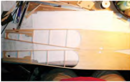
Totally traditional, the fuselage begins with building two side frames over the plan.
