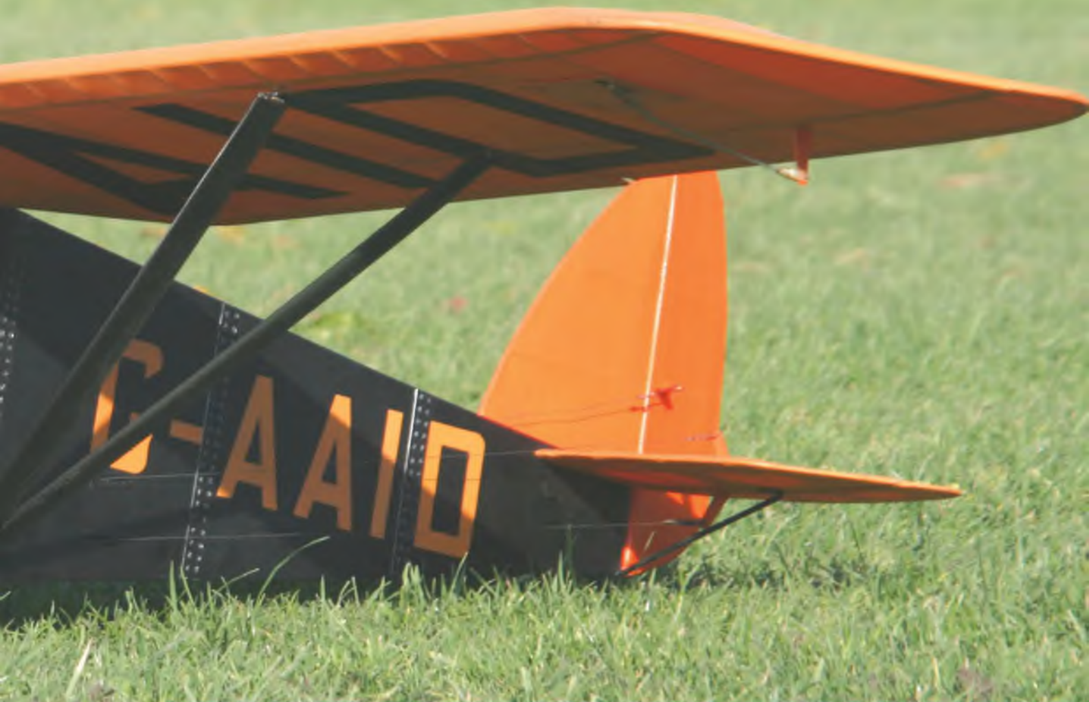
THE PROTOTYPE MODEL MODIFIED TO ROBIN 2 VERSION WITH ITS REVISED TAIL AND WINDSHIELD.
