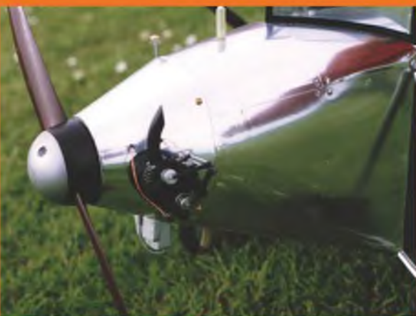
The dummy Scorpion engine cylinder fitted to the side of the cowl opposite the O.S.26 Surpass.
