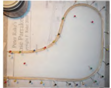
Glenn uses just pins to hold the laminations around the Depron formers but it's worth reading the author's thoughts on the subject.
