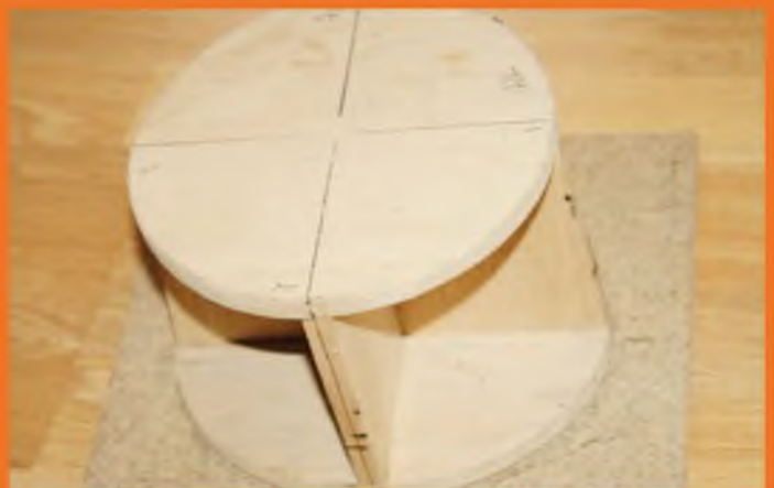
The cowl is formed on this simple jig.
