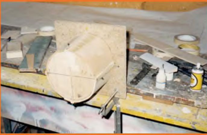
The layers of the cowl awaiting the glue to cure, before removal from the jig.
