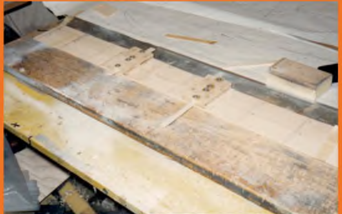
The first step in float build, preparing the top plates and mounting points.
