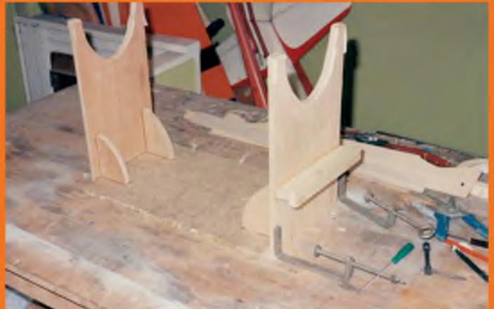
To accurately align the floats when mounting, Ken devised this simple jig to hold the fuse/wing assembly in the right position.
