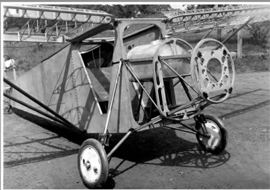
The single-seat ABC Robin in the course of construction at the Walton-on-Thames factory in May 1929 before installation of the ABC Scorpion but showing in detail the engine mounting.
