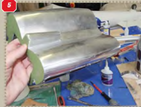
1: The underside of the S6B before the undercarriage was fitted. Note how slender is the fuselage. 2: Wing almost finished, with rivets and tiny hatches being applied. 3: Mass balances on the ailerons. 4: Nose cowl looks suitably metallic. No unsightly extra apertures are required with an electric motor. 5: Aerfoil can be coaxied around compound curves like this top hatch and the cowl. 6: The top rocker-box cover just slots in.
