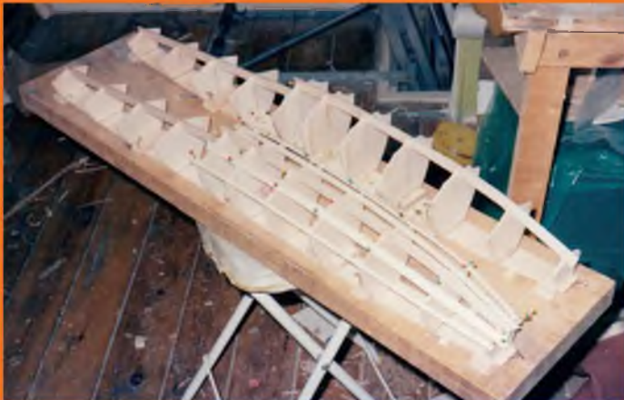
The floats are built inverted - note the fluted bottoms of the forward sections.
