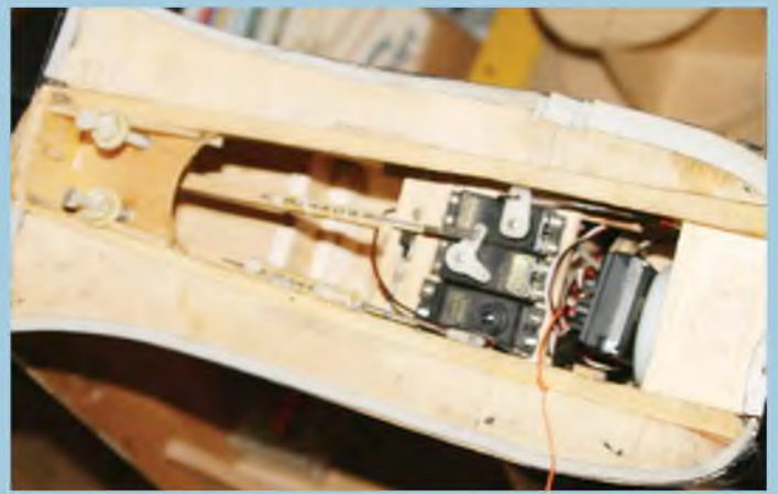
The radio bay with everything fitted well forward. The flight battery fits under the tank. If operating off water, the wing fuselage joint needs to be waterproof.
