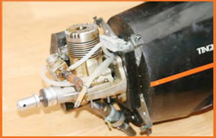
The OS Max 61 mounted on a metal mount with a needle extension to fit outside the cowl. Note the additional lead weight behind the cylinder head.
