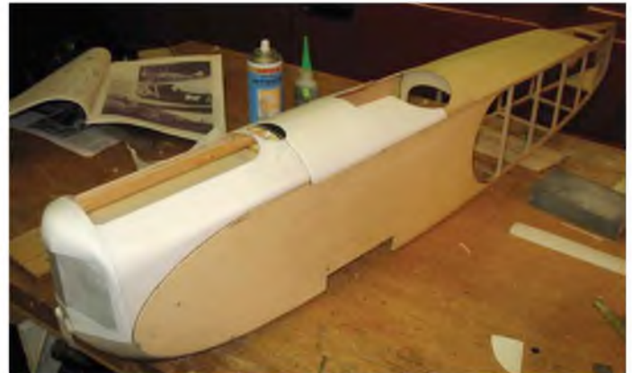
Simple pull mouldings trimmed and fitted to Pat's Fokker DVII represent metal well after painting.
