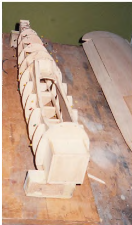
The basic fuselage box, showing the wing seat area, prior to fitting the tail surfaces.
