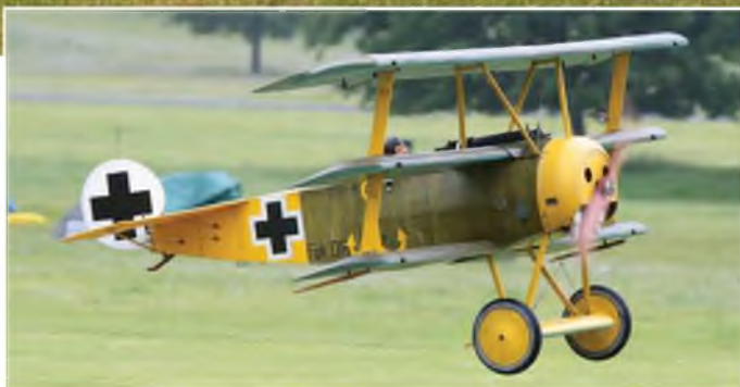
Ian Redshaw's Fokker DR1 Scout, 1/3rd scale, 96" span, weighs around 38 lbs. Zenoajh 38cc geared drive.
