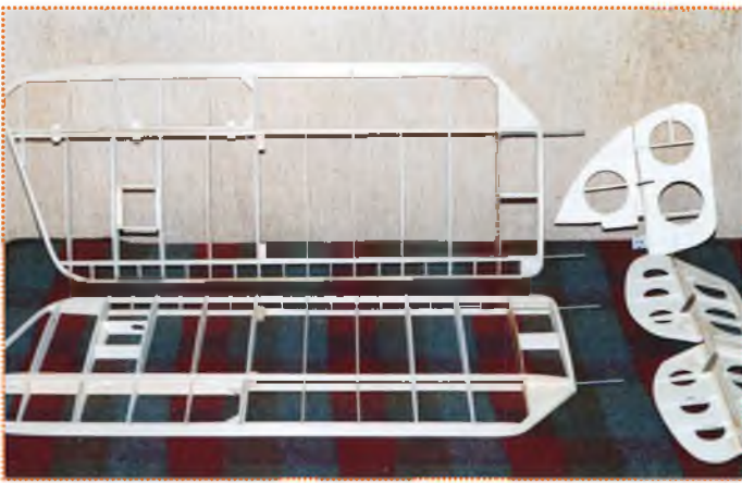
Not very many build photos exist of Brian Hewitt's prototype model, but here's the flying surface construction, before covering.
