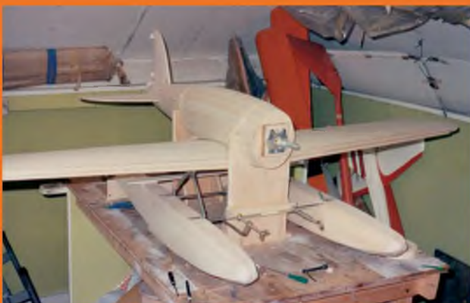
Fitting the float struts and brackets. All bolted together for strength and removability.
