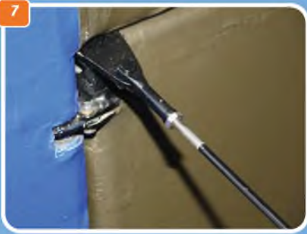
1 & 2: Cockpit viewed from the pilot's seat. A tight fit! 3: Wing bracing wire crossover. 4: Anchor point for wing bracing wire that passes through lower wing surfaces to attachment lug on main undercarriage attachment. 5: Fuselage rear, showing elevator control runs. 6: Tailplane-to-rudder bracing wiring attachments to rudder. 7: Fin/tailplane bracing wire attachment and rudder hinge. 8: Steerable tailskid. 9: Fuselage top deck panel at rear of cockpit, right side. 10: Same panel, left side showing hinged access panel and cockpit mounting stirrup. 11: Control wire runs to rudder and elevator. 12: Elevator control run exits in fuselage side. 13: Typical lacing runs on the rear fuselage fabric covering panels. 14: Lower wing leading edge access panel for aileron control run. Also shows front wing strut anchor point. 15: Lower wing rear strut anchor point and wire link from lower to upper wing ailerons. 16: Lower wing undersurface showing control horn and tie-down ring.
