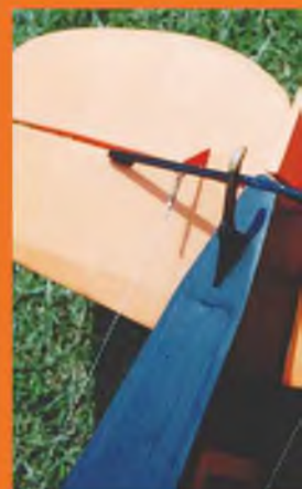
The underside of the tail showing the closed loop elevator control.
