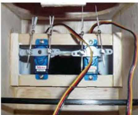
Those little wire loops make for easy adjustment of closed loop cables.
