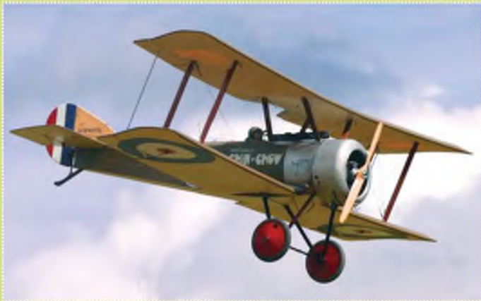
Andy Johnstone's one third scale Dawn Patrol Team Sopwith Pup "Chin Chow". Zenoah 62 petrol power, 28"x10" prop.
