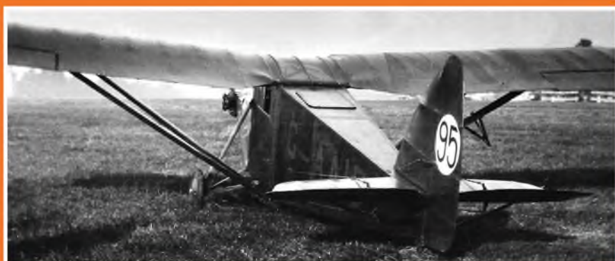
Tail-end view of the Robin, now with the revised fin/rudder shape, numbered 95, competed in the 1930 King's Cup race and was the fourth of 88 aircraft to take off from the Hanworth start. Engine revs were well down and the Robin later force-landed at Old Sarum near Salisbury.
