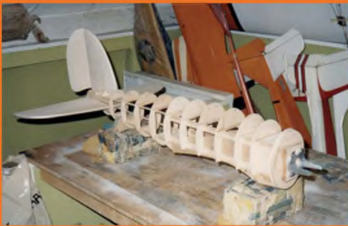
With tail fitted, planking the fuselage begins, using narrow sheet balsa strips.
