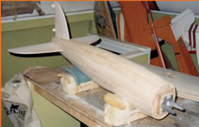
The planked fuselage ready for planing and sanding for a super smooth surface.
