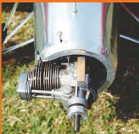
A view of the O.S. 26 installation, showing lead noseweight bolted to the bearers as far forward as possible.
