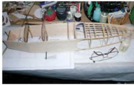
It's more accurate to assemble the basic fuselage with the wires and tubes already attached to the formers.
