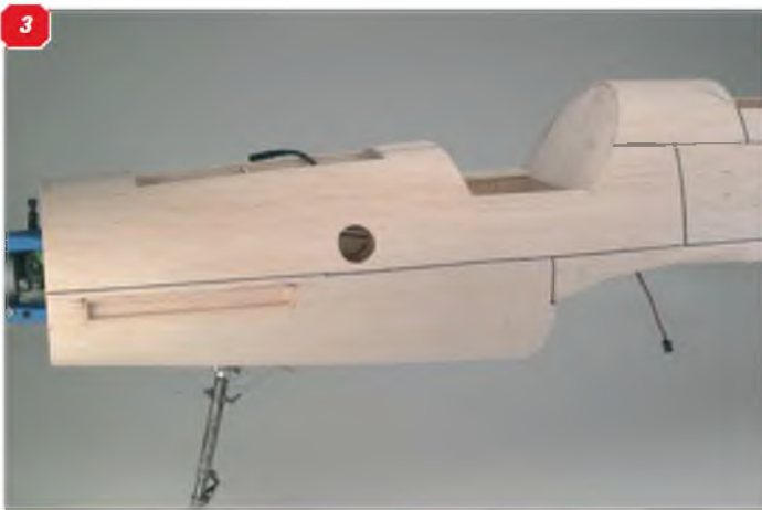
3: The nose skinned - the hole in the side is for cooling air to the esc/battery (scale position of an air intake). The exhaust stub box is flush-mounted, ready for the moulding. 4: The planked rear fuselage with the sheet panel lines highlighted. Well-soaked in water, the soft sheet easily took the double curvatures.
