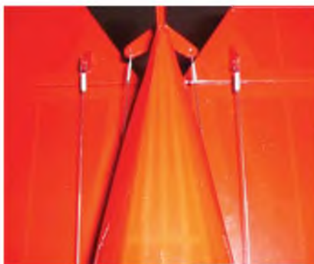
Aluminium tube crimps and a spot of thin CA secure the cables at both servo arms and control horns.
