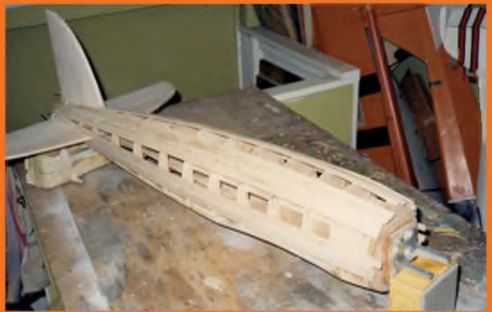
Planking progresses in four separate areas to speed up the process as the glue dries out.
