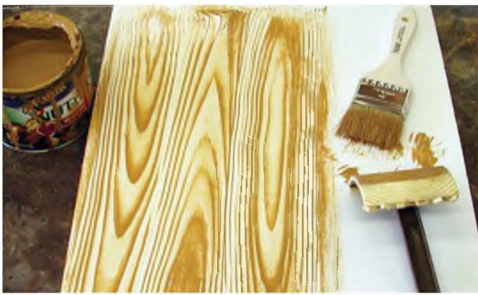
How the 'wood grain' tool is used to apply the finish to a board before it is transferred to waxed paper and then to the model.
