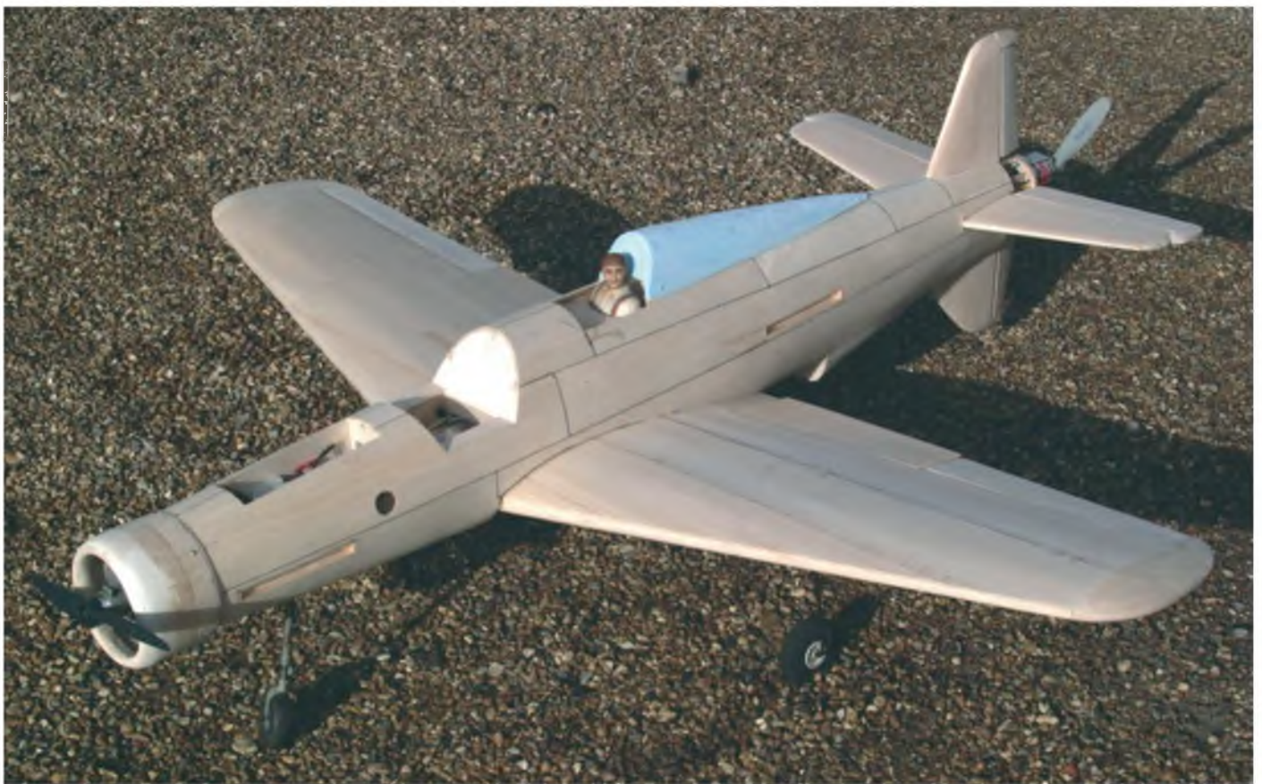
Needing just a top hatch, wing leading edge fairings at the root and wing seat, construction is pretty well complete - got to make the blanks now for the glazing moulds!
