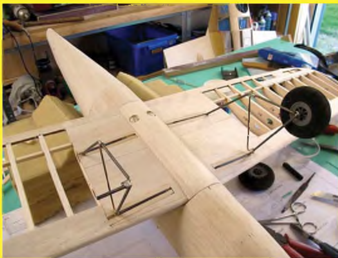
Note how the front undercarriage blocks have been trimmed to match the wing section, and how the u/c legs fit into the grooves.
