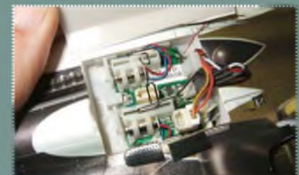
Under the 'bonnet' you can see the rudder and elevator servos/ pushrods plus motor connector (centre right) and aileron servo plug at bottom.
