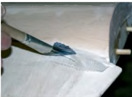
Don't trim the excess where it will be overlapped, work the agent into the cloth and work excess round the curves with the tip of the brush.
