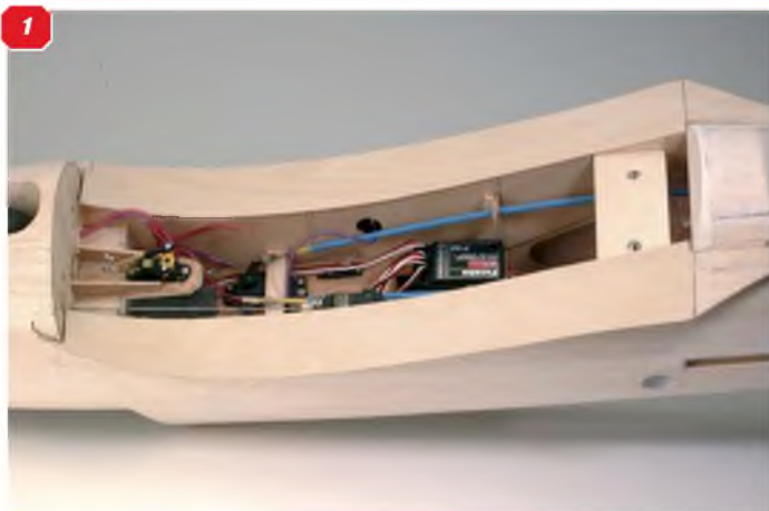
1: The ply wing fairing plates finally trimmed and fitted. 2: The ply plate 'kicks' up at the rear to align with the lower wing surface.
