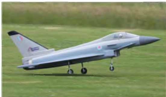
BELOW: Impressive BAe. Typhoon flown by Colin Gardner built from ComArt kit with glass fibre moulded fuselage. 28 lbs model uses Merlin 160 turbine from Spain and features Eurokit retracts.
