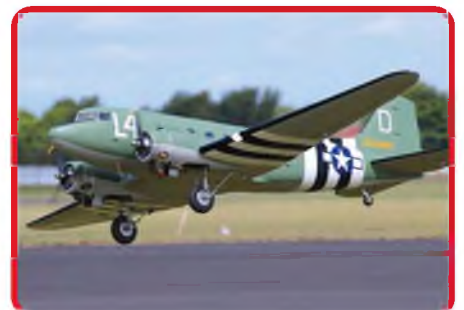
Dave Jones's 140" span C-47 Skytrain from the Nick Zirolli plan. Two Zenoah 38s on 18"x10 three bladers. Weighs 55lbs.
