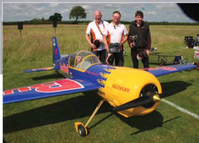
ABOVE: Steve Carr showed the way in 3D aerobatics with his superbly presented YAK 54. Model is 55% of full size and weighs a hefty 63 kg. (139 lbs). Steve created his own engine, machining his own crankcase and matching it to 3W cylinders. Multiplex radio.
