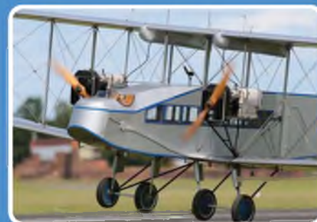
Don Billingham's HP W-10 Airliner, built to 1/4 scale, spans 15 feet, 2xLaser 360V Twin power.
