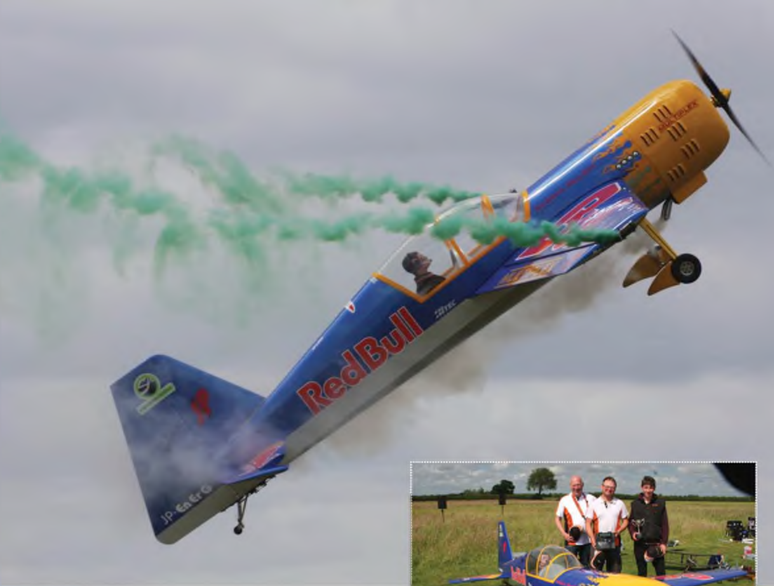
ABOVE: Steve Carr showed the way in 3D aerobatics with his superbly presented YAK 54. Model is 55% of full size and weighs a hefty 63 kg. (139 lbs). Steve created his own engine, machining his own crankcase and matching it to 3W cylinders. Multiplex radio.
