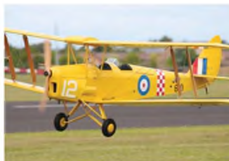
Gerhard Reinsch's huge Tiger Moth from the Toni Clark kit. 3.19 metres in span, Valach VM 120i2-4T In-Line four stroke twin power. Weighs 23.4 kgs.
