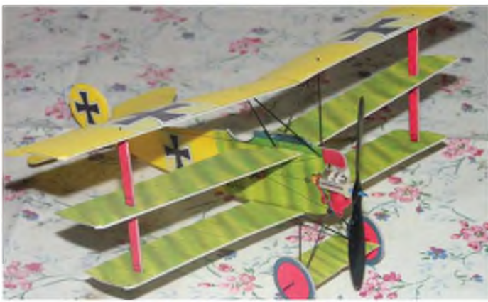
Just about the limit of our indoor venue's capability. 10 inch span and a ready to fly weight well below 10 grams.
