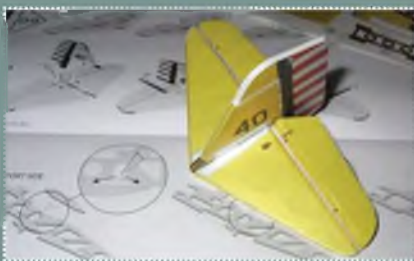
The results of my first evening's labours - chamfering, hinging, gluing and sticking.
