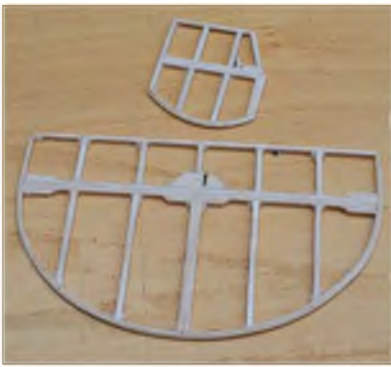
Laminated outlines work out much lighter and stronger than those built up from shaped sections - like in most rubber power kits.
