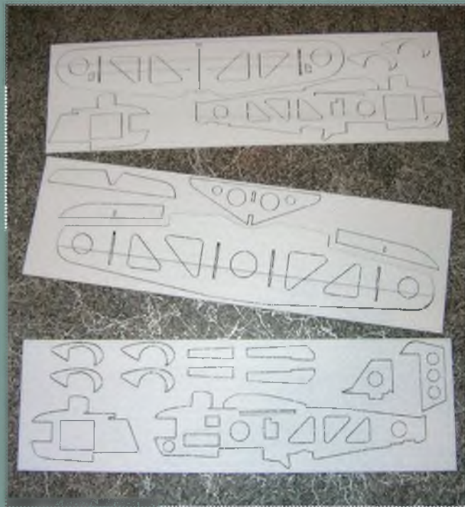
These are the laser cut Depron sheets with all the foam parts apart from the wheels.
