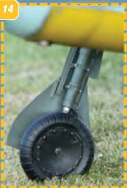
13: Fw 190 uses Sierra Precision wheels. 14: Keith used Sierra retracts and wheels. Note superb struts and oleos. 15: Wheel covers modelled in two parts, nicely stencilled and weathered.
