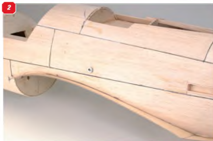
1: The ply wing fairing plates finally trimmed and fitted. 2: The ply plate 'kicks' up at the rear to align with the lower wing surface.
