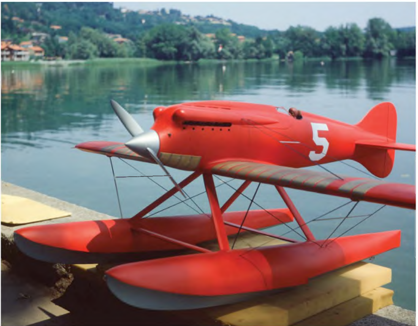
Superb model of one of the three Macchi M.39s flown in the 1926 event at Hampton Roads, USA. Carlo Bergamaschi won the 1981 Coppa Schneider with this Webra Speed 60 powered model. It handled water take-offs and landings perfectly.
