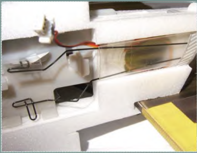
The clear tube housing the push-rods with my cut-away foam modification.
