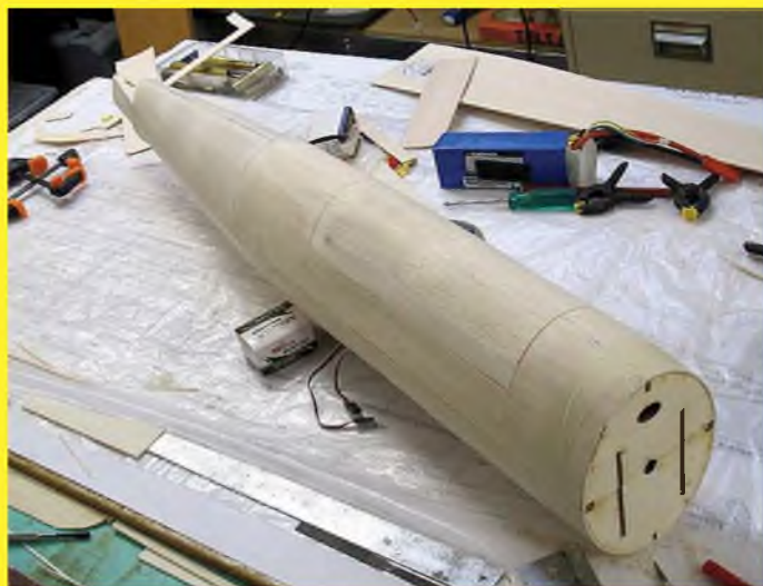
Because of the simpler shape, Pat was able to use pre-curved pieces of sheet to skin his fuselage.
