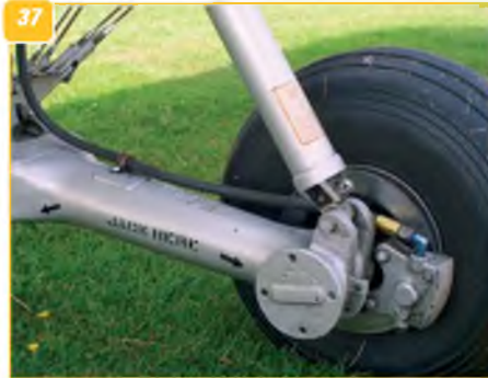
32-38: The main undercarriage in detail - likely to be a major undertaking in the construction of a model of the PT-22. The mechanism features a shock-absorbing arrangement designed to withstand the punishment inevitable when trainee pilots practise landings! With it 'hanging out', damage could be easily detected and parts quickly replaced.
