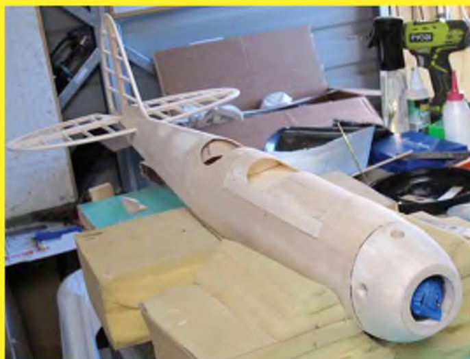
Note how Pat masked his motor while sanding the nose block to final shape.
