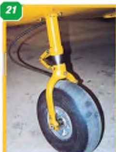
18: Elevator trim tab. 19: Close-up of the tailplane/elevator showing the hinge line and hole through fuselage for the elevator joiner. 20: Panel detail at wing leading edge above the main undercarriage leg. 21 & 22: two views of the main undercarriage leg. Wheel pants were regularly removed at the training establishments. Operating from grass fields, the wheel pants tended to collect mud inside, eventually build-up of which could result in risk of nose-over. 23: The steerable tailwheel unit.
