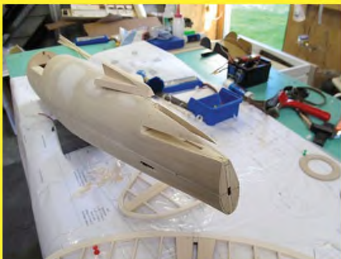
The fatter tail end is also part on the modifications Pat made. Here you see the template he made for shaping the tail blocks in situ.
