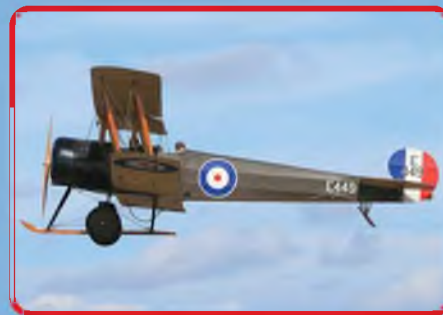
Steve Jackson's lovely 1/4 scale Avro 504 K. Laser 360 V Twin power. Based on the Hendon exhibit.
