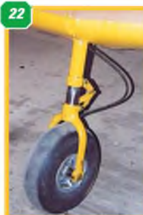
18: Elevator trim tab. 19: Close-up of the tailplane/elevator showing the hinge line and hole through fuselage for the elevator joiner. 20: Panel detail at wing leading edge above the main undercarriage leg. 21 & 22: two views of the main undercarriage leg. Wheel pants were regularly removed at the training establishments. Operating from grass fields, the wheel pants tended to collect mud inside, eventually build-up of which could result in risk of nose-over. 23: The steerable tailwheel unit.
