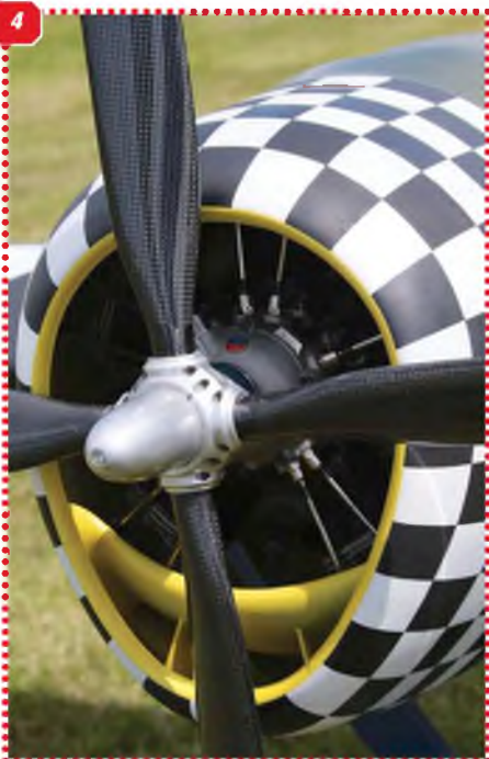
4: This model was designed around the famed Moki 250cc / 5 cylinder petrol radial engine. 5: Exquisite scale-finish variable-pitch carbon prop, hub, and spinner. Pitch can be altered on the ground. 6: Mail undercarriage inner door. 7: Superb Sierra Retracts sag like the real thing at rest. See text. Full size aircraft main U/C legs would foreshorten by 9" during retract sequence: difficult to reproduce in miniature.
