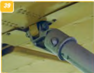
32-38: The main undercarriage in detail - likely to be a major undertaking in the construction of a model of the PT-22. The mechanism features a shock-absorbing arrangement designed to withstand the punishment inevitable when trainee pilots practise landings! With it 'hanging out', damage could be easily detected and parts quickly replaced.
