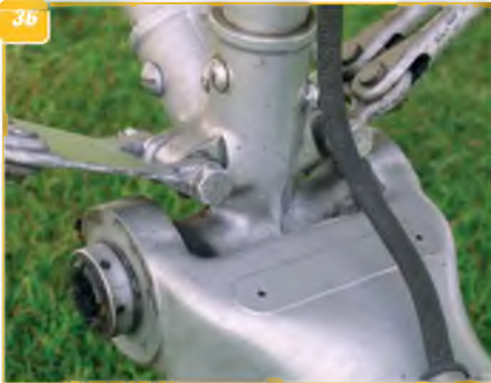
32-38: The main undercarriage in detail - likely to be a major undertaking in the construction of a model of the PT-22. The mechanism features a shock-absorbing arrangement designed to withstand the punishment inevitable when trainee pilots practise landings! With it 'hanging out', damage could be easily detected and parts quickly replaced.
