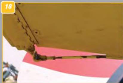
17: Rudder hinge and anchor point for bracing wire. 18: Underside of elevator, showing linkage to trim tab. 19: Tailplane junction with fuselage, showing the metal fairing. 20: The castoring tailwheel unit. 21: Detail of the top of the engine cowl, left side, showing the oil filler cap and top engine cylinder. 22: The fairing on the left fuselage side that covers the wing brace strut anchor point. Also, the anchor point for the bracing wire clevises. Right side similar. 23: Fuselage side detail, showing the pressed metal strake that runs along the side under the two cockpits.
