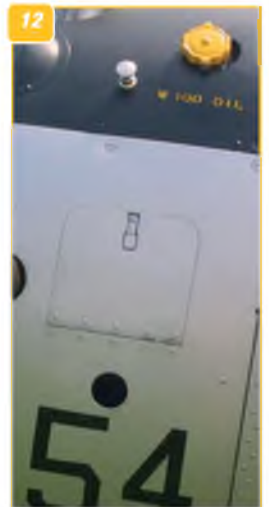
8: Right side of engine cowling showing air intake scoop and engine cylinders. 9: Close up of engine cylinder head (lower right pot). 10: Further detail of the front fuselage and engine cowling showing the wing brace strut and streamlined bracing wires. 11: Close-up detail of access panel on the left side of the engine cowling just behind the engine. 12: The engine cowling left side showing the access panel position and oil filler cap.
