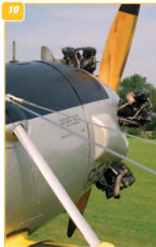
8: Right side of engine cowling showing air intake scoop and engine cylinders. 9: Close up of engine cylinder head (lower right pot). 10: Further detail of the front fuselage and engine cowling showing the wing brace strut and streamlined bracing wires. 11: Close-up detail of access panel on the left side of the engine cowling just behind the engine. 12: The engine cowling left side showing the access panel position and oil filler cap.
