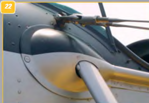
17: Rudder hinge and anchor point for bracing wire. 18: Underside of elevator, showing linkage to trim tab. 19: Tailplane junction with fuselage, showing the metal fairing. 20: The castoring tailwheel unit. 21: Detail of the top of the engine cowl, left side, showing the oil filler cap and top engine cylinder. 22: The fairing on the left fuselage side that covers the wing brace strut anchor point. Also, the anchor point for the bracing wire clevises. Right side similar. 23: Fuselage side detail, showing the pressed metal strake that runs along the side under the two cockpits.
