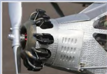
Cowling detail on Martin Fardell's electric powered Ryan Brougham. Weighs 12lbs.
