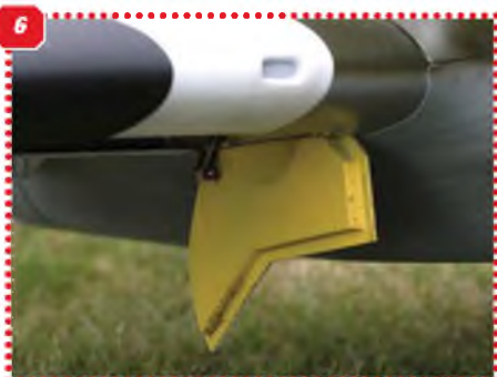
4: This model was designed around the famed Moki 250cc / 5 cylinder petrol radial engine. 5: Exquisite scale-finish variable-pitch carbon prop, hub, and spinner. Pitch can be altered on the ground. 6: Mail undercarriage inner door. 7: Superb Sierra Retracts sag like the real thing at rest. See text. Full size aircraft main U/C legs would foreshorten by 9" during retract sequence: difficult to reproduce in miniature.
