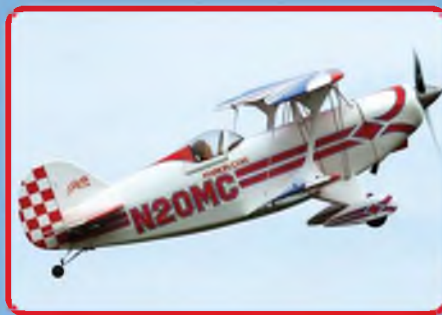
Alan Glover's pretty 1:3.5 scale Pitts Special. Saito 300 Twin, driving a 21"x8" prop.
