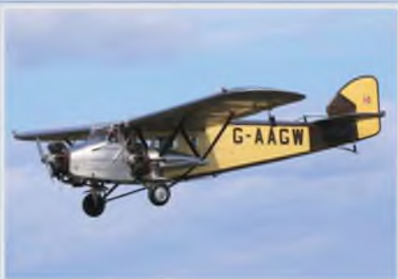
Richard Crapp's astounding Wessex has three engines, one Laser 120 and two Laser 75s.
