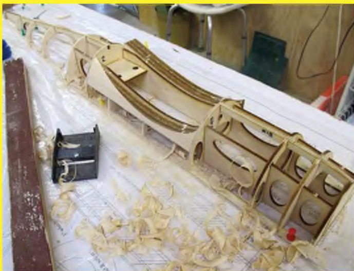
As you see, Pat chose to trim the wing seat parts flush with the formers and sheet over them.
