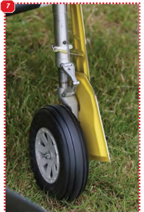
4: This model was designed around the famed Moki 250cc / 5 cylinder petrol radial engine. 5: Exquisite scale-finish variable-pitch carbon prop, hub, and spinner. Pitch can be altered on the ground. 6: Mail undercarriage inner door. 7: Superb Sierra Retracts sag like the real thing at rest. See text. Full size aircraft main U/C legs would foreshorten by 9" during retract sequence: difficult to reproduce in miniature.
