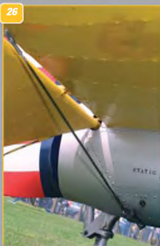
29: Rear fuselage at the tail post, showing the elevator joiner and the flexible control link to the elevator trim tab.
