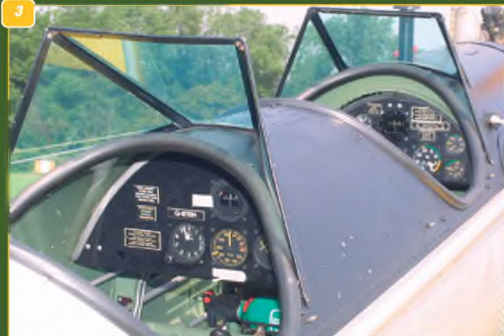
1 & 2: Two views of the front fuselage section and cockpit, showing the windscreen, instrument panel, bracing strut and bracing wires with adjustable clevises. 3: View of the two open cockpits showing both windscreens and the cockpit coamings. 4: Rear cockpit instrument panel. 5: Control column and rudder pedals in the rear cockpit. Front cockpit similar. 6: Throttle quadrant on the left side of the rear cockpit. 7: Rear cockpit coaming and headrest.
