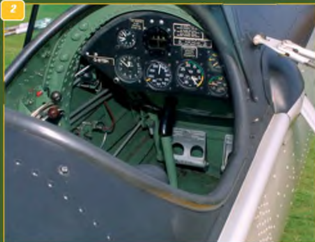
1 & 2: Two views of the front fuselage section and cockpit, showing the windscreen, instrument panel, bracing strut and bracing wires with adjustable clevises. 3: View of the two open cockpits showing both windscreens and the cockpit coamings. 4: Rear cockpit instrument panel. 5: Control column and rudder pedals in the rear cockpit. Front cockpit similar. 6: Throttle quadrant on the left side of the rear cockpit. 7: Rear cockpit coaming and headrest.
