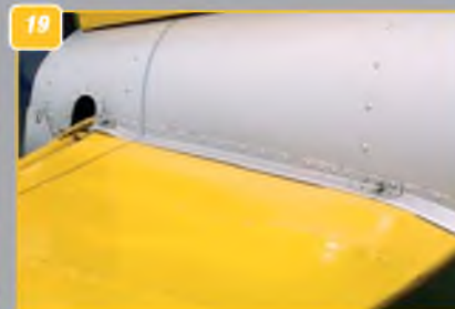
17: Rudder hinge and anchor point for bracing wire. 18: Underside of elevator, showing linkage to trim tab. 19: Tailplane junction with fuselage, showing the metal fairing. 20: The castoring tailwheel unit. 21: Detail of the top of the engine cowl, left side, showing the oil filler cap and top engine cylinder. 22: The fairing on the left fuselage side that covers the wing brace strut anchor point. Also, the anchor point for the bracing wire clevises. Right side similar. 23: Fuselage side detail, showing the pressed metal strake that runs along the side under the two cockpits.
