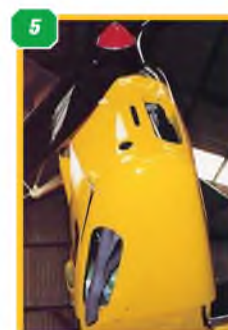
1: The Shuttleworth Collection's machine P6382 at Old Warden is one of the two examples in this photo-detail feature. 2: The line of the engine cowl viewed from across the starboard wing. 3: The nose, showing the panel lines and air intake. Note the size of the panel fasteners. 4: A further view of the cowl from the starboard side. 5: Head-on view of the nose showing the exhaust exit.
