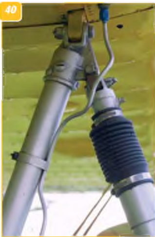
39: The main undercarriage rear anchor point under the wing. 40: Front main undercarriage anchor point on wing underside. 41 & 42: Centre-line bubble fairing on fuselage bottom where the main undercarriage bracing wires attach to the fuselage. 43: Pressed metal fairings and access panels on wing underside. 44: The wing root, right hand side, showing rubber panel seals, the cockpit access tread panel and the main bracing strut. 45: Detail of the pressed metal bubble fairing that covers the wing brace anchor point. 46: The cockpit access tread panel on the right hand wing panel. Left side similar. 47: The pitot head on the left wing panel. 48: The right wing, showing the aileron and flap.
