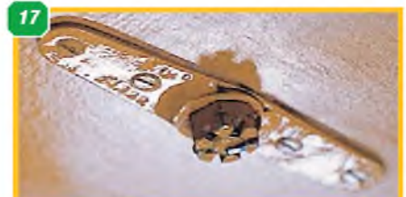
13 & 14: Two views of the tailcone. Note the unshrouded hinge lines and anti-spin strakes. 15: Top surface aileron hinge, reminiscent of typical sport R/C model! 16: Tie-down point on wing underside. 17: Corresponding retainer plate on wing top surface.
