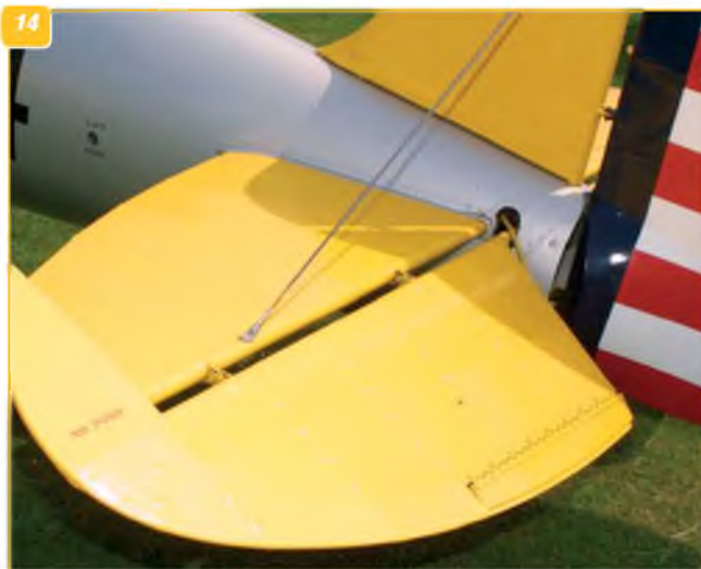
13: The fin and rudder, showing the hinging and the gap between the two vertical surfaces. 14: The tailplane and elevator are similarly hinged and widely separated. 15: Detail of an elevator hinge and anchor point for the bracing wire between the tailplane and the fin. 16: Close-up of the top surface hinge-line of the left side elevator trim tab.
