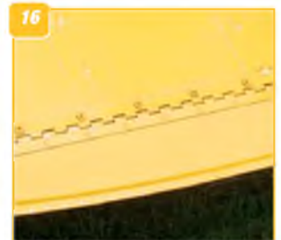
13: The fin and rudder, showing the hinging and the gap between the two vertical surfaces. 14: The tailplane and elevator are similarly hinged and widely separated. 15: Detail of an elevator hinge and anchor point for the bracing wire between the tailplane and the fin. 16: Close-up of the top surface hinge-line of the left side elevator trim tab.
