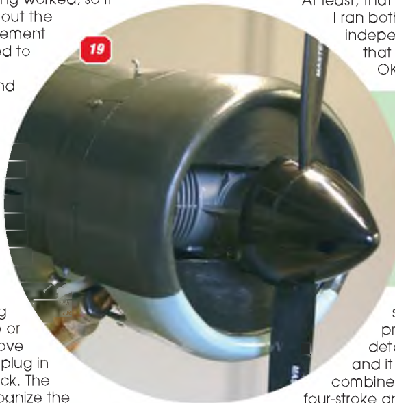
The RCV 58CD fits perfectly into the very small diameter cowl and a front blanking plate ensures that all the air going into the cowl goes through the head fins.
