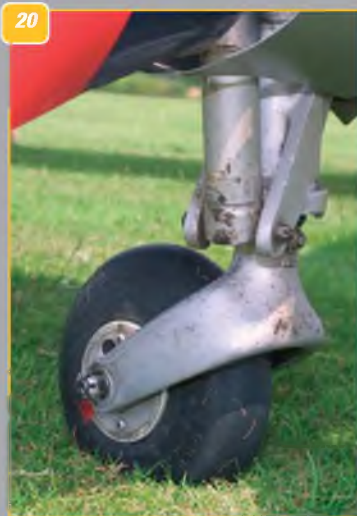
17: Rudder hinge and anchor point for bracing wire. 18: Underside of elevator, showing linkage to trim tab. 19: Tailplane junction with fuselage, showing the metal fairing. 20: The castoring tailwheel unit. 21: Detail of the top of the engine cowl, left side, showing the oil filler cap and top engine cylinder. 22: The fairing on the left fuselage side that covers the wing brace strut anchor point. Also, the anchor point for the bracing wire clevises. Right side similar. 23: Fuselage side detail, showing the pressed metal strake that runs along the side under the two cockpits.
