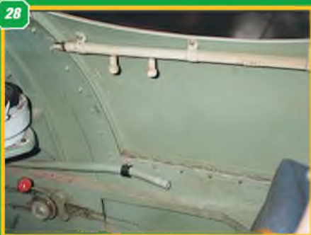
24: Similar view from the Port side. 25: Close up of cockpit interior showing the compass mounted on the Starboard side. 26: Rear of the front cockpit. Note the internal bracing members. 27: Similar view of rear cockpit. Bracing members are different. 28: View of cockpit interior showing the access door. 29: View down the fuselage showing the anti-spin strakes.
