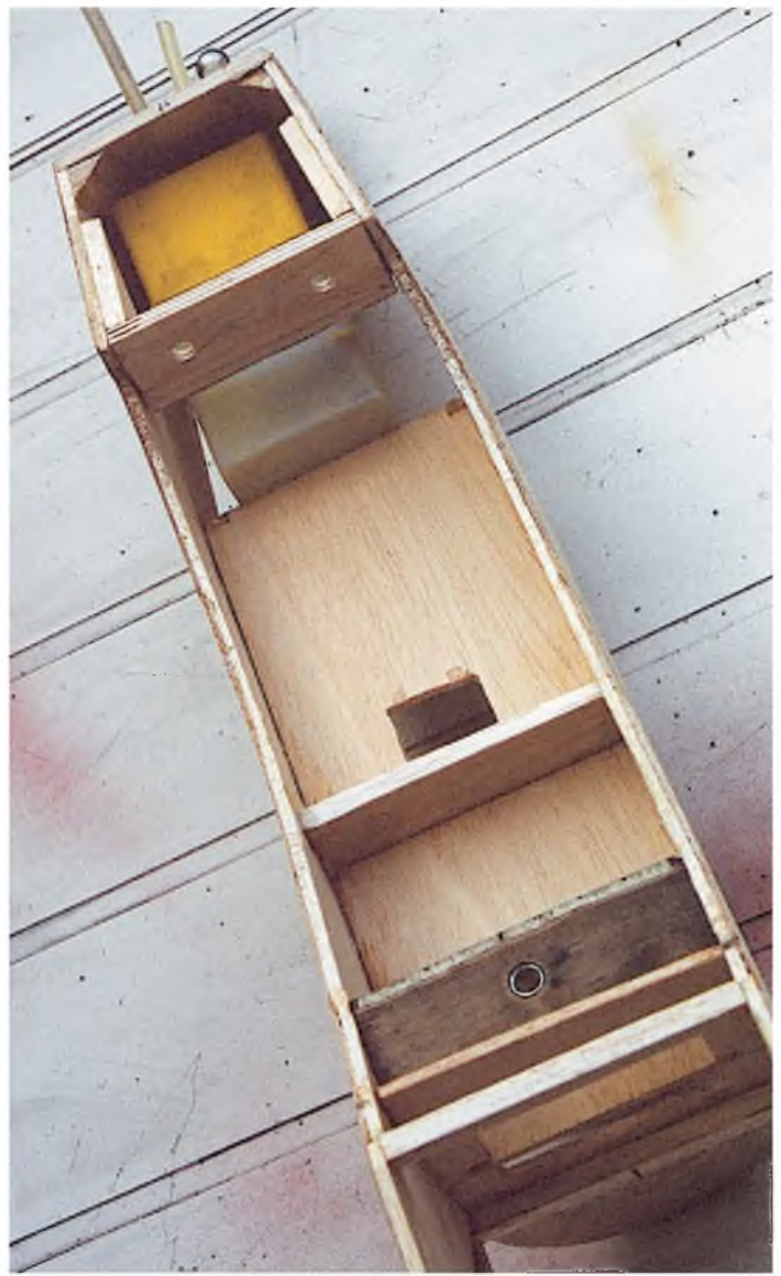
Underside view of the fuselage centre section, showing plenty of space for the radio installation.
