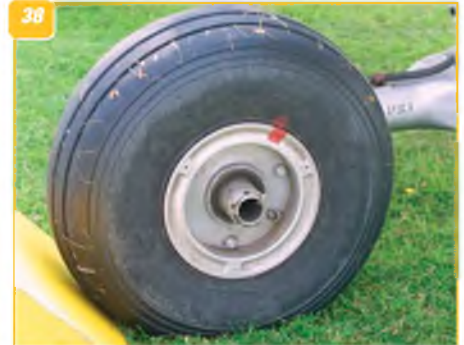
32-38: The main undercarriage in detail - likely to be a major undertaking in the construction of a model of the PT-22. The mechanism features a shock-absorbing arrangement designed to withstand the punishment inevitable when trainee pilots practise landings! With it 'hanging out', damage could be easily detected and parts quickly replaced.
