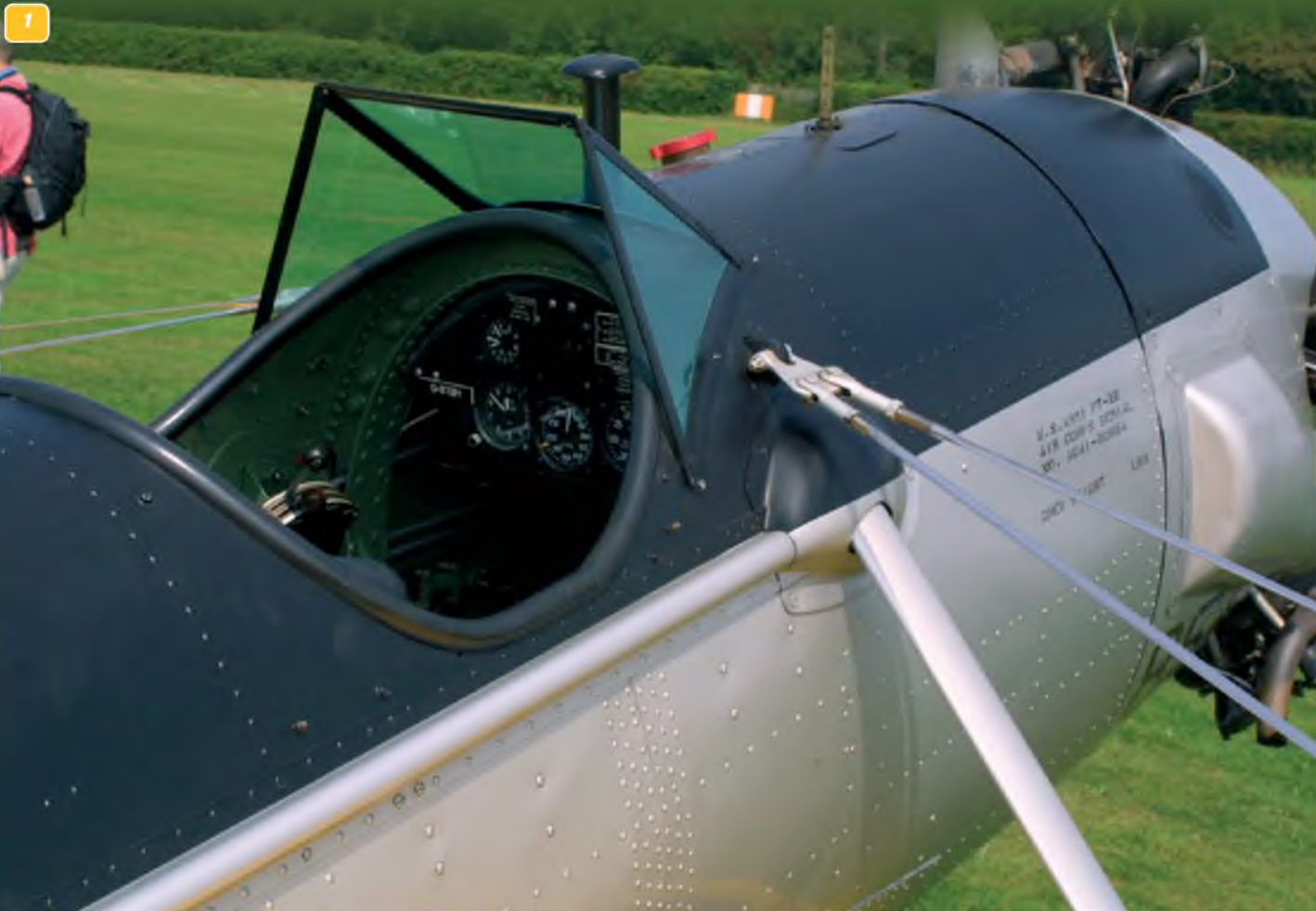
1 & 2: Two views of the front fuselage section and cockpit, showing the windscreen, instrument panel, bracing strut and bracing wires with adjustable clevises. 3: View of the two open cockpits showing both windscreens and the cockpit coamings. 4: Rear cockpit instrument panel. 5: Control column and rudder pedals in the rear cockpit. Front cockpit similar. 6: Throttle quadrant on the left side of the rear cockpit. 7: Rear cockpit coaming and headrest.
