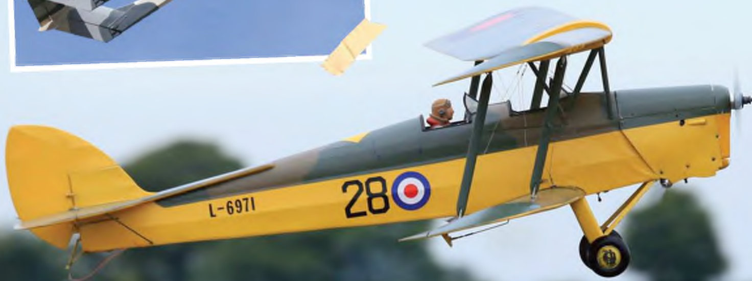
MR MURRAY'S 20 YEAR OLD TIGER MOTH FROM THE AULD PREMIER KIT. 66" SPAN, 1/6TH SCALE, OS 91 FS POWER.
