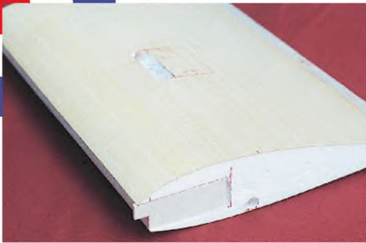
Fully skinned foam core wing panel.
