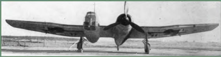
The Bv 141's retracting main undercarriage featured widely spaced legs that retracted outwards. The wide spacing would have been good for rough field operations as would have been the likely case on the Eastern Front.
