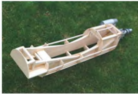
Underside view of the front fuselage, showing the staggered joint line build.
