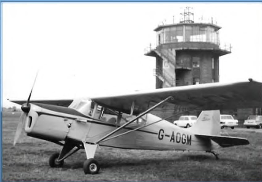
Two views of J-5P Autocar G-AOGM fitted with a 145 hp D.H. Gipsy Major 10 engine and equipped for aerial - see camera port on the starboard side aft of the cabin. The aircraft was based for a while at Elstree, where this photograph was taken in the early 1960s.
