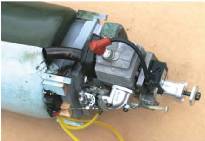
The first engine fitted was a Zenoah 38. Note the throttle servo mounted on the bottom of the motor box and the large lump of lead needed to balance the model.
