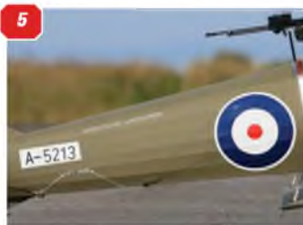
4: As per the full-size example, Tim's FK 10 has an all-flying tailplane. 5: Model is covered in Solartex. Four metres of linen and six metres of green. 6: Tim used white marker pens to legend his model. 7: Anti-drag wires (fishing trace, nylon coated) terminate in the rear lower fuselage.
