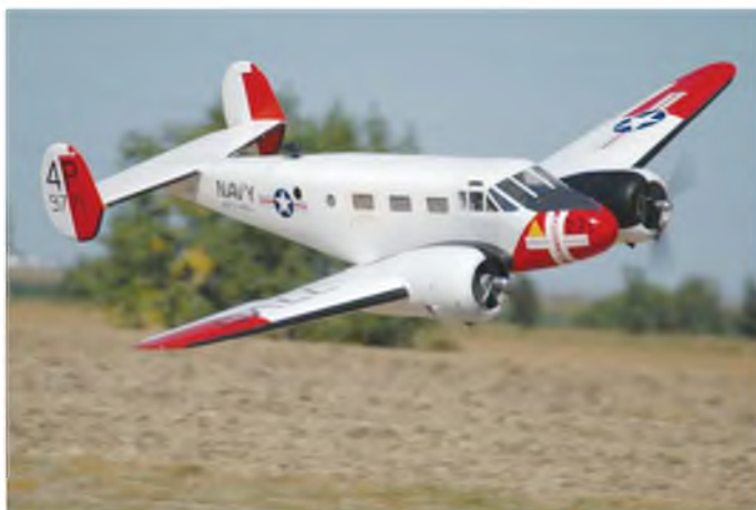
Twin engine type with twin fins, like this Beech C-45 have the advantage that propeller wash over the fin and rudder on the 'live side' can be useful in counteracting and controlling power asymmetry.
