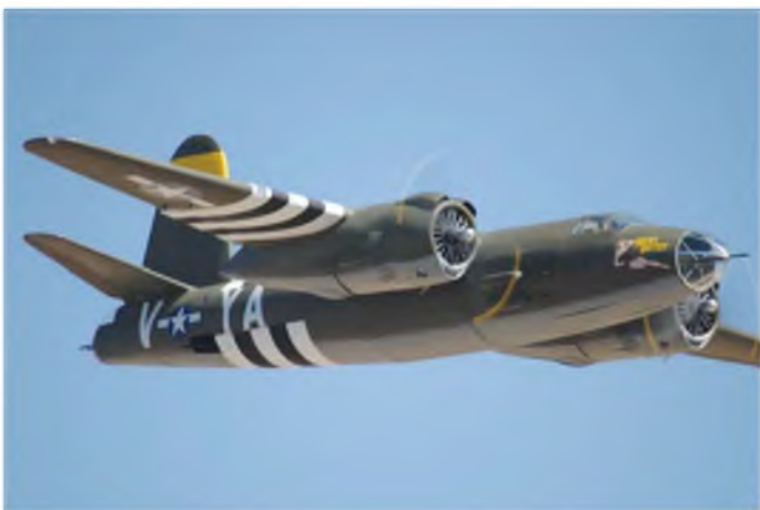
Even the full size Martin B-26 Marauder had a reputation for being a handful! As a model, the lack of dihedral imparts no inbuilt stability, so pre-flight preparation to ensure engine reliability is a wise precaution.
