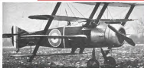
One of the Armstrong Whitworth examples of the FK 10, showing the sturdy nature of the wing strutting. Note the fully rounded metal engine cowl, without the cut-out in the lower part of the cowl ring. The manufacturer's name is written along the rear fuselage upper side longeron.
