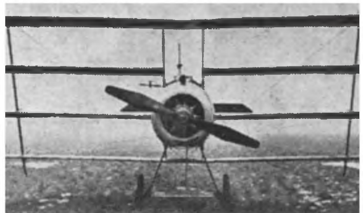
Head-on view reveals the lack of centre section panel on the 3rd (one down from the top) wing to allow space for the pilot's head and shoulders.
