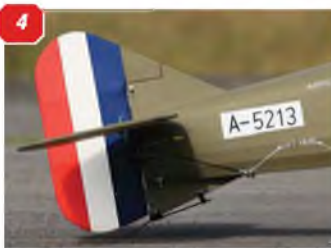
4: As per the full-size example, Tim's FK 10 has an all-flying tailplane. 5: Model is covered in Solartex. Four metres of linen and six metres of green. 6: Tim used white marker pens to legend his model. 7: Anti-drag wires (fishing trace, nylon coated) terminate in the rear lower fuselage.
