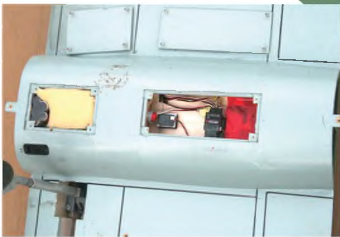
Two hatched in the belly of the motor boom give access to the receiver and flight batteries.
