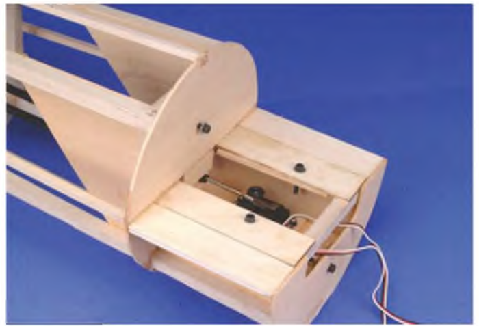
The inverted rear fuselage section, showing the staggered joint, four mounting bolts and the rudder/elevator servos.
