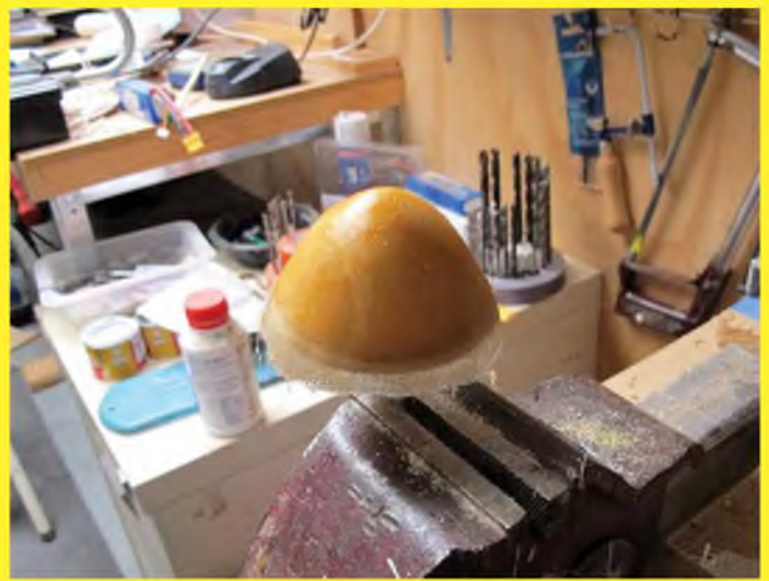
The turned foam, spinner has had a layer of glass cloth smoothed into place with resin and is being allowed to cure.
