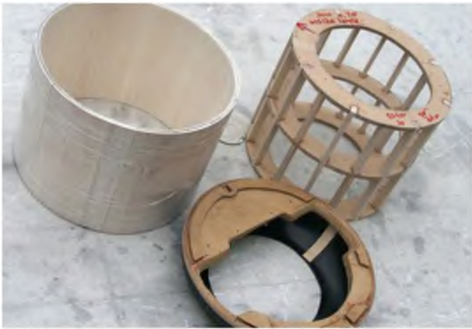
Making your own cowl. In this case, for the bigger, 12ft span Bv. The nosering in this case is moulded plastic, but a simpler, carved balsa, ring on the front of the laminated balsa tube is easy.
