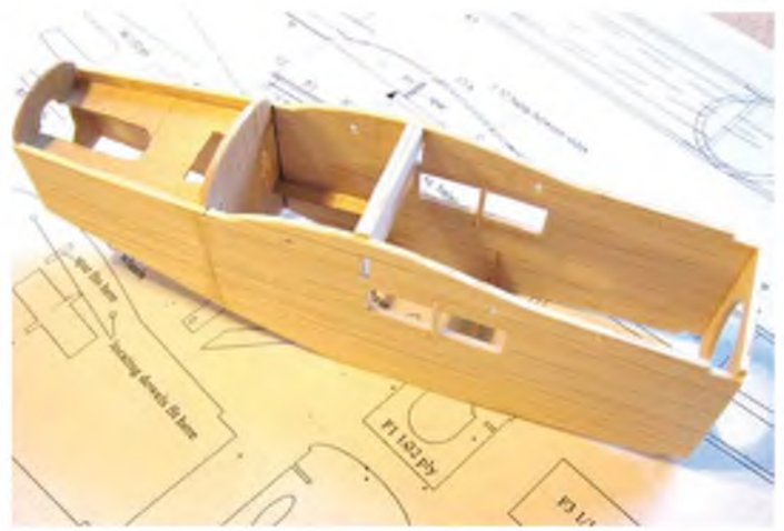
The basic forward fuselage box all assembled and ready to have the rear end fitted.
