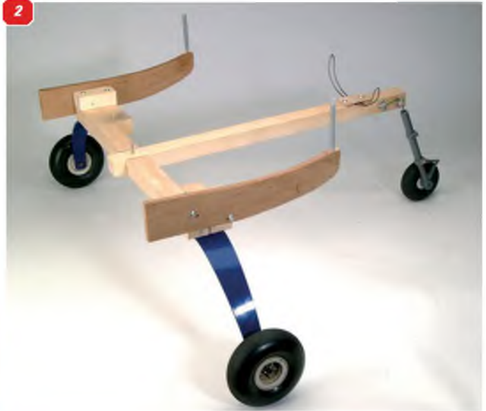
1: Just one shot of her flying! The very first flight - you can see the starboard uc leg hanging off, starting the curse of the retracts saga! She looks good, handles well, is very fast - and sounds great! 2: The dolly - after several retract failures, this seemed the right way to go when flying off of less than billiard table grass!
