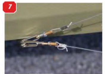
4: As per the full-size example, Tim's FK 10 has an all-flying tailplane. 5: Model is covered in Solartex. Four metres of linen and six metres of green. 6: Tim used white marker pens to legend his model. 7: Anti-drag wires (fishing trace, nylon coated) terminate in the rear lower fuselage.
