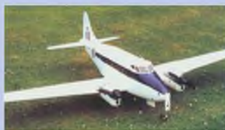
De Havilland Devon has engines particularly close to the centreline, but those narrow wing tips invite a tip stall.
