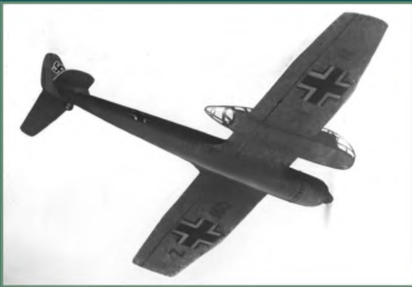
Once accustomed to the unique airframe layout, one appreciates the aerodynamically clean shape of the Bv 141. BMW 801 is closely cowled.
