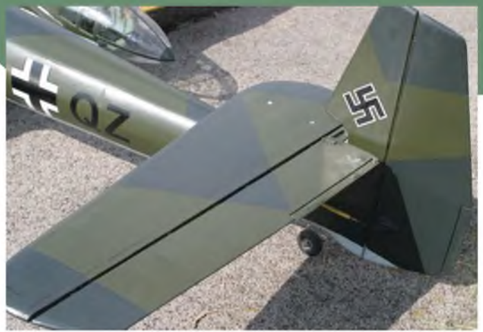
That offset tail which helps give the Bv the asymmetry. The support strut is functional, so needs to be securely fitted.
