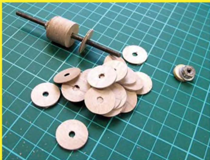
The humble beginnings of the dummy cylinders, a multitude of ply discs.
