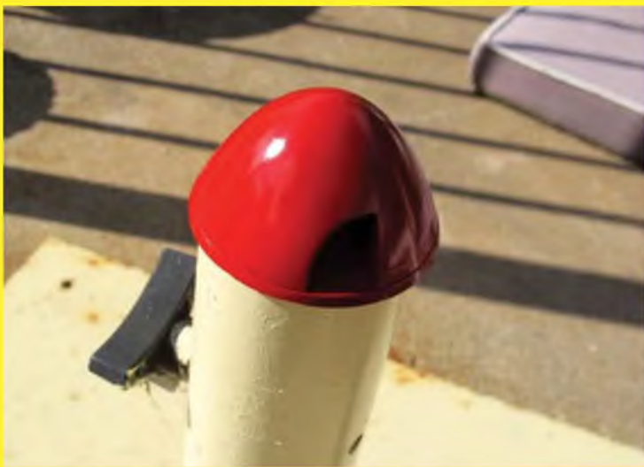
Filled, sanded, primed and painted the finished spinner has a ply back plate and is cut away to clear the prop.
