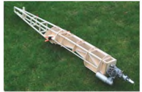
The two sections temporarily joined to allow the four bolt/blind nuts that hold the two parts together to be drilled and fitted.
