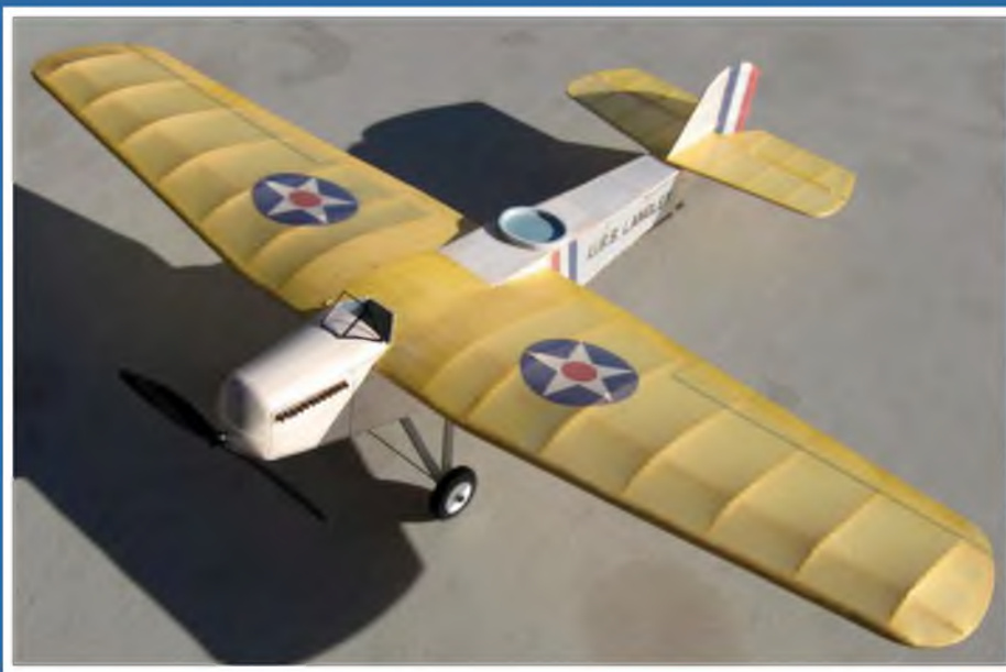
All set to commit aviation, the models shows off its' printed tissue finish nicely.
