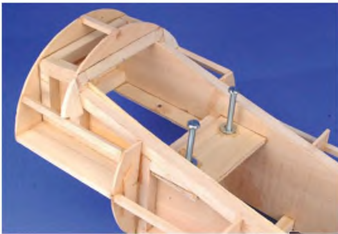
Close-up of the rear for the wing seat, showing the wing mounting bolts and the staggered joint build.
