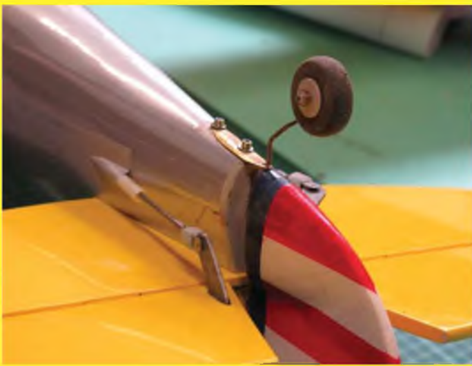
Here you see Pat's thickened lower rudder which matches his modified rear fuselage.
