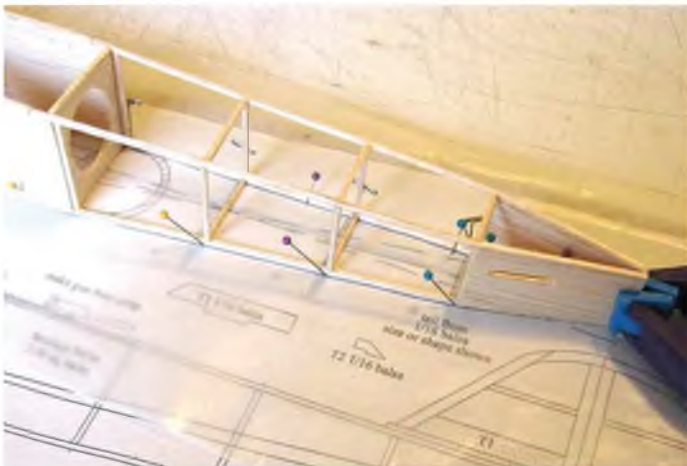
Working over the plan helps ensure a straight fuselage once the front and rear sections are joined.
