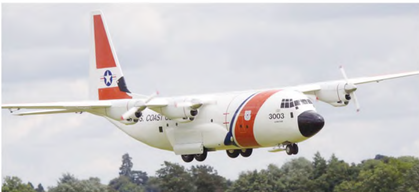
One engine out on a four-engine type has less adverse effect than for a twin, particularly if the dead 'un is one of the inners. Although it looks here as though it's a completely dead-stick landing, it's the port outer that died - the others are as idle for landing and the speed of the camera setting appears to have stopped the lot!
