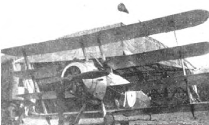
Front view here shows the relief in the lower section of the engine cowl as applied to some of the few FK 10s produced.
