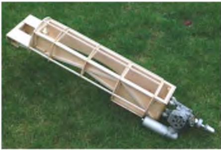
The front section of the two-part fuselage, showing the original S/T 3000 glow motor fitted (retrospectively fitted with a 45cc petrol engine).
