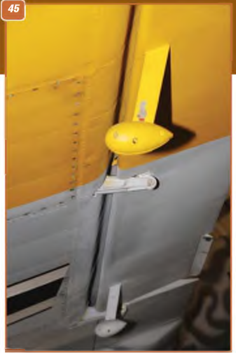
42: Aerial positioned on the outer left wing underside. 43: Variable cooler exit on the wing trailing edge at the engine nacelle position. Also seen in picture 44, 45 & 46: Underside view of the aileron, showing the two mass balances and aileron hinges. 47: Air intake in the left wing leading edge, just outboard of the engine nacelle. 48: Landing light in the left wing leading edge. 49: Further view of the aileron hinges and inner mass balance. 50: Wing tip aileron hinge. 51: Wing flap hinge line on the wing upper surface.
