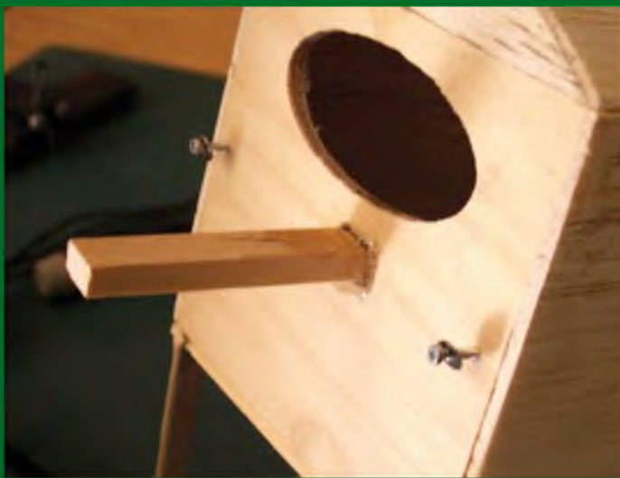
Hardwood motor post suits either basic GWS style unit or, as John did, a brushless equivalent. Plan also shows CD-R type motor installation.
