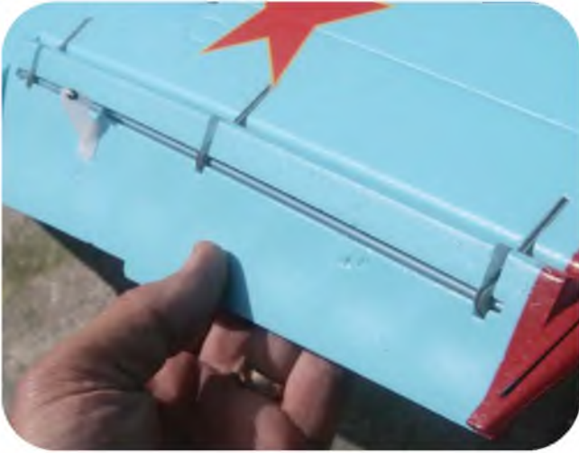
One of the scale-hinged Frise ailerons.
