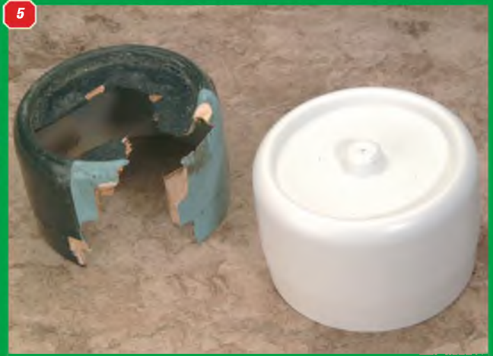
4: One end of the replacement harness - gold connectors, large diameter flux ring and twisted cable between motor and Esc - a combination that worked! 5: The original damaged cowl and the excellent replacement moulding made by Dave Rayner (see text). 6: Ready for final painting. Note the rotation of the RCV from the original position to protect the silencer in a belly landing.
