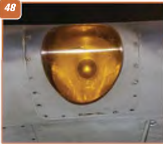
42: Aerial positioned on the outer left wing underside. 43: Variable cooler exit on the wing trailing edge at the engine nacelle position. Also seen in picture 44, 45 & 46: Underside view of the aileron, showing the two mass balances and aileron hinges. 47: Air intake in the left wing leading edge, just outboard of the engine nacelle. 48: Landing light in the left wing leading edge. 49: Further view of the aileron hinges and inner mass balance. 50: Wing tip aileron hinge. 51: Wing flap hinge line on the wing upper surface.
