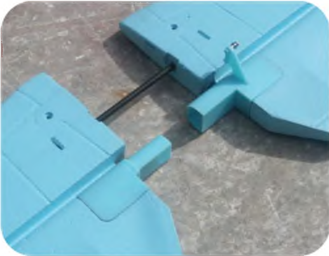
The tail blades, showing joining system.
