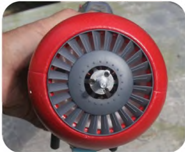
The front of the large cowl with scale shuttering.
