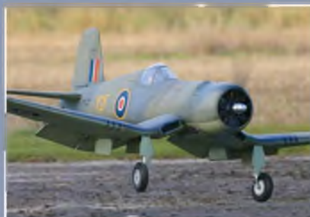
Richard Dalglish's Brian Taylor Corsair. Built to 1/6th scale, weighs 19 lbs, and is powered by a laser 200V Twin, driving an 18"x8" prop.
