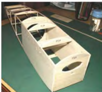
With the basic box structure assembled, John begins to add decking formers.
