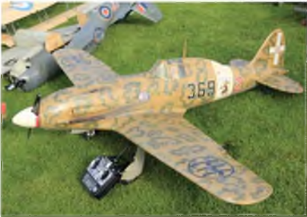
Dennis Richardson's elegant Macchi Folgore. 72" span, weighs 12 lbs, Laser 150 power, driving a 16"x82 prop.
