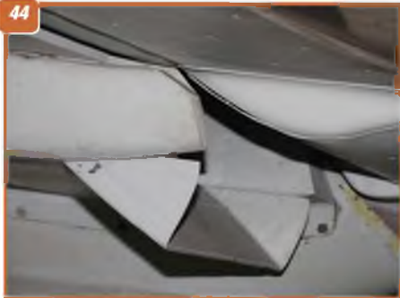
42: Aerial positioned on the outer left wing underside. 43: Variable cooler exit on the wing trailing edge at the engine nacelle position. Also seen in picture 44, 45 & 46: Underside view of the aileron, showing the two mass balances and aileron hinges. 47: Air intake in the left wing leading edge, just outboard of the engine nacelle. 48: Landing light in the left wing leading edge. 49: Further view of the aileron hinges and inner mass balance. 50: Wing tip aileron hinge. 51: Wing flap hinge line on the wing upper surface.
