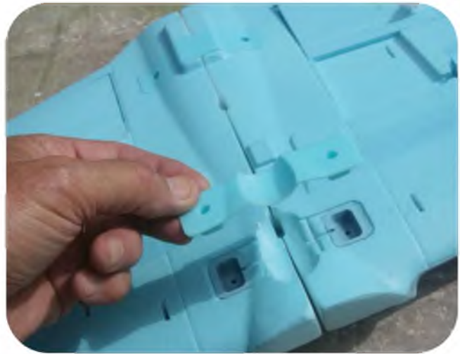
Two plastic fittings hold the wing halves together - with four bolts.
