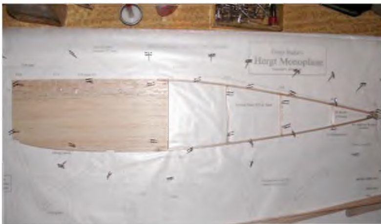
Nothing complicated about the fuselage side frames. Getting a straight fuselage is easy with this one -what you see here is the only taper involved.
