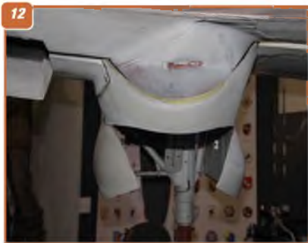
6 & 7: front and rear angles of one of the auxiliary fuel tanks carrier under the wings, outboard of the engine nacelles. 8: The fuel tank retainer shackles, also showing the fuel feed lines. 9: General view of the left engine nacelle. 10: Underside air scoop. 11: Rear view showing the wing skin fairing over the engine nacelle. 12: Further rear view, showing the main undercarriage fairing doors. 13 & 14: Two views of the nose spinner. 15 & 16: Two views of the fin and rudder assembly. 17: Aerial running along the rear fuselage underside centreline.
