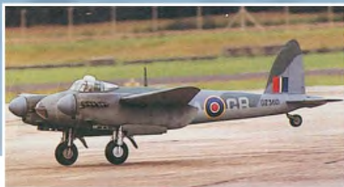
De Havilland Mosquito's sharply tapered wings would be an added disadvantage in a one-engine-out situation. Keep the speed up - even with both running, a 'wheelie' landing is perhaps best with this type.
