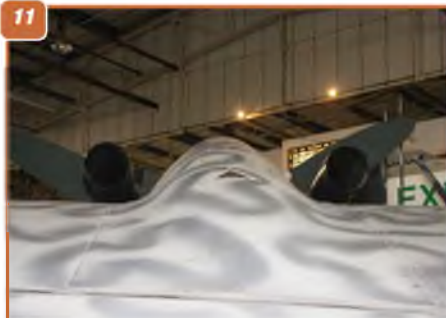
6 & 7: front and rear angles of one of the auxiliary fuel tanks carrier under the wings, outboard of the engine nacelles. 8: The fuel tank retainer shackles, also showing the fuel feed lines. 9: General view of the left engine nacelle. 10: Underside air scoop. 11: Rear view showing the wing skin fairing over the engine nacelle. 12: Further rear view, showing the main undercarriage fairing doors. 13 & 14: Two views of the nose spinner. 15 & 16: Two views of the fin and rudder assembly. 17: Aerial running along the rear fuselage underside centreline.
