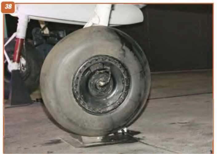
33: Main undercarriage leg and view up into the wheel well.
