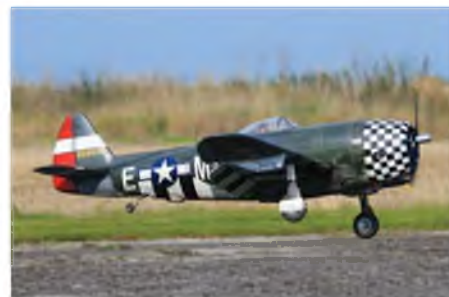
Topflight kit-built Thunderbolt, 85" span, Zenoah 62 power, owned by Chris Berry. Robarts retracts.
