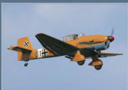
Neil Armstrong flew his lovely Stuka from the Nic Zirolli plan. 100" span, DLE 55 petrol power, driving a 24"x8" prop.
