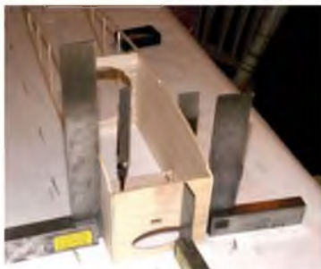
Models fly better with square fuselages so take care to keep it that way. This is especially important while adding sheet decking.
