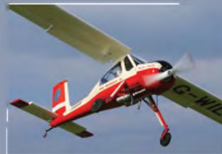
Tony Hill's PZL Wilga, 1/3rd scale / 3.5 metres in span. DLE 170 petrol engine driving a 33"x10" prop.
