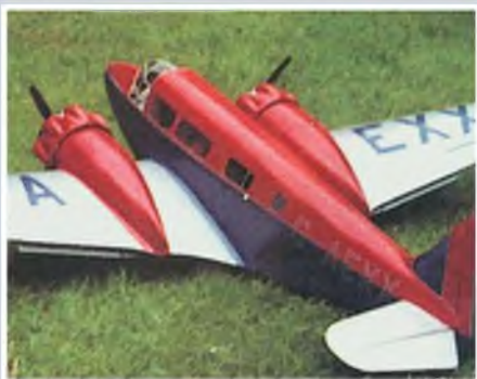
Airspeed Envoy is an example of a twin engine type with engines reasonably close to the centre line - which makes 'one-engine-out' a more manageable problem.
