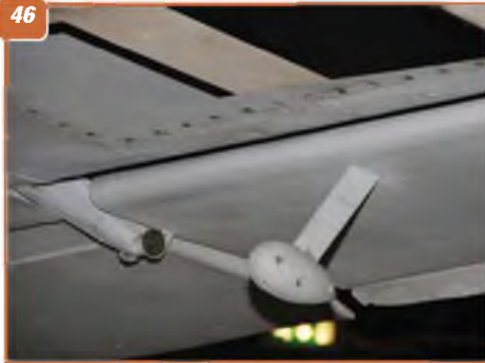
42: Aerial positioned on the outer left wing underside. 43: Variable cooler exit on the wing trailing edge at the engine nacelle position. Also seen in picture 44, 45 & 46: Underside view of the aileron, showing the two mass balances and aileron hinges. 47: Air intake in the left wing leading edge, just outboard of the engine nacelle. 48: Landing light in the left wing leading edge. 49: Further view of the aileron hinges and inner mass balance. 50: Wing tip aileron hinge. 51: Wing flap hinge line on the wing upper surface.
