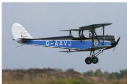
Peter Smedley's DH 60 from the Ripmax ARTF. 882 span, Zenoah 38 power, driving an 18"x12" prop.
