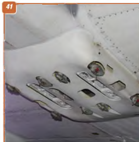
40: Further view of the rear fuselage underside showing the position of the aerial array along the centre line.
