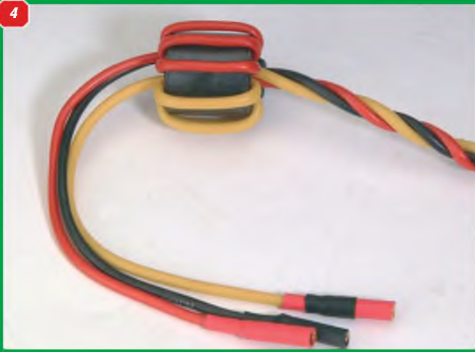
4: One end of the replacement harness - gold connectors, large diameter flux ring and twisted cable between motor and Esc - a combination that worked! 5: The original damaged cowl and the excellent replacement moulding made by Dave Rayner (see text). 6: Ready for final painting. Note the rotation of the RCV from the original position to protect the silencer in a belly landing.
