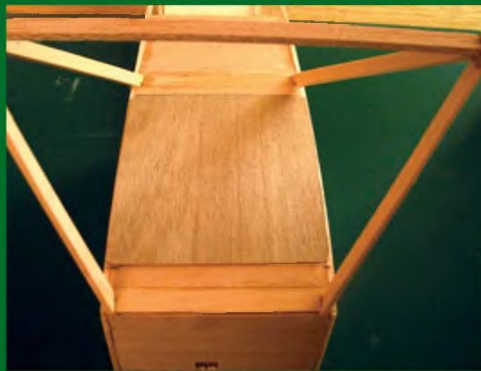
The all wood u/c legs glue in place and the access hatch fits between them.
