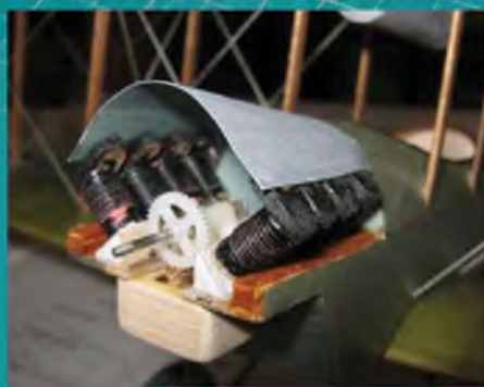
This shot should reveal just how much drag Larry built into his model. That enormous scoop must gather in a lot of air.
