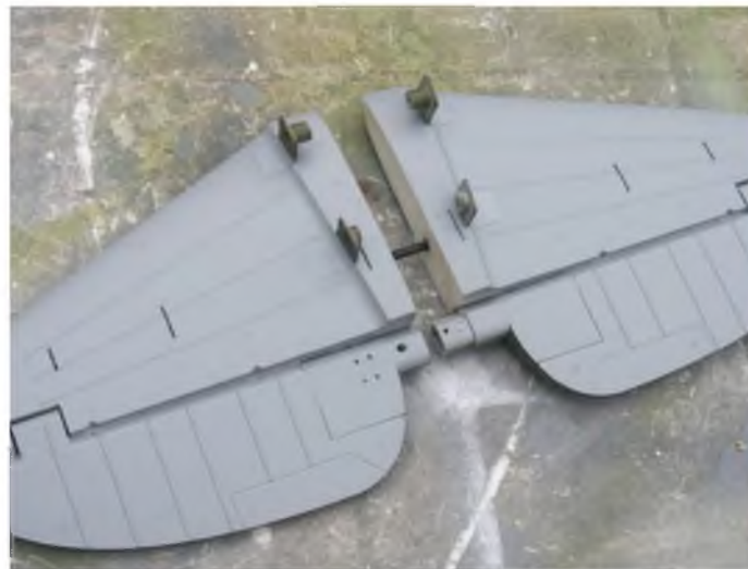
The two tail blades pushed together to show joiners and retaining lugs.
