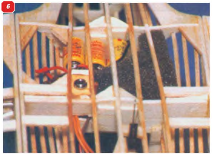
5: Mk.2 unit, showing the fuselage nose of the West Wings Spitfire Mk.22 into which it plugs. 6: Detail of the battery, mounted in the rear wing bay. Note the charging socket and on/off switch. 7: Mk.3 CRP unit, using Scientext ST-2 motor. 8: Mk.3 unit extracted from the Spitfire nose.
