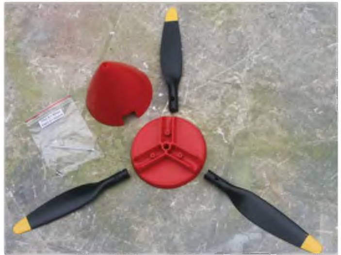
The prop blades a positively located and retained with a single self-tapping screw into the spinner backplate.
