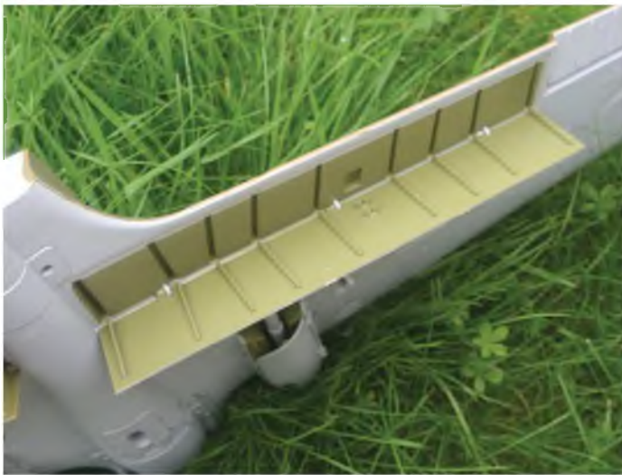
One of the flaps in full 'down' position - a little 'down' elevator mixed in is advised.
