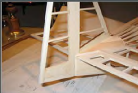
How the tail surfaces will fit once the packing pieces have been removed.
