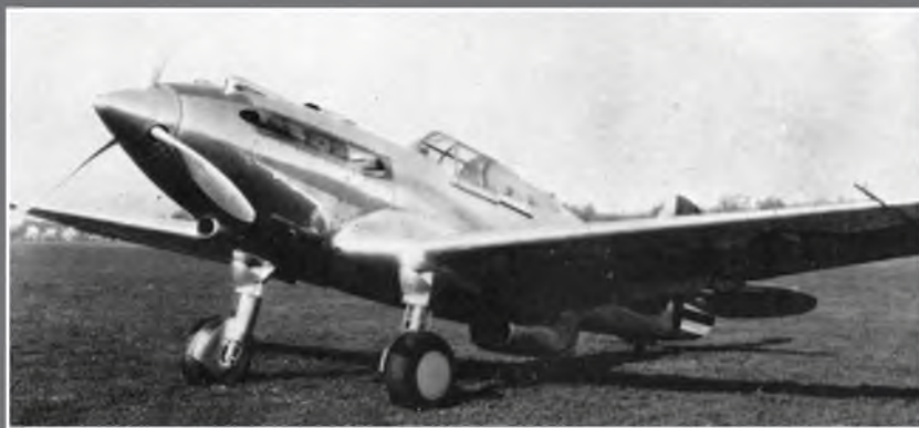
The XP-40 prototype as it first appeared, with fuselage underside air scoop at the wing trailing edge position. Later, during the prototype stage, this was moved forward under the nose.
