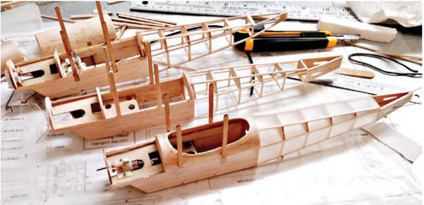
Tom's assorted fuselages using differing motor units, radio positioning and laminating film covering. Note that Top opted for upper decking hatches on his models.
