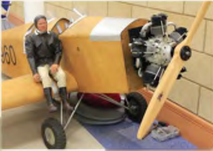
John Greenfield's 6.5 metre span Klemm 25. Built to 1/2 scale, and powered by a Valach 420cc radial.
