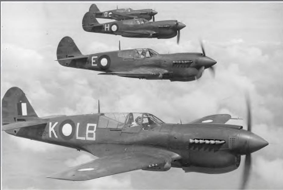
No.84 Sqdn RAAF Kittyhawks in formation over the Torres Strait island archipelago, right at the extreme northern tip of the eastern side of the Great Australian Bight. Machine in foreground is a Mk.IV, others Mk.III's. As with all RAF/Commonwealth aircraft in the Pacific combat theatre, the red centres of the roundels are omitted to avoid confusion with Japanese 'meat ball' insignia.
