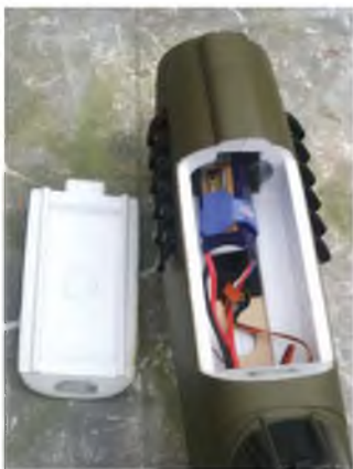
The top hatch gives access to the battery pack - note the pack is angled to get it fully forward.
