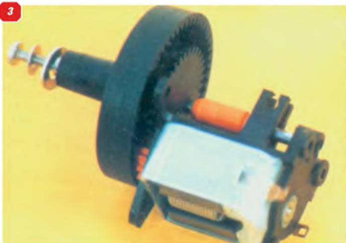
1: The original Mk.1 unit. 2: Mk.2 CRP system with modified KP-01 and KP-02 gears ready for assembly. 3: The Mk.2 unit in fully assembled state. 4: The Mk.2 unit with six prop blades and spinner in place.
