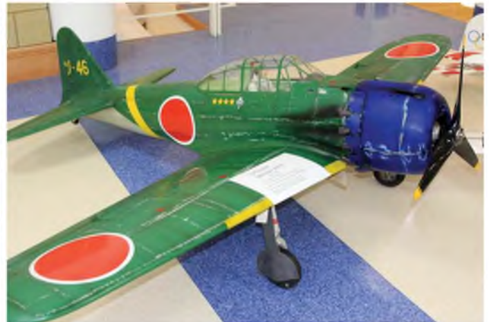
Fine 108" span Meister Zero, fitted with a Moki 150cc radial. Built by David Brown, with scale detailing by Dave Clarke.
