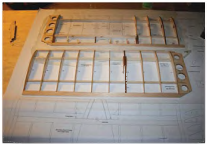
One top wing panel ready for trimming and sanding and a lower panel under construction. Just ensure you end up with a pair of each.
