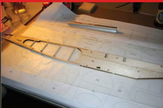
A basic fuselage side under construction. Note the c/s strut slots and the exit hole for the aileron servo lead.
