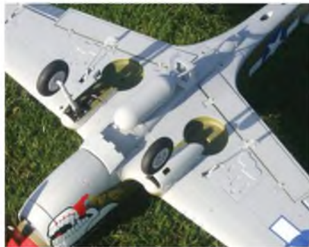
Underside view showing the cooling air exit points - rear of the cowl and two holes in the rear fuselage belly. Note also the flap linkages.
