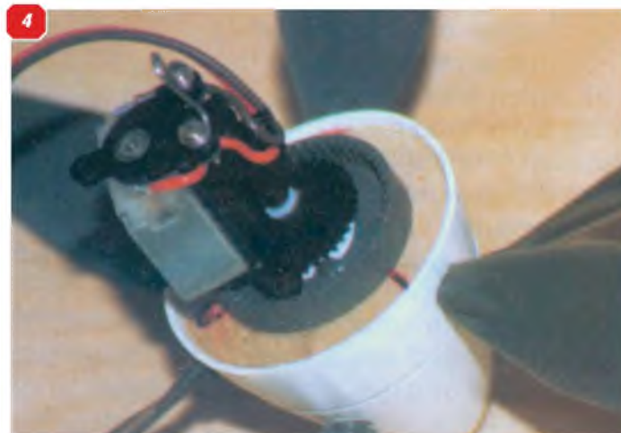
1: The original Mk.1 unit. 2: Mk.2 CRP system with modified KP-01 and KP-02 gears ready for assembly. 3: The Mk.2 unit in fully assembled state. 4: The Mk.2 unit with six prop blades and spinner in place.
