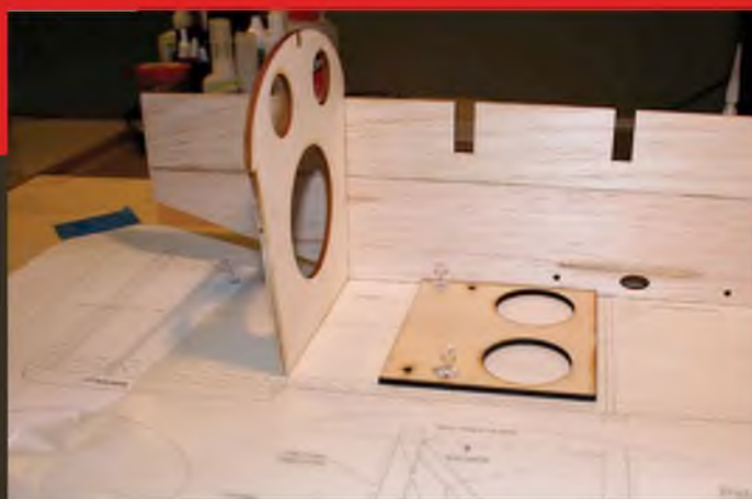
Working over the plan Alby uses the flat bottom of the former to assist with getting the u/c plate at the correct angle to the sloping fuselage side.
