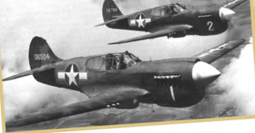
A flight of P-40E and Fs.. The one in the foreground is a P-40E, showing the fin leading edge extension, while the other two are Packhard Merlin powered P-40Fs as identified by the lack of air scoop on top of the nose.
