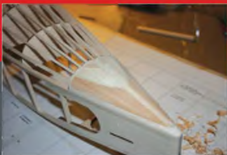
Note the packing pieces used to support the tail blocks during shaping and sanding.
