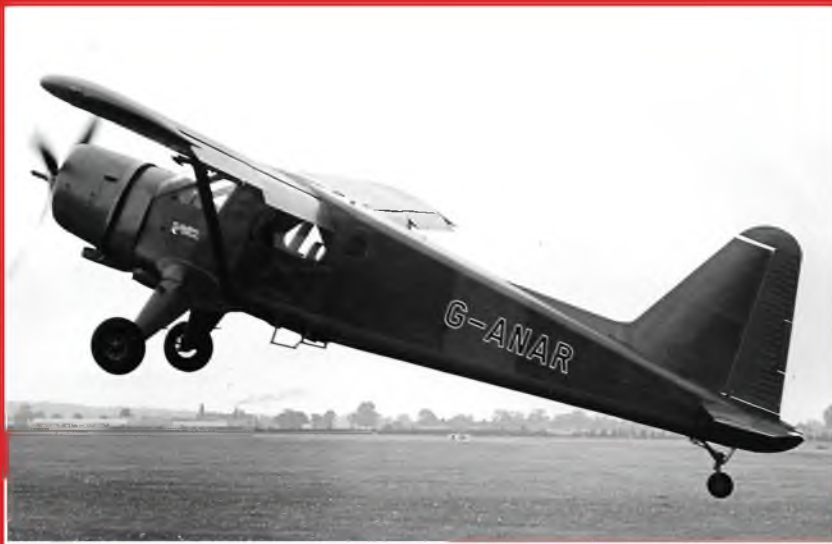
ABOVE & BELOW: These two views of the Beaver 2 G-ANAR, formerly CF-GQE, show it being put through its paces in 1953. Fitted with the more powerful 550 hp Alvis Leonides 502/4 engine the Mk 2 also featured main planes of slightly increased length and revised tail surfaces, including deletion of the curved fillet forward of the fin. G-ANAR was temporarily serialled XH463 and evaluated by the RAF in 1954. Four years later it was trialled by the Army as XN142 before returning to Canada to become CF-CNR.
