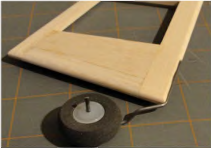
How the tail wheel leg is bent around the wheel and fits into the rudder to provide steering on the ground.
