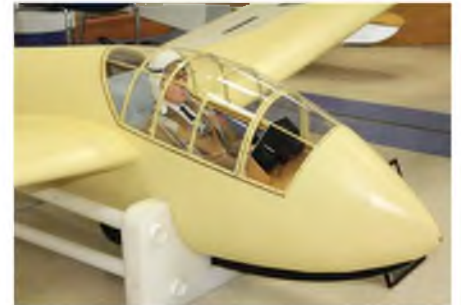
Ghost Squadron (John Greenfield design) Oriik glider built by Darren Maple. 7.5 metre span, weighs 29 kg.
