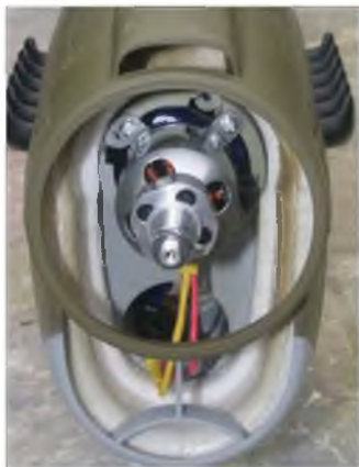
View of the motor installation before the spinner and prop are fitted.
