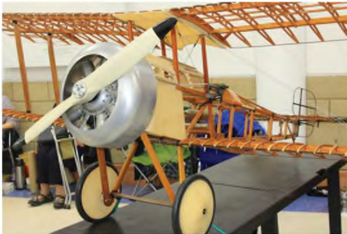
Outstanding scratch-built 1/3rd scale / 98" span Bristol Scout Type D by Andy Craddock. 3W 75 petrol power.
