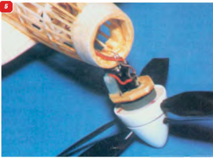
5: Mk.2 unit, showing the fuselage nose of the West Wings Spitfire Mk.22 into which it plugs. 6: Detail of the battery, mounted in the rear wing bay. Note the charging socket and on/off switch. 7: Mk.3 CRP unit, using Scientext ST-2 motor. 8: Mk.3 unit extracted from the Spitfire nose.
