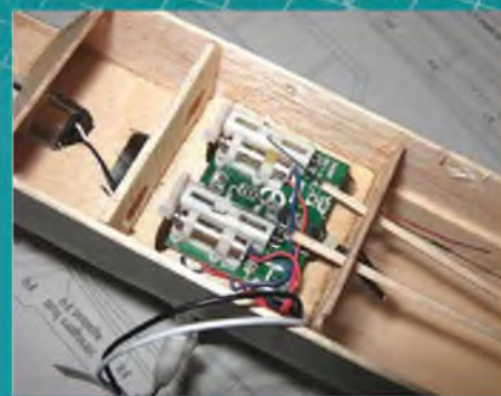
Larry's very 'old school' pushrods and the easy to access receiver brick. What ever you do, keep glue and grit away from those servo gears.
