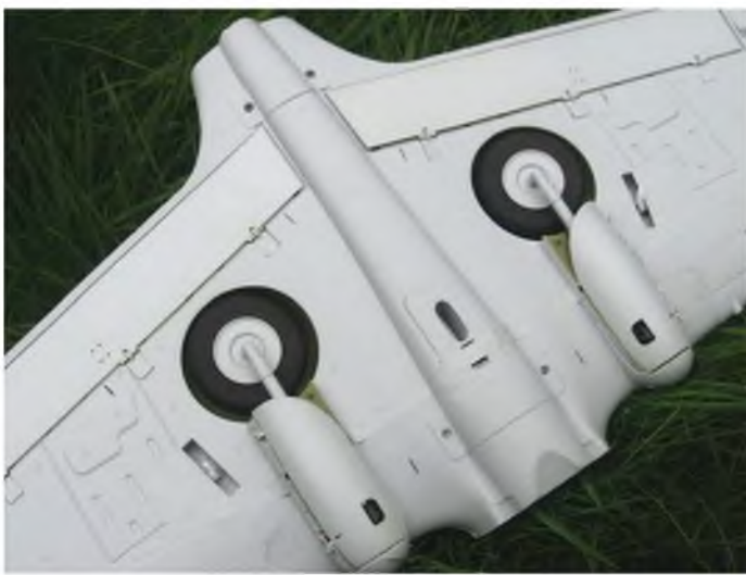
The factory fitted electric retracting UC is a good fit in the wheel wells - note the hinged doors covering the oleo legs.
