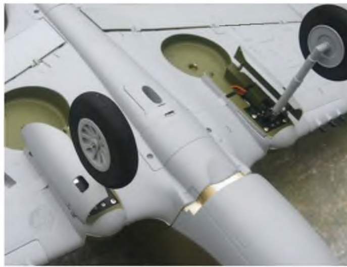
The wheels down showing more detail of the uc installation.
