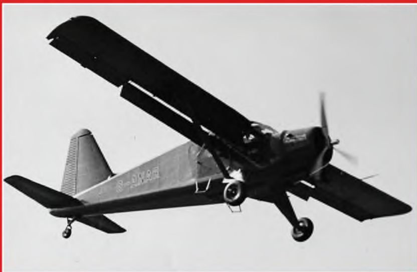
ABOVE & BELOW: These two views of the Beaver 2 G-ANAR, formerly CF-GQE, show it being put through its paces in 1953. Fitted with the more powerful 550 hp Alvis Leonides 502/4 engine the Mk 2 also featured main planes of slightly increased length and revised tail surfaces, including deletion of the curved fillet forward of the fin. G-ANAR was temporarily serialled XH463 and evaluated by the RAF in 1954. Four years later it was trialled by the Army as XN142 before returning to Canada to become CF-CNR.
