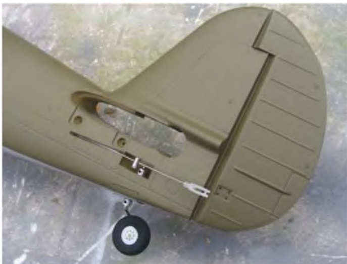
Detail of the fin/rudder and the steering tailwheel linkage.
