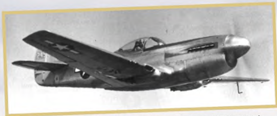
LAST OF THE LINE. One of the three P-40Q prototypes with bubble cockpit canopy and cut-down rear fuselage. Originally, a rounded wing tip shape was applied as with previous versions, but later, like this one, the tip shape was changed to a Mustang-like square-cut. Although offering a better performance than any previous P-40, it really did only what other in-service USAAC fighters were already doing.
