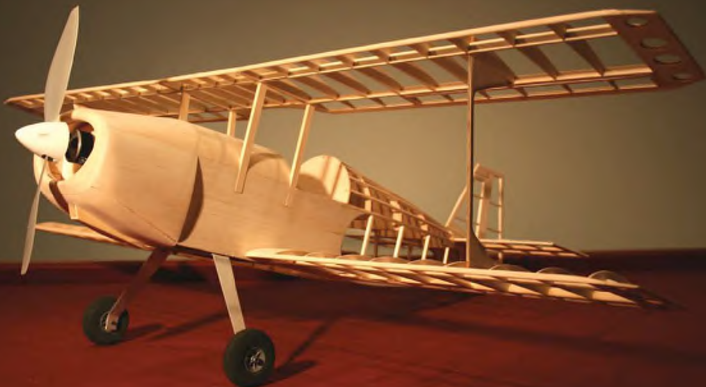
The obligatory naked model shot reveals the simple construction that results in a very attractive model.
