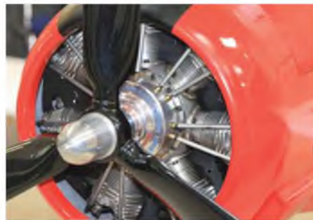
Evolution 260cc four stroke power in Harold Dowbekin's new North American T-28 Trojan.
