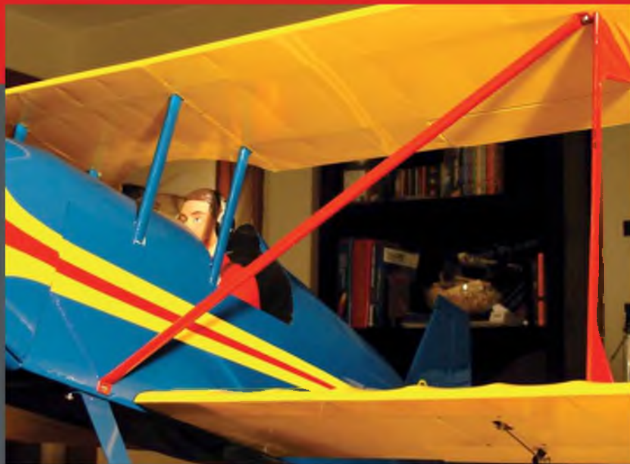
How that diagonal strut goes. In this case screwed in place streamline tubing.
