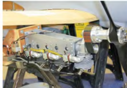
186 cc petrol engine, with 2:1 reduction drive destined for David Brown's 1/3rd scale Spitfire from Rob Elliss kit.
