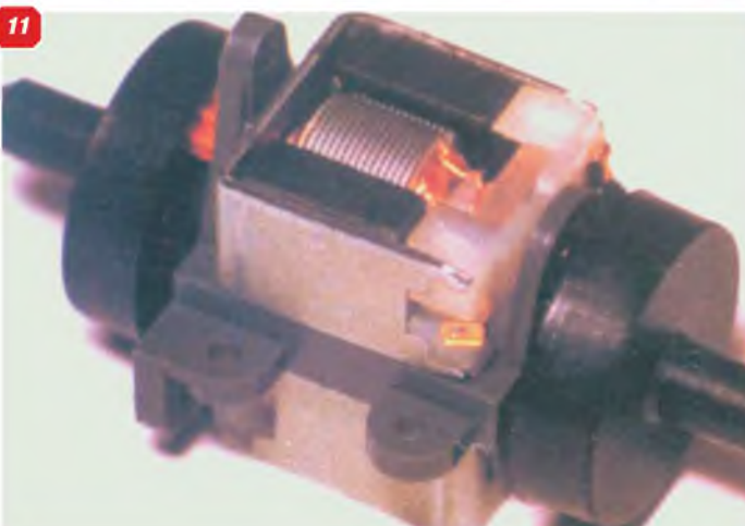
9: Contra-rotating unit set up for rubber power and shown in Fig.1b. 10: Components of Derek Knight's CRP unit for two KP-01 motors. 11: Derek Knight's twin-motor CRP assembled motor and drive mechanism. 12: Derek's completely assembled twin KP-01 unit with trial propellers mounted.
