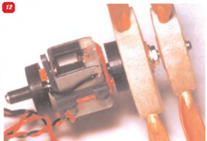
9: Contra-rotating unit set up for rubber power and shown in Fig.1b. 10: Components of Derek Knight's CRP unit for two KP-01 motors. 11: Derek Knight's twin-motor CRP assembled motor and drive mechanism. 12: Derek's completely assembled twin KP-01 unit with trial propellers mounted.
