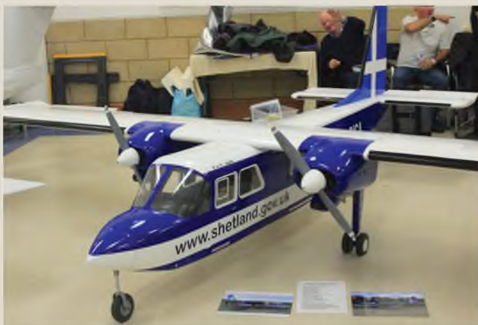
Richie Robinson's immaculate 28% scale Britten-Norman BN2B-20 Islander. 14 feet in span, weighs 88 lbs, 2 x 3W 60cc petrol power.
