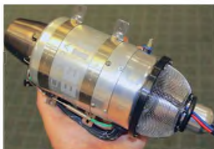
Jet Central Bee II KS gas turbine on the www.turbinesolutions.co.uk stand. 7 kgs of thrust, weighs less than two pounds!
