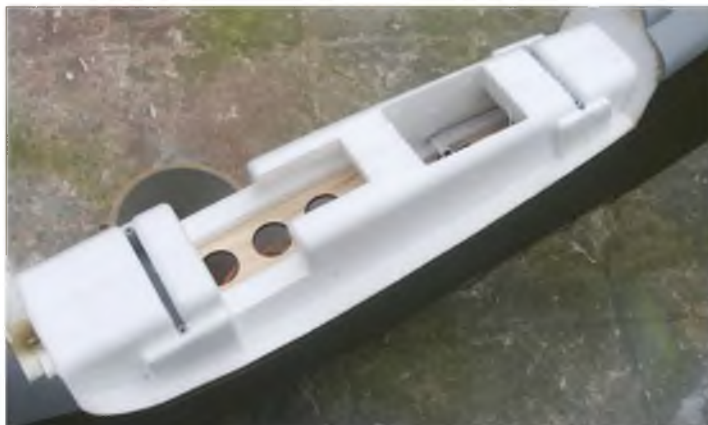
The moulded wing seat is very substantial and a very good fit with the wing.
