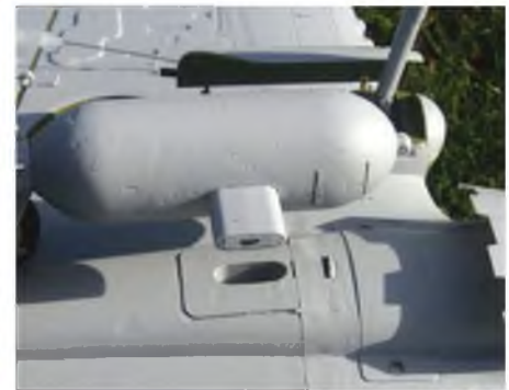
The clever bomb release - the black mark on the end of the bomb pylon indicates the magnet which holds it in place.
