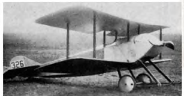
An early example of a military version of the Tabloid, with wing warping for lateral control.
