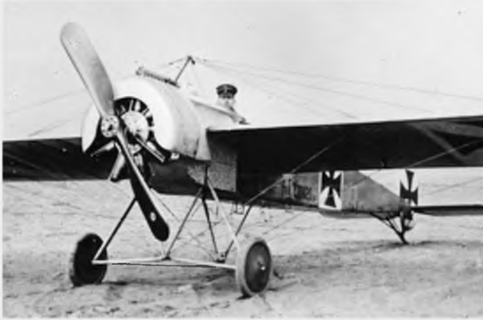
Leutenant Diemer poses in the cockpit of his Fokker E.III 420/15. Some of the undercarriage is usefully revealed here.
