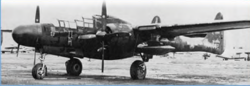
A P-61B equipped with underwing fuel tanks, seen at Clark Field, Philippines in August 1945.
