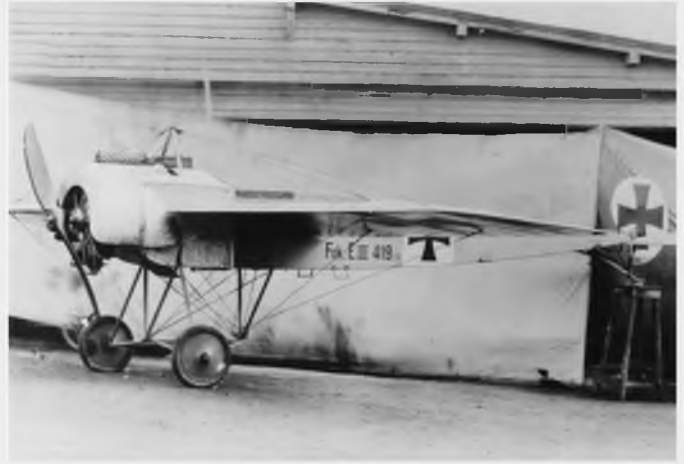
A brand new Fokker E.III. The undercarriage struts are also visible here, together with the V-strut anchor for the wing warping mechanism.
