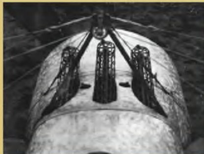
Viewed from the cockpit of the E.IV seen at left shows, much better, the three-gun installation.
