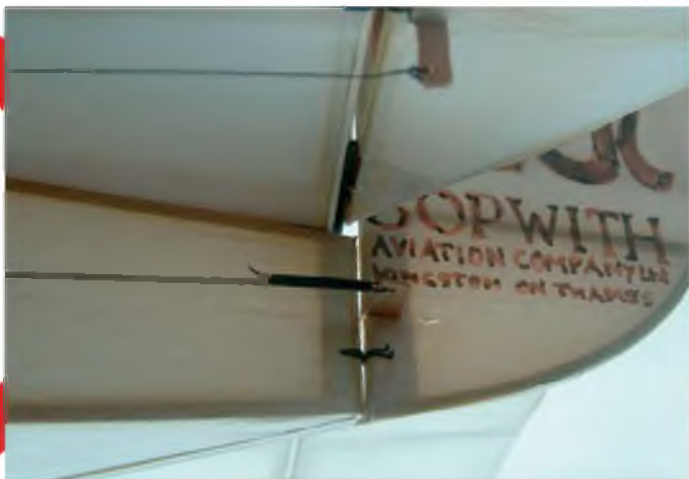
Assembly is straightforward and I used thread for a closed-loop control system - so much more elegant than pushrods. The Sopwith trademark is just drawn on using a pen. Now, I would use Lazertran transfers generated in Microsoft Word to get a much sharper result, or even print direct onto the Lifespan before covering.
