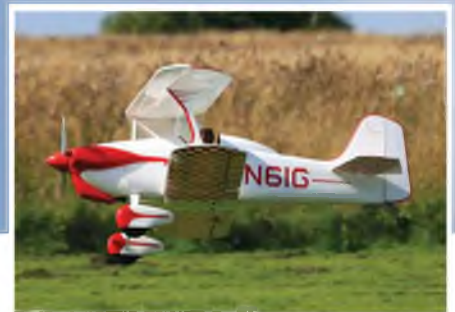
Colin Terry's Little Toot from the famous Dennis Tapsfield plan. 1/4 scale and Laser 120 powered. 57" span/ weighs 10.5 lbs.
