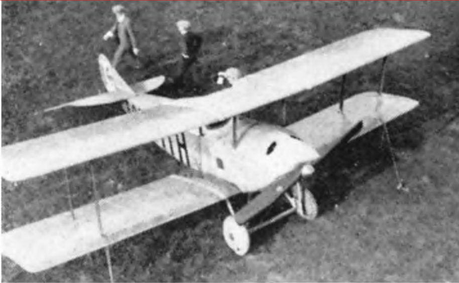
An civilian example of the Tabloid used for air racing, and featuring V-strut undercarriage. Note the air intakes in the upper engine cowl.
