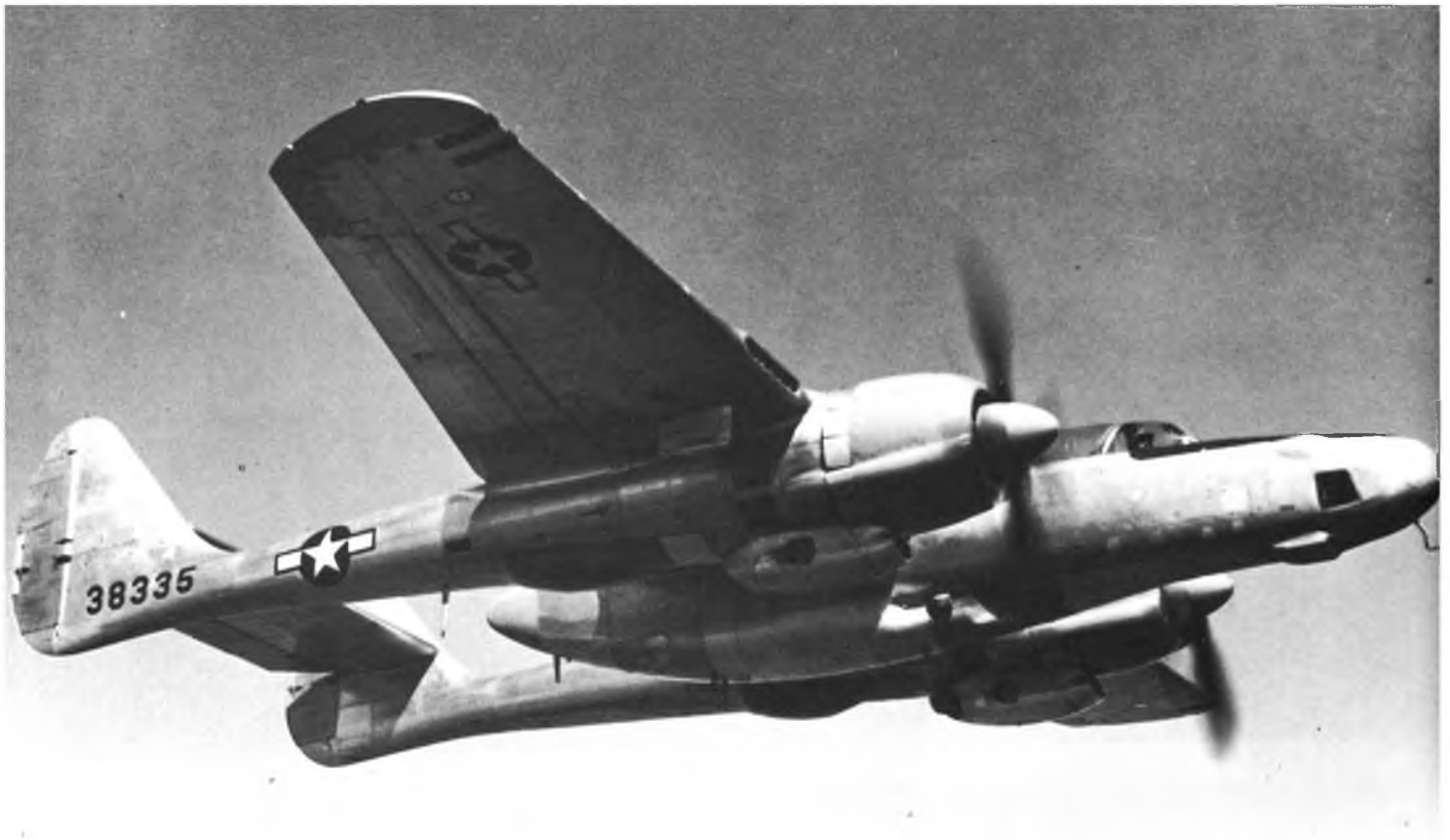
The prototype XP-61E airframe became the basis for the F-15 Reporter aircraft re-engineered for the task of photographic reconnaissance. This is the prototype XF-15A.
