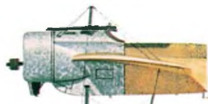
E I armed with synchronised Parabellum gun.
