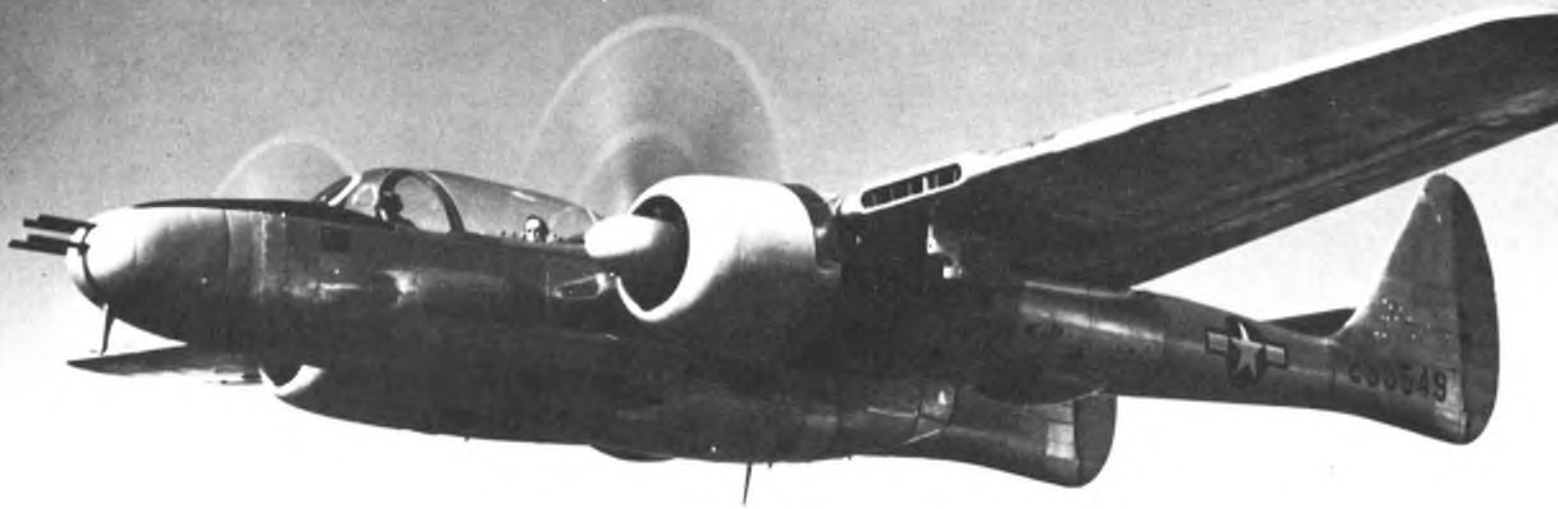
The XP-61E was the final version of the P-61 line, intended as a heavily armed long-range day escort fighter to shepherd aircraft of the Boeing B-29 force in their aerial assault on the Japanese home islands. All the guns were concentrated in the forward fuselage and the aircraft had a crew of only two. It never went beyond the prototype stage.
