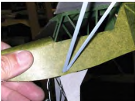
The struts are only cosmetic on the 'as designed' model and simply glued in place. See text if you have any doubts about the strength of your spars.
