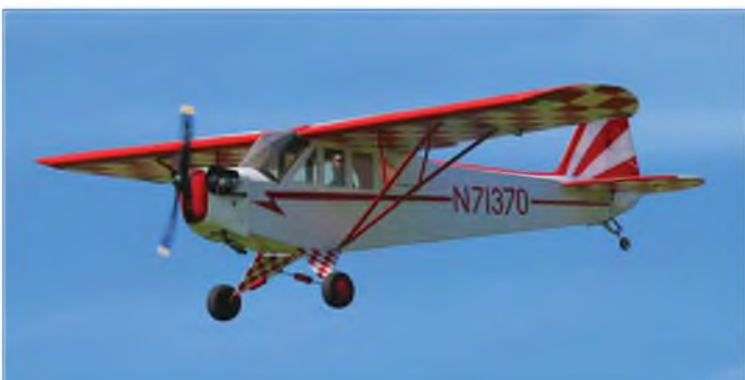
Andy Bowman's 84" span clipped wing Cub from the World Models kit. OS 120 FS powered and covered in Sig Koverall. Rib tapes cut with mini pinking shears.
