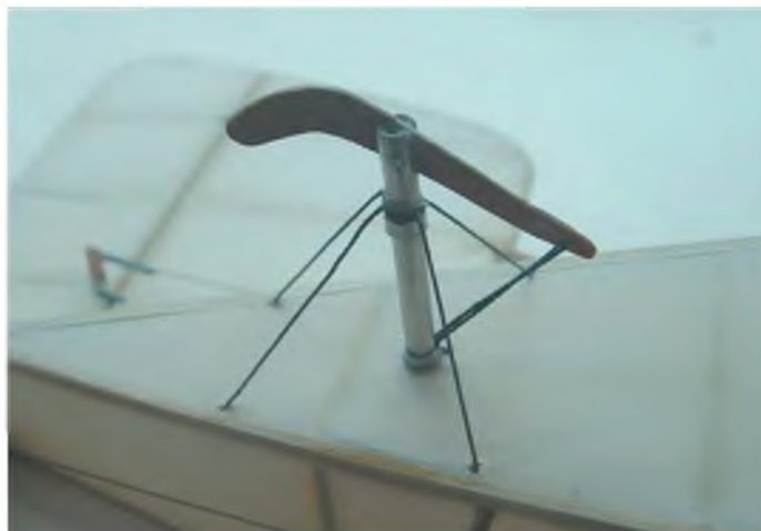
The tailskid is so distinctive that it needs a bit of care. Alloy tube, ply, thread and shirring elastic are all that is needed (but it does look a bit furry close up!).
