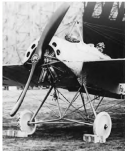
The cut-outs in the front of the engine cowl immediately identify this machine as an example of the later Fokker E.IV.
