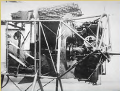
The bare bones of the prototype E.IV, showing the installation of the 14 cylinder double-row Oberursel engine and the experimental three-gun armament installation.
