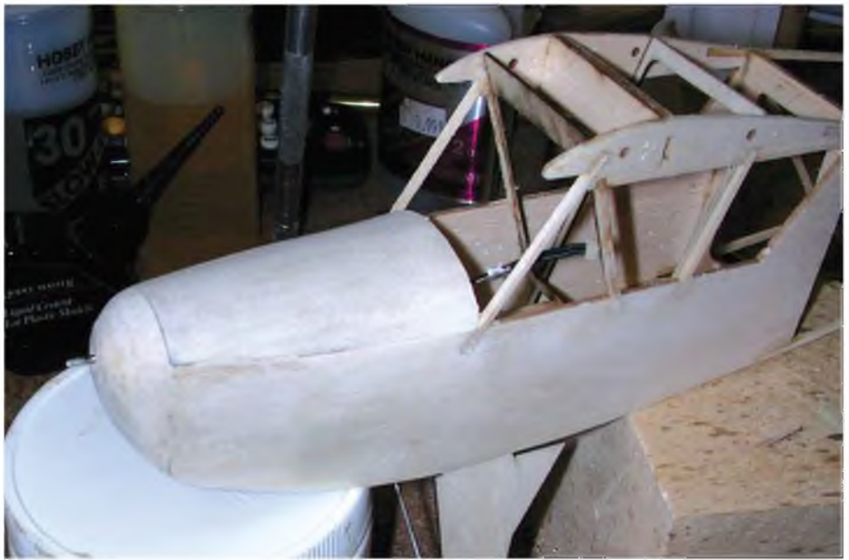
With the nose block and forward decking in place the model starts to resemble an Aeronca.
