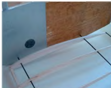
The carbon fibre wing spars just slide into holes drilled in the extended cabane struts. Scale rigging holds the aircraft together.
