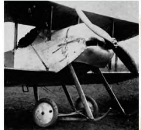
Close-up of an early military Tabloid, showing the undercarriage 'horns' to help prevent nose-overs.
