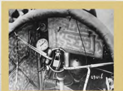
A clear view of the sparse cockpit interior of an E.III reveals the absolute minimum of instrumentation. What looks like a blank instrument panel in front of the control column is a box for empty cartridge belts. The control column surmounted by a ring and twin hand grips was typical of the type carried over to other German fighter aircraft, of which the Albatros D.I and D.II were examples.
