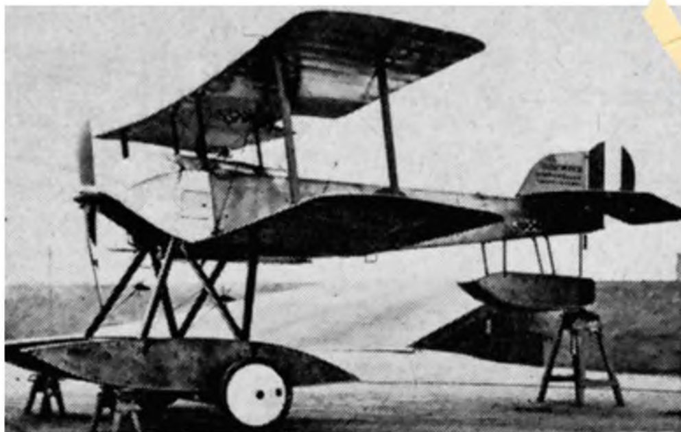
A Naval example fitted with pontoon floats front and rear. Note the increased fin area.
