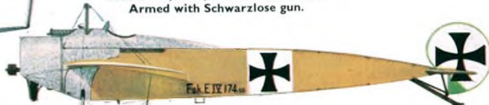
Fokker E IV, E IV 174/16. Armed with twin Spandau and streamlined cockpit decking.
