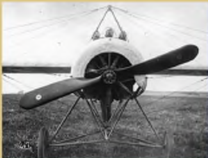
Head-on view of the prototype E.IV, werk No.298, delivered from the Fokker factory on September 27th 1915, showing the experimental three-gun armament installation. Note - no cooling frets in the cowl front at this stage.
