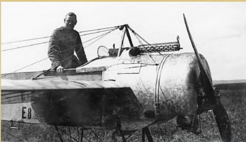
Head-on view of the prototype E.IV, werk No.298, delivered from the Fokker factory on September 27th 1915, showing the experimental three-gun armament installation. Note - no cooling frets in the cowl front at this stage.
