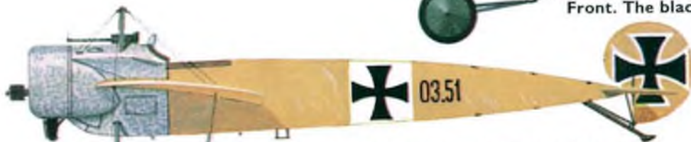
Fokker E I, E I 03.51, Austrian Air Force. Armed with synchronised Schwarzlose gun.
