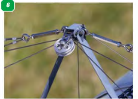
3: Pilot Helmut is nicely dressed and the cockpit is edged in leather. 4: Crisp detailing on machine gun and the king post. 5: Nicely executed riveted windscreen frame in aluminium. 6: The wing warping king post assembly is a work of art. Model comes complete with all cable terminations, turnbuckles, pulleys, cables and turnbuckles. 7: The cowl, side fairings and metal cowling on the fuselage uses aluminium. Note slots for undercarriage travel. 8: Dummy Oberursel engine expertly masks Valach 120 Petrol Twin. 9: Sheet metalwork and fastenings are executed to an astounding standard. 10: Laser cut steel fittings abound. Note engine turning on aluminium cowl.
