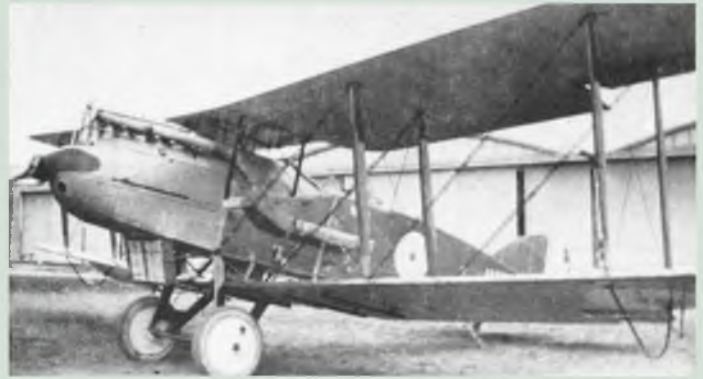
An example of the F2B with Siddeley Puma engine reveals its distinctly different nose contours.
