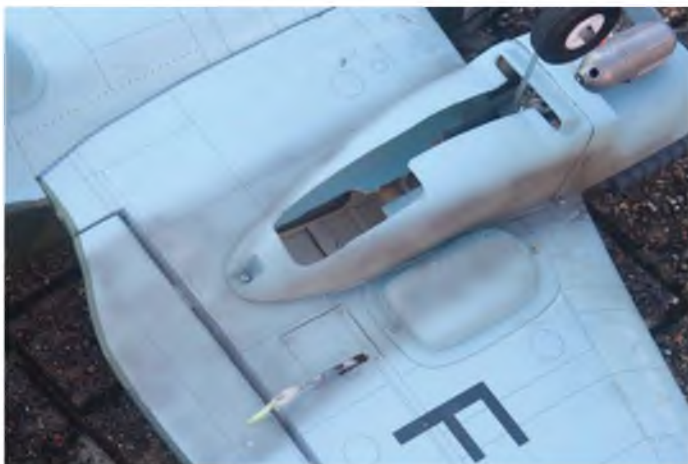
Gently airbrushed build up of exhaust 'oil' stains on and around the nacelles, greatly add to the overall effect.
