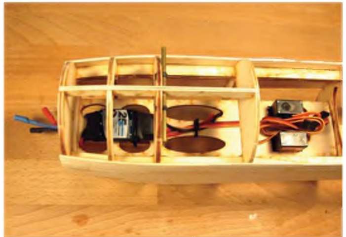
Ulrich opted to join the shells before completing the sheeting but it allows us to see much of his radio installation.
