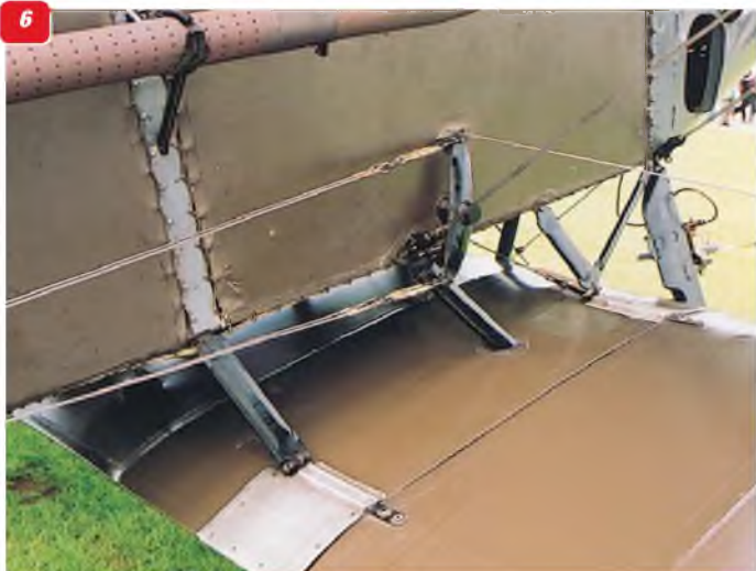
4: Nose of Shuttleworth's RR Falcon III V-12 powered F2B Mk.III showing radiator shutters. 5: Earlier style shutter arrangement on The Fighter Collection's F2B. 6: Lower wing centre section showing the anchor points to the fuselage. 7: Tail end, showing the control runs to the rudder and elevator, and the tail bracing wires. 8: Tailplane trim linkage wire connects direct to leading edge crank turnbuckle. 9: Close-up view of the double control wires to the rudder control horn and fabric panel lacing on The Fighter Collection's machine. 10: Control wires all out in the breeze are very much part of the character of the Bristol F2B. 11 & 12: Wing interplane struts showing the upper and lower wing anchor points.
