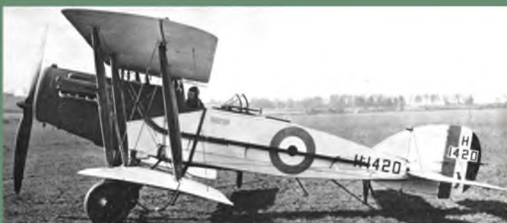
The F2B Mk.III was a post-WW1 development introduced in 1926, redesigned to take higher stress loads.
