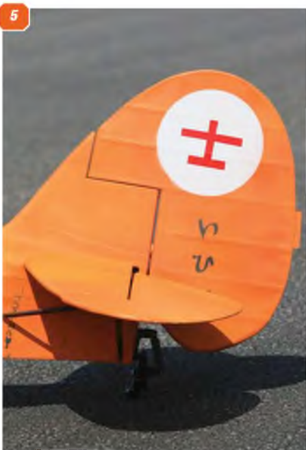
5: Aerodynamically balanced rudder areas, apparent in this view. 6: Rudder and fin use a balsa core and riblet construction. 7: Jeff built up the wheels from commercial tyres, plywood hubs, and home-moulded GRP covers. 8: The top fairing on the undercarriage is more apparent from this view. Note oil filler cap.
