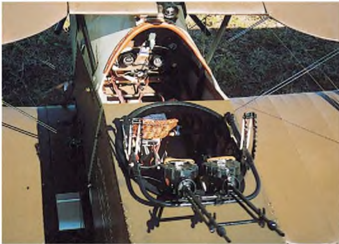
High level of cockpit detail includes the twin Lewis MG mount, pilot's wicker seat and instrument board with compass mounted in the upper centre-section. A scale 'throttle' operates the Rx on/off switch.
