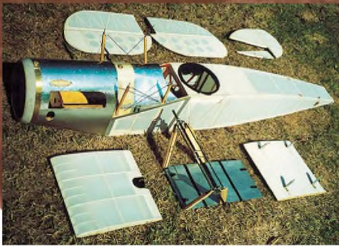
Fuselage parts completed and covered, prior to painting. Metal panel areas are covered with lithoplate aluminium sheet, epoxied over balsa sheet.
