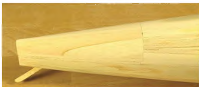
Here you can just make out the spacers used while shaping the tail fairing blocks.
