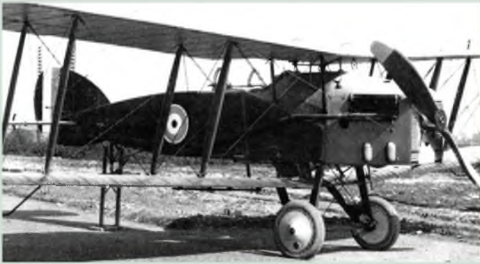
One of the early Sunbeam Arab powered F2Bs, which featured a blunt nose with radiator shutters, reminiscent of those used on the SE 5a, some of which also had Sunbeam Arab engines.
