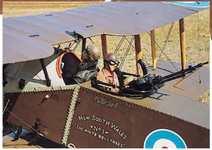
Pilot and observer figures in close-up; the fuselage fabric lacing is linen thread and uses over 1000 brads. Twin Lewis gun barrels are from old paint brush handles - their aluminium ferrules were reversed to represent the muzzles.
