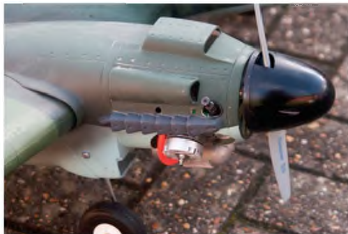
Detail of the starboard cowl before the engine change to O.S. 25 motors, showing the scale profile of the scale spinner supplied.
