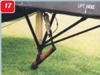
13: Elevator horn with duplicated control wires and turnbuckle adjusters. 14: Wing tip underside, showing the protective skid and the aileron horn. 15: Upper wing top surface, showing aileron control horn. 16: Close-up of the Rotherham Pump mounted on the starboard front undercarriage strut - pressurises the fuel tank. 17: The tail skid. Note bungee cord shock absorber. 18 & 19: The main undercarriage and its mounting.
