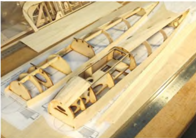
The sheeting process started with the frames still pinned to the board for support.
