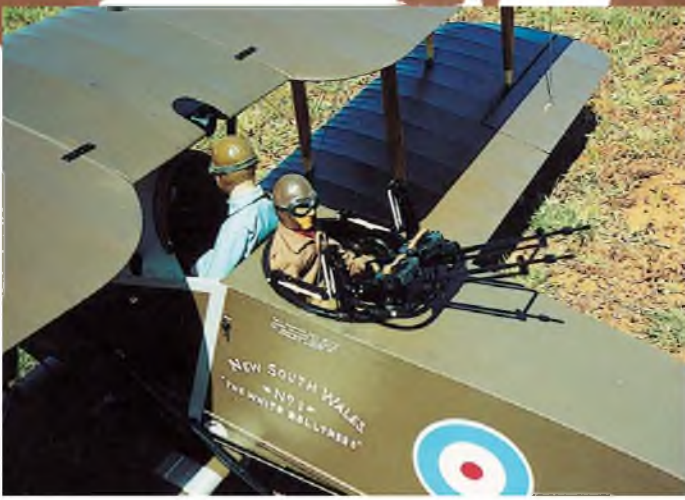
Pilot and observer figures in close-up; the fuselage fabric lacing is linen thread and uses over 1000 brads. Twin Lewis gun barrels are from old paint brush handles - their aluminium ferrules were reversed to represent the muzzles.
