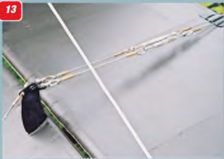
13: Elevator horn with duplicated control wires and turnbuckle adjusters. 14: Wing tip underside, showing the protective skid and the aileron horn. 15: Upper wing top surface, showing aileron control horn. 16: Close-up of the Rotherham Pump mounted on the starboard front undercarriage strut - pressurises the fuel tank. 17: The tail skid. Note bungee cord shock absorber. 18 & 19: The main undercarriage and its mounting.
