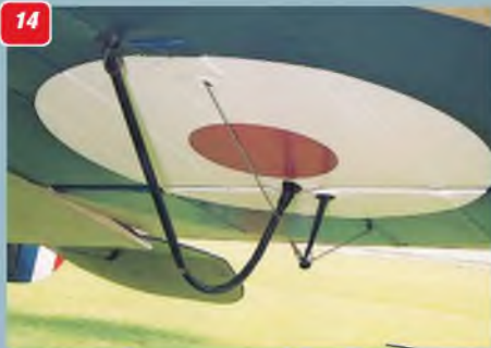
13: Elevator horn with duplicated control wires and turnbuckle adjusters. 14: Wing tip underside, showing the protective skid and the aileron horn. 15: Upper wing top surface, showing aileron control horn. 16: Close-up of the Rotherham Pump mounted on the starboard front undercarriage strut - pressurises the fuel tank. 17: The tail skid. Note bungee cord shock absorber. 18 & 19: The main undercarriage and its mounting.
