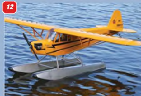
7: Stately long range patrol form David Barker's Sunderland. 8: She stoops to conquer; David Barker's Sunderland dips her starboard float. 9: Quayside maintenance! 10: Float detail on the Sunderland. Note bracing. 11: Phil Cross's 106" span electric powered Hangar 9 ARTF Cub. e-flite brushless 110 outrunner motor. 12: Phil Cross's Cub uses an e-flite brushless 110 outrunner motor.
