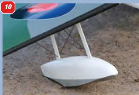
7: Stately long range patrol form David Barker's Sunderland. 8: She stoops to conquer; David Barker's Sunderland dips her starboard float. 9: Quayside maintenance! 10: Float detail on the Sunderland. Note bracing. 11: Phil Cross's 106" span electric powered Hangar 9 ARTF Cub. e-flite brushless 110 outrunner motor. 12: Phil Cross's Cub uses an e-flite brushless 110 outrunner motor.
