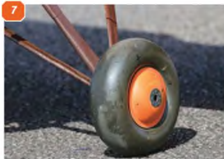
5: Aerodynamically balanced rudder areas, apparent in this view. 6: Rudder and fin use a balsa core and riblet construction. 7: Jeff built up the wheels from commercial tyres, plywood hubs, and home-moulded GRP covers. 8: The top fairing on the undercarriage is more apparent from this view. Note oil filler cap.
