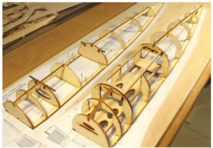
Here you see the formers in place along with the remaining keels, radio tray and hatch seat. See text about order of fitting.
