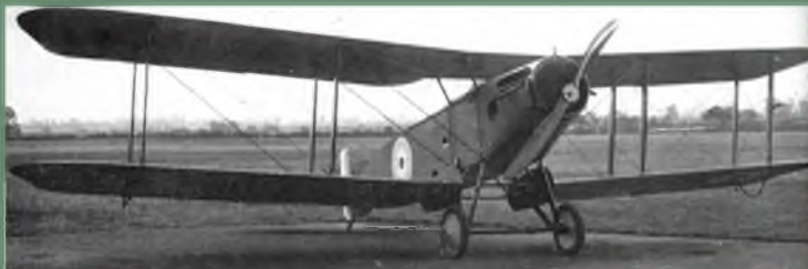
In its original form, the second prototype Bristol F2A had a 150 h.p. Hispano-Suiza engine. Note the two flank radiators mounted adjacent to the lower wing roots.
