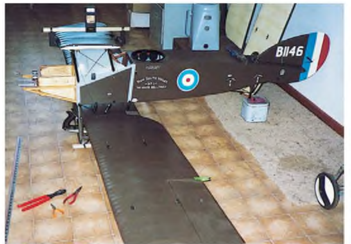
After final painting, the wings are being rigged. Note incidence meter clamped to upper centre-section, also that the nose cone is removed to access engine mounts. Engine and tail are at zero degrees, wings at one degree incidence.
