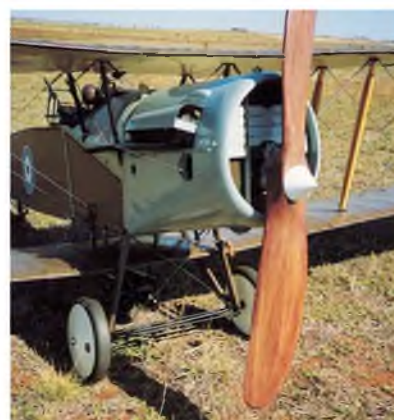
The Moki 180 30cc two-stroke is mounted on a Du-Bro mount. Exhaust via a J-Tek muffler is into a welded aluminium box and then into two scale exhaust outlets.
