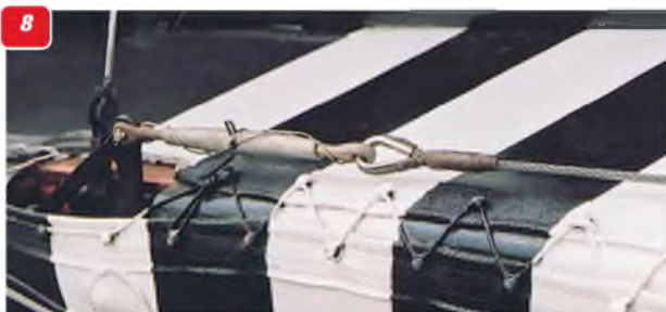
4: Nose of Shuttleworth's RR Falcon III V-12 powered F2B Mk.III showing radiator shutters. 5: Earlier style shutter arrangement on The Fighter Collection's F2B. 6: Lower wing centre section showing the anchor points to the fuselage. 7: Tail end, showing the control runs to the rudder and elevator, and the tail bracing wires. 8: Tailplane trim linkage wire connects direct to leading edge crank turnbuckle. 9: Close-up view of the double control wires to the rudder control horn and fabric panel lacing on The Fighter Collection's machine. 10: Control wires all out in the breeze are very much part of the character of the Bristol F2B. 11 & 12: Wing interplane struts showing the upper and lower wing anchor points.
