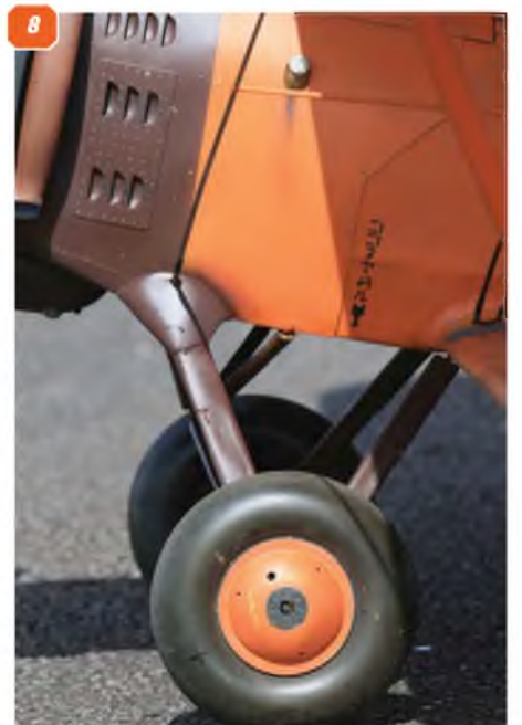
5: Aerodynamically balanced rudder areas, apparent in this view. 6: Rudder and fin use a balsa core and riblet construction. 7: Jeff built up the wheels from commercial tyres, plywood hubs, and home-moulded GRP covers. 8: The top fairing on the undercarriage is more apparent from this view. Note oil filler cap.
