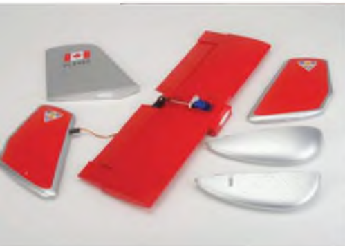
The tail end flying surfaces. One bolt holds on the tailplane; fins need gluing.
