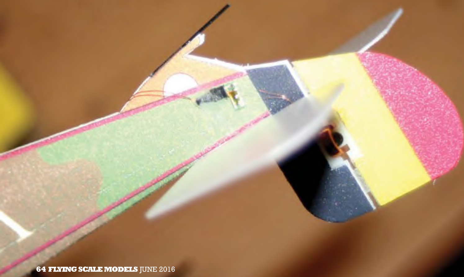
The Nano Stik hinged actuator is very good, just as long as you have that little plug you see hiding beneath the tape. Unfortunately it isn't available as a spare.
