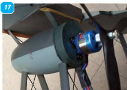
10: Plug-on wing floats; note locking wire. 11 & 12: Wheels can be fitted easily for land use. 13 - 17: The electric motor positioned on its pylon. 18: The power pod, supported by the interplane struts, viewed from the front.
