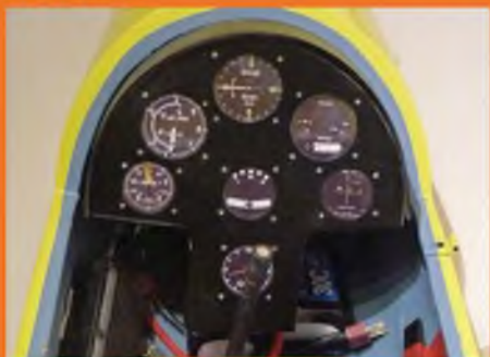
Inside the Dart's cockpit: The pilot and instrument panel are easily removable.
