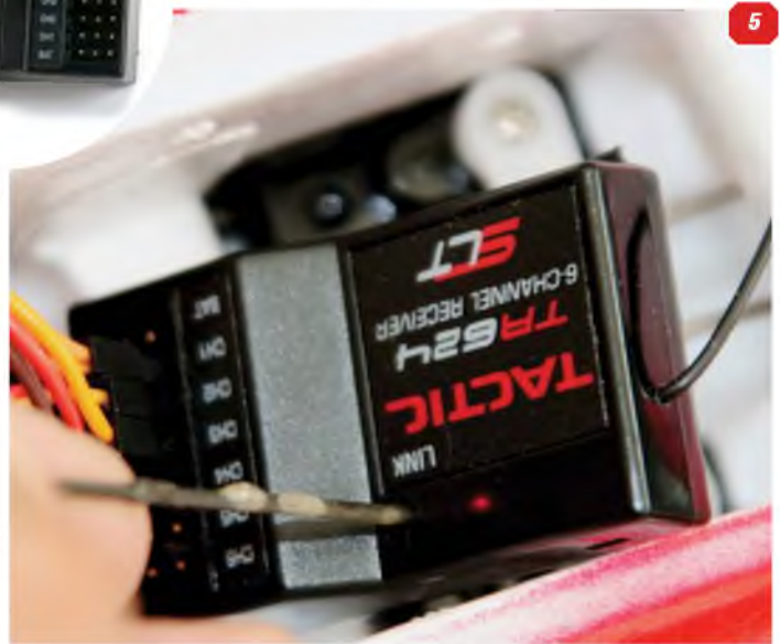
1: The 6-channel Tactic TR624 Rx used with the ANY LINK2 during testing. 2: The ANY LINK2 unit is powered by its own 1S x 450mAh lipo cell. 3: The battery can be charged using the USB charger supplied. 4: An LED on the back of ANY LINK2 confirms the brand of Tx being used (F for Futaba, in this case). 5: Binding the Tactic Rx to the Tx fitted with ANY LINK2.
