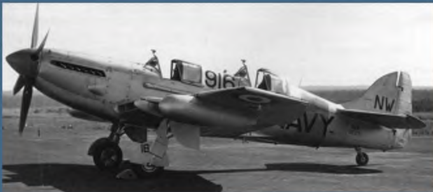
This T.Mk.5 supplied to the Royal Australian Navy was converted from FR.Mk.5 configuration and well illustrates the raised rear cockpit with semi-bubble rearward sliding canopy.
