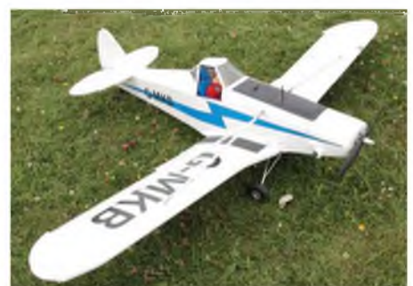
Martin Barrett's hand crafted electric Piper Pawnee. 60" span, weighs 5.5 lbs. NTM328 motor; 11x8 prop; 4 cell lipo.
