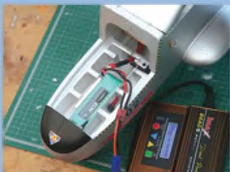
The battery bay. Even with the battery placed as far back as possible in the bay, the model was still nose heavy.
