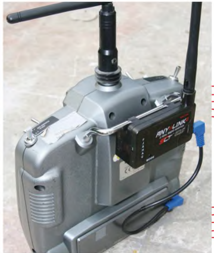
The ANY LINK 2 unit fitted to a Spectrum Tx .
