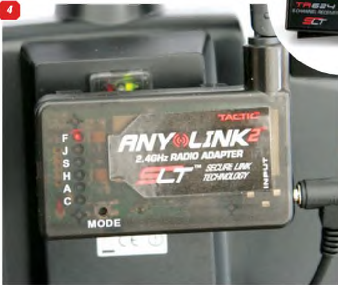
1: The 6-channel Tactic TR624 Rx used with the ANY LINK2 during testing. 2: The ANY LINK2 unit is powered by its own 1S x 450mAh lipo cell. 3: The battery can be charged using the USB charger supplied. 4: An LED on the back of ANY LINK2 confirms the brand of Tx being used (F for Futaba, in this case). 5: Binding the Tactic Rx to the Tx fitted with ANY LINK2.
