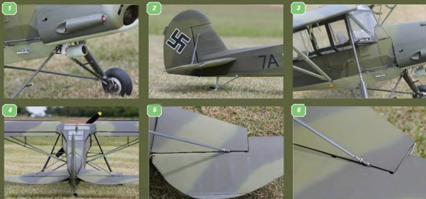
1: Front underside has much detailing. 2: The stabiliser is adjustable like the full-size example. Note tail wheel assembly. 3: Model looks like an in-service example. Beautiful detailing on fuselage. 4: Rear view show the flat slatted and flapped wing, and large elevator surfaces. 5: Shapely elevators have large area for power. Note tabs and simulated rib tapes and stitching. 6: Note strut fixing and terminations.
