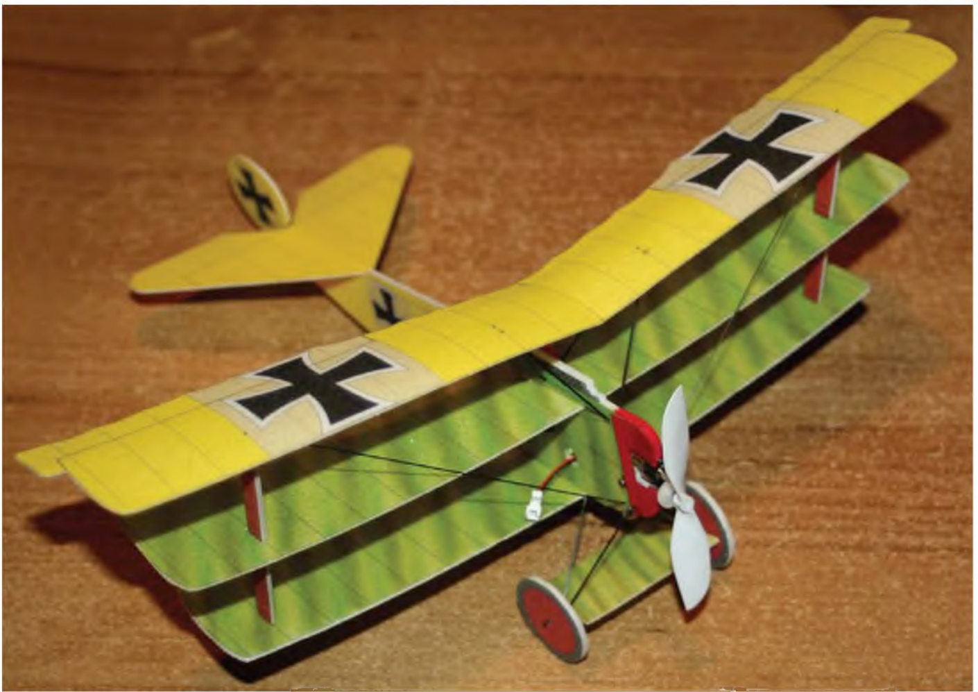
Here you see the carbon bracing that prevents the wings gaining dihedral in flight.
