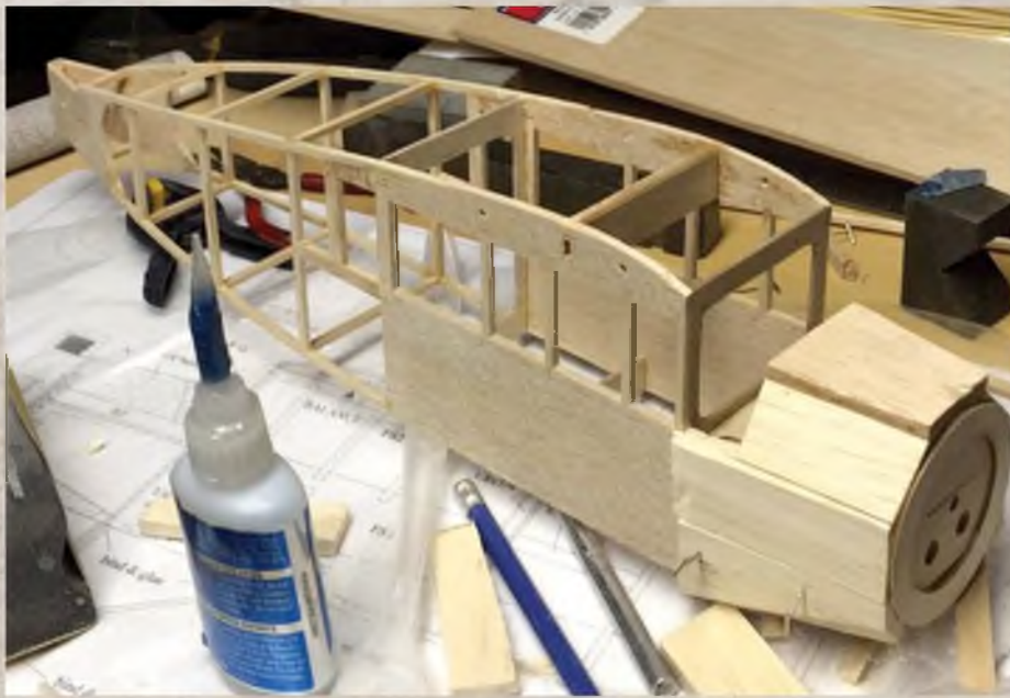
Rather than use expensive block balsa Pat made his upper nose section from thick sheet balsa, a perfectly viable option.
