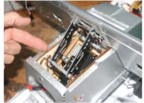
Make sure the top edge of the wing lift unit lines up with the top edge of the fuselage sides.
