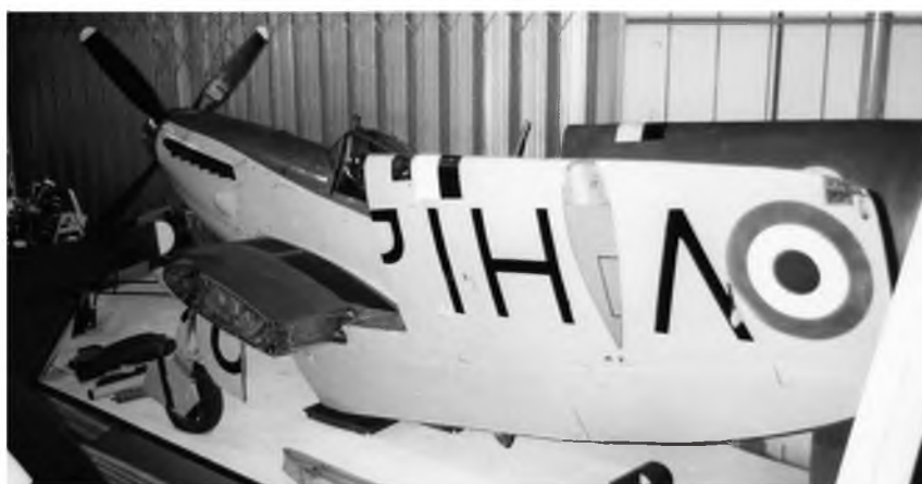
A further view of the fully folded outer wing panel on a Firefly Mk.5.
