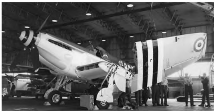
The wing-fold geometry is well illustrated in this view as its port side outer wing panel is craned into place.
