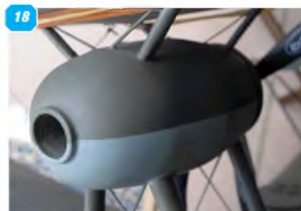
10: Plug-on wing floats; note locking wire. 11 & 12: Wheels can be fitted easily for land use. 13 - 17: The electric motor positioned on its pylon. 18: The power pod, supported by the interplane struts, viewed from the front.
