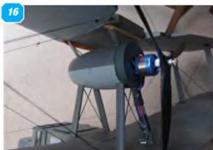
10: Plug-on wing floats; note locking wire. 11 & 12: Wheels can be fitted easily for land use. 13 - 17: The electric motor positioned on its pylon. 18: The power pod, supported by the interplane struts, viewed from the front.
