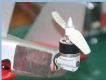
Lead taped to the end of the tail boom to achieve correct fore/aft balance.
