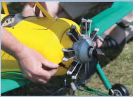
Richard Harris tweaks the needle on the PCA-2's Magnum .91 Four stroke engine. Note neat dummy engine.
