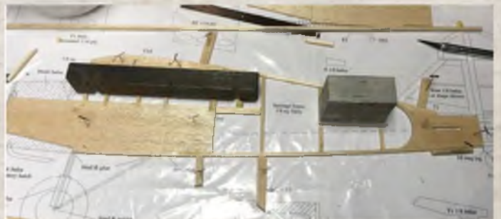
A basic fuselage side drying. Note how Pat avoids pushing pins through the strip wood.
