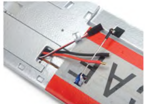
View of one of the aileron servo linkage and the motor nacelle wiring.
