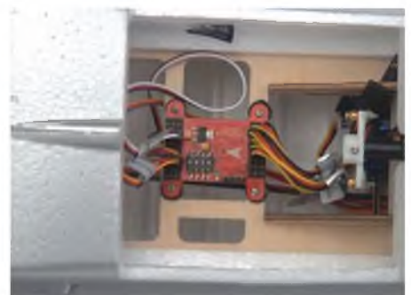
The electronic auto stability board mounted off of the wing.
