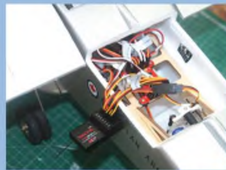
The Tactic receiver wired to the control board, before fitting into the fuselage. Note all the leads are clearly labeled.
