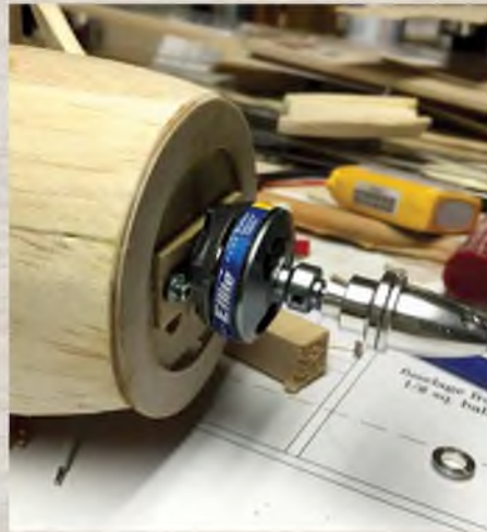
Notice the shaped wedge Pat used to set the thrust lines on his model, without obstructing the holes for the motor leads in F1.
