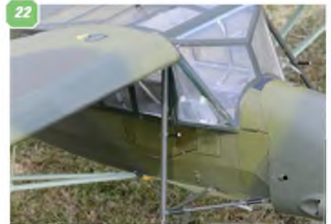
20: Derrick's Storch exudes character and has a myriad of crisp scale details. 21: No shortage of undercarriage or wing struts. 22: True scale tubular construction visible beneath the fabric skin. Note extensive detailing. 23: Wings in the folded position.
