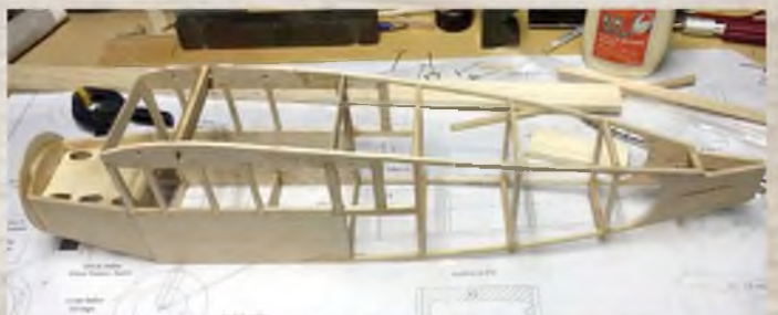
With formers in place, nose and tail pulled in and cross braces fitted it begins to resemble a fuselage.
