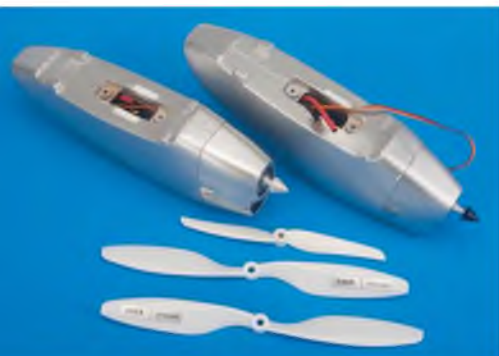
Ready-to-connect-up and bolt-on wing nacelles. Note the black painted prop nut - it's a left hand thread, not mentioned in the instructions!
