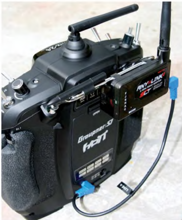
The ANY LINK 2 unit fitted to a Graupner SJ HOTT Tx (note the different lead).
