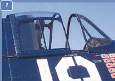
1: The full cockpit canopy. Note the rivetted frame. 2: Close-up of the sliding canopy guide rail. Note wire and pulley. 3: Further close-up, exposing the guide rail at the front. 4: It's a long way up to that cockpit, but you can see the shape of the windscreen.
