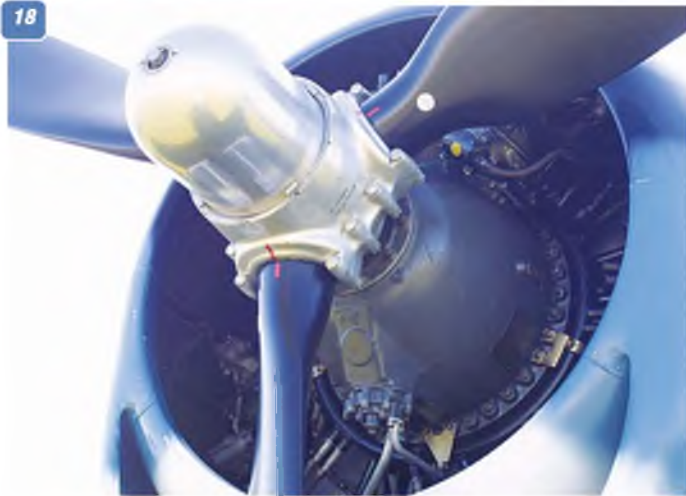
15: Exhaust pipes at the rear of the engine cowl side. 16: View of the exhaust outlet on the right hand side, viewed from the front. Left side similar. 17: Close-up of the prop. boss. An important item to replicate in a model for realism. 18: A view inside the cowl of the Pratt & Whitney R-2800 engine. 19: Air intakes in the lower engine cowl. 20: Main undercarriage Leg viewed from rear. 21: Catapult launch hook. One is positioned on each wing just outboard of the main undercarriage wheel well. 22: Main undercarriage wheel.
