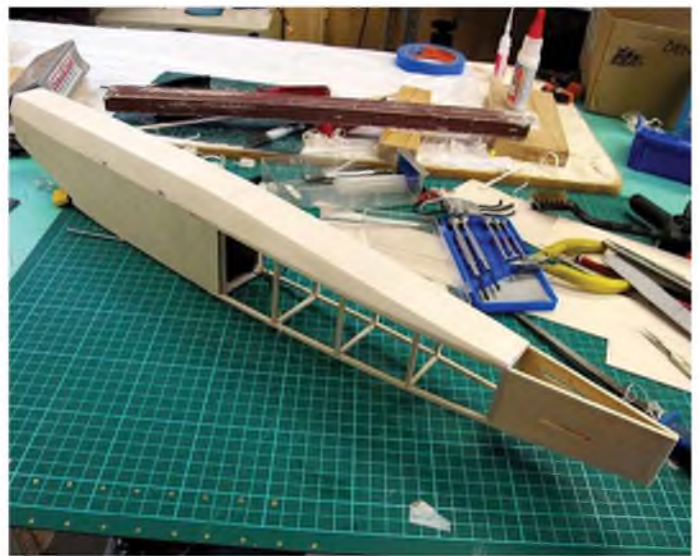
Once the balsa decking is in place the model begins to show her boxy nature.
