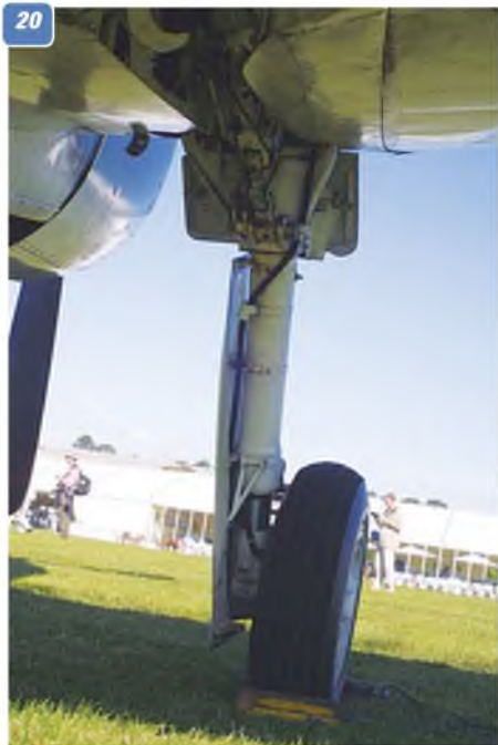
15: Exhaust pipes at the rear of the engine cowl side. 16: View of the exhaust outlet on the right hand side, viewed from the front. Left side similar. 17: Close-up of the prop. boss. An important item to replicate in a model for realism. 18: A view inside the cowl of the Pratt & Whitney R-2800 engine. 19: Air intakes in the lower engine cowl. 20: Main undercarriage Leg viewed from rear. 21: Catapult launch hook. One is positioned on each wing just outboard of the main undercarriage wheel well. 22: Main undercarriage wheel.
