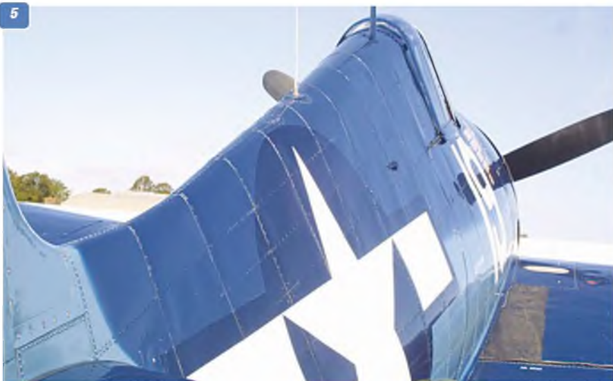
5: View of the rear upper fuselage. The rivet lines define the panels which do not have concave curves - just overlapped flat sheets wrapped around the fuselage formers. 6: The arrestor hook has been removed on this example, but the position at the extreme rear of the fuselage is clear. 7: View of the rear fuselage underside, Beneath the tailplane position.
