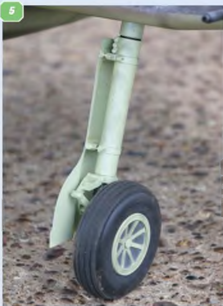
5, 6 & 7: Richard fitted Sierra Retracts. These twist 90 degrees as they retract as per the full size. Note the home made fibreglass undercarriage doors, the accurately follow the curvature of the wing underside surface skin when in the retracted position
