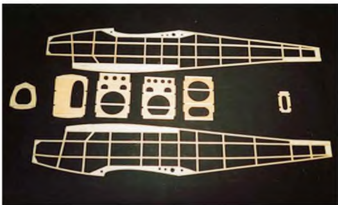
A kit of fuselage parts - really just a Keil Kraft structure, brought forward by about 50 years...
