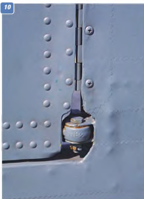
8: The complete tailcone, showing the rudder shape. 9: The rudder trim tab is hinged on the right hand skin surface. 10: Further close up of the rudder trim tab, showing the hinge. 11: Close-up of the cuff fairing over the rudder hinge line. 12: The rudder aerodynamic balance at the top of the fin/rudder assembly. 13 & 14: Two views of the fuselage front underside, just behind the engine cowl, showing the adjustable cooling channel.
