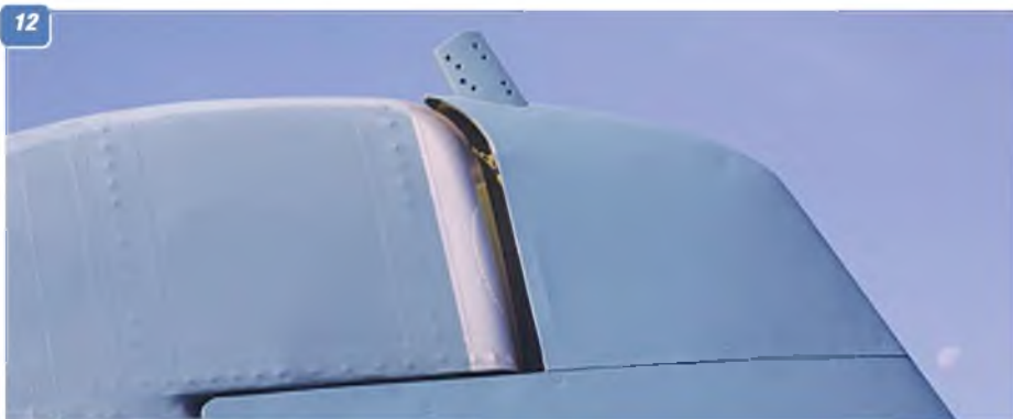
8: The complete tailcone, showing the rudder shape. 9: The rudder trim tab is hinged on the right hand skin surface. 10: Further close up of the rudder trim tab, showing the hinge. 11: Close-up of the cuff fairing over the rudder hinge line. 12: The rudder aerodynamic balance at the top of the fin/rudder assembly. 13 & 14: Two views of the fuselage front underside, just behind the engine cowl, showing the adjustable cooling channel.
