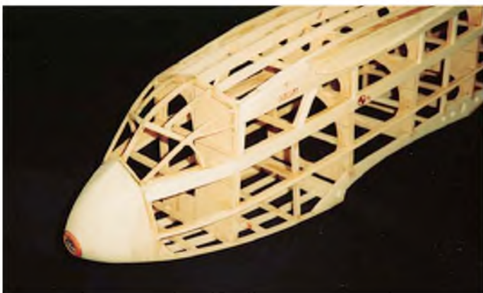
Finished fuselage with nose block and cockpit framing now in place.
