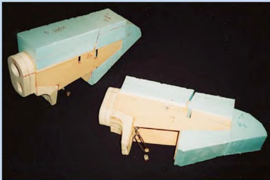
Both nacelles, now blocked and with blue foam added.
