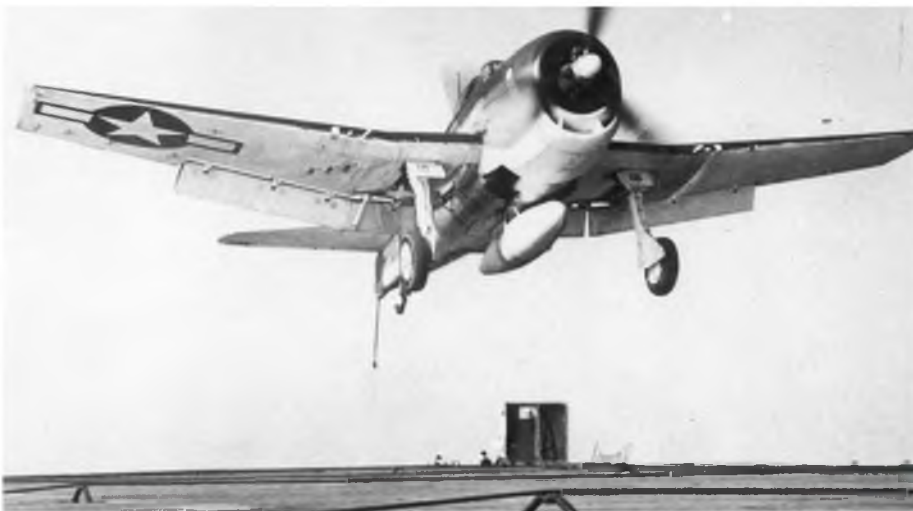
Perfect arrival! With flaps and tail hook fully deployed, this F6F-3 Hellcat passes the rear deck round-down and settles into the arrestor wires.
