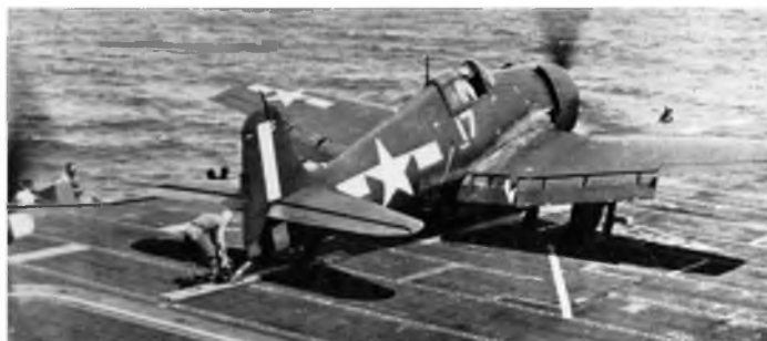
A ground crew checks the rear catapult attachment ready to launch this F6F-5 of VF-29 from the deck of U.S.S. Cabot in October 1944. All-over dark blue finish.
