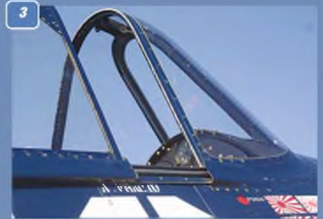
1: The full cockpit canopy. Note the rivetted frame. 2: Close-up of the sliding canopy guide rail. Note wire and pulley. 3: Further close-up, exposing the guide rail at the front. 4: It's a long way up to that cockpit, but you can see the shape of the windscreen.
