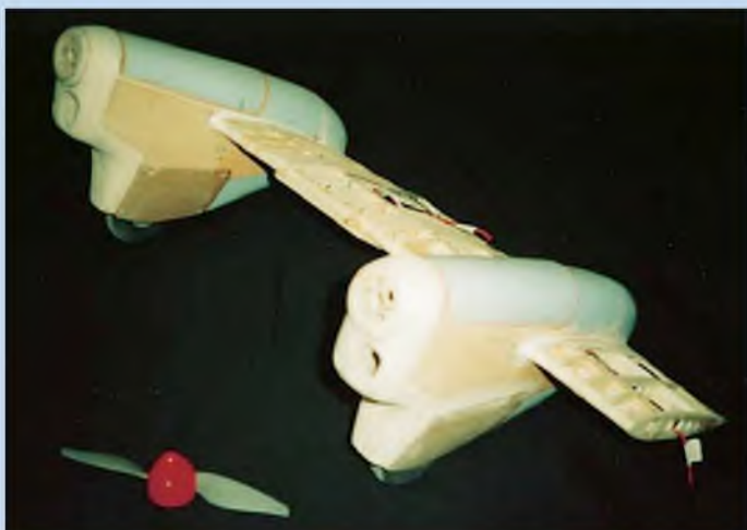
The nacelles, finally shaped and filled.
