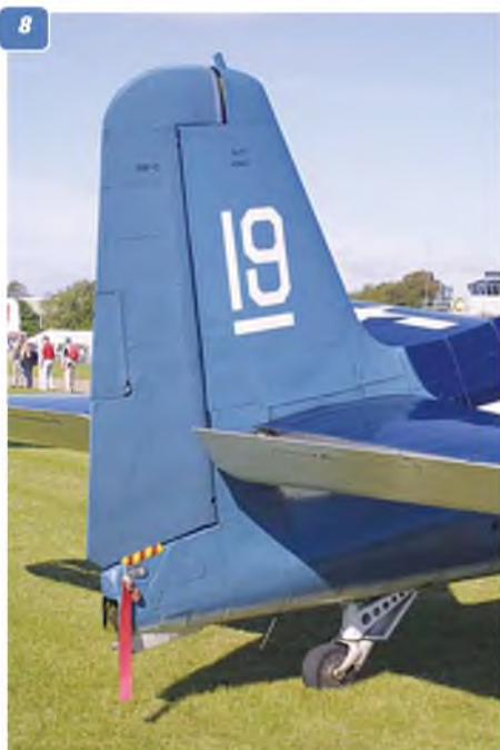
8: The complete tailcone, showing the rudder shape. 9: The rudder trim tab is hinged on the right hand skin surface. 10: Further close up of the rudder trim tab, showing the hinge. 11: Close-up of the cuff fairing over the rudder hinge line. 12: The rudder aerodynamic balance at the top of the fin/rudder assembly. 13 & 14: Two views of the fuselage front underside, just behind the engine cowl, showing the adjustable cooling channel.
