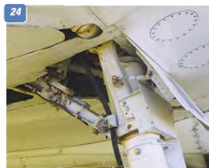
23: View of a main undercarriage leg. Wheel covers are rigidly fixed to the legs, inboard and turn with the leg during retract sequence. Front auxiliary door folds backwards. 24: Close-up of the top of the main undercarriage leg. Note the link from the leg to the front auxiliary door. 25: Bottom of the main undercarriage leg and fairing, viewed from the rear. 26: View of the main undercarriage, viewed from inboard, showing the shape of the main undercarriage fairing. 27: View of the top of the main leg, viewed from the rear.
