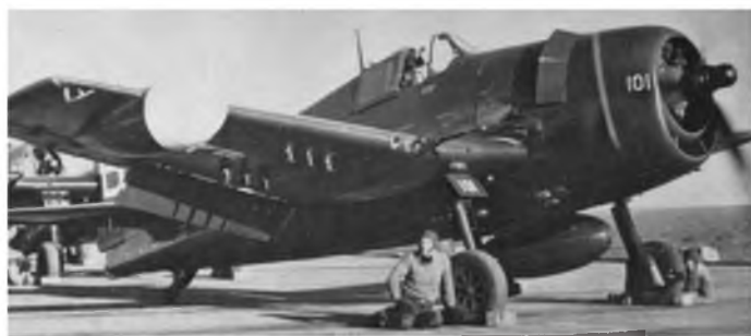
With wing leading edge radar pod prominently visible, this F6F-5N night fighter prepares to launch from U.S.S. San Jacinto in the summer of 1945. Note the two 20mm cannon also visible, in lieu of the three 0.5" machine guns as used on the night fighter variant.
