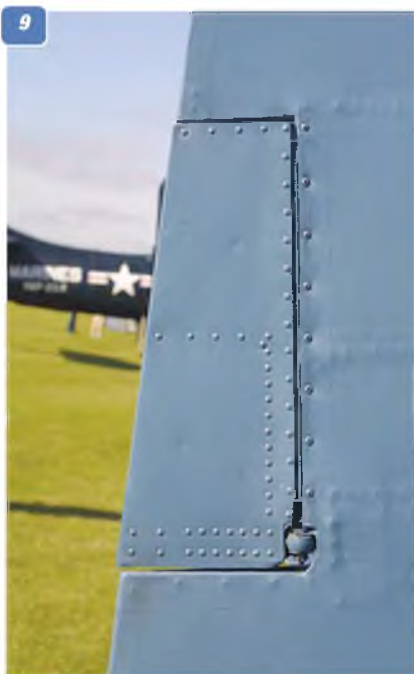
8: The complete tailcone, showing the rudder shape. 9: The rudder trim tab is hinged on the right hand skin surface. 10: Further close up of the rudder trim tab, showing the hinge. 11: Close-up of the cuff fairing over the rudder hinge line. 12: The rudder aerodynamic balance at the top of the fin/rudder assembly. 13 & 14: Two views of the fuselage front underside, just behind the engine cowl, showing the adjustable cooling channel.
