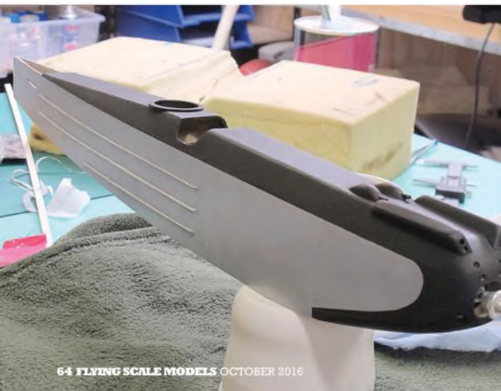
The fuselage detail in all its' glory. Stiffening ribs, gun humps and rocker covers add detail while the holes provide cooling for the motor.
