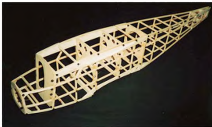
Basic fuselage box structure awaiting nose block and cockpit framing.
