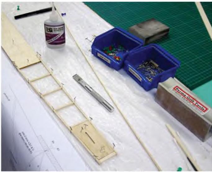
The totally traditional build begins with the usual two fuselage side frames.
