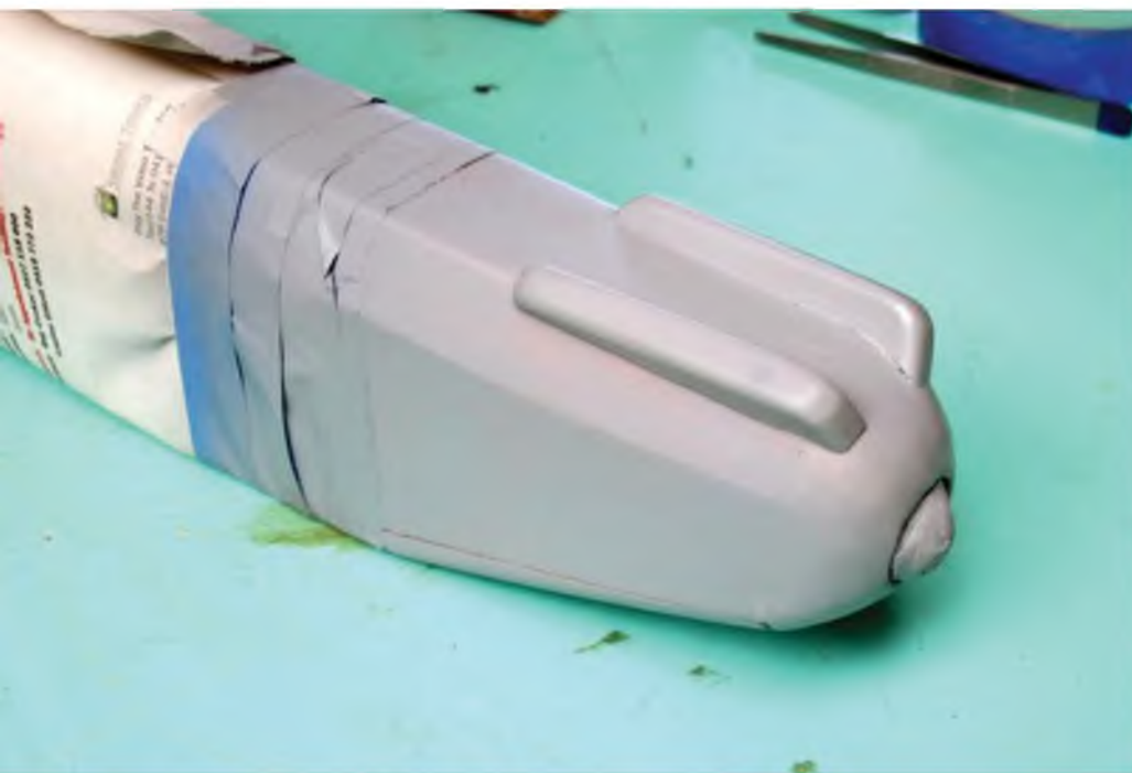
With the nose smoothed the rocker cover mouldings are fitted and the whole given an undercoat of matt grey.
