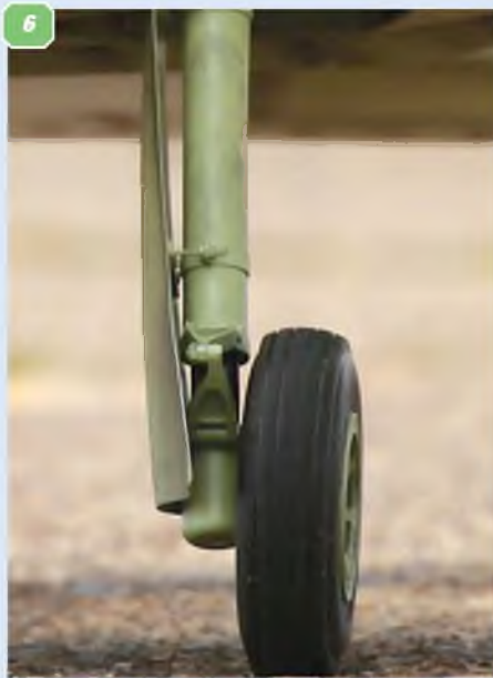
5, 6 & 7: Richard fitted Sierra Retracts. These twist 90 degrees as they retract as per the full size. Note the home made fibreglass undercarriage doors, the accurately follow the curvature of the wing underside surface skin when in the retracted position
