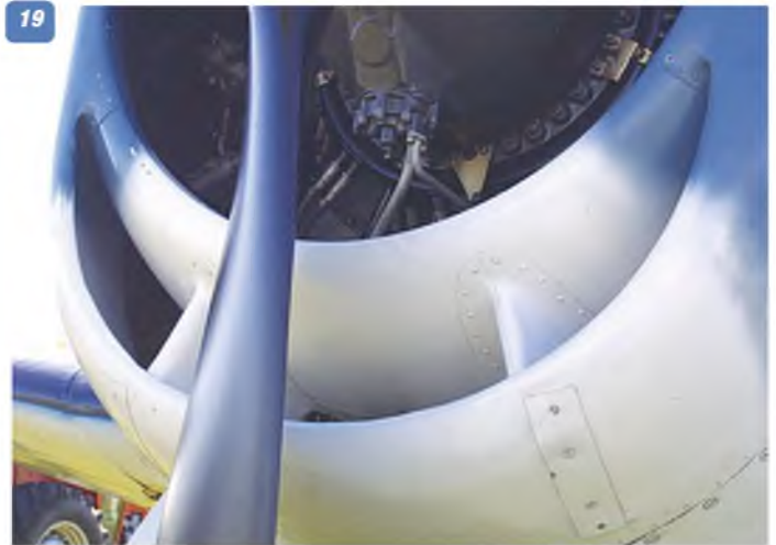
15: Exhaust pipes at the rear of the engine cowl side. 16: View of the exhaust outlet on the right hand side, viewed from the front. Left side similar. 17: Close-up of the prop. boss. An important item to replicate in a model for realism. 18: A view inside the cowl of the Pratt & Whitney R-2800 engine. 19: Air intakes in the lower engine cowl. 20: Main undercarriage Leg viewed from rear. 21: Catapult launch hook. One is positioned on each wing just outboard of the main undercarriage wheel well. 22: Main undercarriage wheel.
