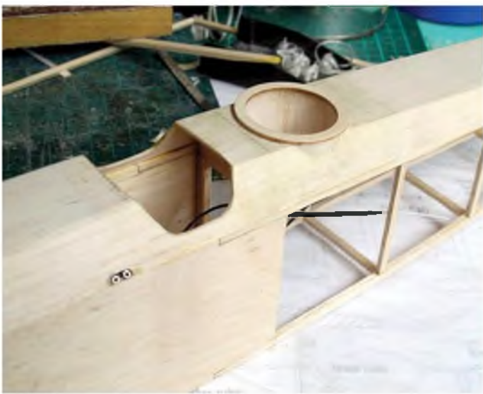
How the cockpit is cut out and the tube that forms the basis of the gunner's position is fitted.
