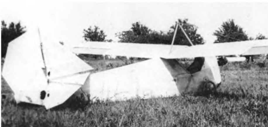
Jean A. Roche's original homebuilt aircraft, as first powered by a Henderson motorcycle engine. The shape, that led to the Aeronca C-2 and C-3 is clearly there.
