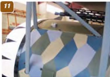
10: View of the left forward fuselage side, showing access panel, wing struts and undercarriage anchor points. 11: View of the forward fuselage looking forward toward the cowl, showing the wing struts and the fuel tank cap. 12: Detail of the foot stirrup on the left fuselage side below the cockpit. 13: Lifting handle at the bottom of the rear fuselage side. 14: View of the fuselage rear, underneath the tailplane, showing the control wire runs to the rudder and elevator control horns. Note the leather facings where the control wires exit the fuselage. The wire at the top goes through the tailplane to the top surface elevator horn. 15: The anchor points on the lower fuselage for the rear undercarriage member and a wing strut. 16: View looking forward along the fuselage, showing the general arrangement of wing struts.
