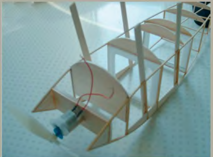
Once the formers are added, the motor dowels can be fitted and the motor taped to them to check its location is correct.
