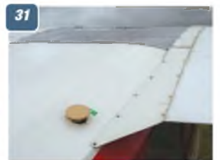
24 & 25: Aileron, port wing panel. 26: Port wing tip. 27: Wing root cuff. 28: Front fuselage, showing the cockpit windows and line of the port side cabin door. 29: Venturi for driving the cockpit instruments, Starboard side, immediately below the cockpit. 30 & 31: Radio aerial and fuel filler cap on the fuselage top deck immediately behind the cabin, also showing the shape of the shape of the wing-to-fuselage fairing..
