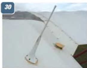
24 & 25: Aileron, port wing panel. 26: Port wing tip. 27: Wing root cuff. 28: Front fuselage, showing the cockpit windows and line of the port side cabin door. 29: Venturi for driving the cockpit instruments, Starboard side, immediately below the cockpit. 30 & 31: Radio aerial and fuel filler cap on the fuselage top deck immediately behind the cabin, also showing the shape of the shape of the wing-to-fuselage fairing..
