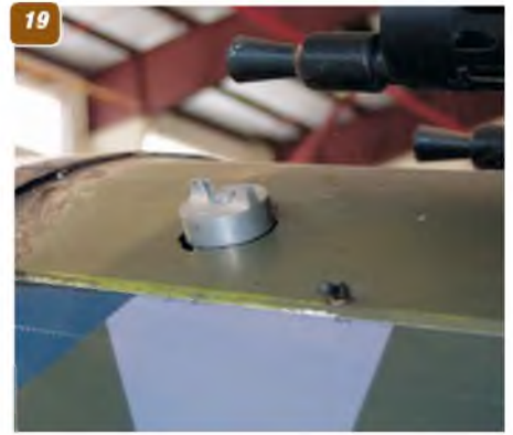
17: View, right side of fuselage, just behind the engine cowl, showing wing strut, where it enters the fuselage. 18: View of the right side of the rear fuselage, showing the control cable runs. 19: Detail of the upper fuselage behind the engine cowl, showing the fuel tank cap. 20: Rear fuselage upper decking, showing the tailplane leading edge and fin anchor point. 21: Top surface elevator horn. Note the leather reinforcement where the control wire enters the tailplane fabric. 22: Tailplane and elevator, showing the elevator aerodynamic balance.
