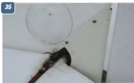
32: Close-up of the elevator trim tab, port side. 33: Tailplane anchor point of the rudder-to-tailplane brace. 34: Rear fuselage starboard side showing the rudder control horn and control wire at exit from the fuselage. Note also the disc shaped inspection panel. 35: Tailplane and elevator at the root, also showing port side inspection panel.
