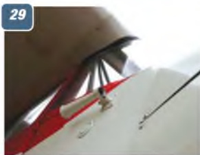
24 & 25: Aileron, port wing panel. 26: Port wing tip. 27: Wing root cuff. 28: Front fuselage, showing the cockpit windows and line of the port side cabin door. 29: Venturi for driving the cockpit instruments, Starboard side, immediately below the cockpit. 30 & 31: Radio aerial and fuel filler cap on the fuselage top deck immediately behind the cabin, also showing the shape of the shape of the wing-to-fuselage fairing..
