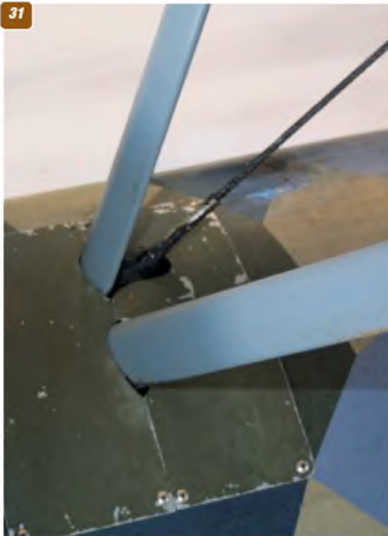
30: General view of the main undercarriage, showing the struts and the cross brace wires.
