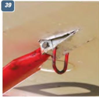
37: The unusual pitot head mounted on the mid-span wing-to-wing-strut brace, starboard side as seen in photo 38 . 39: Wing strut upper anchor point on wing underside. Note also the tie-down loop for lashing down the parked aircraft. 40: Wing strut upper rear anchor point on wing underside. 41: Wing strut lower anchor point on lower fuselage. 42: The Main undercarriage. 43 - 48: Close-up details of the main undercarriage and its mounting points.
