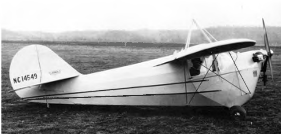
The Aeronca C-3 went through a series styling improvements that cleaned up the shape to streamline the fuselage. This is the C-3 Master, with enclosed cabin.
