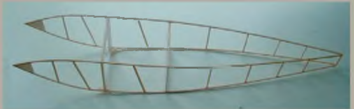
The fuselage is just a 1/16" square box. Joining at the sternpost, then adding F3 and F2 is the easiest way to get a true structure, and the longeron curve will be to scale.
