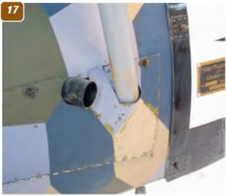
17: View, right side of fuselage, just behind the engine cowl, showing wing strut, where it enters the fuselage. 18: View of the right side of the rear fuselage, showing the control cable runs. 19: Detail of the upper fuselage behind the engine cowl, showing the fuel tank cap. 20: Rear fuselage upper decking, showing the tailplane leading edge and fin anchor point. 21: Top surface elevator horn. Note the leather reinforcement where the control wire enters the tailplane fabric. 22: Tailplane and elevator, showing the elevator aerodynamic balance.
