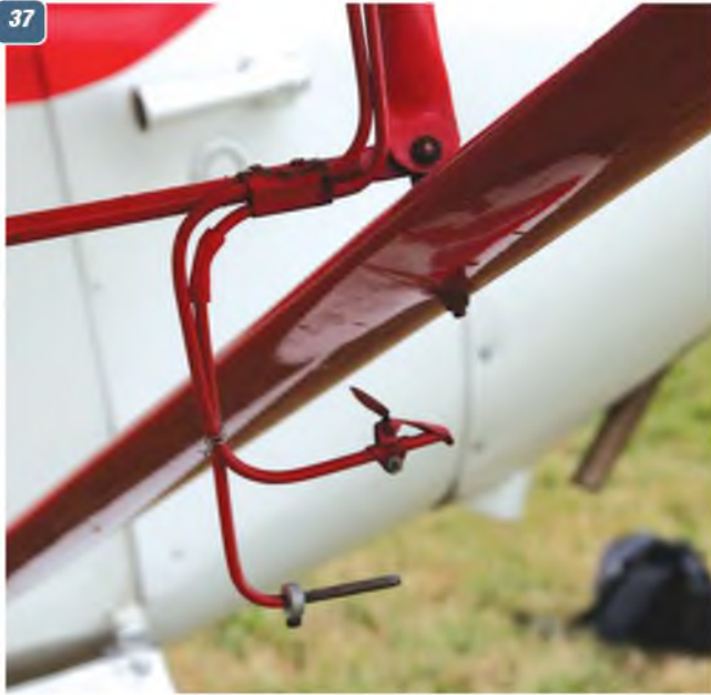
37: The unusual pitot head mounted on the mid-span wing-to-wing-strut brace, starboard side as seen in photo 38 . 39: Wing strut upper anchor point on wing underside. Note also the tie-down loop for lashing down the parked aircraft. 40: Wing strut upper rear anchor point on wing underside. 41: Wing strut lower anchor point on lower fuselage. 42: The Main undercarriage. 43 - 48: Close-up details of the main undercarriage and its mounting points.
