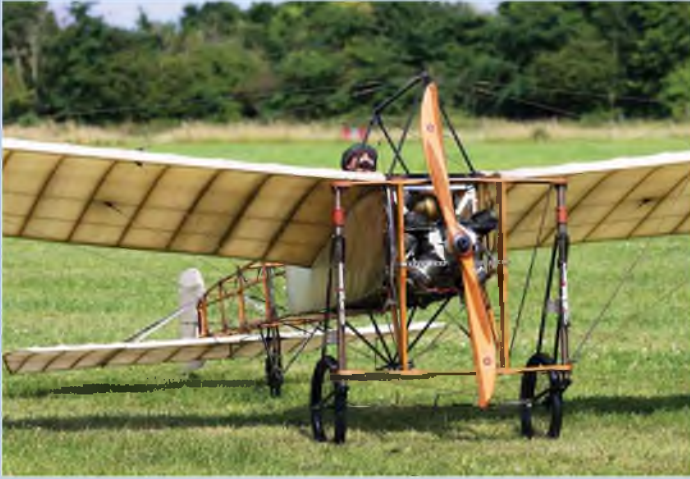
Bleriot IX (1909), 1/3rd scale, owned by James Gordon. Laser 360V power, driving a 28"x7" prop.
