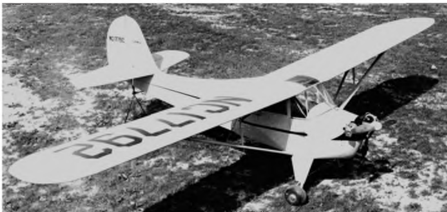
The departure from the 'wire-and-fabric' style of the C-2 and C-3 came with the Aeronca Model K which, in one stride, looks far more of a modern aeroplane.
