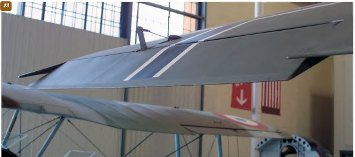
23: Upper surface of the aileron, showing the control horn. 24: Lower surface of the aileron showing the control horn. 25: Close-up of the aileron control horn, control link and aileron hinge. 26, 27 & 28: Three views of the anchor point on the wing undersurface of the front wing strut. 29: Detail of the anchor point on the wing undersurface for the rear wing strut.
