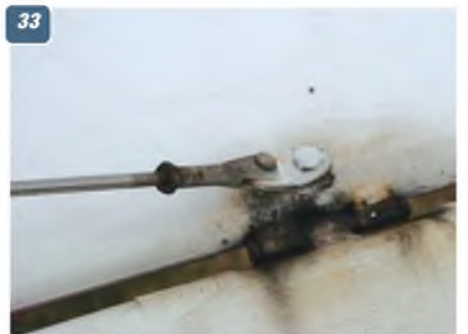
32: Close-up of the elevator trim tab, port side. 33: Tailplane anchor point of the rudder-to-tailplane brace. 34: Rear fuselage starboard side showing the rudder control horn and control wire at exit from the fuselage. Note also the disc shaped inspection panel. 35: Tailplane and elevator at the root, also showing port side inspection panel.
