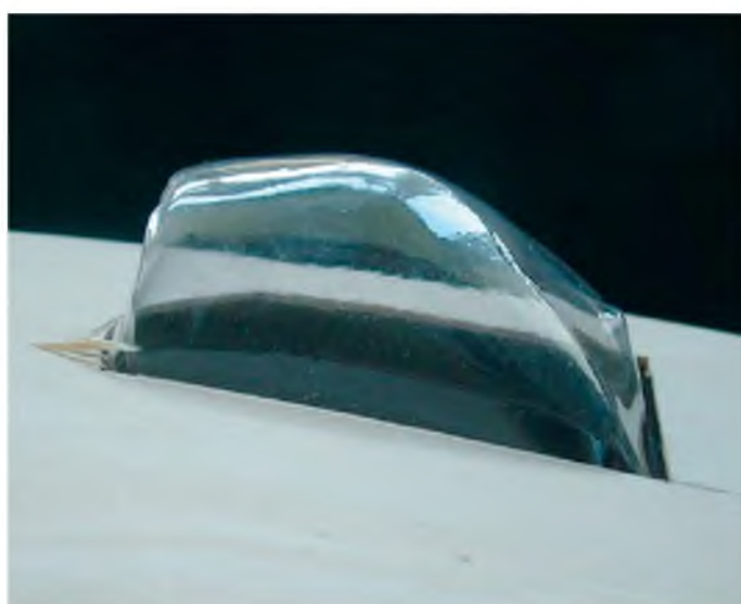
The cowling was moulded from Easter egg packaging scrounged from a skip.
