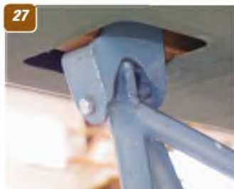
23: Upper surface of the aileron, showing the control horn. 24: Lower surface of the aileron showing the control horn. 25: Close-up of the aileron control horn, control link and aileron hinge. 26, 27 & 28: Three views of the anchor point on the wing undersurface of the front wing strut. 29: Detail of the anchor point on the wing undersurface for the rear wing strut.
