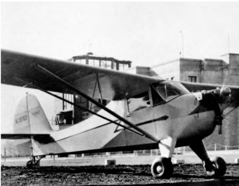
When the Model K went into production, it had been cleaned up a little from the prototype, had more wing dihedral and greater wing area.
