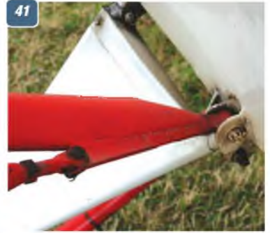
37: The unusual pitot head mounted on the mid-span wing-to-wing-strut brace, starboard side as seen in photo 38 . 39: Wing strut upper anchor point on wing underside. Note also the tie-down loop for lashing down the parked aircraft. 40: Wing strut upper rear anchor point on wing underside. 41: Wing strut lower anchor point on lower fuselage. 42: The Main undercarriage. 43 - 48: Close-up details of the main undercarriage and its mounting points.
