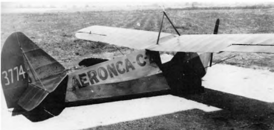
Jean Roche refined his design to this stage, which served as the prototype for the Aeronca C-2.
