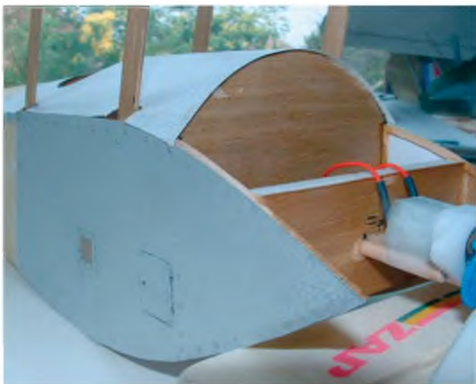
Now the top and side panels can be added from copier paper. The access hatch is just a paper addition, while the inspection panel is cut out of the paper and backed with a patch of very thin acetate.
