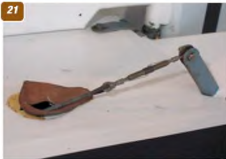
17: View, right side of fuselage, just behind the engine cowl, showing wing strut, where it enters the fuselage. 18: View of the right side of the rear fuselage, showing the control cable runs. 19: Detail of the upper fuselage behind the engine cowl, showing the fuel tank cap. 20: Rear fuselage upper decking, showing the tailplane leading edge and fin anchor point. 21: Top surface elevator horn. Note the leather reinforcement where the control wire enters the tailplane fabric. 22: Tailplane and elevator, showing the elevator aerodynamic balance.
