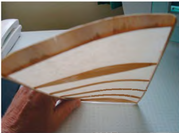
I tried to water-shrink the tissue on a wing panel, which promptly warped and curved. Pre-shrunk tissue is the answer, but plain unshrunk, pulled nice and taut, works well in a dry environment.
