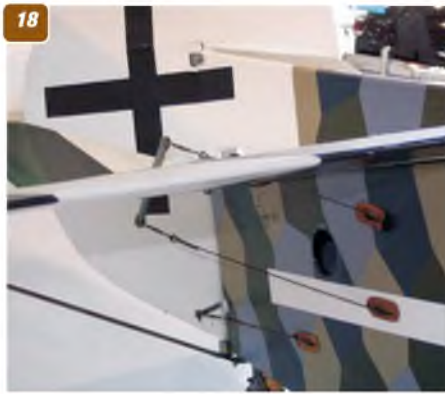
17: View, right side of fuselage, just behind the engine cowl, showing wing strut, where it enters the fuselage. 18: View of the right side of the rear fuselage, showing the control cable runs. 19: Detail of the upper fuselage behind the engine cowl, showing the fuel tank cap. 20: Rear fuselage upper decking, showing the tailplane leading edge and fin anchor point. 21: Top surface elevator horn. Note the leather reinforcement where the control wire enters the tailplane fabric. 22: Tailplane and elevator, showing the elevator aerodynamic balance.
