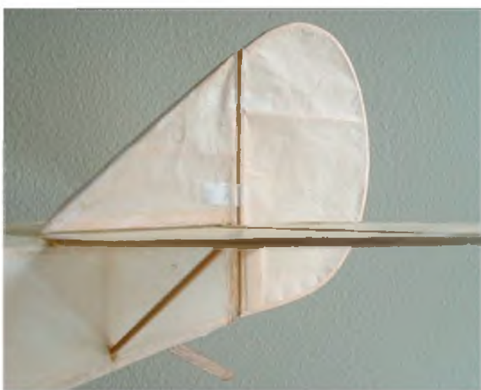
The tailplane is covered on the top only, but the fin and rudder on both sides. A little shrinking is needed here!
