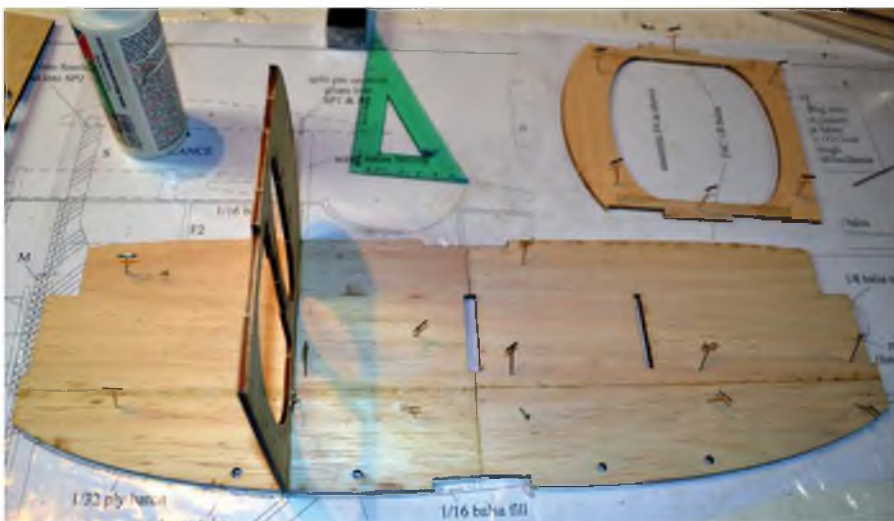
How the formers key into the fuselage sides.
