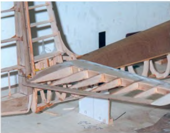
One of the completed tailplane panels, with leading edge fully skinned.
