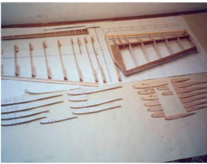
Tailplane construction, with ribs, spar and trailing edge components laid out. Note the rib jigs in place.
