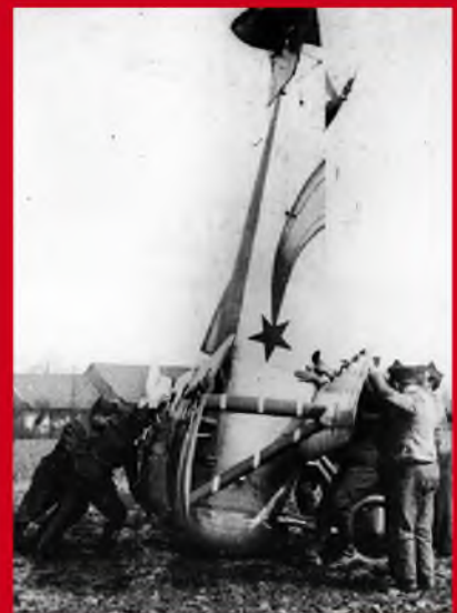
Just about got away with it! N.17c of the Belgian 5th Escadrille, mired in the mud after a nose-over, is manhandled by ground crew. Rough, ill prepared WW1 airfields were a major cause of such incidents.
