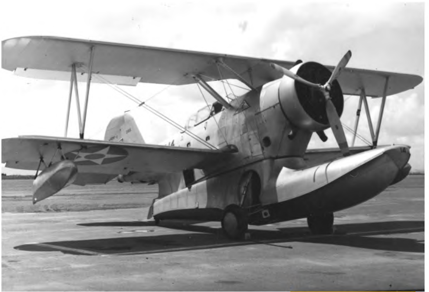
J2F-1 Duck, showing the outrigger floats and the main undercarriage. From a modeller's viewpoint, there may be a lot of work in the airframe, but there is not too much interplane rigging.
