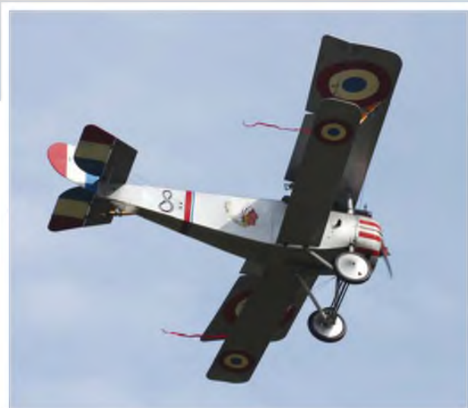
The sesquiplane wing platform is well illustrated in these pictures of this replica Nieuport 17. Narrow chord lower wing provided improved downward view for the pilot.
