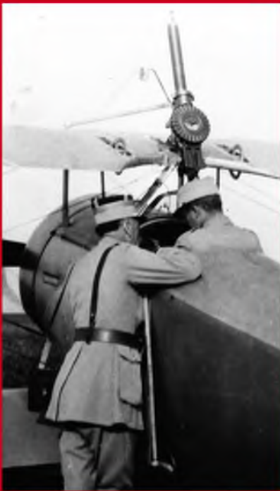
A good view of one of the different types of over-wing Lewis gun mounts fitted to Nieuports of various types. This Lewis is a Mk.II (RFC Pattern), fitted with a No.2 magazine containing 47 rounds. Also well illustrated here are the direct-drive crank to the ailerons, either side of the gun on the top wing.
