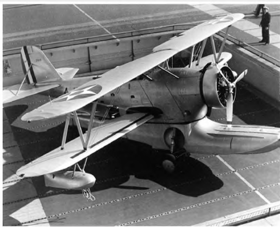
Grumman J2F-1 on the hangar deck lift of USS Yorktown in November 1937. Note the black walkway on the lower wing.
