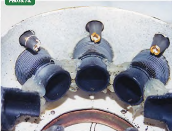
View inside of cowl from the rear showing how cylinders are held with silicone sealant.
