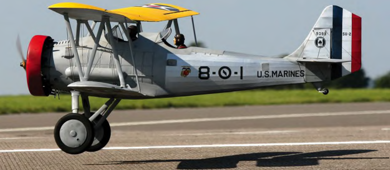
Loening OL-8A. The Prophets of Doom were proved wrong on this one! In spite of the ungainly appearance, it flies really steadily and handles wind well. Nearly defeated on the third day at the Nationals this year though, when the wind speed more or less equaled the forward speed of the model. Home-made retracts (on a screw jack principle) have so far not given any trouble.
