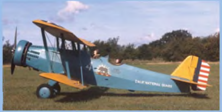
1997. Douglas O38 - 100" span, Laser 180 power.
