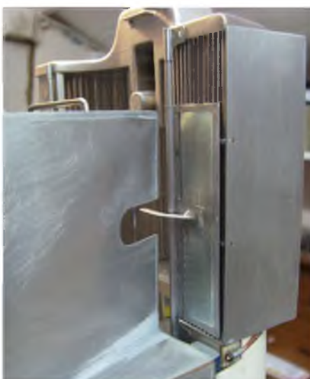
For aesthetics only, the cooling dampers at the rear.
