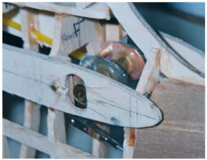
The tailplane is 'all-flying' (i.e.- no separate elevator). This view shows the wing root failing rib and the 'elevator' mechanism.
