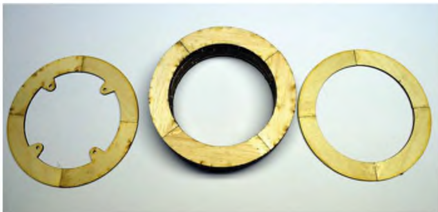
The assembled cowl sections. Note the lugs I made mention of in the text.
