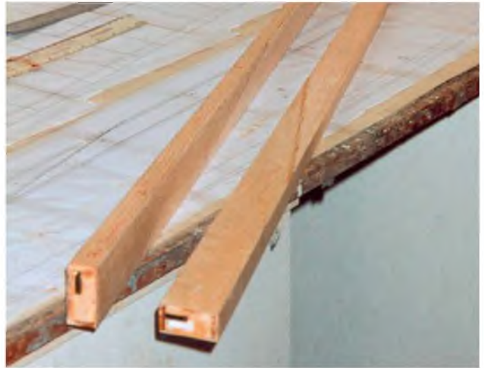
The completed mainspars.
