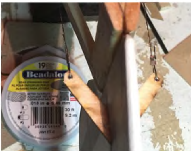
That bushed control horn I mentioned, and the way the control cables are crimped in place.
