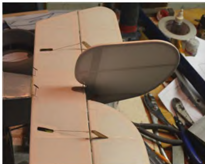
How the elevator cables pass through the tailplane. Just visible beneath the covering are the laser cut parts that enable this.
