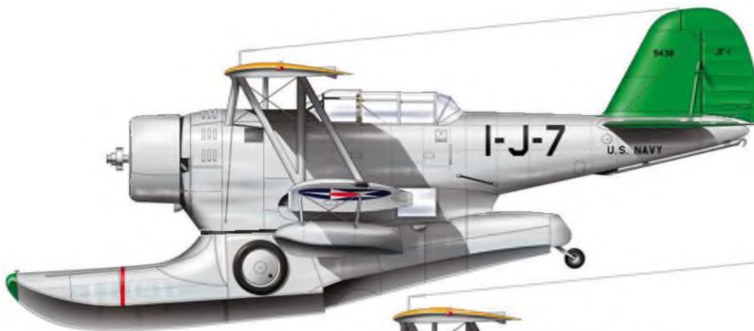
Grumman JF-1 Duck, U.S. Naval Air Station Pensacola, Florida, 1937. Aluminium doped overall with Chrome Yellow top wing upper surfaces; lettering in black. Star markings in six wing positions; '6' repeated in black at centre above top wing. Note arrestor hook removed
