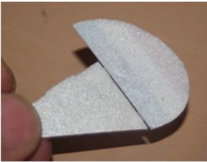
Although they're hard to see, there are two narrow strips of Blendertape used to hinge the rudder before joining the laminated halves.
