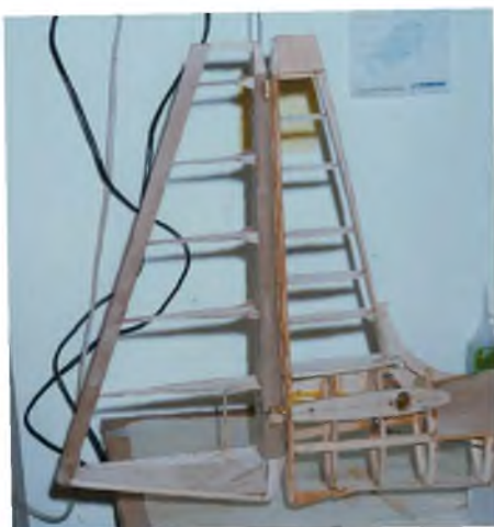
The complete fin and rudder assembly, installed and hinged.
