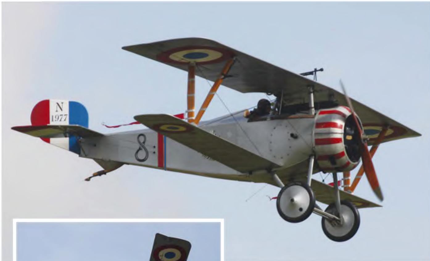
The sesquiplane wing platform is well illustrated in these pictures of this replica Nieuport 17. Narrow chord lower wing provided improved downward view for the pilot.
