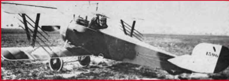
French Nieuport 17 with left and right V-strut mounted salvos of four Le Prieur incendiary rockets for attacks on Observation balloons.
