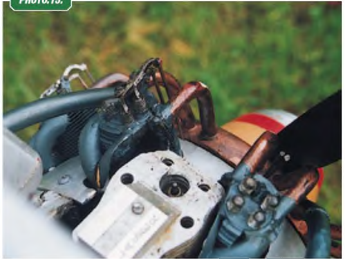
The 'valve springs' from M6 studding.
