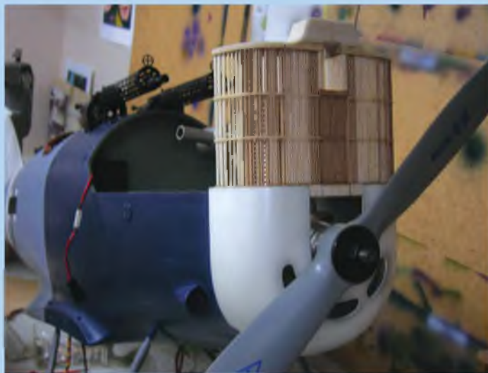
Test fitting of the basic radiator in previously manufactured fiberglass cowling.
