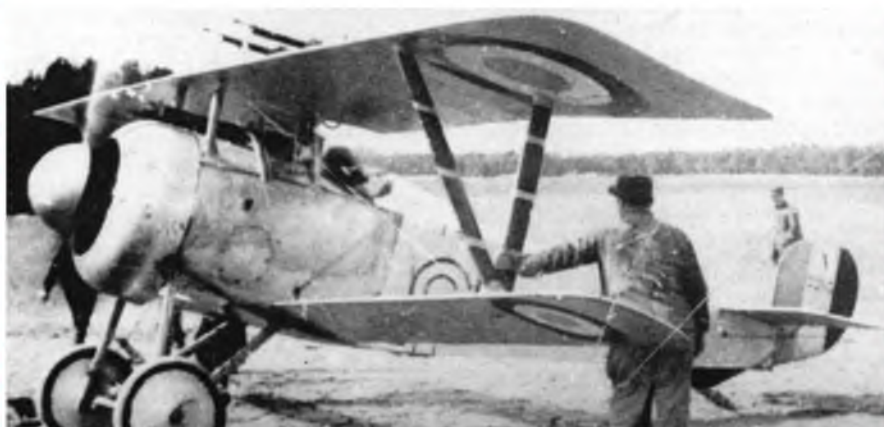
A further example of a French Nieuport 17 with large nose spinner, but more noteworthy for the serious armament of two Vickers Guns on the fuselage front upper decking and two Lewis Guns mounted on the upper wing centre section. By the standards of the day, a massive punch!
