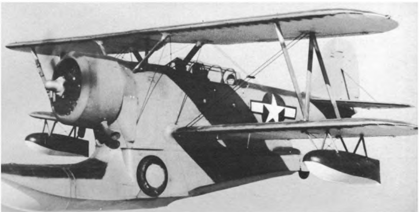
A J2F-6 Duck, with the wide-chord engine cowl in late WW2 US Navy two-tone finish of bark blue upper surfaces and light grey wing undersides and fuselage.
