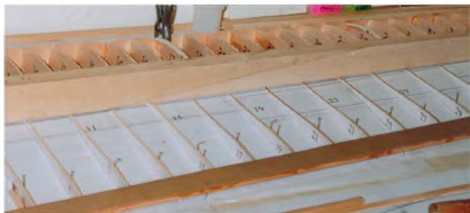
The wing going together. Mainspar in place together with leading edge ribs. Note the rib jigs placed ready to support the ribs behind the mainspar.
