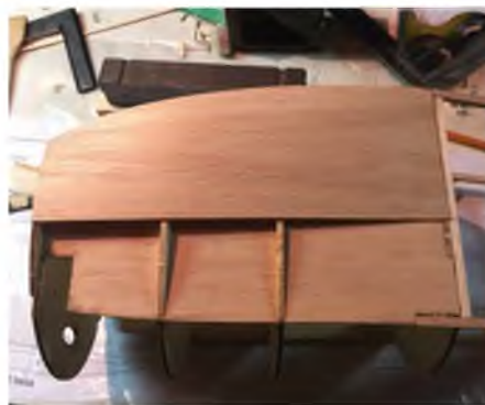
This shot shows the side sheeting going onto the right hand fuselage side. Note the shape and number of formers.
