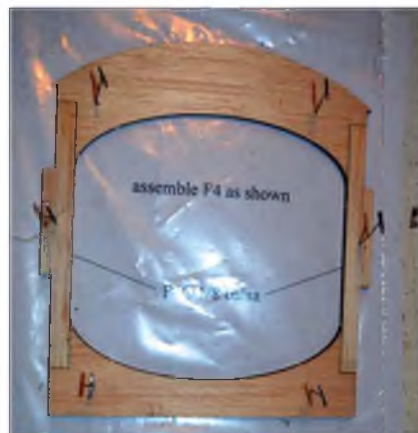
Another part to be assembled over the drawing is F4 which is built up from laser cut parts.
