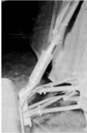
RIGHT: The right side retracting undercarriage that lifts and folds into the side of the lower fuselage/float.
