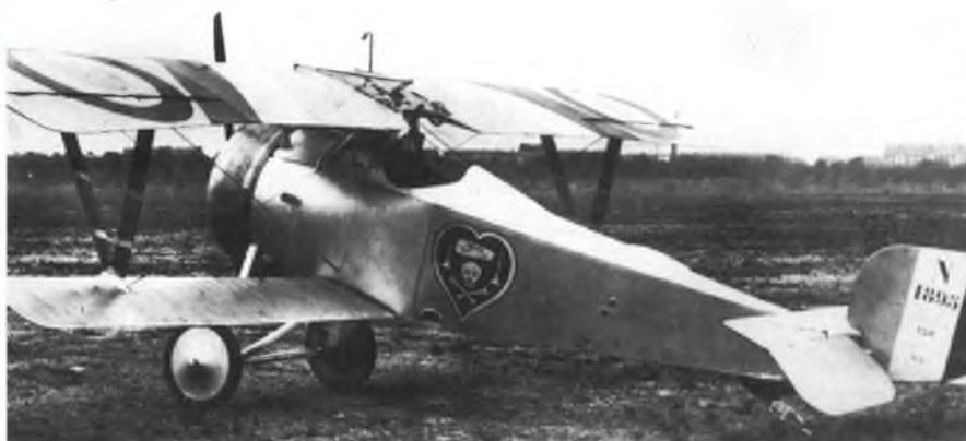
Type 17c with Gnome 80hp engine in the famous markings of Lt. Charles Nungesser. Note red & white personal identifier stripes on top wing upper surface, applied after Nungesser was attacked by allied aircraft.
