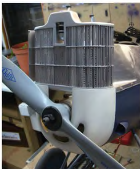
Deflector screen in position would aid cooling to the left side.
