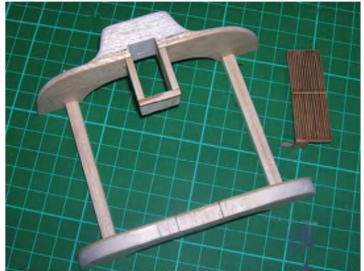
1/4" (6mm) square spacers to hold sections at correct distance apart.
