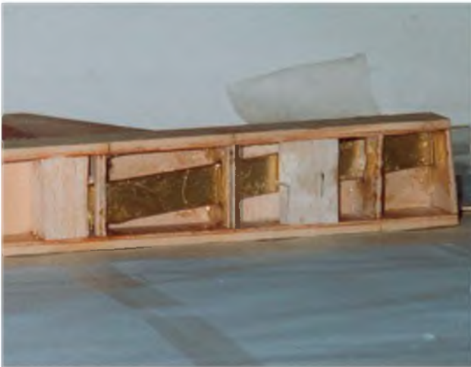
Mainspar at the wing root before adding the side - showing the brass dihedral tongue box.
