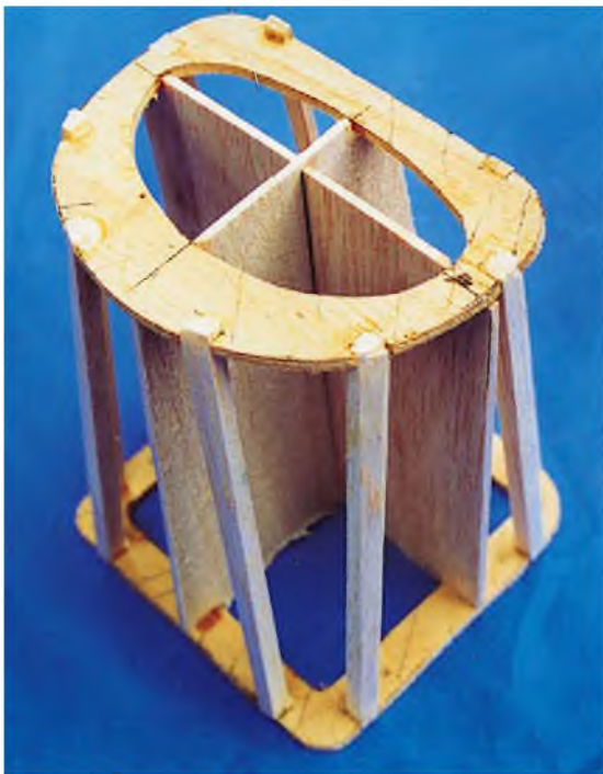
Building the cowl, stage 1 - jig is knocked out later.
