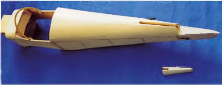
The fuselage with the top sheet on - note slot for fin. Canopy frame is not glued in place at this stage.
