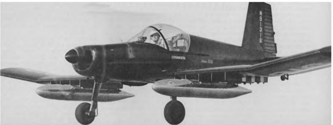
Prototype in flight, carrying two napalm tanks slung on hard points under the wing.
