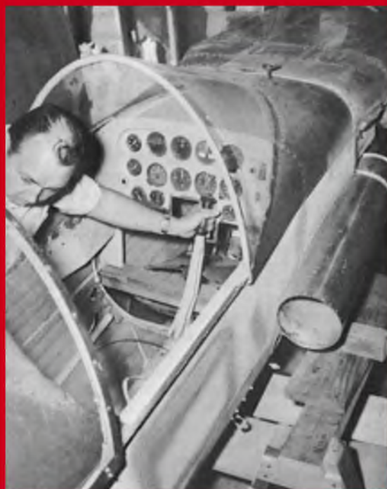
Cockpit interior of what may well have been a pre-prototype static inspection mock-up. The large diameter external exhaust pipe dubbed as an augmentor device.
