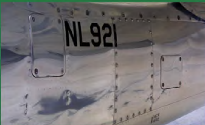
The North American P-51D Mustang was an excellent example of butt-joined surface skin panels and flush riveting.
