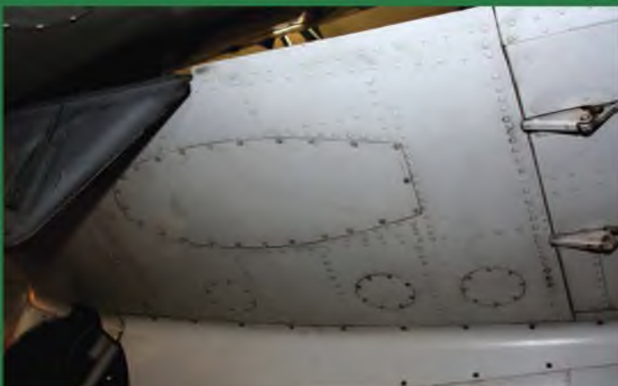
The Grumman F4F Wildcat was festooned with both overlapping and butt-joined surface skin panels, plus many access panels. The latter tended to sit proud of the basic surface skin - something else to be simulated, possibly with lithoplate, thick paper or thin card.
