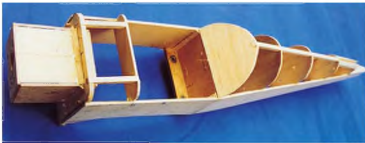
Basic fuselage with engine mount box. Note triangular stock in all corners.
