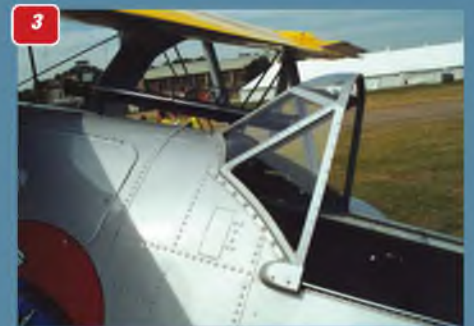
1 - 3 Three views of the cockpit front windscreen. 4 A view of the multiple-frame sliding rear canopy. Note also the extensive use of exposed round-head surface rivets, a construction feature that extended beyond the F3F to its immediate successor, the F4F Wildcat and the subsequent F6F Hellcat.
