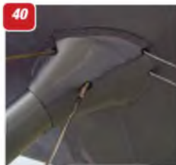
34 & 35: Two views of the main undercarriage fairing panel attached to the main undercarriage struts that folds with the leg to fair with the fuselage.
