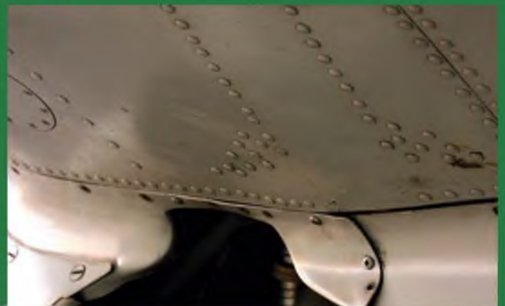
The Grumman F4F Wildcat was festooned with both overlapping and butt-joined surface skin panels, plus many access panels. The latter tended to sit proud of the basic surface skin - something else to be simulated, possibly with lithoplate, thick paper or thin card.
