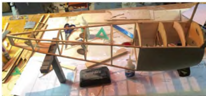
Everything jugged up to ensure the front and rear boxes align correctly.
