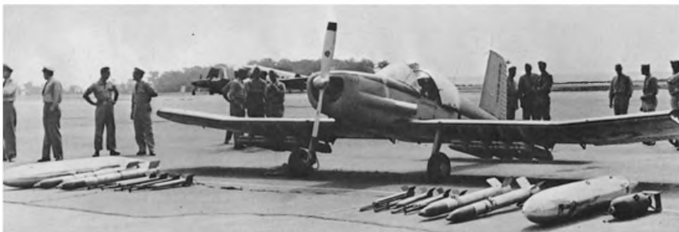
FD-25 could carry a wide range of weapons stores. In addition to two 0.30 calibre guns, of could carry four 5~" HVAR rockets, thirty-two 2.75" folding-fin rockets, twenty 8cm Oerlikon rockets, two 40 gal. napalm bombs or two 250 lbs general purpose bombs.
