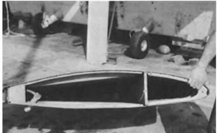
View of one of the wing panels, reveals the shape of the airfoil section and some of the structure.
