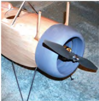
Here you see how the cowl is shaped and then sealed and primed ready for painting. Pat also added stiffening ribs to his cowl but not all aircraft had them.
