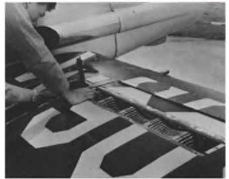
The ammunition trays in the wings of the FD-25 could accommodate 1000 0.30" calibre rounds.
