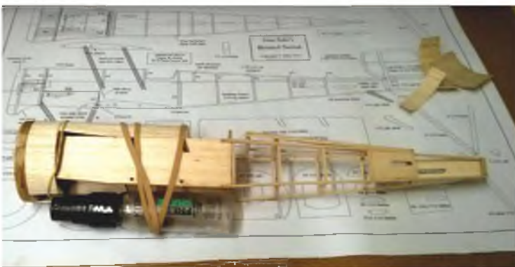
All the basic components ready for sanding. As you can see, Paul opted for a strip and gusset tailplane.
