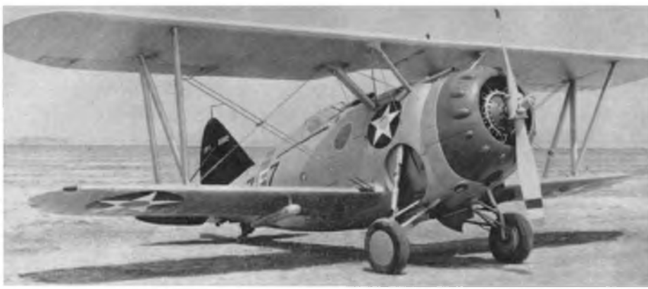
An F3F-1 of VF-7 (Fighting Squadron Seven) with the black fin and rudder with of U.S.S. Wasp with large 'Neutrality Star' applied to mid-fuselage, April 1940. Note bomb rack under starboard wing.
