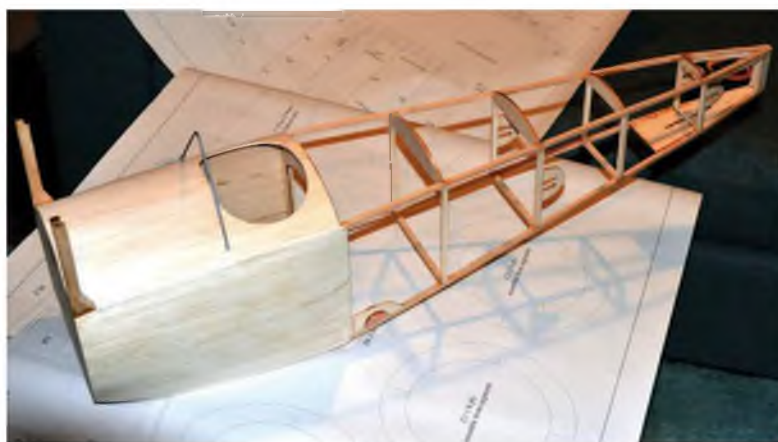
The same fuselage but now with the struts installed and the forward areas sheeted.
