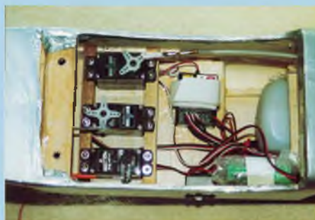
Radio bay, no lack of space. Note access to Rx - saves even more extension leads.
