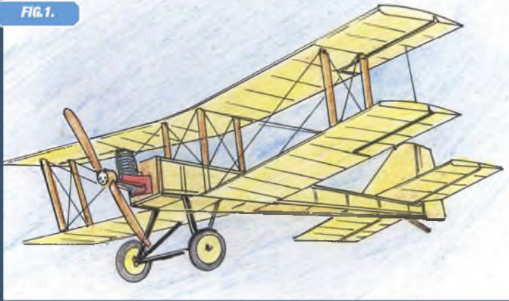
FIG 1: The simplest biplane - Clark Y section, box fuselage. FIG 2: Typical forward fuselage cross section. 1/4"sq. spruce main box structure, balsa formers and 1/8" planking. NOTE: The main box structure will be close to the surface at the corners, for attachment of the cabane struts and main undercarriage legs.
