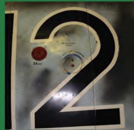
The Messerschmitt Bf 109E featured mostly butt-joined surface skin panelling
