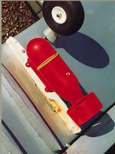
Under-wing stores pylons. The dummy ones are only held on with spots of glue so that they will knock off without damaging the wing skins.
