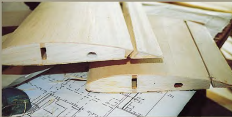
The ends of the wing panels showing the flap (top) and the aileron (bottom). Also holes for dihedral braces. Note: control surfaces are built with the wing and cut away later.
