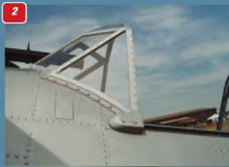
1 - 3 Three views of the cockpit front windscreen. 4 A view of the multiple-frame sliding rear canopy. Note also the extensive use of exposed round-head surface rivets, a construction feature that extended beyond the F3F to its immediate successor, the F4F Wildcat and the subsequent F6F Hellcat.
