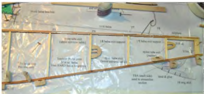
The basic rear fuselage side. Note the darker, harder wood used for the longerons.
