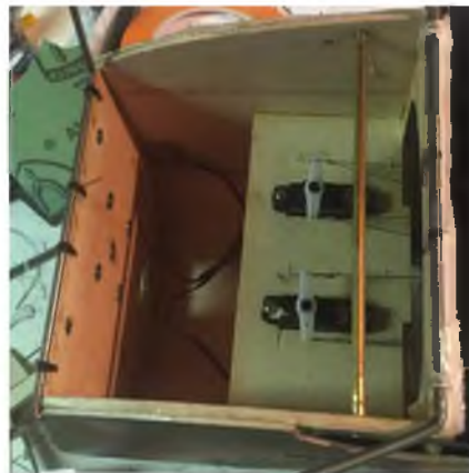
Servos in the tray, closed loop cables connected and ample room for the battery pack immediately behind the firewall.
