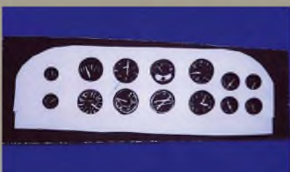
Instrument panel from Scraperboard and thin polystyrene sheet. Finished panel is basic, but layout is correct.
