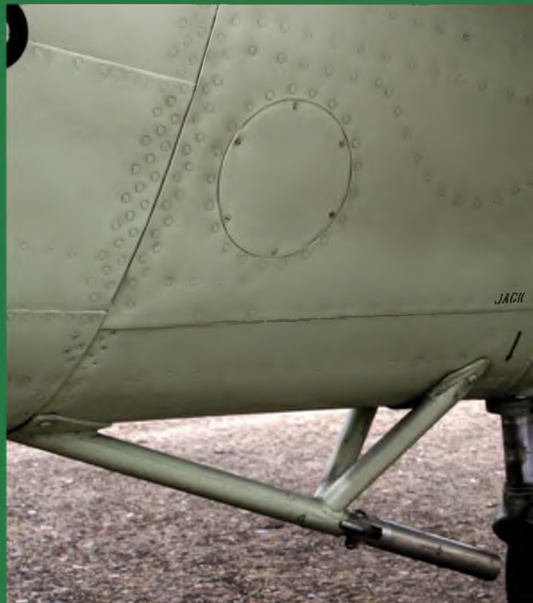
Overlapping panels were typical on the Royal Navy's Seafires. This is a bubble-canopy Mk.17. WW2 carrier-borne aircraft were subject to serious rough and tumble, so quickly acquired considerable surface panel dents - something else to think about!
