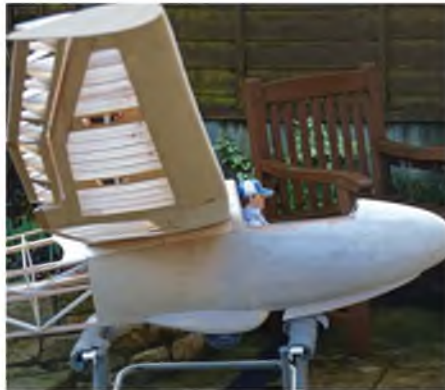
Author's version of the full size monocoque on the front of the glider
