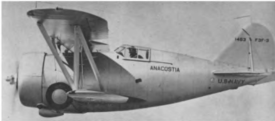
A plain finished Grumman F3F-3 assigned to Naval Air Station Anacostia. On the F3F-3, the cowling was faired around the exhaust stacks in contrast to the F3F-2's cut-out.
