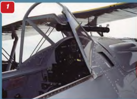
1 - 3 Three views of the cockpit front windscreen. 4 A view of the multiple-frame sliding rear canopy. Note also the extensive use of exposed round-head surface rivets, a construction feature that extended beyond the F3F to its immediate successor, the F4F Wildcat and the subsequent F6F Hellcat.
