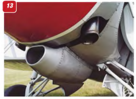
5: Pilot's seat and headrest. 6: Further view of the headrest, also showing the rear canopy guide rail. 7 - 9: Cockpit instrument panel features modern instrumentation. 10: Cockpit instrument panel features modern instrumentation. 11: Cowl & prop. 12: Propeller hub. 13: Air scoop under the engine cowl. 14: View rearward under the fuselage. 15: Cooling louvres on forward fuselage. 16 & 17: Fin & rudder.
