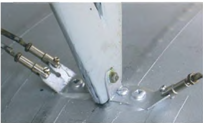
Close up of strut end and wire termination, including the Mick Reeves adjustable end fittings.
