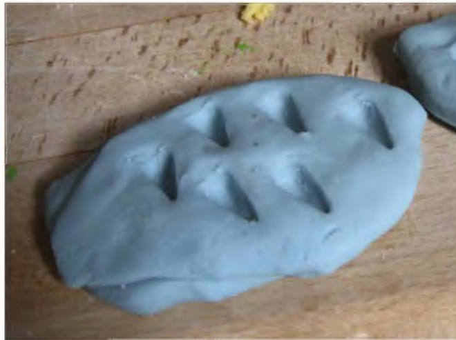
The simple mould Vicky made for producing the cowl blisters.
