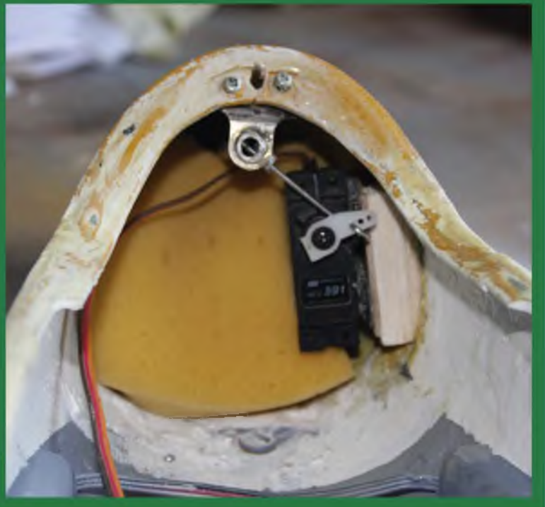
Fig.11: This towline release comprises a length of tube, buried in the fuselage nose. The towline link at the glider end has a long, slim loop, which is fed up the tube to the inside end. The servo mounted on the fuselage side withdraws the piano wire lock/release pin sideways across the fuselage at 90 deg. to the line of flight.
