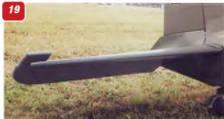
16: A little bit of history! 17 & 18: Rear fuselage detail just ahead of the tailcone. 19: Tailpane, showing the aerodynamic balance at the tip. 20: The cabin showing the full run of the clear side panels. 21 & 22: Two views of the fuselage rear showing markings. 23: Front cockpit showing the windscreen and the mass of fully visible structural members. 24: The cockpit area, with the crew access panels folded down. 25: Further view of the cockpit windscreen revealing the double curvature of the clear screen.
