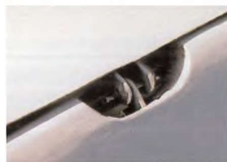
Detail of one of the elevator hinges in the elevator-to-tailplane cuff.
