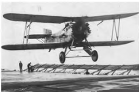
Flycatcher landing on HMS Glorious. Note the lack of arrestment wires, either longitudinally along the length of the deck, or transverse across it.
