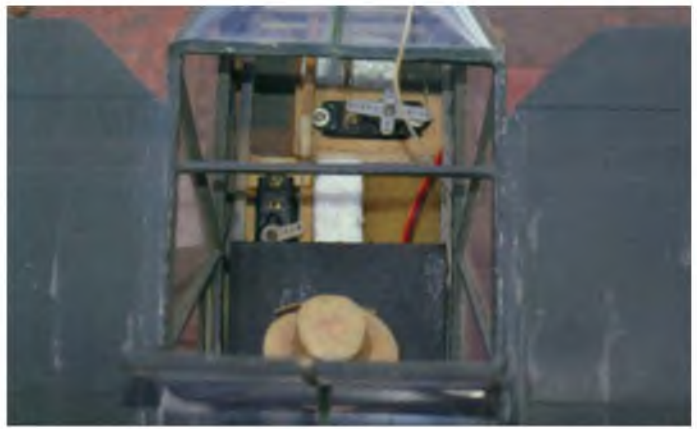
The top clear-visibility hatch is hinged for access to the receiver, servos and power pack.
