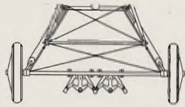
Flycatcher Mk.1 undercarriage showing earlt arrestment mechanism for fore/aft run arrestment wires
