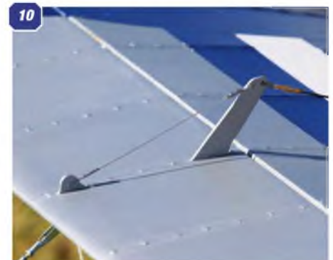
5: The rear fuselage is full of character. 6: Fuselage tape and lacing detailing is all present. 7: Rear fuselage is top is stringered. 8 & 9: Rib tapes and stitching faithfully simulated on the wings. 10: Scale aileron horn and anchor points.
