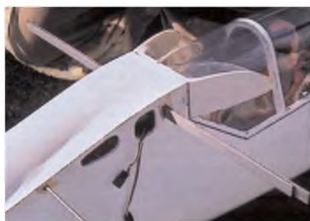
Detail of the metal wing joiners that slot into the wing. Extension leads for the aileron and spoiler servos hand ready.
