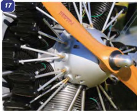
16: From this view, it is obvious why Ken had to get the dummy engine convincing. Look closely for the Saito. 17: Hand crafted dummy engine took two months to complete. 18: Dummy engine "cone" was moulded from a blue foam plug turned on the lathe. 19: The model uses Williams Brothers 6" diameter wheels. 20: Undercarriage struts and wires are carefully terminated. 21: The Flycatcher's working "sprung and oleo'd" undercarriage is complex. 22: Two wings and a round engine: a scale model formula that never fails.
