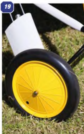
16: From this view, it is obvious why Ken had to get the dummy engine convincing. Look closely for the Saito. 17: Hand crafted dummy engine took two months to complete. 18: Dummy engine "cone" was moulded from a blue foam plug turned on the lathe. 19: The model uses Williams Brothers 6" diameter wheels. 20: Undercarriage struts and wires are carefully terminated. 21: The Flycatcher's working "sprung and oleo'd" undercarriage is complex. 22: Two wings and a round engine: a scale model formula that never fails.
