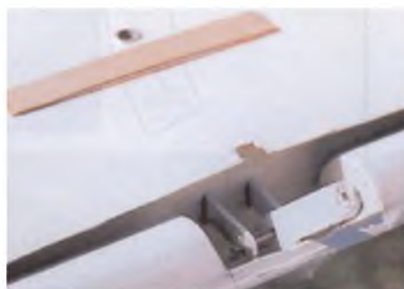
Detail of the centre line elevator horn and centre line hinge, all cut from sheet metal. Note also the hole for the tailplane retainer bolt.
