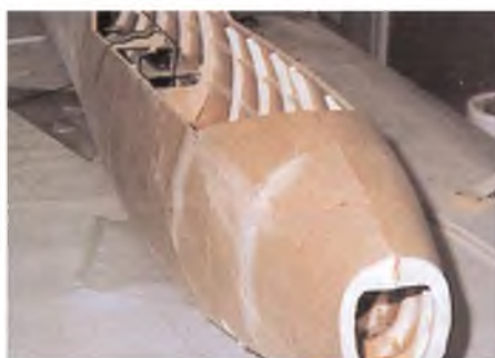
Here the entire nose section of the fuselage is fully surface panelled and the servo tray and servos are installed.
