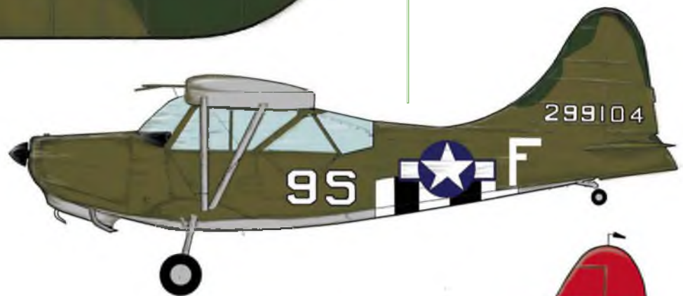
Stinson L-5A operated by a unit of the USAAF 9th Air Force liaison squadron in Europe. Two-tone Olive Drab upper surfaces. Invasion stripes applied to lower fuselage only and to lower surface of both wings.
