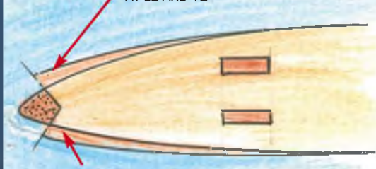
FIG. 5 - SHAPING RIB LE/TE TO MATCH LE/TE STRIP SECTION.
