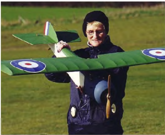
Built years ago, and not actually a scale model, this 56" span monoplane was powered by a geared 600 brushed motor and 7 or 8 Ni-Cad cells. Flew really well.
