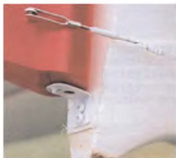
The lower hinge point of the rudder, pivots on this piano wire pin located on metal bracket screwed to the bottom of the fin tailpost.
