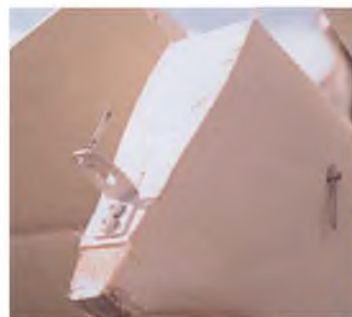
The lower hinge point of the rudder, pivots on this piano wire pin located on metal bracket screwed to the bottom of the fin tailpost.
