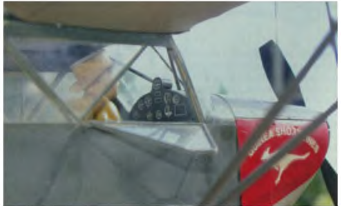
Detail of the cabin side windows. One side is hinged for switch access - don't forget to fit a pilot!
