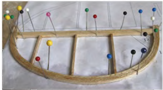
Although I don't advocate the pin 'fence' method (see text) this is how the laminated outlines are built into the tail surfaces. In this case, one elevator.
