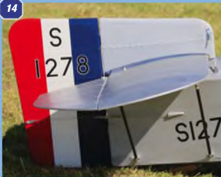
11: Ken has achieved a realistic patina on his (Williams Brothers)Vickers machine gun kit. 12: Forward fuselage is doped tissue, painted; rear is painted and sealed Solartex. 13: Note interplane strut detail. 14: Adjustable tailplane supported on carbon fibre struts with turned aluminium terminations. 15: Ken built the wooden tail skid from hardwood.
