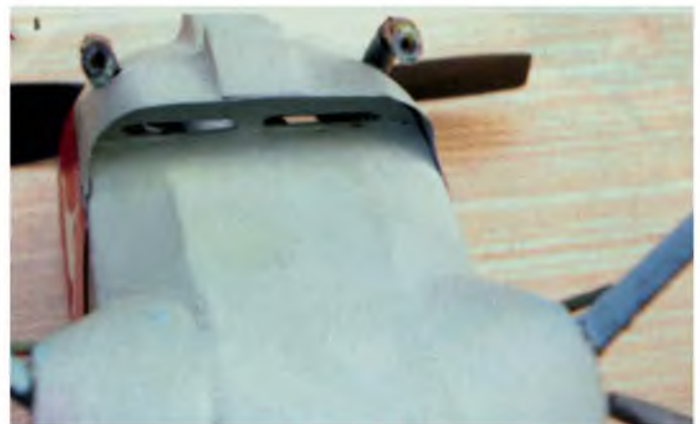
The under view of the cowl and 'exhaust' stacks, showing the original Mills exhaust exit slots under the rear edge.
