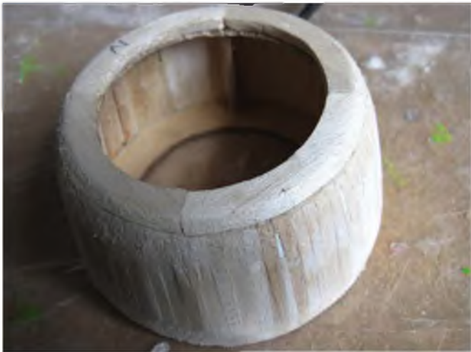
How the cowl is planked and sanded to shape.
