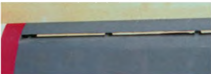
John built in fixed slats on the wing LE just like the full size - easy to do and certainly adds to the 'look'.
