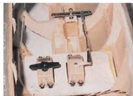
Typical servo installation showing the elevator and rudder servos with remote bellcrank line to the closed loop rudder linkage.
