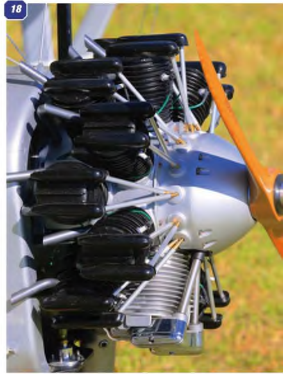
16: From this view, it is obvious why Ken had to get the dummy engine convincing. Look closely for the Saito. 17: Hand crafted dummy engine took two months to complete. 18: Dummy engine "cone" was moulded from a blue foam plug turned on the lathe. 19: The model uses Williams Brothers 6" diameter wheels. 20: Undercarriage struts and wires are carefully terminated. 21: The Flycatcher's working "sprung and oleo'd" undercarriage is complex. 22: Two wings and a round engine: a scale model formula that never fails.
