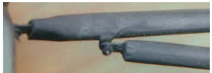
The strut attachments are bolted in the manner of the full-size - could be made a lot simpler and more 'arrival' resistant, if building for free flight.
