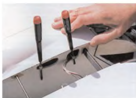
Screwdrivers hold the rubber band wing retainers ready for hook-up to the wing root hooks.
