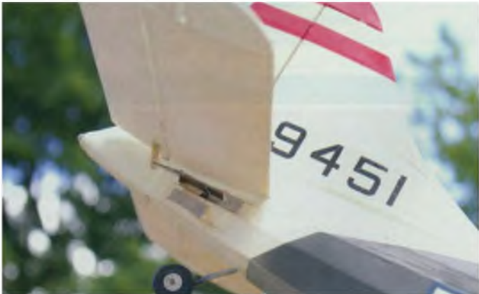
The tail could be a bit tidier, but the radio system and associated control linkages are a retro-fit after initial free flight activity.
