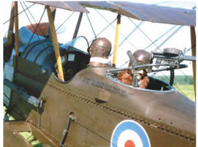
A birds nest of wires! The earlier the aeroplane, the worse was the tangle of wires. This is my RE8.
