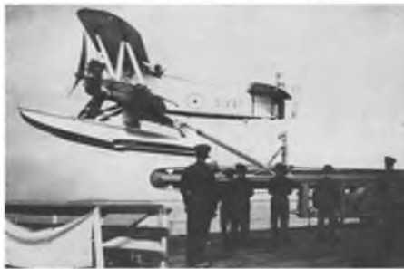
Catapult launch of a Flycatcher in floatplane configuration. Recovery on return was by crane.
