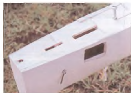
Rear fuselage showing the tailplane seat, retainer bolt and access hatch to the elevator control horn.
