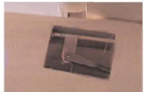
Removable panel in fuselage rear under the tailplane, allows access to the elevator horn for adjustment.
