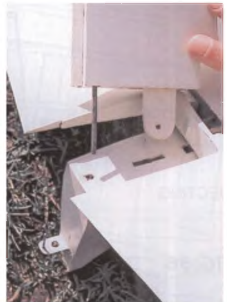
Tongue-and-slot mounting of the tail fin allows it to be removable for transport if required.
