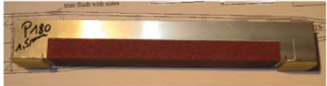
Not from Vicky's build but a useful example of a simple tool to ensure you don't sand the tail surfaces too thin.
