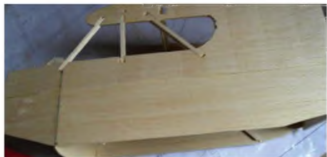
The basic forward fuselage box provides a solid base around which everything else fits.
