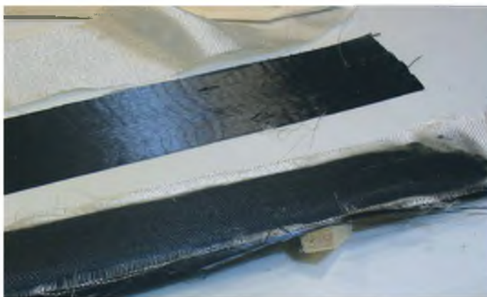
Covering the balsa strut with carbon and glass cloth.
