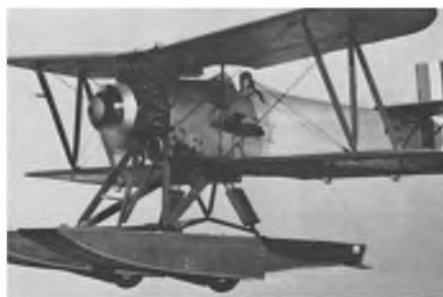
WHEELS AND FLOATS TOGETHER: In amphibian configuration, the Flycatcher had barely visible wheels let into the planing undersides of the floats and presented an odd sight when taxiing at a shore base. Note also the propeller spinner, only occasionally applied.
