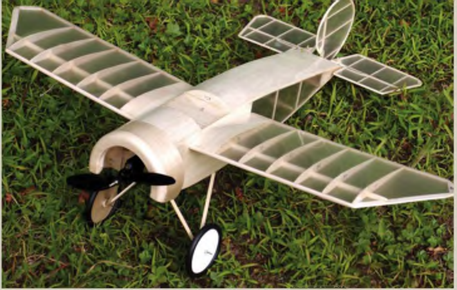
This 32" model demonstrates, through the doculam covering, my favoured reinforced rubber power style of construction.
