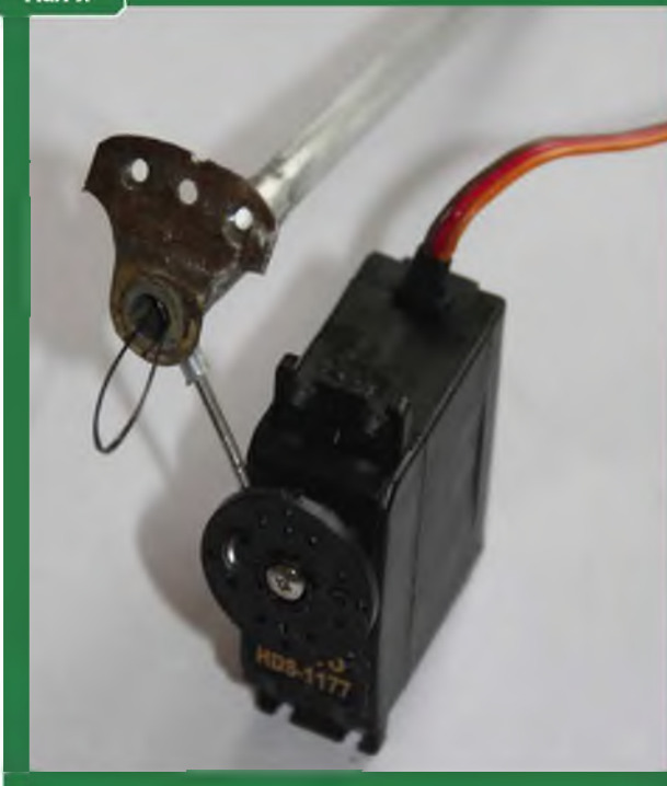
Fig.11: This towline release comprises a length of tube, buried in the fuselage nose. The towline link at the glider end has a long, slim loop, which is fed up the tube to the inside end. The servo mounted on the fuselage side withdraws the piano wire lock/release pin sideways across the fuselage at 90 deg. to the line of flight.
