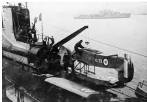
Besson MB 411, extracted from the Surcouf's hangar, being assembled on the rear deck.
