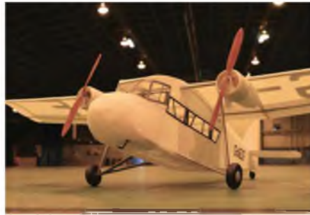
Graham Smith's ambitious electric powered Short Scion has twin geared props.
