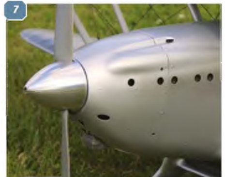
5: The formers between the fuselage stringers were scalloped so as not to show through the covering. 6: For convenience, and to reduce rigging time, the model parts just behind the cockpit. 7: The cowled OS engine has an on-board glow system and drives an APC 15"x6" prop.
