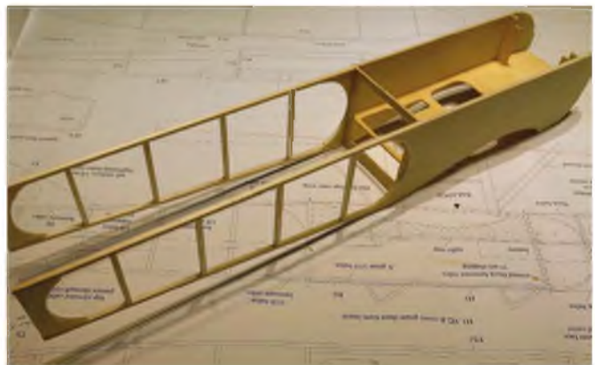
Fuselage sides joined using a couple of formers and the radio tray.
