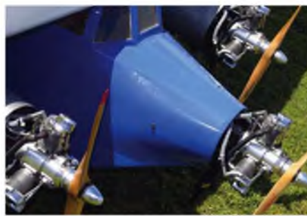
Three lovely Saito 30cc three-cylinder radial engines power the 'Southern Cross'.
