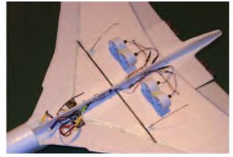
The busy bits of Eric Strefford's AVRO Vulcan B2: four 30mm electric Ducted-Fan units.
