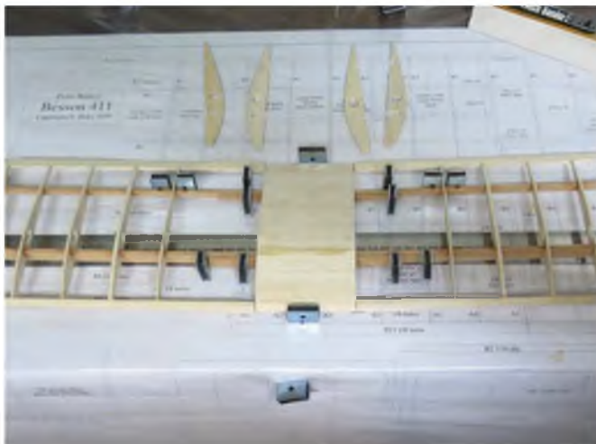
Wings joined to centre section prior to adding the last few ribs and top surface sheeting.
