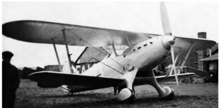
Apparently devoid of any identification marking, what can be seen here is the cannon barrel at the tip of the propeller spinner and the barrels of the two 0.30" machine guns in the lower wing leading edges. (Photo: Richard Riding).
