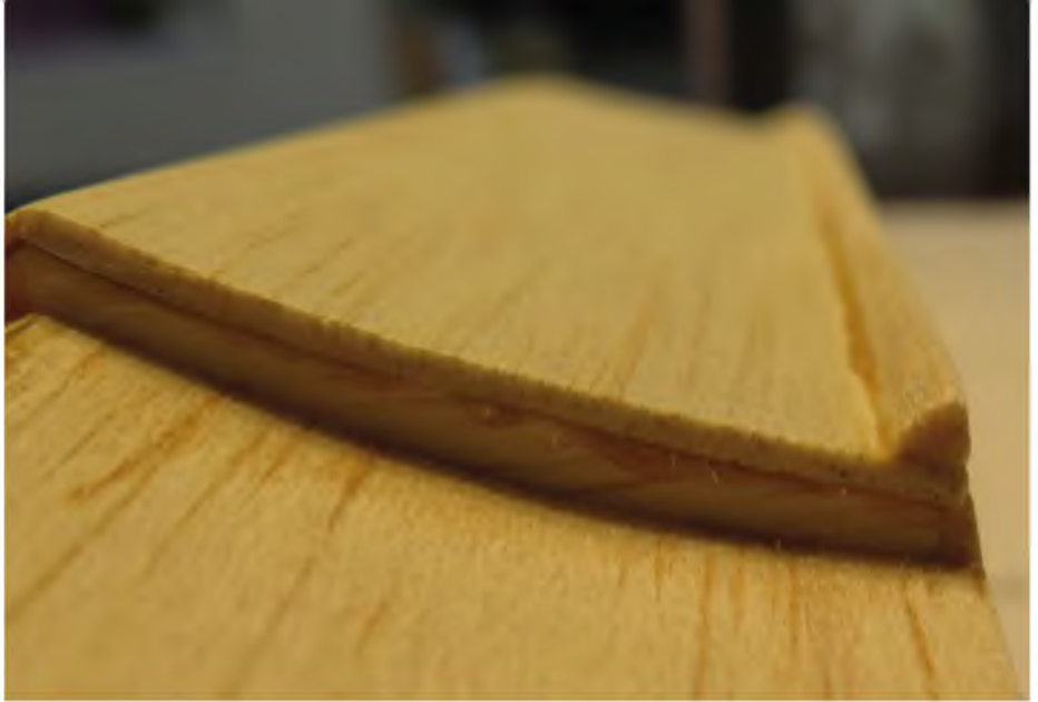
Here you see how Mat reduced the curve on the planing surface to ease sheeting. The anti spray strakes are a work in progress.
