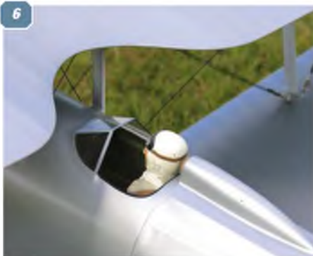
5: The formers between the fuselage stringers were scalloped so as not to show through the covering. 6: For convenience, and to reduce rigging time, the model parts just behind the cockpit. 7: The cowled OS engine has an on-board glow system and drives an APC 15"x6" prop.
