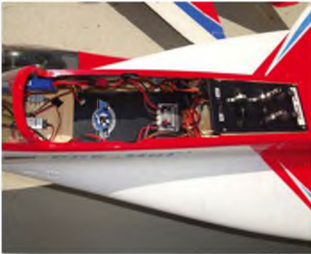
Neat control layout in the Skymaster turbine MIG 29.
