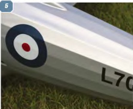
5: The formers between the fuselage stringers were scalloped so as not to show through the covering. 6: For convenience, and to reduce rigging time, the model parts just behind the cockpit. 7: The cowled OS engine has an on-board glow system and drives an APC 15"x6" prop.
