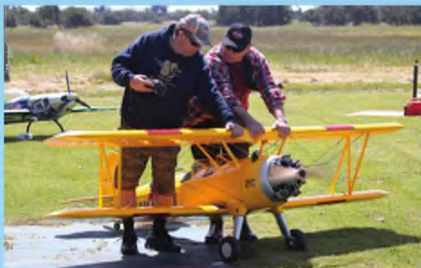
Vince Belshaw and helper restrain Vince's new Balsa USA 1/3rd scale Boeing Stearman as he revs the Moki 250 seven-cylinder radial four-stroke.
