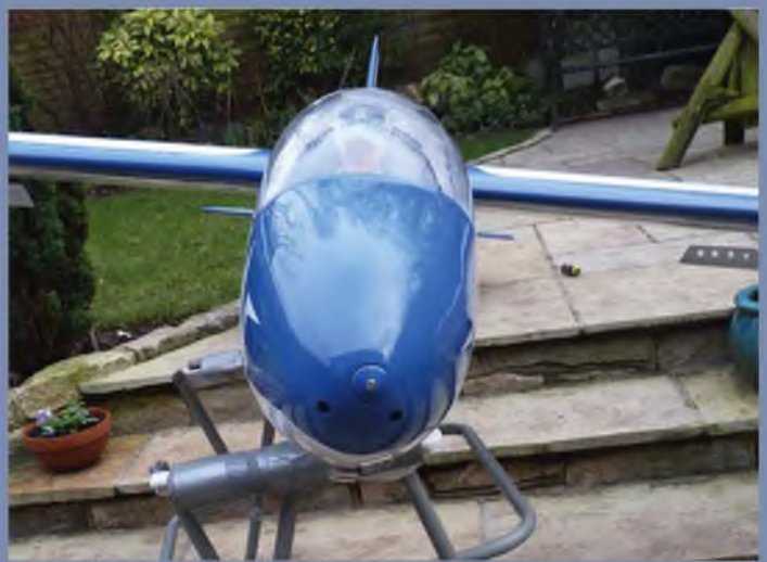
Propeller shaft hidden by small blanking plate.
