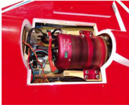
Shane's KingTech K180 turbine in the Skymaster MIG.
