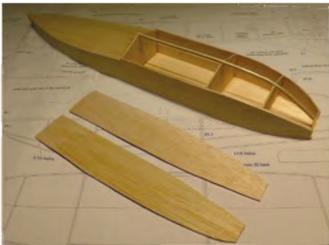
Here you see the extra keel piece Mat added to the main float in order to provide more gluing area for attaching the skins.
