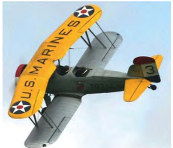
The Curtiss Helldiver. Most of these US Navy biplanes make great flying models. Chunky layout and Clark Y wing section mean they handle wind well.
