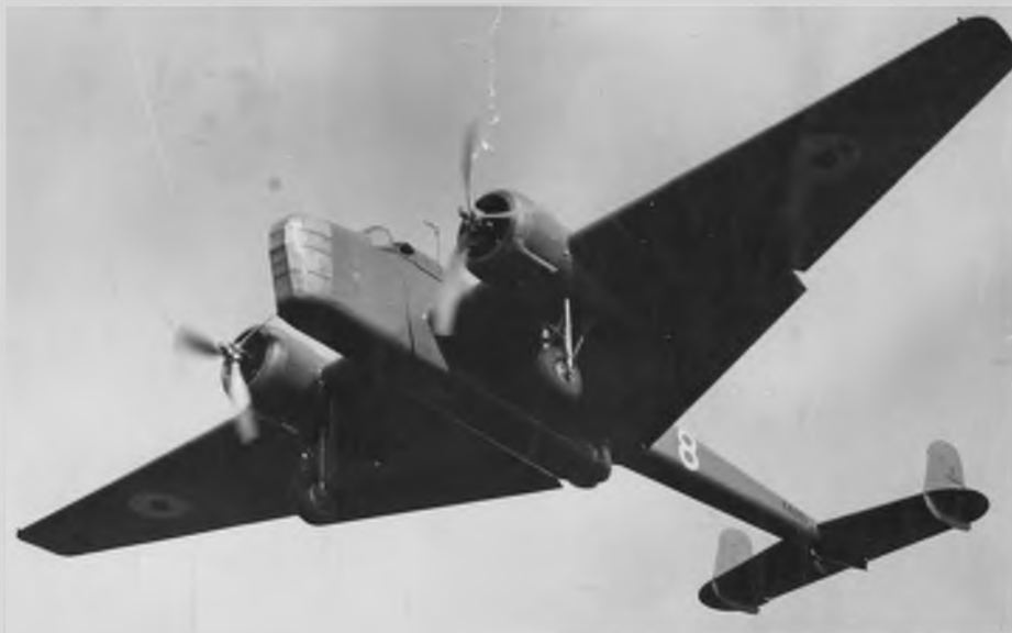
Prototype H.P.52 on final approach, with wing flaps fully extended. The extreme 'boxey' shape prior to subsequent refinement is clear here.
