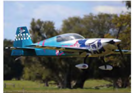
Scott Pittick's Composite ARF Super Extra 330 - 3.1m/ 10ft span and DLE 170 2-cylinder 2-stroke powered, with a 28.5 x 12 three-blade carbon prop.
