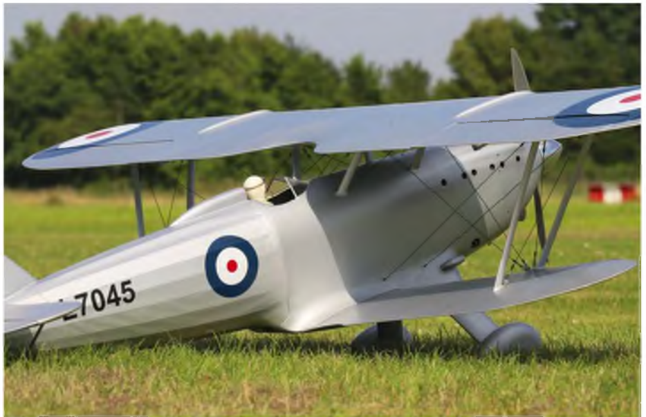
There is a surprising unity between the cowled front and the stringered rear of the fuselage.
