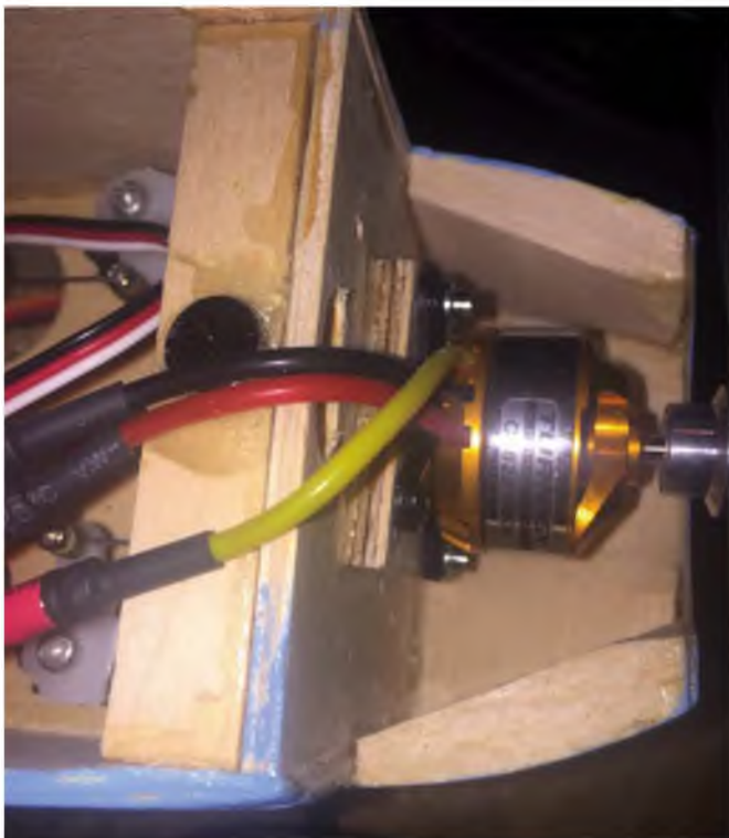
Pat's replacement motor in place. Those wires will ultimately pass through the hole you see just above the mount plate.
