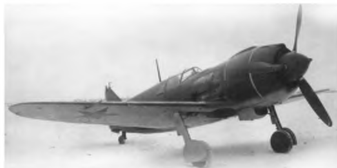
In its original format the La-5 perpetuated the fuselage shape of the previous LaGG-3 on which the cockpit canopy faired into the rear fuselage shape.
