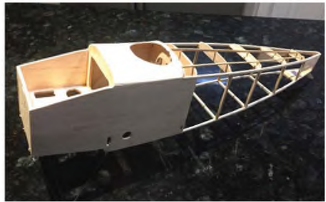
As you can see, there's nothing too involved with getting the fuselage to this basic box stage. Just the remaining stringers and nose blocks to go.
