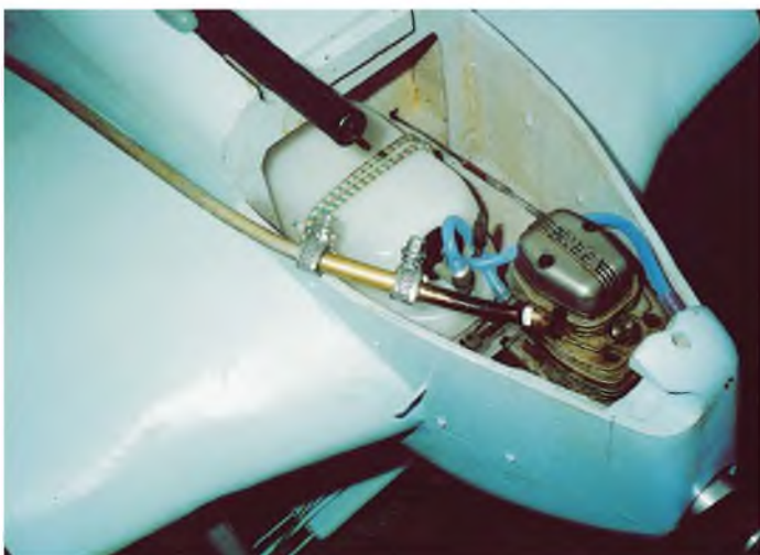
The engine compartment is a tight squeeze for the Enya 60. A smaller engine could be fitted but additional lead would be required to compensate for a lighter engine. Note the brass tube in the nose to provide pitot pressure to the fuel tank.
