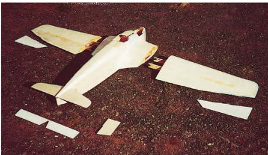
The model is now ready for tissue covering to be applied, using Balsaloc or dope.
