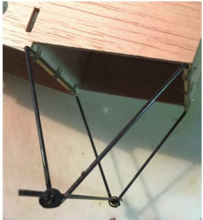
Landing gear legs plugged into their tubes and the axle soldered in place. No way are those legs coming out of the tubes.
