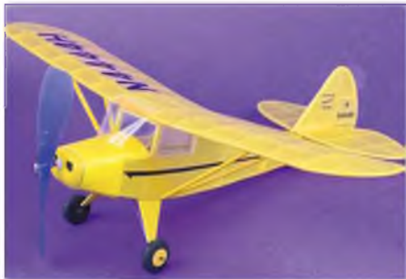
Jim Crossley Piper Vagabond. Thomas Designs's Plan, Wingspan 13cms, weighs 14grams.
