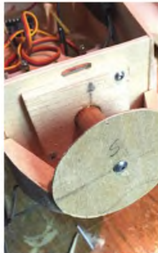
Pat's temporary spacer used to hold part N while he builds up the balsa block sections around it.
