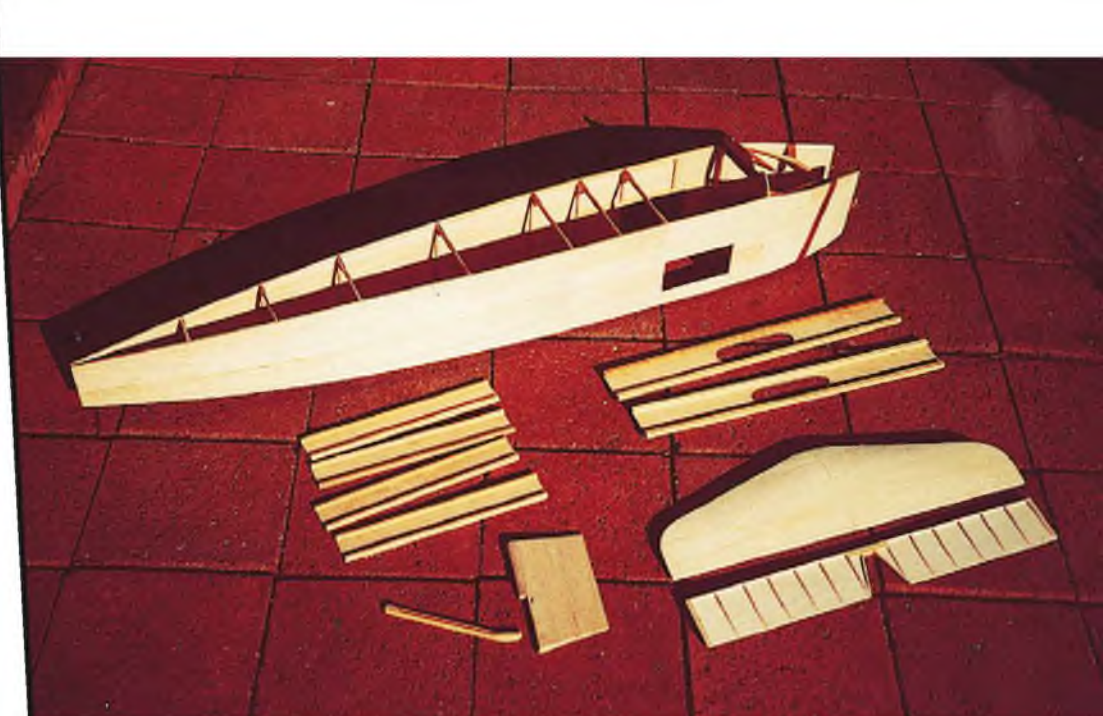
The simple box fuselage is shown here with the hole cut in the side for the central spars, which are ready to assemble. The wing joiners are also ready, together with the tailplane elevators, rudder and tail skid.
