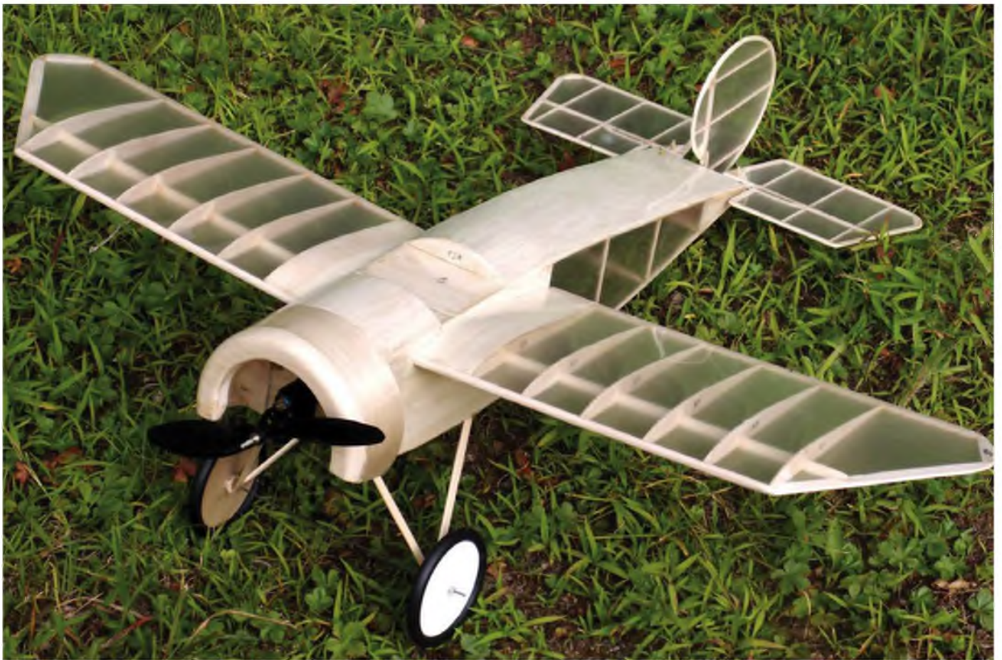
Another covering option is the document laminating film seen on this 32" span model.
