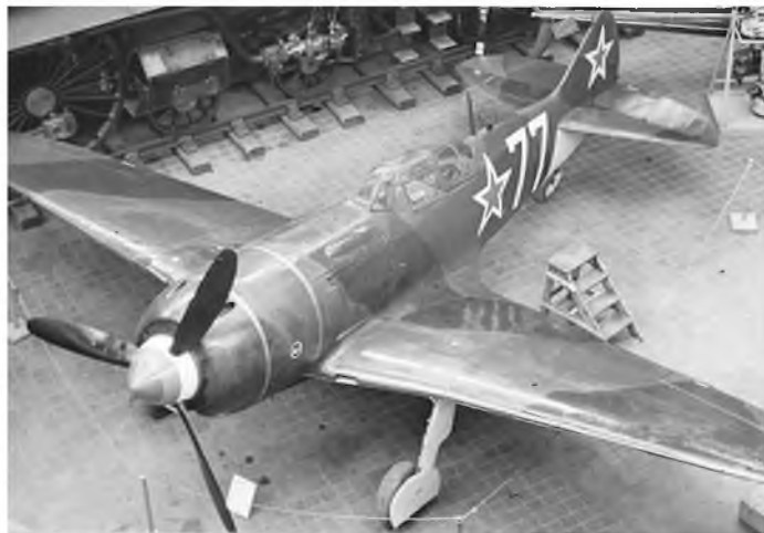
ABOVE LEFT: Near head-on view reveals the engine fan just behind the propeller, not unlike one of its primary adversary, the Focke Wulf 190A. Note also the wide track main undercarriage, ideal for the rough-field conditions from which the type operated in support of the Soviet Army in its push westward through eastern Europe. ABOVE RIGHT: Sharply tapered wings were a feature of the La-5 and La-7. All control surfaces were fabric covered.
