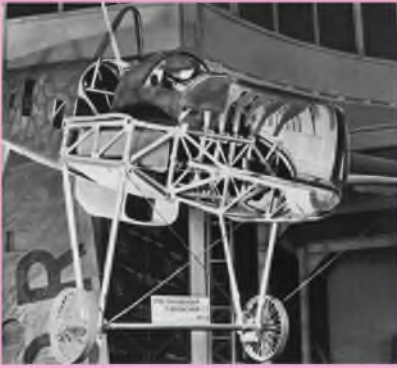
This Junkers Company photograph of the third in the series, E252/16, shows some of the modifications incorporated after tests with E252/16. The upper and side areas have also been sprayed a dark colour (dark green or brown?).
