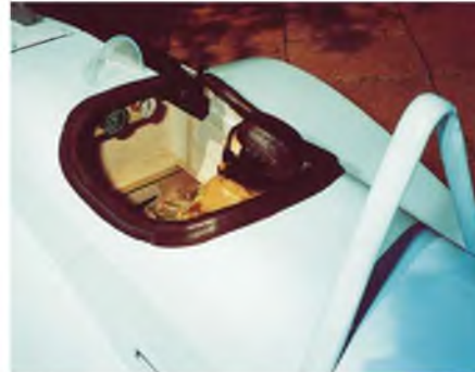
A view of the cockpit shows the cowl top in place, the windscreen cut from a clear plastic pill bottle and the leather cockpit surround.
