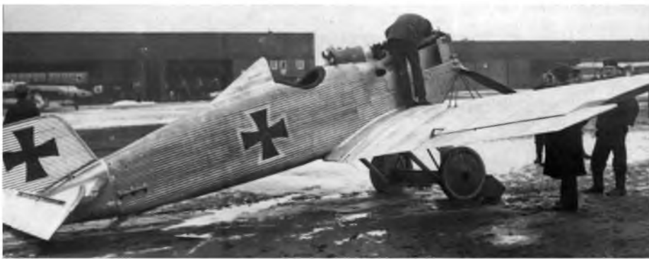
Immediate predecessor for the Junkers J.9/D.1 was the J.7, of which this is the third variant with new ailerons and revised rudder shape. See here during the January 1918 Fighter Competition at Adlershof.
