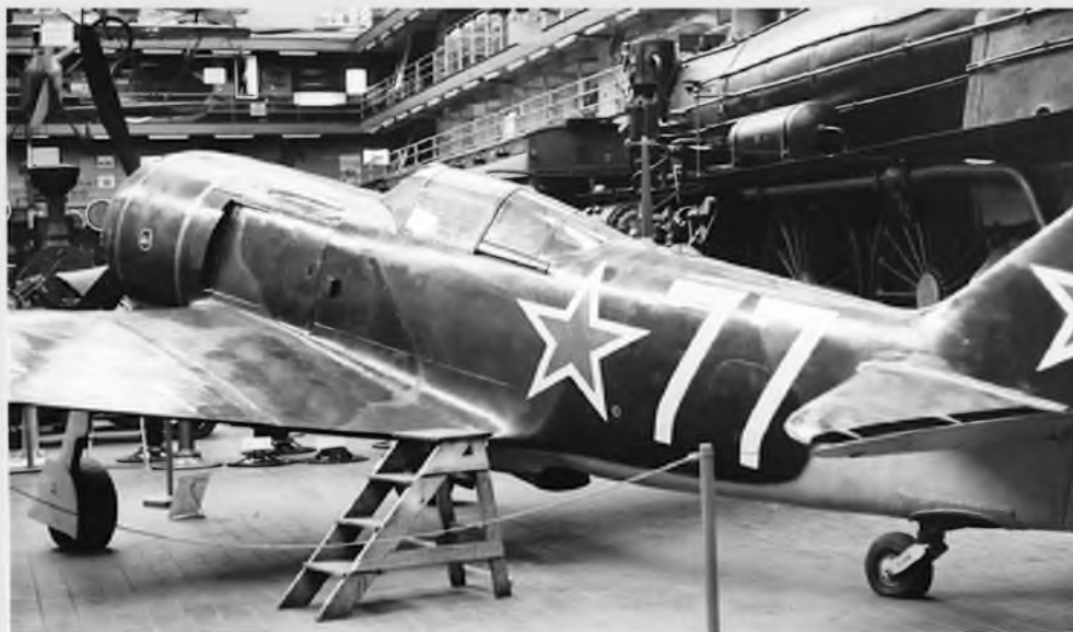
This late production Lavochkin La-7 seen at the Prague Museum in Czech Republic is a restored example. Rear three-quarter view reveals the tight wing-to-fuselage fairing and the elevator hinge arrangement. Tailwheel unit is fixed, the retraction fairing having been deleted earlier in the series to avoid problems with mud clogging the tailwheel well.
