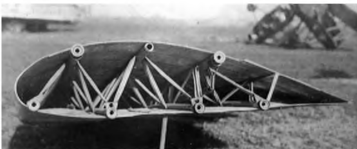
View showing the internal structure of the J.9/D.1 wing in which the thick wing section is formed by vertical diagonal braced attached to multiple upper and lower surface tubes to support the aerfoil shape.
