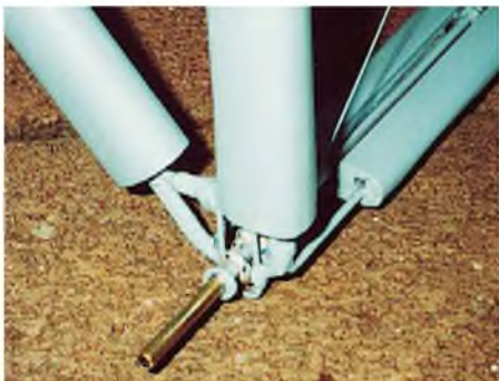
Undercarriage detail shows the wire cross-axle bound and soldered in the middle to take side loads. The ends are sprung with 3mm rubber bungee cord. The Williams wheels are retained on brass tube axle extensions with split-pins. The legs have substantial pine fairings epoxy-glued in place.
