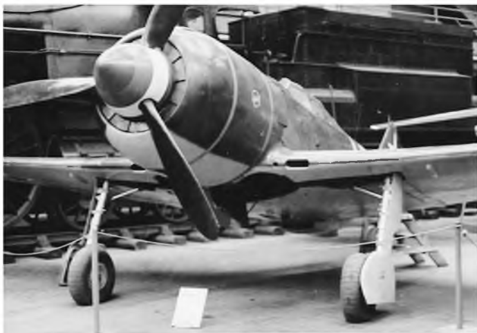
ABOVE LEFT: Near head-on view reveals the engine fan just behind the propeller, not unlike one of its primary adversary, the Focke Wulf 190A. Note also the wide track main undercarriage, ideal for the rough-field conditions from which the type operated in support of the Soviet Army in its push westward through eastern Europe. ABOVE RIGHT: Sharply tapered wings were a feature of the La-5 and La-7. All control surfaces were fabric covered.
