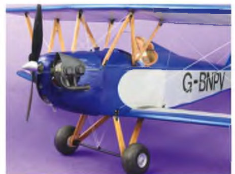
Kevin Wallace's Flybaby Biplane, 23" span, weighs 85 grams. SAMS model electroflite unit.
