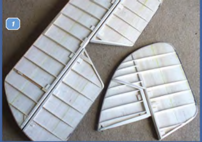
Tail surfaces made by the Eric Coates method. See text.
