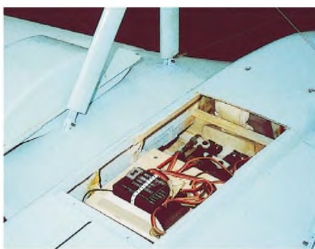
Rudder, throttle and elevator servos are located immediately behind the front spar, with the battery just forward and the receiver aft. Note the belly hatch with the dummy radiator, undercarriage attachments and drain holes from the engine compartment.
