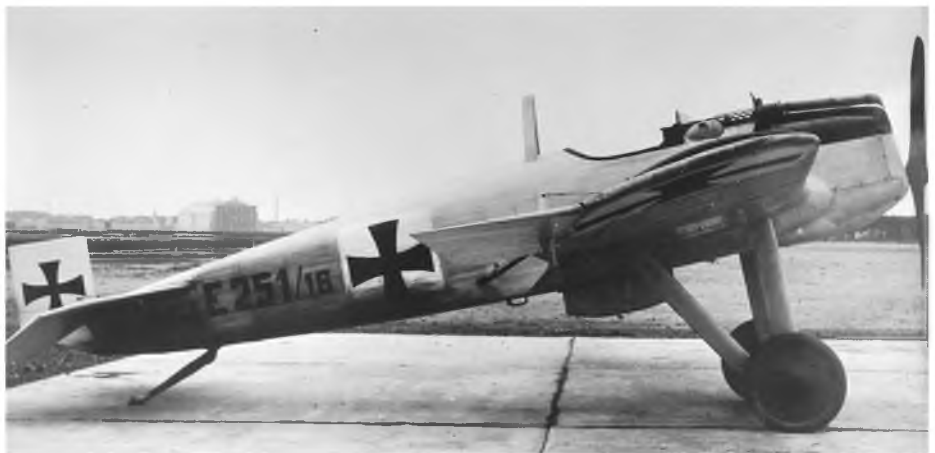
A full side profile of J.2 serial E251/16. Note the rippling of the iron skin and the very modern belly radiator.
