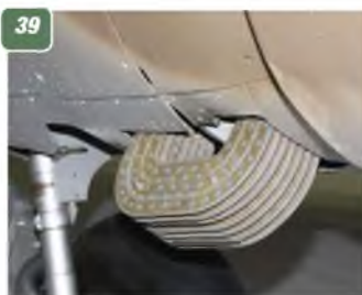
38: Retainer latches on engine cowl access panel. 39: Oil cooler positioned just behind the cowl. Position also revealed in pic. 40. 41: The forward radio aerial mast. 42: Cabin access door, right fuselage side only. 43: The long glazed cabin area. Note the deep wing-to-fuselage fairing and fairing bulge just below the cabin access door.
