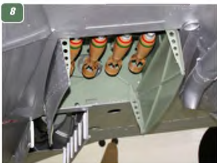
5, 6 & 7: The Avis Leonides engine that powered the Anson. 8: The central bomb bay positioned close to the wing leading edge, showing four 20 lbs. bombs. 9: Two further bomb bays are position left and right of centreline closer to the wing trailing edge. These carried larger bombs. 10: Landing light, wing leading edge. 11: Upper wing surface showing left aileron hinges and control horn. 12: Lower wing surface, showing aileron control horn. 13: Navigation light on wing. 14: Detail of the aileron control horn on wing upper surface.
