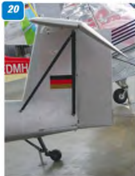
18: Cockpit interior - note rudder pedals have been demounted and are lying on cockpit floor. 19: Starboard cockpit interior. 20: General view of tail; note D-EBCQ is now fitted with a tailwheel.
