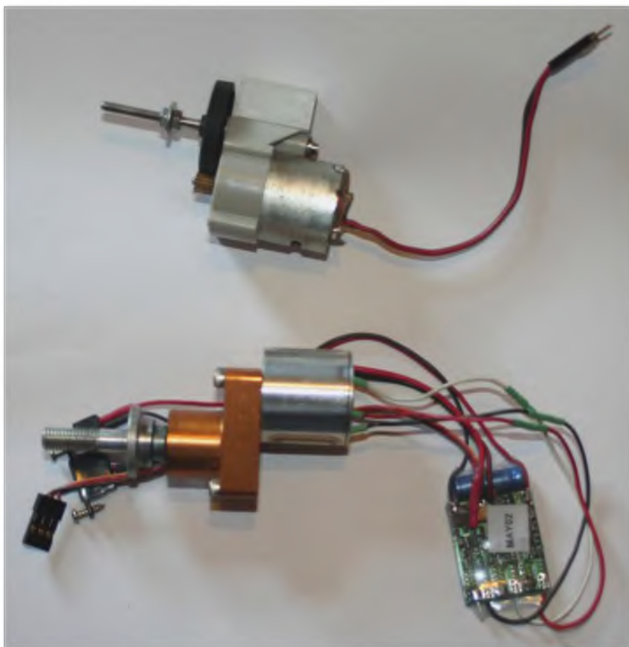
A geared, brushed motor and an old Astro geared inrunner complete with its' dedicated ESC. Believe me, that gearbox is HEAVY!!!
