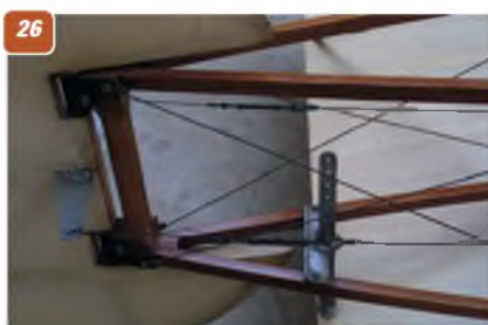
21: Detail of the propeller hub. 22: Slightly scimitar shape to the propeller. 23: Typical example of turnbuckles for adjusting the bracing wires. 24: Typical anchor point for wing bracing wires - this one on top wing surface. 25: The all-moving fin (no separate rudder) also showing the control horn. 26: Close-up detail of the rudder horn. The vertical metal post ahead of the ruder post is for adjusting the tailplane incidence. 27: Rear fuselage structure. 28: Longerons strengtheners at tailwheel mount position. 29: Typical wire bracing on rear fuselage 30: Linen covering to fuselage sides from pilot position forward. 31: Detail of typical wooden fuselage cross brace.
