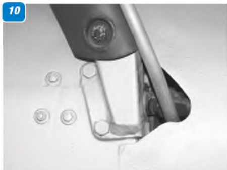
6: Aileron horn, pushrod & shroud. 7: Flap hinge (aileron hinge identical). 8: Top of oleo strut fitting to fuselage. 9: Wing strut end-fitting at underside of wing. 10: Front (starboard) cabane strut fitting at fuselage. 11: Starboard rear wing strut fitting at fuselage. 12: Upper end of cabane struts at wing centre-section. 13: Port rear cabane strut fitting showing flap actuating torque rod. 14: Starboard rear undercarriage leg fitting - note port leg fits forward of starboard leg. 15: Port undercarriage and wheel. 16: Outside face of wheel. 17: Cockpit showing throttle and flap controls.
