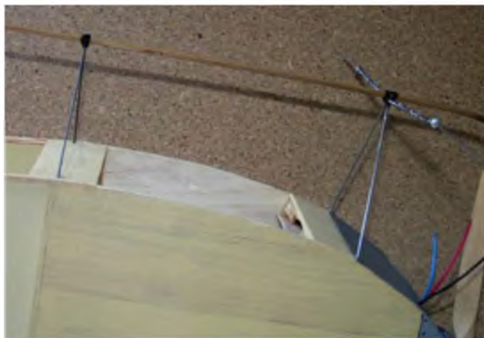
How the undercarriage wires glue in place and the bamboo skid bound and glued to them. Note the double thickness axle to help prevent flexing - it almost does the job.
