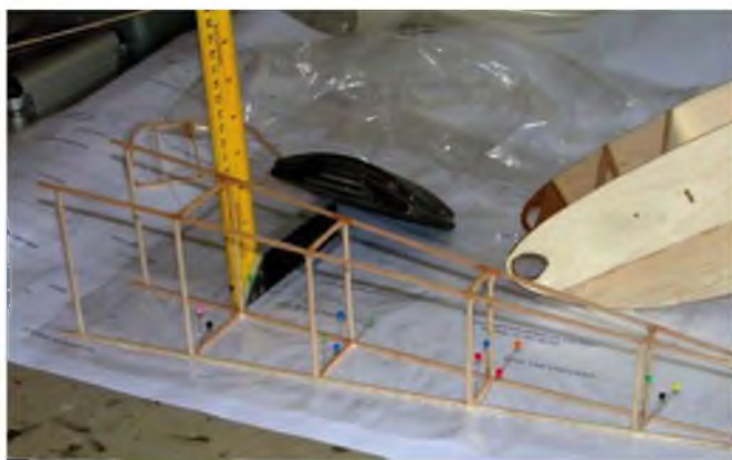
The rear fuselage frame jugged up for square and the ready assembled basic forward box ready to have the rear part attached to it.
