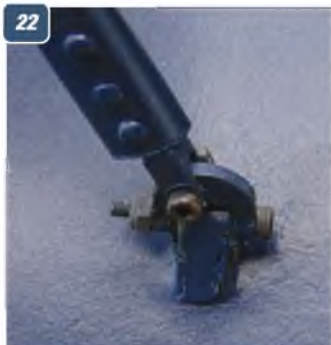
16: Headrest; note 'quitting' effect of thin ply covering. 17: Windscreen. 18: Engine and exhaust installation on removable 'power egg'. 19: Engine installation - receiver nicad and on-board glow driver behind engine. 20: Elevator horns - note one horn per elevator half. 21: Detail of rear tail strut to fuselage fitting. 22: Detail of front tail strut to fuselage fitting. 23: Detail of tailplane strut to tailplane fitting.
