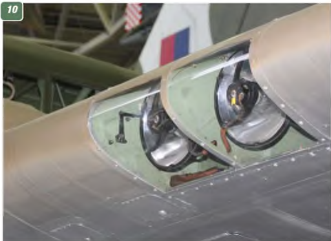
5, 6 & 7: The Avis Leonides engine that powered the Anson. 8: The central bomb bay positioned close to the wing leading edge, showing four 20 lbs. bombs. 9: Two further bomb bays are position left and right of centreline closer to the wing trailing edge. These carried larger bombs. 10: Landing light, wing leading edge. 11: Upper wing surface showing left aileron hinges and control horn. 12: Lower wing surface, showing aileron control horn. 13: Navigation light on wing. 14: Detail of the aileron control horn on wing upper surface.
