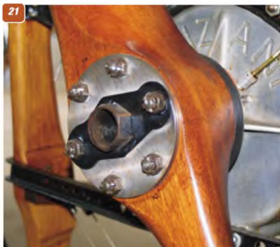
21: Detail of the propeller hub. 22: Slightly scimitar shape to the propeller. 23: Typical example of turnbuckles for adjusting the bracing wires. 24: Typical anchor point for wing bracing wires - this one on top wing surface. 25: The all-moving fin (no separate rudder) also showing the control horn. 26: Close-up detail of the rudder horn. The vertical metal post ahead of the ruder post is for adjusting the tailplane incidence. 27: Rear fuselage structure. 28: Longerons strengtheners at tailwheel mount position. 29: Typical wire bracing on rear fuselage 30: Linen covering to fuselage sides from pilot position forward. 31: Detail of typical wooden fuselage cross brace.
