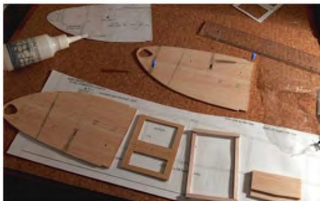
Although actually from a larger model, the forward fuselage parts remain much the same. Note the laminated former that sets the dihedral.
