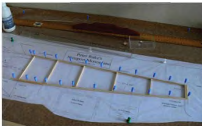
Rear fuselage frame is built in the time honoured fashion, and the second frame built over the first to ensure they are identical.
