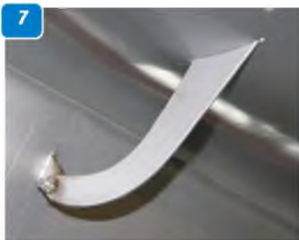
6: Aileron horn, pushrod & shroud. 7: Flap hinge (aileron hinge identical). 8: Top of oleo strut fitting to fuselage. 9: Wing strut end-fitting at underside of wing. 10: Front (starboard) cabane strut fitting at fuselage. 11: Starboard rear wing strut fitting at fuselage. 12: Upper end of cabane struts at wing centre-section. 13: Port rear cabane strut fitting showing flap actuating torque rod. 14: Starboard rear undercarriage leg fitting - note port leg fits forward of starboard leg. 15: Port undercarriage and wheel. 16: Outside face of wheel. 17: Cockpit showing throttle and flap controls.
