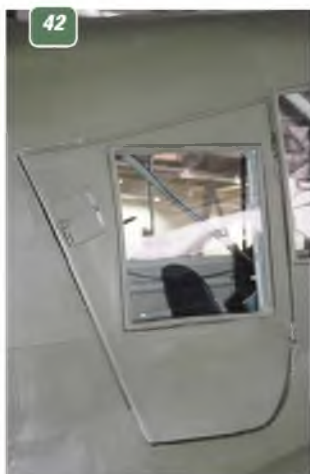
38: Retainer latches on engine cowl access panel. 39: Oil cooler positioned just behind the cowl. Position also revealed in pic. 40. 41: The forward radio aerial mast. 42: Cabin access door, right fuselage side only. 43: The long glazed cabin area. Note the deep wing-to-fuselage fairing and fairing bulge just below the cabin access door.
