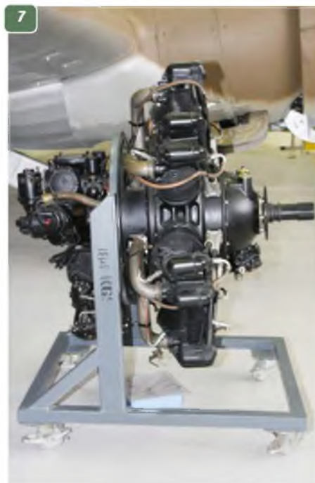
5, 6 & 7: The Avis Leonides engine that powered the Anson. 8: The central bomb bay positioned close to the wing leading edge, showing four 20 lbs. bombs. 9: Two further bomb bays are position left and right of centreline closer to the wing trailing edge. These carried larger bombs. 10: Landing light, wing leading edge. 11: Upper wing surface showing left aileron hinges and control horn. 12: Lower wing surface, showing aileron control horn. 13: Navigation light on wing. 14: Detail of the aileron control horn on wing upper surface.
