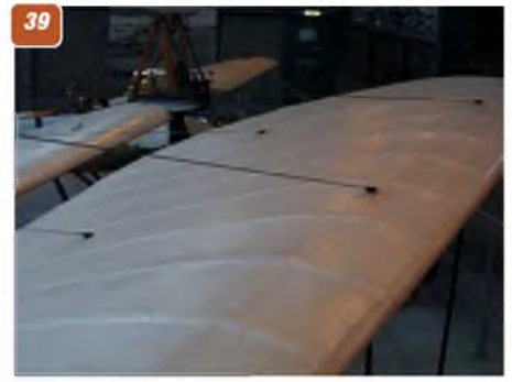
37: Wing leading edge. 38: Wing underside wire brace anchor point. 39: Wire braces on wing upper surface. 40: Anchor point for main undercarriage brace strut. 41: The left undercarriage leg. 42: Detail of upper main undercarriage support. 43: Close-up of the attachment for the castoring mainwheel. 44: Close-up of the bungee cord undercarriage shock absorbers. 45: The full main undercarriage shock absorber, top mount of which is detailed in 46. 47: Detail of cast metal spacer on the front vertical mainwheel fork. 48: Mainwheel unit and castor. 49: Another view of the main wheels, showing the metal vertical and horizontal fork braces.
