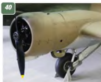
38: Retainer latches on engine cowl access panel. 39: Oil cooler positioned just behind the cowl. Position also revealed in pic. 40. 41: The forward radio aerial mast. 42: Cabin access door, right fuselage side only. 43: The long glazed cabin area. Note the deep wing-to-fuselage fairing and fairing bulge just below the cabin access door.
