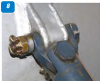
6: Aileron horn, pushrod & shroud. 7: Flap hinge (aileron hinge identical). 8: Top of oleo strut fitting to fuselage. 9: Wing strut end-fitting at underside of wing. 10: Front (starboard) cabane strut fitting at fuselage. 11: Starboard rear wing strut fitting at fuselage. 12: Upper end of cabane struts at wing centre-section. 13: Port rear cabane strut fitting showing flap actuating torque rod. 14: Starboard rear undercarriage leg fitting - note port leg fits forward of starboard leg. 15: Port undercarriage and wheel. 16: Outside face of wheel. 17: Cockpit showing throttle and flap controls.
