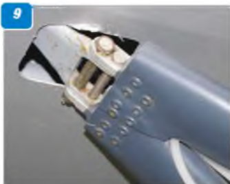
6: Aileron horn, pushrod & shroud. 7: Flap hinge (aileron hinge identical). 8: Top of oleo strut fitting to fuselage. 9: Wing strut end-fitting at underside of wing. 10: Front (starboard) cabane strut fitting at fuselage. 11: Starboard rear wing strut fitting at fuselage. 12: Upper end of cabane struts at wing centre-section. 13: Port rear cabane strut fitting showing flap actuating torque rod. 14: Starboard rear undercarriage leg fitting - note port leg fits forward of starboard leg. 15: Port undercarriage and wheel. 16: Outside face of wheel. 17: Cockpit showing throttle and flap controls.
