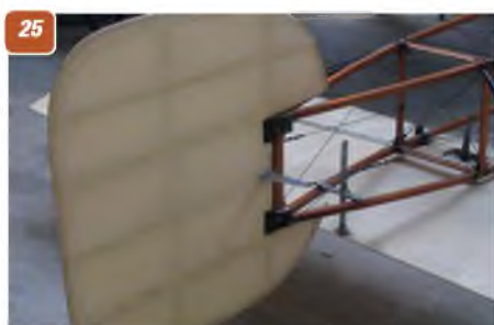
21: Detail of the propeller hub. 22: Slightly scimitar shape to the propeller. 23: Typical example of turnbuckles for adjusting the bracing wires. 24: Typical anchor point for wing bracing wires - this one on top wing surface. 25: The all-moving fin (no separate rudder) also showing the control horn. 26: Close-up detail of the rudder horn. The vertical metal post ahead of the ruder post is for adjusting the tailplane incidence. 27: Rear fuselage structure. 28: Longerons strengtheners at tailwheel mount position. 29: Typical wire bracing on rear fuselage 30: Linen covering to fuselage sides from pilot position forward. 31: Detail of typical wooden fuselage cross brace.
