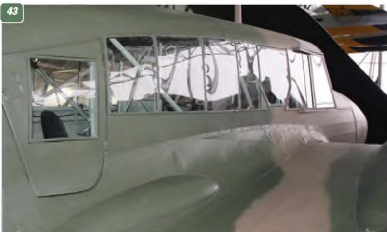
38: Retainer latches on engine cowl access panel. 39: Oil cooler positioned just behind the cowl. Position also revealed in pic. 40. 41: The forward radio aerial mast. 42: Cabin access door, right fuselage side only. 43: The long glazed cabin area. Note the deep wing-to-fuselage fairing and fairing bulge just below the cabin access door.
