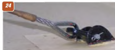
21: Detail of the propeller hub. 22: Slightly scimitar shape to the propeller. 23: Typical example of turnbuckles for adjusting the bracing wires. 24: Typical anchor point for wing bracing wires - this one on top wing surface. 25: The all-moving fin (no separate rudder) also showing the control horn. 26: Close-up detail of the rudder horn. The vertical metal post ahead of the ruder post is for adjusting the tailplane incidence. 27: Rear fuselage structure. 28: Longerons strengtheners at tailwheel mount position. 29: Typical wire bracing on rear fuselage 30: Linen covering to fuselage sides from pilot position forward. 31: Detail of typical wooden fuselage cross brace.
