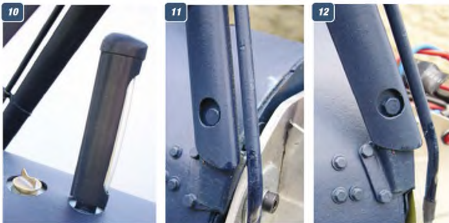
10: Fuel sight gauge and filler cap. 11: Front cabane strut fuselage fitting. 12: Front cabane strut fuselage fitting.
