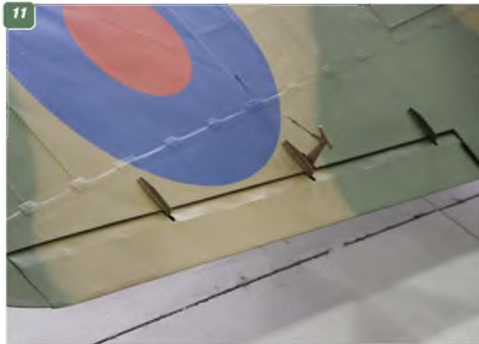
5, 6 & 7: The Avis Leonides engine that powered the Anson. 8: The central bomb bay positioned close to the wing leading edge, showing four 20 lbs. bombs. 9: Two further bomb bays are position left and right of centreline closer to the wing trailing edge. These carried larger bombs. 10: Landing light, wing leading edge. 11: Upper wing surface showing left aileron hinges and control horn. 12: Lower wing surface, showing aileron control horn. 13: Navigation light on wing. 14: Detail of the aileron control horn on wing upper surface.
