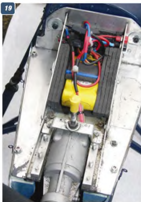
16: Headrest; note 'quitting' effect of thin ply covering. 17: Windscreen. 18: Engine and exhaust installation on removable 'power egg'. 19: Engine installation - receiver nicad and on-board glow driver behind engine. 20: Elevator horns - note one horn per elevator half. 21: Detail of rear tail strut to fuselage fitting. 22: Detail of front tail strut to fuselage fitting. 23: Detail of tailplane strut to tailplane fitting.
