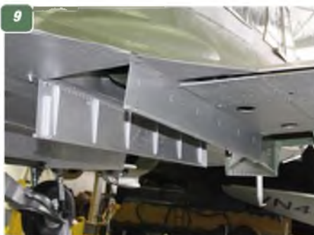
5, 6 & 7: The Avis Leonides engine that powered the Anson. 8: The central bomb bay positioned close to the wing leading edge, showing four 20 lbs. bombs. 9: Two further bomb bays are position left and right of centreline closer to the wing trailing edge. These carried larger bombs. 10: Landing light, wing leading edge. 11: Upper wing surface showing left aileron hinges and control horn. 12: Lower wing surface, showing aileron control horn. 13: Navigation light on wing. 14: Detail of the aileron control horn on wing upper surface.
