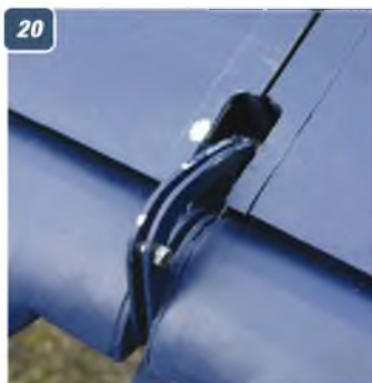
16: Headrest; note 'quitting' effect of thin ply covering. 17: Windscreen. 18: Engine and exhaust installation on removable 'power egg'. 19: Engine installation - receiver nicad and on-board glow driver behind engine. 20: Elevator horns - note one horn per elevator half. 21: Detail of rear tail strut to fuselage fitting. 22: Detail of front tail strut to fuselage fitting. 23: Detail of tailplane strut to tailplane fitting.
