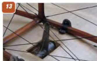
4: Rim of the cockpit. 5: One arm of the wooden rudder bar on the front 'floor' of the cockpit well. 6: The manually operated pump to the fuel tank looking from a position ahead of the cockpit area. Pump is mounted on the right hand cockpit edge and also seen from the pilot's position in picture 7 : Tank needs to be regularly pumped during flight. 8: Ignition switch in left hand upper corner of cockpit. 9: Fuel gauge - left hand side of fuel tank tank. 10: The front truss above the fuselage ahead of the cockpit, for the wing bracing wires. Rear truss seen in pic 11 . 12: The tailplane, showing metal bracing and 'all-flying' elevator outer panel. 13: Elevator control horn and the barckets that secure the tailplane to the fuselage longerons.
