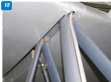
6: Aileron horn, pushrod & shroud. 7: Flap hinge (aileron hinge identical). 8: Top of oleo strut fitting to fuselage. 9: Wing strut end-fitting at underside of wing. 10: Front (starboard) cabane strut fitting at fuselage. 11: Starboard rear wing strut fitting at fuselage. 12: Upper end of cabane struts at wing centre-section. 13: Port rear cabane strut fitting showing flap actuating torque rod. 14: Starboard rear undercarriage leg fitting - note port leg fits forward of starboard leg. 15: Port undercarriage and wheel. 16: Outside face of wheel. 17: Cockpit showing throttle and flap controls.
