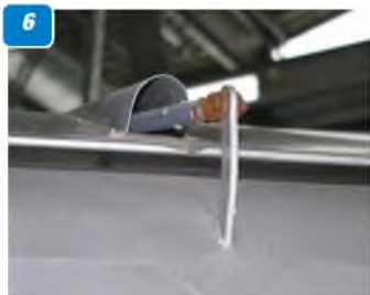
6: Aileron horn, pushrod & shroud. 7: Flap hinge (aileron hinge identical). 8: Top of oleo strut fitting to fuselage. 9: Wing strut end-fitting at underside of wing. 10: Front (starboard) cabane strut fitting at fuselage. 11: Starboard rear wing strut fitting at fuselage. 12: Upper end of cabane struts at wing centre-section. 13: Port rear cabane strut fitting showing flap actuating torque rod. 14: Starboard rear undercarriage leg fitting - note port leg fits forward of starboard leg. 15: Port undercarriage and wheel. 16: Outside face of wheel. 17: Cockpit showing throttle and flap controls.
