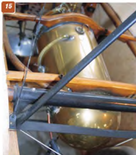
14 & 15: The brass fuel tank mounted ahead of the cockpit. 16 & 17: Two views of the three cylinder Anzani engine installation. 18: Close-up of the metal engine mounting brackets. 19: Underside of the fuselage below the pilot's position showing pulley guides for control wires leading to rear control surfaces. Vertical wires lead down to the wing warp mechanism, braces to which are the angled metal tubes also in view. 20: The wing warp mechanism below the fuselage. Vertical wires lead up to the control column, others to the outer wings.
