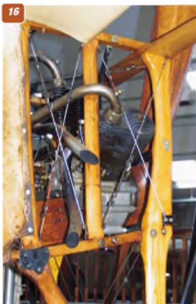
14 & 15: The brass fuel tank mounted ahead of the cockpit. 16 & 17: Two views of the three cylinder Anzani engine installation. 18: Close-up of the metal engine mounting brackets. 19: Underside of the fuselage below the pilot's position showing pulley guides for control wires leading to rear control surfaces. Vertical wires lead down to the wing warp mechanism, braces to which are the angled metal tubes also in view. 20: The wing warp mechanism below the fuselage. Vertical wires lead up to the control column, others to the outer wings.
