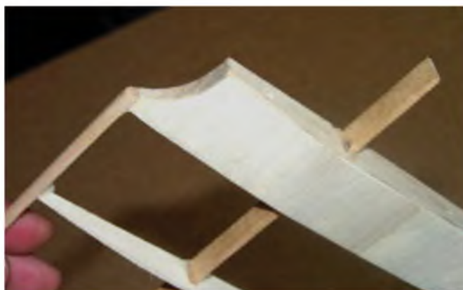
A wing root showing the sheeting in place and that optional leading edge cut-out.
