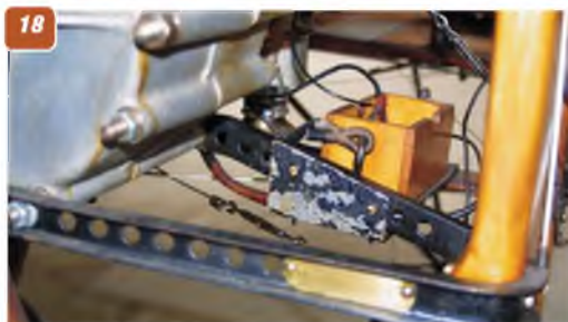
14 & 15: The brass fuel tank mounted ahead of the cockpit. 16 & 17: Two views of the three cylinder Anzani engine installation. 18: Close-up of the metal engine mounting brackets. 19: Underside of the fuselage below the pilot's position showing pulley guides for control wires leading to rear control surfaces. Vertical wires lead down to the wing warp mechanism, braces to which are the angled metal tubes also in view. 20: The wing warp mechanism below the fuselage. Vertical wires lead up to the control column, others to the outer wings.
