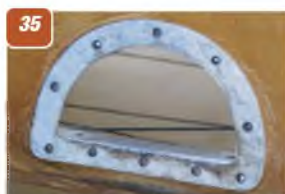
32: Tailwheel. This one is steerable and non-authentic, although structure is basically correct. Modification by Shuttleworth makes aircraft easier to handle. 33: Detail of the steering linkage. 34: Coil sprung tailwheel strut. 35: Foot stirrup on the left side of the fuselage behind the wing. 36: View down the fuselage from the front.
