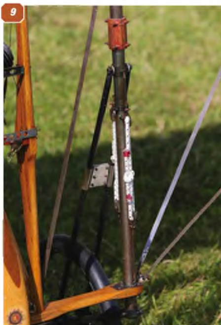
5: Ultra thin undercambered section is apparent in this view. Note engine right on leading edge. 6: A great shot for all stirrup and step fanciers. 7: Don used the core element of the Mick Reeves Models dummy engine to make up the Anzani. 8: I defy you to tell this from the original. 9: Undercarriage faithfully models the original. Note bungees and their terminations. 10: The magnificent dummy engine is based around Mick Reeves Models core parts with Don's additions.
