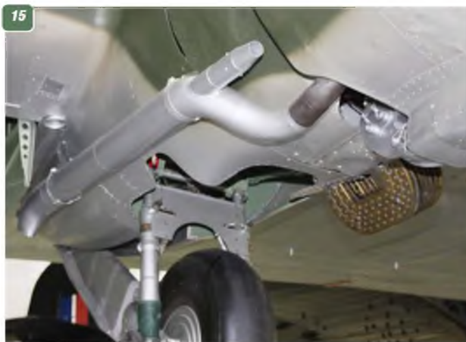
15: Exhaust damper on right side engine, also showing the undercarriage leg and oil cooler.
