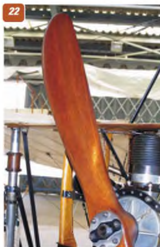
21: Detail of the propeller hub. 22: Slightly scimitar shape to the propeller. 23: Typical example of turnbuckles for adjusting the bracing wires. 24: Typical anchor point for wing bracing wires - this one on top wing surface. 25: The all-moving fin (no separate rudder) also showing the control horn. 26: Close-up detail of the rudder horn. The vertical metal post ahead of the ruder post is for adjusting the tailplane incidence. 27: Rear fuselage structure. 28: Longerons strengtheners at tailwheel mount position. 29: Typical wire bracing on rear fuselage 30: Linen covering to fuselage sides from pilot position forward. 31: Detail of typical wooden fuselage cross brace.
