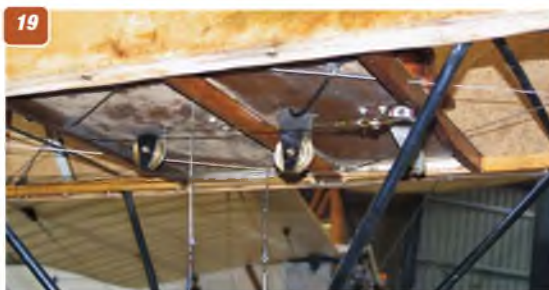
14 & 15: The brass fuel tank mounted ahead of the cockpit. 16 & 17: Two views of the three cylinder Anzani engine installation. 18: Close-up of the metal engine mounting brackets. 19: Underside of the fuselage below the pilot's position showing pulley guides for control wires leading to rear control surfaces. Vertical wires lead down to the wing warp mechanism, braces to which are the angled metal tubes also in view. 20: The wing warp mechanism below the fuselage. Vertical wires lead up to the control column, others to the outer wings.
