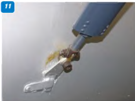
6: Aileron horn, pushrod & shroud. 7: Flap hinge (aileron hinge identical). 8: Top of oleo strut fitting to fuselage. 9: Wing strut end-fitting at underside of wing. 10: Front (starboard) cabane strut fitting at fuselage. 11: Starboard rear wing strut fitting at fuselage. 12: Upper end of cabane struts at wing centre-section. 13: Port rear cabane strut fitting showing flap actuating torque rod. 14: Starboard rear undercarriage leg fitting - note port leg fits forward of starboard leg. 15: Port undercarriage and wheel. 16: Outside face of wheel. 17: Cockpit showing throttle and flap controls.
