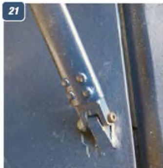
16: Headrest; note 'quitting' effect of thin ply covering. 17: Windscreen. 18: Engine and exhaust installation on removable 'power egg'. 19: Engine installation - receiver nicad and on-board glow driver behind engine. 20: Elevator horns - note one horn per elevator half. 21: Detail of rear tail strut to fuselage fitting. 22: Detail of front tail strut to fuselage fitting. 23: Detail of tailplane strut to tailplane fitting.
