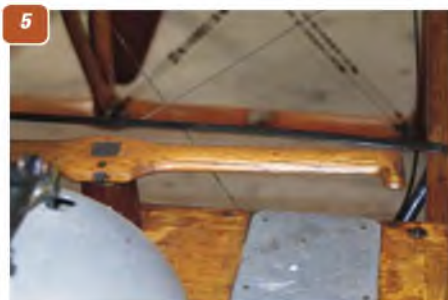
4: Rim of the cockpit. 5: One arm of the wooden rudder bar on the front 'floor' of the cockpit well. 6: The manually operated pump to the fuel tank looking from a position ahead of the cockpit area. Pump is mounted on the right hand cockpit edge and also seen from the pilot's position in picture 7 : Tank needs to be regularly pumped during flight. 8: Ignition switch in left hand upper corner of cockpit. 9: Fuel gauge - left hand side of fuel tank tank. 10: The front truss above the fuselage ahead of the cockpit, for the wing bracing wires. Rear truss seen in pic 11 . 12: The tailplane, showing metal bracing and 'all-flying' elevator outer panel. 13: Elevator control horn and the barckets that secure the tailplane to the fuselage longerons.
