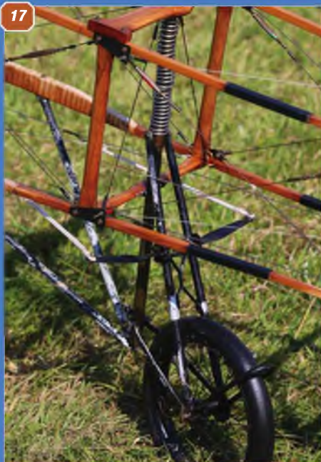
17 & 18: Rear undercarriage springing arrangements.
