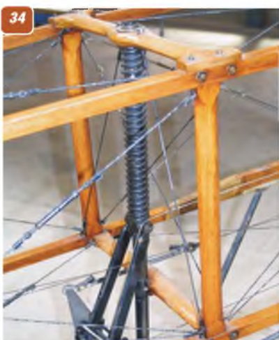
32: Tailwheel. This one is steerable and non-authentic, although structure is basically correct. Modification by Shuttleworth makes aircraft easier to handle. 33: Detail of the steering linkage. 34: Coil sprung tailwheel strut. 35: Foot stirrup on the left side of the fuselage behind the wing. 36: View down the fuselage from the front.
