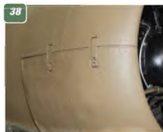
37: Air intake fairing in bottom of engine cowl.
