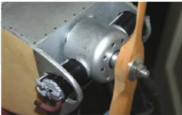
A suitably drilled bottle cap and commercial cylinders not only provide a dummy engine but also add a little nose weight.
