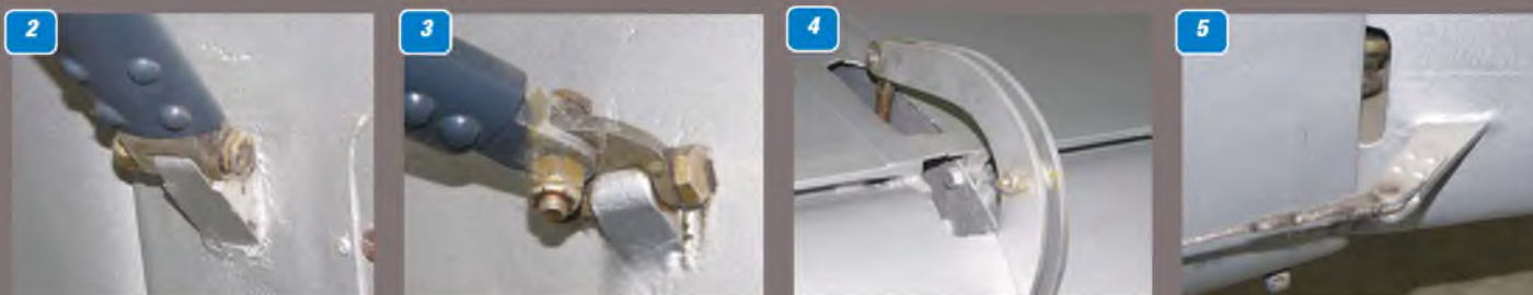
1: Top view of D-EBCQ. 2: Rear tailplane strut-to-fuselage fitting. 3: Front tailplane strut-to-fuselage fitting. 4: Elevator horn; note one horn per elevator half. 5: Rudder control horn and lower hinge.
