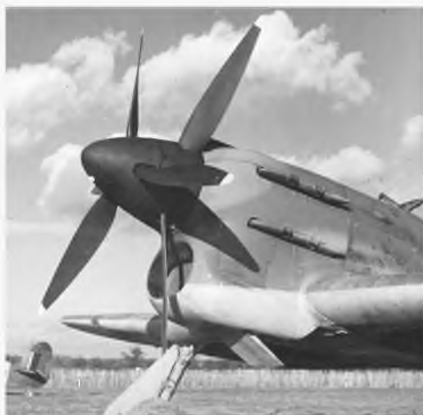
Both Typhoon and Tornado were subject to some pretty outlandish experimental installations during development. This example is the 2nd prototype Tornado with a six-blade contra-prop installation.
