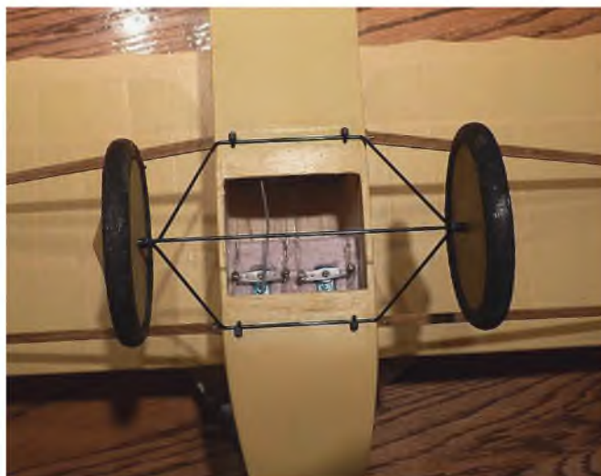
Just how tidy the underside can look if the landing gear is fitted after the lower fuselage is covered.
