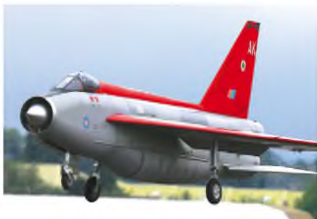
Dave Johnson flew this 4.1 metre span twin-turbine EE Lightning. Twin Jetcat P120s, weighs 88lbs.
