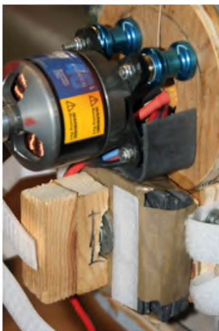
A close up of the battery mount with wood block spacer and Velcro grip strips. Note also the significant amount of lead behind the battery mount and wrapped around the lower standoffs.
