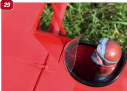
29 Detail of aileron push-rod and cockpit coaming.
