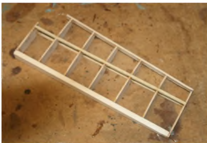
One of the tailplane halves first stage assembly before skinning.
