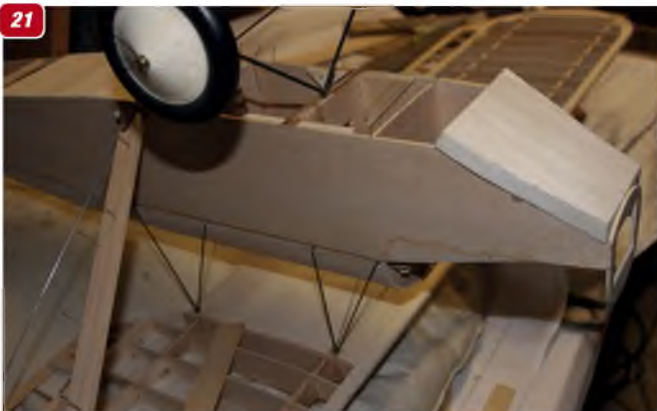
21: Front of fuselage showing basic wire undercarriage members and bottom balsa block. Wing strut has wood fairing in place.
