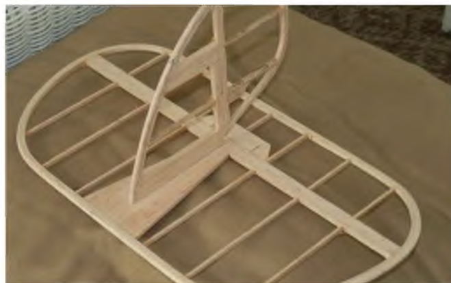
All sanded and with the edges rounded off the tail surfaces are test assembled. Control surfaces are yet to be separated.
