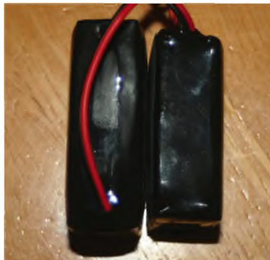
TOP LEFT: Costing about £100 and bought for a specific model this pack hasn't been used since. Why I don't buy high tech packs any more. TOP RIGHT: Sometimes it's more convenient to use two single cells wired in series than a 2S pack. Capable of 40 amp draw but fitted to a model only drawing 20 amps. ABOVE LEFT: A typical helicopter pack. Note the quoted C rating clearly shown, ample for most small models. ABOVE RIGHT: Two very similar packs, but notice the more rounded appearance of one. This puffy pack is destined for the bin.
