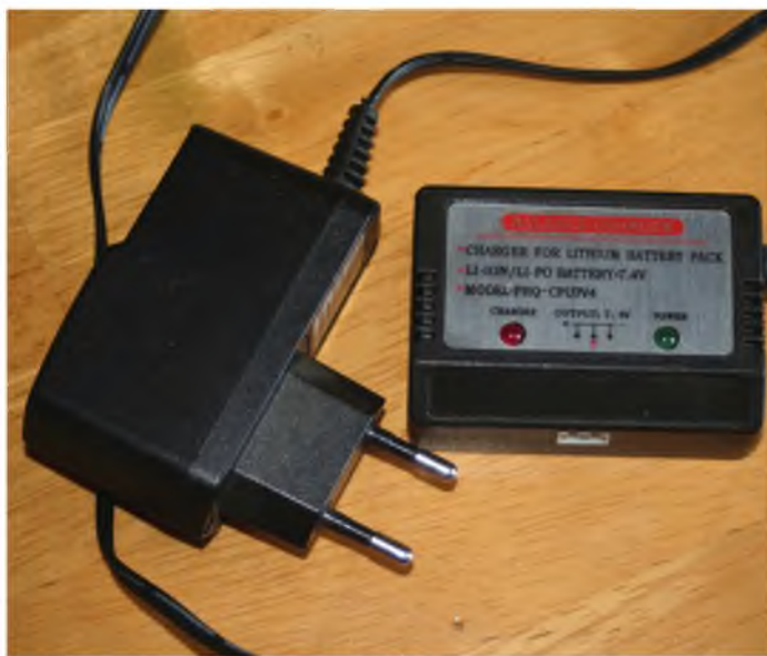
The more common type of heli charger with just power and charge lights. Still a balance charger though.
