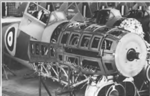
The powerful and heavy Napier Sabre engine used by the Typhoon required a suitably tough and heavy mounting. Also revealed here, is the 'car-door' cockpit access applied to the early Typhoons.
