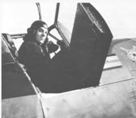
The Typhoon 1A featured this 'car door' access similar to that also applied to the Bell P-39 Airacobra. In the cockpit is Wing Commander Roland Beamont, a great exponent of the Typhoon and later, a celebrated test pilot.
