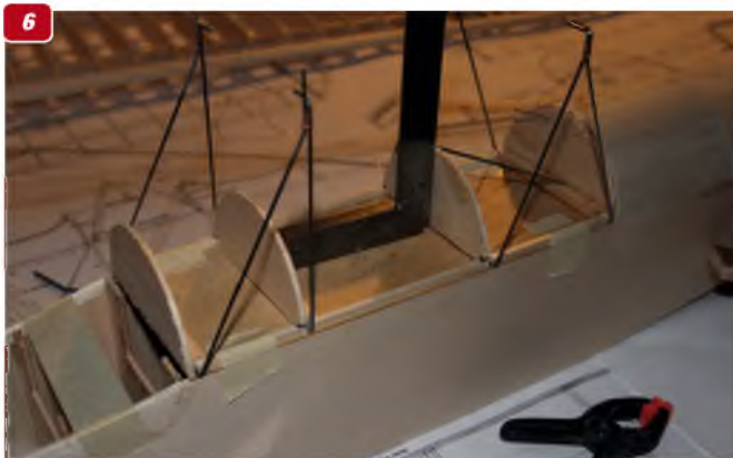
4: The basic balsa box fuselage, built inverted over the plan. 5: Front end of the basic fuselage. 6: Wire entre section wing struts, prior to addition of streamline wood fairings. 7: Sheet balsa ready to roll over the fuselage decking (see also Picture 8).
