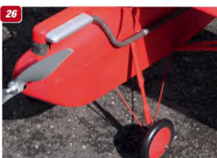
26 Nose section, showing dummy scale exhaust and main undercarriage.
