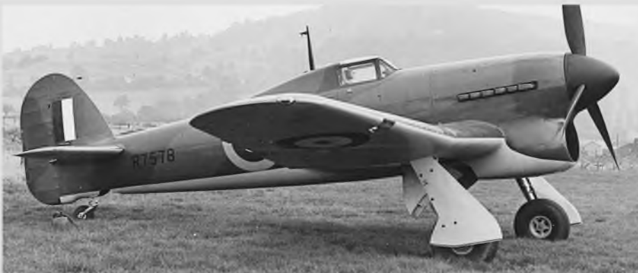
This is the third production Typhoon, fresh from the factory in June 1941. The fin and rudder are now much larger, but that rear cockpit fairing blanks off the pilot's rear view completely.
