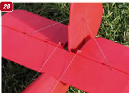
28 Tail section, showing rigging and close-loop elevator control wires.
