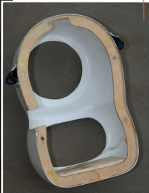
A view of the completed cowl, showing the inset former glued in place, the retaining screw holes and the thick balsa sheet fitted in the bottom to strengthen the cowl - in the case of noseovers!
