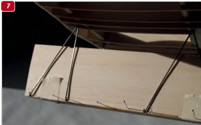
4: The basic balsa box fuselage, built inverted over the plan. 5: Front end of the basic fuselage. 6: Wire entre section wing struts, prior to addition of streamline wood fairings. 7: Sheet balsa ready to roll over the fuselage decking (see also Picture 8).
