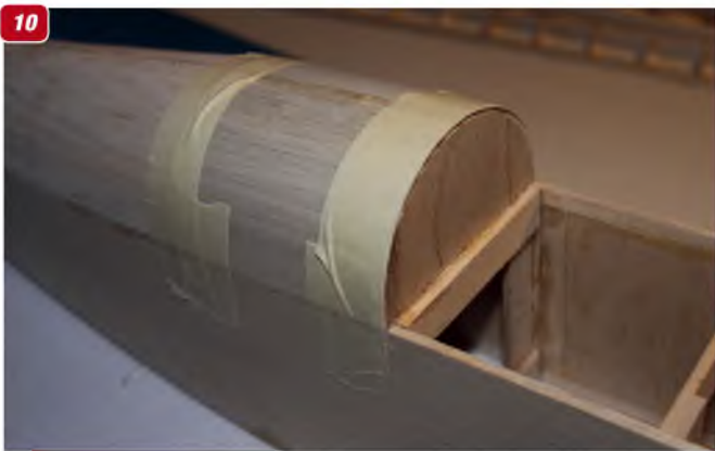
10: The sheet balsa rear top decking, in place, rolled over the upper fuselage formers and held in place with masking tape. 11: The fin and tailplane mount.
