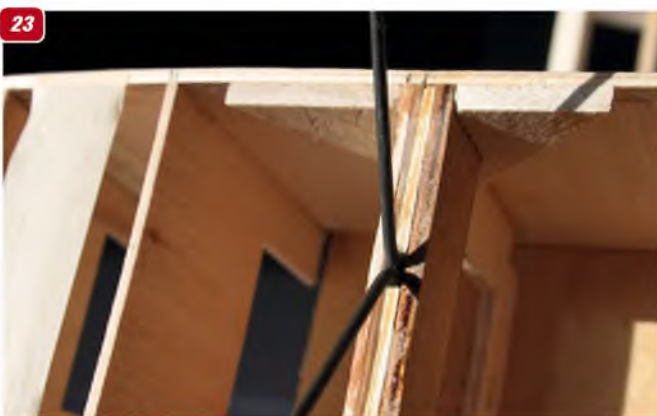
23: The anchor point for the wire main undercarriage, secured between laminations of the fuselage former.
