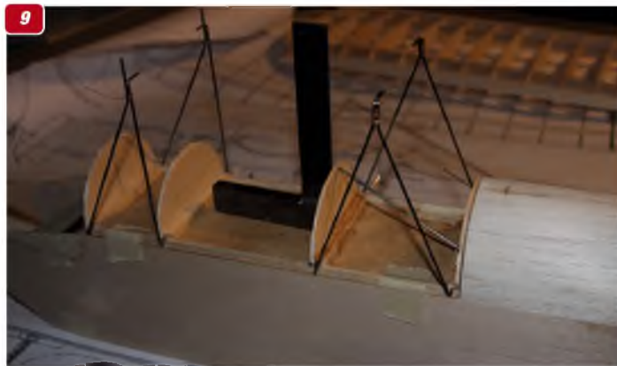
8: The sheet balsa covering in place, ready to roll over the fuselage upper structure. 9: Another view of the basic wire wing support struts, prior to adding the balsa fairings, that go on later.
