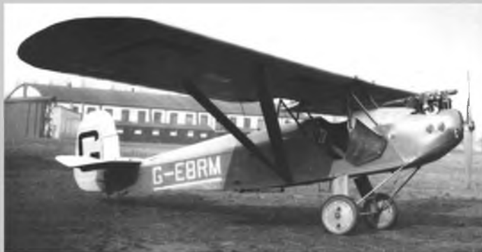
Westland Widgeon III G-EBRM in its original form, with wooden fuselage, Cirrus III and original undercarriage.
