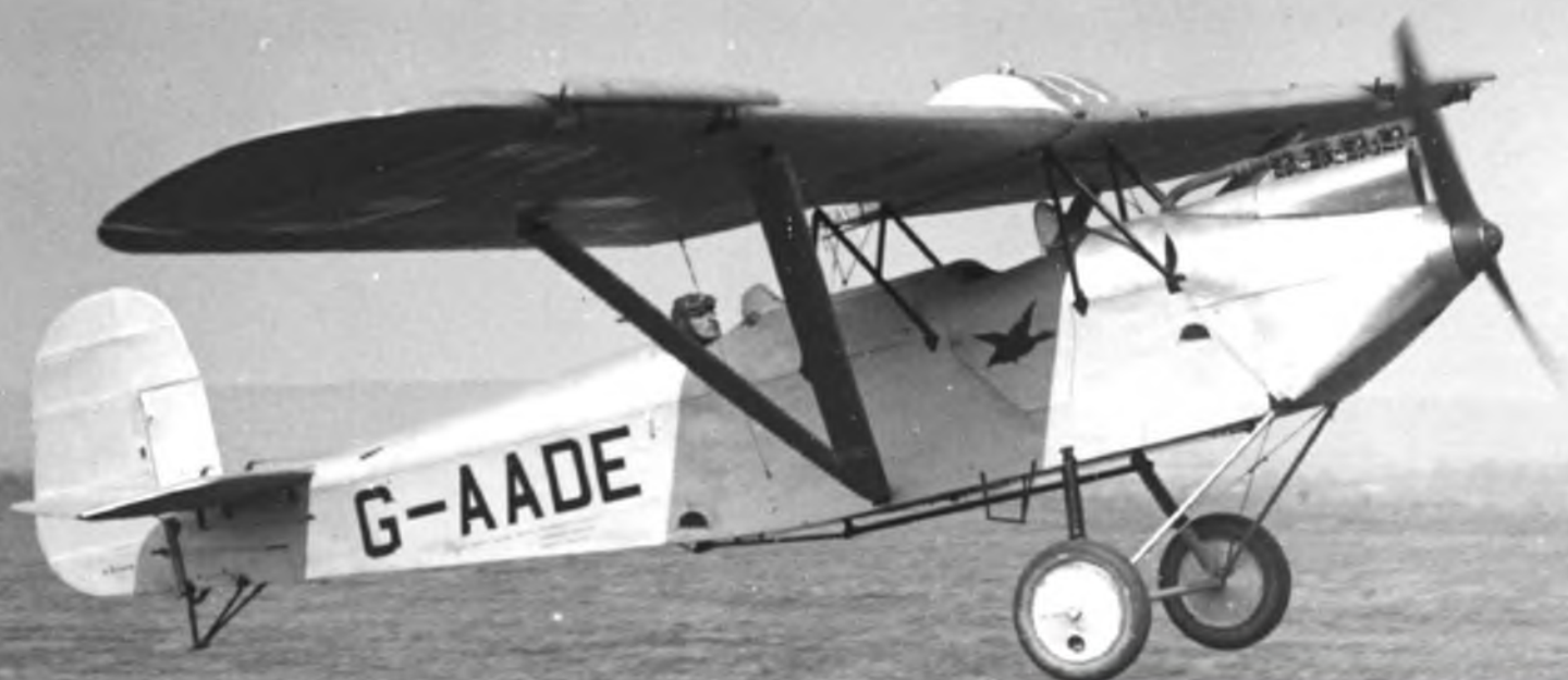
The Gipsy I engined Widgeon III G-AADE displaying its fully opened leading edge slats prior to a perfect three-point. It crashed at Beaulieu, Hampshire in July 1932.
