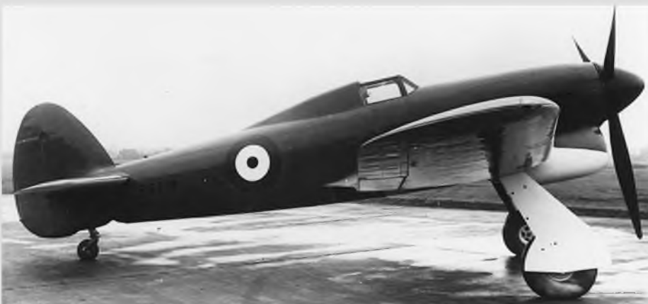
Typhoon prototype P5212, showing the small fin & rudder shape that proved quite inadequate and which was quickly changed. Equally unacceptable to anyone who had to take the type into combat was the 'solid' rear cockpit fairing that killed the rearward view from the cockpit. Whatever was the designer thinking of - did they actually talk to pilots at the sharp end of the war?
