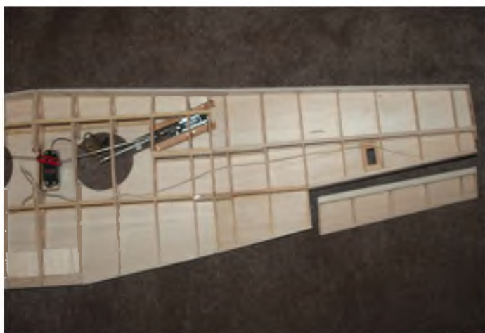
Lower wing sheeting complete starboard side, showing aileron and servo mounting plate. Note also piece of string taped in place to allow servo lead to be drawn through after covering/finishing.
