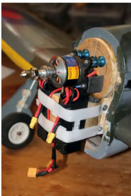
The finalised EP outrunner installation with twin Lipos underneath. Note ply disc used to extend length of standoffs. Also note the battery connectors as originally configured - unsafe! (see main text).
