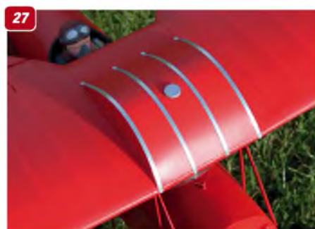
27 Wing centre section showing dummy fuel tank. Note filler cap.
