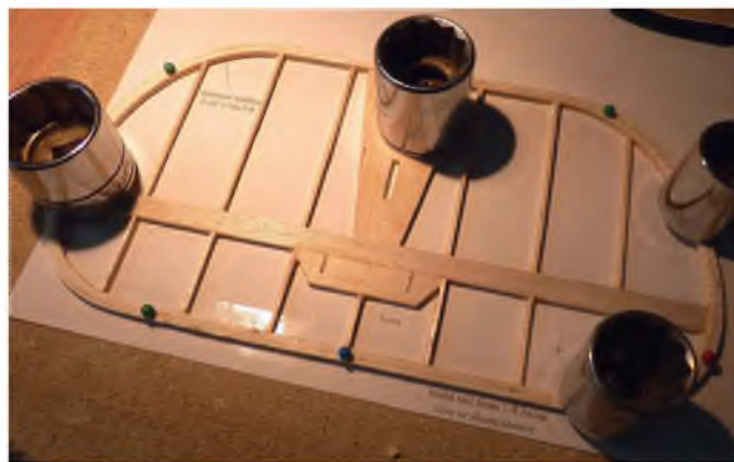
With the outline dry the tailplane/elevator assembly is very straightforward.
