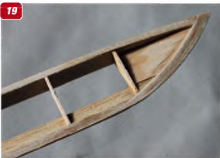
12: Wing ribs being slipped onto spars. 13: The basic wing structure of ribs, spars, leading and trailing edges. 14: Wing tip added. 15: Wing centre section with centre ribs spaced for the dummy fuel tank. 16: Wing tip, laminated from balsa strip. 17: The finished wing tip with leading edge sanded to shape, viewed from the underside. 18: Laminated tip of aileron. 19: Aileron tip after final shaping. 20: One of the wing support struts, now with laminated balsa fairing over the basic wire.
