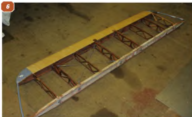
6: The complete, fully restored tailplane unit, ready for covering
