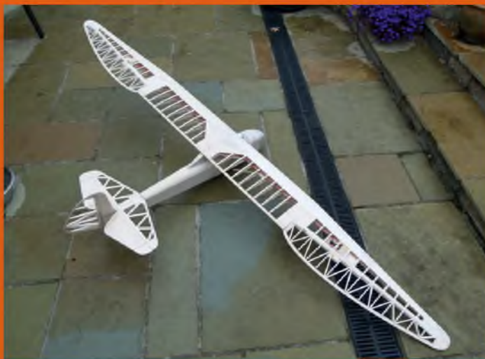
Traditional construction on the Wolf's airframe.
