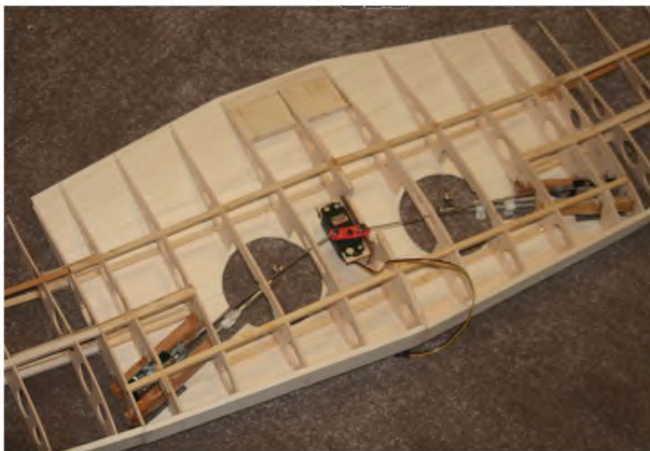
The wing centre section with mechanical retracts, servo and linkage fitted. Outer panels also attached.
