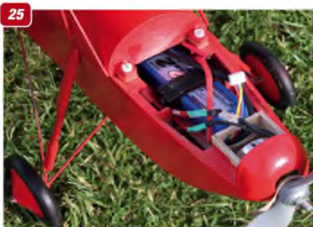
25 Battery, held in place with Velcro. Note also the faired main undercarriage strut
