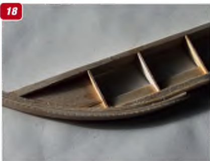
12: Wing ribs being slipped onto spars. 13: The basic wing structure of ribs, spars, leading and trailing edges. 14: Wing tip added. 15: Wing centre section with centre ribs spaced for the dummy fuel tank. 16: Wing tip, laminated from balsa strip. 17: The finished wing tip with leading edge sanded to shape, viewed from the underside. 18: Laminated tip of aileron. 19: Aileron tip after final shaping. 20: One of the wing support struts, now with laminated balsa fairing over the basic wire.
