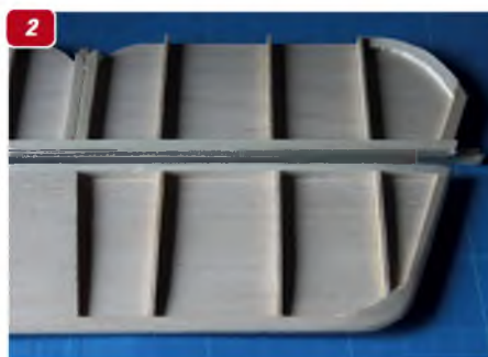
1: The elevator construction begins over a sheet balsa core. 2: Tailplane and elevator structure now formed with leading edge, hinge spar line and tips all added. 3: Rudder, elevator and tailplane sanded to shape.
