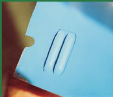
The twin louvers on the upper Aeronca cowl.
