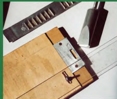
A strip of louvers for the Alexander Bullet with the punch and die.
