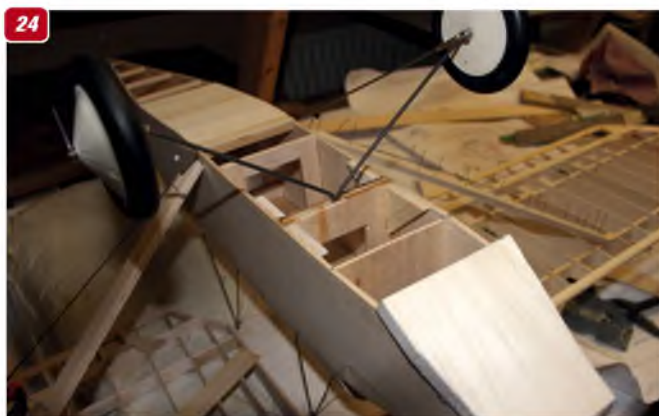
23: The anchor point for the wire main undercarriage, secured between laminations of the fuselage former.
