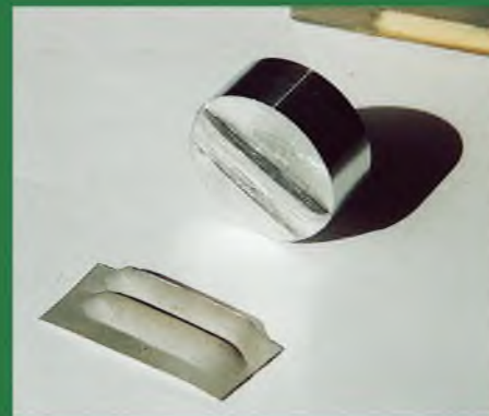
Another view of the punch with the die and a couple of sample louvers.
