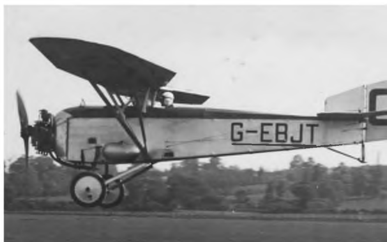
ABOVE, LEFT & BELOW: Three views of the Widgeon prototype, first registered in 1926 as the sole Mk 1 powered by a 35 hp Blackburne Thrush. Hugely underpowered the prototype crashed at the 1924 Lympe Trials and was rebuilt as Mk II G-EBJT, re-engined with a 60 hp Armstrong Siddeley Genet. Note the thick lozenge-shaped parasol wing, a shape that was to reappear in the company's Lysander in 1936. G-EBJT was sold to Dr E. D. Whitehead Reid who used it on his rounds until he crashed into trees in poor light at East Sutton Park, Kent in October 1930.
