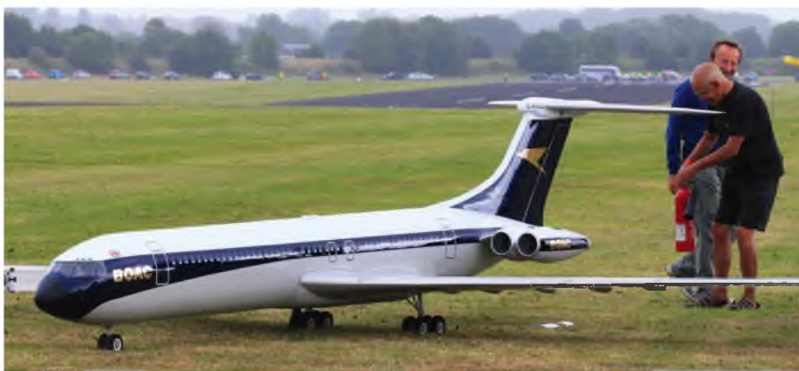
Elegant BOAC-liveried 4.9 metre span Vickers VC-10, powered by 4xWren Supersport gas turbines, and weighs 63 kgs.
