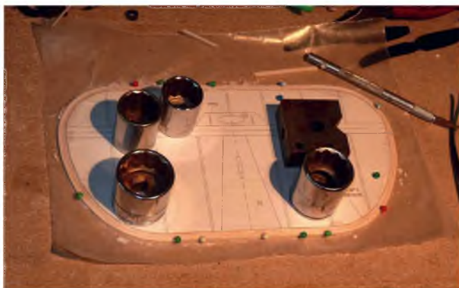
The tailplane outline being formed. Note the alternative method to that mentioned in the text. This easiest done as tailplane outline and elevator outline rather than a single piece.
