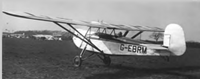
Widgeon G-EBRM in its original form, with wooden fuselage and Cirrus III engine. When it was converted to become the first Mk IIIA it emerged with a metal fuselage and flying surfaces and sported a wide divided undercarriage; a Hermes I replacing the original Cirrus III engine. After spending its last years with the Brooklands School of Flying it was scrapped there in 1931.
