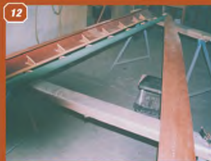
8: Awaiting restoration, the wing centre section, showing the ribs that cradle the gravity-feed fuel tank.
