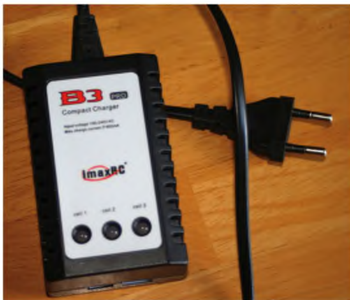
An after market 2 or 3 cell helicopter balance charger with lights to indicate the charge of individual cells within the pack.
