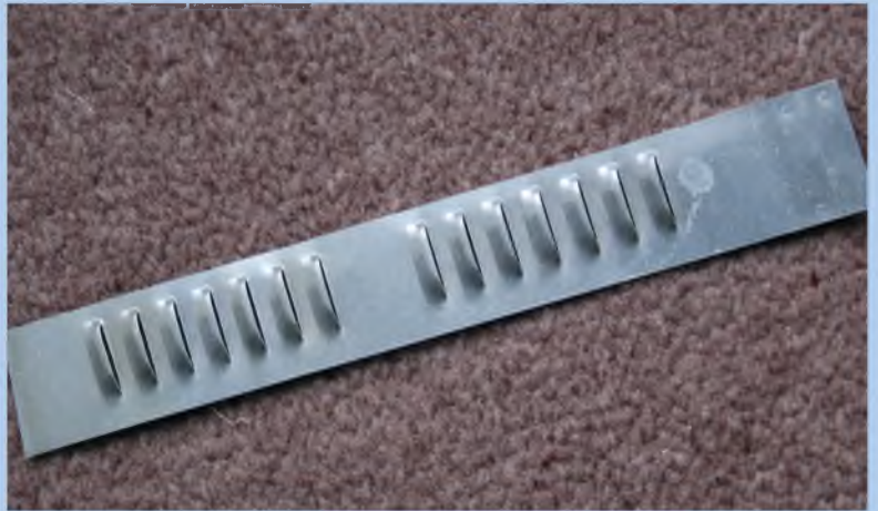
Two good examples of metal louvers punched into lito plate as described here by the author.
