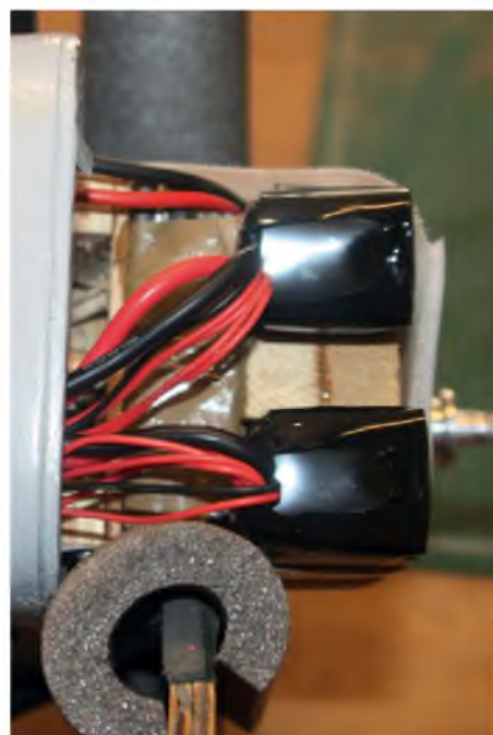
An underside view of the Lipo installation, showing revised connectors position - access now from rear of aircraft, well away from propeller.
