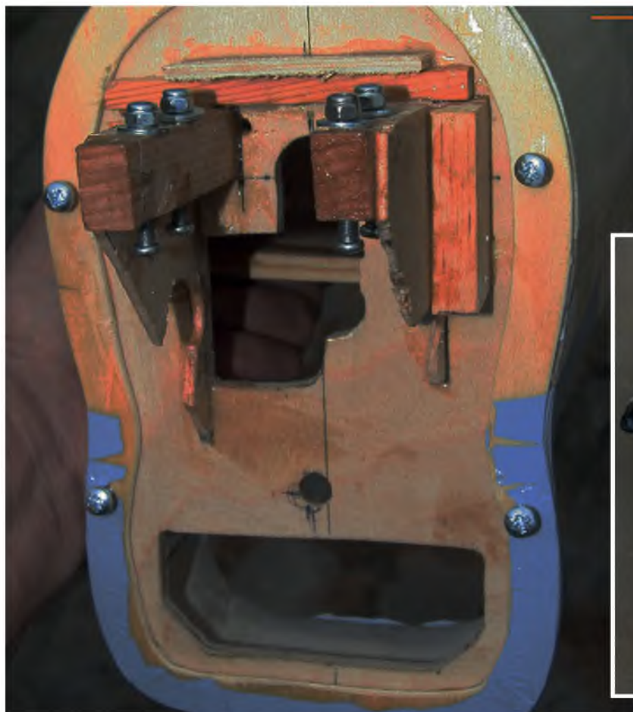
A view of the firewall with the original IC mounting system. Note large hole in firewall to clear the rear-mounted carburettor on the four-stroke engine. Note also the thin, profiled former fitted to firewall to positively locate the cowl (see main text).
