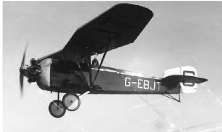
ABOVE, LEFT & BELOW: Three views of the Widgeon prototype, first registered in 1926 as the sole Mk 1 powered by a 35 hp Blackburne Thrush. Hugely underpowered the prototype crashed at the 1924 Lympe Trials and was rebuilt as Mk II G-EBJT, re-engined with a 60 hp Armstrong Siddeley Genet. Note the thick lozenge-shaped parasol wing, a shape that was to reappear in the company's Lysander in 1936. G-EBJT was sold to Dr E. D. Whitehead Reid who used it on his rounds until he crashed into trees in poor light at East Sutton Park, Kent in October 1930.
