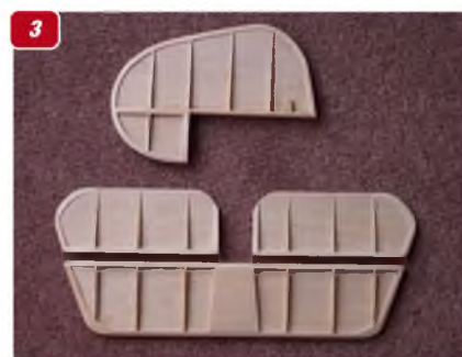
1: The elevator construction begins over a sheet balsa core. 2: Tailplane and elevator structure now formed with leading edge, hinge spar line and tips all added. 3: Rudder, elevator and tailplane sanded to shape.
