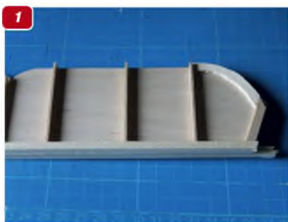
1: The elevator construction begins over a sheet balsa core. 2: Tailplane and elevator structure now formed with leading edge, hinge spar line and tips all added. 3: Rudder, elevator and tailplane sanded to shape.
