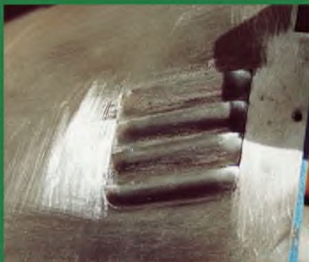
A bank of four louvers on the Aeronca lower cowl.
