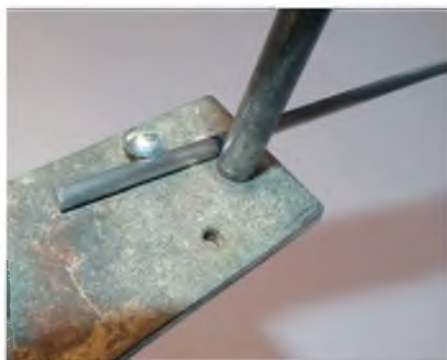
Position the mark on the wire touching the bending post
