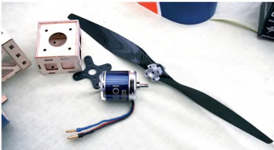
High quality 400 KV motor with stand-off box to provide correct spacing with the cowl
