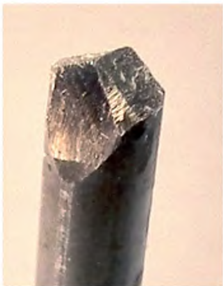
This drill is made from 8 SWG wire. Similar drills can be made with any gauge of wire
