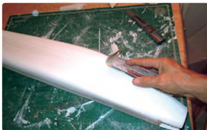
After gluing on the remaining fuselage side, round off the sharp edges with a sanding block
