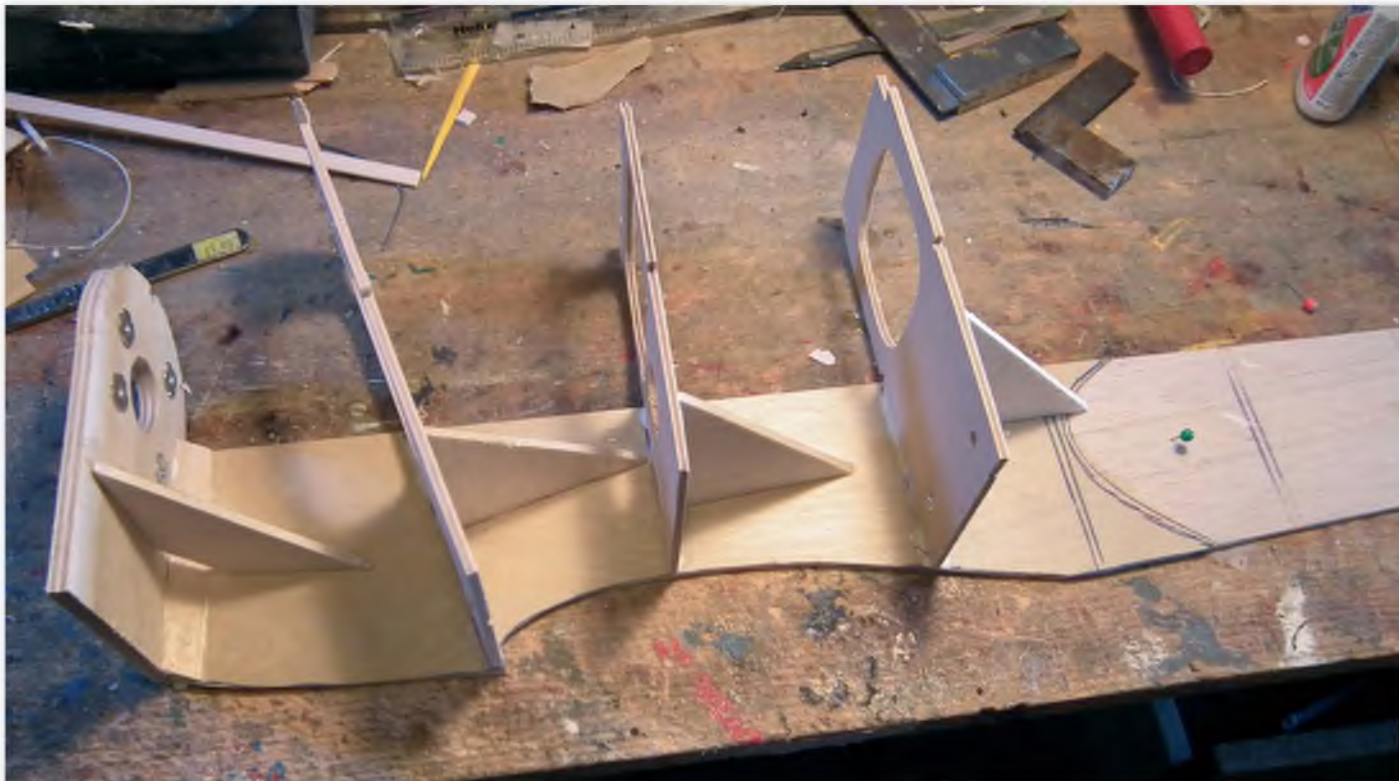
Glue the first four formers to one fuselage side. Triangles make sure that they are vertical
