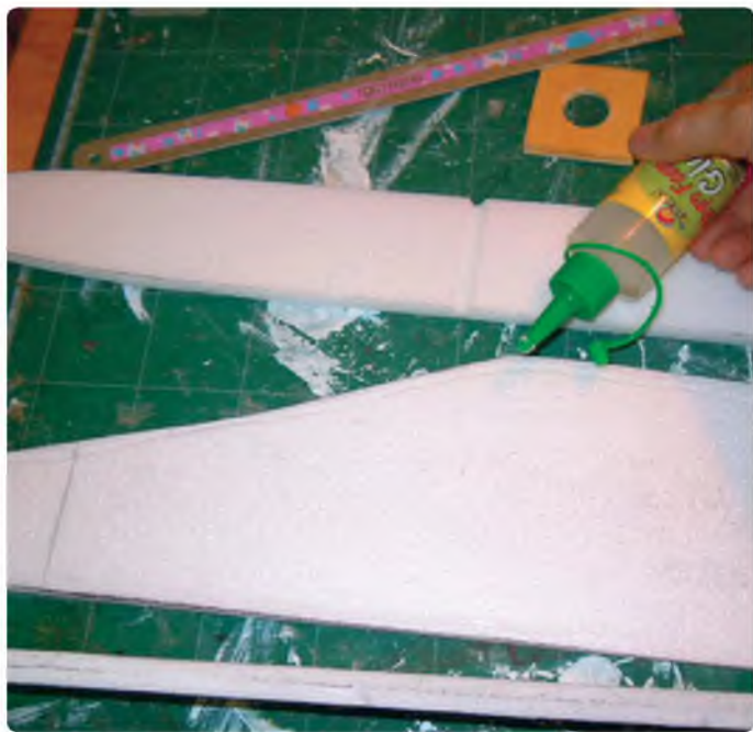
Cut out and prepare the fuselage parts. Note the groove in the top sheeting to allow it to bend over the canopy hump
