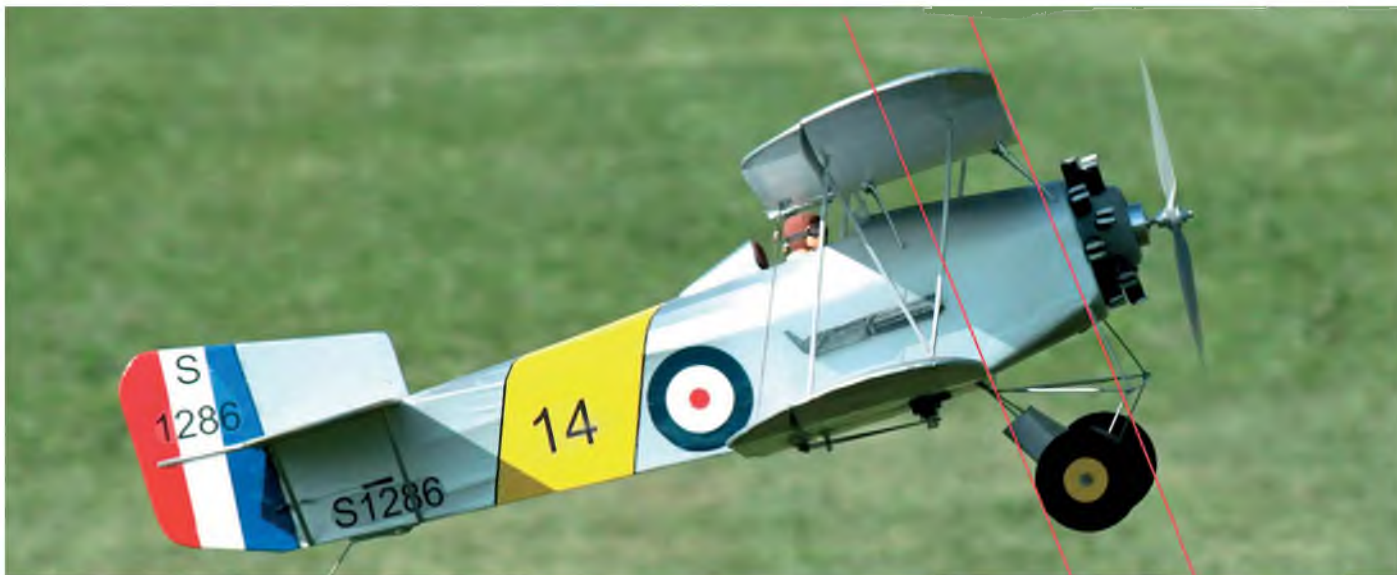
Fairey Flycatcher has two equal area/equal span wings, so the landing gear axle sits under what would be the LE of the averaged wing. Red lines show the top and bottom wings' leading edges
