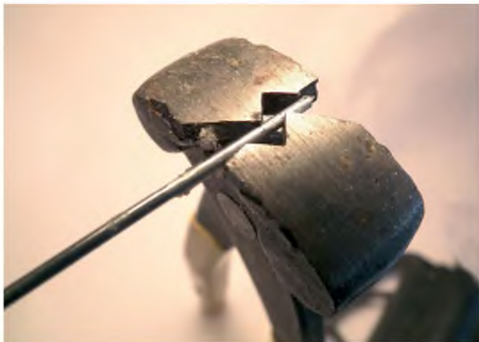
The normal 'Z' bend pliers. Position the wire and...
