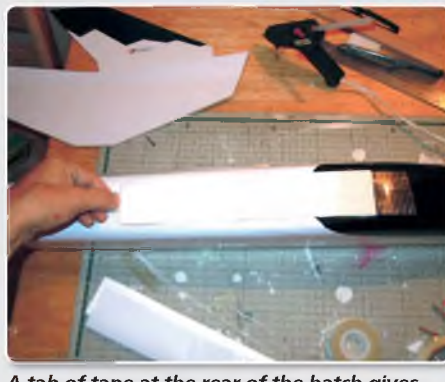
A tab of tape at the rear of the hatch gives you something to grip when pulling it clear to reach the battery
