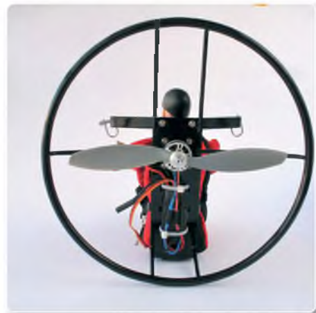
The cage is essential in order to stop the riser lines from tangling with the prop
