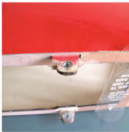
There's not a lot of meat left after drilling out the canopy lugs for the blind nuts so proceed with care
