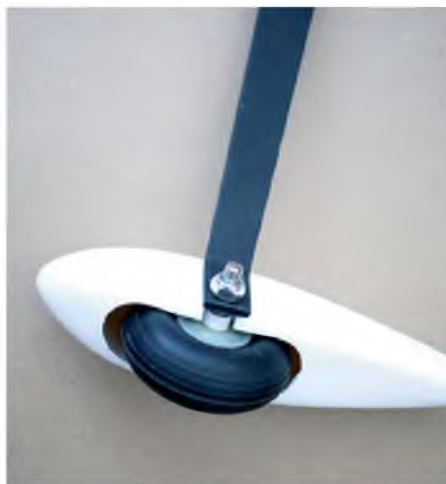
Wheel spats are a good fit on the undercarriage. Note the supplied plastic spacer to provide wheel alignment
