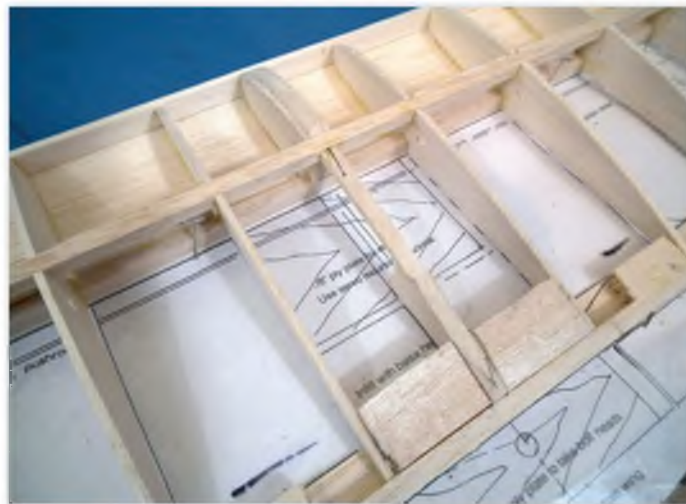
Close-up of centre section before sheeting is added
