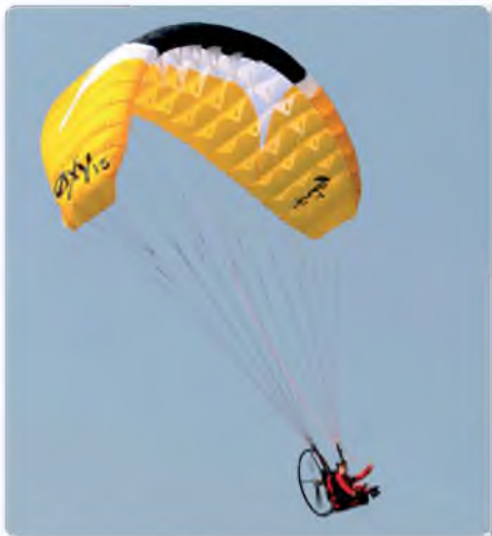
This side profile gives a good shot of the single skin wing and its 23 cells
