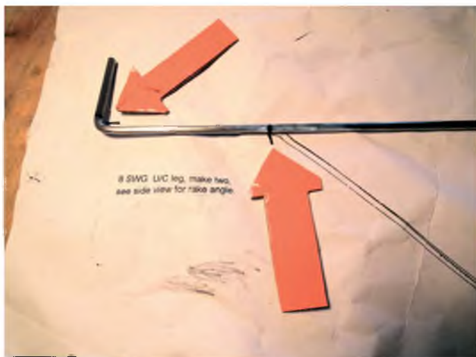
Marking the second bend. By marking each bend after the previous one has been bent you get better accuracy
