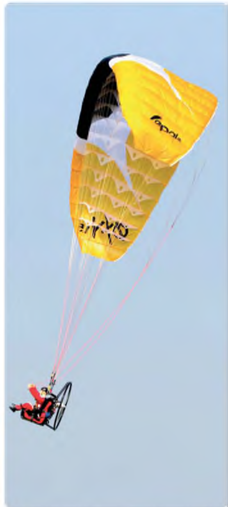
Side view in flight showing how the brake lines at the rear need some slack for normal flight
