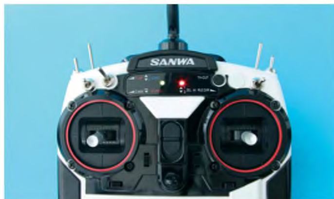
Top half of the Tx showing the main stick units. The Power and RF Output LEDs are nice and bright!
