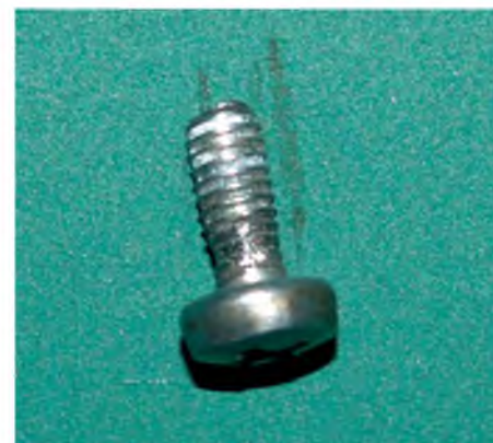
Inspection of the offending screw revealed the true source of the problem – the epoxy board had worn the threads off the screw! At least it was an easy fix
