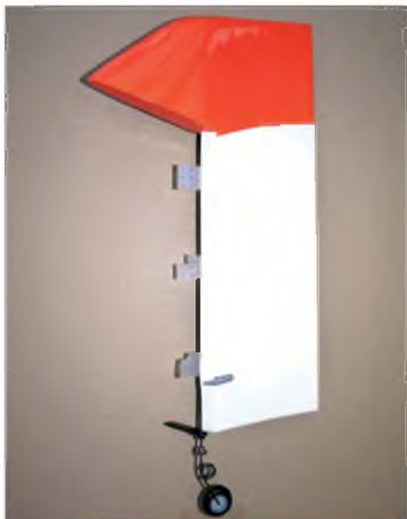
Rudder assembly. Note the modifications to the lower hinges to prevent them fouling on the fin's internal structure
