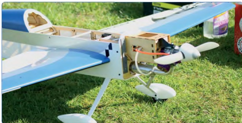
With the cowl and canopy off there's a good view of the engine mounting, showing how the Genesis mini pipe sits in a hole in the firewall
