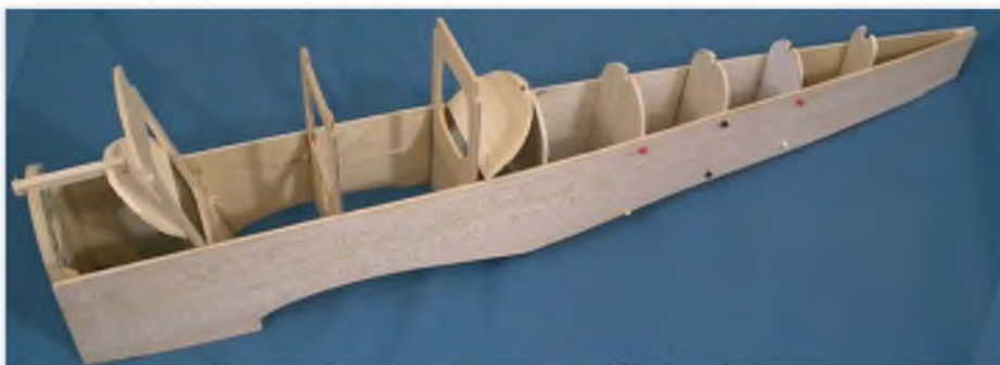
Pull in the sides at the rear and add remaining formers
