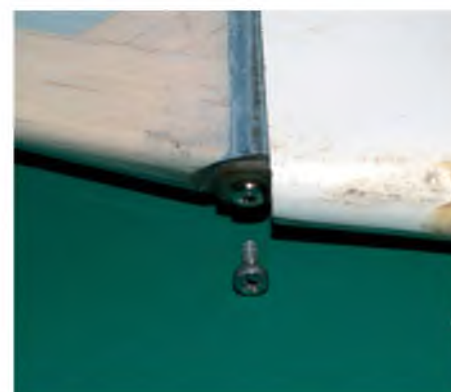
This lower pivot, made by a 2.5 mm screw, which goes through the fixed plate and up into the rudder, was the next suspect. Had the metal screw worn the hole in the board and caused looseness? No!
