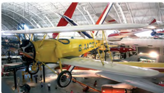
The Arrow Sport A2-60 was innovative. It had a tandem dual control cockpit and cantilever wings. The N struts were added as pilots felt insecure without them!
