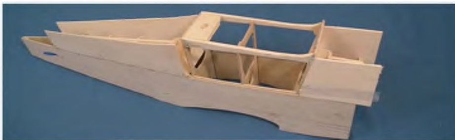
Glue the turtle deck sheets on vertically and leave to dry. Note 1/4" sheet cabin top member and ply window frames. Also the 1/8" sq forming rebate where the ply joins the sides
