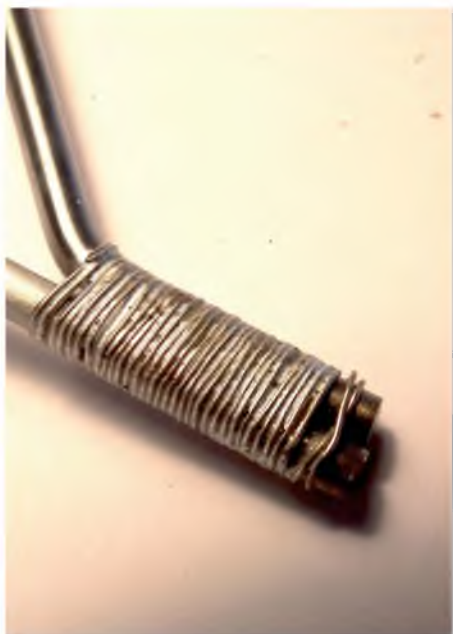
The neat way to join two pieces of piano wire. Note how the solder has flowed right into the wire wrapping
