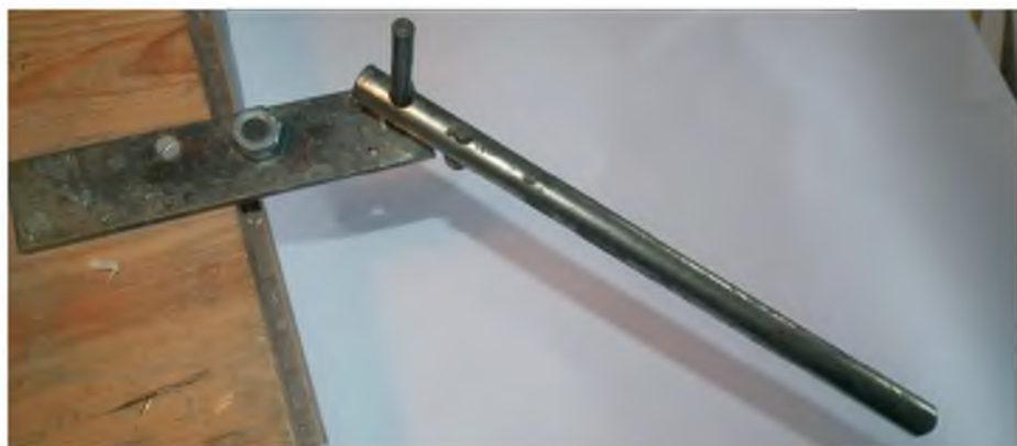
This wire bender will handle 8 SWG with ease and can bend coils. It has even been used to bend 6 SWG wire, although it protested by snapping three of the stop bolts
