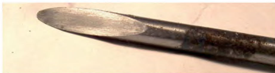
This reamer will work on most materials and will open up holes to a perfect fit for the wire
