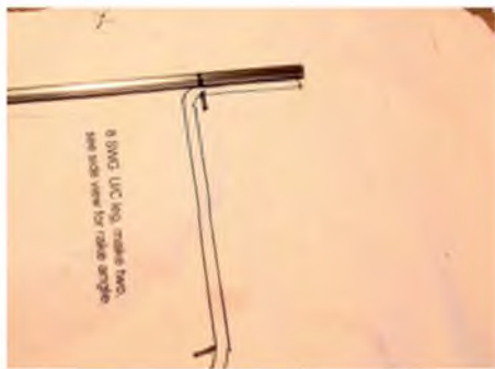
Making the first mark on an undercarriage leg. Note that the mark on the plan is at the start of the bend
