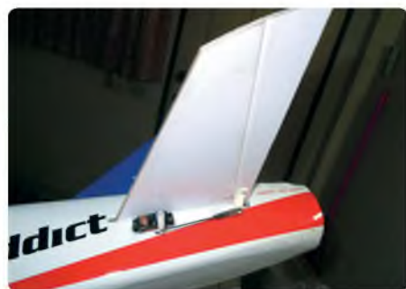
The elevator servo also uses a short wire pushrod
