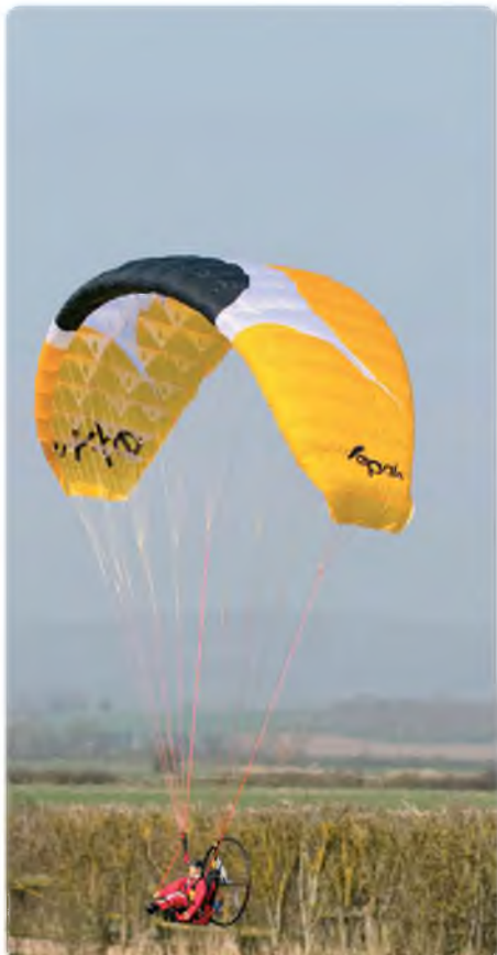
Coming in to land. Pulling against the rubber band on the Tx causes the arms to drop, thus pulling on the brake lines and drooping the trailing edge of the wing
