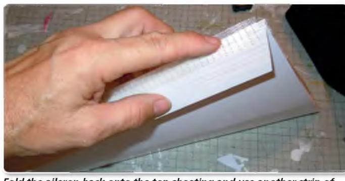
Fold the aileron back onto the top sheeting and use another strip of tape to seal the underside of the hinge line
