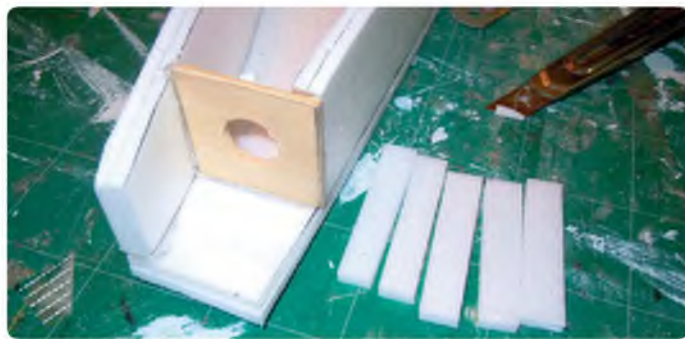
Above & below: Add the ply firewall and reinforce behind with rectangles of foam
