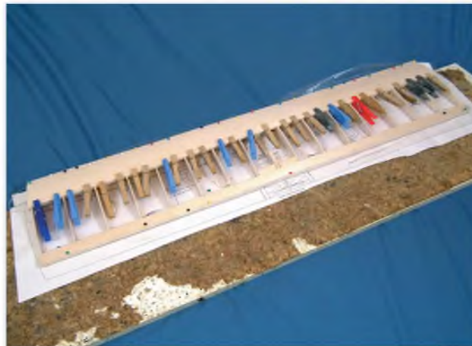
Top sheet and rear spar capstrip added
