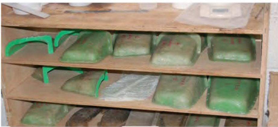
All fibreglass mouldings are currently fabricated in-house. The moulds themselves are constantly being refurbished to ensure a quality product
