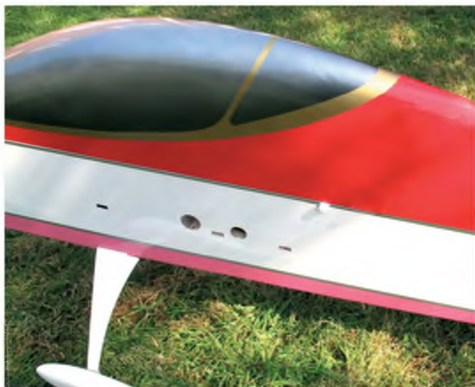
Monolog's large canopy is now retained using R/C helicopter canopy screws to provide faster access in case of battery problems
