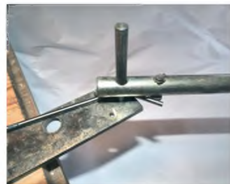
Making a bend is simply a matter of pulling on the lever
