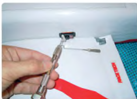
Fit the aileron servos above the wing and link up using short wire pushrods
