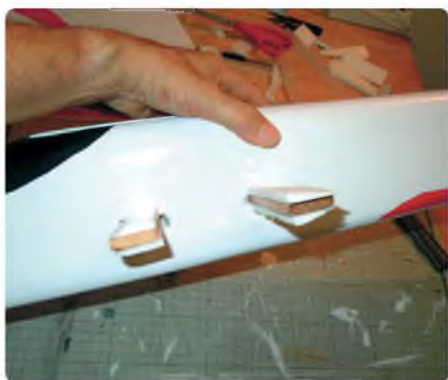
Chamfer the foam strips to match the inside profile of the wing roots
