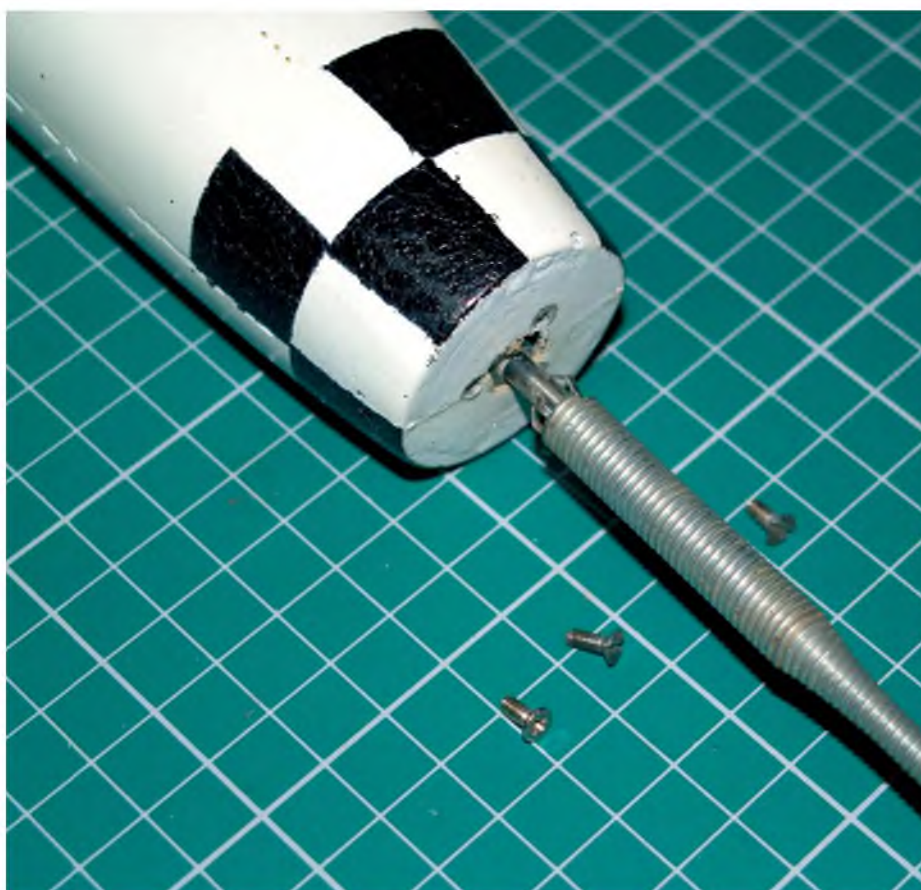
With the tool inserted into the nose ring the motor can be pulled into place and the hold down screws secured quite easily. But don't forget to connect the ESC as well if the motor wires won't reach a convenient opening!
