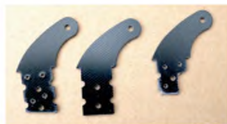
Control horns had to be trimmed to fit the slots in the ailerons (left) and elevator (right)
