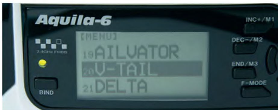
Wing and tail mixes are offered for Ailvator (taileron), V-Tail and Delta (elevon) set ups
