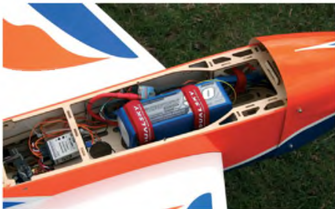
Plenty of room under the canopy for a 5000 mAh 6S battery. I made a small plate to mount the receiver above the wing joiner tube so that the battery could be moved further back if required
