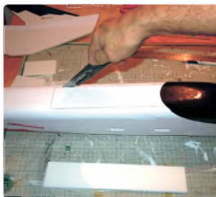
Next, mark and cut out the battery hatch
