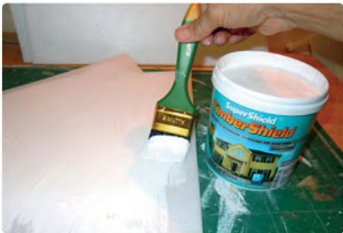
Coat the outer surfaces of the wings with water based varnish
