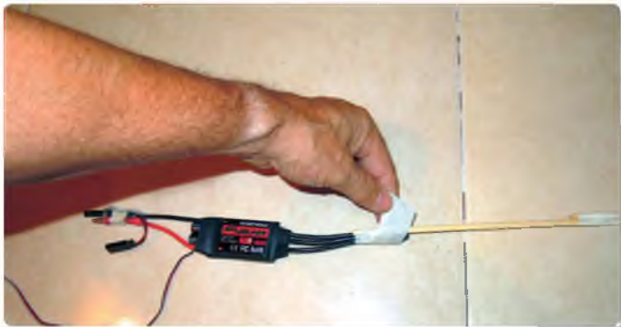
Tape the motor wires to a stick so that the ESC can be fed down inside the nose.
