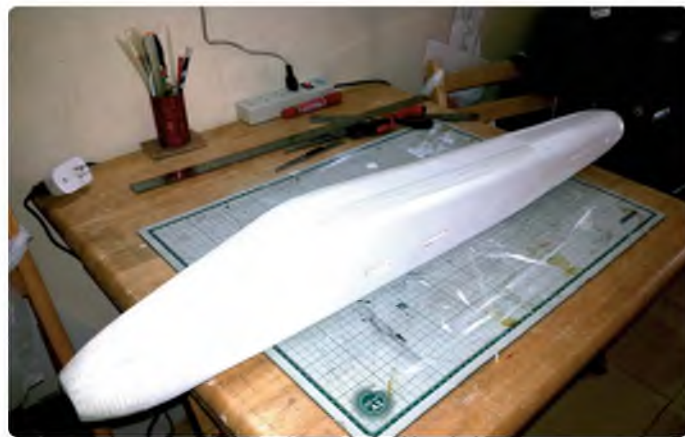
Reinforce the fuselage joints with strips of glass tape
