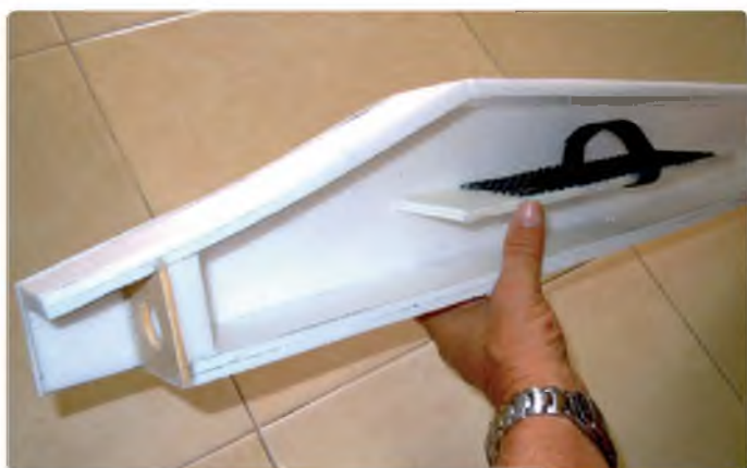
Glue in the battery mount. Line this with a piece of non-slip mat and fit a hook and loop strap
