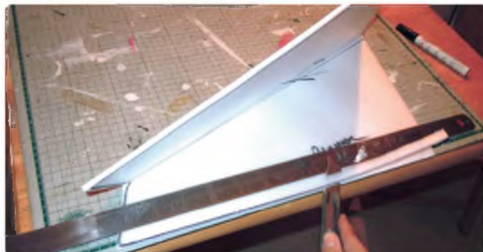
Carefully chamfer the trailing edge of the bottom sheet and sand smooth
