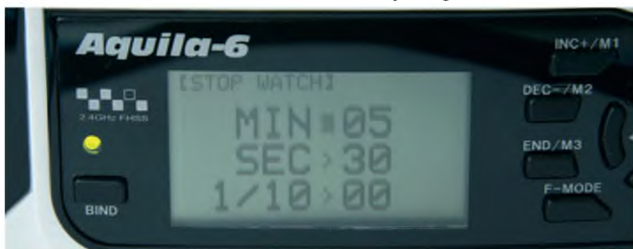
If you input a time then the Stopwatch function automatically works as a Count Down Timer. If you leave it at zero then it works as a Count Up timer
