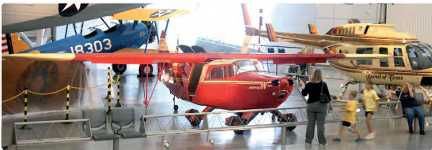
Fulton Airphibian roadable aircraft of 1946. Note the propeller attached to the right side of the rear fuselage for storage while the front becomes a car
