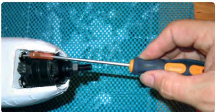
Use a short piece of fuel tubing over the screwdriver blade and motor mounting screws. This makes it much easier to keep the blade in place as you nip the screws up tight
