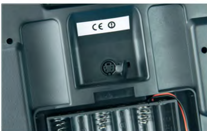
A plastic lid covers the multi-pin trainer socket
