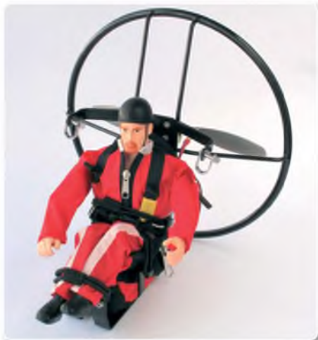
The ready to fly version of Max comes fitted with a high torque servo fitted to each shoulder, while the RTF Backpack S is complete with a Dualsky brushless motor, ESC and an 8-inch prop
