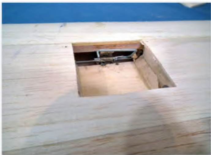
Typical connection of pushrods to servo
