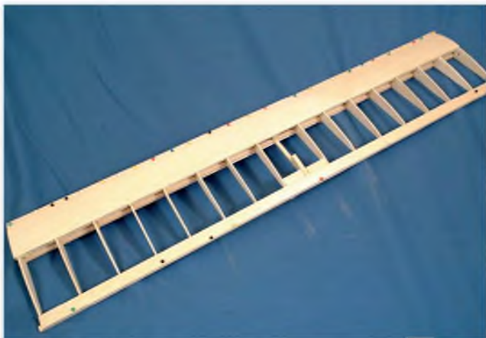
Lower wing lifted from the board and ready for fitting controls, centre section sheet and capstrips etc.
