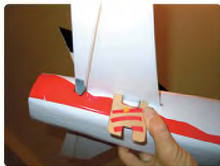
Use a ply template to mark out the cut-outs for the elevator and aileron servos
