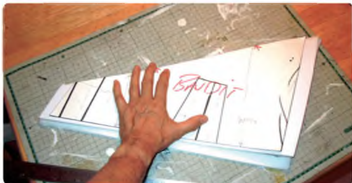
Use the template to trim off excess material around the edges of the wing
