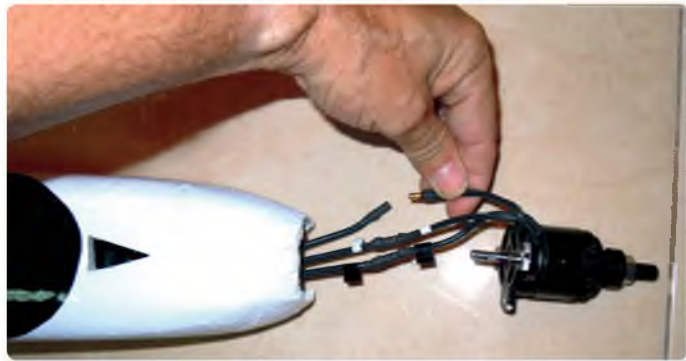
Feed the stick through the hole in the firewall and pull through until the motor wires appear
