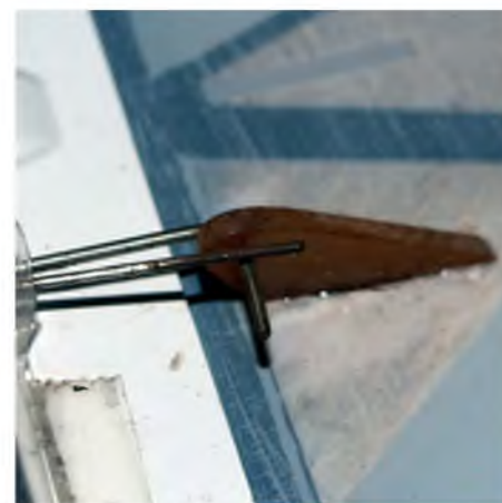
This simple wire drive into a piece of epoxy board, on the rudder of the AVA, was suspected of having worn over four years, and to be the cause of a floppy connection. But it was innocent!
