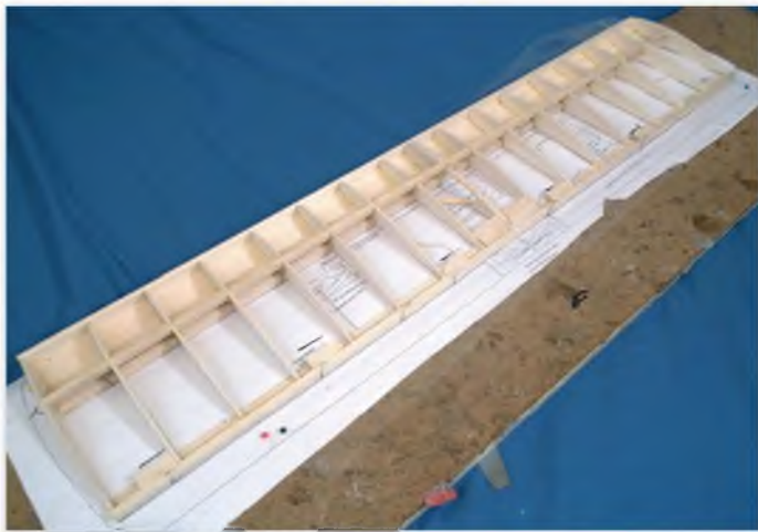
Stage one of building the wing. All blocks etc. added. LE sheet raised to leading edge
