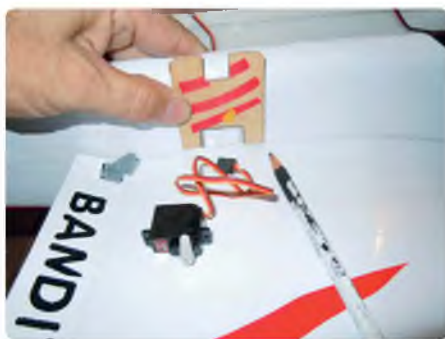
Use a ply template to mark out the cut-outs for the elevator and aileron servos
