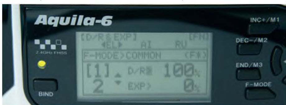
Dual Rates and Exponentials are easy to set. The two numbers on the left show the position of the single D/R switch
