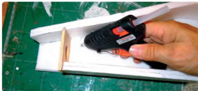
Above & below: Add the ply firewall and reinforce behind with rectangles of foam
