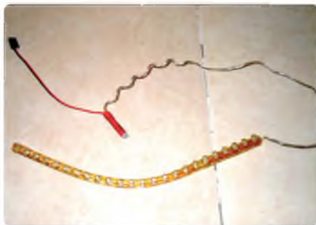
A strip of yellow LEDs are used to simulate an afterburner in the tailpipe
