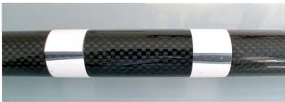
Two rings of tape were wrapped around the middle of the wing tube. The carbon joiner tube is now a close fit within the fuselage tube
