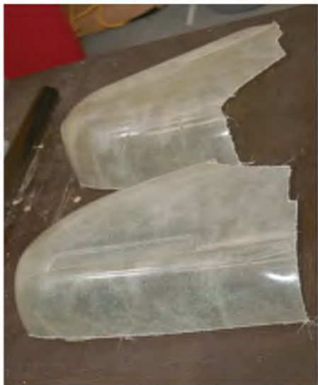
Two halves of an 80" Spitfire cowling just out of the mould
