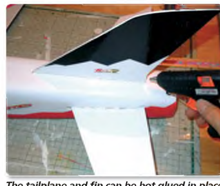
The tailplane and fin can be hot glued in place after making sure that they are square to the wings
