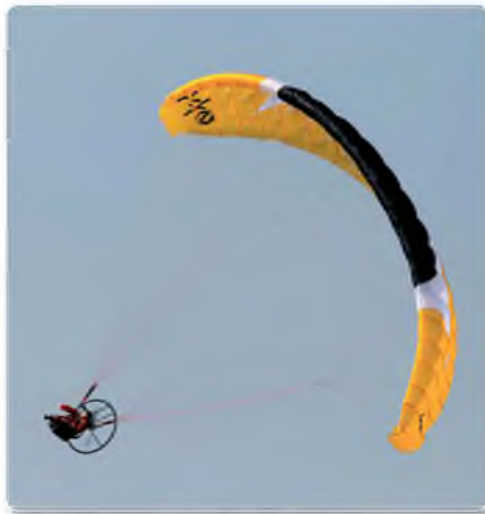
The model turns quite steeply if you apply some braking whilst steering. Just don't try it too low!
