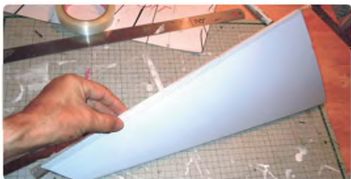
Fold the wing shut and roll the tape over the trailing edge to secure it
