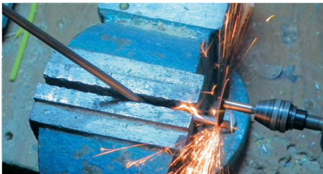
A cutting disc is the best way to cut thicker wire to length
