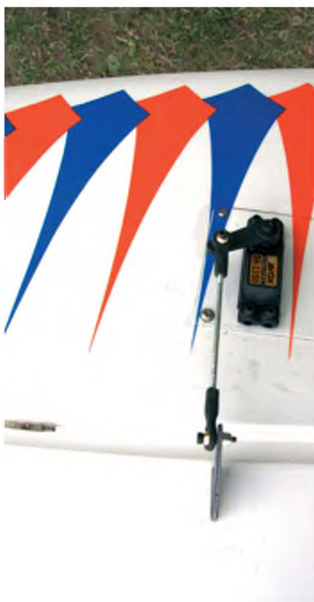
Aileron and elevator control rods have ball connectors at each end for smooth, slop free, precision linkages
