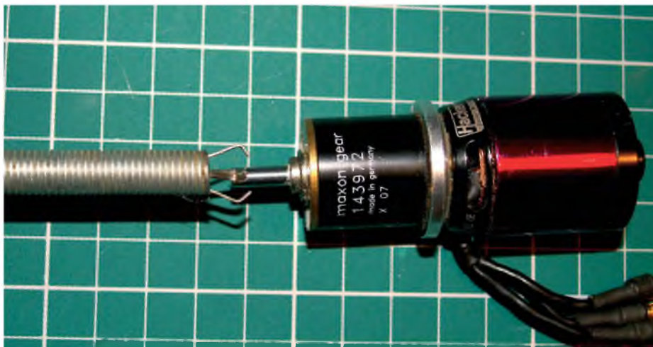
The prongs on the business end have a fair amount of grip and can easily hold the shaft of much bigger motors than this small, geared outrunner when they need to go into a longish nose
