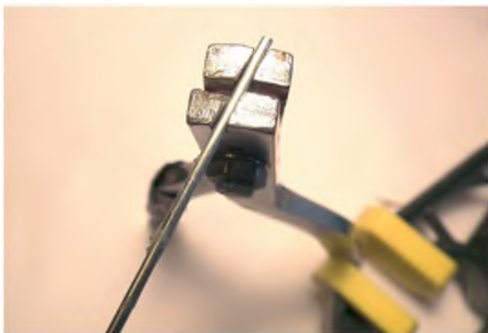
These American 'Z' bend pliers produce an really excellent 'Z' bend but are not so good for thinner gauges
