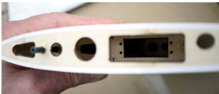
Below: Elevator servos are fitted into the horizontal stabilisers before they are attached to the fuselage. I opened the mounts to accept the Savox SH1350 servos that I used
