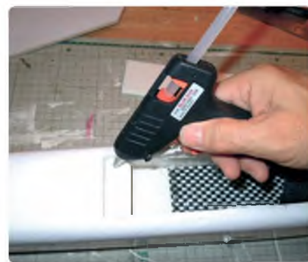
Glue in a piece of Correx or ply to act as a stop for the hatch
