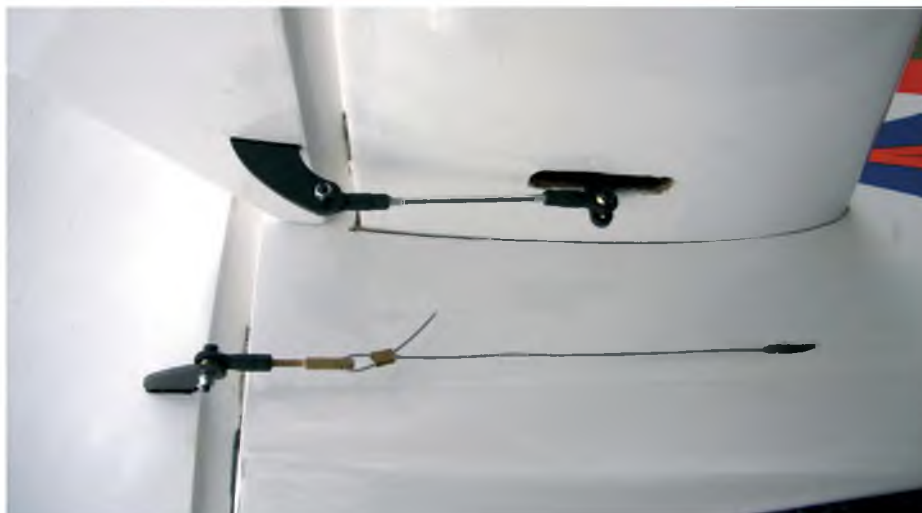
Rudder control uses a closed loop system. Note positive dual ball link control to elevator
