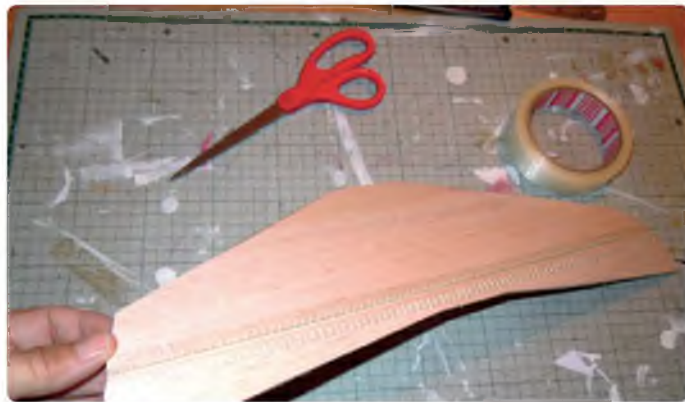
Use more strips of glass tape to hinge the elevator
