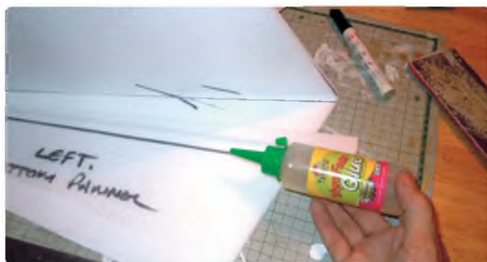
Mark the spar location and glue in place
