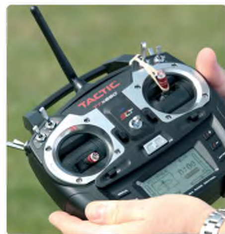
A rubber band maintains full down 'elevator' and keeps the arms up for cruise flying
