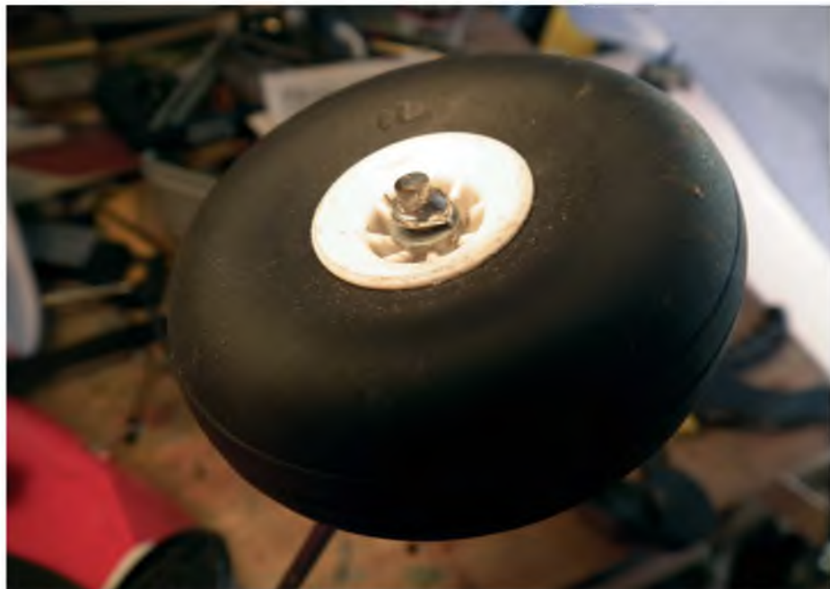
This wheel will never come off until you want it to. A washer and a few turns of wire and some solder
