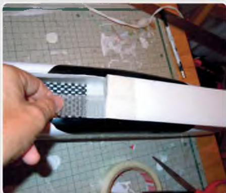
Hinge the front edge of the hatch using glass tape
