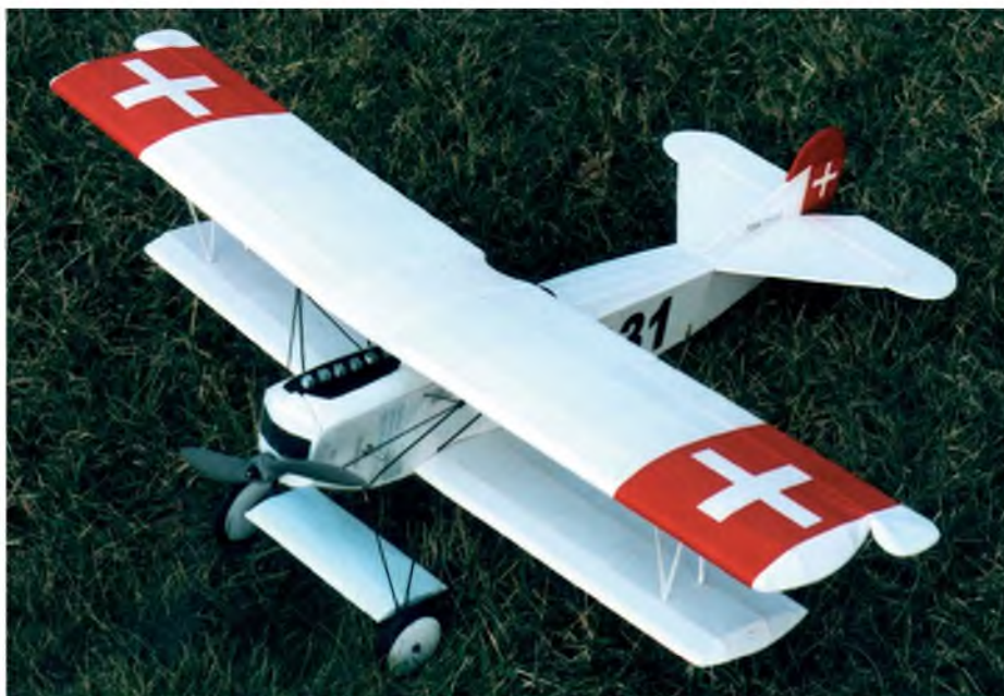
Fokker D-VII, stablemate to our Pup and another fun flyer on a geared Speed 400. Being a sesquiplane, the D-VII's C of G had to be computed based on the two different wing areas and a bit of stagger
