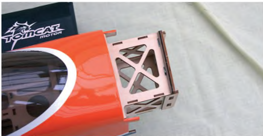
Motor mounting has side thrust and offset built-in
