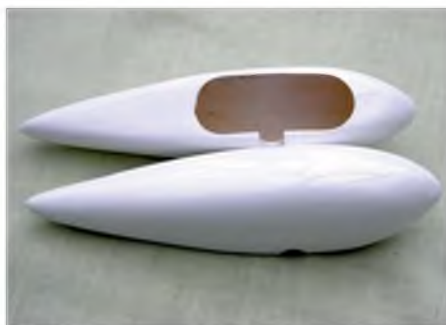
Fibreglass wheel spats have ply reinforcement where they are secured to the undercarriage
