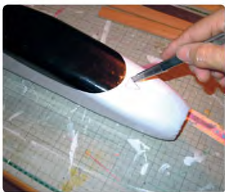
Cut out a hole for cooling air to reach the battery
