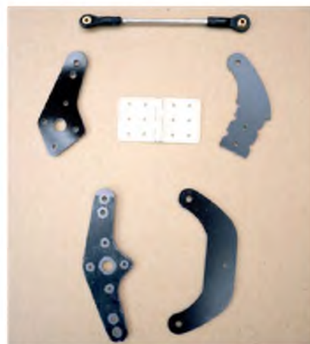
Control horns, rudder closed loop horn and servo adaptors are made from carbon fibreboard. Control rods are short and direct with ball joints at each end. Hinging is by high quality pinned hinges
