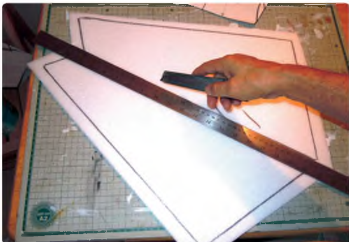
Lightly score along the leading edge line
