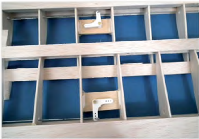
The bell cranks are mounted. Note that the orientation of these needs to be reversed on one wing
