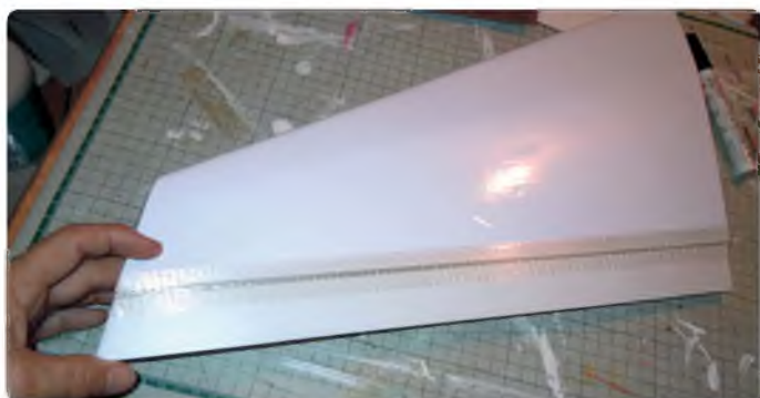
Use another strip of glass tape to attach the aileron to the wing panel
