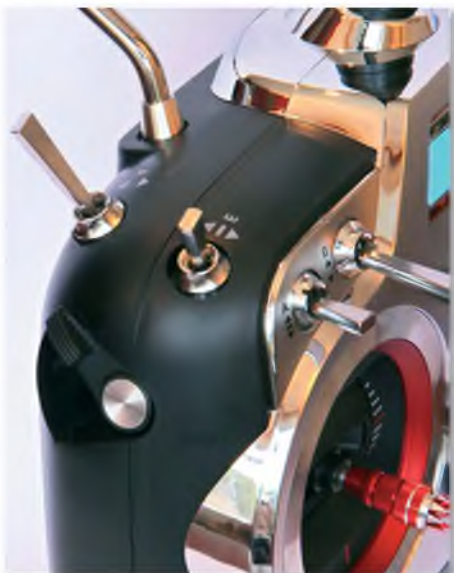
The left hand side has a slider and two 2-position and two 3-position switches. All switches are assignable
