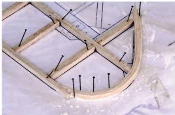
Wet balsa can be formed to virtually any shape if the pins are in the right place
