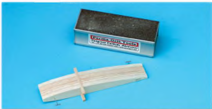
Stack ribs and sand smooth with a sanding block – preferably a Perma-Grit!
