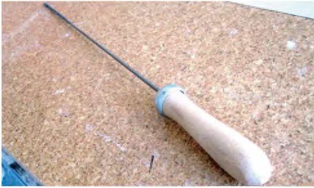
Snake tunnel tool – push through when hot!
