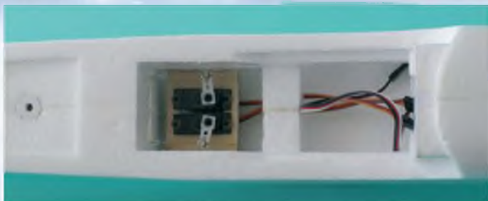
WOT 4 Foam-E comes pre-fitted with four 9 g micro servos. Two for the tail, seen here, and two for the wing. (Right) There's plenty of room in the front bay for a modern receiver such as the R2006GS used for this review (not supplied in the kit)
