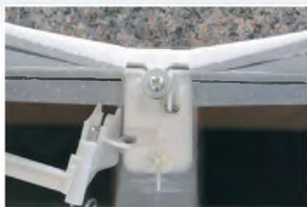
Neat inboard elevator hook up, also via a Z-bend in the pushrod
