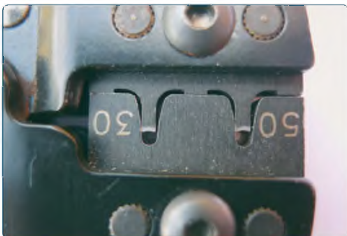
The jaws have two slots and both have important uses when making a good crimp
