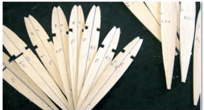
After cutting out the wing rib blanks, mark their centrelines
