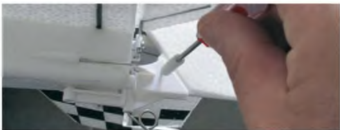
Fixing the small rudder retaining screw is a fiddly business. The old trick of using a short piece of fuel tubing to hold it onto the screwdriver worked a treat!
