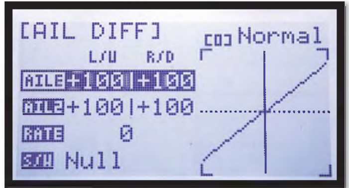
Aileron differential screen with curves
