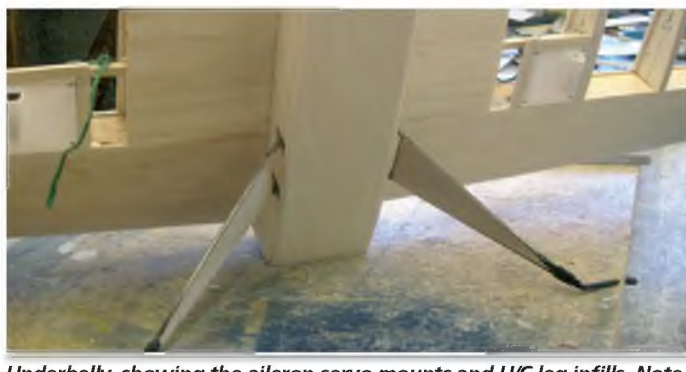
Underbelly, showing the aileron servo mounts and U/C leg infills. Note the string for pulling the servo cables through
