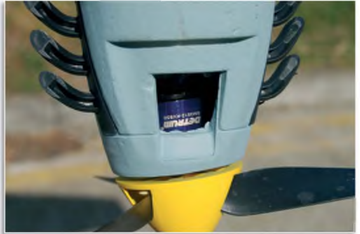
The cowlings hide a pair of 850 KV brushless motors
