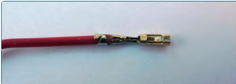
Here the short inner tangs have not been bent around properly when being crimped, which can happen if the connector is twisted in the tool so that the tangs are not facing down
