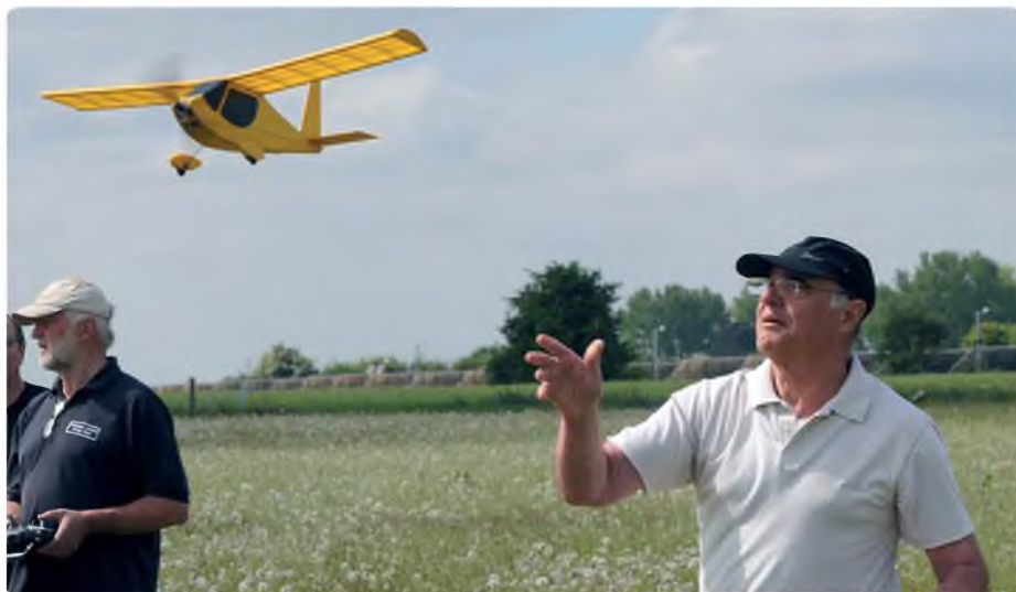
Brian Brundell from Melksham launches his tiny Buttercup, built from an American plan. Designed for a Cox 020, it is powered by a Hyperion HP21705 electric motor
