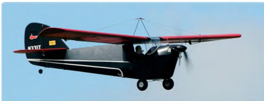
David Lovegrove from Wallingford flew an Aeronca C3 Collegian. Acquired as a wreck, it is rebuilt and converted to electric. E-Max 35 motor with a 6-cell 5000 mAh LiPo power supply
