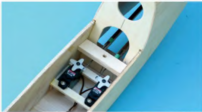
Install servos and linkages before closing in rear fuselage
