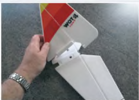
The fin simply plugs into the tailplane
