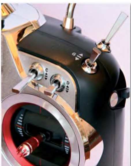
The right hand side features a slider, plus three 3-position switches and a temporary switch
