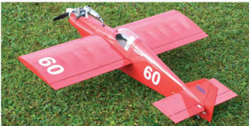
Above & below: After a thorough fuel proofing of the engine and fuel tank bays the model was covered in Super Monokote and trimmed with vinyl race numbers
