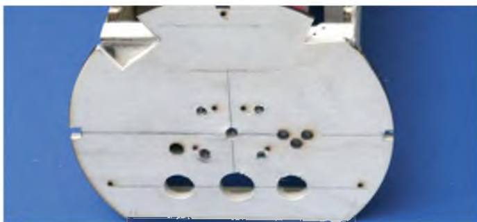
Plenty of space for battery cooling holes in the front former on the electric version
