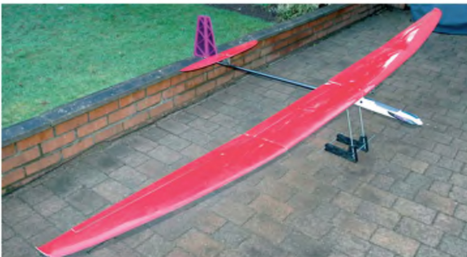
The prototype Claymore 3.6 m sitting on its balancing jig. This first version weighed around 2 kg and the subsequent development for 2015, detailed here, was produced in composite materials with the aim of a lighter flying weight of around 1800 g
