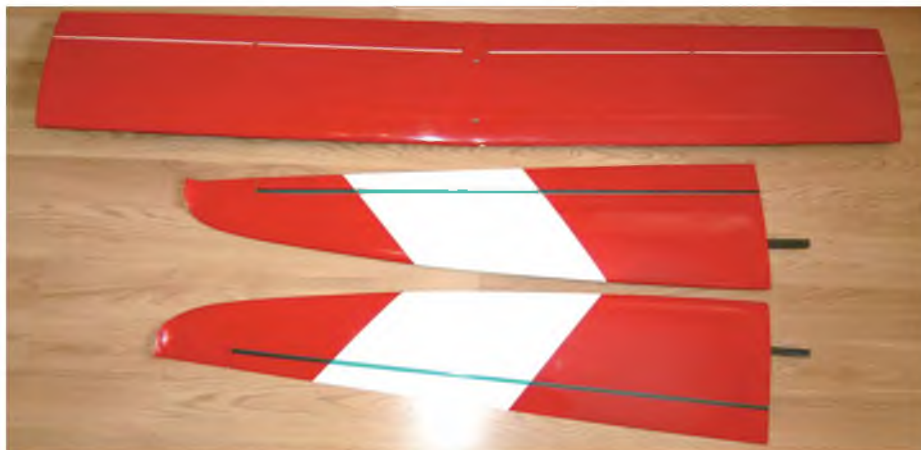
Centre panel from triple spread tow carbon on Herex core and tips using the same technique but a lighter lay-up. These are the latest Claymore mouldings from Rick Lloyd
