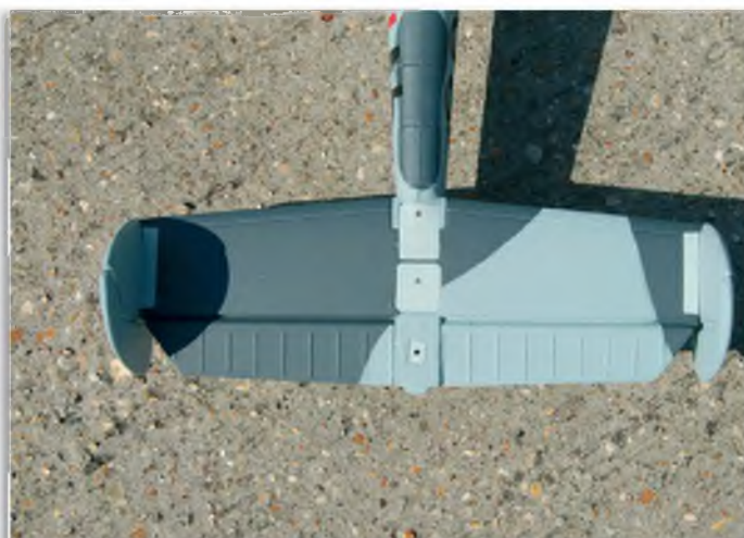
Plastic covers hide the tail linkages
