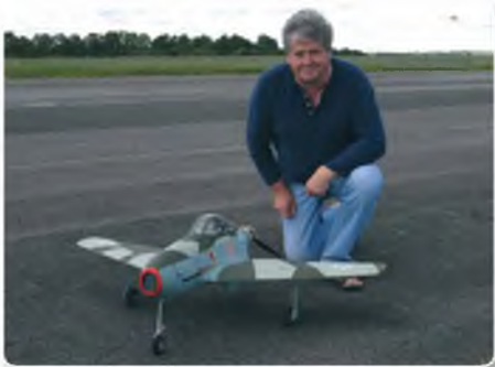
Above & Right: We look forward to seeing something new from Peter Illiffe at LM each year. This time he brought along his Messerschmitt Me 334, which spans 52 inches. A Hacker H30 motor powers the 4 lb model, via a 60 A ESC and 3S 2700 mAh LiPo. Traditional balsa/tissue/dope construction
