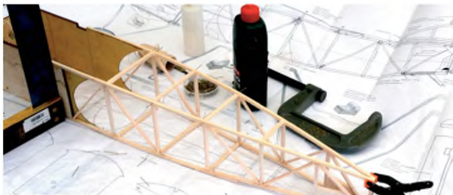
If the fuselage is built over the plan and pinned down it must end up being accurate when it is finished. Much cheaper than a fuselage jig
