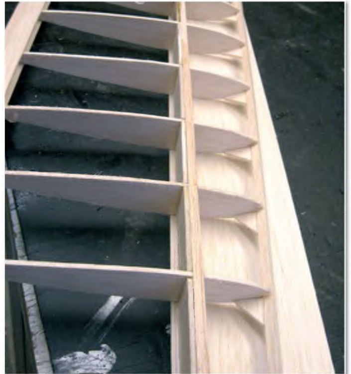
Adding the leading edge sheeting
