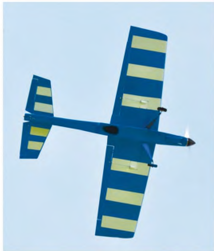
Use orientation stripes so there's no mistaking which way is up!
