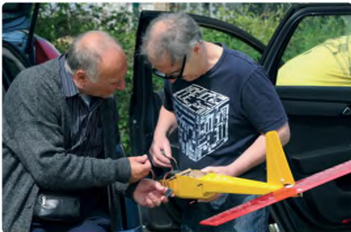
Gordon and Derek Parker sort out the wiring for the Graupner Amigo, adapted to electric power with a pod on the wing, after which Gordon gives it a sedate launch
