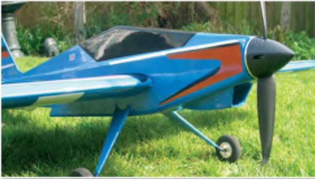
Cooling air enters the large inlet, runs over the ESC and through the underbelly
