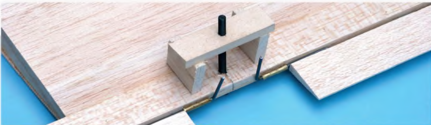
Temporary packing sets the location of the rear wing mounting block to clear linkages prior to installing in the fuselage
