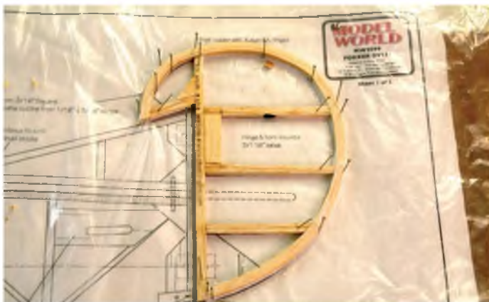
You've paid for the wood, so use it! The holders for the laser cut parts are perfectly cut, which means that they can be used to build other parts of the plane, like the fin
