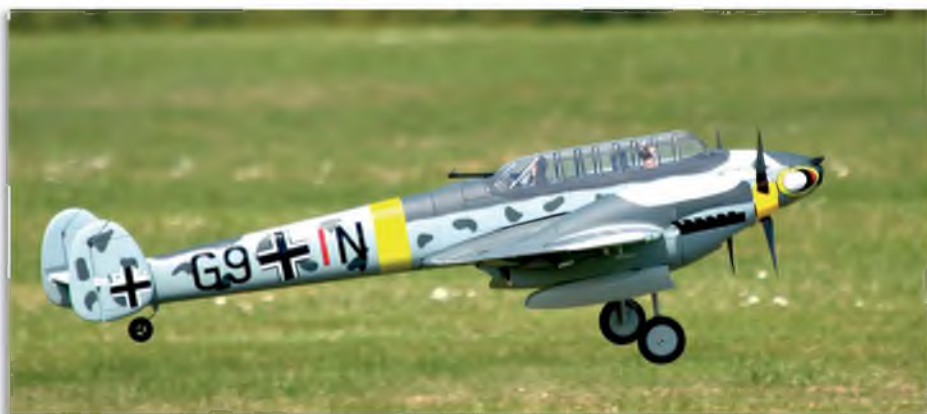
The best way to land the Messerschmitt is to run it in level and do a 'roller' landing on the main gear. Three point landings are more hit and miss!
