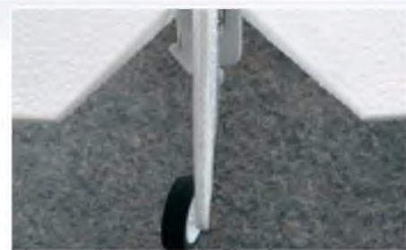
When first assembled the tailwheel had a large offset. But this was easily bent back in to line with the rudder
