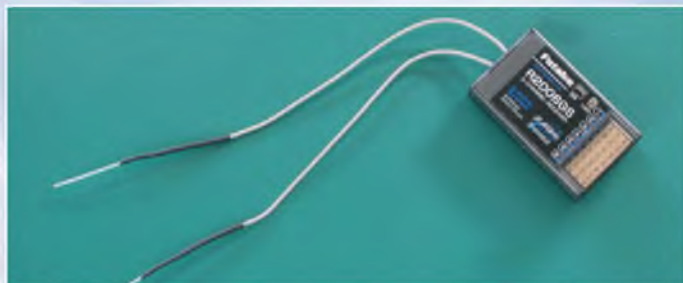
WOT 4 Foam-E comes pre-fitted with four 9 g micro servos. Two for the tail, seen here, and two for the wing. (Right) There's plenty of room in the front bay for a modern receiver such as the R2006GS used for this review (not supplied in the kit)
