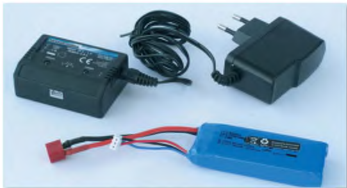
Hexatron is powered by a 2S 1500 mAh LiPo, for which a mains powered balance charger is supplied
