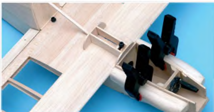
Centre section formers in place on top of wing. Front fuselage curvature is set by the cheek cowlers
