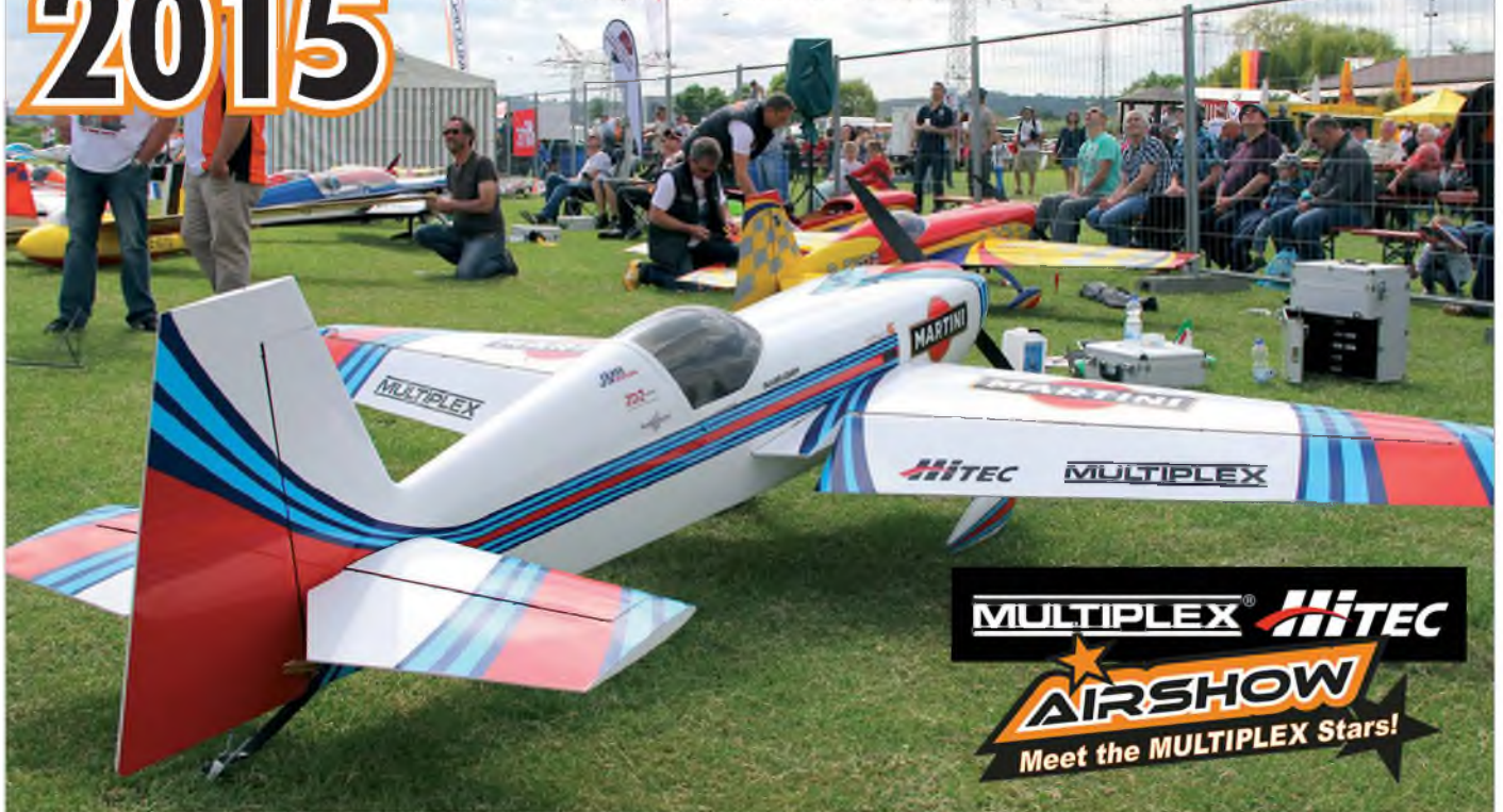
Krill Extra 330 SC in Martini colours, as flown by 19 year old Oliver Gräff. His model spans 3.1 m and is powered by a ZDZ 180. R/C is via a Multiplex PROFI TX 16 operating 12 Hitec 7990 servos
