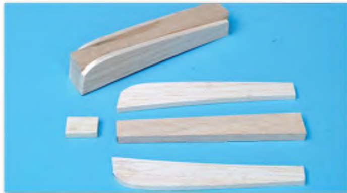
Cheek cowlers are built up from 1/4" sheet
