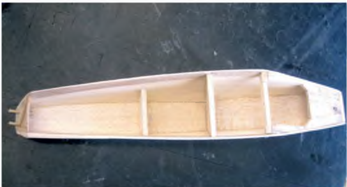
Strengthen the canopy's inner edges with micro-ply
