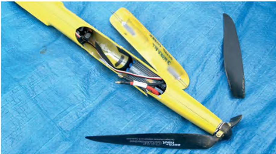
This is the damage to Dave Worrall's Ascot soarer, which occurred after a large portion of prop blade came off about 70 m into the climb. The huge out-of-balance force thus created twisted open the fuselage and threw out the battery, stopping the motor very quickly. See the text for the likely cause of the blade breakage
