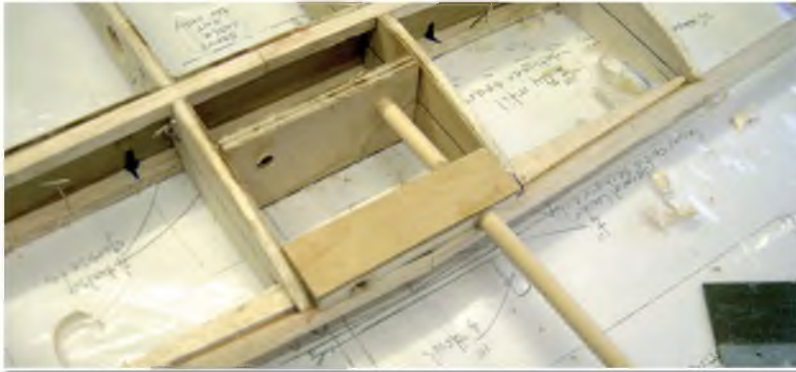
Strong wing down plates form part of the undercarriage mount
