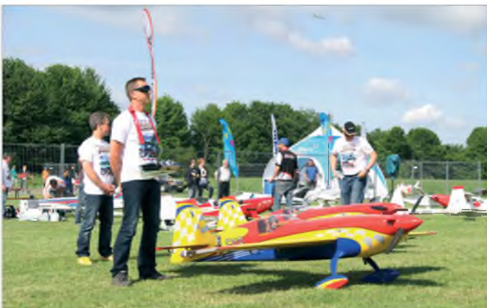
The 'German Aerobatic Team' of Ingo Brauer, Randolph Bromer and Andreas Merhout flew synchronised displays with their Krill Extra 330SC's. The 3.1 metre span models are powered by MVVS 175 NP Twinspark engines, with flight controls operated by Hitec HS-M7990 Digital servos
