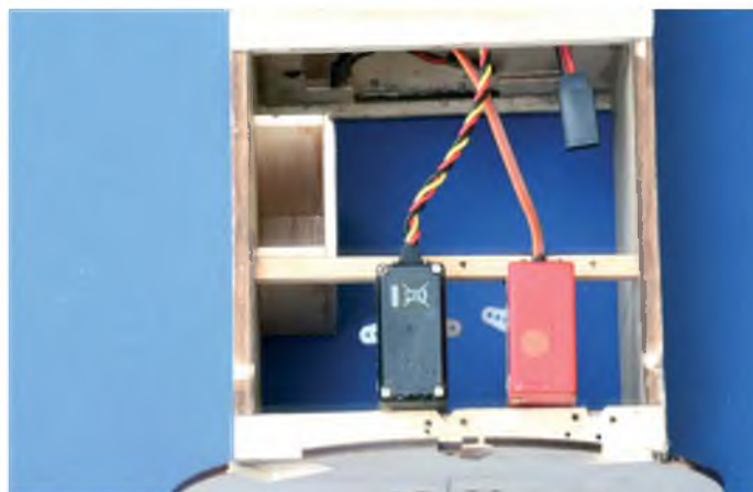
Receiver battery box in place
