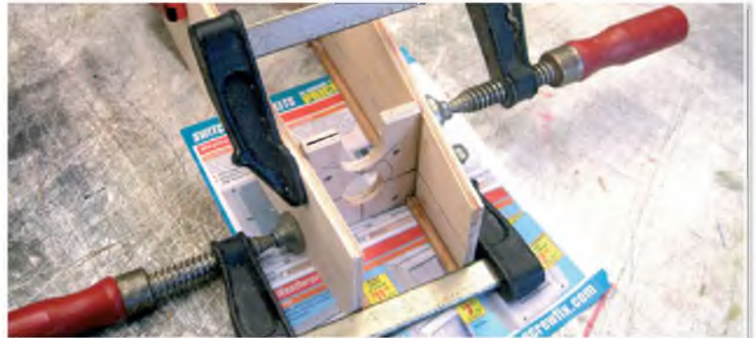
Epoxy in F1 and clamp until set
