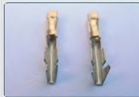
Folding up the tangs will help them to grip the insulation
