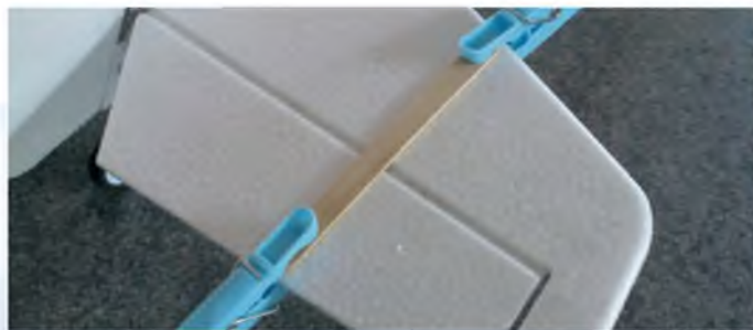
Lolly sticks are used as splints top and bottom to hold the elevator at neutral. The same tip can be used when setting up the rudder
