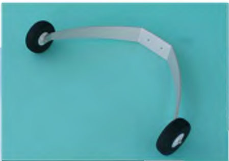
Stylish, ready made undercarriage needs to be fitted with a forward sweep
