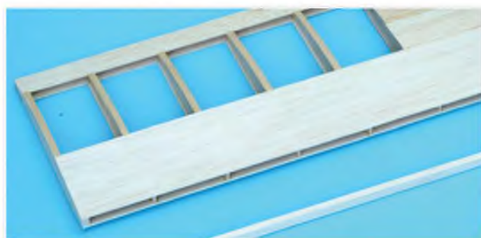
Sand LE sheeting flush with ribs prior to attaching LE
