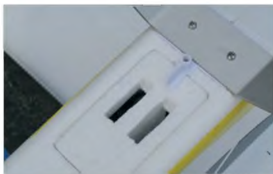
A loose Velcro strap holds the ESC in place
