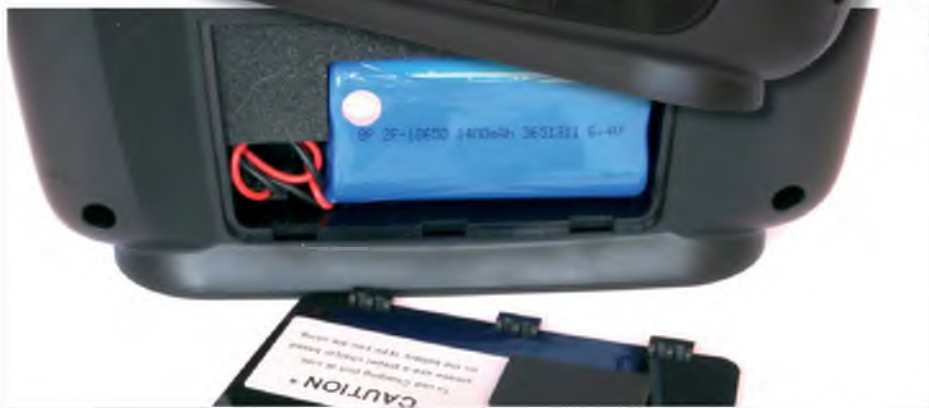
The 1400 mAh LiFe battery pack is accessed through a panel at the rear of the transmitter
