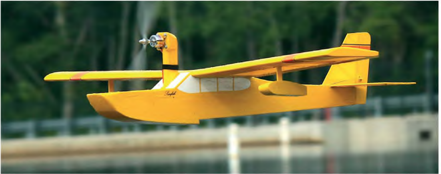
The Sunfish flying boat needs no down thrust on the motor
