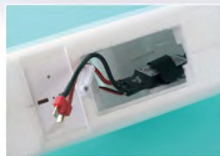
A loose Velcro strap holds the ESC in place
