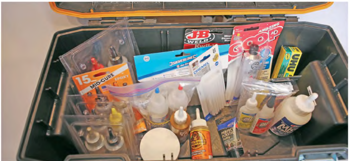
A cheap plastic toolbox makes a dark, dry, home for all my glues. Note: do not store accelerant in the same box!
