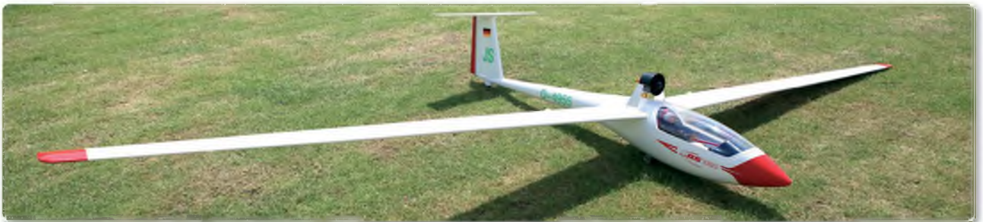
Horizon's gorgeous new ASW 20 glider, fitted with an electric ducted fan for self-launching
