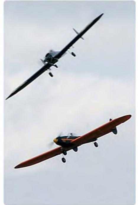
A pair of Mars models, scaled up to 67 inch span from a control line stunt plan. John Mellor's is electric powered and Mike Spencer's has glow power
