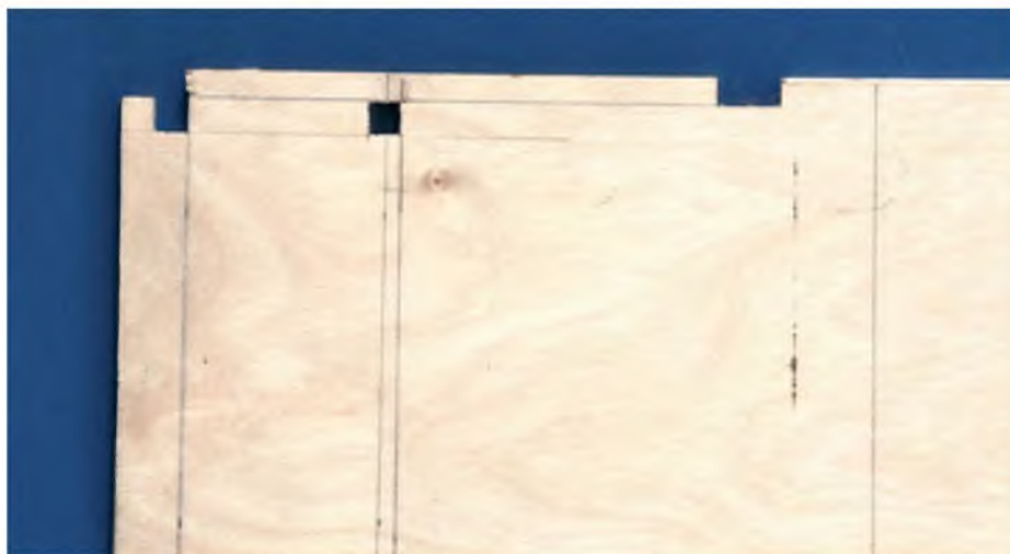
Pre plan the electrical installation. Servo bearers that are held in place with a straight through joint (through the square holes) are better than butt joints against the fuselage side
