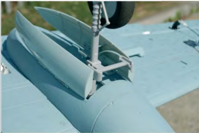
Cam operated gear doors have proved to be very reliable
