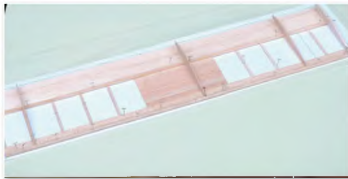
Bottom sheeting, capstrips, spar and trailing edge pinned flat and placement of ribs in progress. Don't glue ribs to leading edge sheeting yet
