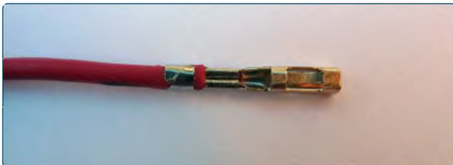
A good quality crimp. The long outer tangs are wrapped firmly around the insulation and the short inner tangs are folded tightly over the bare copper wire in an 'm' shape
