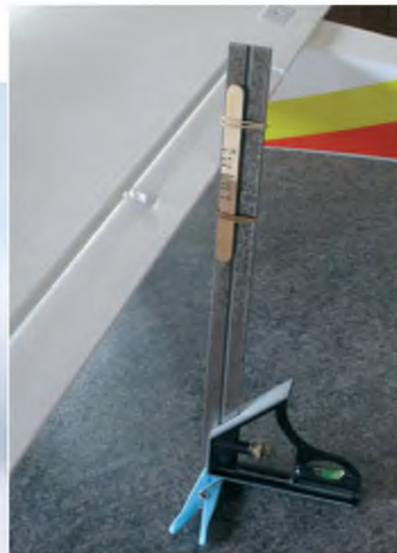
A propped up T-square was used to hold up a lolly stick marked off with the recommended control throws. Not terribly precise but good enough for setting up a sports model
