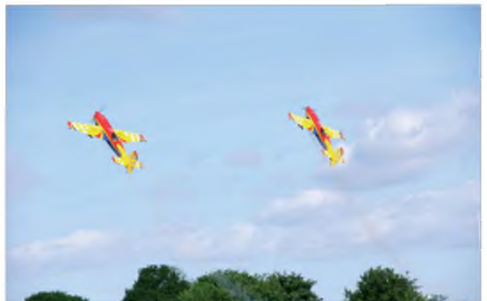
The 'German Aerobatic Team' of Ingo Brauer, Randolph Bromer and Andreas Merhout flew synchronised displays with their Krill Extra 330SC's. The 3.1 metre span models are powered by MVVS 175 NP Twinspark engines, with flight controls operated by Hitec HS-M7990 Digital servos
