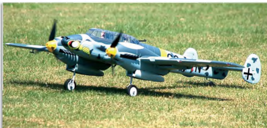
The best way to land the Messerschmitt is to run it in level and do a 'roller' landing on the main gear. Three point landings are more hit and miss!
