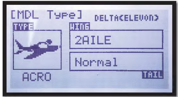
The Flash 8 also supports programming for delta/flying wing models
