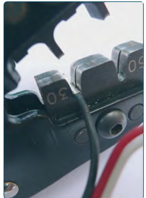
The smaller slot is then used to further tighten the crimp to make it fully secure
