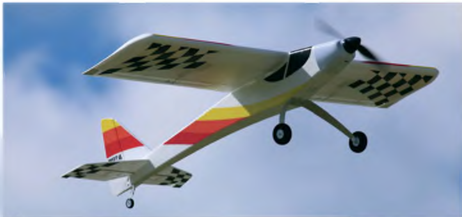
Chequerboard stickers on the underside help with orientation
