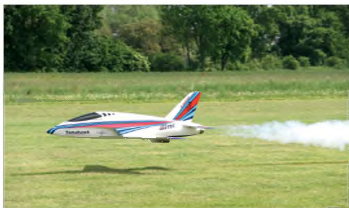
Oliver also flew this 2.5 m Futura jet. The Tomahawk Design kit is powered by a Turbine IQ Hammer 220+ and is controlled using Hitec 7954 servos
