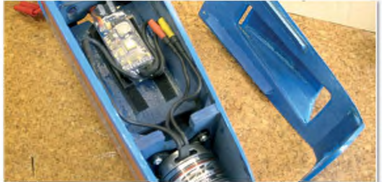
The ESC gets plenty of draft from the inlet in the lower cowl
