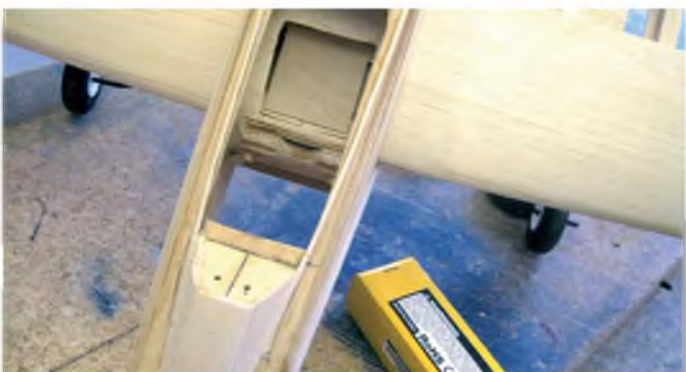
Adjust the LE and F2 to suit the LiPo pack being used
