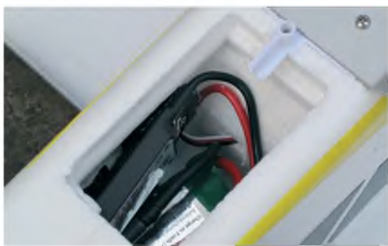
Left: I did away with the strap and Velcro'd the ESC to the fuselage side so that it could be kept above the LiPo with a good flow of cooling air
