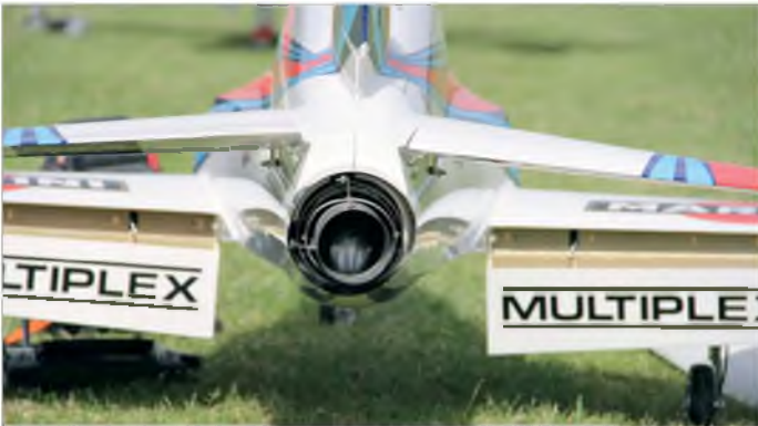
A view of the Vector Thrust Control fitted to the back end of Oliver Gräff's Futura jet
