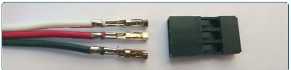
The underside of the plug and the bent tangs on the connectors should all be facing upwards. The signal wire is at the top and the negative wire is at the bottom
