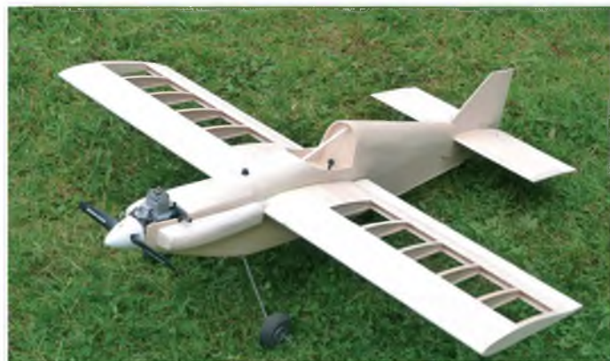
Ready for covering
