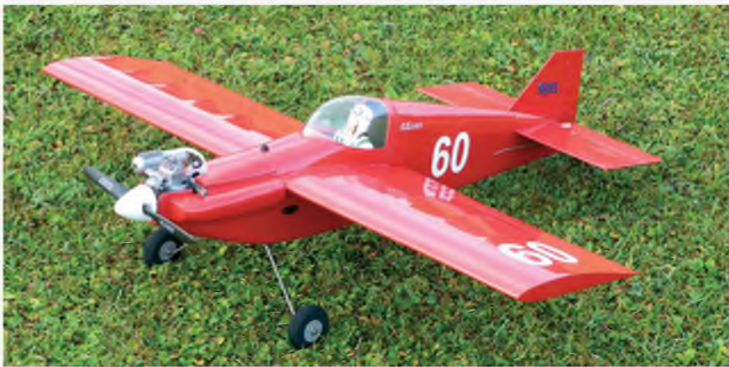
Above & below: After a thorough fuel proofing of the engine and fuel tank bays the model was covered in Super Monokote and trimmed with vinyl race numbers
