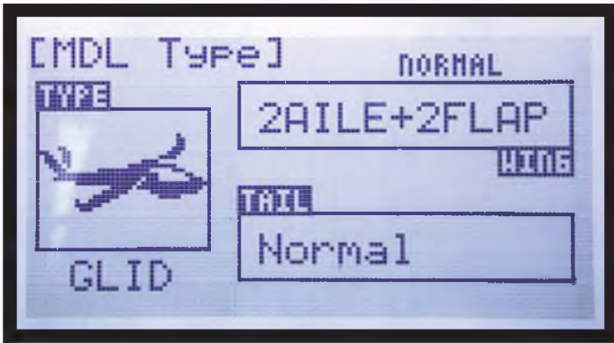
Templates, such as this one for glider wings, help speed up programming
