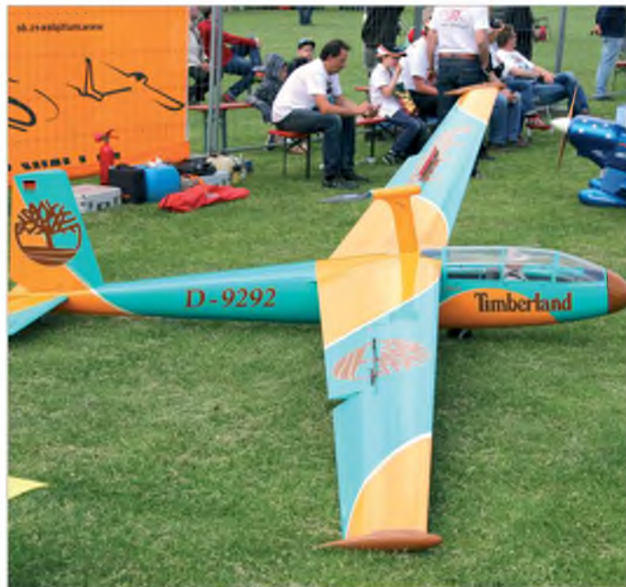
Ulf Reichmann from Hessen is a four times German Aerotow Champion. Decorated in an unusual colour scheme, his Blanik L-13 is to 1:2.83 scale and has a wingspan of 5.8 metres. Manufactured by HB-Model (Heiko Baumgärtner), the near 25 kg glider is hauled aloft by a pylon mounted Hacker C50-13 XL, via a 6.7:1 gearbox. Ulf uses an M-Link Multiplex Royal Pro 16 Tx to operate the control surfaces, including extendable Fowler flaps for increased lift
