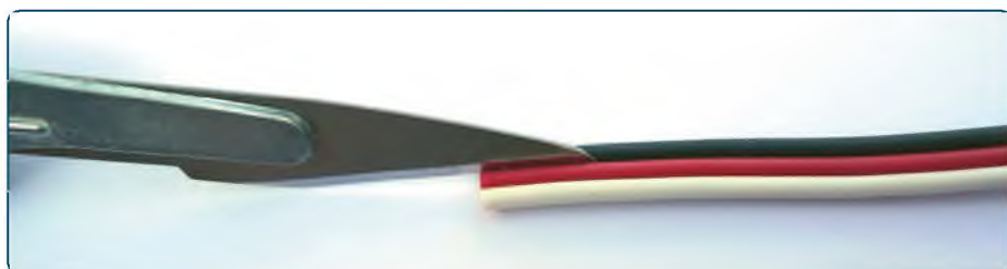
Use a sharp blade to separate the wires
