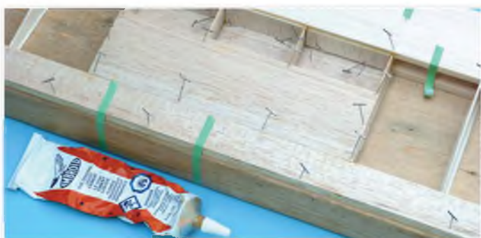
Don't forget the shear webs before closing in the centre section. Old school model cement is used for joints that require sanding, such as sheeting seams
