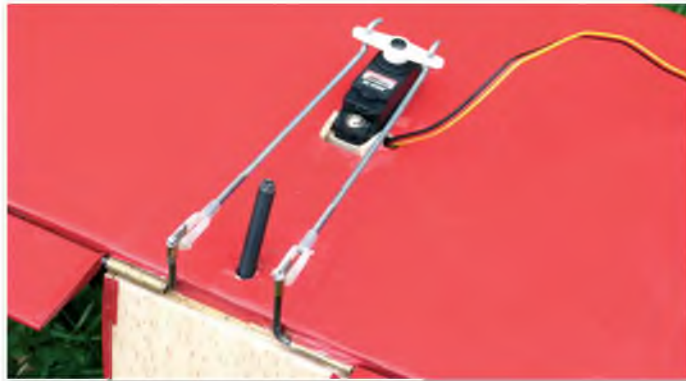
Aileron servo and linkages
