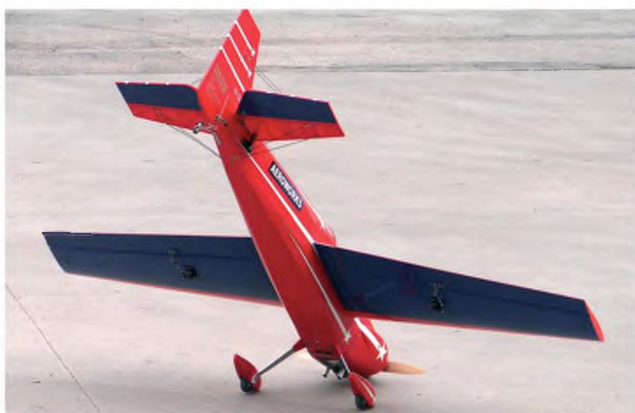
The model is pre-covered in neatly applied Ultracote, red on top, with blue undersides. Next time we show how to check over the covering and apply some additional stickers
