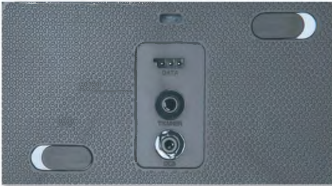
Rear ports for PC Data Interface (top), Trainer Socket (middle) and DCS port (bottom) for powering accessories like FPV goggles
