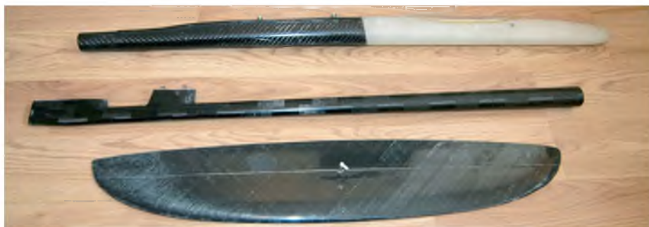
Two-piece Claymore fuselage, made in carbon/glass/Kevlar with radio friendly front section, before joining. The tailplane is from 26 g spread tow carbon on a rohacell core. High quality of construction is apparent in all these components made in the UK
