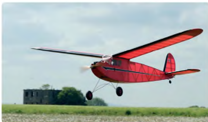
Mike Spencer's Privateer, built from plans, has an AXI 2820 turning a 2:1 belt driven gearbox. RAF Broadwell WW2 control tower in the background
