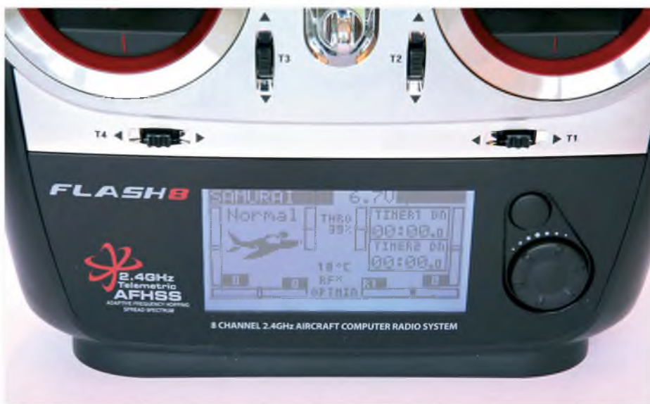
The Flash 8 has a super bright LCD screen. The radio is programmed via the Jog Dial and Back Button at the right of the screen
