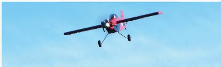
With neither dihedral nor tapered chord, the Super Sytky wing is easy to build and behaves well in flight
