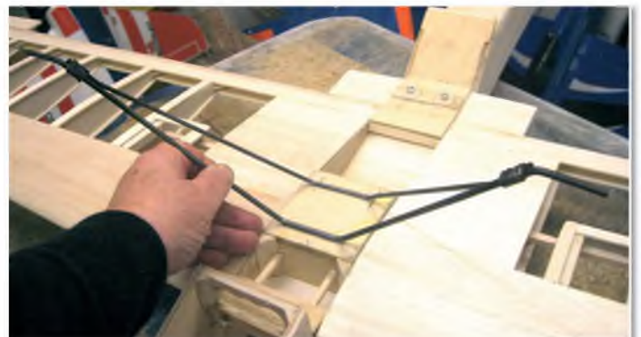
Wire U/C's are resilient and are cheap and easy to make
