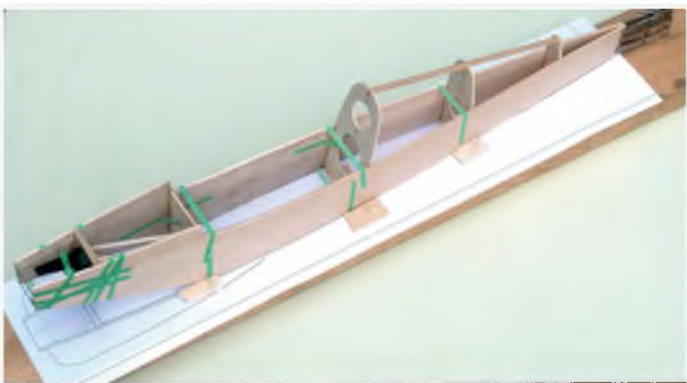
Fuselage construction underway, with rear portion flat on the board
