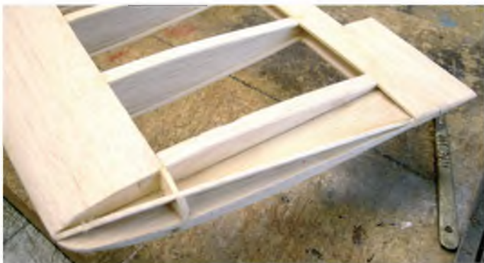
Construction of the simple wing tips
