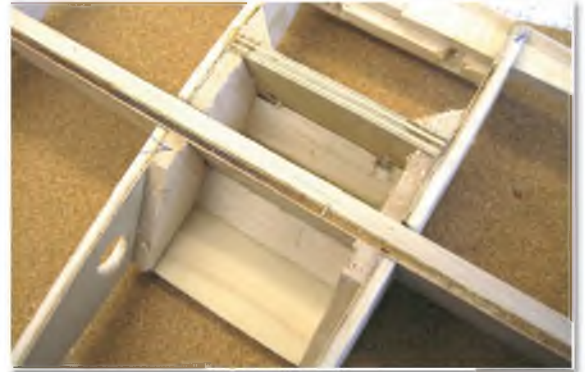
U/C mounting plate and gussets
