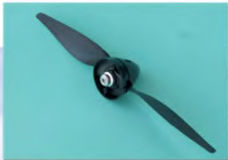
The prop, adapter and spinner assembly are the final parts to be fitted
