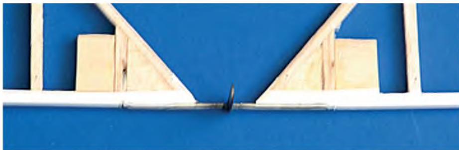
A standard ready built elevator joiner is fine for this size of aeroplane
