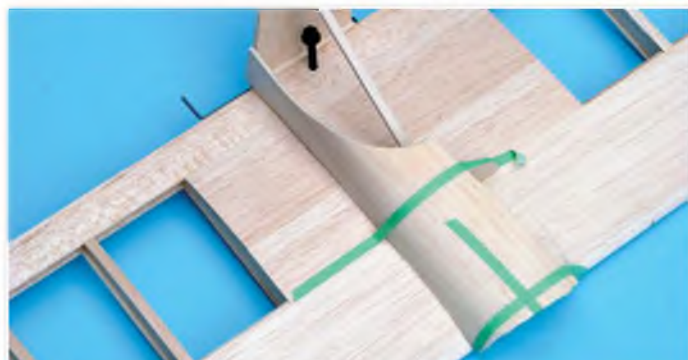
Temporary brace holds W4 as sheeting is applied
