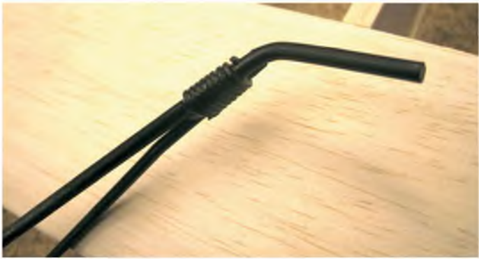
Bind the joints with copper wire and then solder
