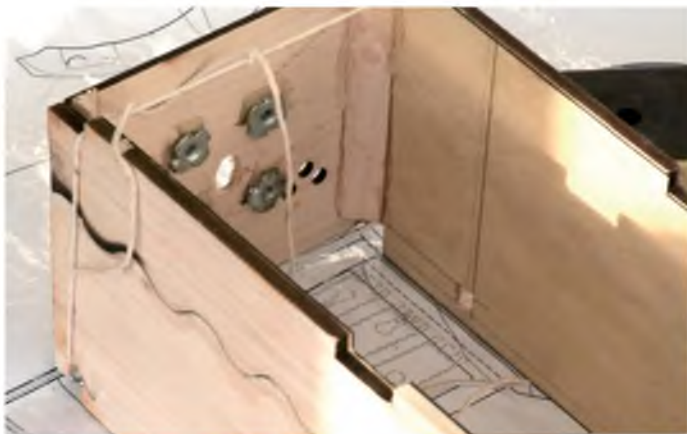
Use string as an alternative to a clamp. You don't have to have hi-tech equipment to build a model
