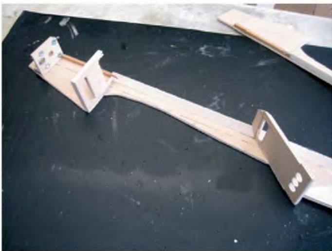
F2 and F3 in position on the fuselage side
