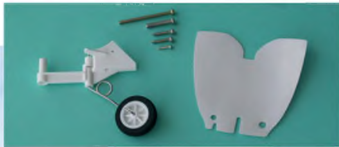
A small accessory box contains the tailwheel assembly, fixing screws and a butterfly shaped rudder reinforcement sticker
