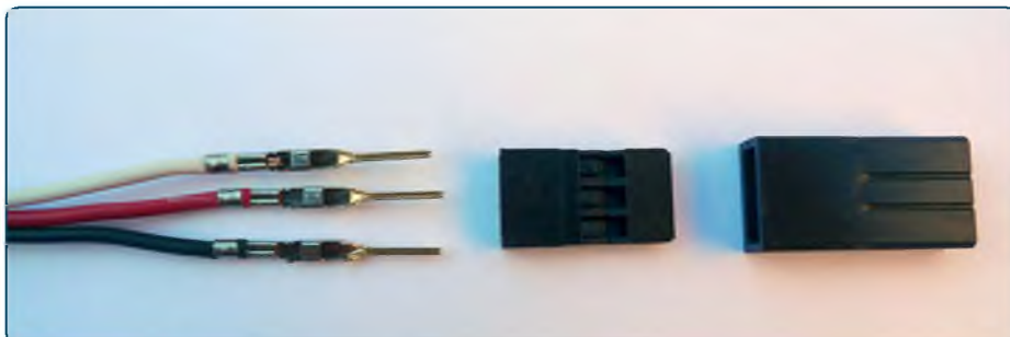
The only difference for male plugs is that the connectors will be long pins instead of sockets and there is an extra plastic part. The plug in the middle is fitted in exactly the same way
