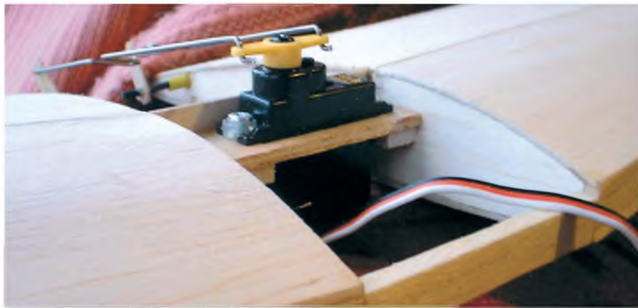
Aileron servo in place
