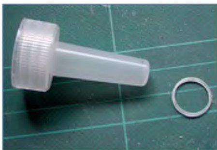
The bezel was made by cutting it from the spout of a bottle top
