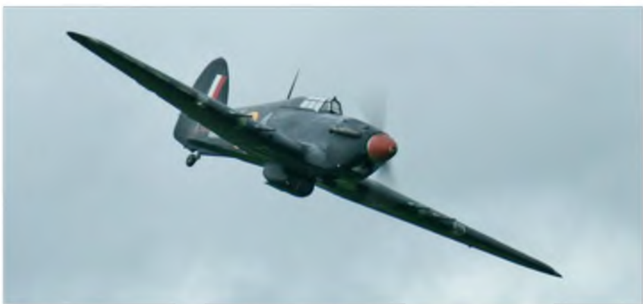
Above & below: Bickershaw MFC club member Brian Wood scratch-built this beautifully-detailed 92 inch span Hawker Hurricane (and incorporated his own design scale retracts) from a plan designed by Brian Taylor. The model uses an OS 200 for power
