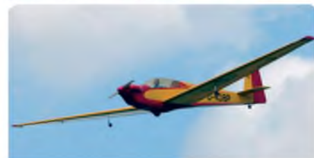
Robert Mahoney's SF24A motor glider, now flown by Gordon Tarling has 4 metre span, 8 kg weight and flies on an 8S battery, driving a brushed Plettenburg motor. Inset flight photo by Bob Corfield
