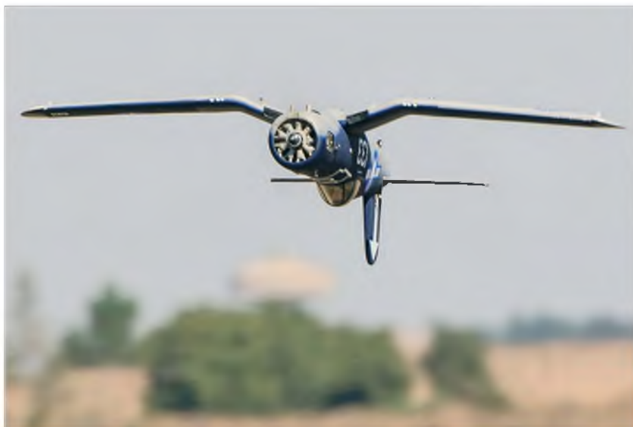
WW2 warbirds had large and heavy engines so their nose moments are short. Consequently scale models usually require the addition of lead to achieve the correct C of G (Peter Connan picture)
