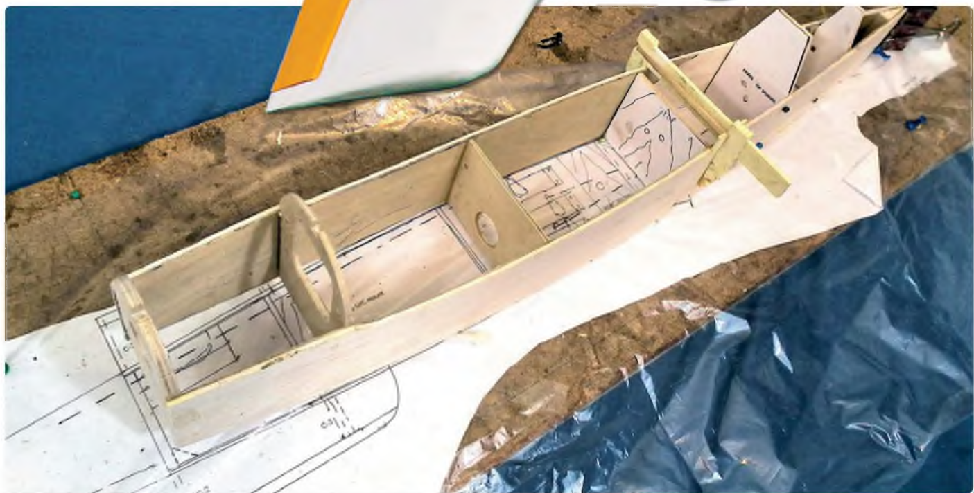
Fuselage sides and formers being assembled over the plan
