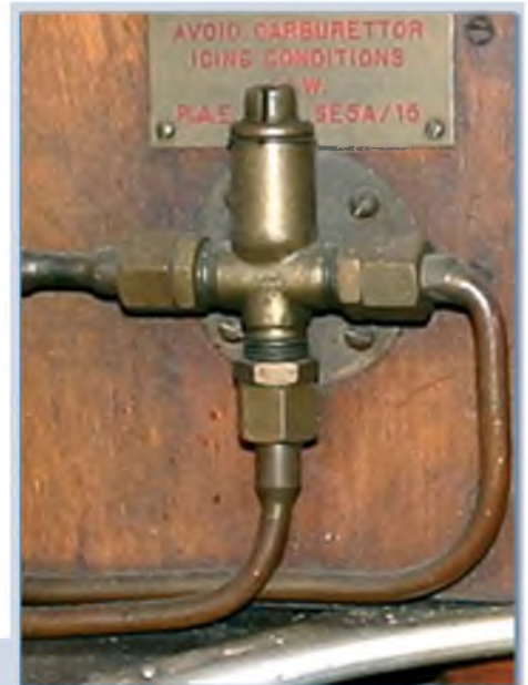
Air pressure regulator and the air and petrol selectors of the full size aircraft
