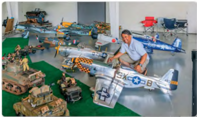
The Tidewater Radio Control Ghost Squadron, based at Chesapeake, Virginia, regularly display their models at MAM shows. I had a long chat with Ruperto Asiatico about the superb models on show. The Mustang P-51D is a beautiful replica of Jerry Yagen's 'Double Trouble Two'. The model has an 86" wingspan and a DA 50 cc petrol engine. The P-51 is covered with Flite Metal, which gives it a lovely scale finish
