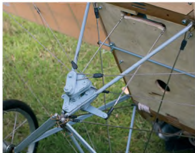
The clever wing warping mechanism, powered by a single servo, is true to scale
