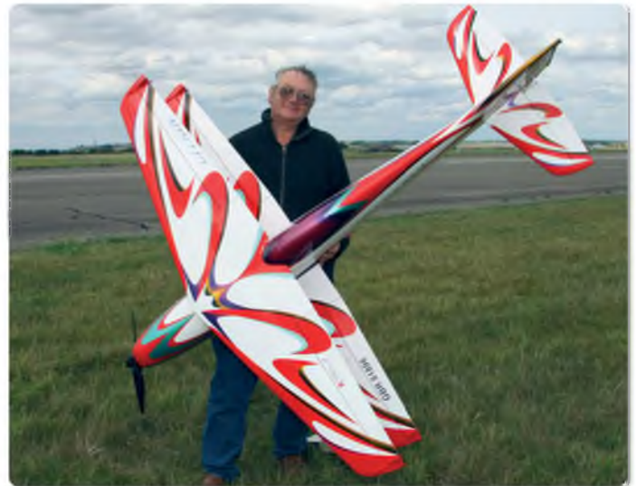
Isle of Man resident Arthur Silsby was another to favour the Oxai Citrin. Arthur's model is powered by a Q80-14 XS, fitted with a 21" x 13.5" Falcon carbon prop
