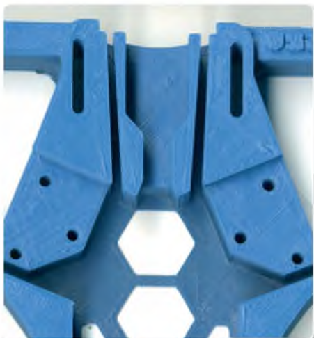
This close-up of a 3D printed quadcopter chassis shows how the shell is created then filled in
