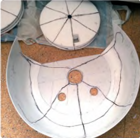
Cowling reinforcement from carbon thread soaked in epoxy
