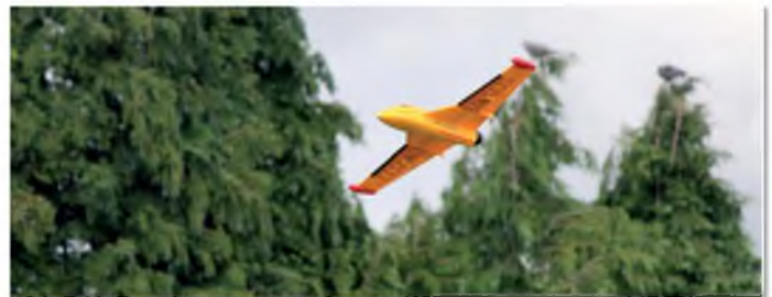
Tony Oliver's Multiplex Funjet has a 400W Keda motor on 3S 2200 mAh LiPos and a 5" x 5" prop – it goes like stink!
