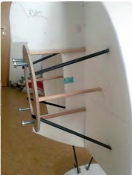
Motor mount is reinforced with wooden sticks, Depron and a bit of carbon cloth
