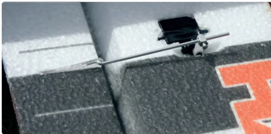
Control rods provide a direct slop free linkage
