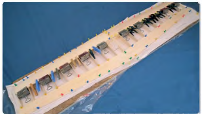
Top sheet being applied using lots of clamps and map pins
