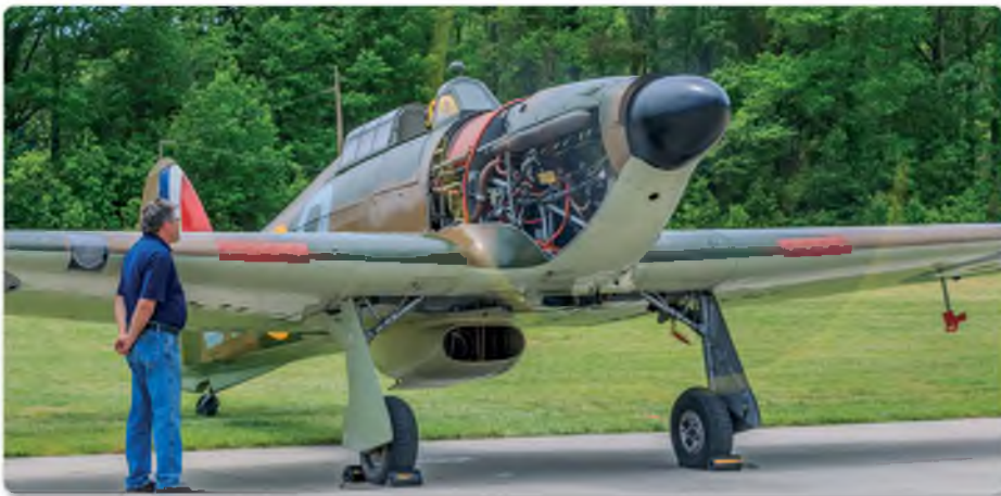
Hawker Hurricane LF Mk XII undergoing magneto checks prior to its first flight of the week
