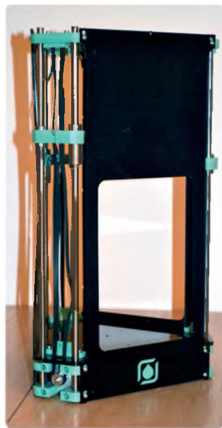
The acrylic sides provide stiffness to resist twisting. Remember to peel off the protective film
