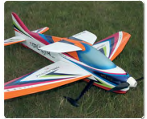
Canalisers (small upper wings) are common on F3A models, but the one fitted to Gerhard Fehringer's Oxai Galactik is huge!
