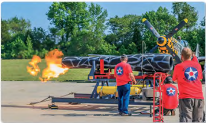
One of the most sinister sounds I have ever heard – an original working V-1 pulse jet!
