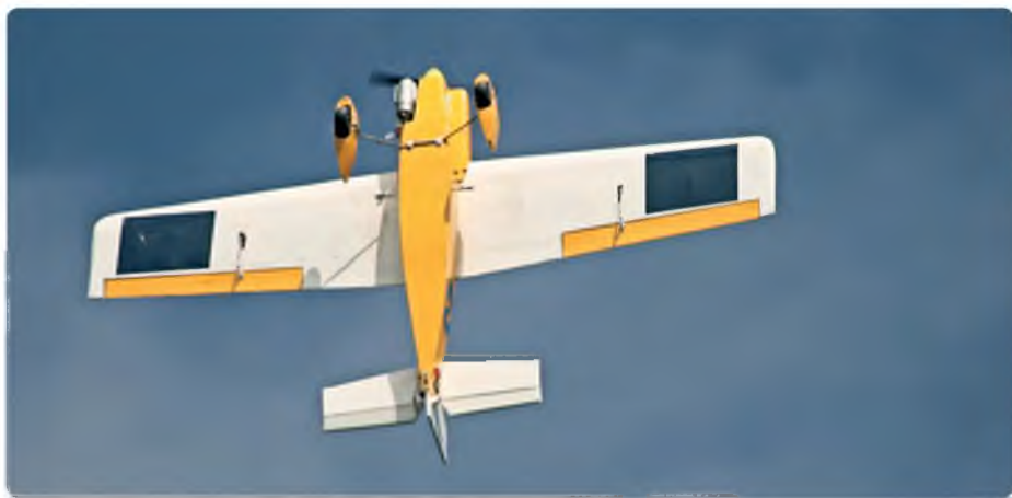
Black squares on the underside of each wing help with orientation of this speedy model
