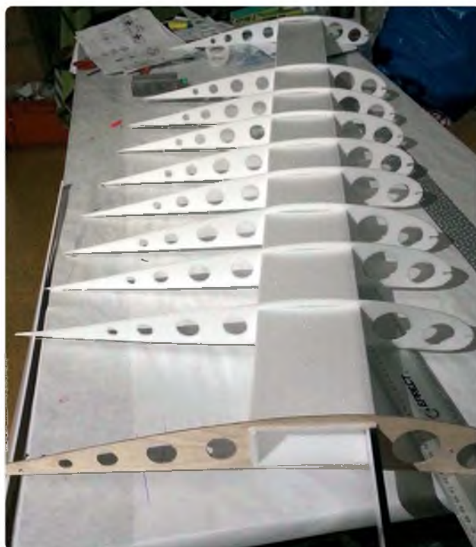
Wings partially assembled. Notice that the wing spar is formed as rectangular tube, with a flat carbon reinforcing front edge
