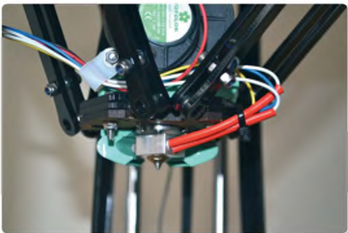
The completed Hot End mounted on its connecting rods. Correctly wiring the heater, thermistor and cooling fan is a critical step
