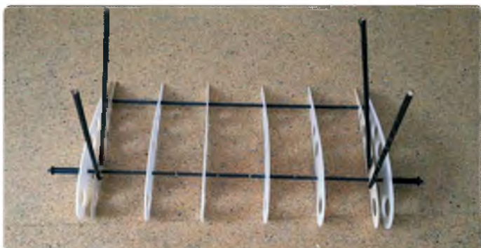
Landing gear beginning to take its shape. The additional lifting surface is built the same way as the main wing
