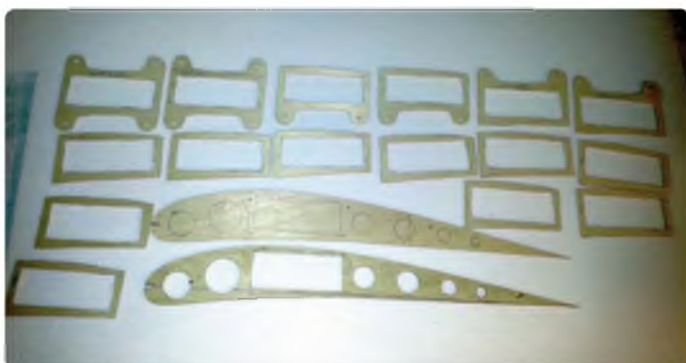
Some of the parts and ribs that will hold the wing structure together must be rigid are made from thin plywood
