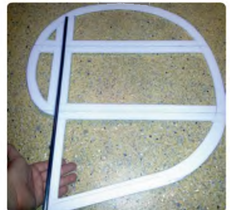
The rudder is built from 6 mm Depron and reinforced with carbon tube before covering all surfaces with thinner Depron
