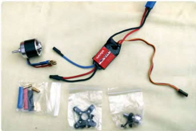
Hacker motor and 22 amp ESC with the supplied battery connector, which accepts both XT60 and EC3 plugs
