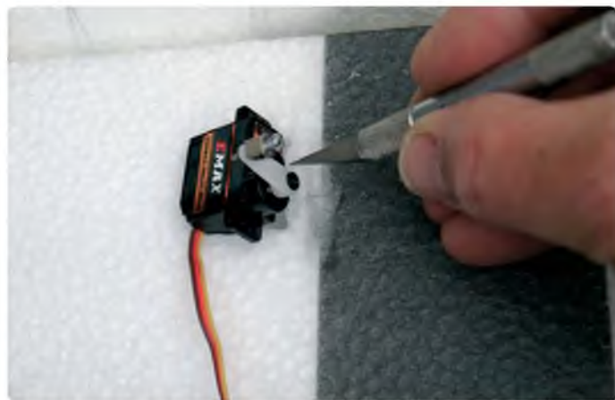
Recesses for the servos need trimming with a sharp knife to take your chosen units
