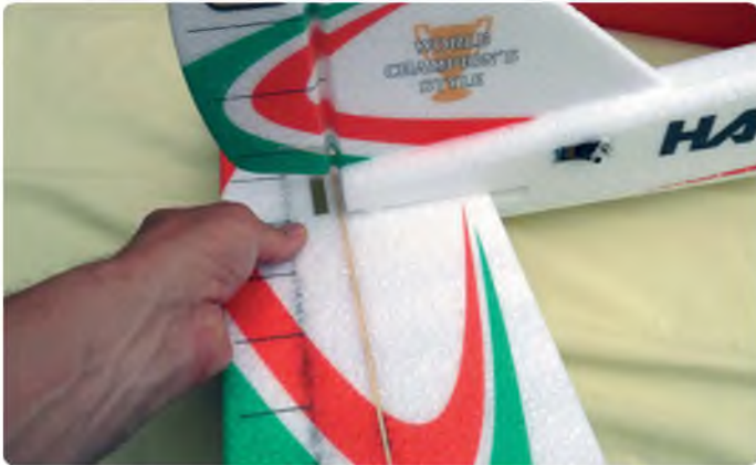
Horizontal stabiliser slots into position
