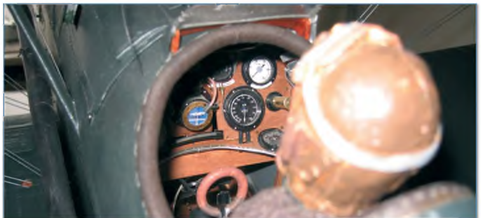
Most cockpits are located near to the C of G so the additional weight of extra scale detailing doesn't have too great an effect
