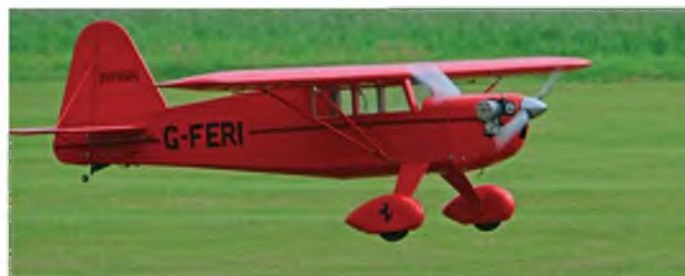
After acquiring it, Liverpool club member Barry Sherborne re-covered and lightened this 1:4 scale Rearwin Speedster 01, powered by a Moki 210
