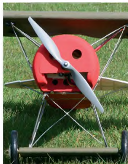
Holes in the cowl and in F1 former make for a cool running installation
