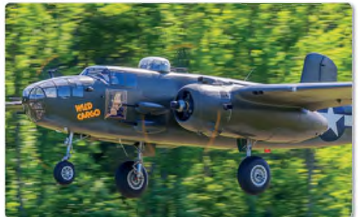
Gerry Yagen's B-25J Mitchell 'Wild Cargo'. It started its military career as a surveillance aircraft with a 'solid' nose section. The B-25 was restored in 1997 and the clear nose section was added, taking the B-25 back to the original 'J' specification
