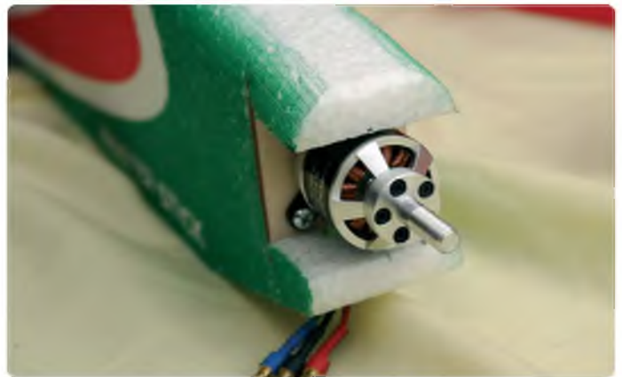
Motor is easy to fit and the exposed location will provide good cooling
