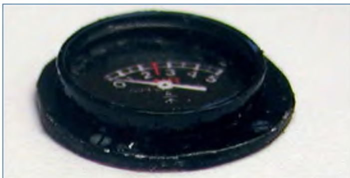
The bezel was made by cutting it from the spout of a bottle top
