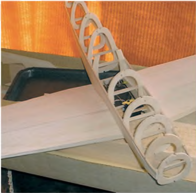
Fuselage formers in place
