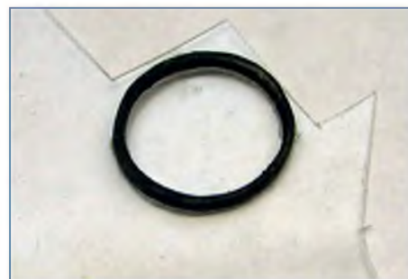
The bezel was made by cutting it from the spout of a bottle top
