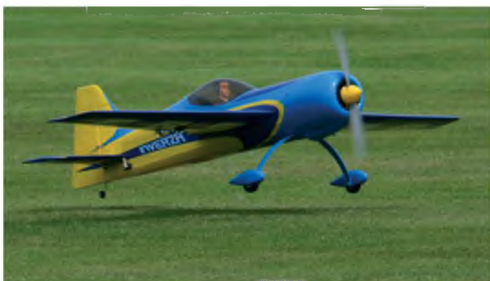
Blackpool MFC member John Higgins flew his 72 inch span electric powered Hangar 9 Inverza, fitted with a Hyperion Z5035-20 motor, a 100 A ESC and 12S 5000 mA LiPos turning an APC 20" x 10" E prop
