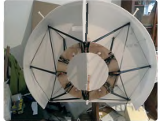
Final view of reinforced motor mount
