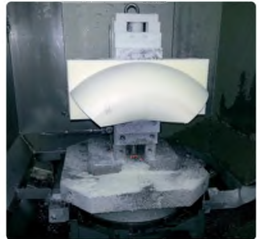
Cowling parts are made using a milling machine. Hard styrodur foam is used for this
