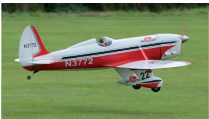
Ian Bottell's 92 inch span Blackhorse Ryan STA has a CRRC 26 cc petrol engine up front. Ian is a member of the Wirral MFC
