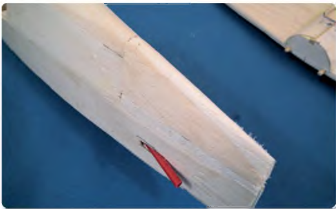
Tail fairing blocks being shaped
