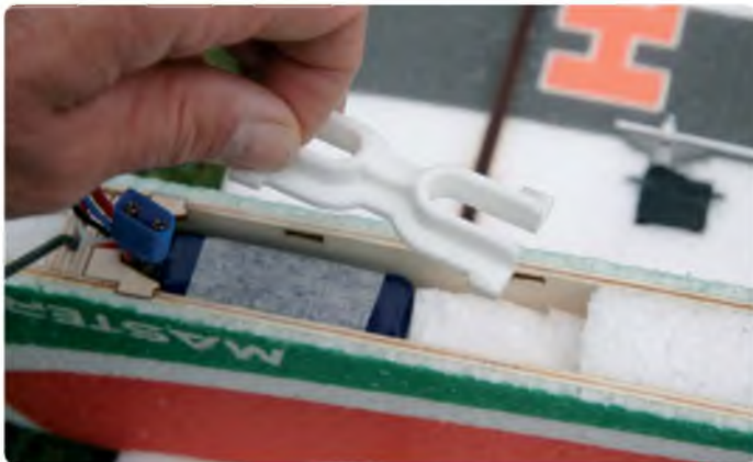
The LiPo is fitted from the underside and held in with a simple plastic 'X' brace, which locks into slots in the ply reinforcement. Note the foam spacer to make sure battery doesn't slide backwards
