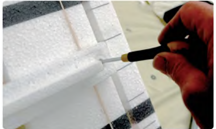
The horizontal stabiliser is held in place with a machined screw. On the review model the plastic housing in the fuselage hadn't been tapped to suit
