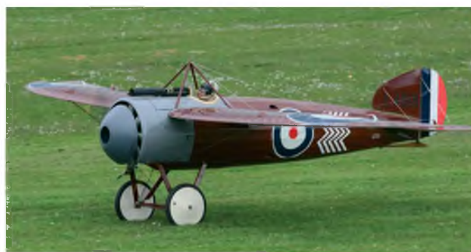
Jim Reeves (allegedly from Yorkshire!) brought along his Mick Reeves Models 1:3 scale, 122 inch span Bristol M1c, which was designed by his father, Mick. The model weighs under 15 kg, including 3 kg of batteries and a Turnigy motor
