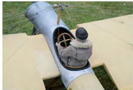
In the Yorkshire event Peter Willis from the Thirsk MFC flew his Blackburn Monoplane, built around 15 years ago from a K&W kit. Note the yards of wire rigging and complicated wing-warping pulley system
