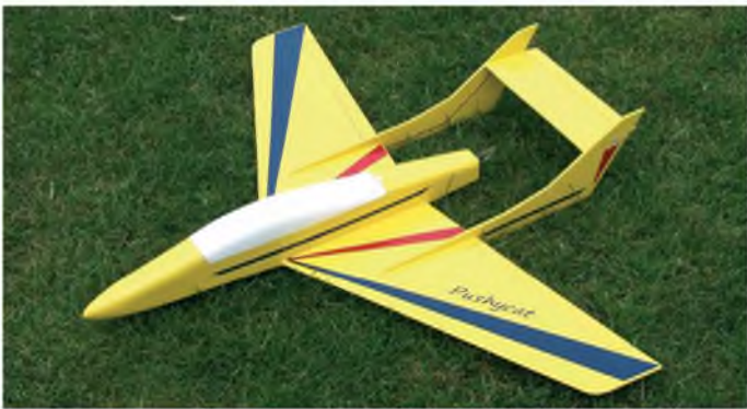
Built-up twin-boom pusher Pushy Cat 'prop-jet' from Dave Sanderson – great performer, re-engined from brushed to brushless power
