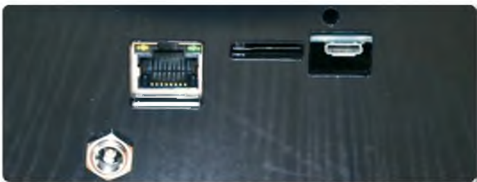
The rear panel connectors to the Duet board. From left to right: DC power, Ethernet, MicroSD, USB
