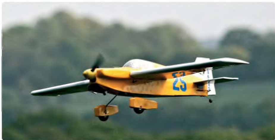
Spats don't like grass very much. A quick bend and they are straight and ready to go
