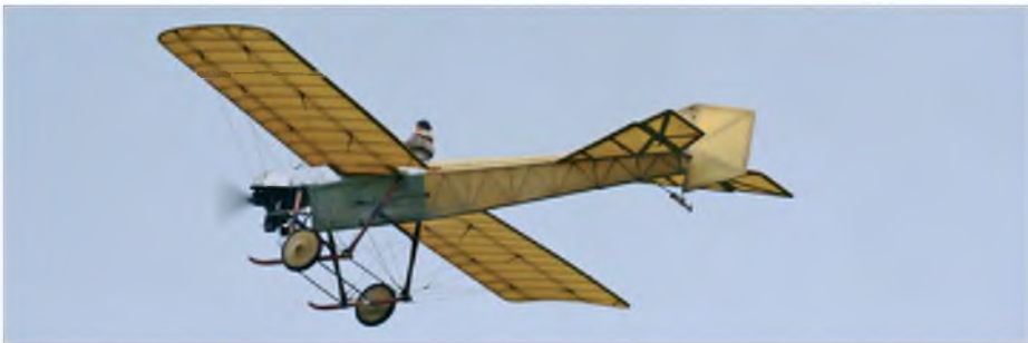
In the Yorkshire event Peter Willis from the Thirsk MFC flew his Blackburn Monoplane, built around 15 years ago from a K&W kit. Note the yards of wire rigging and complicated wing-warping pulley system
