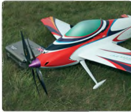
Close-up of contra-rotating props used by many competitors. The props free-wheel in one direction only, to provide braking and control the model's speed on the downside of the loop
