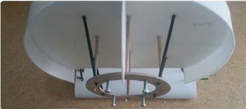
Motor mount ring is made from plywood
