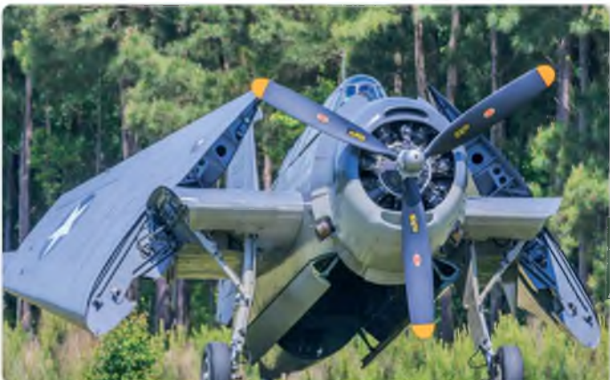
Douglas TBM-3E Avenger sits with its wings folded back waiting to fly
