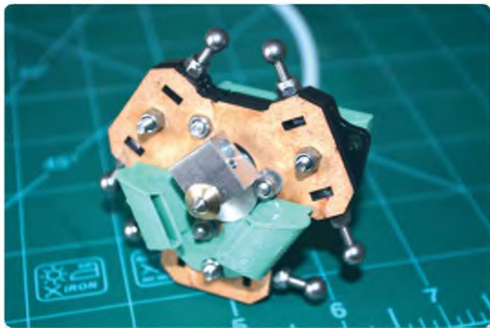
A close-up of the assembled Hot End showing the heater block, extruder nozzle and air duct
