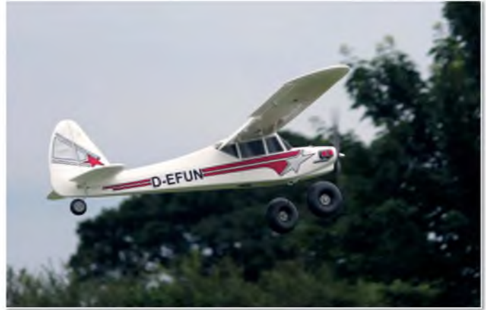
Jason Rigg flew this Multiplex Fun Cub on 2200 3S LiPos – the big wheels work very well
