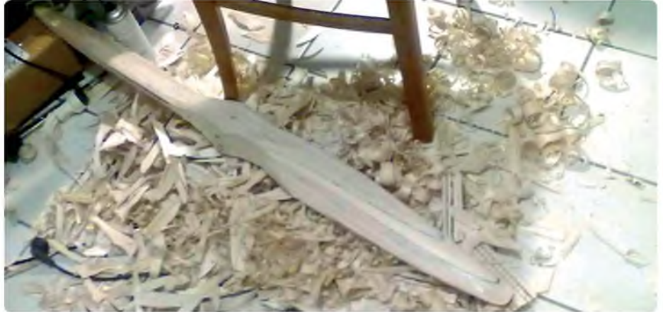
The old style way of making something special! A pile of balsa wood is left on the ground before the masterpiece, a 52 inch (127.5 cm) propeller, is born
