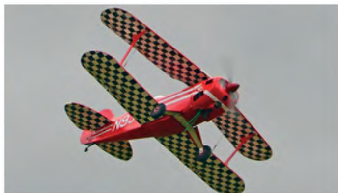
This Laser 1.80 four - stroke powered 1:4 scale FSM Pitts Special ARF was flown by Keith Fear from Skelmersdale MFC. The model spans around 63 inches and weighs in at around 13 lb
