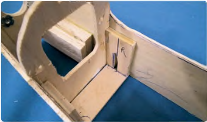
Showing the undercarriage mounting inside the fuselage
