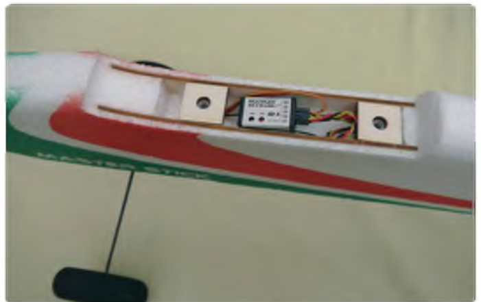
Receiver sits below the wing. Space is tight so a compact receiver is required
