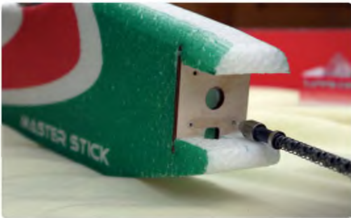
Motor bulkhead is pre-drilled for the self-tapping screws. Two of the holes were plugged with glue and needed to be re-drilled before the screws would 'bite'
