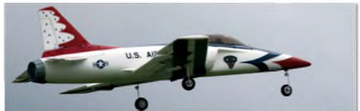
The Habu has the optional retracts which handle grass landings well but it prefers the bungee for take-off
