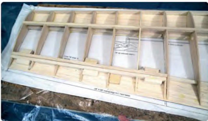
Blocks and ply plate in the aileron before adding top sheet
