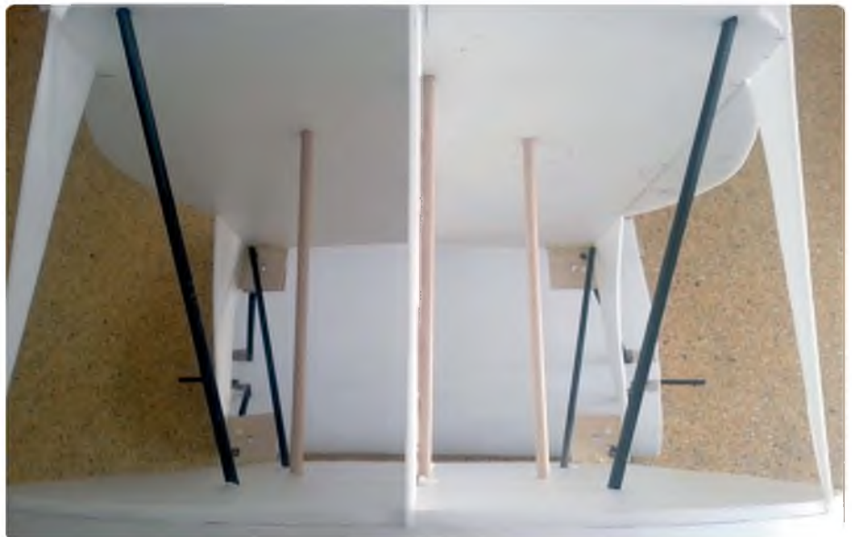
Motor mount reinforcement does not end at the firewall. The wooden sticks go deep inside the fuselage and are glued in several places. This noticeably increases strength
