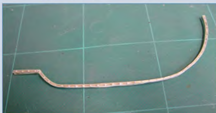
Making the cockpit coaming from litho plate
