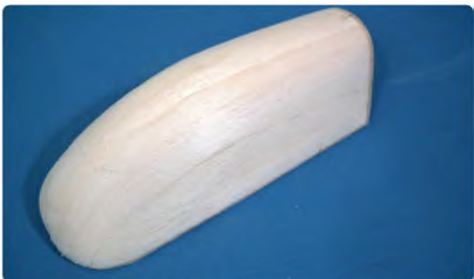
Canopy pattern carved from balsa wood. Line the bottom and end with light ply as the shrinking bottle will crush the balsa
