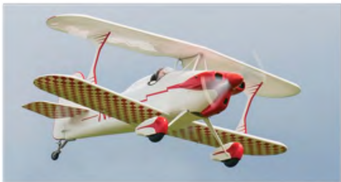
This 1:4 scale L'il Toot is only 57 inches span! It was constructed by West Yorkshire MFC member Colin Terry from a Phillip Kent plan (Traplet plan MW2762) and has a flying weight of 10 lb. It is powered by a Laser 1.20 four-stroke
