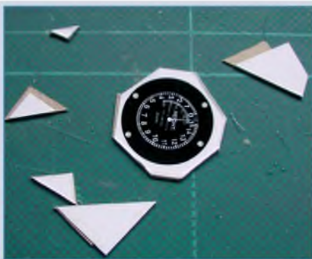
The printout is glued to thin ply and carefully trimmed to size
