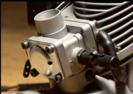
Pumped-carburettor for greater consistency and ease of operation
