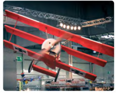
Fokker Triplane in flight at the 2015 Dortmund Intermodellbau Expo. The hall was about 30 m by 30 m and 10 metres in height. This was enough to make safe flights for this big, yet very light (just 6 kg) aeroplane
