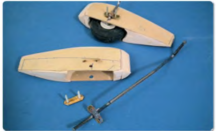
Spats completed and showing the mounting system
