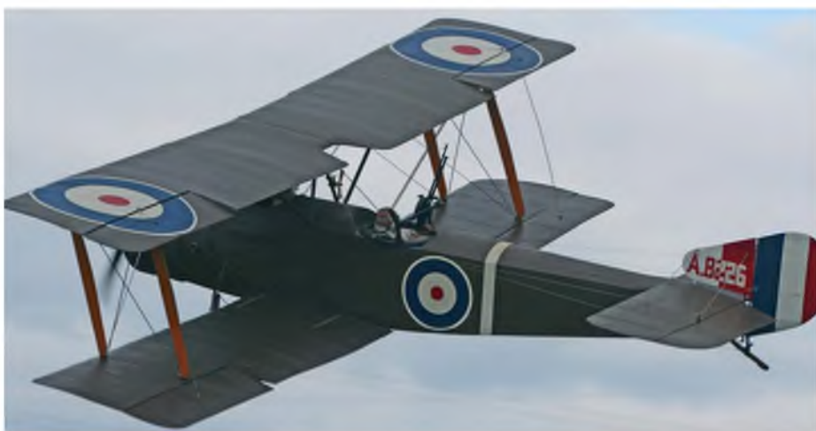
Above & below: Representing Yorkshire (in his dreams!), Mick Reeves flew his own design 112 inch span kit Sopwith 1½ Strutter at 1:3.6 scale with a Laser 360 twin
