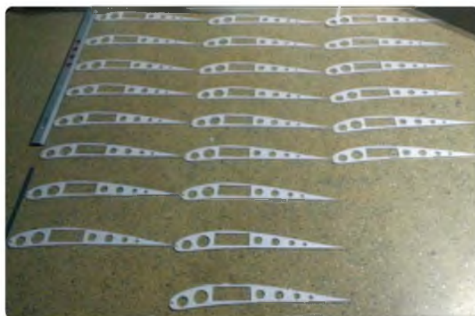
Wing ribs are made from 3 mm Depron
