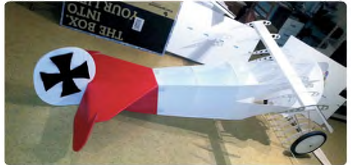
The tail section is painted. Painting the entire airframe took 14 spray cans (each 300 ml) and added 150 g of weight
