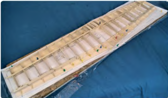
Wing construction. The lower leading edge sheet has to be raised and glued to the leading edge and ribs next
