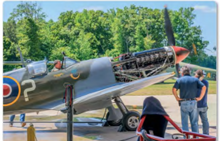
The aircraft at MAM are really well looked after but occasionally things go wrong. The Spitfire's Merlin was running very lean and could not be fixed in time for the show. A sticking carburettor diaphragm was later found to be the cause
