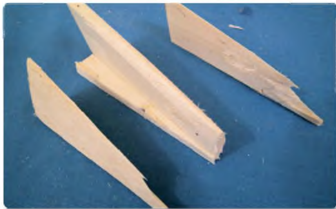
Fairing blocks separated from the sacrificial pieces
