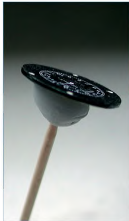
A cocktail stick and a blob of Blu-Tac holds the instrument for sanding and whilst the edge is painted
