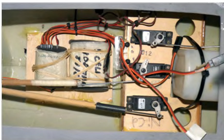
I like to try to keep my installations as neat as possible. The 35 MHz receiver and NiCad are packed with foam to reduce the effect of vibration. A 2.4 GHz receiver should not be wrapped in foam due to the heat it creates but it is also less sensitive to vibration
