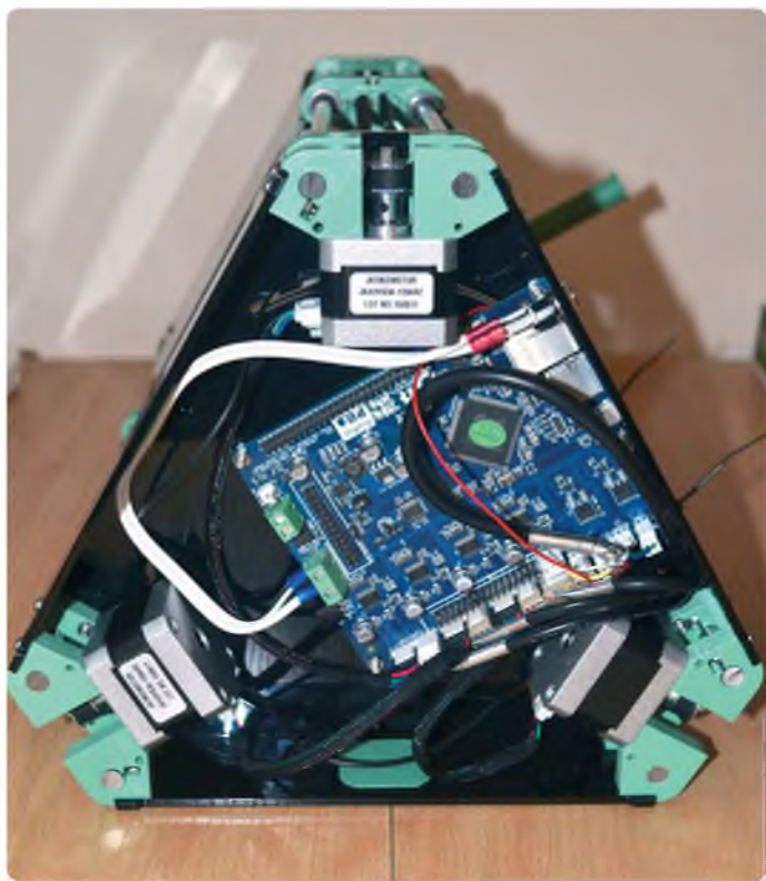
Follow the wiring diagram carefully when connecting components to the Duet board
