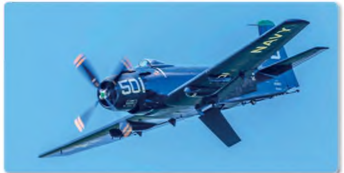
Best display of the weekend was undoubtedly by Kevin Sinibaldi in the massive Douglas AD-4 Skyraider. Seen here diving down with the huge dive brakes deployed
