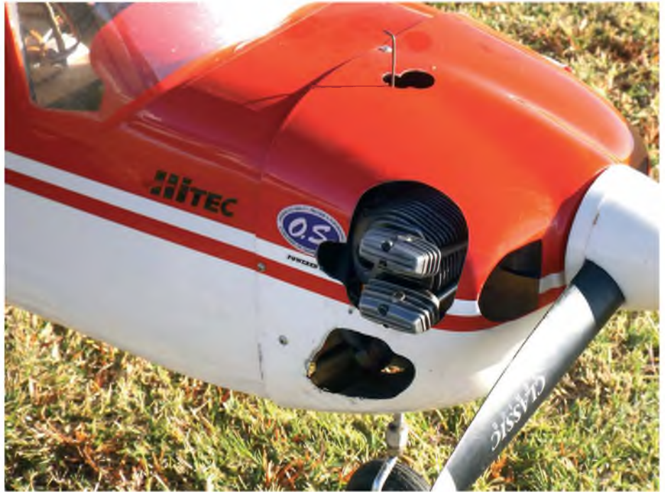
The Phoenix Cessna cowl showing the large holes leftover after fitting an over-sized OS 200
