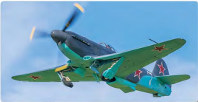
The Yak-3 was restored by the Yakovlev Company in Russia and uses many original parts. The engine is an American Allison V-12 engine
