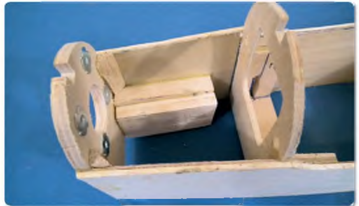
View inside the tank bay showing the sheet where the silencer recess is carved out
