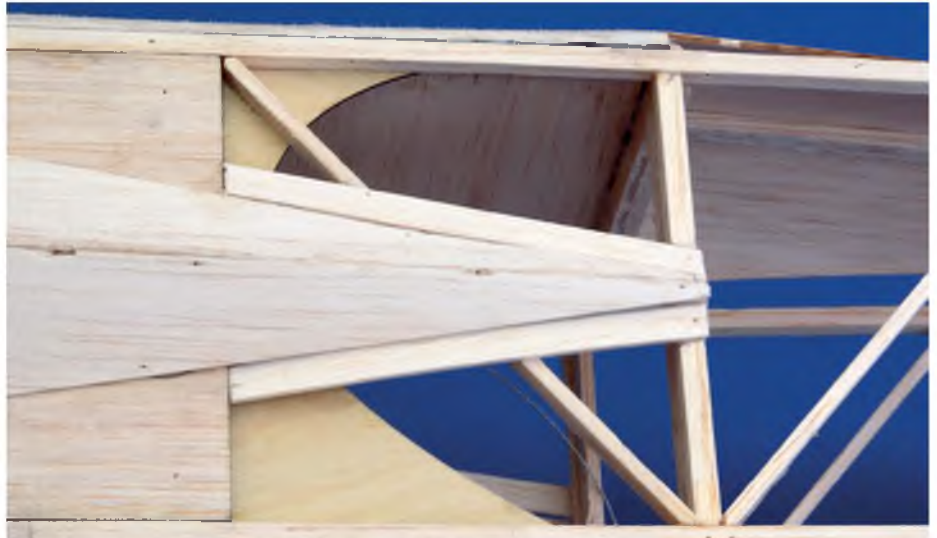
Overcoming the problem of fixing heat shrink covering to a convex shape. The extra balsa can be coated with BalsaLoc or a strip of Solartex and then iron the covering into the crease between the side sheeting and fuselage side
