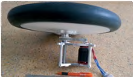
Having fun with a wheel. Using a motor mount to make sure the wheel axle is in the right position. The tyre used is from a small bicycle and is inflatable
