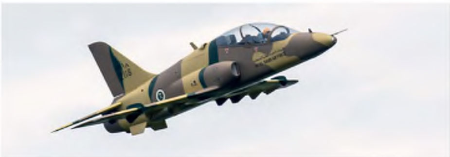
Above & Below: This highly-detailed BAE Hawk is from a Fly Eagle composite 2 m kit and is fitted with a ATJ 170 turbine. It flew superbly in the hands of its owner, Paul Lawton from the Bickershaw MFC
