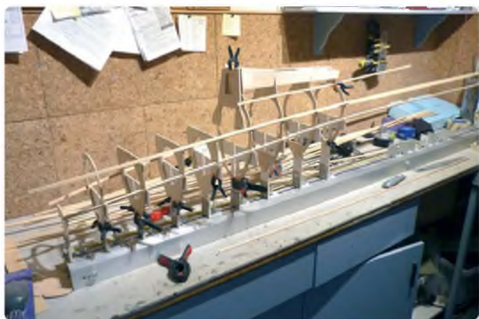
First stage of construction. Note the purpose built aluminium jig used on prototype
