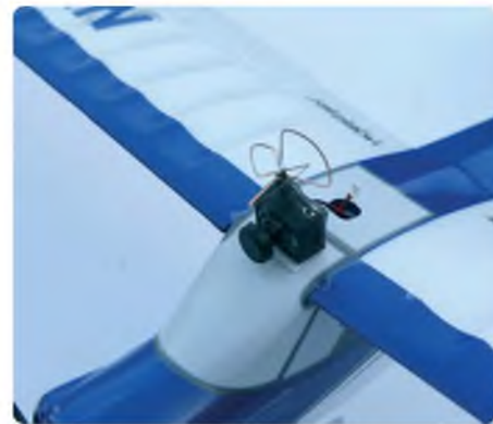
Open up the top of the cub and the Y-lead for the camera is exposed and ready to use
