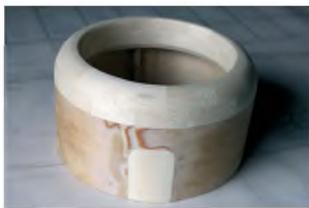
Cowl showing the patch where the Laser cylinder head protruded. But it was not required for the OS brushless motor
