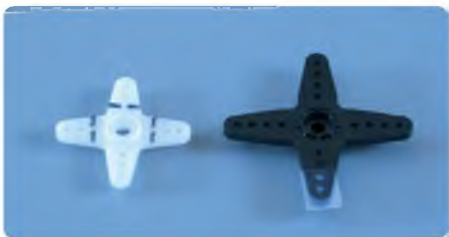
Once you have identified the arm that gives you the most neutral setting you may want to cut off the other arms to give the servo a neater appearance. With white arms, like the JR one on the left, the unwanted arms can simply be marked using a permanent marker pen. But for black arms, like the Savox ones we intend to use on the Laser, a small tag of clear tape provides easy identification of which arm to keep
