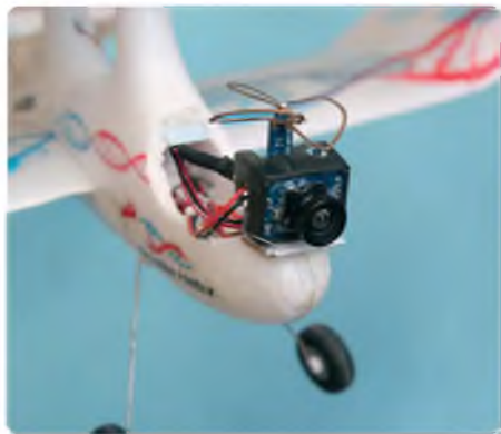
The nose mounted camera gives a superb forward view
