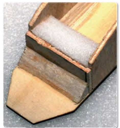
Rear support faced with foam and reinforced with triangular balsa
