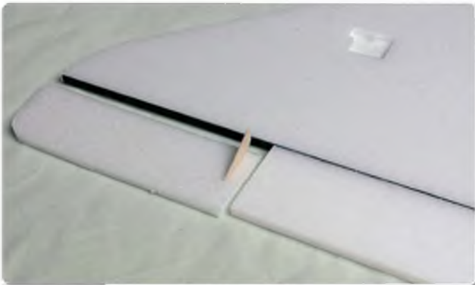
The wing is reinforced with carbon strip
