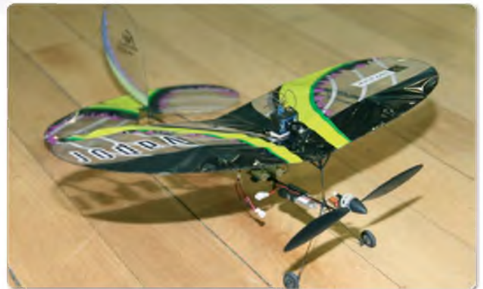
My original Vapor fitted with the mid-wing camera mounted on a 0.5 mm ply plate supported underneath by two balsa triangles
