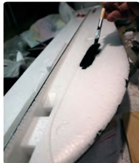
The 'canopy' has to be painted. I found it easier to paint before the wings and tailplane had been attached
