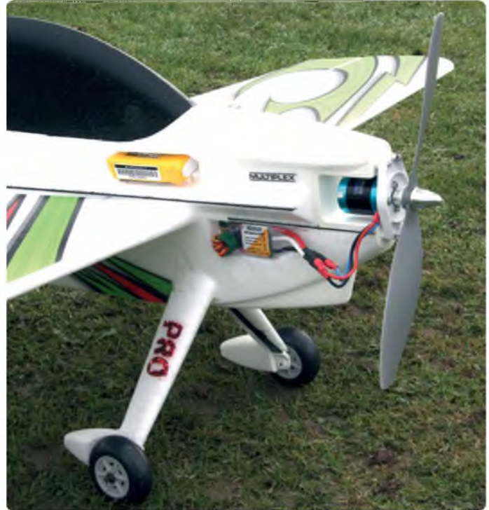
The motor fixes to the adjustable bulkhead and the speed controller is held in a recess with hook and loop tape. Servo cable and battery wires are routed through the fuselage for a tidy installation. The wings have a slot for the ESC plug, which is an exact fit for the Multiplex six pin plug supplied
