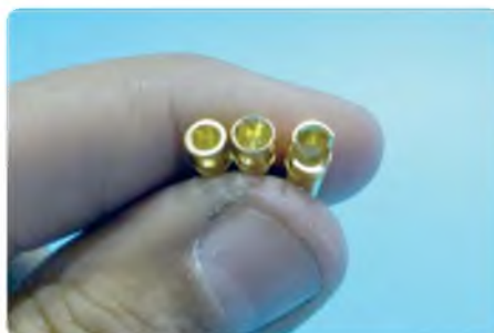
Three 4 mm gold connectors, which all have different sized soldering buckets! A bigger bucket makes fitting larger wire much easier
