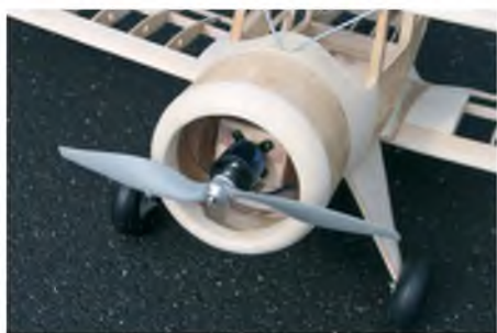
After experimenting with small EP models, Phillip converted his latest scale ship to electric power, building a motor box around the original engine bearers
