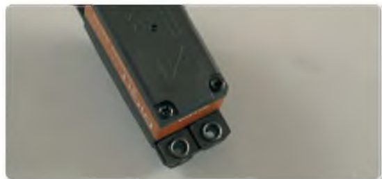
When correctly installed the grommets and spacers should look neat and tidy
