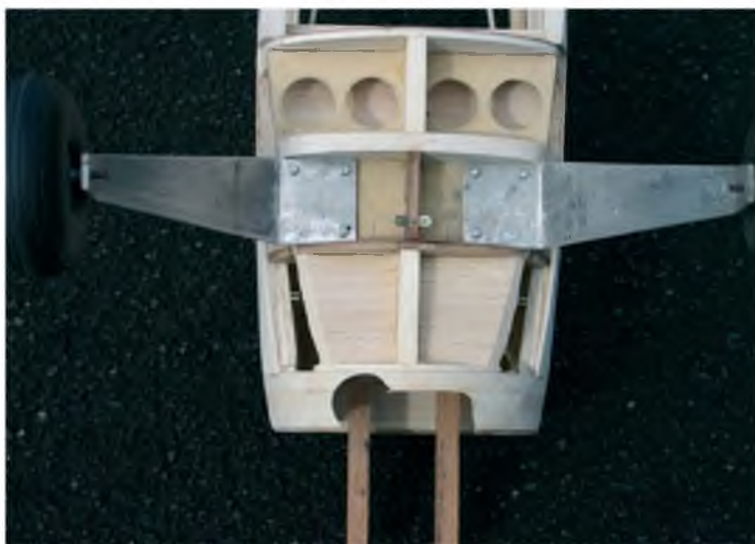
The undercarriage was adapted from a spare aluminium blank
