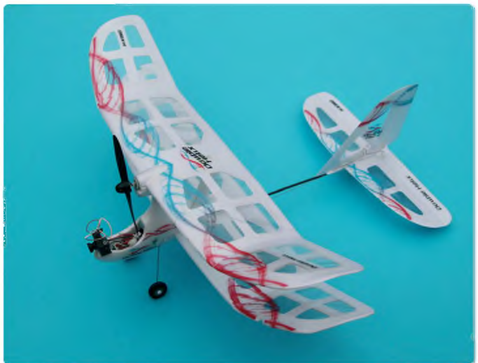
The position of the prop makes the Double Helix ideal for safe indoor flying
