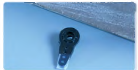
After cutting off the unwanted arms the cut edges can be smoothed off with a sanding block. A fine Perma-Grit block is our preferred tool for this job as it provides a good grip
