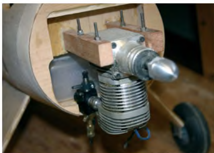
Laser 70 bolted in position. The fuel tank can just be seen, mounted transversely across the fuselage
