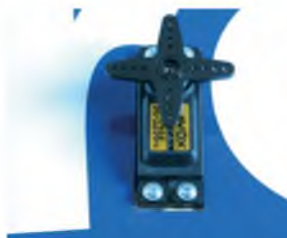
the case of JR servo arms you will often see a number 1 to 4 marked on the underside, so it is worth keeping a master set containing one of each number with which to make your final selection
