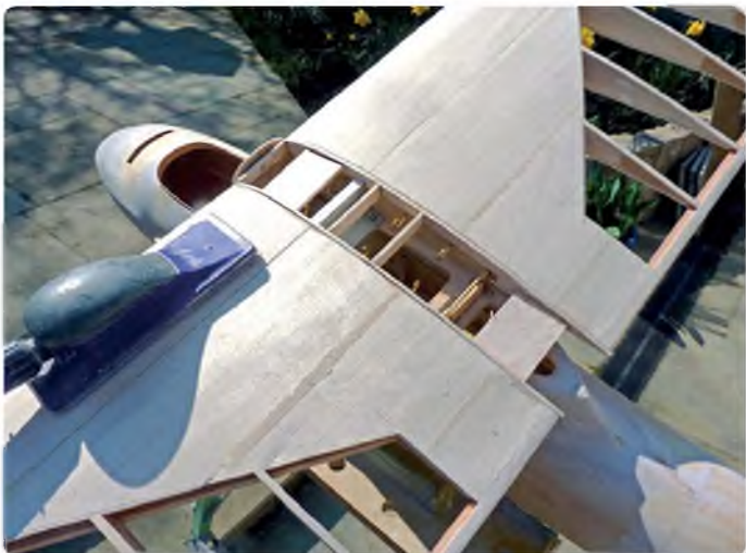
First stage of wing fairing construction
