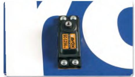
The mounting screws should be tightened down until the rubber grommet just starts to twist. Then back the screw off a little bit until the grommet lines up square to the mounting lugs once again. If your grommets are too tight then they will not be able to help isolate the servo from any vibrations. Also, be sure to use all the servo mounting screws, grommets and spacers provided. If you only use two screws to mount a servo supplied with four mounting lugs then the servo will rock in use. This will cause slop in the controls and stress the lugs. They may even break, causing the servo to break loose
