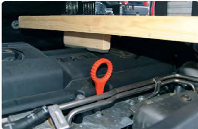
Some wooden skirts support the table board in order to bring it in an equal, horizontal position when sitting above the engine compartment
