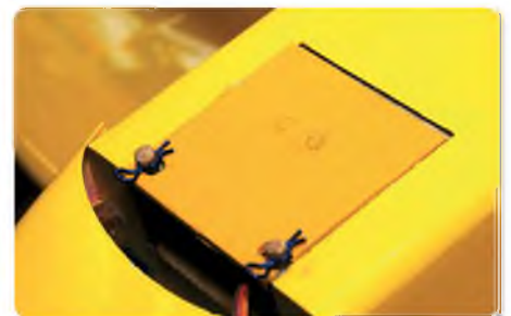
Hatch held in place with R clips in pegs
