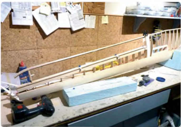
First stage of aileron construction
