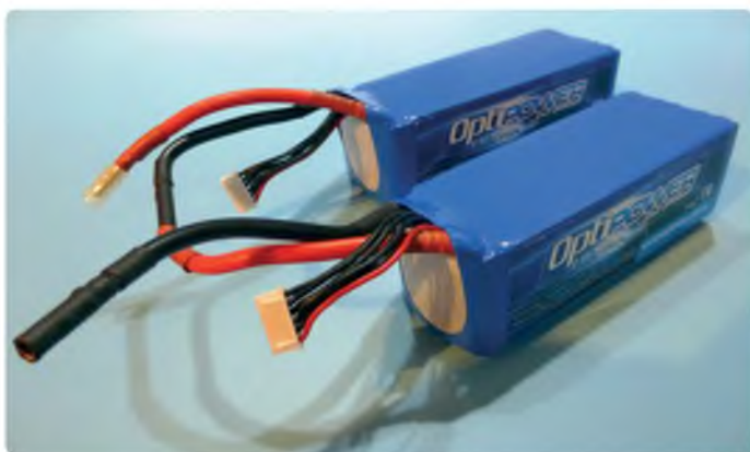
Using stand-alone bullet connectors allows batteries to be easily wired in series without the need of a patch lead (2 x 5S packs = 10S). However, the risk of a direct short is there so this method is NOT RECOMMENDED
