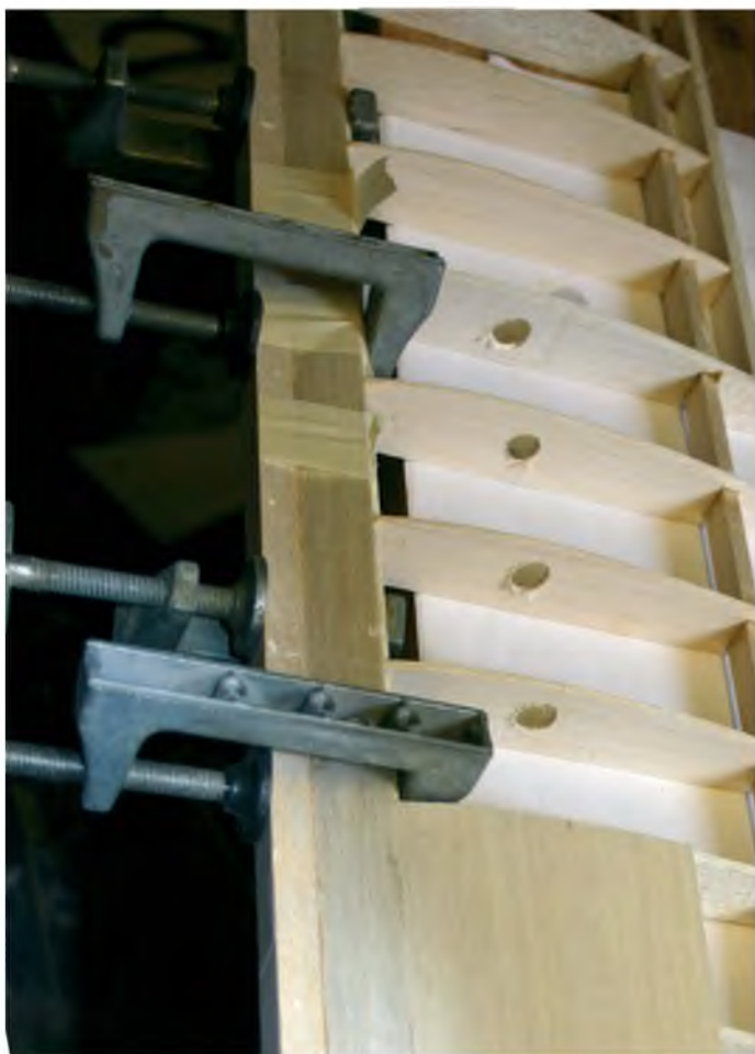
Capping the leading edge on the lower wing
