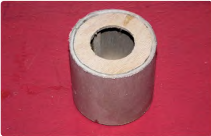
Basic crankcase. The front face is covered with 1/64" ply before the 1/2" balsa ring is glued on
