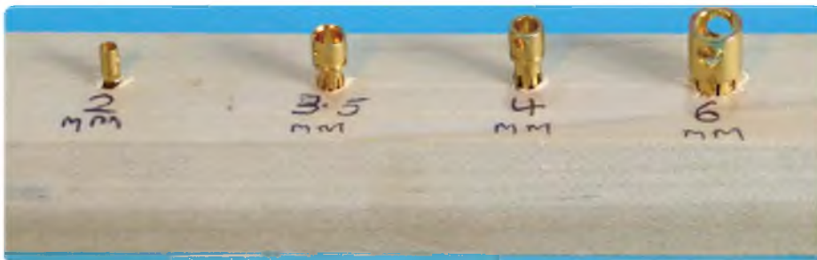
A piece of wood drilled with relevant sized holes makes an ideal soldering jig – simple but effective!
