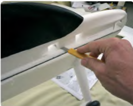
A foam block has to be removed from the battery bay in the fuselage. A sharp knife makes short work of this
