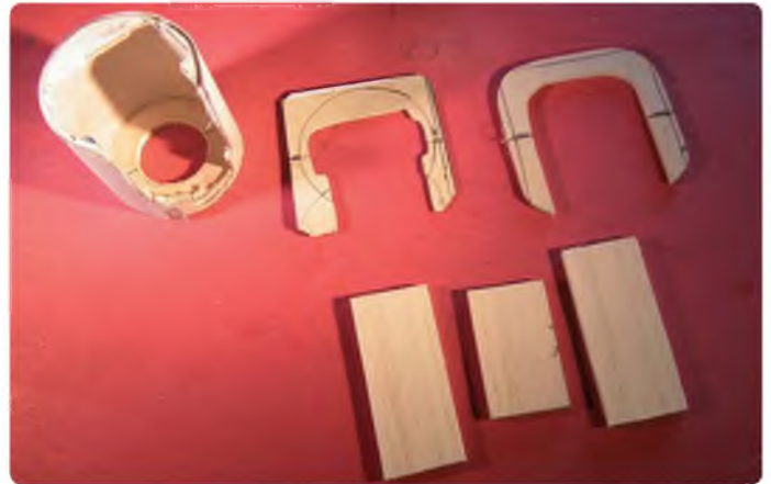
The crankcase and rear mounting box parts
