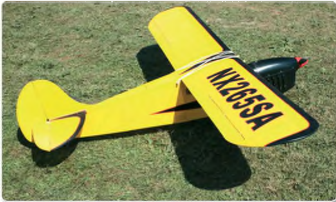
Chad demonstrated an electrified version of Balsa USA's Student Trainer (the glow-powered version having been reviewed earlier this year in RCMW). With a Rimfire 46 and a 4S 5000 pack the trainer flies just as sweetly as a glow ship, only without the noise
