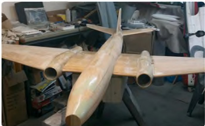
Let us away to the South Seas, to Auckland in New Zealand to be exact, where we see Gerry Glover's build of my E.E. Canberra B(1)8 for twin 90 mm EDF units. Thanks Gerry, we look forward to seeing her finished and flying
