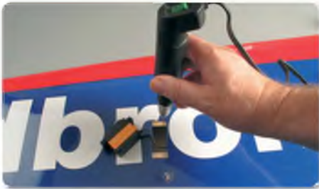
A powered mini-drill makes short work of drilling all the servo screw holes in both wings. You'll need to use a fine drill bit. We used a 1.8 mm drill
