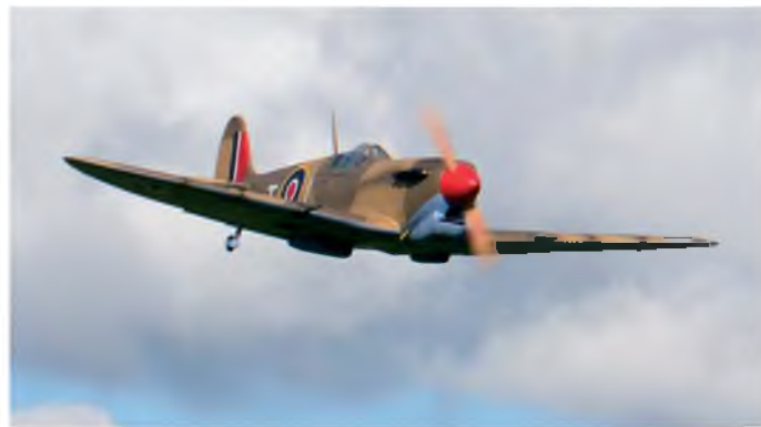
This highly detailed Spitfire Mk.Vb was built by Lee Smalley from a DB Mk.I kit and is powered by an MVVS 40 cc petrol engine
