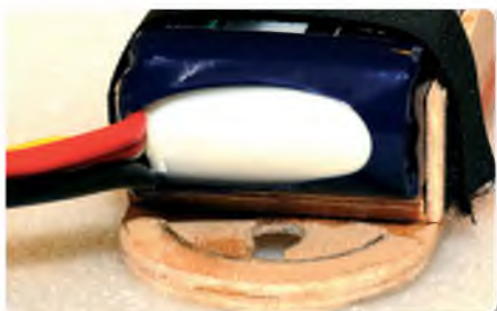
New battery holder needed the front to be raised slightly
