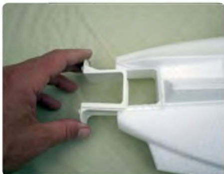
Motor mount being glued into its recess in the fuselage
