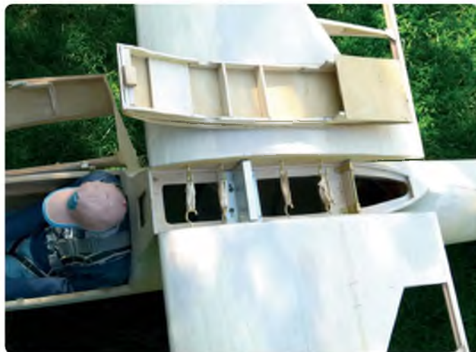
View of wing joining arrangement
