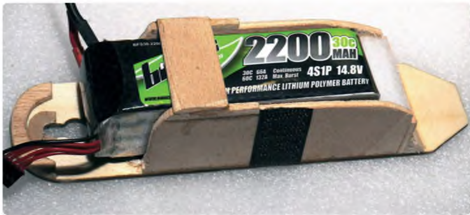
2200 mAh battery in place. Note top brace and fabric fastening
