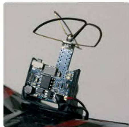
The specially 'stripped down' camera on the FPV Vapor
