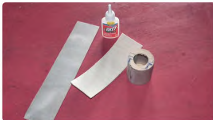
The balsa and second ply layers ready to be glued on
