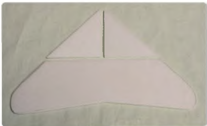
Tail parts are made from 3 mm Depron otherwise they look too thick
