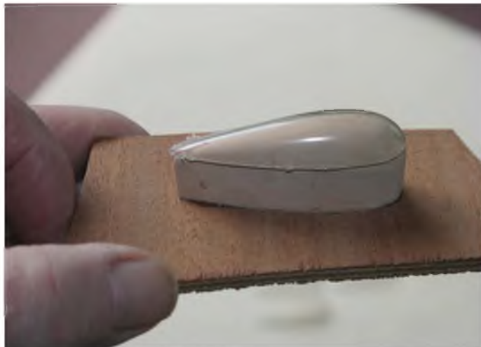
A finished blister sits on top of the male plug
