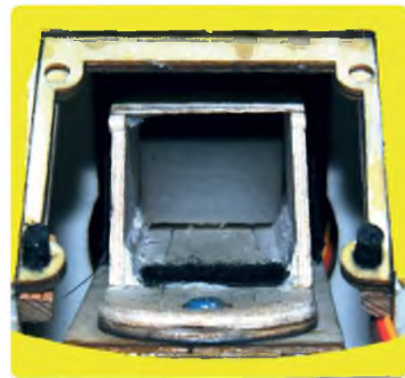
Original battery box in place. Note screw retainer
