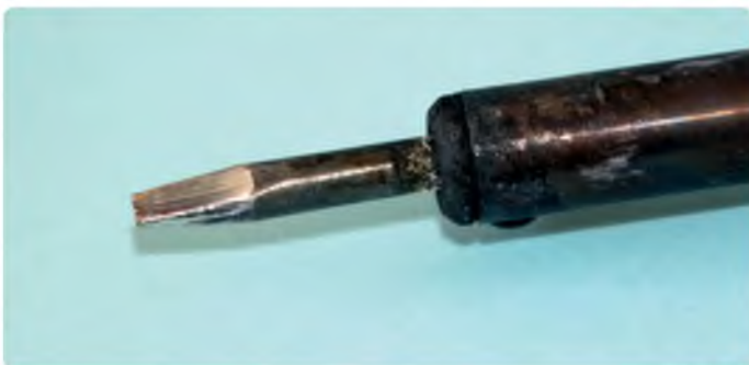
Cleaning the tip of the soldering iron will allow the solder to flow better
