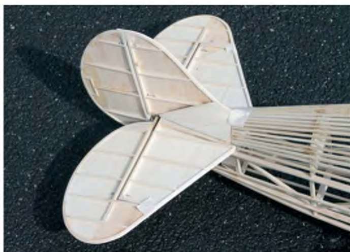
Tail ribs and spars can be replicated by using a sheet balsa core, then adding scale details to one side before turning the component over and repeating the process
