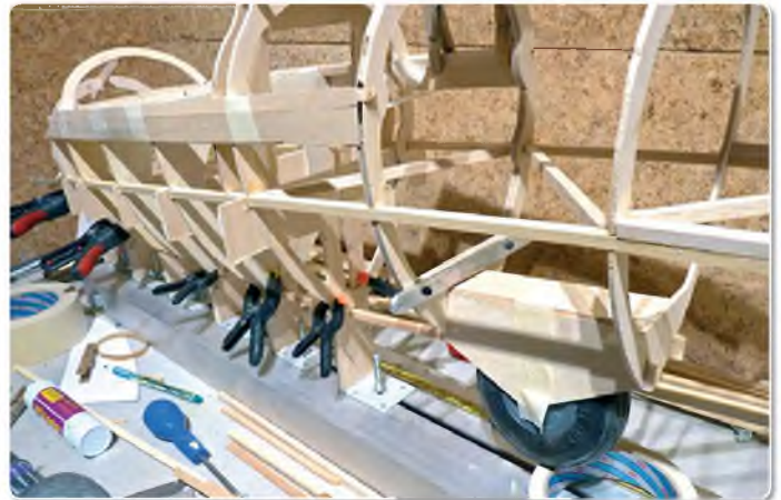
J7 and J8 removed to attach wheel box
