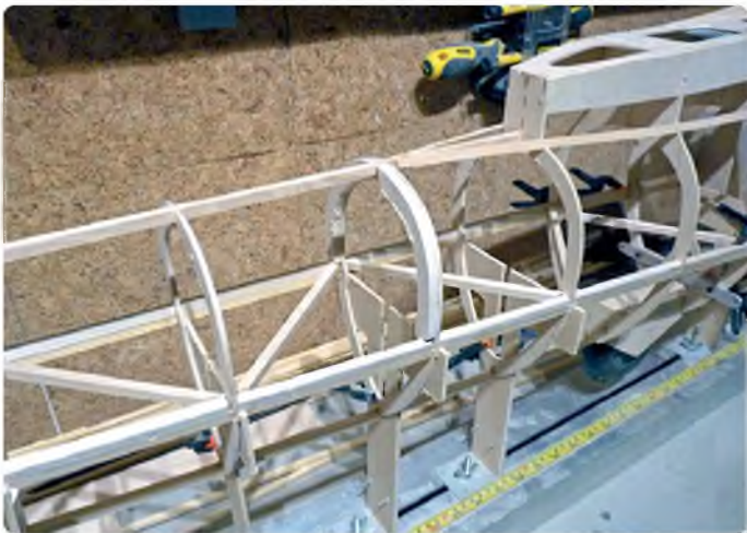
Diagonal cross-bracing shown here
