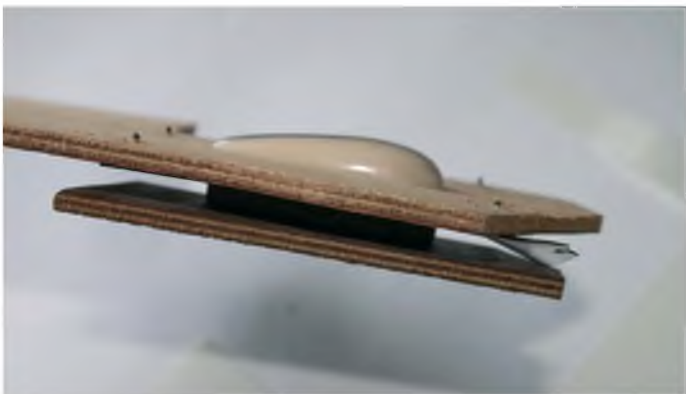
After heating up the clear plastic sheet the plug is pushed through the matching cut-out to form the blister
