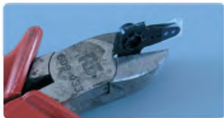
A sharp pair of large side cutters is the best tool for snipping off the unwanted arms. Do watch your eyes as depending on the material used the remnants can ping off at alarming speed. For this reason we would recommend that you always point the underside of the tool away from your face
