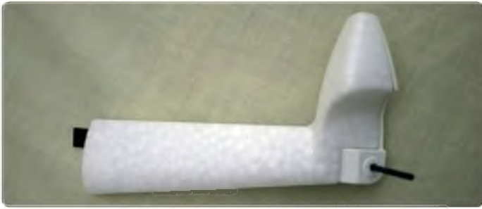
The undercarriage is a mixture of carbon fibre, plastic and foam, which goes together to make a lightweight, sturdy structure
