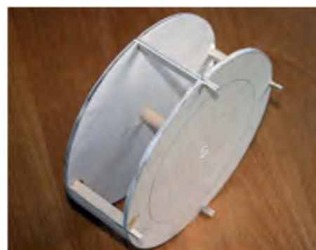
Cowl formers assembled prior to applying the outer skin
