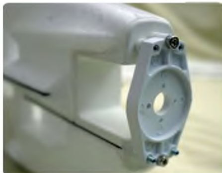
The motor mount is reinforced with carbon fibre rods. The bulkhead bolts on with two cap head screws and has four jacking screws for easy thrust line adjustment
