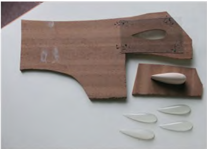
Making the cowl blister patterns from a scrap piece of ply
