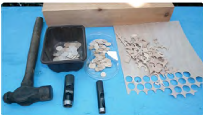
Cutting out all the ply discs is not hard
