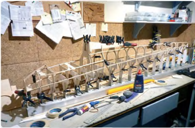
Wing pylon plates fitted
