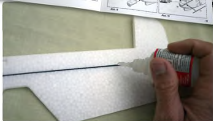
Carbon fibre rods are cyano'd in to moulded slots to provide strength and stiffness. Here the elevator stiffening rod is being glued in
