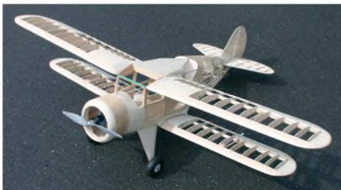
A proper scale model build, ready for covering
