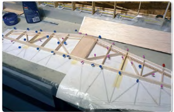
Tailplane being constructed over the plan
