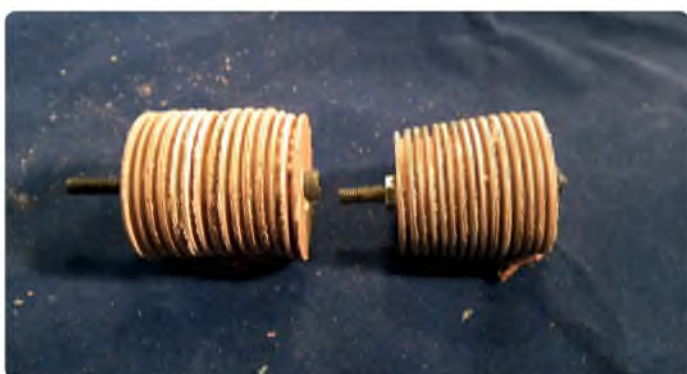
One cylinder in the rough. The other has been sanded, chucked in a power drill
