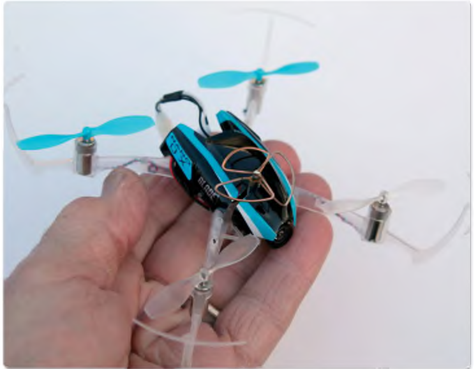
The Nano QX FPV offers a new challenge! The camera lens projects from the 'nose' with an antenna head dress
