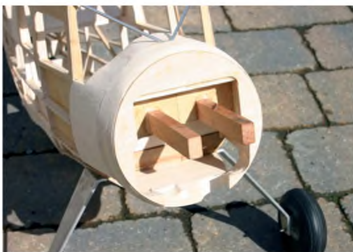
Sturdy wooden engine bearers were fitted to take a Laser 70 four-stroke
