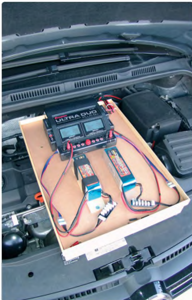
Even big, heavy quick chargers like the Graupner/SJ Ultra Duo Plus will find a solid place on the table board
