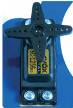
Most modern servos are supplied with splines on their output shafts. This allows for the servo arms to be fitted at a wide range of angles, such as the slight offsets required to provide mechanical aileron differential (as opposed to electronic differential when set up using an R/C transmitter). But each arm engages in a slightly different set of splines, so it is worth checking each arm with the servo switched on and set to neutral. With this four-pronged arm the servo label provides a good reference point to check that the bottom arm is lined up parallel to the servo. You will notice that it is sitting slightly to the right
