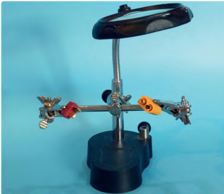
A 'helping hands' unit is well handy for soldering housed connectors. This one even has LED lights!
