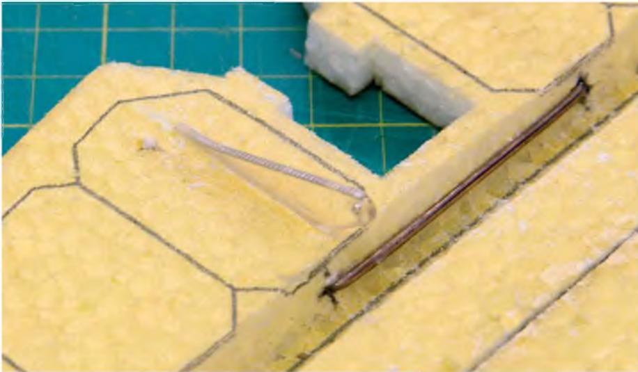
Elevator joiner and laser cut transparent control horn. The horns simply cyano in to slots cut in the EPP foam
