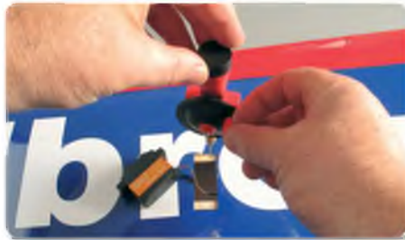
On thinner wings than those fitted to the Laser it's easy for a powered mini-drill to get dragged through the hole and to hit and even penetrate the opposite wing skin. To prevent this from happening you may want to use a hand drill. A miniature version is ideal for chucking up the small diameter bit. But beware of cheap tools – the gears on this little thing slipped as soon as the drill started to bite!
