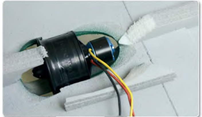
The fan unit is fitted
