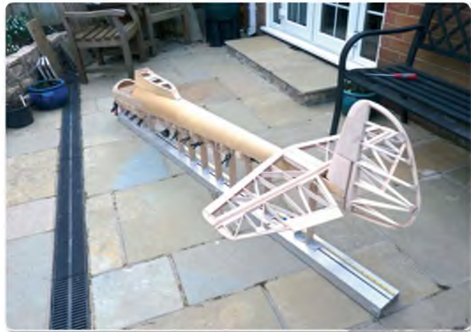
Tailplane set up whilst still in the jig. Note the fin is unglued at this stage until the setting up of the wings
