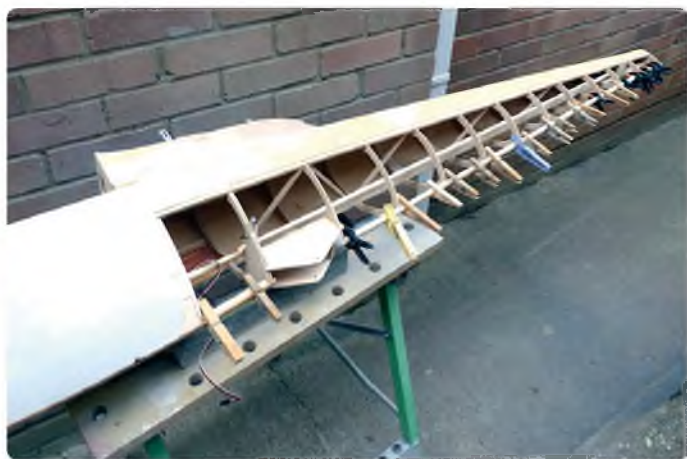
Filling in each side of lower longeron to increase gluing area
