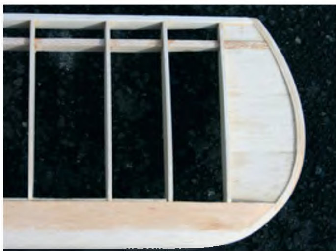
Wingtip showing laminations
