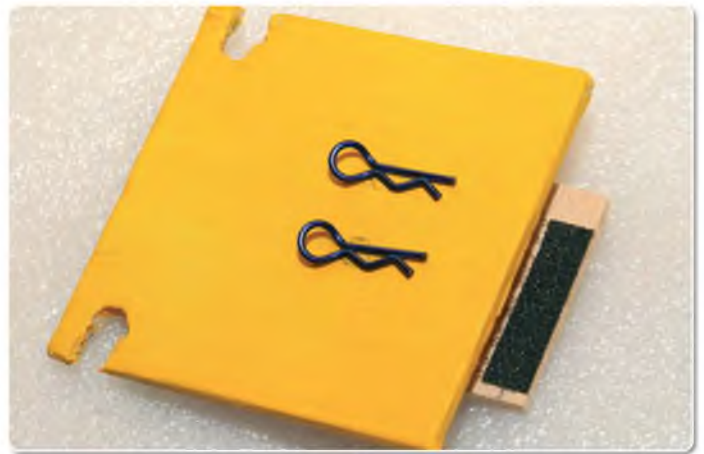
R pins securely held by magnets. It's easy to lose them otherwise
