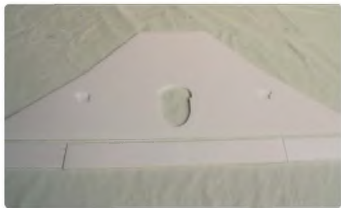
Wing parts are also cut from 6 mm Depron
