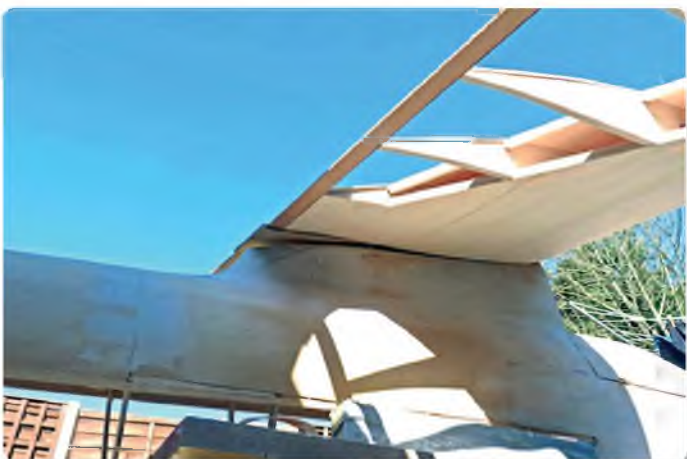
Underside view of wing fairing
