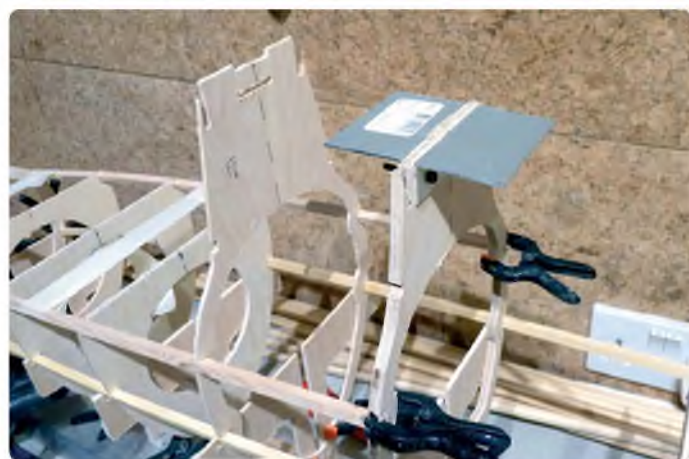
Wing joiner box attachment plates bolted to F7
