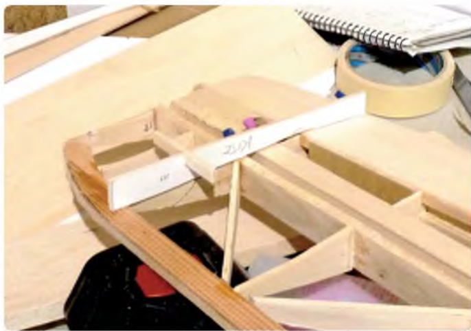
Using the template to set aileron TE
