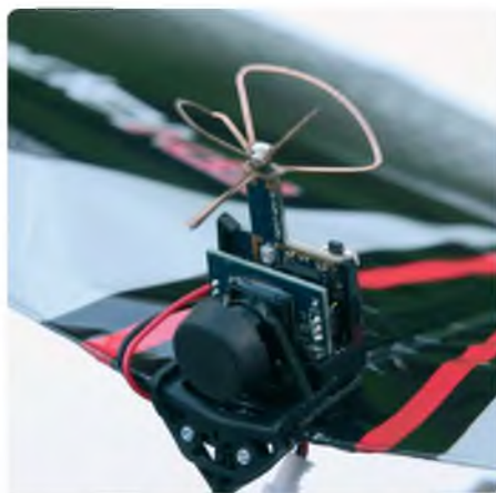
The camera is firmly fitted into a clip mount on the wing leading edge
