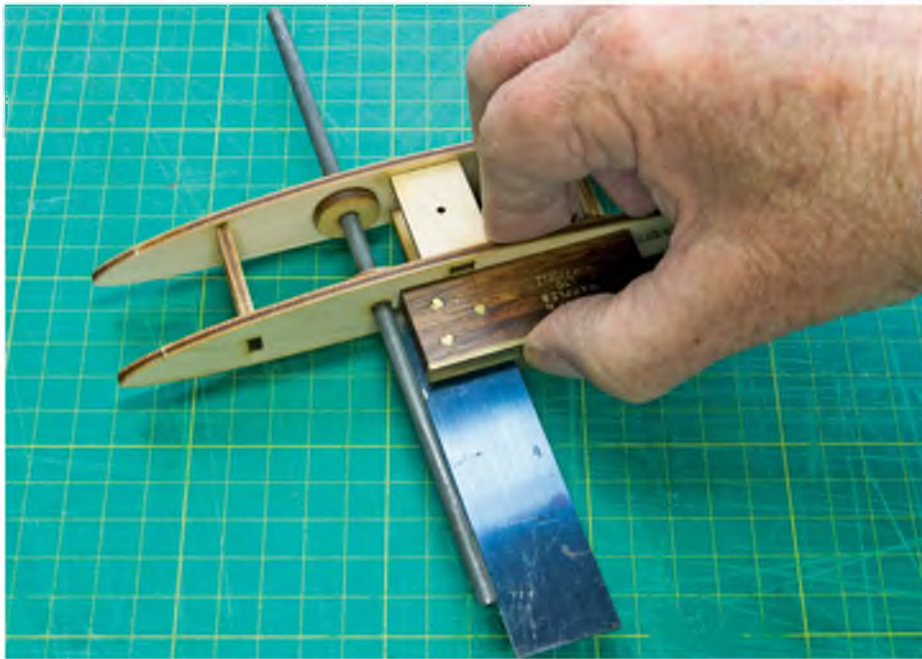
Checking that the carbon wing rod is all square
