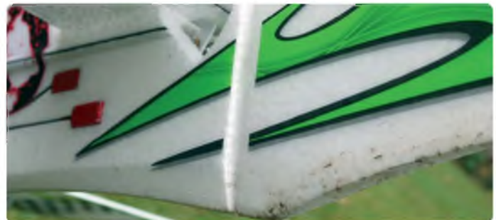
The same area after a few flights. The underside of the rudder rubs along the ground and can get scuffed. Some additional protection would be worthwhile
