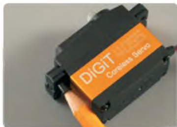
Alternatively use a sharp pencil to guide the spacer into position
