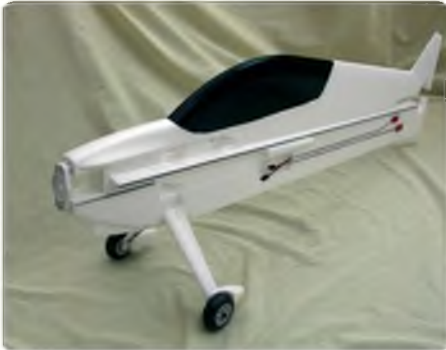
The fuselage ready for fitting the wings, horizontal stabiliser and rudder
