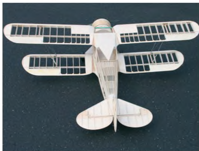
Rear view of the completed model showing the balsa core tailplane, upper deck stringers and the curvaceous wings
