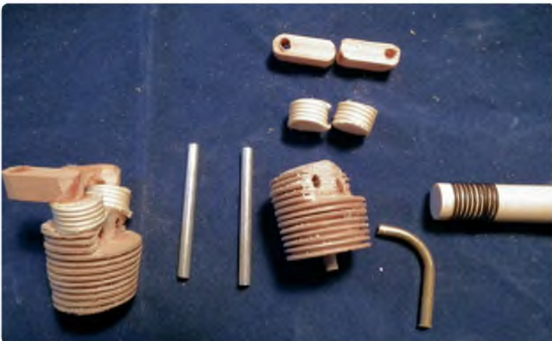
The kit of parts for the cylinders, and showing the rocker boxes
