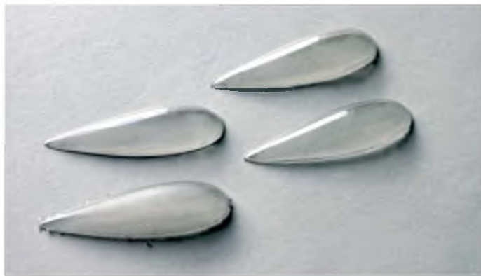
A set of finished cowl blisters
