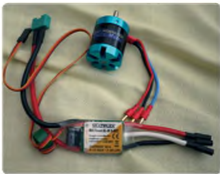
Left: Multiplex tuning motor set includes a Himax 2816 1220KV motor and 30 amp ESC
