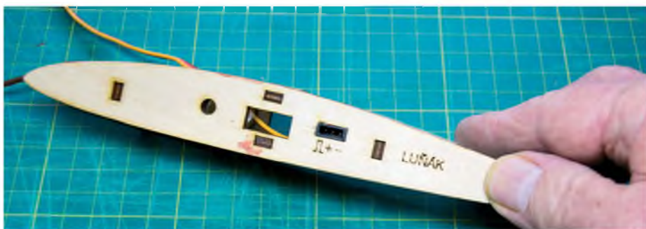
Side view showing the signal and polarity annotations below the servo plug holder
