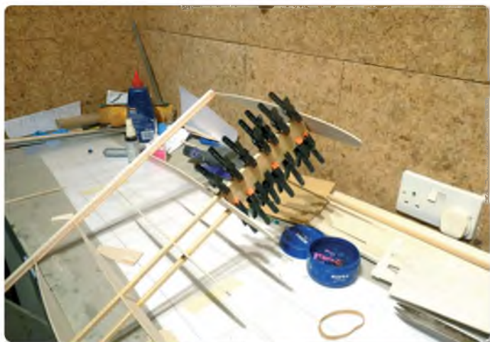
Gluing in the wing joiner box
