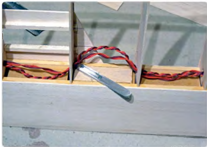
View of spar attachment bracket in the wing
