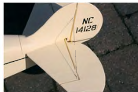
Tail feathers are reinforced using piano wire struts with flattened brass tube ends
