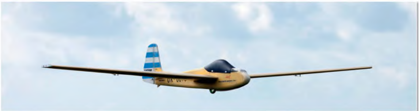
Whilst the extra chunk of lead taped to the nose didn't help the Lunak's appearance it did improve the aerobatic performance
