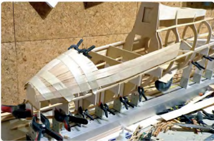
Top part of front planking completed
