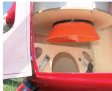
Inlet cone on the lower face of the drum feeds air to the double-sided Notar fan
