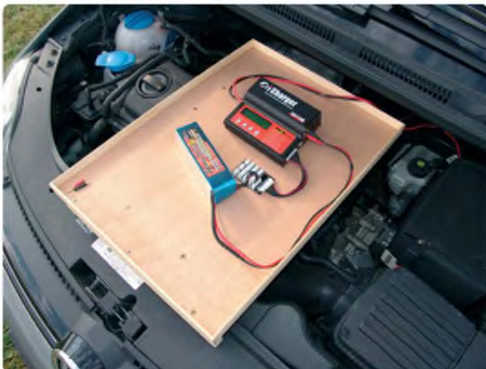
The little helper is perfect for instant quick charging, as it can be put in place in seconds. Surrounding borders prevent accessories from falling into the engine compartment
