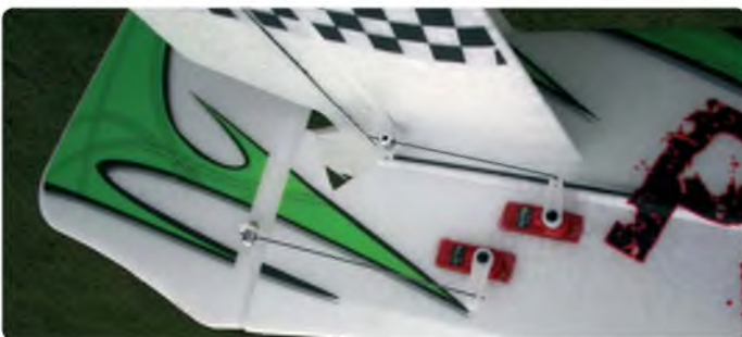
Elevator and rudder servos are situated underneath the horizontal stabiliser and are connected with short, direct control runs
