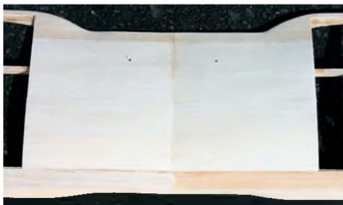
Curvy lower centre section ready for covering
