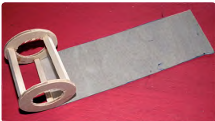
Starting to roll on the first layer of 1/64" ply
