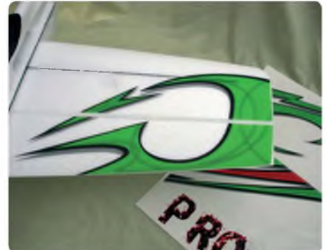
The decals are easy to apply and are designed to accommodate the gaps for control surface movement
