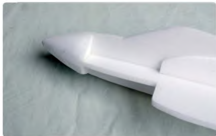
Nose block after cutting and sanding to shape
