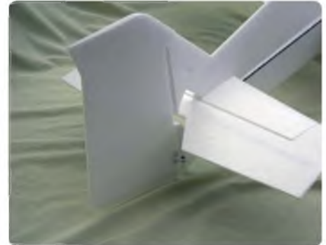
The horizontal stabiliser is slotted into place before the rudder is fitted
