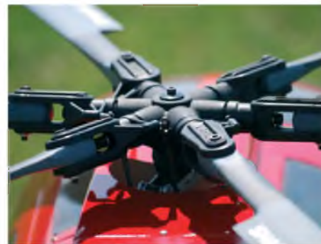
Really impressive counter clockwise rotating Vario 6-blade rotor head, equipped with Vario Shark Skin rotor blades
