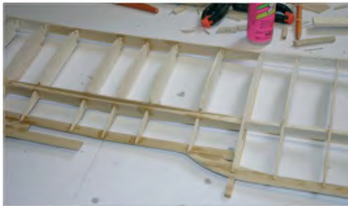
Lower wing centre section under construction
