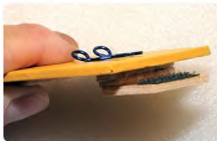
The tongue on the new hatch cover slots into the fuselage
