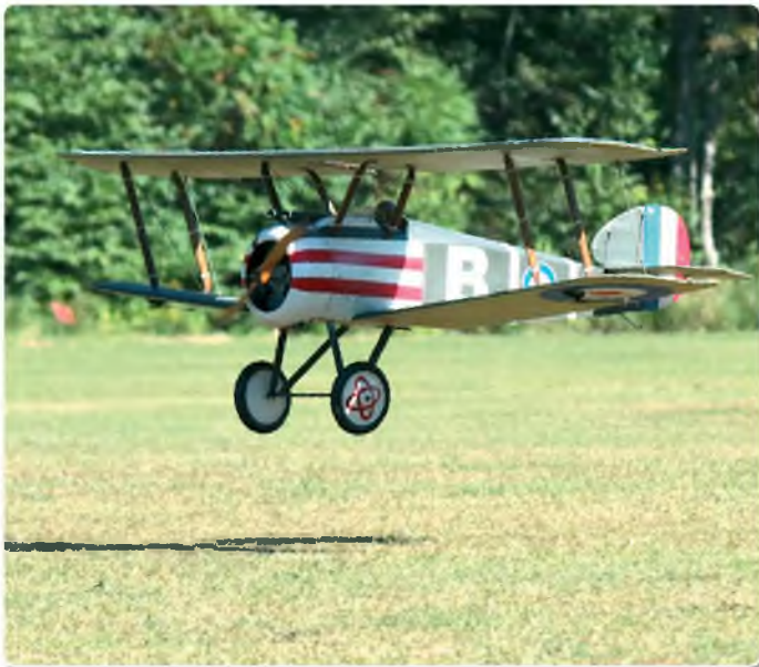
Chad says it's easy to do a wheeled landing with the model but that the model can easily get away from the pilot if a three-pointer is attempted
