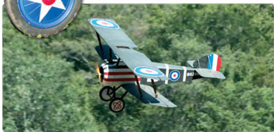
Like the SPAD, the Camel is covered with Solartex and painted with latex paints
