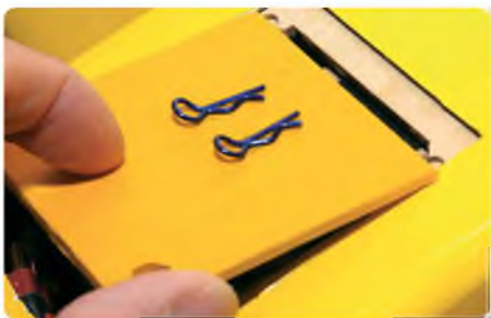
Modified hatch cover being slid into place. Magnets let into the wood stores the R clips when changing batteries
