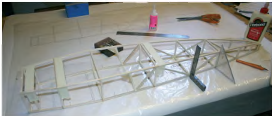
Fuselage framework under construction
