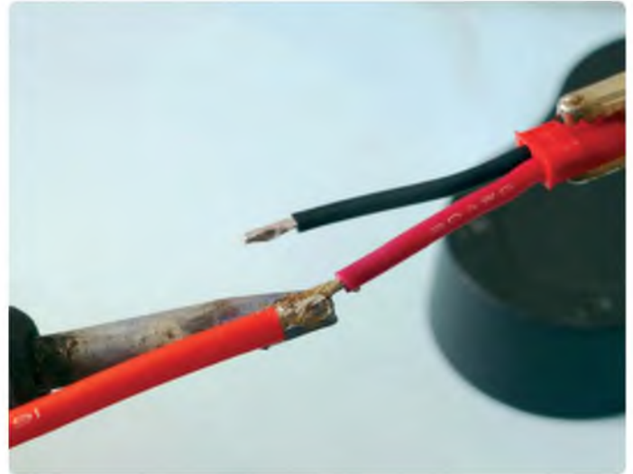
Tinning the wires of a JST connector prior to joining the wires
