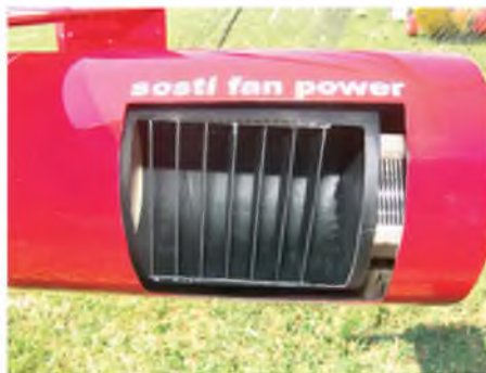
The slotted one-piece end cap is rotated by a servo, controlling the air stream from the internal fan. The yaw servo sits inside the tip
