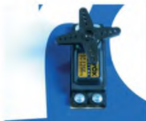
And with the third arm the offset is even more pronounced
