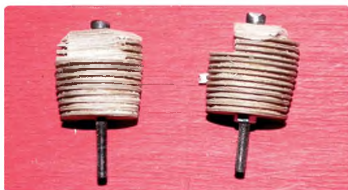
The locations for the intake and exhaust tubes, and the plugs has been cut away
