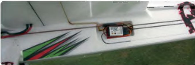
The receiver fits in a recess just underneath the wing. Note the slots provided for the servo cables and also to route an aerial. A Multiplex RX5 receiver fitted easily but the recess should accommodate most compact receivers without requiring any modifications
