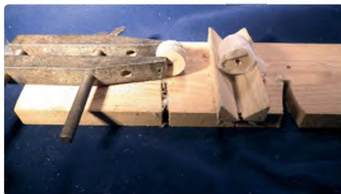
A small V block helps line the discs up for drilling. The clamps hold them firmly
