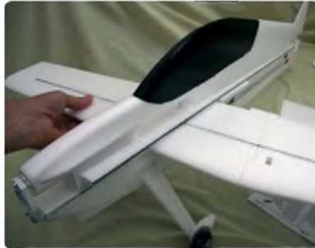
The wing is fed through the fuselage before the second aileron is fitted. Marks in the foam mouldings make alignment easy
