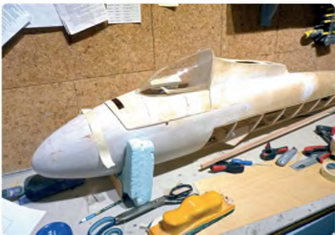
Fitting the canopy
