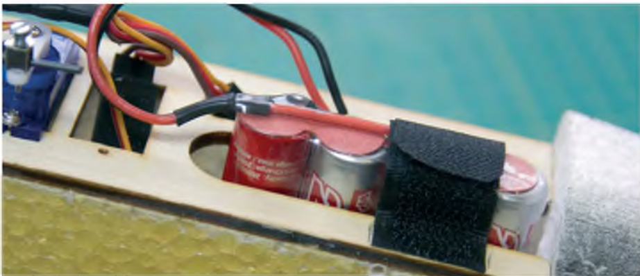
The forward slot in the ply radio tray is just the right size for a four cell pack of AA NiMH batteries
