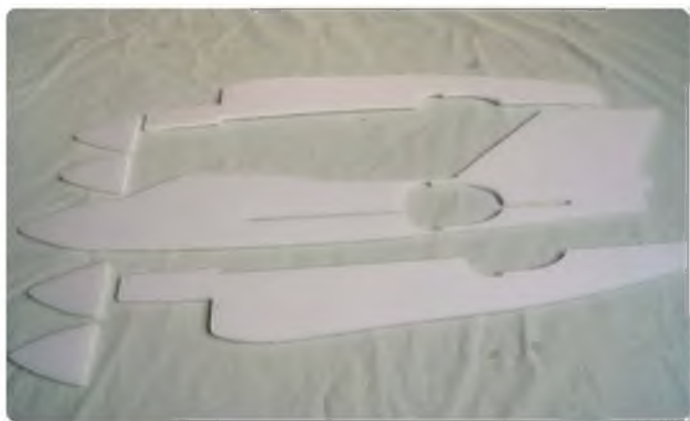
Fuselage parts cut from 6 mm Depron
