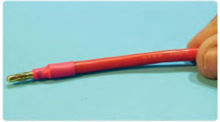
Fitting large diameter wire (in this case 8 AWG) to gold connectors can be tricky. This is where a larger solder bucket can be of benefit!
