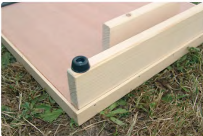
Two rubber pads prevent the car's front end from being scratched and give a proper alignment
