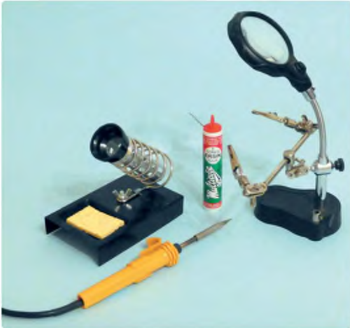
Basic soldering equipment consisting of a soldering iron, a stand with sponge cleaning pad, solder and a 'helping hands' unit
