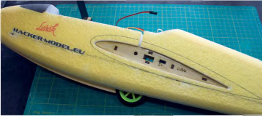
The completed wing box is pushed into position in the aerofoil shaped cut-out in the foam fuselage. Note the faint cut line under the wing and Hacker sticker, inlaid with carbon reinforcement rods
