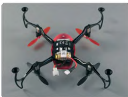
The LiPo sits in a cage underneath the main body
