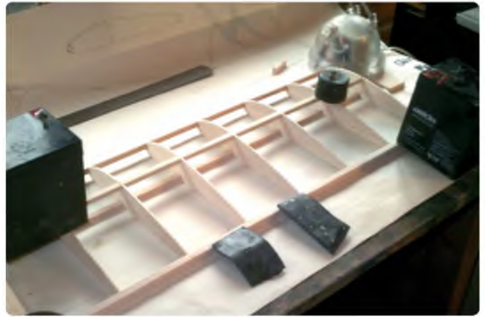
Weights are used during wing construction to hold everything straight
