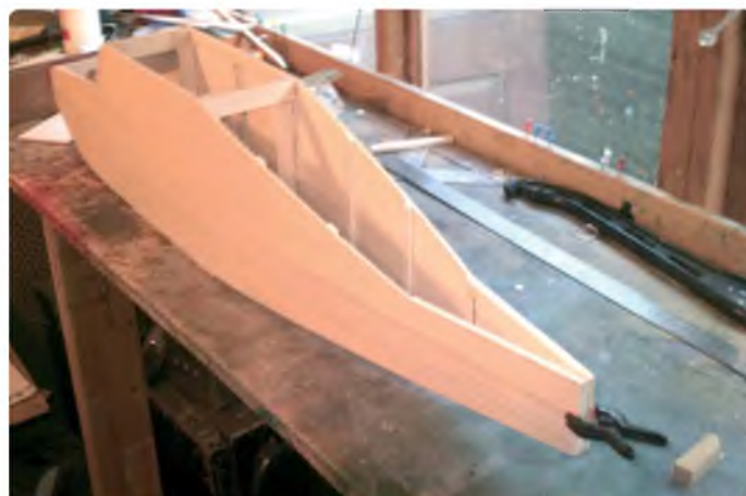
Bring the tail end together and hold with a suitable clip
