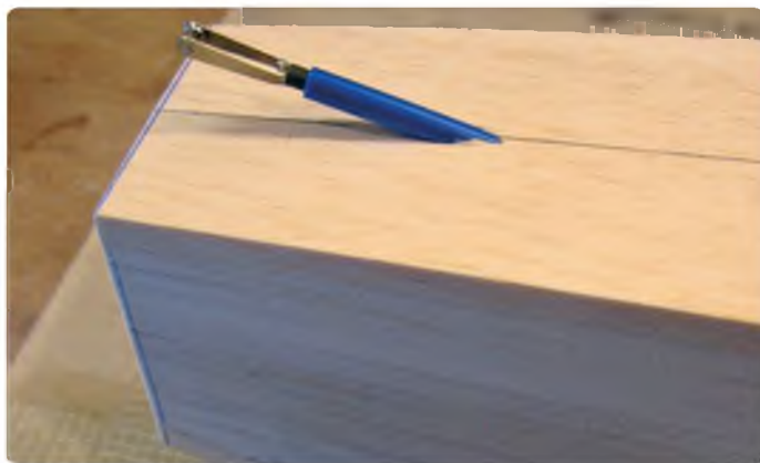
Snake exit through top skin rear of fin post. Ensure a good fit here and glue the snake outer securely!
