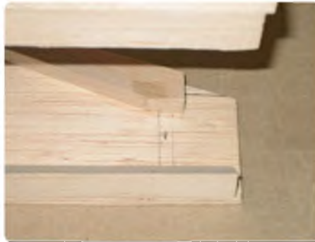
Forward fuselage 1/4" doubler cut back to sit on top of F1 when fuselage sides are pulled in at the nose
