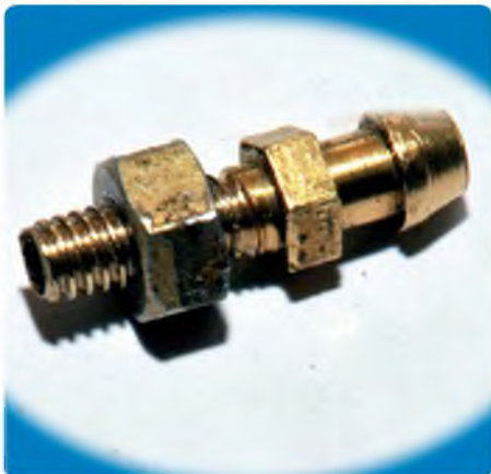
Replacement filler nipple from the spares box with re-cut thread and lock nut
