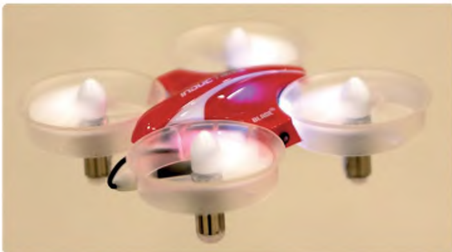
The coreless motors are used as the landing gear
