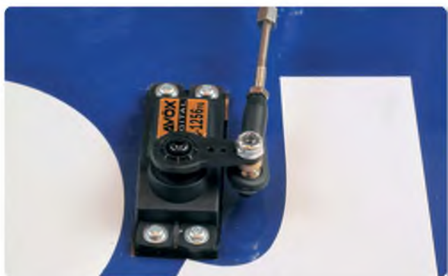
Here's that problem posing photo once again. Look closely and you can see that the ball link that is fitted to the servo arm is very close to the servo case. There's a very good chance that at full throw the pushrod could foul against the side of the servo
