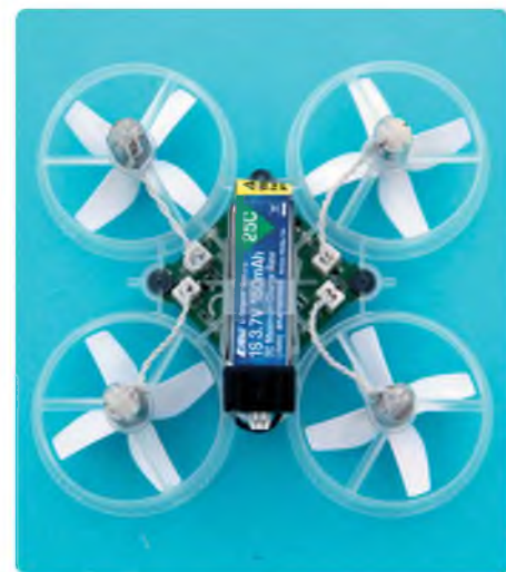
A standard 150/200 1S LiPo is used in the Inductrix
