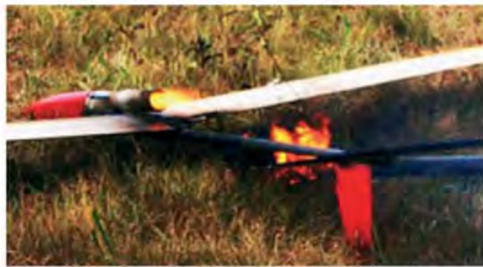
And if you get unlucky? This motor suffered a 'cato' – a catastrophic failure, and went POP!
