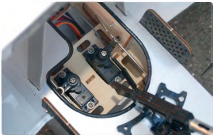
The micro servos (not supplied) are connected using EZ-Link connectors
