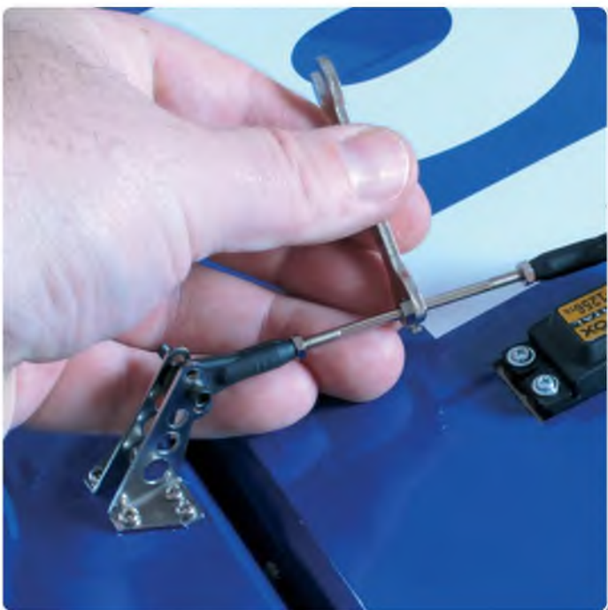
We just love the turnbuckle style pushrods supplied with the Aeroworks Laser 200 kit. By simply turning the central hex shaped section using the spanner supplied the control surfaces can be finely tuned without having to pop off any of the ball links or un-clip clevises. A neat idea that is very popular with R/C car enthusiasts (to quickly alter toe-in/out settings), we are amazed that it hasn't been used more often for R/C model aircraft pushrods
