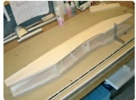
Second fuselage side is added to form a basic box structure. Take care to check alignment over the plan
