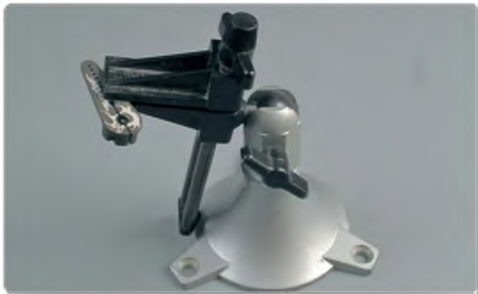
The holes in the servo arms need opening up to fit the ball link retaining screws. You'll need to find a sturdy support to hold each arm whilst drilling them out. This handy ball-headed clamp proved to be ideal and it also has soft(ish) nylon jaws, so preventing damage to the anodised surface of the metal servo arms
