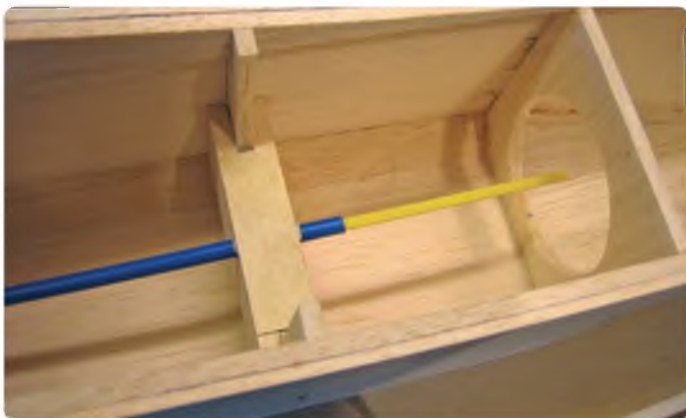
Snake supports fitted either side of F5 to suit required height of chosen servo
