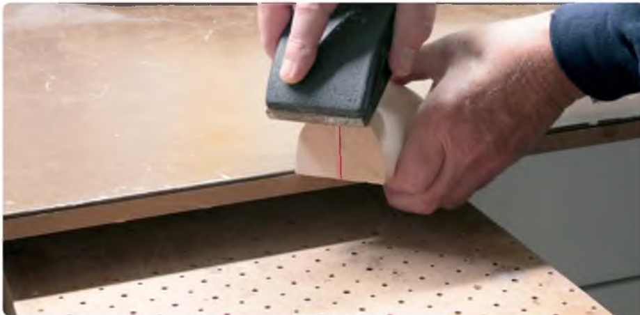
Simple sandbox at work, sucking up balsa dust
