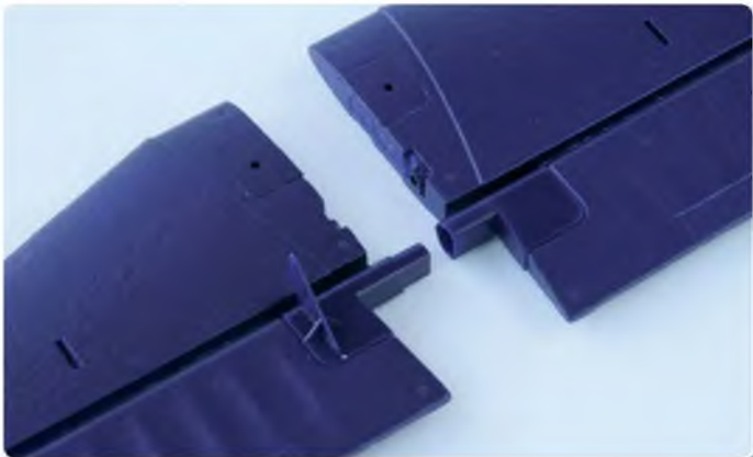
Close up detail of the push together elevator joiner
