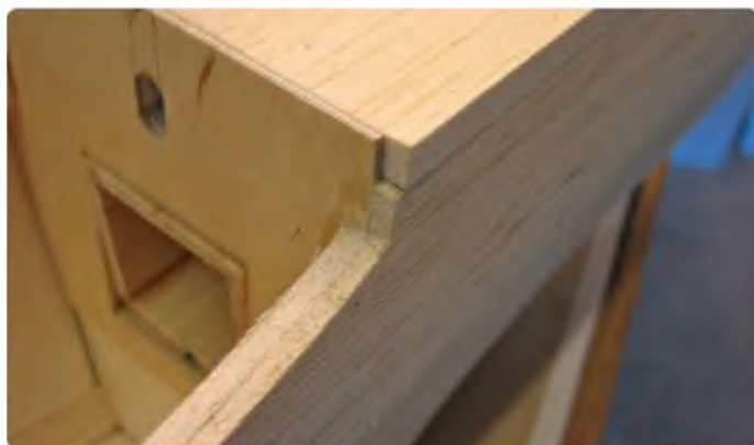
View at F3 wing L/E. The doublers and fuselage sides need to be relieved at an angle to allow the wing to seat fully
