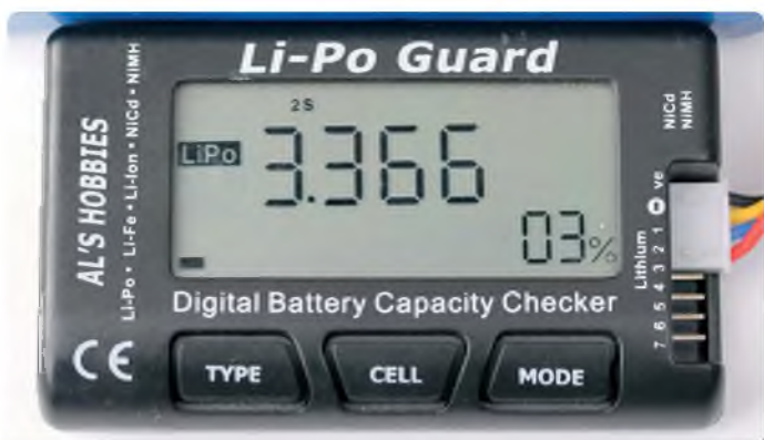
Cell 2 is a bit over but should be reading 4.2 V
