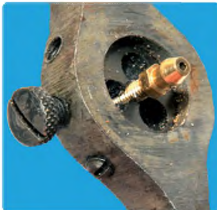
The die used to cut the new thread. Experts will note the missing grub screw. It was lost years ago
