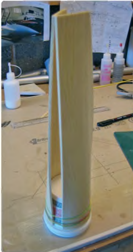
Wrap intake skins around a tub of diameter similar to A1, then leave to dry out in this condition as this will aid assembly on the model
