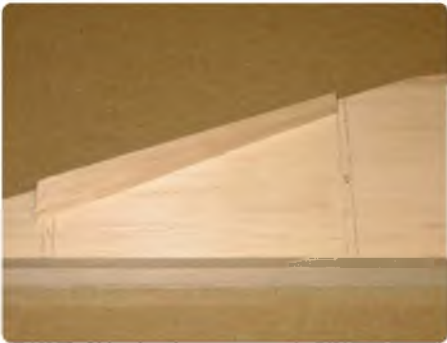
Forward fuselage side showing position of F1 and F2. The 1/4" doubler requires trimming to clear F1 as assembled
