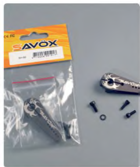
The simple answer is to fit a longer servo arm. Most servo manufacturers can provide a 'super servo arm' to fit their premium servos. Here's a couple of examples of Savox's high quality metal arms, with and without packaging. Besides the central servo output screw and anti-vibration lock washer (internal tooth type), each SH-82 arm comes with two additional socket head bolts. These are inserted each side side of the central split collar and when tightened they provide additional security and help the servo deal with the additional side loads that can result from using the longer arms
