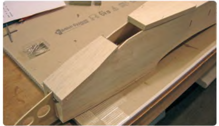
Balsa sheeting added behind the canopy to F4. The false cockpit floor from 1/8" balsa should also be added at this stage
