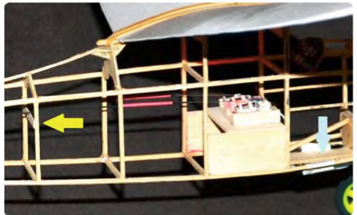
The receiver 'brick' on its balsa tray. I added a small piece of balsa to support the pushrods and prevent flexing (yellow arrow). The friction is negligible. Notice also the battery tray at the front (light blue arrow)
