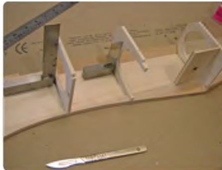
Formers F4 and F5 are glued square onto the fuselage side
