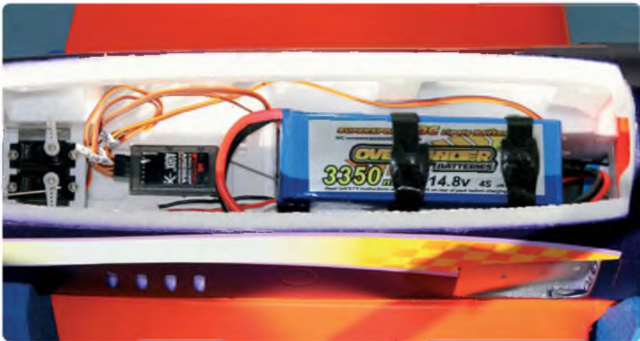
Spacious avionics bay showing the factory fitted AR636A Spektrum receiver and 16 g servos. Plenty of space for the recommended 4S LiPo
