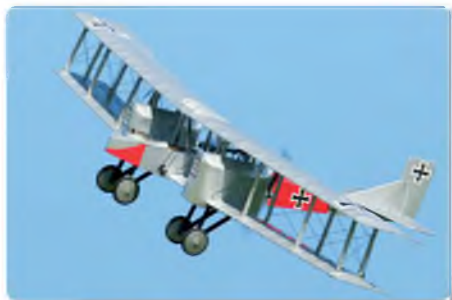
No, the props haven't dropped off! They are spinning around behind the wing, pusher style
