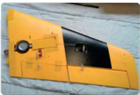
Wing panel straight from the box with flap and ailerons linked up and electric retracts in position
