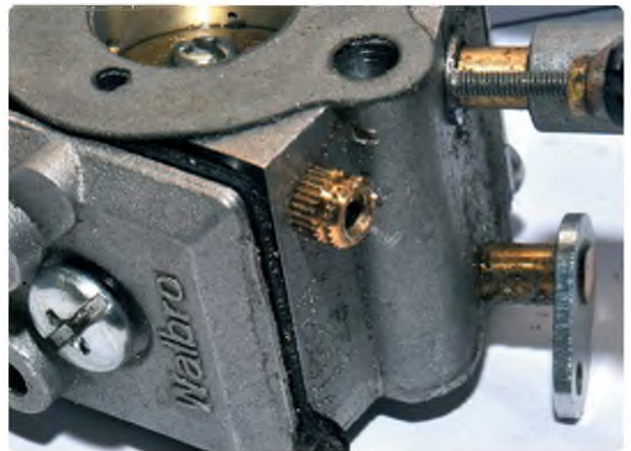
The plastic filler is moulded over and retained by the teeth of this brass insert
