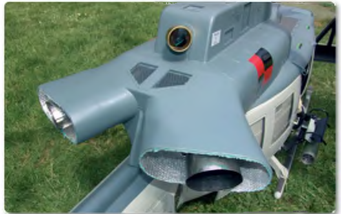
Here we see details of the stainless steel double exhaust outlets. A JetCat SPH5 turbine powers the custom modified Vario Sky Crane mechanics
