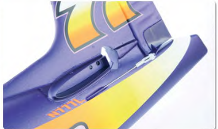
The tailplane halves push into cuffs moulded into the rear fuselage
