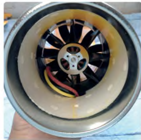
Rear view of the 1450 KV motor and 11 blade fan unit
