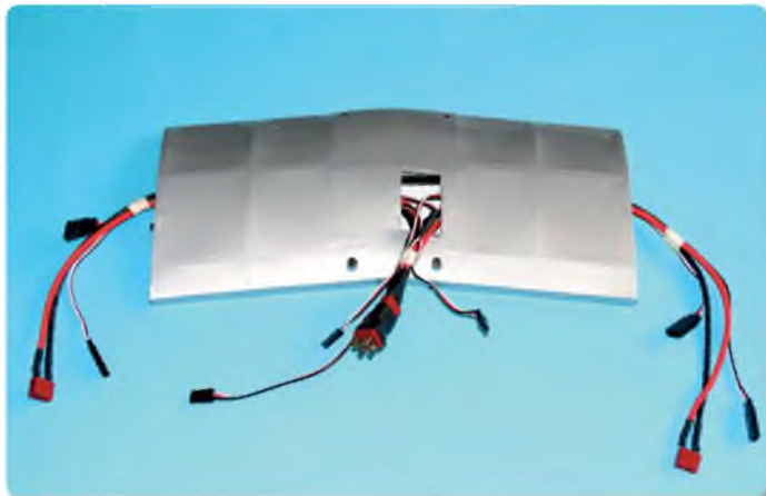
Centre section is fitted with a wiring harness
