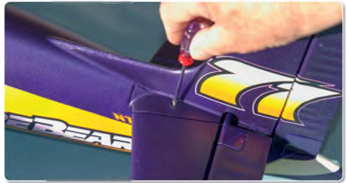
BNF planes often use clear tape to secure the tailplane, which works well, but the high performance of Rare Bear dictates the use of screw fixings
