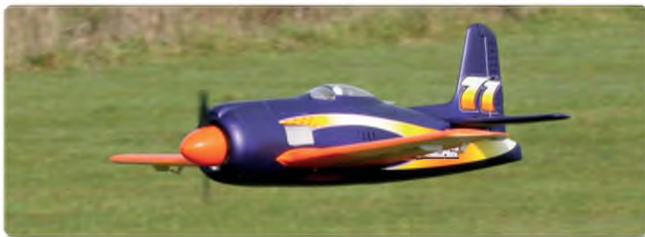
That large cowl produces a bit of drag so keep the power on during the approach and chop it just before touchdown
