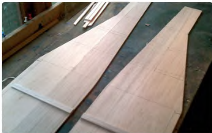
Make a pair of opposite fuselage sides by joining two lengths of balsa sheet
