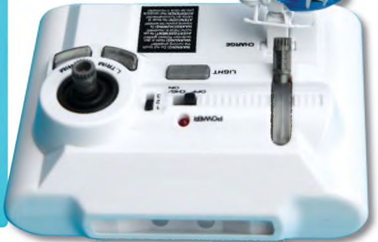
Nano Falcon XS sits on the Tx mounted jack plug for charging
