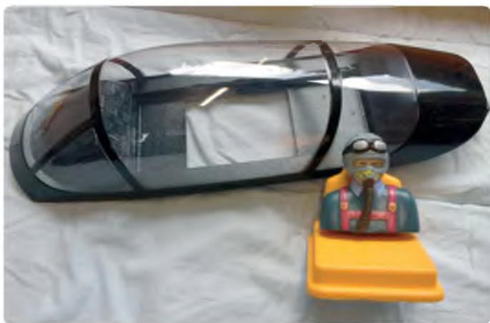
A neat canopy with instrument panel and the nicely painted pilot, which needs to be glued in securely
