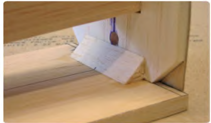
Triangular support between F3 and fuselage floor. Note 1/16" ply overlap
