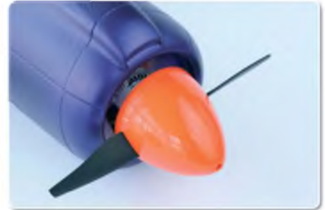
The stubby 8" x 8" prop is covered by a nearly 3-inch diameter spinner
