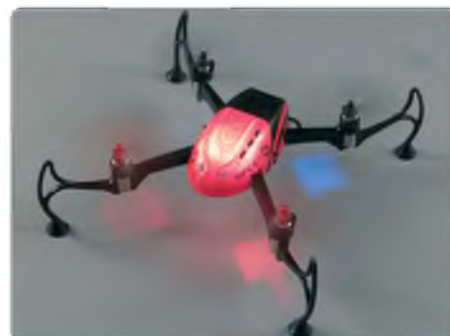
Spinning up for take-off, this shot shows the different coloured LED lights and coloured front props, both of which aid orientation
