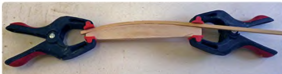
Forming a bend in a fuselage longeron
