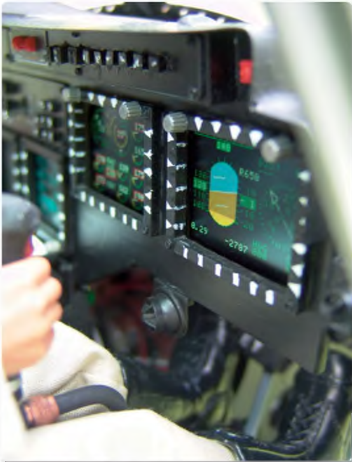
The cockpit features six coloured LCD displays showing static pictures and video sequences, just like with the real one
