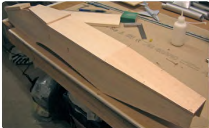
Rear top 1/4" balsa sheeting added to fuselage
