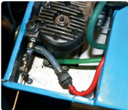
The engine is fitted to a Paxolin board, which is then screwed to the bearers
