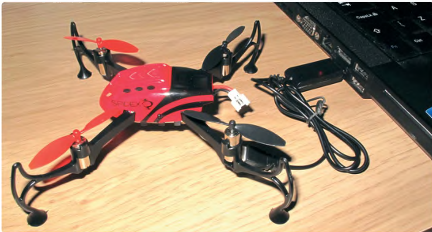
Plug the USB charger into a spare computer port and the Spidex can be recharged while you carry on working
