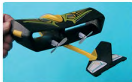
Twin motors are mounted on the lower wing
