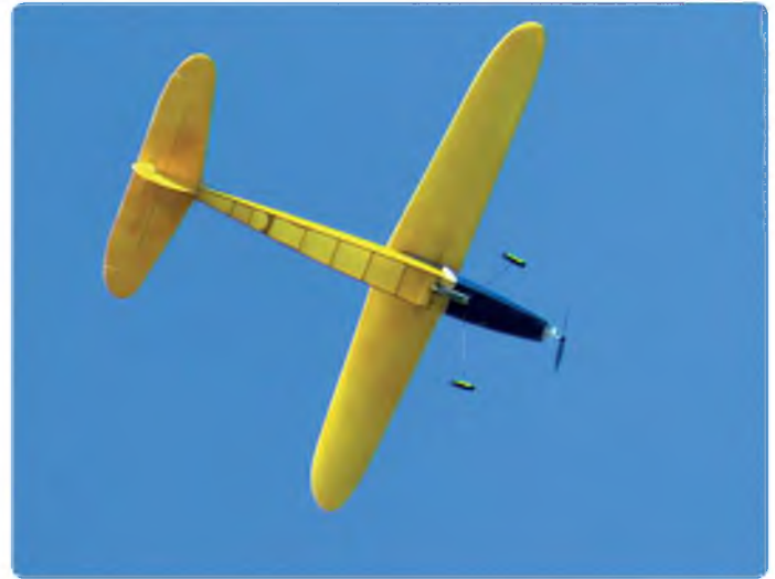
Underside view showing the 1S LiPo taped on just aft of the undercarriage
