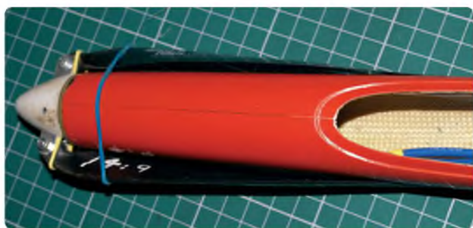
In a conventional model these days the motor is enclosed within the nose area and is nigh on invisible. But somehow Andy's motor managed to come apart, 'reverse' up the fuselage to the canopy area, then allow the rotor to fly out without any other damage being done!
