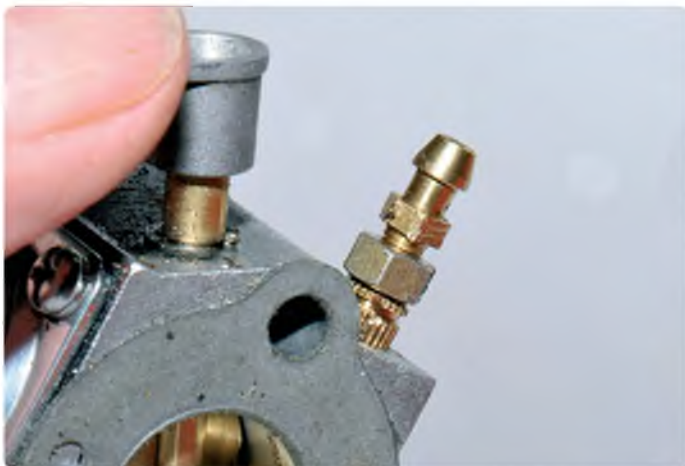
In place with the lock nut, looking very neat and in the second picture with the petrol fuel pipe attached. In the model it will probably be routed a slightly different way
