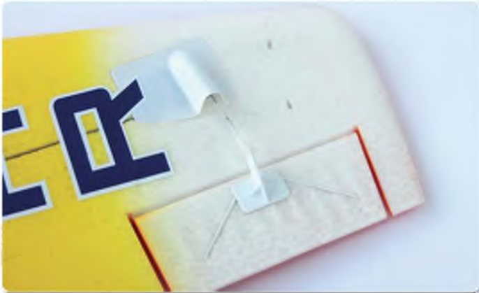
Short span ailerons are operated using 16 g metal geared micro servos
