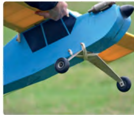
The undercarriage is 'banded on' to prevent damage in case of a heavy landing
