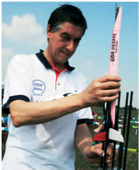
Nige Bathe (GBR) sets up his 'Toblerone Special'. This S4A-Boost Glider's wing swivels 90 degrees and is then 'rolled up' around the fuselage and becomes a 'rocket'. At the top of the boost it all unrolls and becomes a glider again
