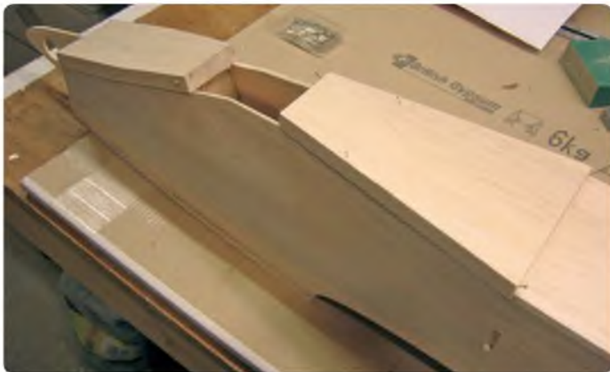
Recess for air-intake former in fuselage side, with three each side for each semi-former A1 to A3
