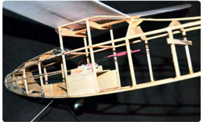
The Rx tray is simplicity itself, made out of a few pieces of scrap balsa. The letters on the cog-wheels are there to remind me of the function of each servo, D standing for Direction (or rudder)
