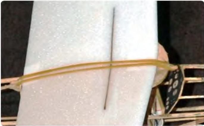
Wings are reinforced in the middle by a small dihedral shaped piece of thin plywood. All flying surfaces are fixed with rubber bands, as per the original
