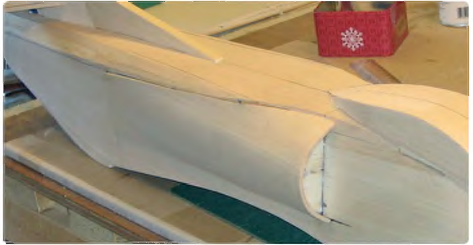
Intake skins glued to fuselage sides. Overhang over A1 will be dressed back later
