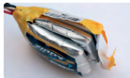
This 3S 500 mAh LiPo was found like this in the flight box
