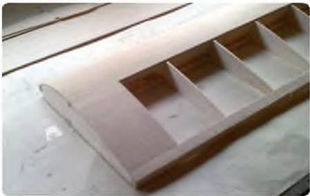
The wing is sheeted with 1/16" balsa top and bottom
