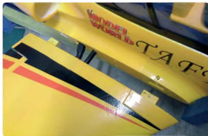
Wing panels are located using sturdy tabs. A carbon rod provides the main support
