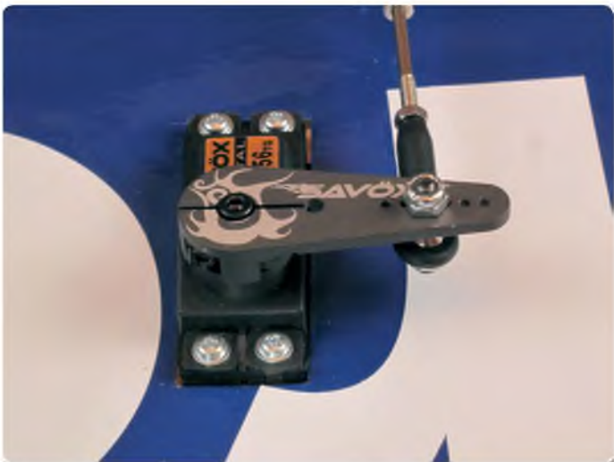
A few blips of sub trim and the servo arm was taken back to its neutral position. In this shot you can also see that the pushrod is angled very slightly. The hole was carefully chosen to allow for this...
