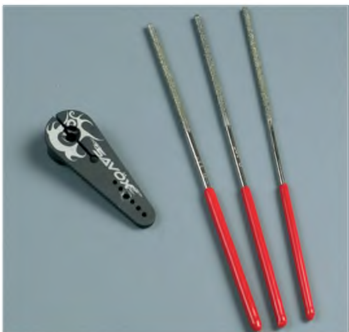
Other brands of needle files are available! We have just received review samples of some sanding tools from the USA and inside the package we found a set of diamond coated round micro files. These high quality tools are of finely incremental sizes so they can be used just like the drills we used to originally open up the hole, starting with the one that only just fits and progressively using larger sizes until the ball link screw only just drops through
