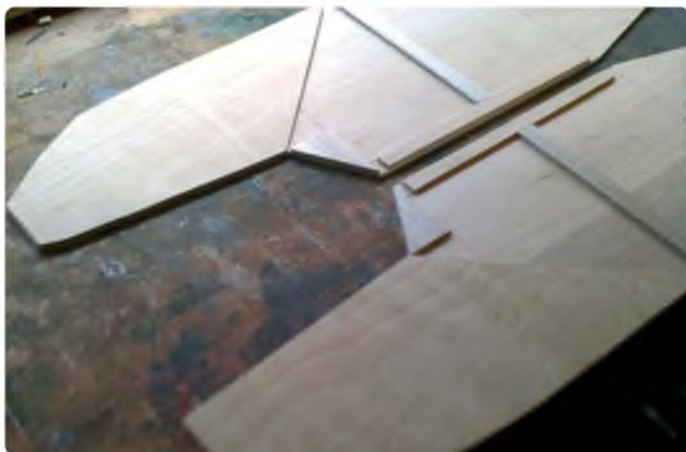
1/16" plywood doublers are added to the front sections
