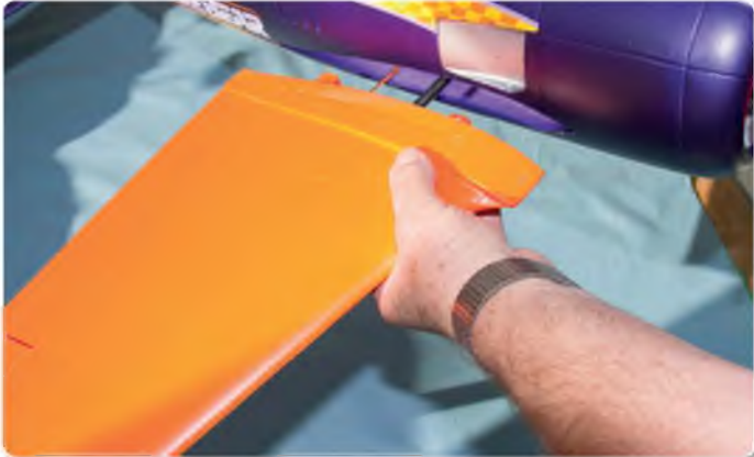
Sliding the wing panels over the carbon joiner rod
