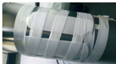
A pair of wings (in this case 3 mm Depron ones for an indoor Tiger Moth) already wrapped up and ready for hot water moulding
