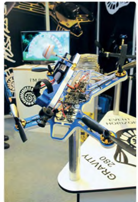
Fossil Stuff are UK manufacturers of FPV racing quads, such as the Gravity 280 pictured here that features durable HDPE (High Density Polyethylene) frames for improved crash resistance
