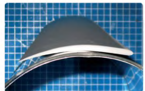
A ready to use moulded 6 mm Depron wing panel
