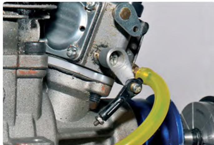
In place with the lock nut, looking very neat and in the second picture with the petrol fuel pipe attached. In the model it will probably be routed a slightly different way
