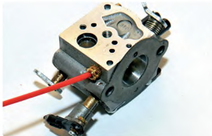
It is essential to remove all swarf from any of the jets. I blew through the newly made hole and then flushed it with WD40
