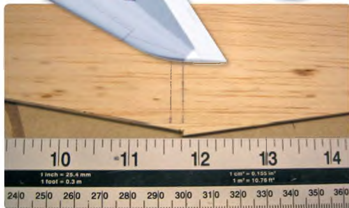
Fuselage sides are formed from three pieces of 1/8" balsa to achieve full depth. This picture shows the small piece fitted at the wing T/E position, just above the ruler
