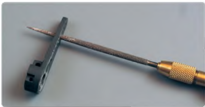
Final reaming out can be done with a round needle file, whilst constantly checking to see if the mounting screw will fit snugly into the modified hole. We found that the needle nosed version from Perma-Grit was ideal for the job
