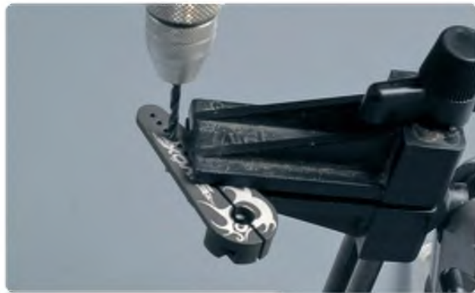
With the arm held securely we used a Dremel miniature power tool to open up the mounting hole for the ball link screw. To help prevent elongating the hole it is worth starting with a drill bit that is only just a bit larger in diameter than the existing hole, then working your way up in small steps with increasingly large diameter bits until you get to the correct size. It's far better to stop when the hole is still a fraction under-size than just ploughing on and finding that your new hole is way too big and that the ball link bolt is a sloppy fit in the hole. Remember, as this is a North American kit the bolts supplied are of an Imperial size, so the metric drills that UK modellers most frequently use will only provide an approximate reaming out of the hole
