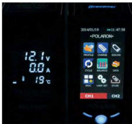
Lights out so we can show you the display panels. The figures on the left monitor the PSU output, whilst on the right is the main menu for the charger
