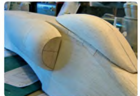
Intake fronts are temporarily glued to the fuselage for final shaping and gap filling, then removed for covering. The prototype flew with a solid balsa canopy prior to a vac-form version being released by Traplet
