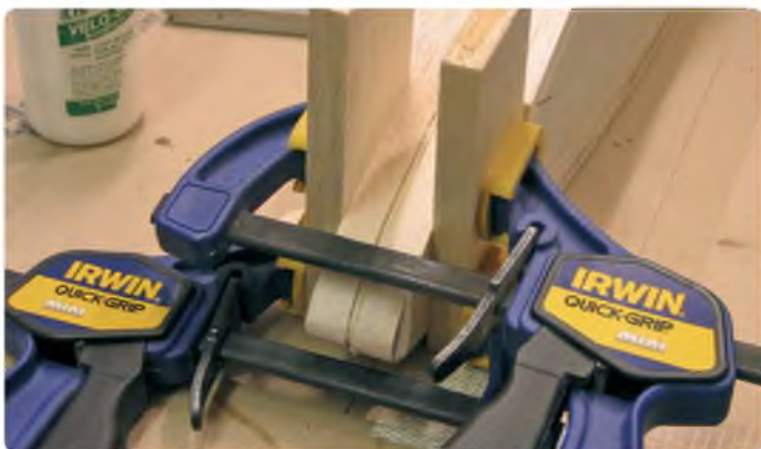
Laminating the nose section with soft 1/2" balsa
