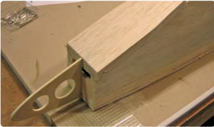
Fuselage sides cut back flush to F1 and front top fuselage 1/2" soft balsa sheeting added
