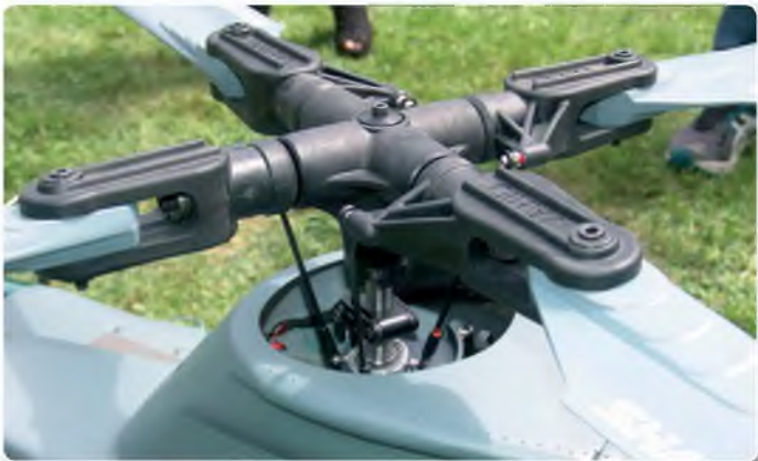
The counter clockwise rotating Vario rotor head is equipped with Vario Shark Skin rotor blades
