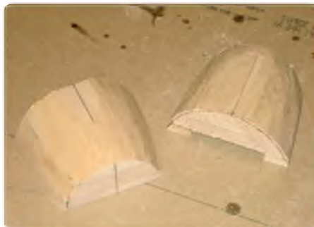
Intake fronts made from balsa laminate, rough planed to shape
