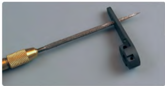
Be sure to ream out the hole from both sides. If you just do it from the one side then the top of the hole will be slightly wider than the bottom (nearest the tip of the file) and this could lead to slop in the final linkage. Elf and safety note (well, we are writing this over Christmas!); be sure to use a handle when using needle files (a.k.a. rat tail files) otherwise the tang can easily dig into the palm of your hand
