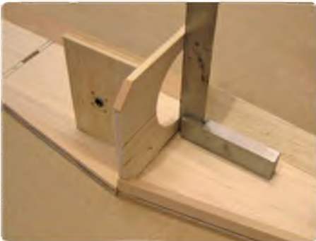
Composite wing bolt former F6 from 1/8" ply and balsa laminate glued square into slot in fuselage doubler. The captive nut 'pulls' against the ply face on the top side of F6. F7 is glued square onto the fuselage side
