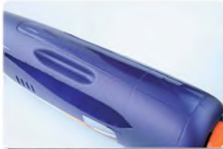
A long underbelly skid plate protects the fuselage during landing
