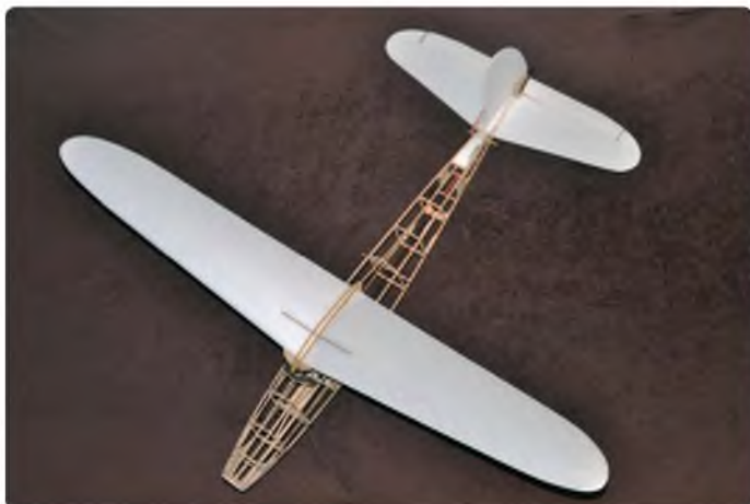
A 'bare bones' photo showing the new Depron flying surfaces mated to the 30+ year old balsa airframe
