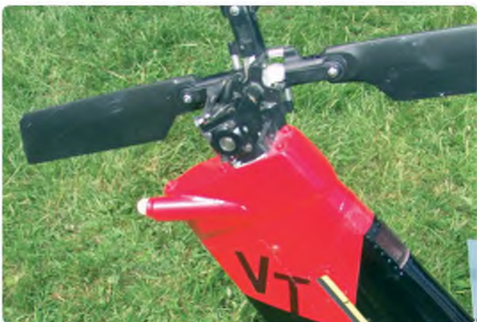
Unfortunately the Vario tail gearbox isn't quite right...
