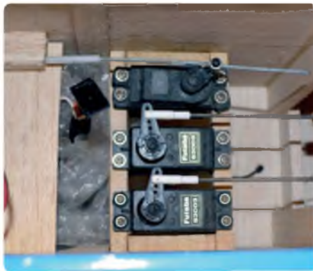
Radio compartment follows the standard layout
