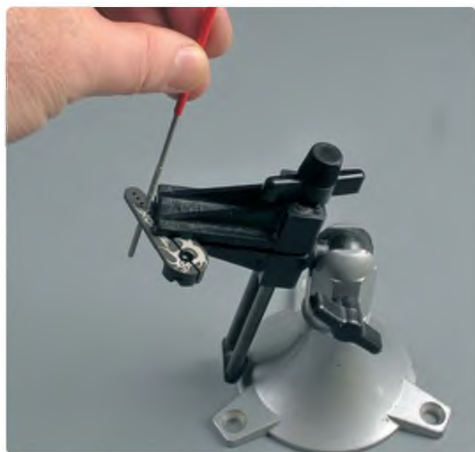
Other brands of needle files are available! We have just received review samples of some sanding tools from the USA and inside the package we found a set of diamond coated round micro files. These high quality tools are of finely incremental sizes so they can be used just like the drills we used to originally open up the hole, starting with the one that only just fits and progressively using larger sizes until the ball link screw only just drops through
