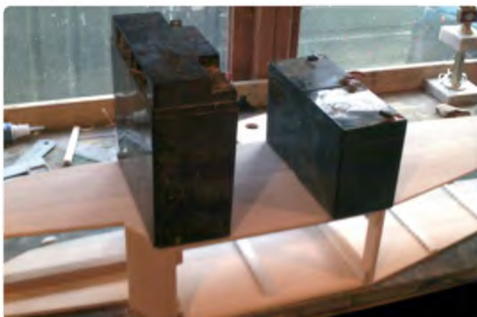
Heavy weights are used to hold the fuselage sides in place whilst joining them together
