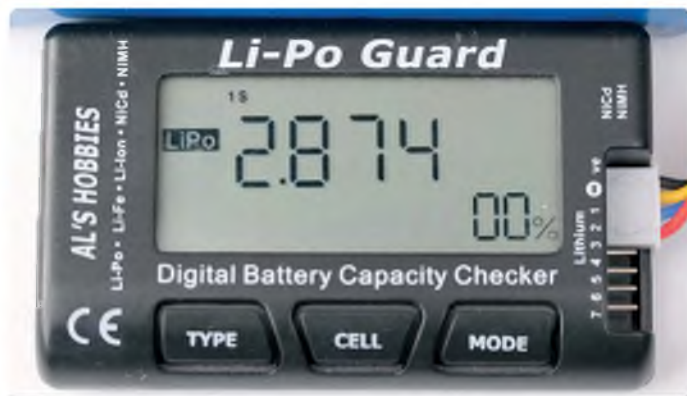
Cell 1 is below the 3 V threshold
