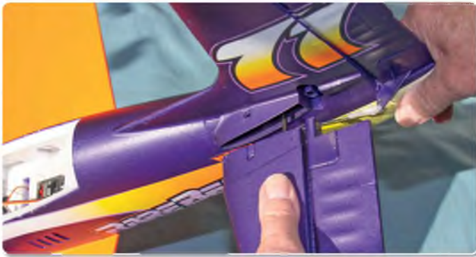
Sliding the tailplane halves into place
