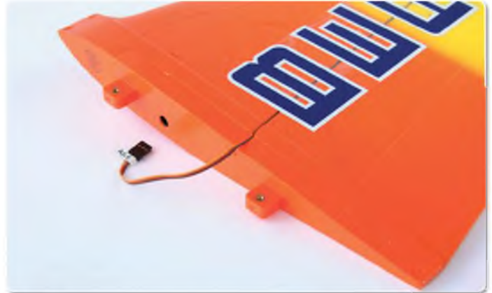
Plastic root cuffs have sturdy wing mounting tabs
