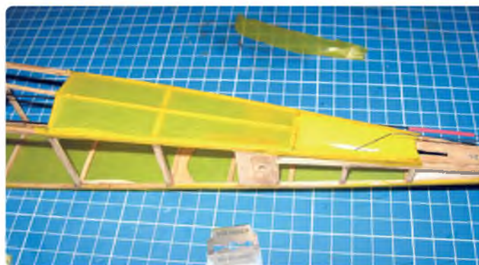
A new blade (in this case, a time-honoured razor blade!) is highly recommended for trimming the iron-on tissue. Or you can use a new No. 11 blade. The top of the fuselage has a concave 'double curvature' so I opted to cover it in small sections to prevent wrinkles
