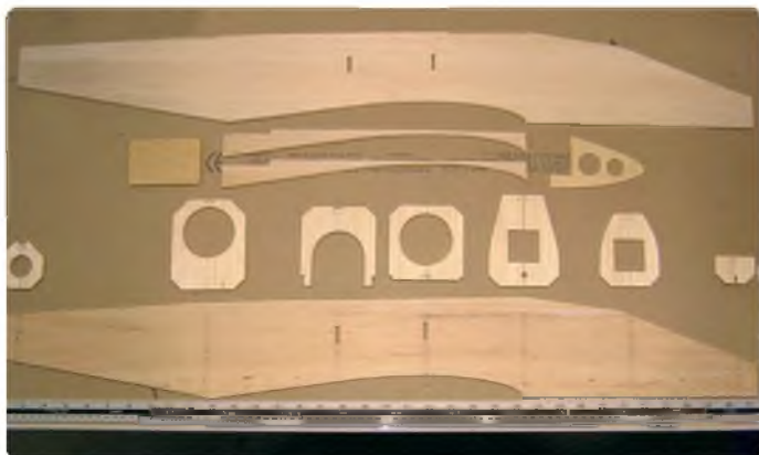
Basic fuselage component layout: F1 to F8, wing bay doublers, litemply nose profile
