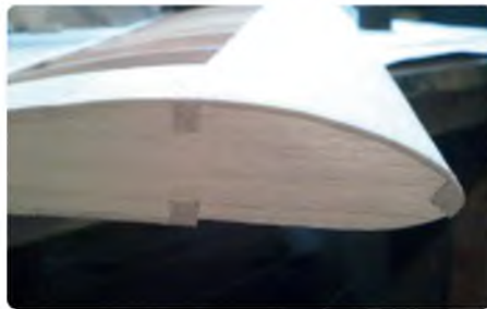
The wing is sheeted with 1/16" balsa top and bottom
