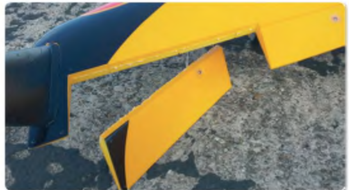
And the live foam hinges on the ailerons separated. Quickly fixed all round using pin hinges
