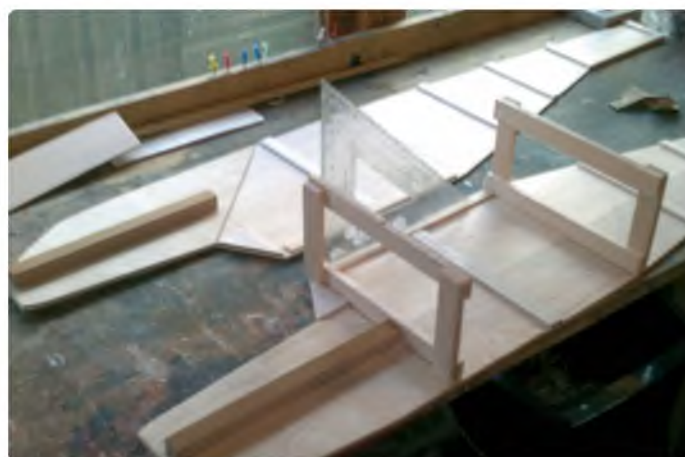
Make up and fit formers F3 and F4 from 1/2" x 3/16" balsa strip
