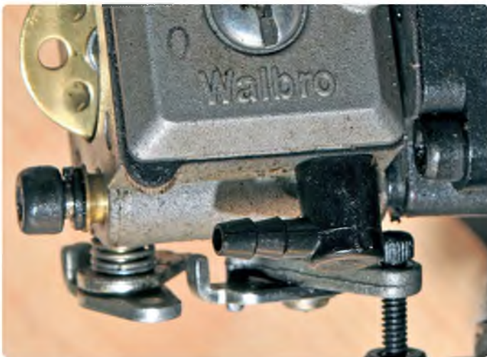
The normal plastic filler on a standard Walbro carburettor
