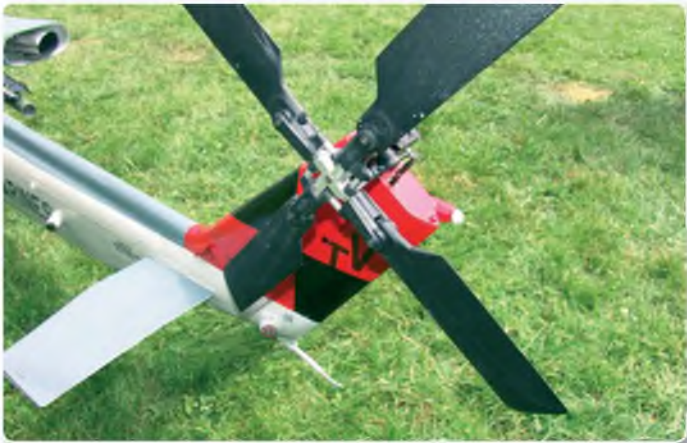
A Vario tail rotor gearbox and four-blade tail rotor are used. You will notice that one of the tail blades is attached the wrong way round. Even top modellers get stressed when preparing for this competition!
