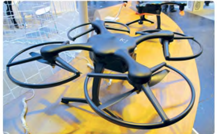
A noticeable feature of the Ghost is the very sturdy guard rings around each rotor for added flight safety
