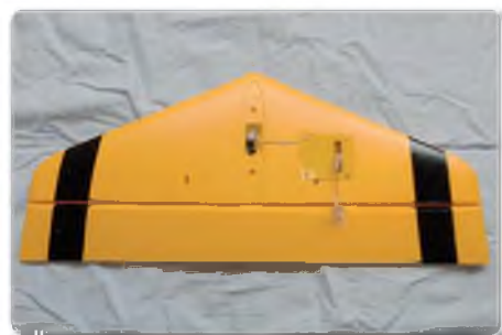
And again on the tailplane. Note the use of ball links at each end of the pushrods
