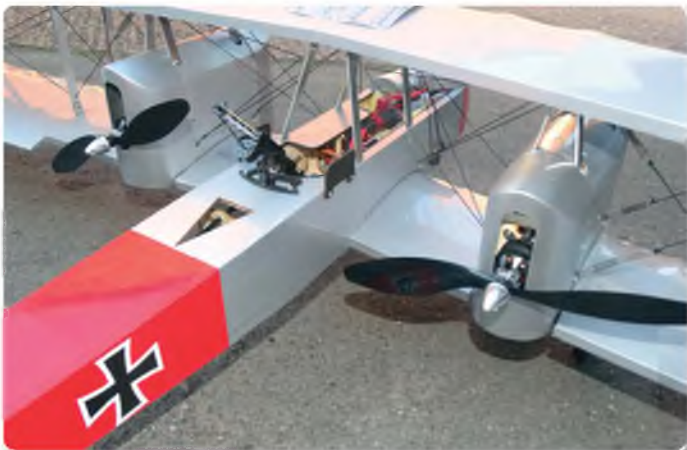
View of the twin pusher set up
