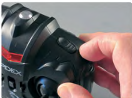
Pressing the top right hand shoulder switch initiates flip mode
