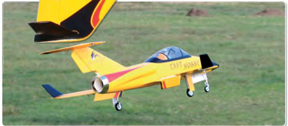
The electric retracts proved to be robust, even when flying off a rough strip at the local common
