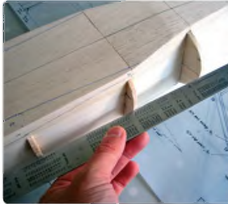
The three 3/16" balsa air-intake formers A1 to A3 are glued into the recess slots in the fuselage side. The former tops should create a straight line running into the fuselage at F7
