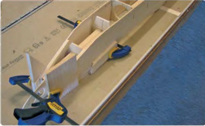
Nose section pulled in and clamped, with 1/8" packing under F7 at rear of wing to correctly level fuselage onto front base sheeting, which is pinned to the board. Scrap blocks are used to protect the model from clamp damage
