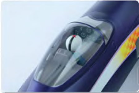
The nicely moulded canopy/radio hatch includes a painted pilot and an instrument panel
