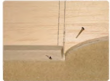
Detail at base of F3. The triangular section runs short to allow the 1/16" ply overhang on F3
