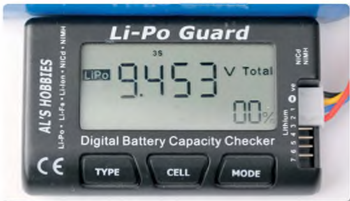
This 3S LiPo pack is not charging properly and the voltage is too low
