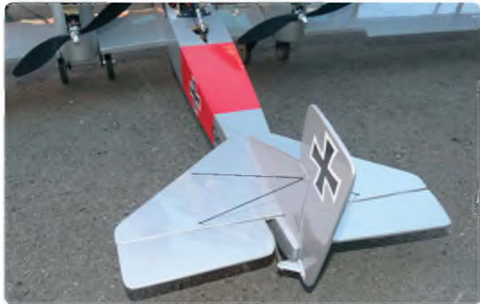
Simulated bracing wires run through holes in the tailplane and fin
