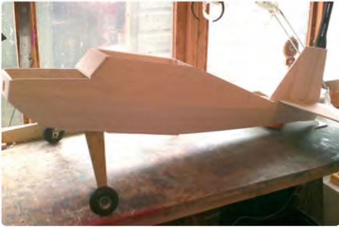
Fuselage complete with tail parts fitted and Dural undercarriage
