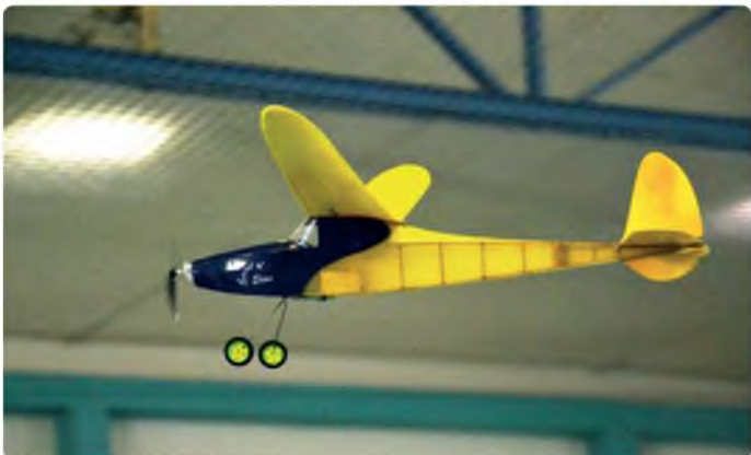
The Depron wing allows Sparky to fly slowly and without risking a stall, even in tight circles
