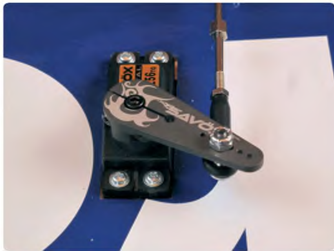
...The reason for the angled pushrod at neutral is now clear. At maximum control throws, up and down, the pushrod is able to run parallel to the servo, so maximising the servo's performance during extreme aerobatics (at least it would if we could fly that well!). The sturdy ball links at each end of the pushrods also help greatly in this regard as they eliminate any unwanted twisting motion in the linkages
